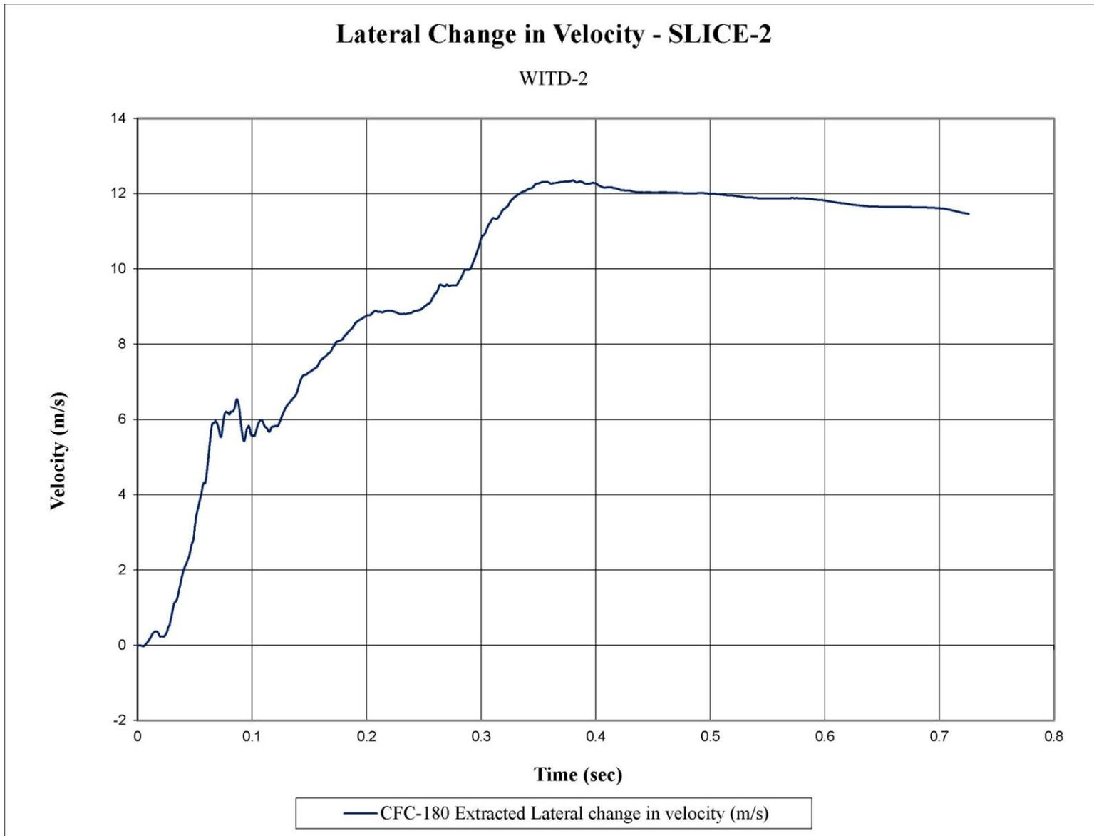
Figure F-13. Lateral Occupant Impact Velocity (SLICE-2), Test No. WITD-2
