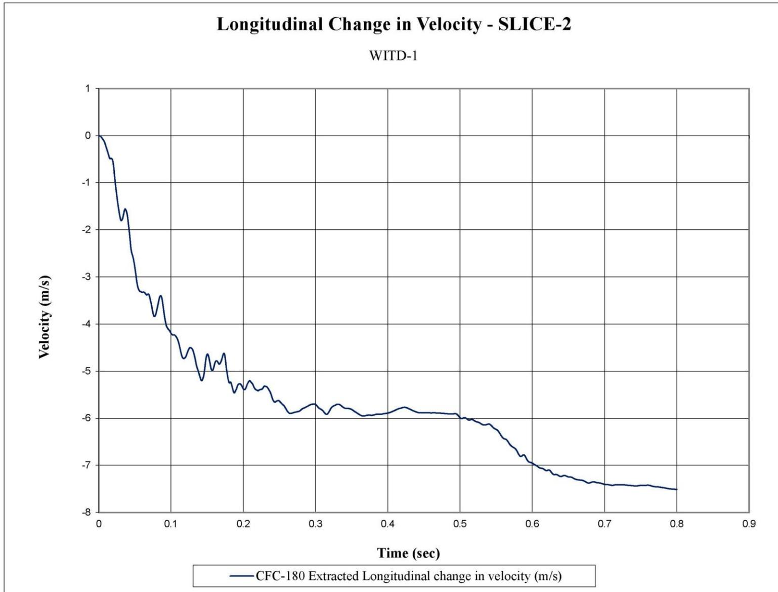
Figure E-10. Longitudinal Occupant Impact Velocity (SLICE-2), Test No. WITD-1
