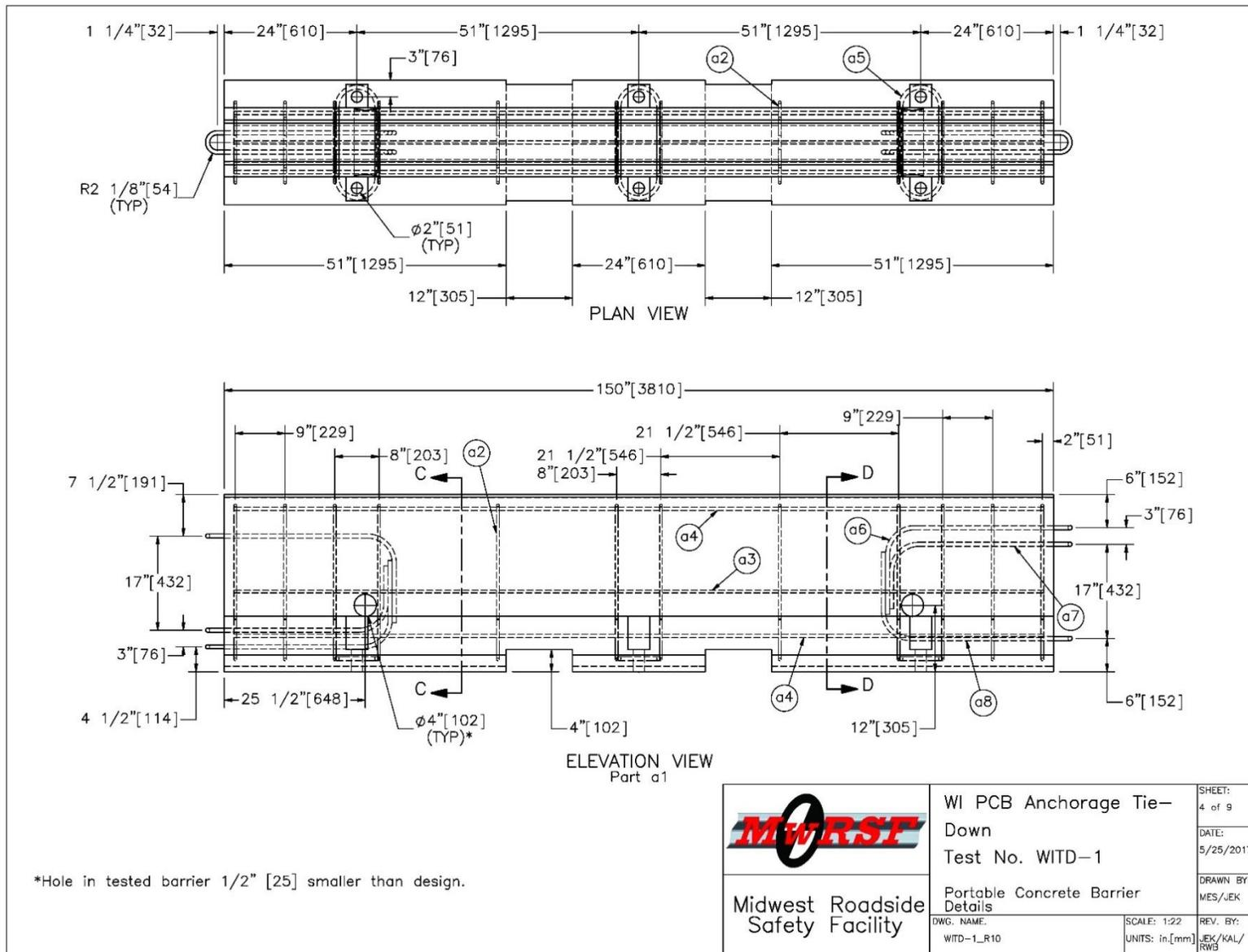
Figure 16. Portable Concrete Barrier Details, Test No. WITD-1
