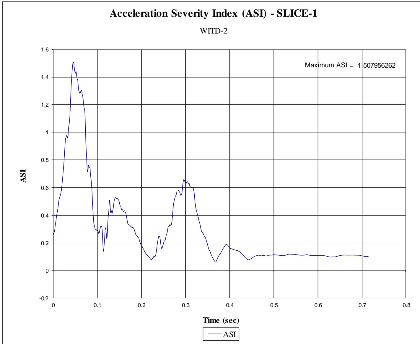
Figure F-8. Acceleration Severity Index (SLICE-1), Test No. WITD-2
