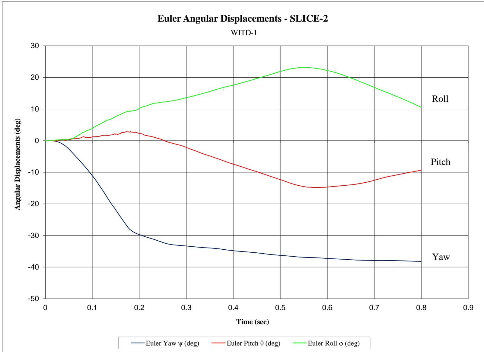
Figure E-15. Vehicle Angular Displacements (SLICE-2), Test No. WITD-1
