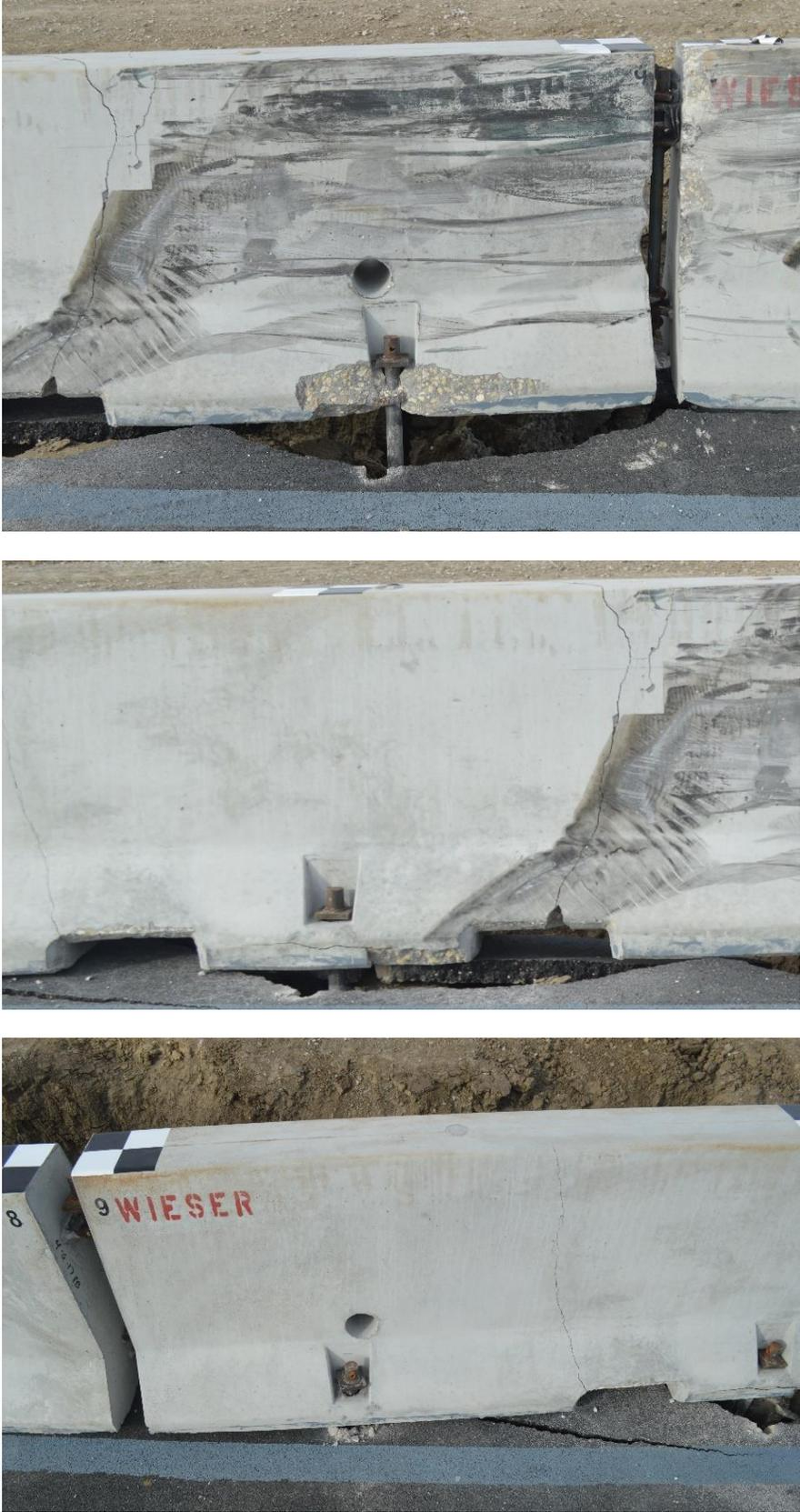
Figure 69. Barrier No. 9 Asphalt Pin Damage and Displacement, Test No. WITD-2
