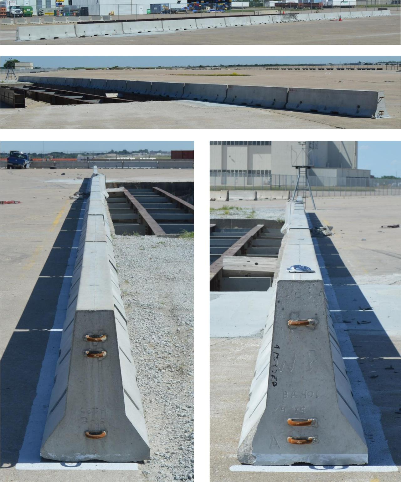
Figure 30. System Damage – Front, Back, Downstream, and Upstream Views, Test No. WITD-1
