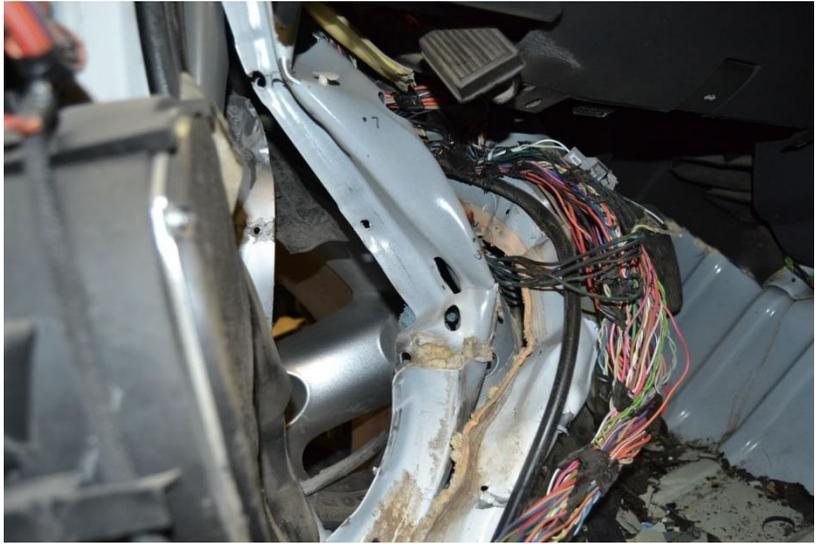
Figure 76. Occupant Compartment Damage, Test No. WITD-2
