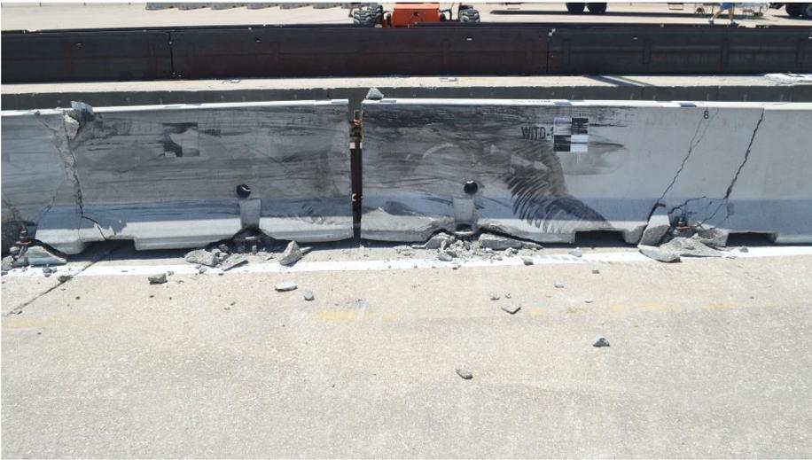
Figure 31. System Damage at Impact Location, Test No. WITD-1
