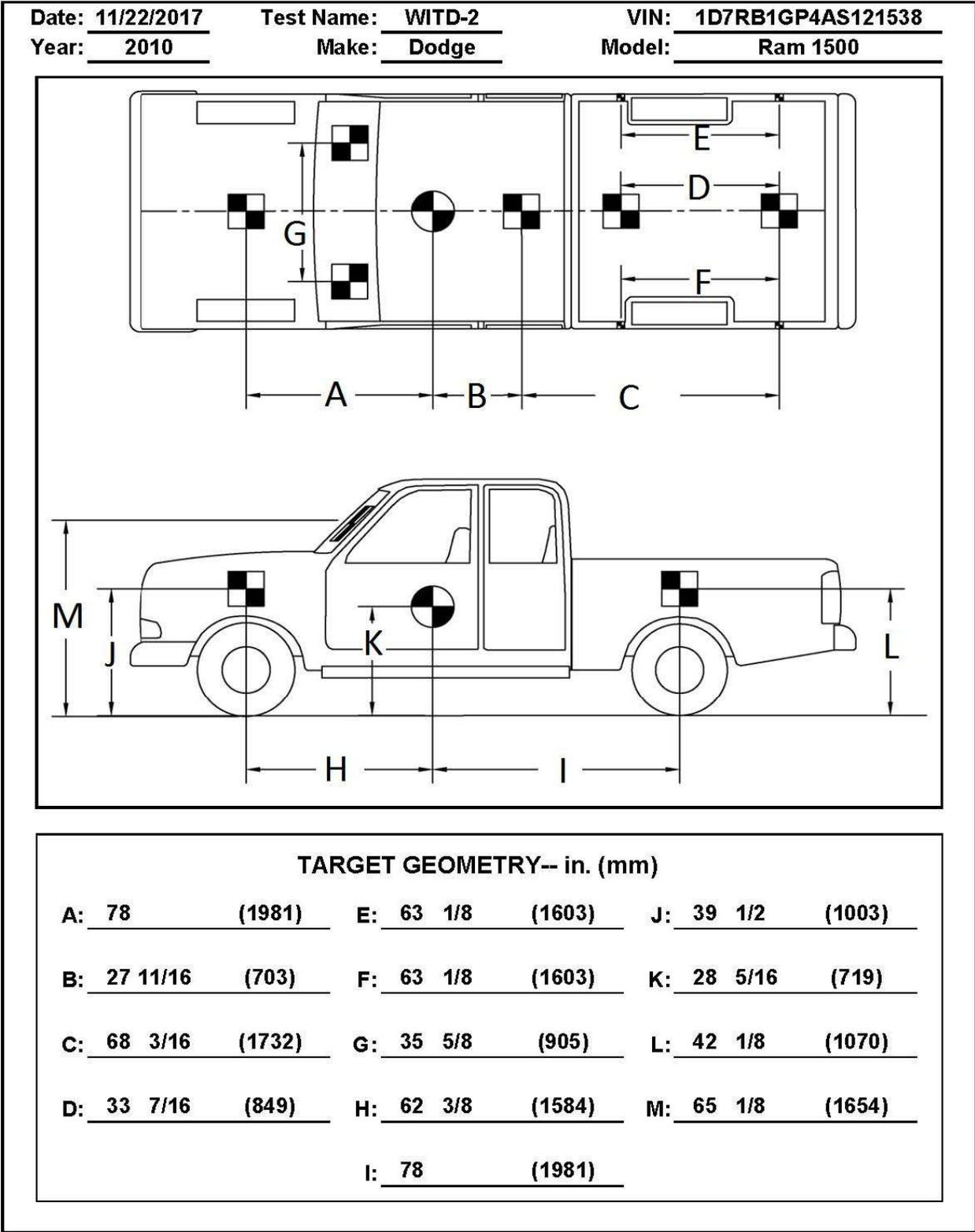
Figure 10. Target Geometry, Test No. WITD-2
