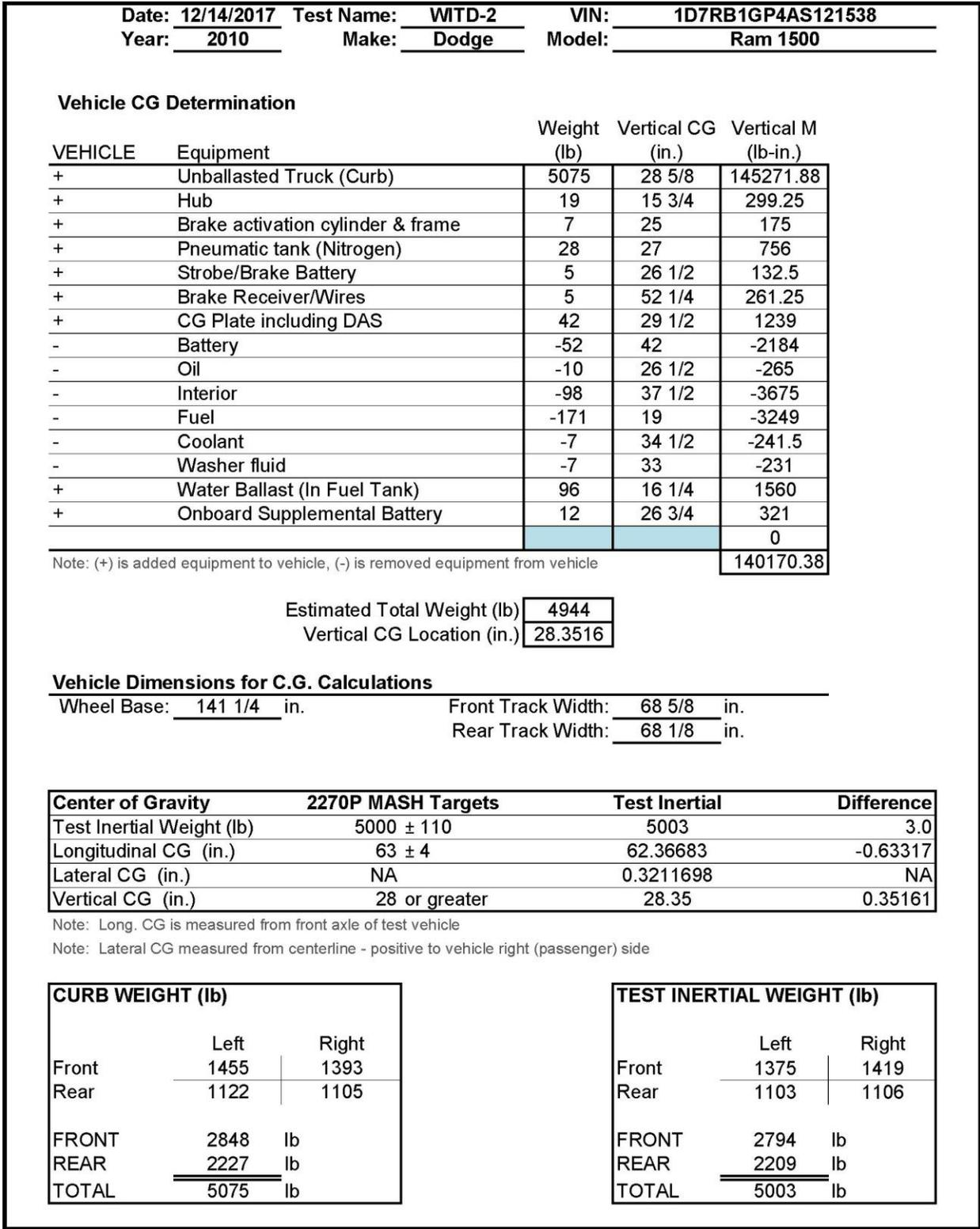
Figure B-2. Vehicle Mass Distribution, Test No. WITD-2
