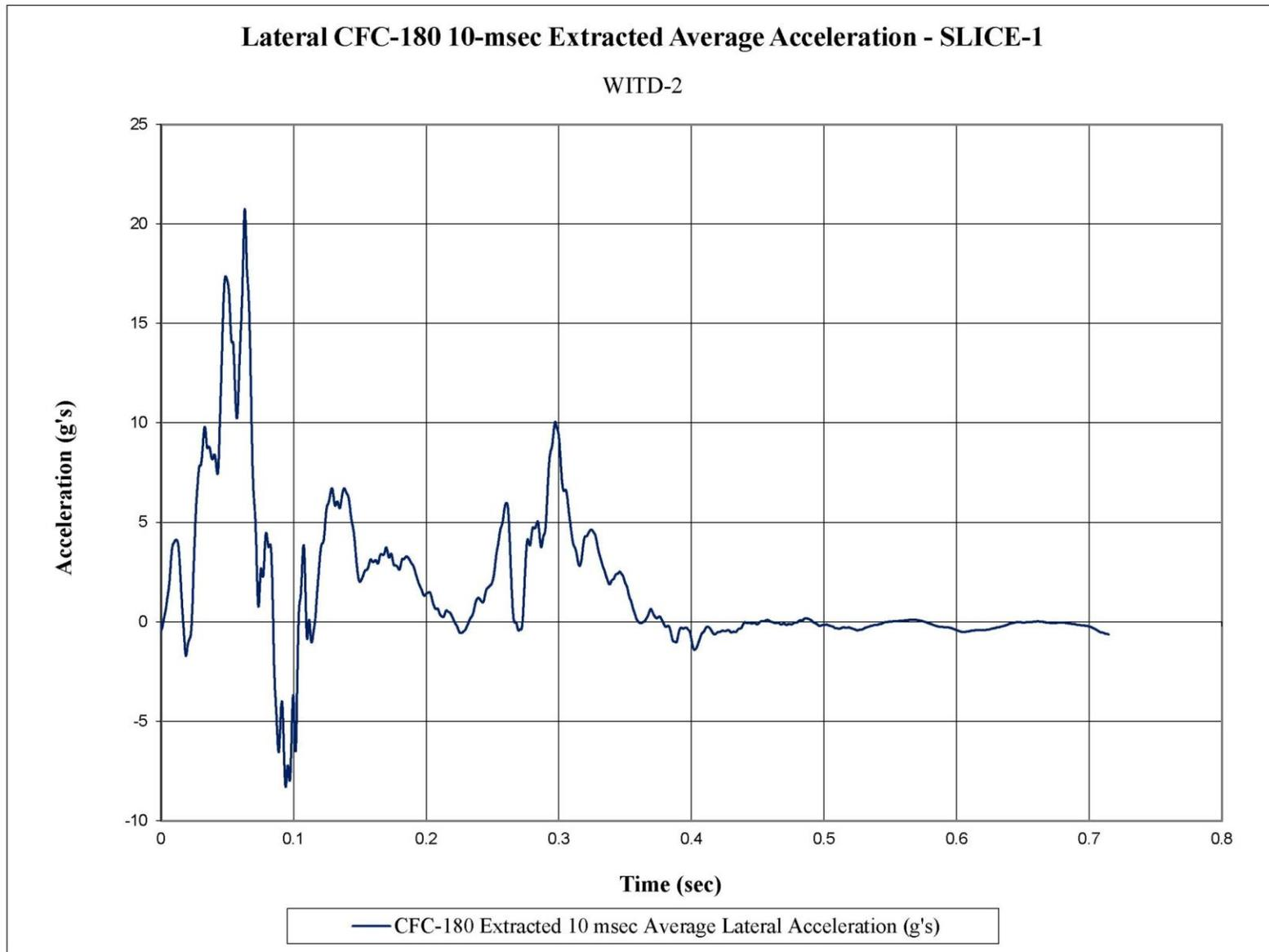
Figure F-4. 10-ms Average Lateral Deceleration (SLICE-1), Test No. WITD-2
