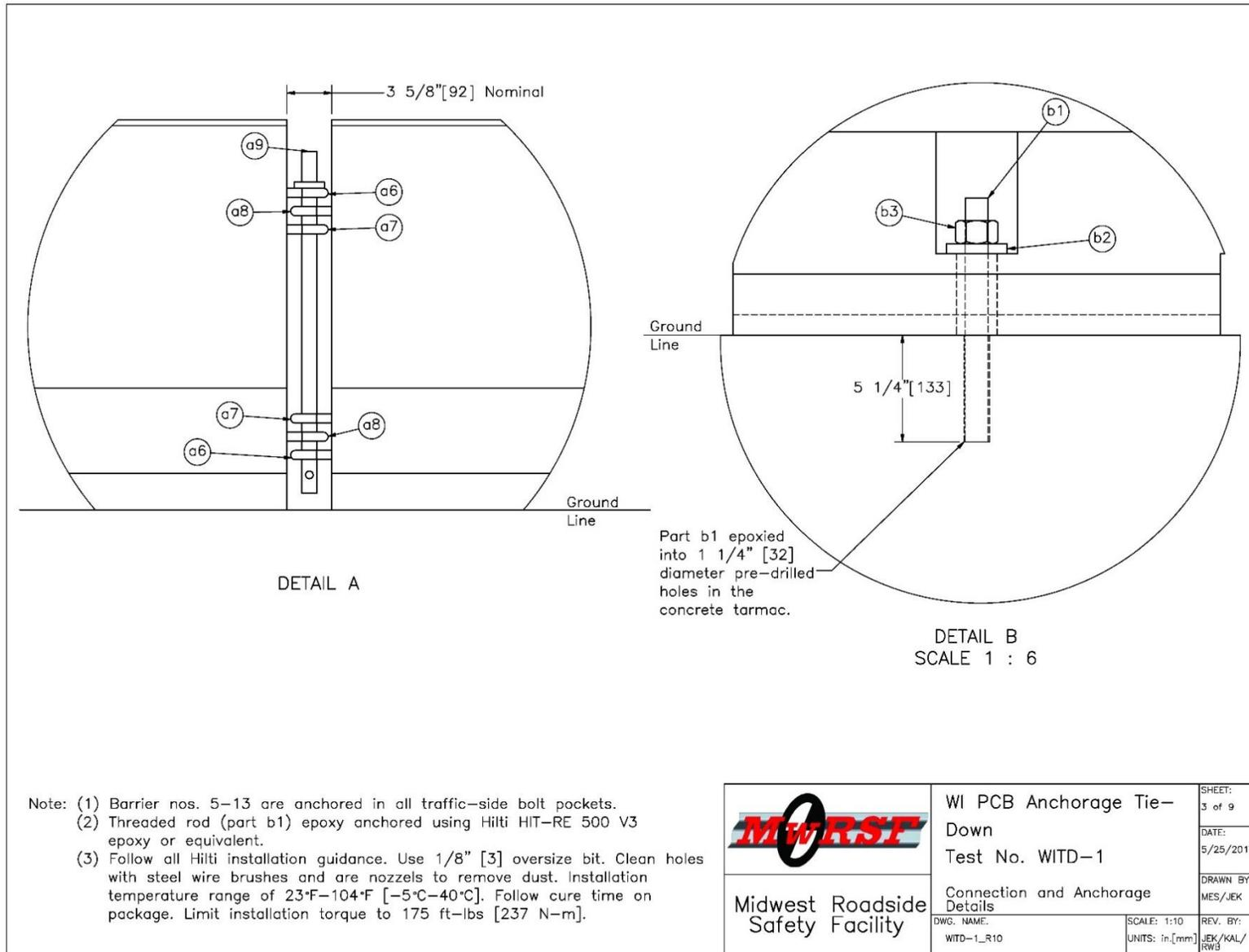
Figure 15. Connection and Anchorage Details, Test No. WITD-1
