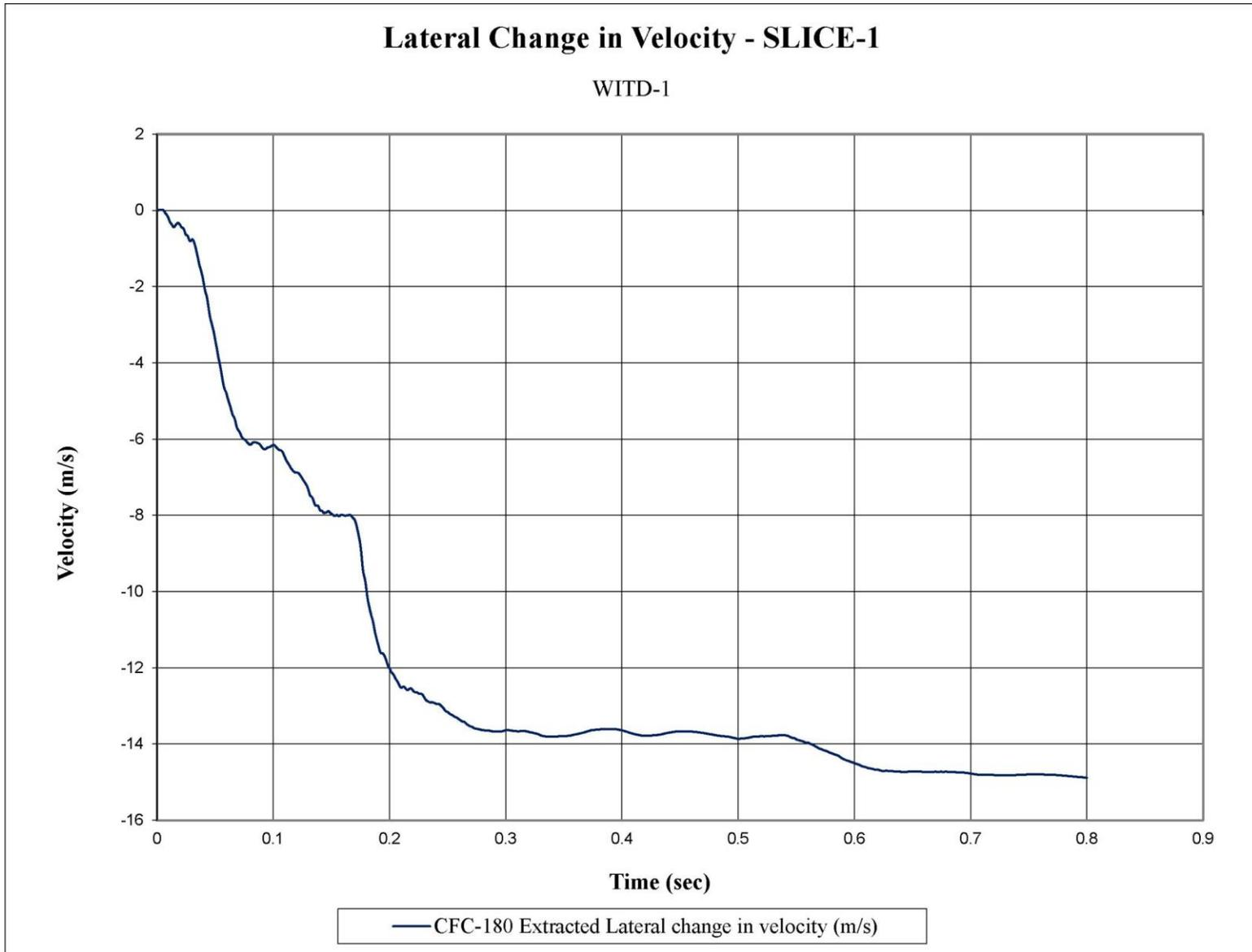
Figure E-5. Lateral Occupant Impact Velocity (SLICE-1), Test No. WITD-1
