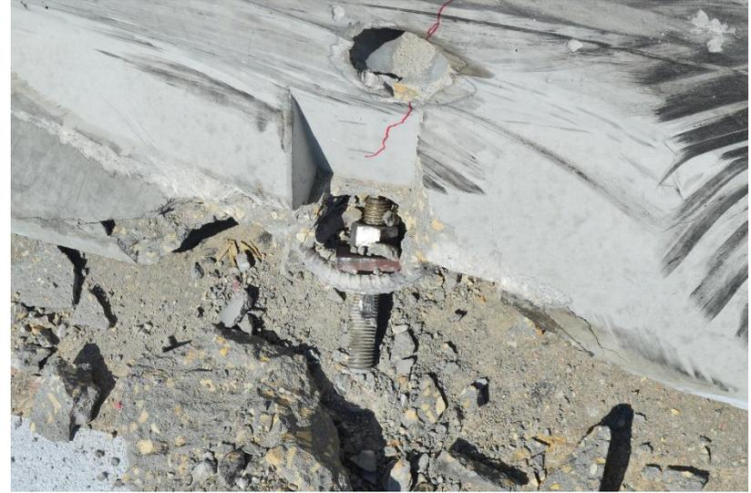
Figure 33. System Damage – Additional Views of Damage on Barrier No. 8 Traffic Side, Test No. WITD-1
