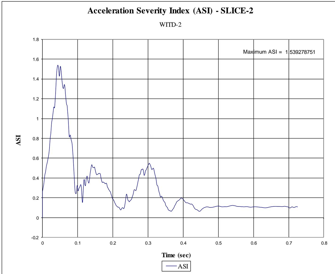
Figure F-16. Acceleration Severity Index (SLICE-2), Test No. WITD-2
