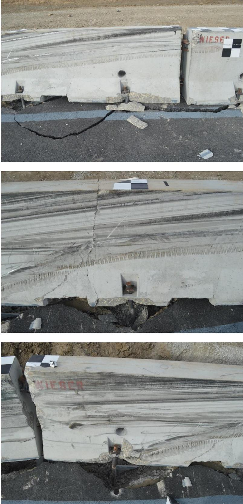
Figure 68. Barrier No. 10 Asphalt Pin Damage and Displacement, Test No. WITD-2
