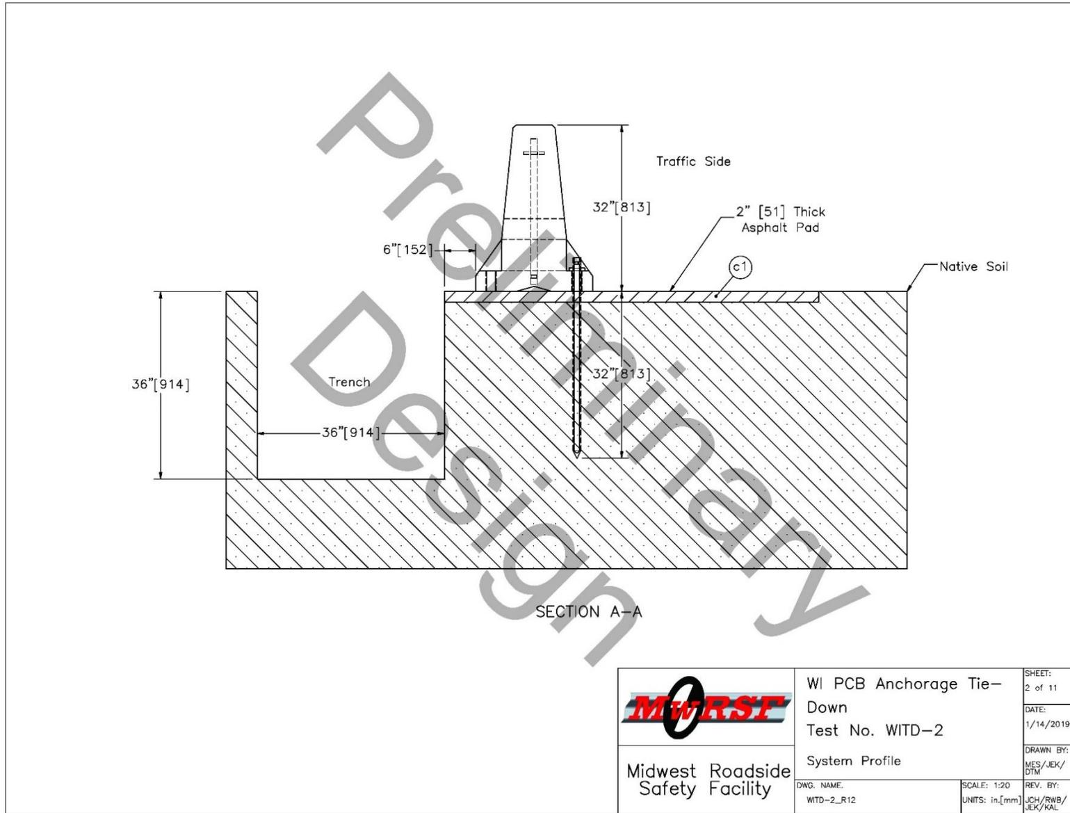
Figure 46. System Profile, Test No. WITD-2
