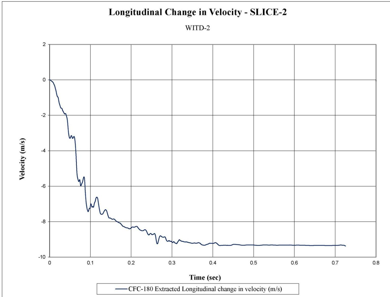
Figure F-10. Longitudinal Occupant Impact Velocity (SLICE-2), Test No. WITD-2
