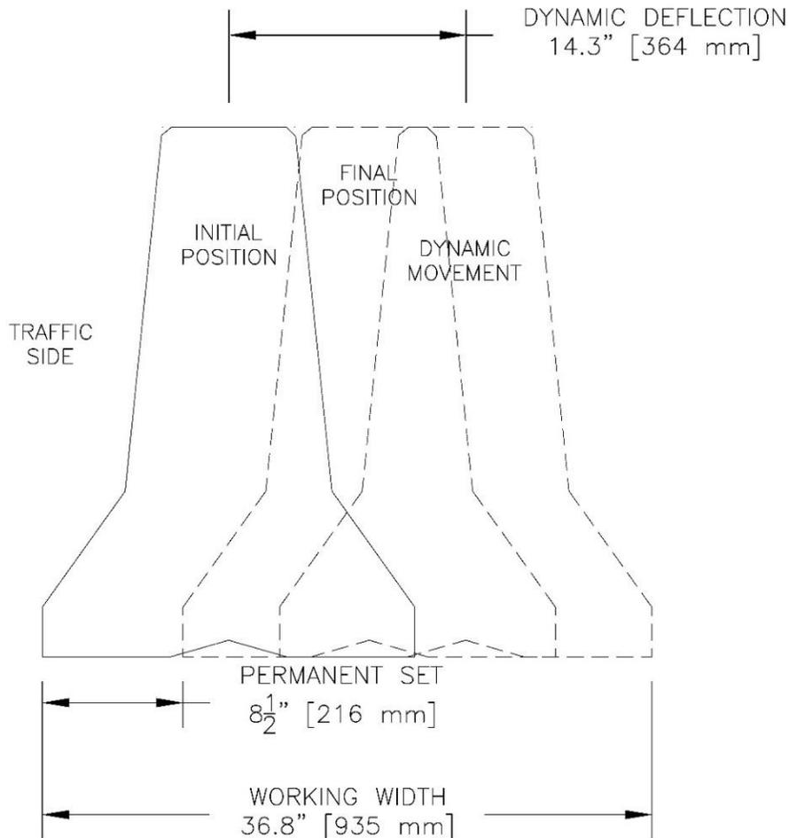
Figure 37. Permanent Set Deflection, Dynamic Deflection and Working Width, Test No. WITD-1
