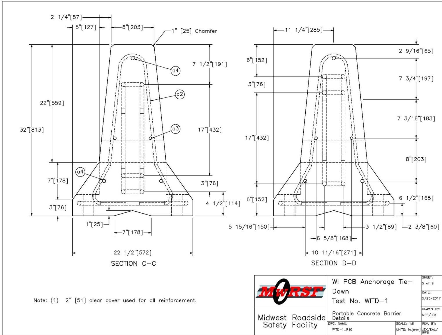
Figure 17. Portable Concrete Barrier Details, Test No. WITD-1
