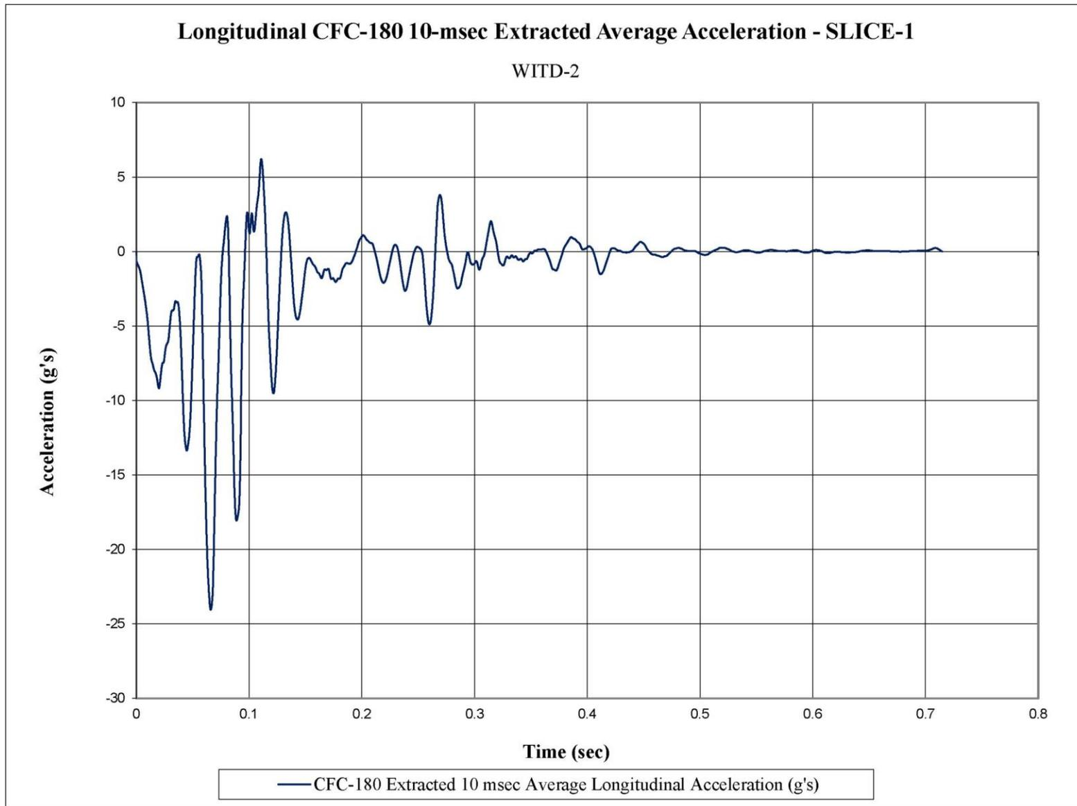
Figure F-1. 10-ms Average Longitudinal Deceleration (SLICE-1), Test No. WITD-2
