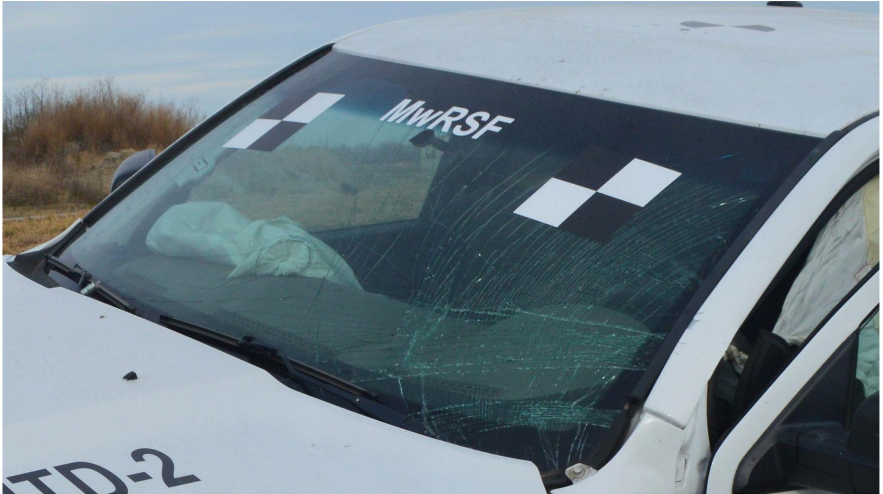
Figure 73. Vehicle Damage, Windshield Damage Test No. WITD-2
