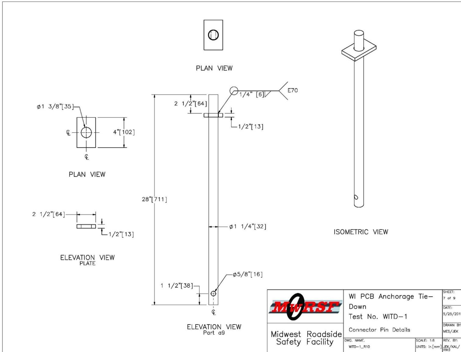
Figure 19. Connector Pin Details, Test No. WITD-1
