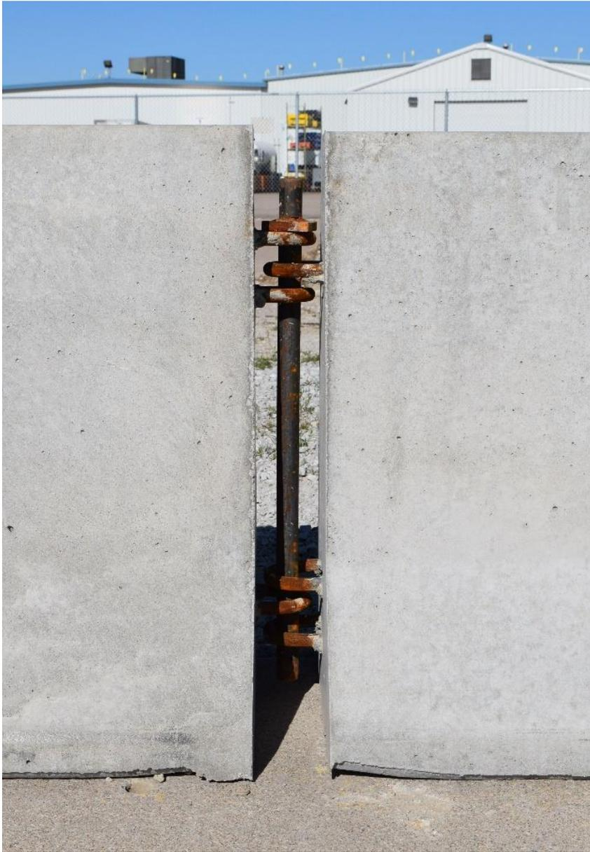
Figure 23. Connection and Anchor Pin Details, Test No. WITD-1
