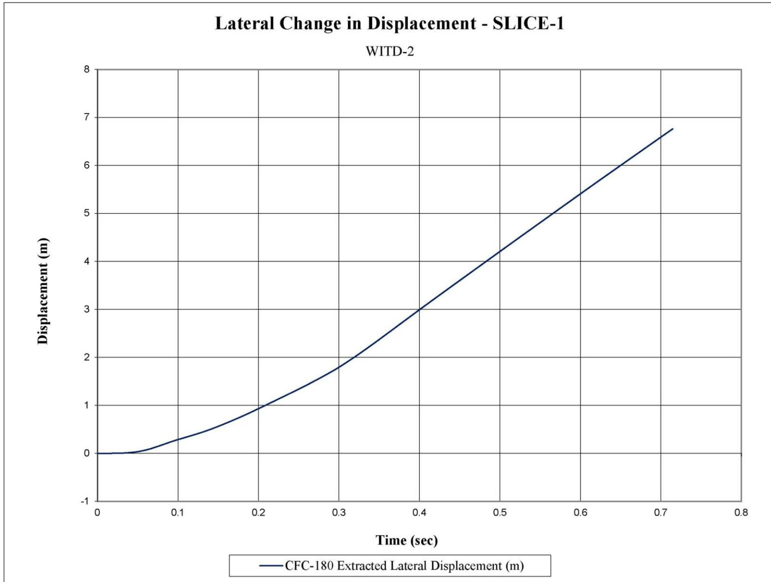
Figure F-6. Lateral Occupant Displacement (SLICE-1), Test No. WITD-2
