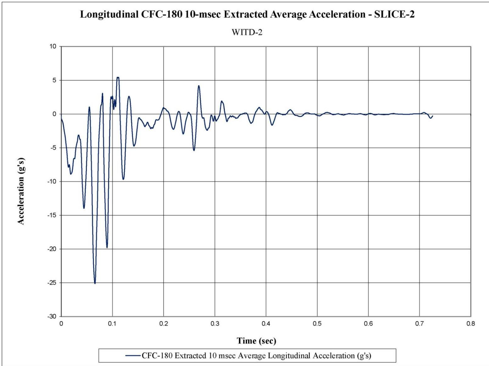
Figure F-9. 10-ms Average Longitudinal Deceleration (SLICE-2), Test No. WITD-2
