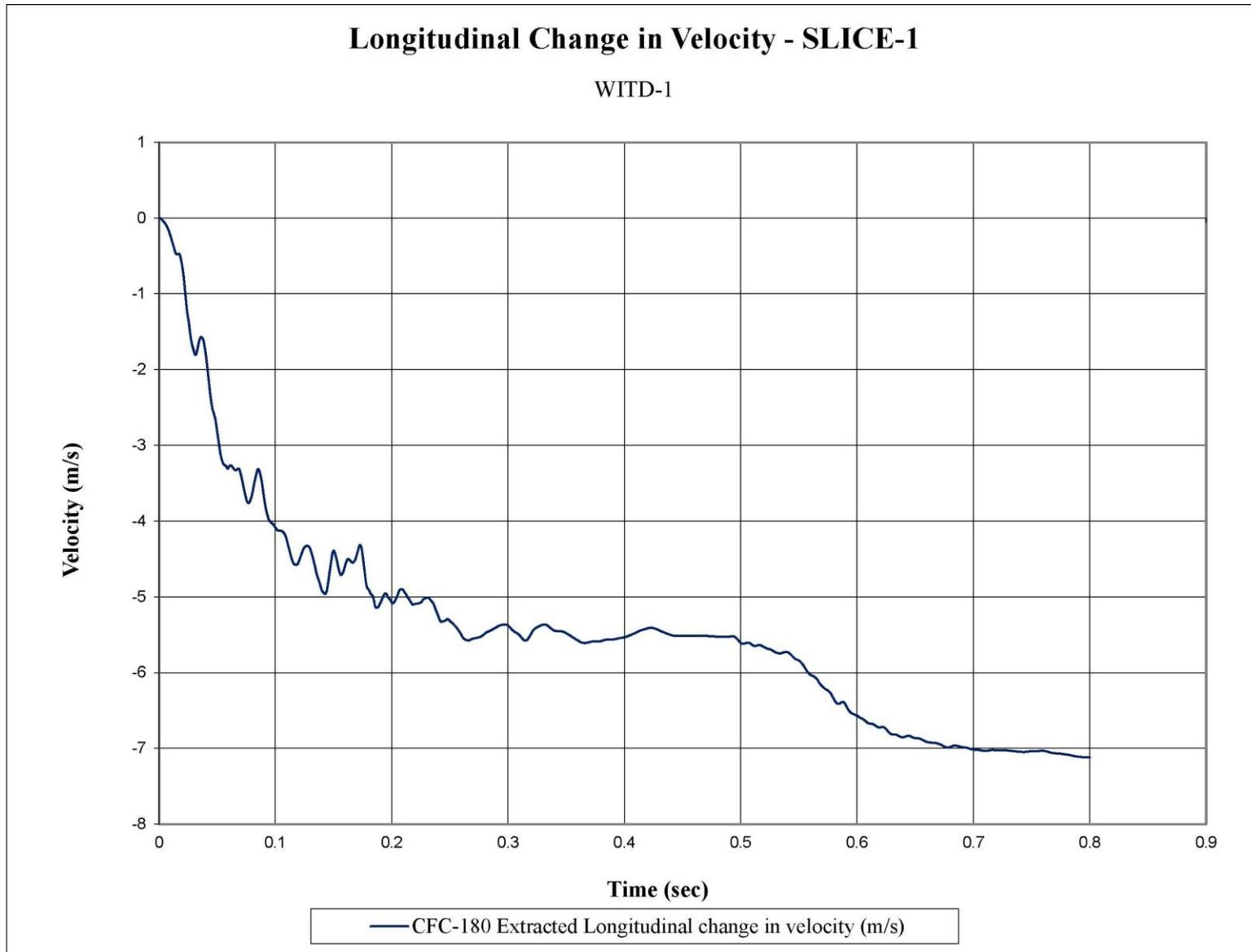
Figure E-2. Longitudinal Occupant Impact Velocity (SLICE-1), Test No. WITD-1
