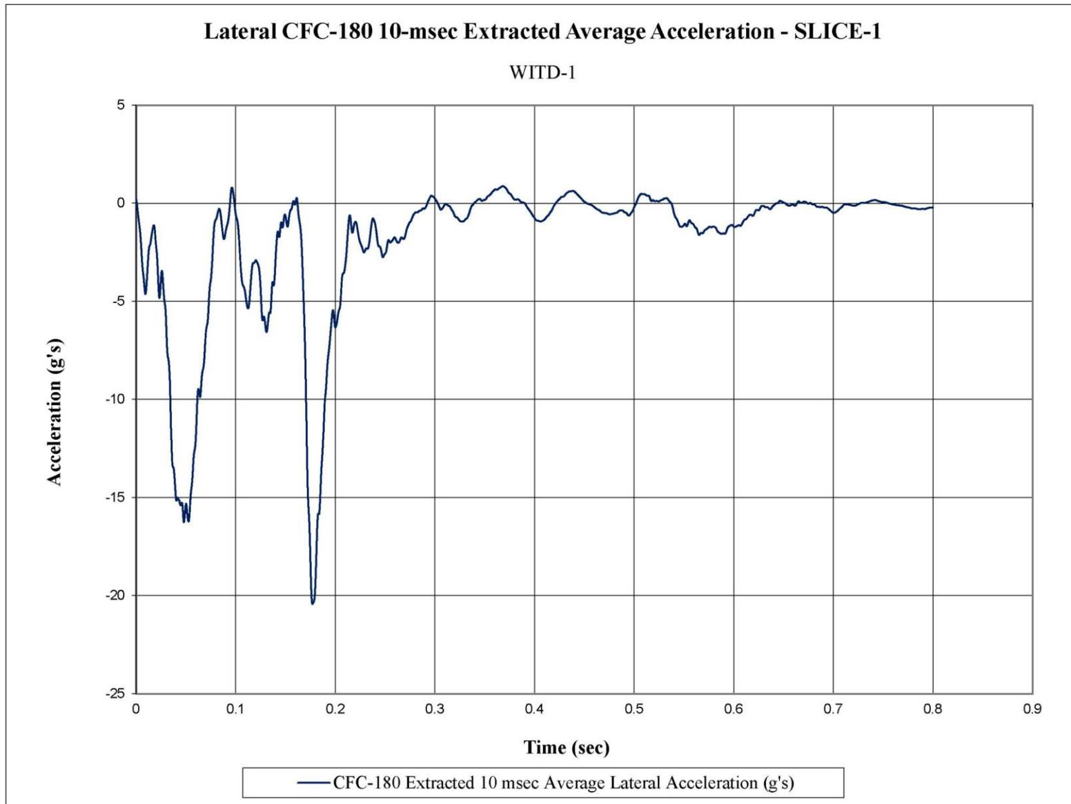
Figure E-4. 10-ms Average Lateral Deceleration (SLICE-1), Test No. WITD-1
