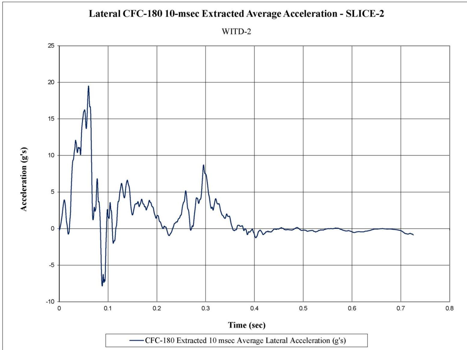
Figure F-12. 10-ms Average Lateral Deceleration (SLICE-2), Test No. WITD-2
