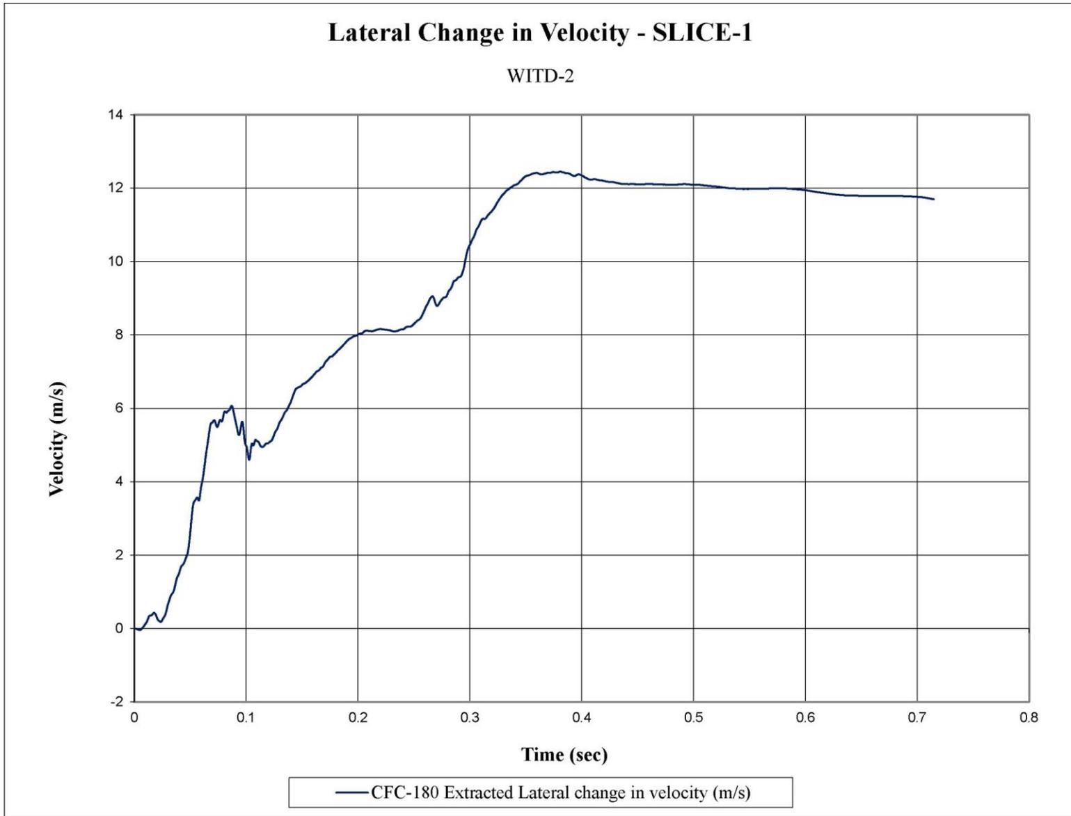
Figure F-5. Lateral Occupant Impact Velocity (SLICE-1), Test No. WITD-2
