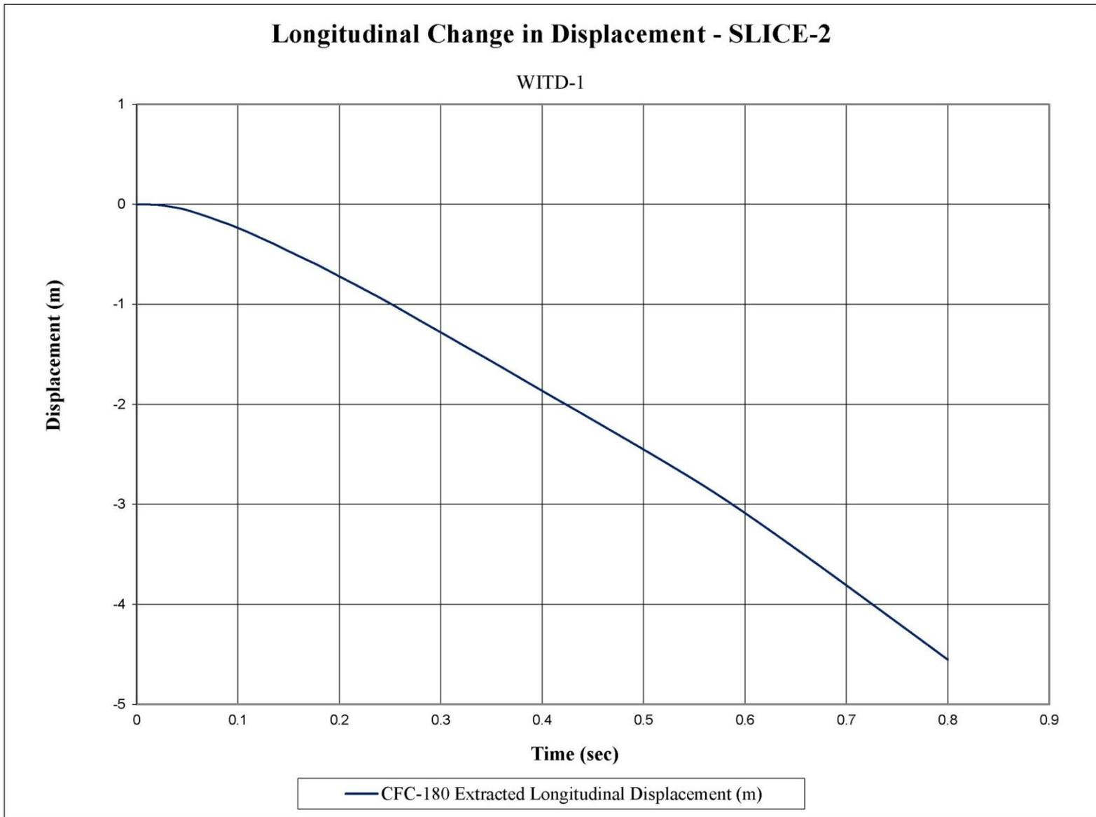
Figure E-11. Longitudinal Occupant Displacement (SLICE-2), Test No. WITD-1
