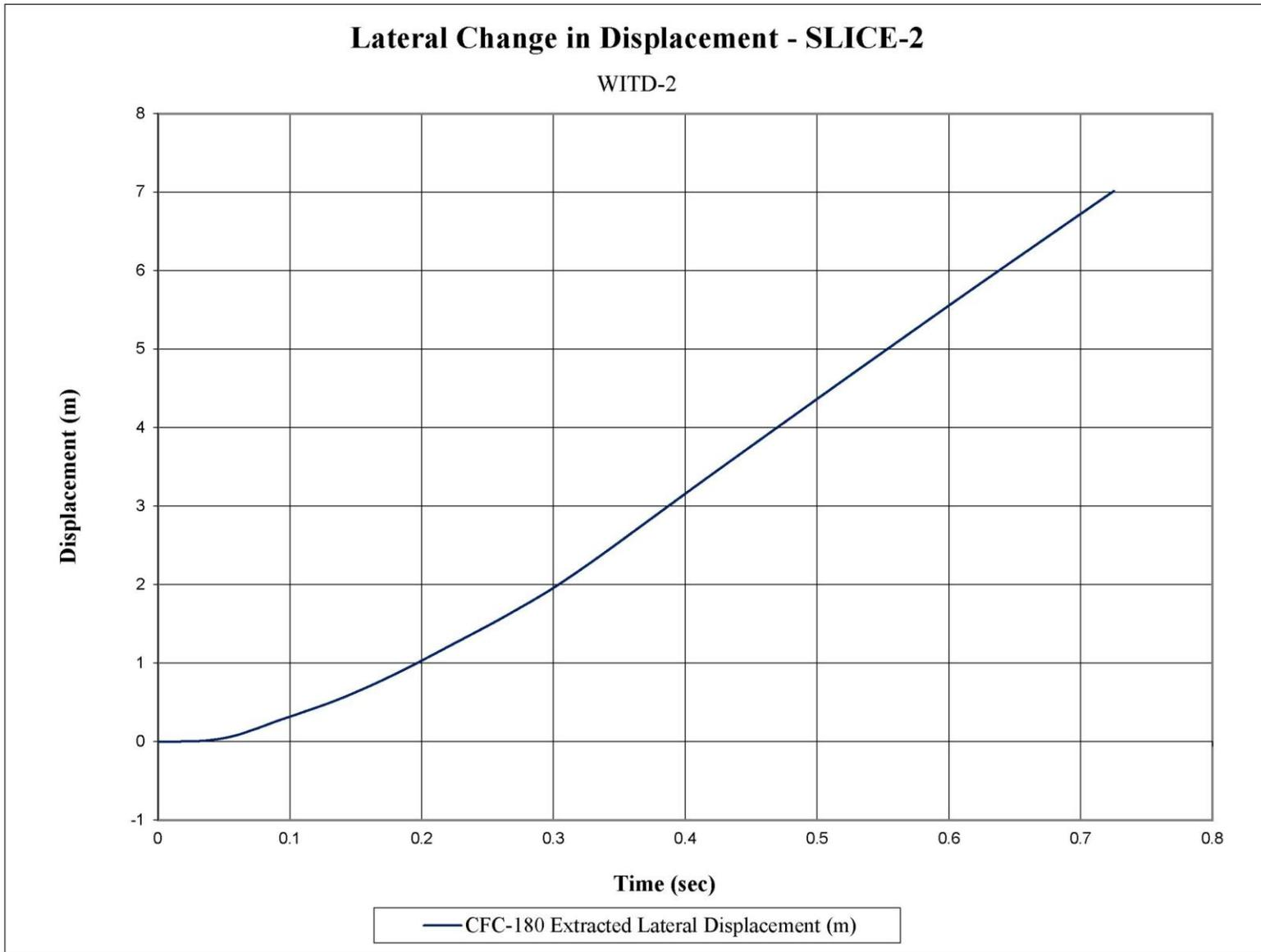
Figure F-14. Lateral Occupant Displacement (SLICE-2), Test No. WITD-2
