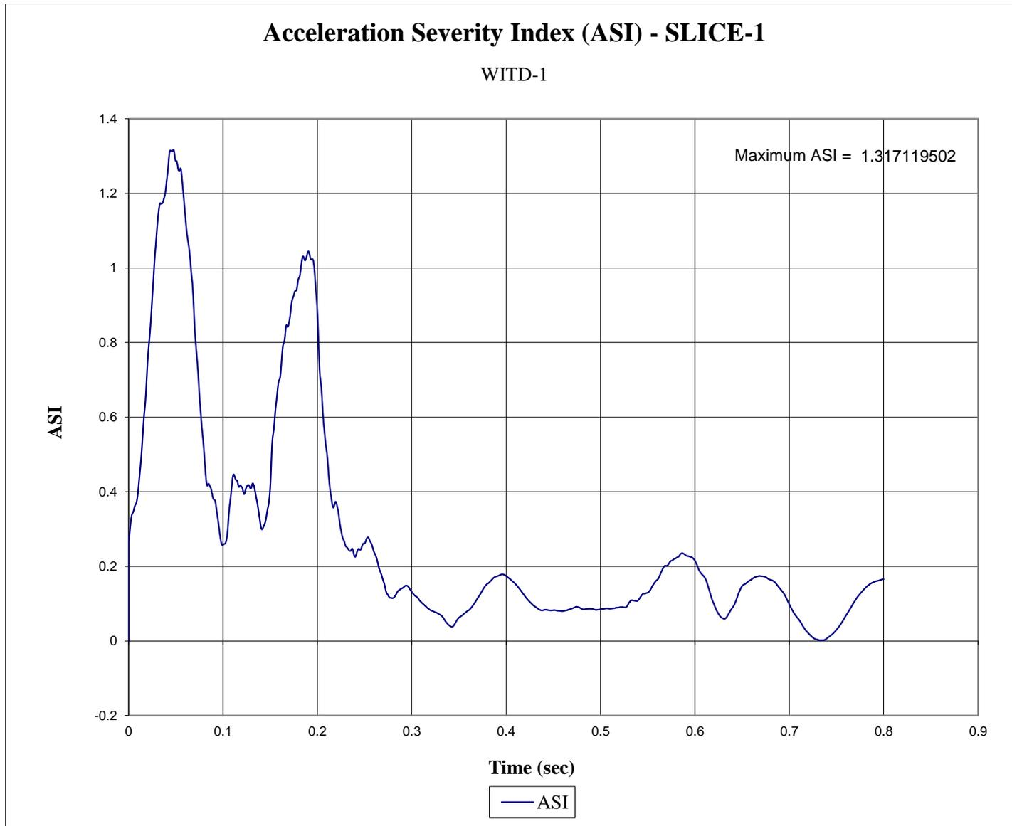
Figure E-8. Acceleration Severity Index (SLICE-1), Test No. WITD-1
