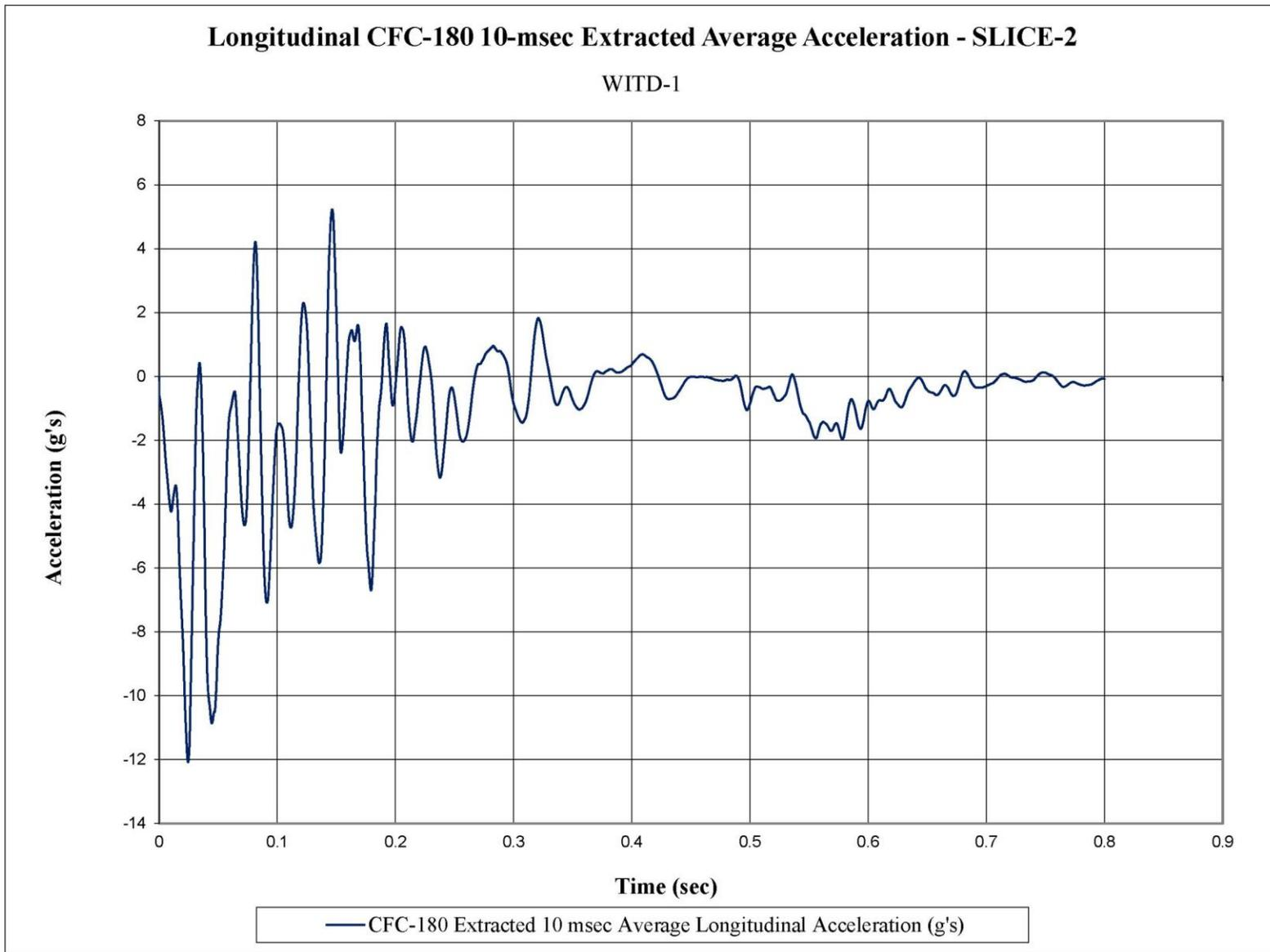
Figure E-9. 10-ms Average Longitudinal Deceleration (SLICE-2), Test No. WITD-1
