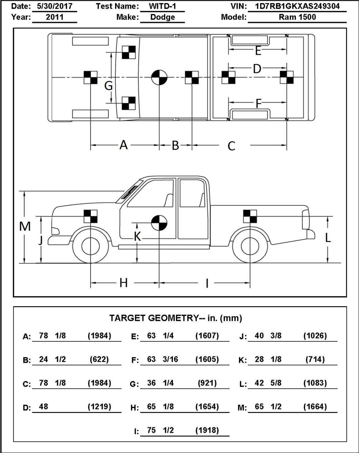
Figure 9. Target Geometry, Test No. WITD-1
