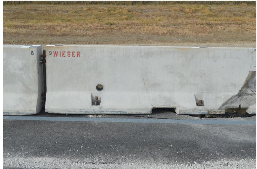
Figure 66. Barrier No. 9 Barrier Damage, Test No. WITD-2
