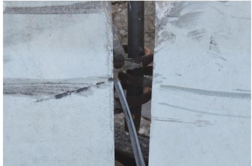
Figure 67. Barrier Nos. 9 and 10 Connection Pin Damage, Test No. WITD-2
