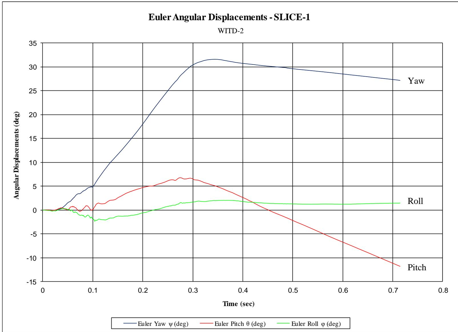
Figure F-7. Vehicle Angular Displacements (SLICE-1), Test No. WITD-2
