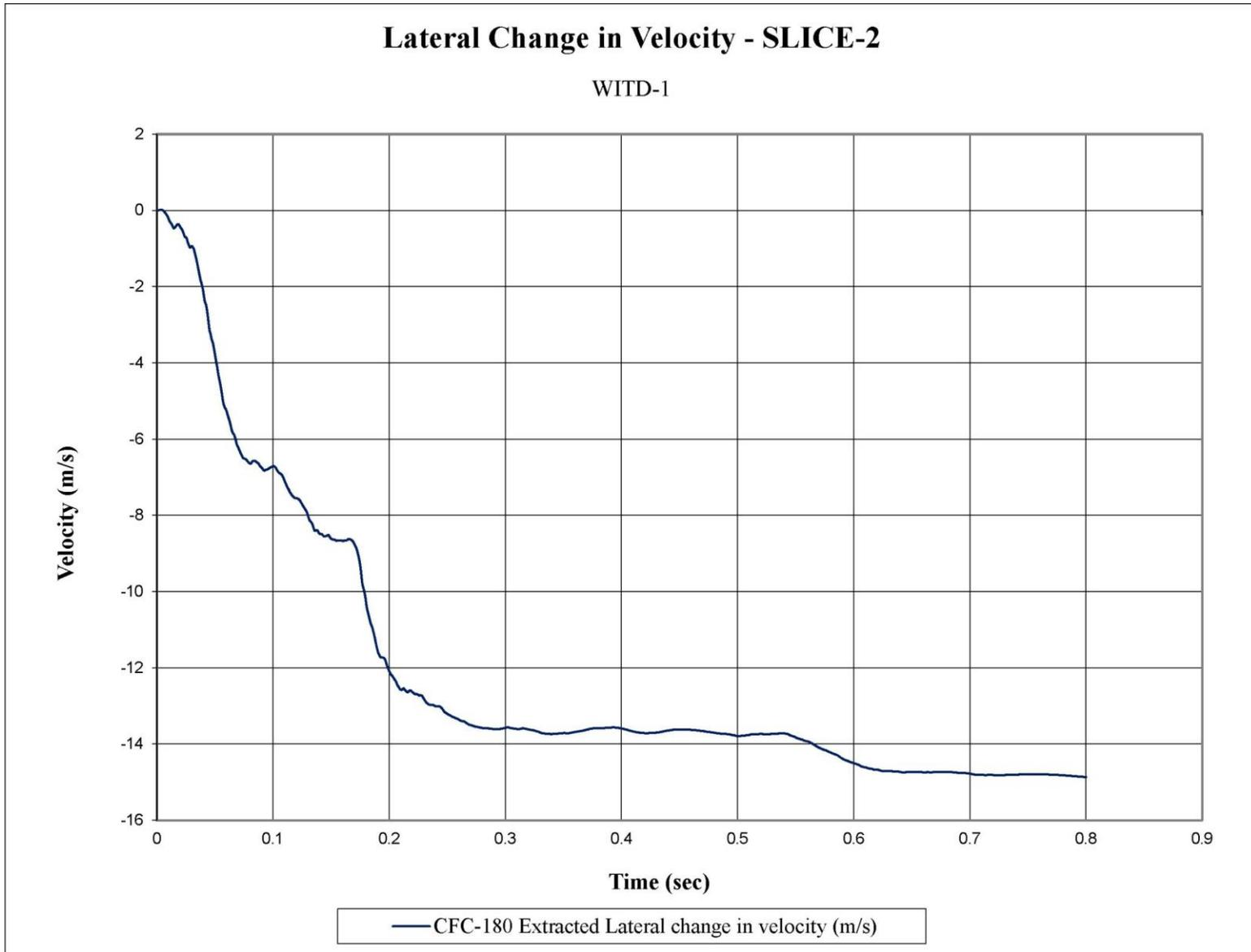
Figure E-13. Lateral Occupant Impact Velocity (SLICE-2), Test No. WITD-1
