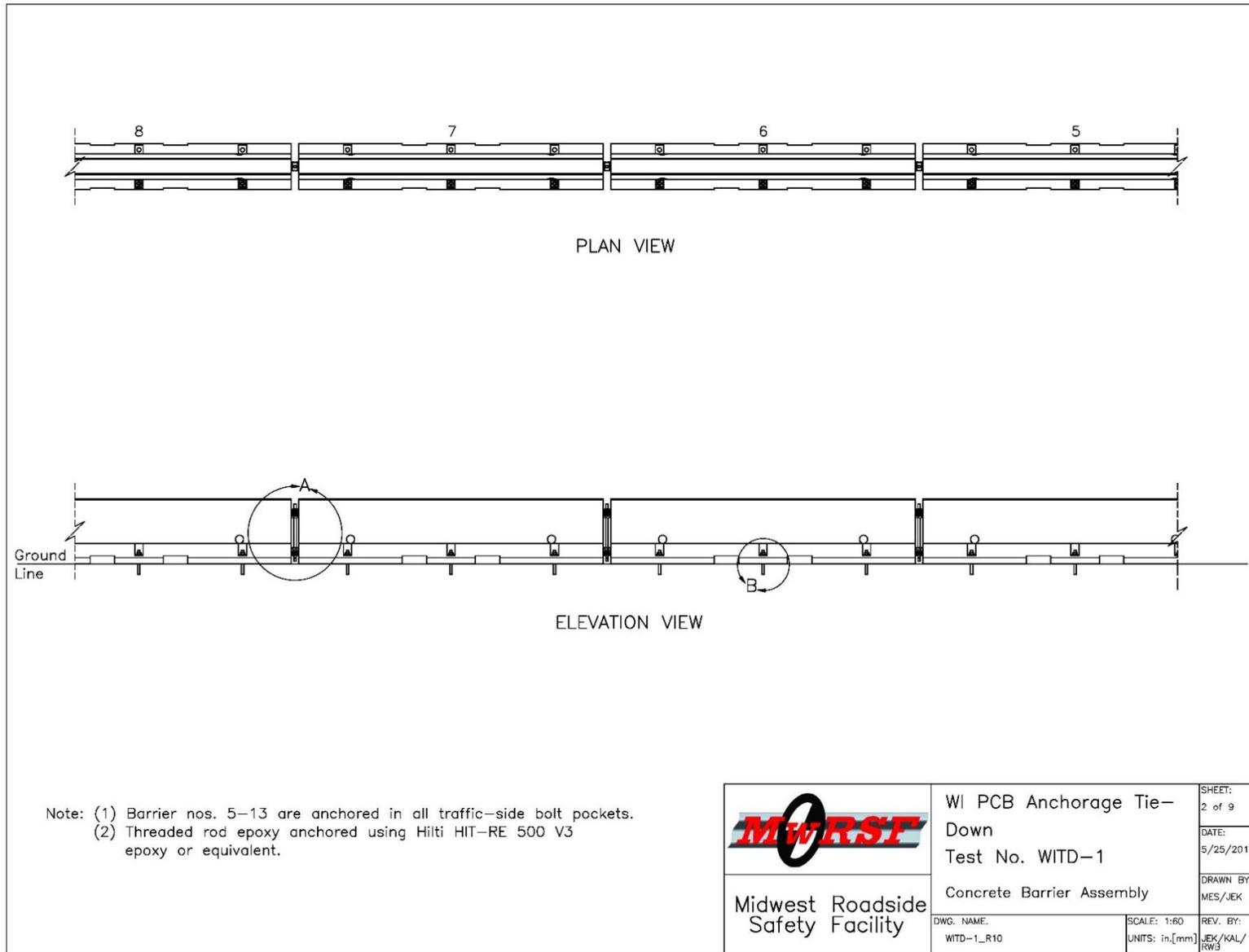
Figure 14. Concrete Barrier Assembly, Test No. WITD-1
