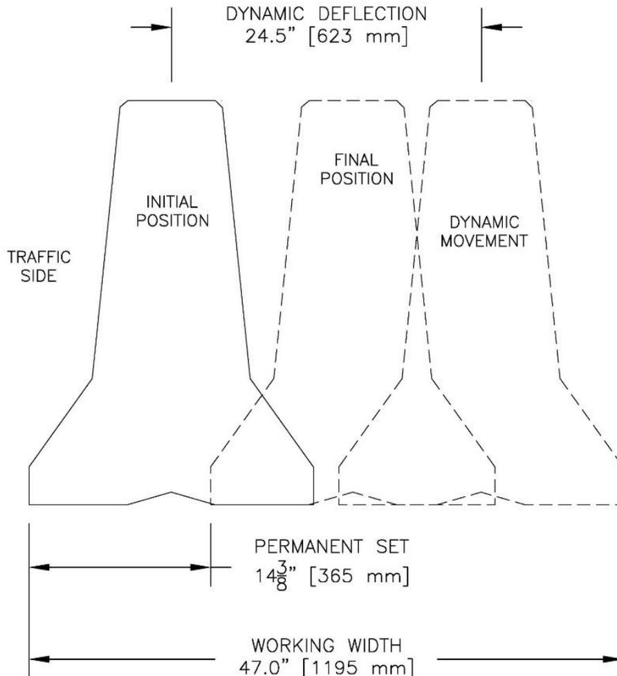
Figure 71. Permanent Set Deflection, Dynamic Deflection, and Working Width, Test No. WITD-2
