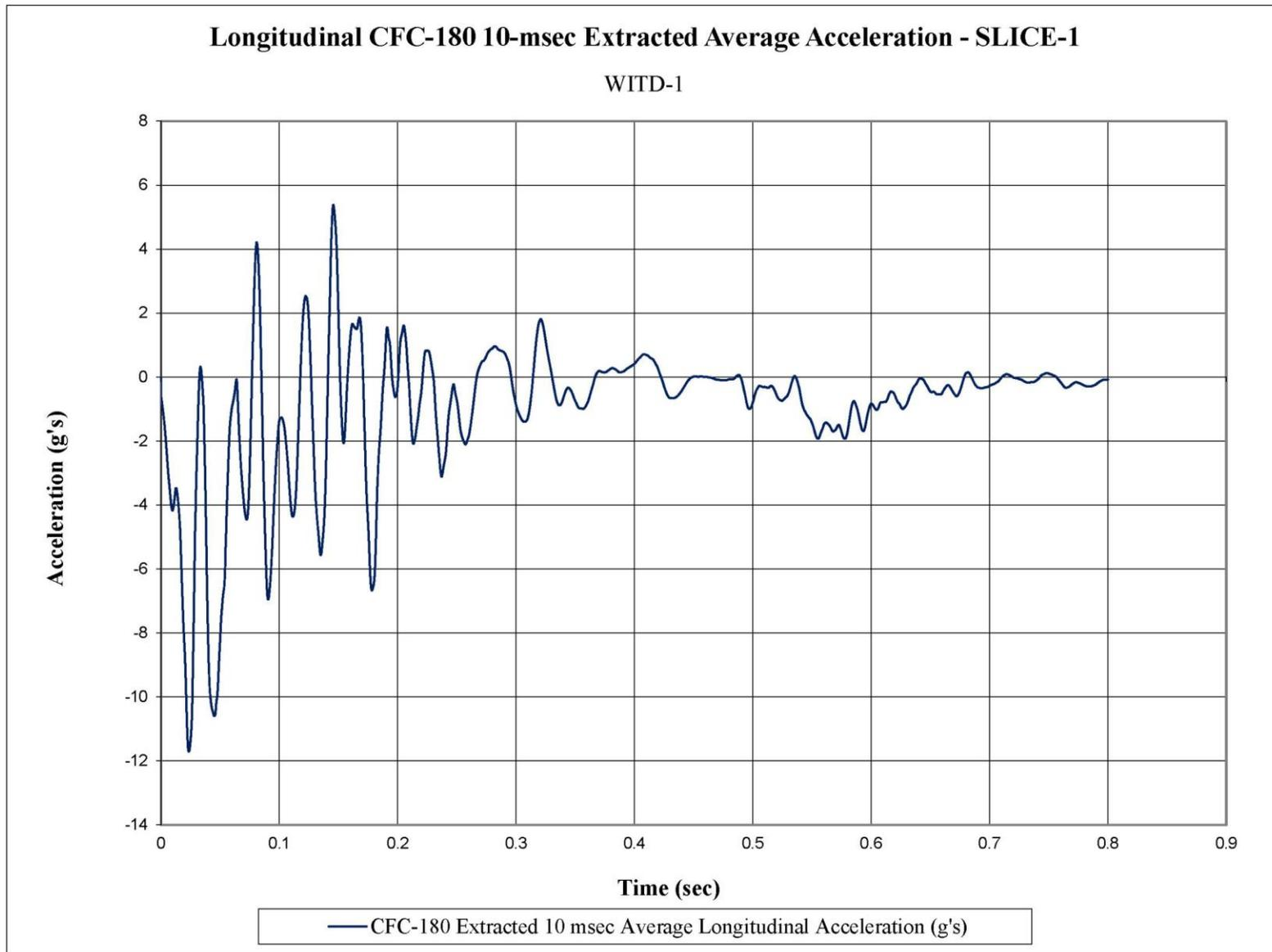
Figure E-1. 10-ms Average Longitudinal Deceleration (SLICE-1), Test No. WITD-1
