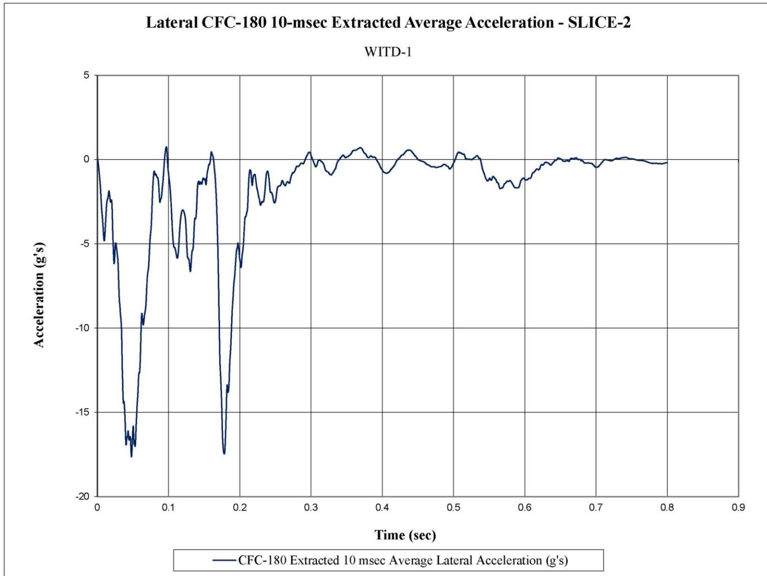
Figure E-12. 10-ms Average Lateral Deceleration (SLICE-2), Test No. WITD-1
