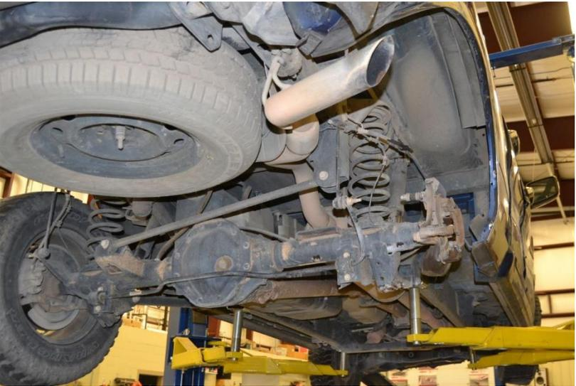
Figure 43. Undercarriage Vehicle Damage, Test No. WITD-1
