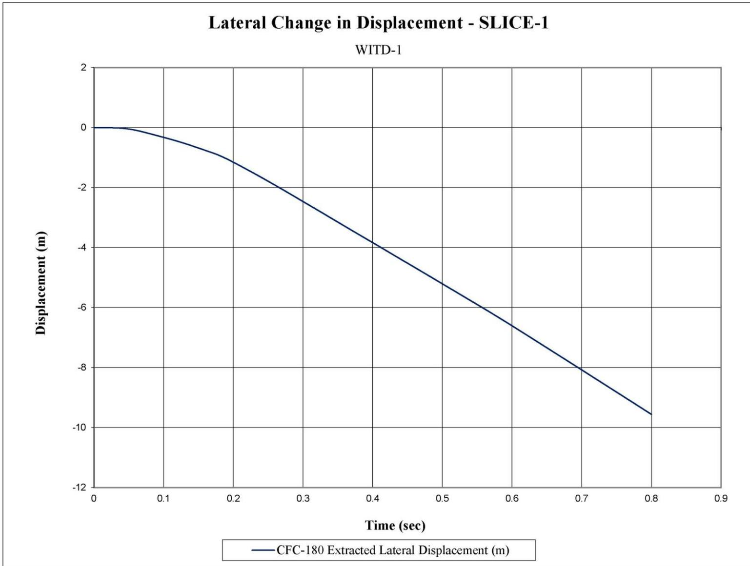
Figure E-6. Lateral Occupant Displacement (SLICE-1), Test No. WITD-1
