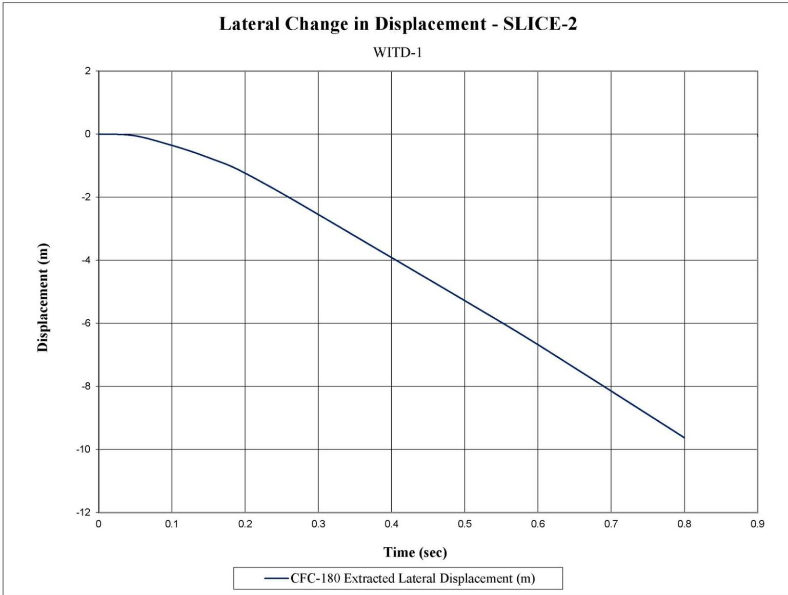
Figure E-14. Lateral Occupant Displacement (SLICE-2), Test No. WITD-1
