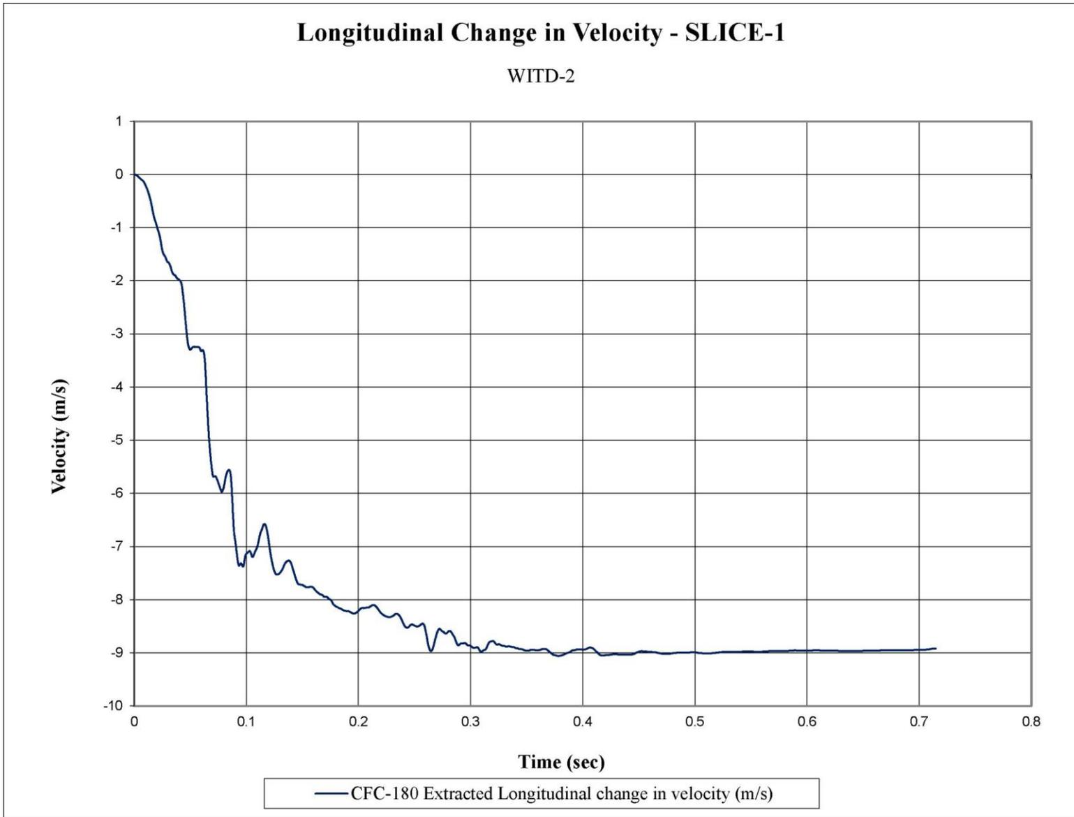
Figure F-2. Longitudinal Occupant Impact Velocity (SLICE-1), Test No. WITD-2
