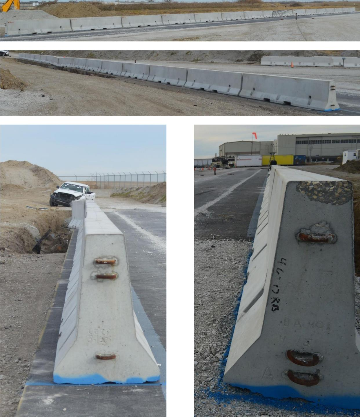
Figure 63. System Damage – Front, Back, Downstream, and Upstream Views, Test No. WITD-2
