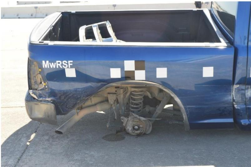
Figure 39 Vehicle Damage – Impact Side, Test No. WITD-1
