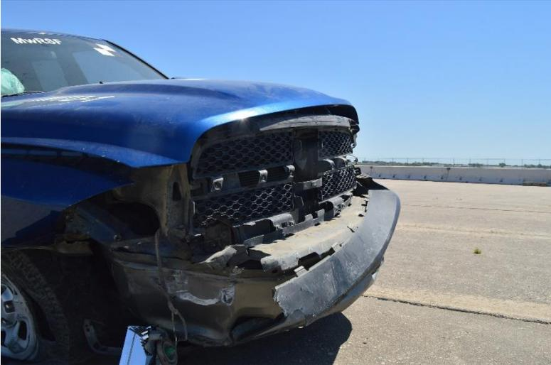
Figure 40. Vehicle Damage – Impact Side, Test No. WITD-1
