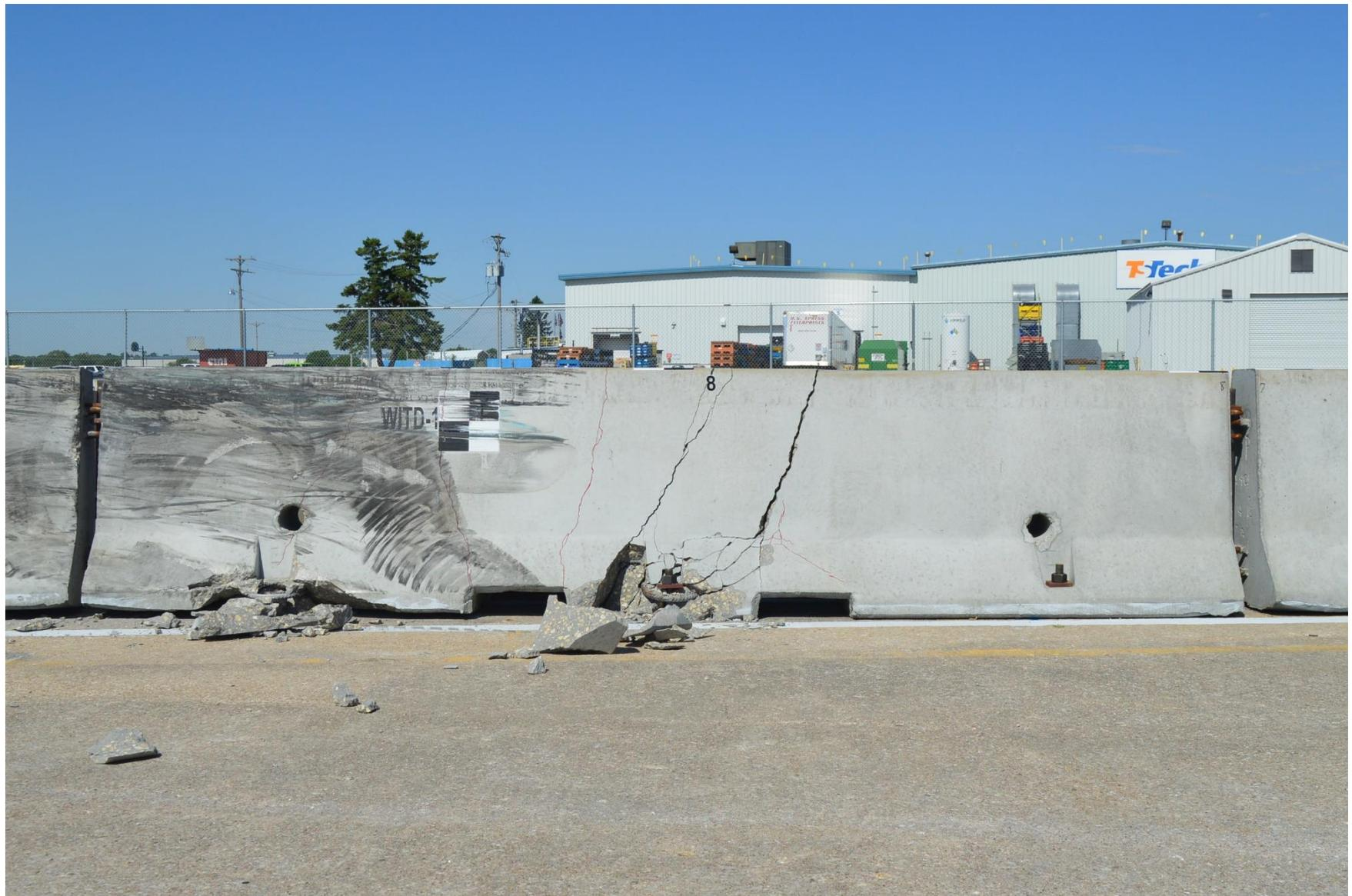
Figure 32. System Damage – Barrier No. 8 Traffic Side, Test No. WITD-1
