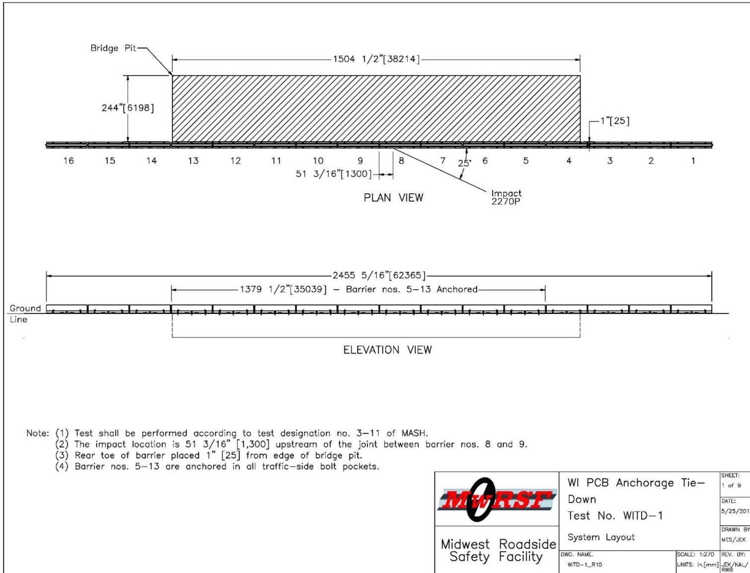
Figure 13. System Layout, Test No. WITD-1
