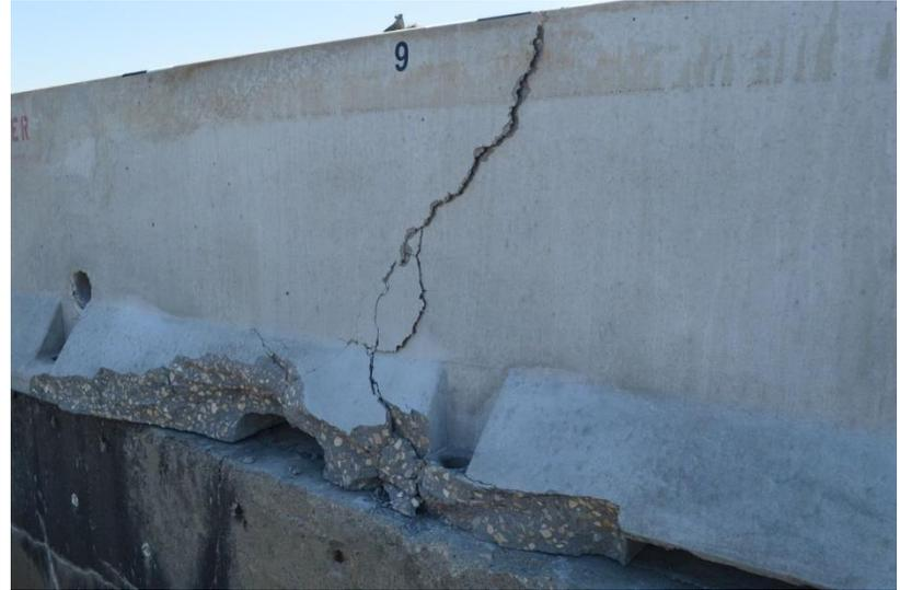
Figure 36. System Damage – Barrier Nos. 8 and 9 Non-Traffic Side, Test No. WITD-1
