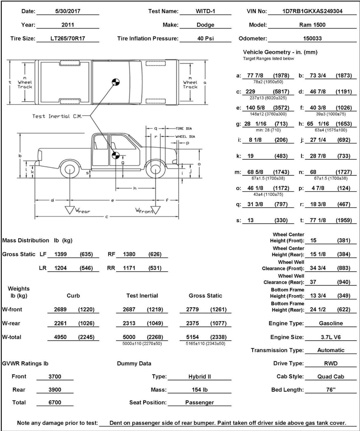
Figure 5. Vehicle Dimensions, Test No. WITD-1
