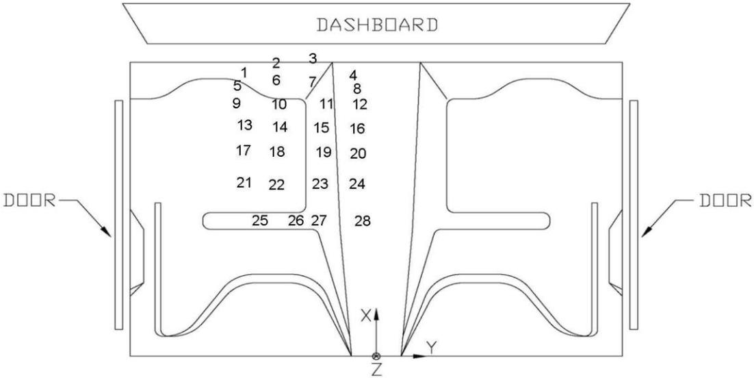
Figure D-8. Floor Pan Deformation Data – Set 2, Test No. WITD-2
