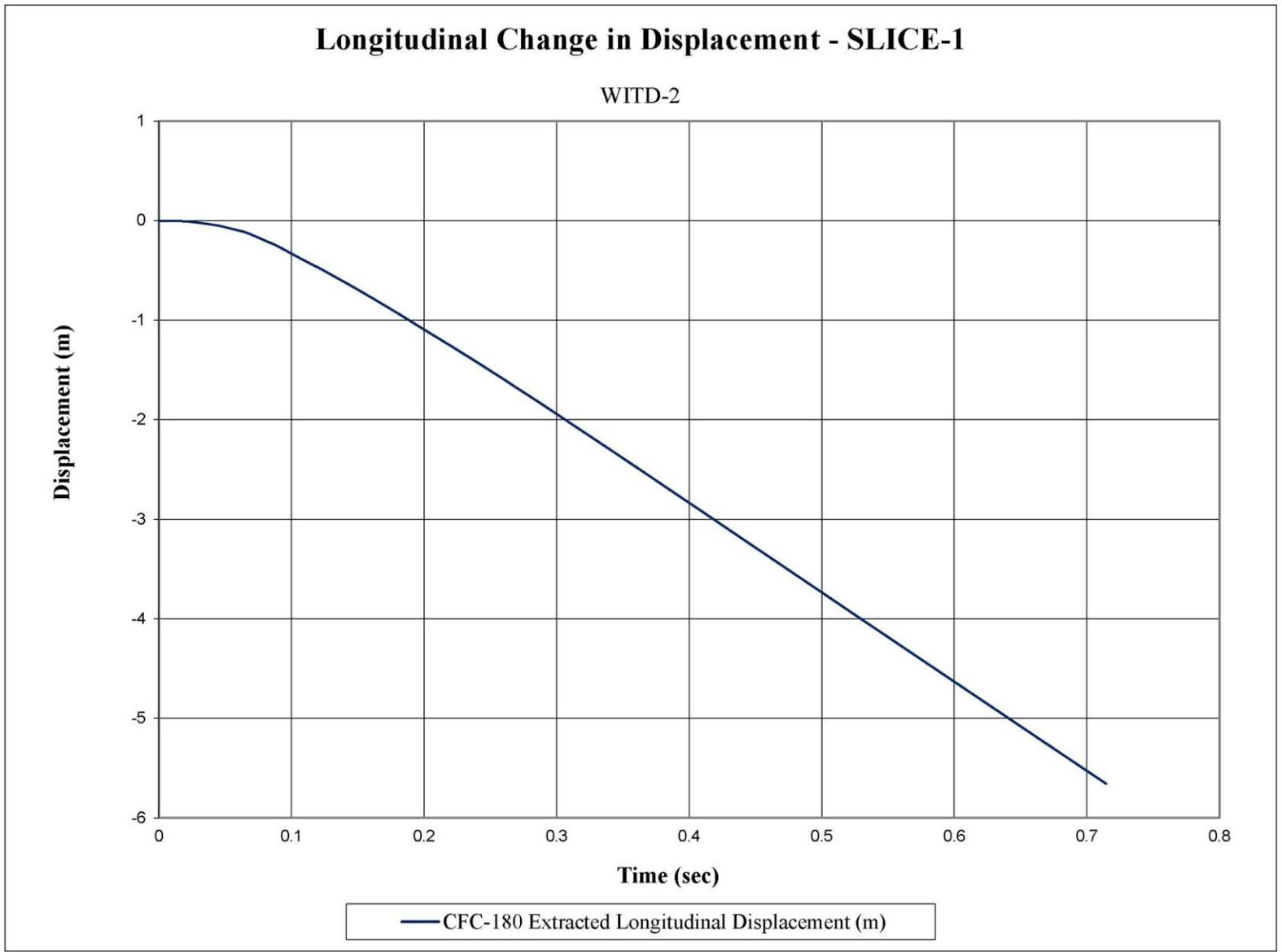
Figure F-3. Longitudinal Occupant Displacement (SLICE-1), Test No. WITD-2
