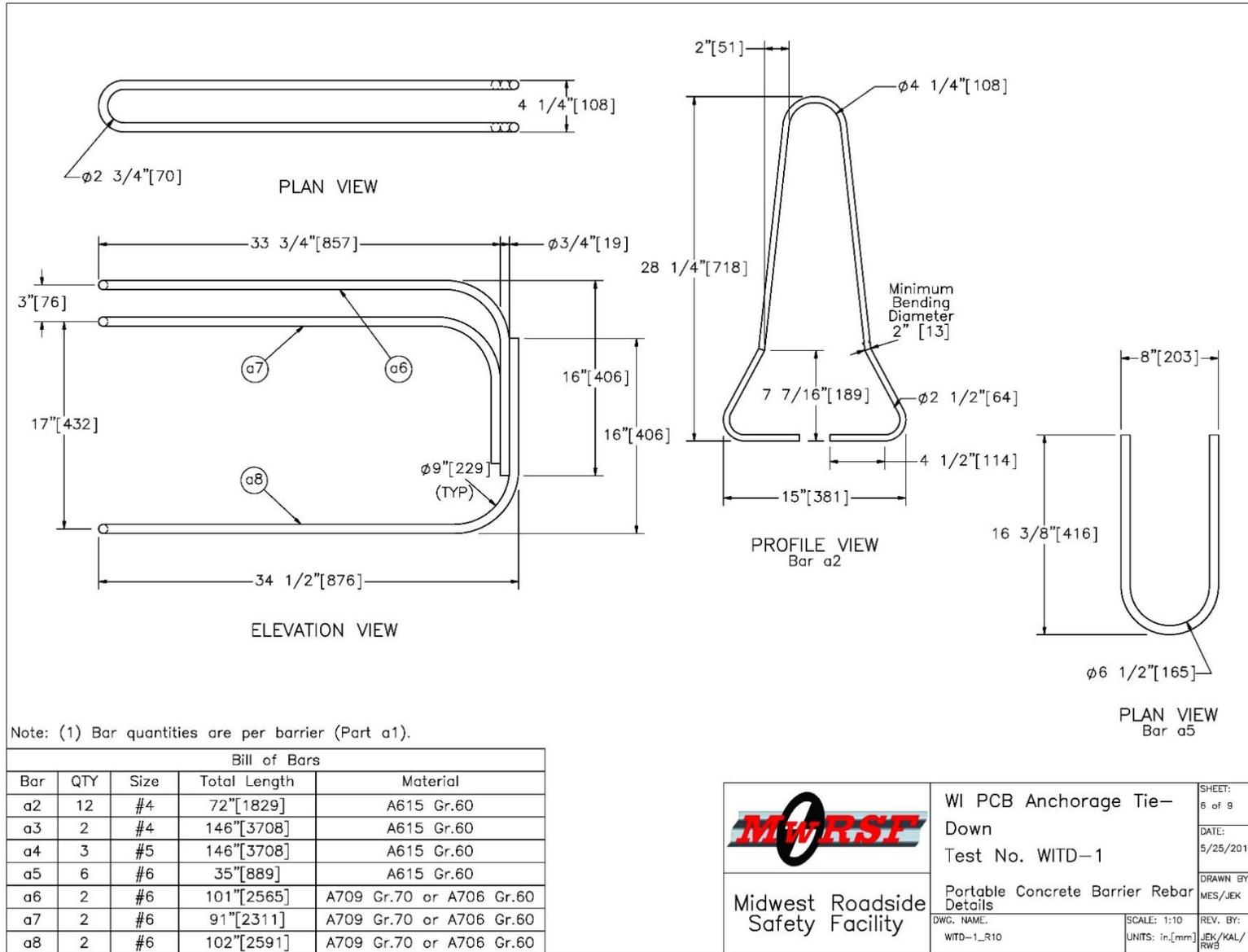
Figure 18. Portable Concrete Barrier Details, Test No. WITD-1
