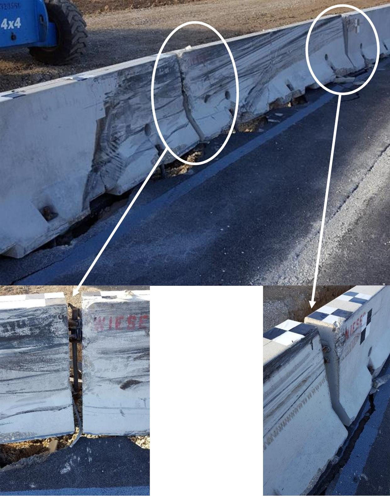
Figure 70. Barrier Joint Snag, Test No. WITD-2
