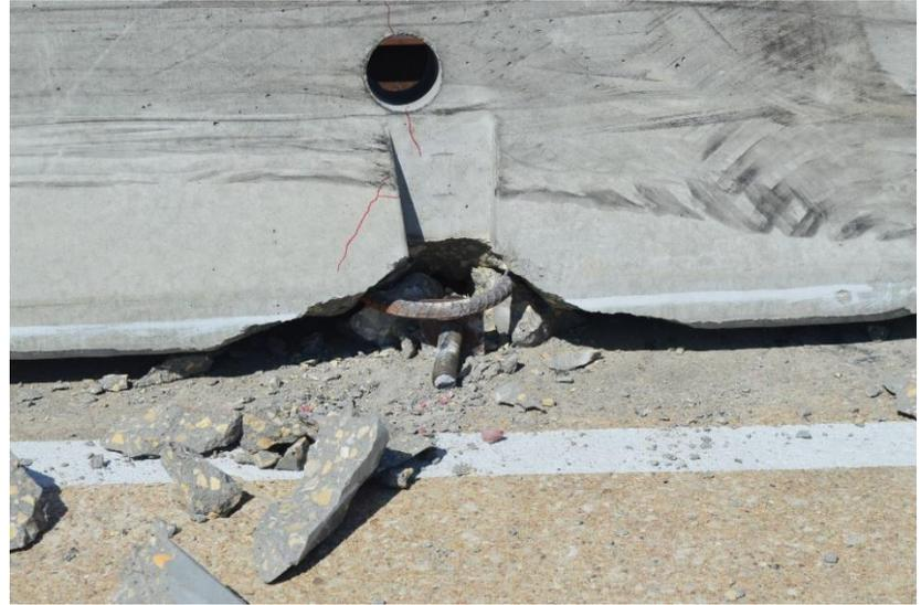
Figure 35. System Damage – Additional Views of Damage on Barrier No. 9 Traffic Side, Test No. WITD-1
