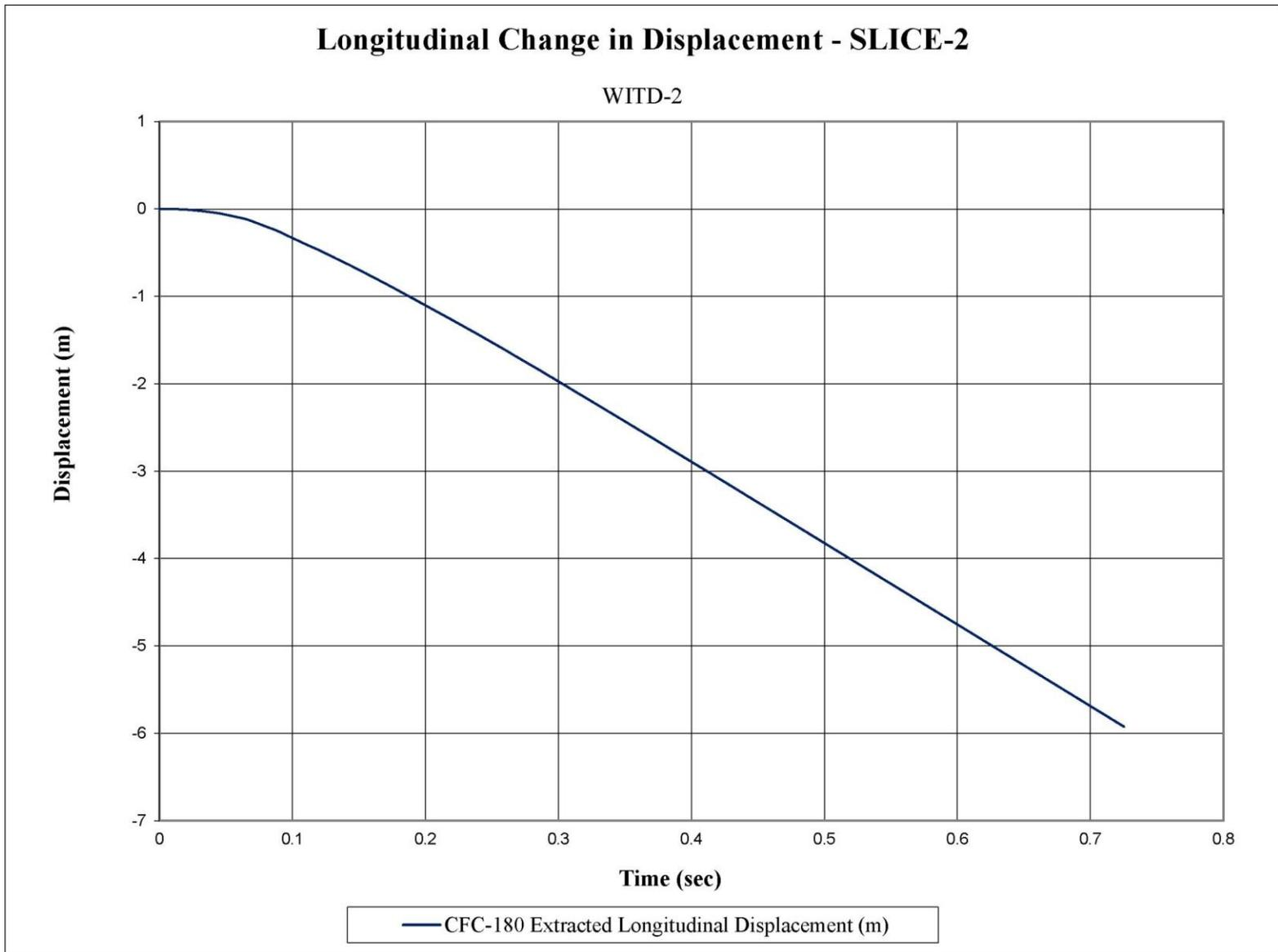
Figure F-11. Longitudinal Occupant Displacement (SLICE-2), Test No. WITD-2
