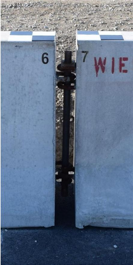
Figure 57. Connection and Anchor Pin Details, Test No. WITD-2
