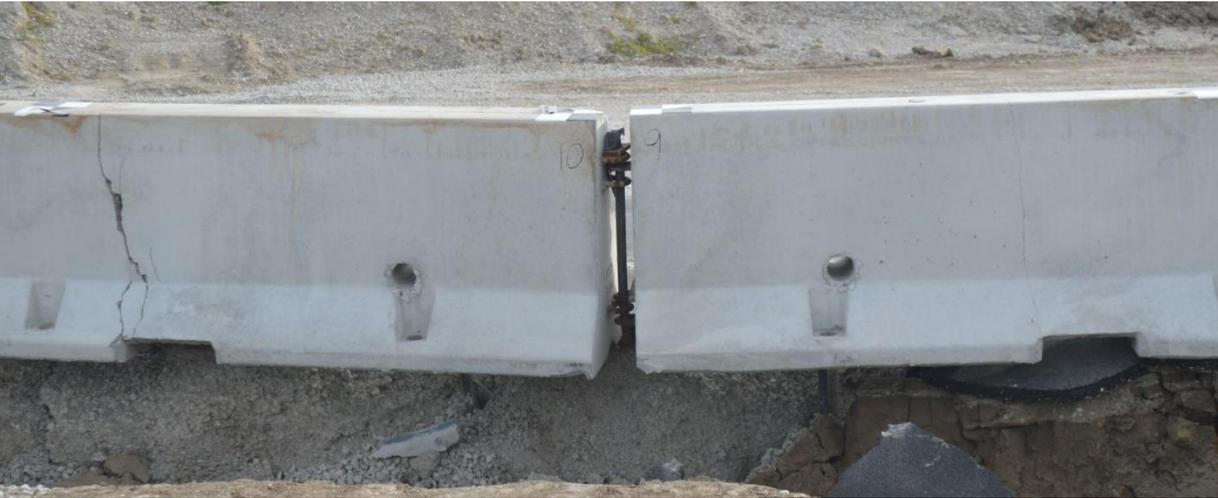
Figure 64. System Damage at Impact Location, Test No. WITD-2
