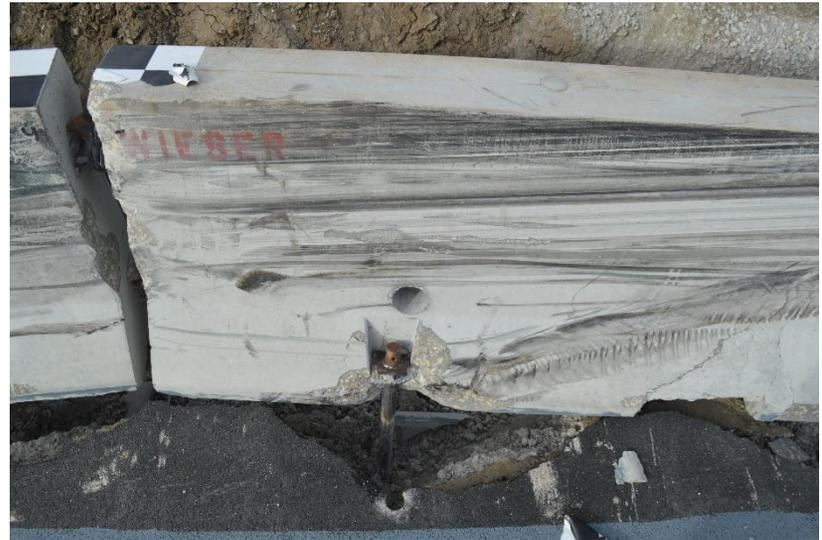
Figure 65. Barrier No. 10 Barrier Damage, Test No. WITD-2
