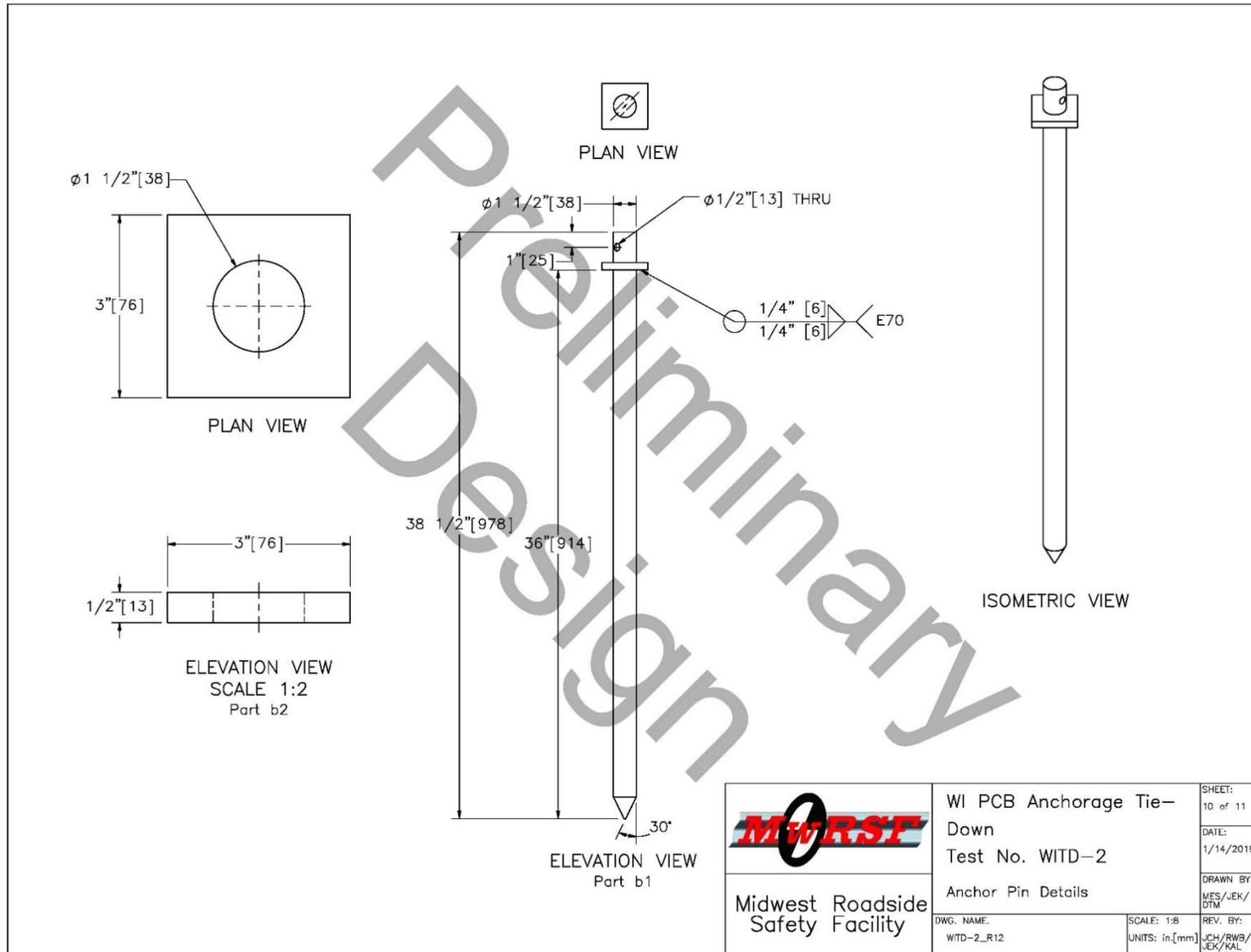
Figure 54. Anchor Pin Details, Test No. WITD-2
