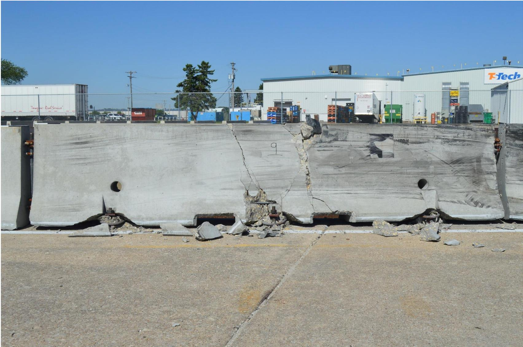
Figure 34. System Damage – Barrier No. 9 Traffic Side, Test No. WITD-1
