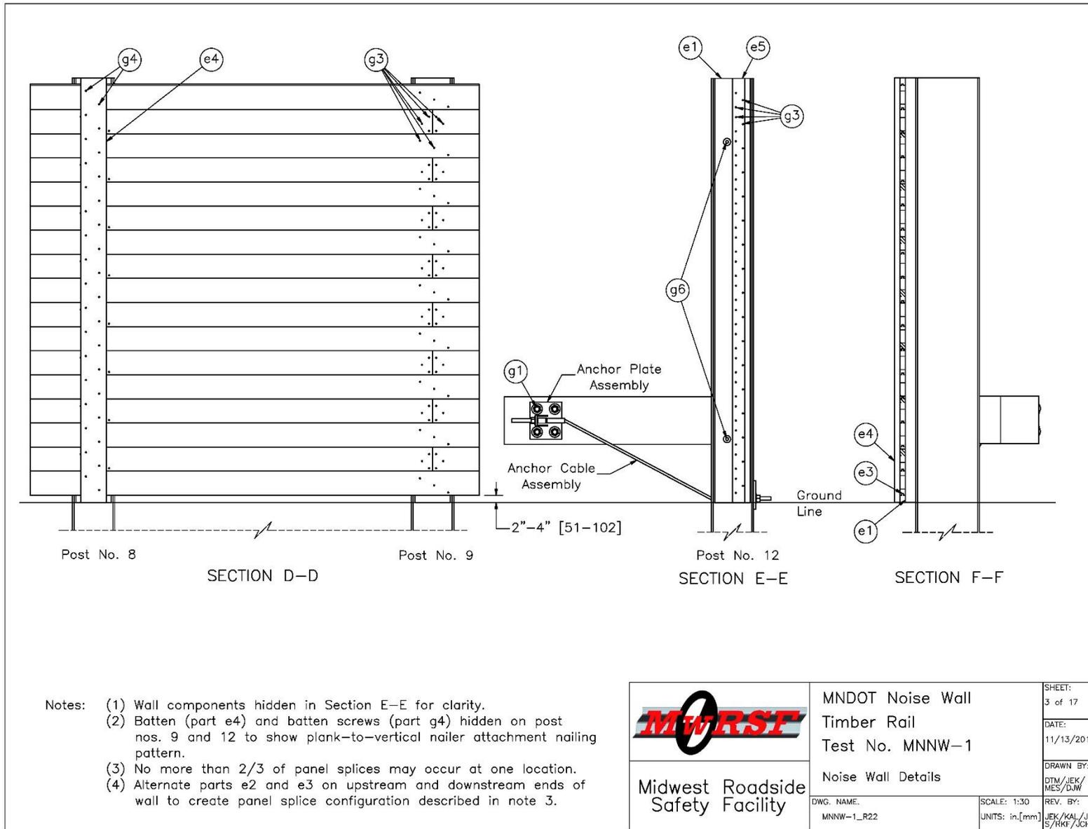
Figure 20. Noise Wall Details, Test Nos. MNNW-1 and MNNW-2 (Recommended updates provided in Chapter 12)
