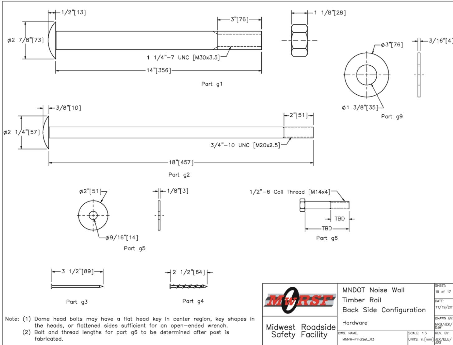
Figure 115. Hardware, Back-Side Noise Wall
