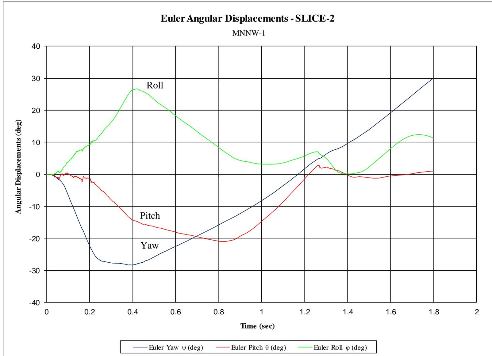
Figure F-15. Vehicle Angular Displacements (SLICE-2), Test No. MNNW-1
