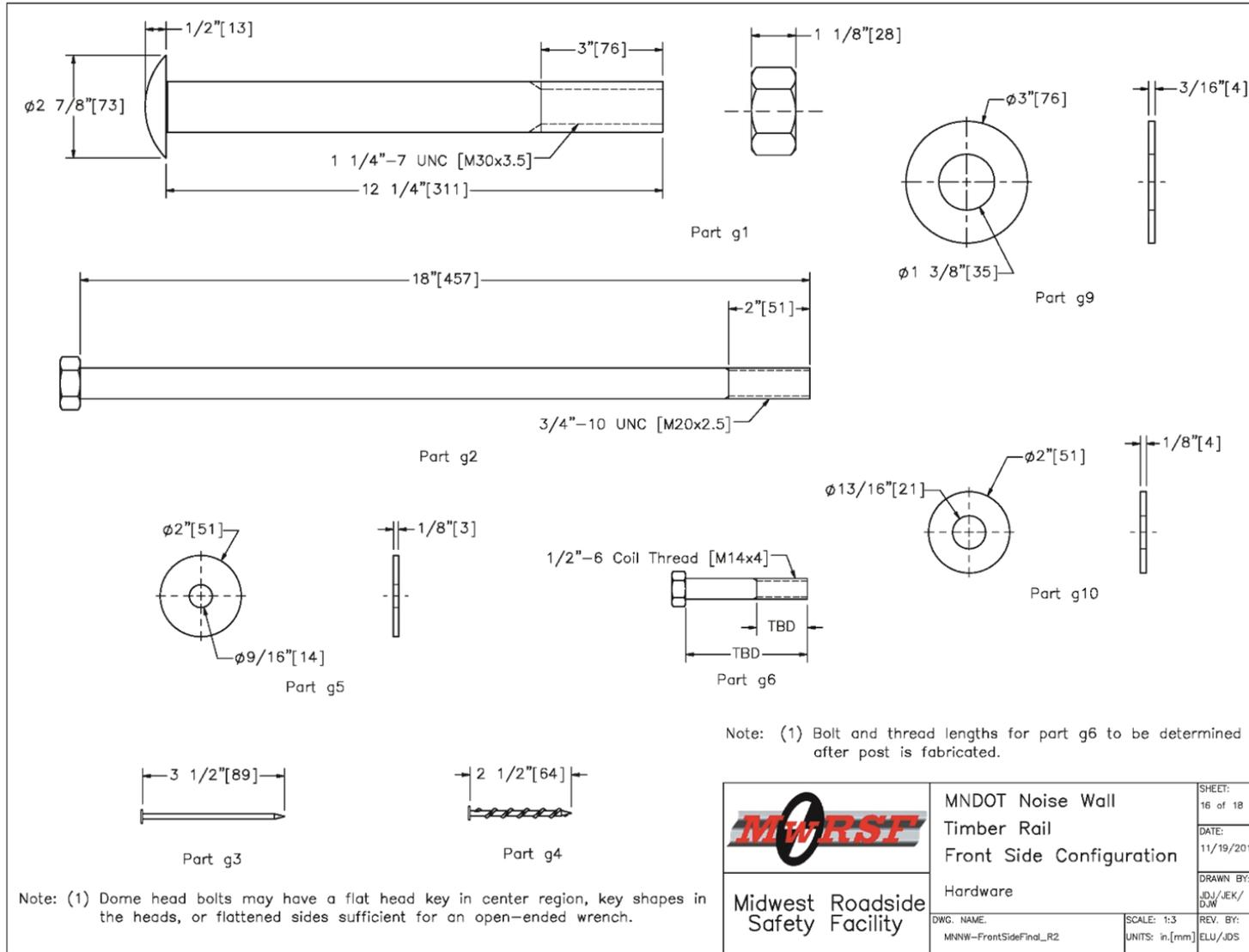
Figure 133. Hardware, Front-Side Noise Wall
