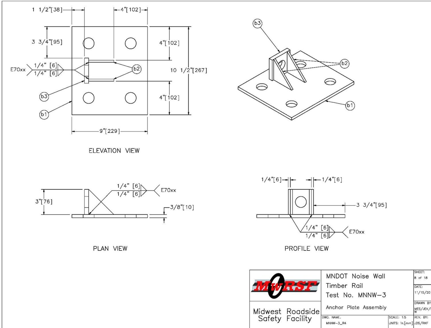
Figure 73. Anchor Plate Assembly, Test No. MNNW-3 (Recommended updates provided in Chapter 12)
