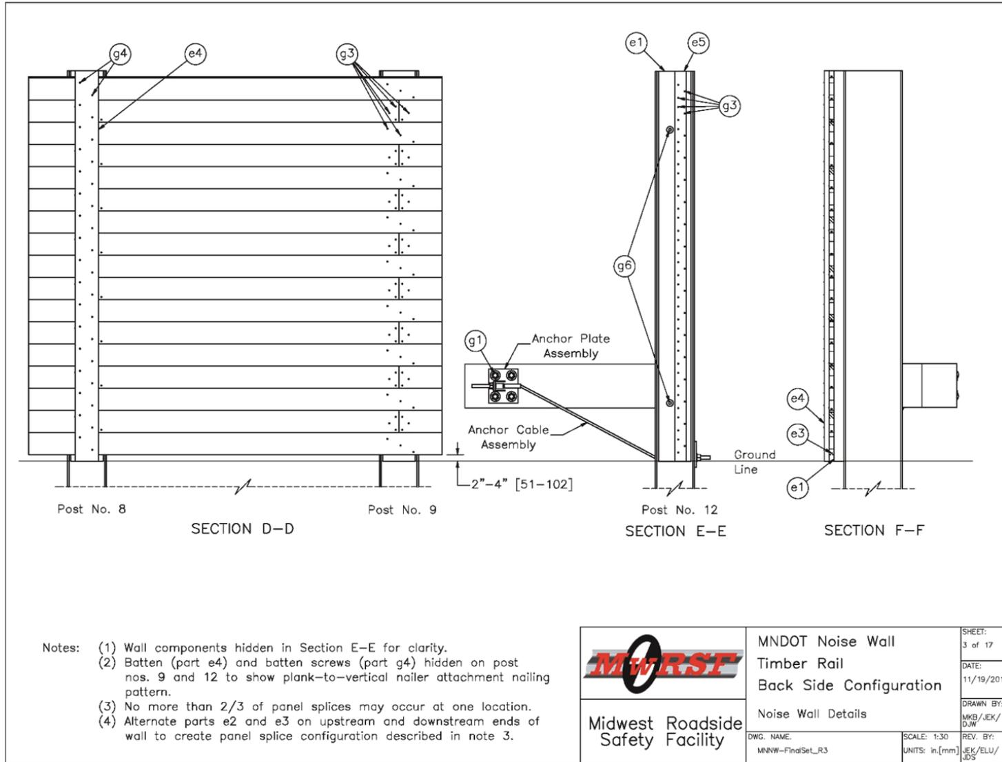
Figure 103. Noise Wall Details, Back-Side Noise Wall
