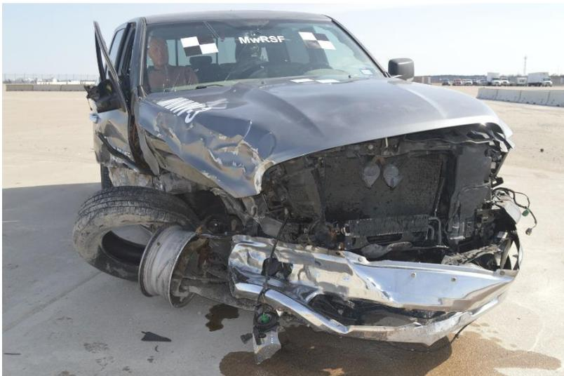
Figure 99. Vehicle Damage, Test No. MNNW-3
