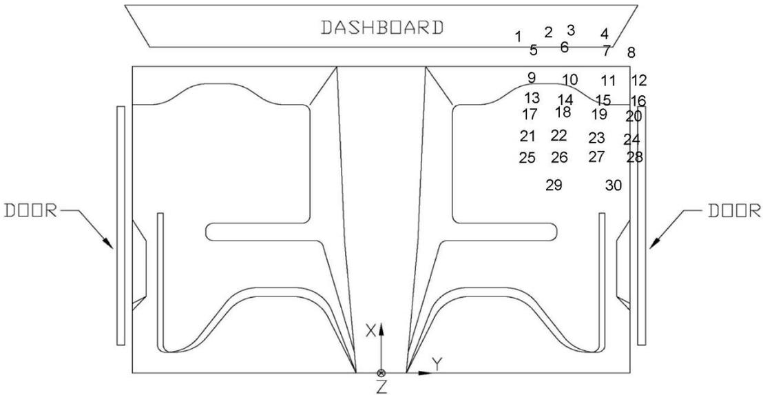
Figure E-8. Floor Pan Deformation Data – Set 2, Test No. MNNW-2
