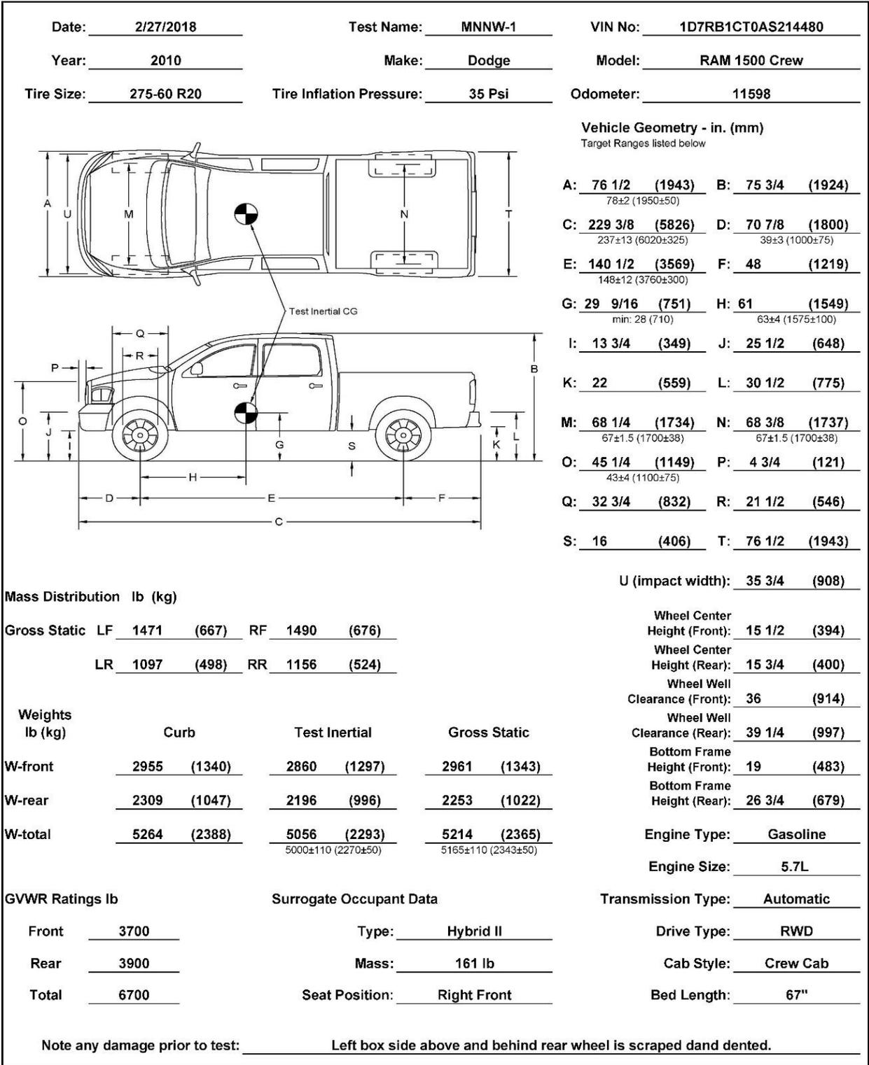
Figure 4. Vehicle Dimensions, Test No. MNNW-1
