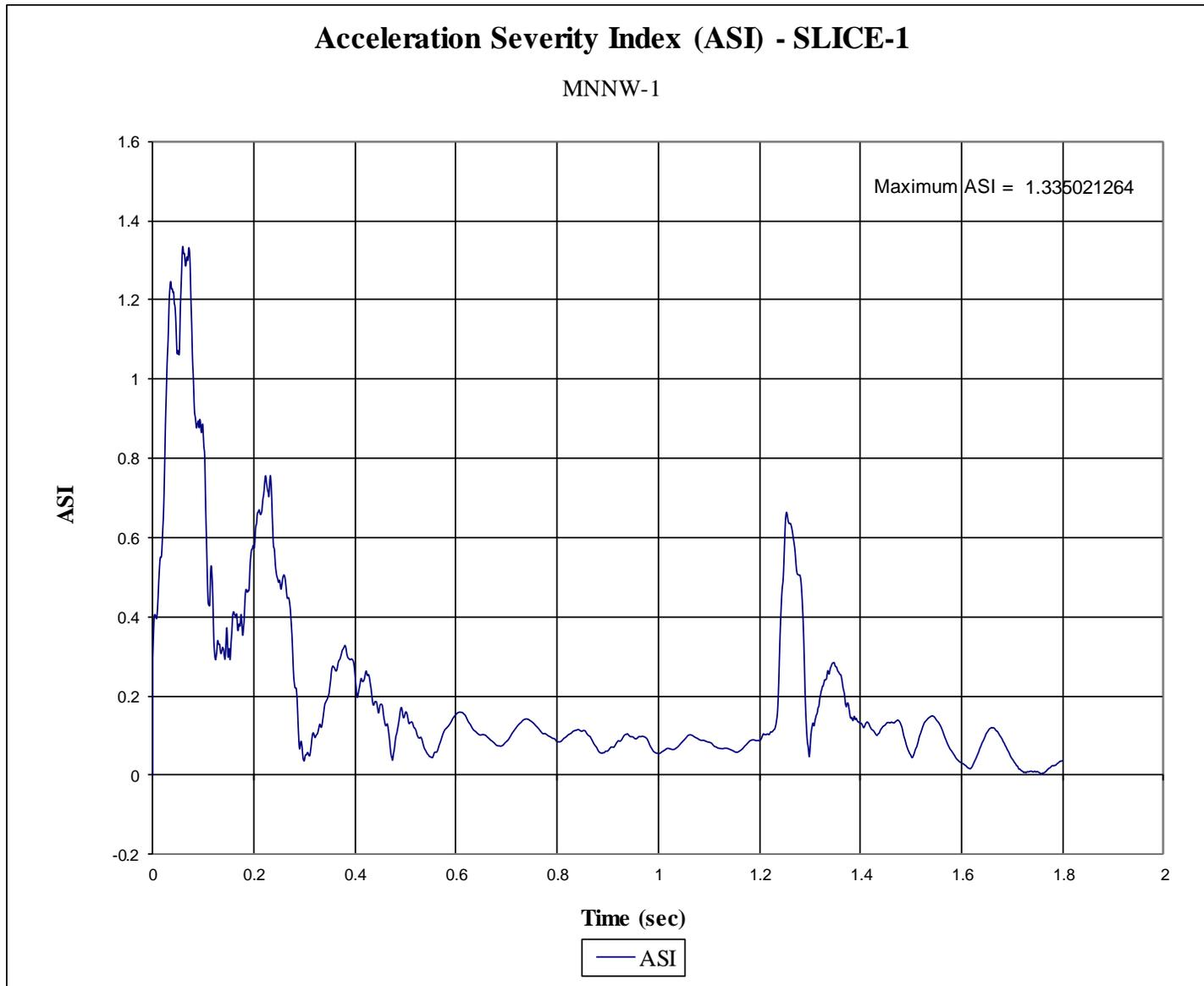
Figure F-8. Acceleration Severity Index (SLICE-1), Test No. MNNW-1
