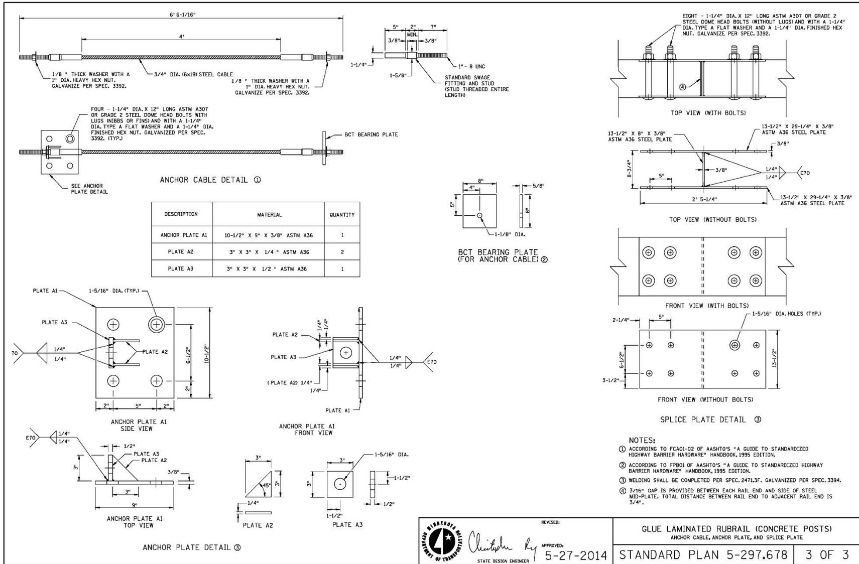
Figure A-6. Glue Laminated Rubrail (Concrete Posts) – Anchor Cable, Anchor Plate, and Splice Plate
