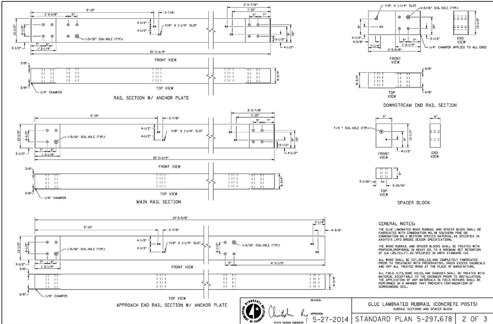
Figure A-5. Glue Laminated Rubrail (Concrete Posts) – Rubrail Sections and Spacer Block
