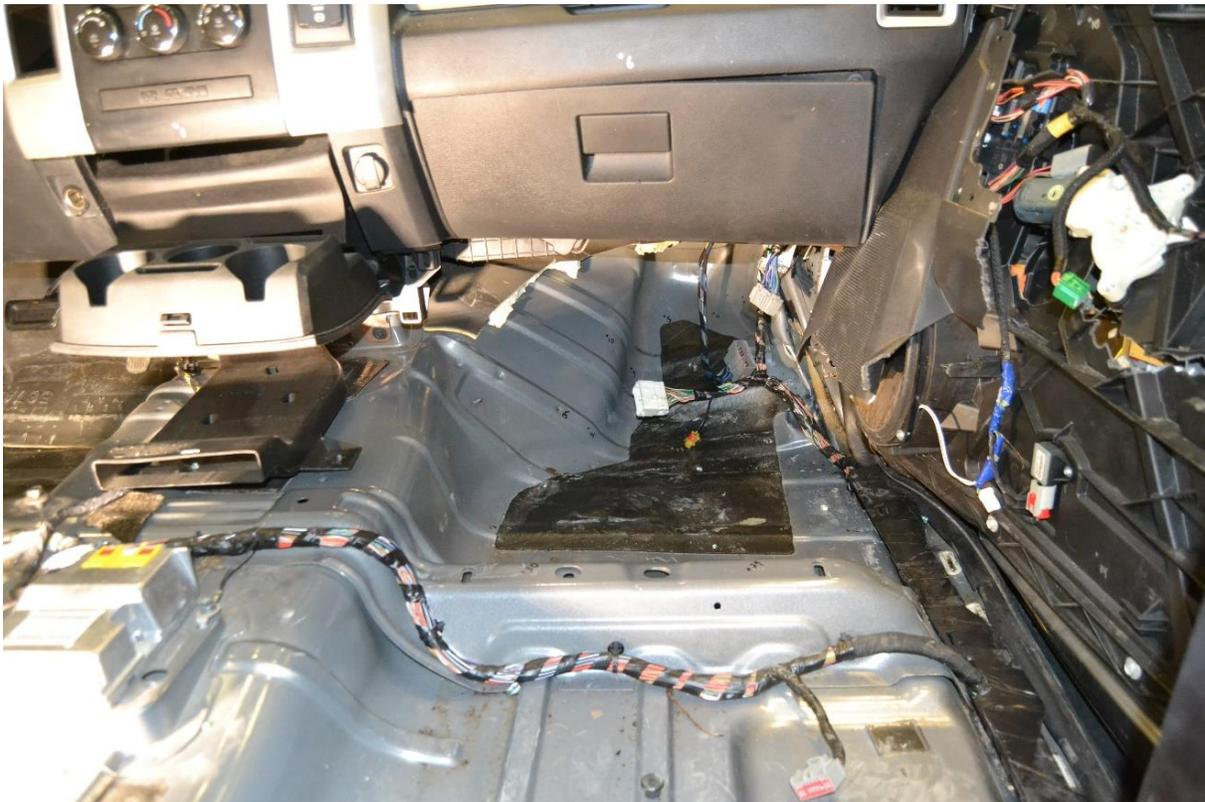
Figure 97. Vehicle Undercarriage and Occupant Compartment Damage, Test No. MNNW-3
