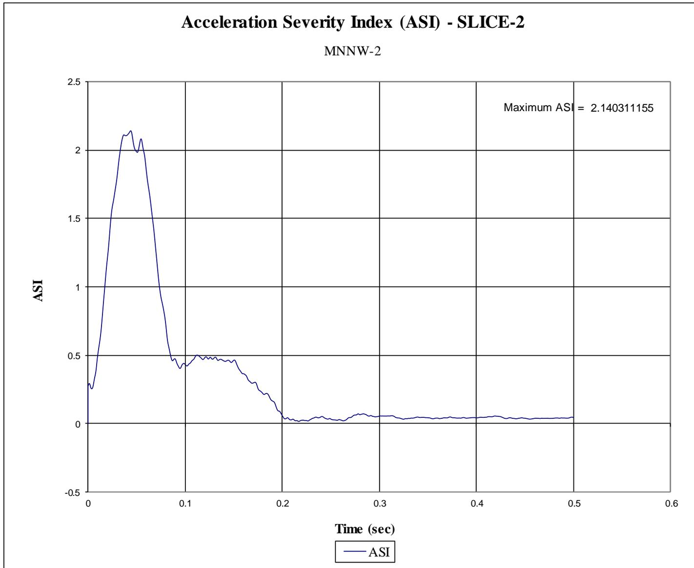
Figure G-16. Acceleration Severity Index (SLICE-2), Test No. MNNW-2
