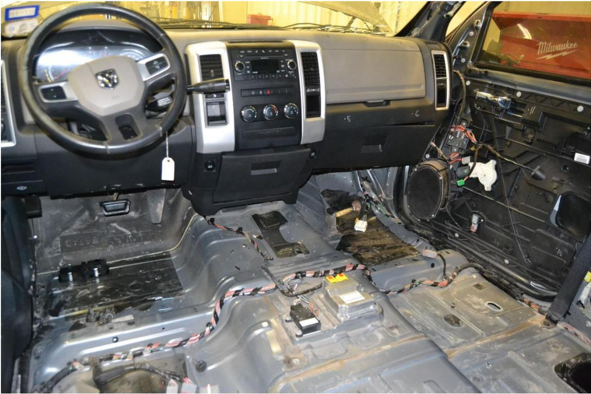
Figure 50. Vehicle Undercarriage and Occupant Compartment Damage, Test No. MNNW-1
