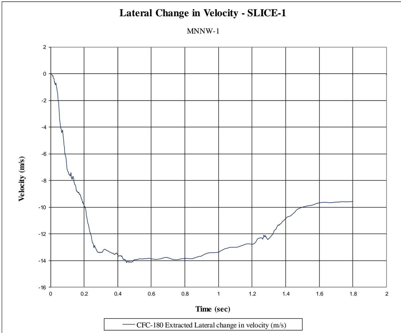
Figure F-5. Lateral Occupant Impact Velocity (SLICE-1), Test No. MNNW-1
