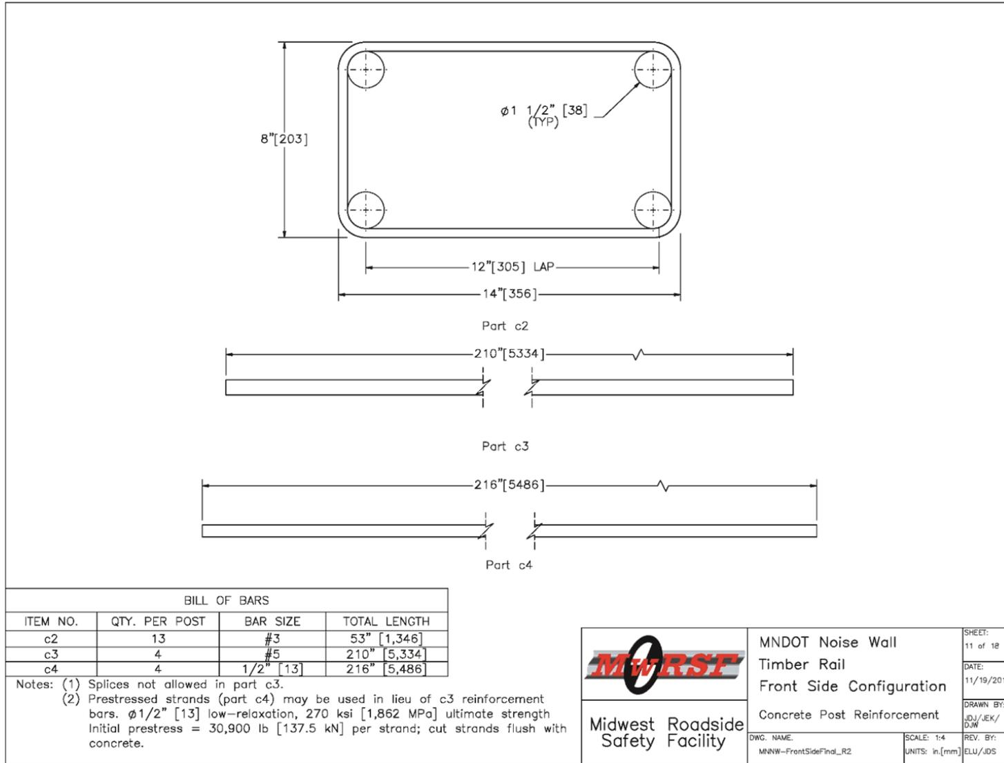
Figure 128. Concrete Post Reinforcement, Front-Side Noise Wall
