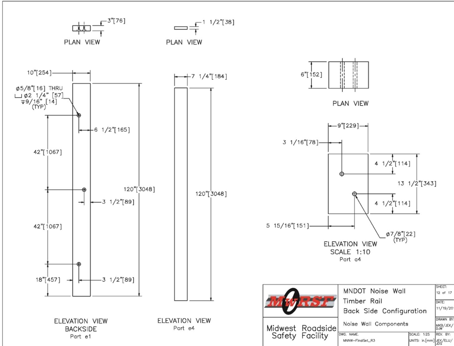
Figure 112. Noise Wall Components, Back-Side Noise Wall
