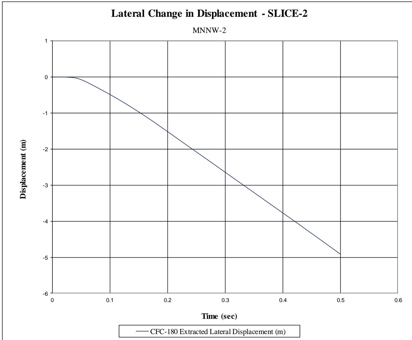
Figure G-14. Lateral Occupant Displacement (SLICE-2), Test No. MNNW-2
