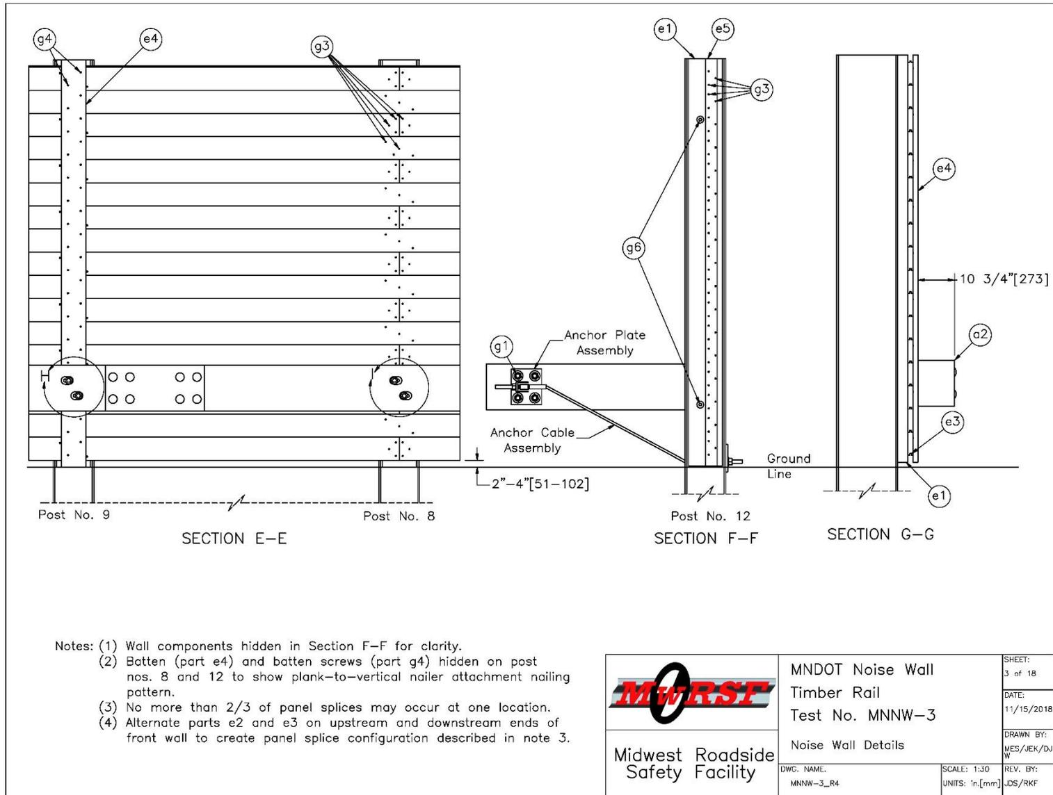
Figure 68. Noise Wall Details, Test No. MNNW-3 (Recommended updates provided in Chapter 12)
