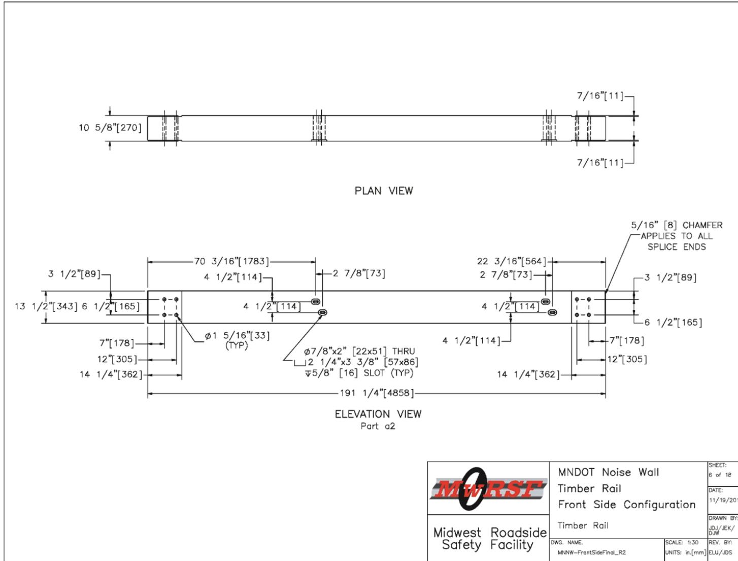
Figure 123. Timber Rail, Front-Side Noise Wall
