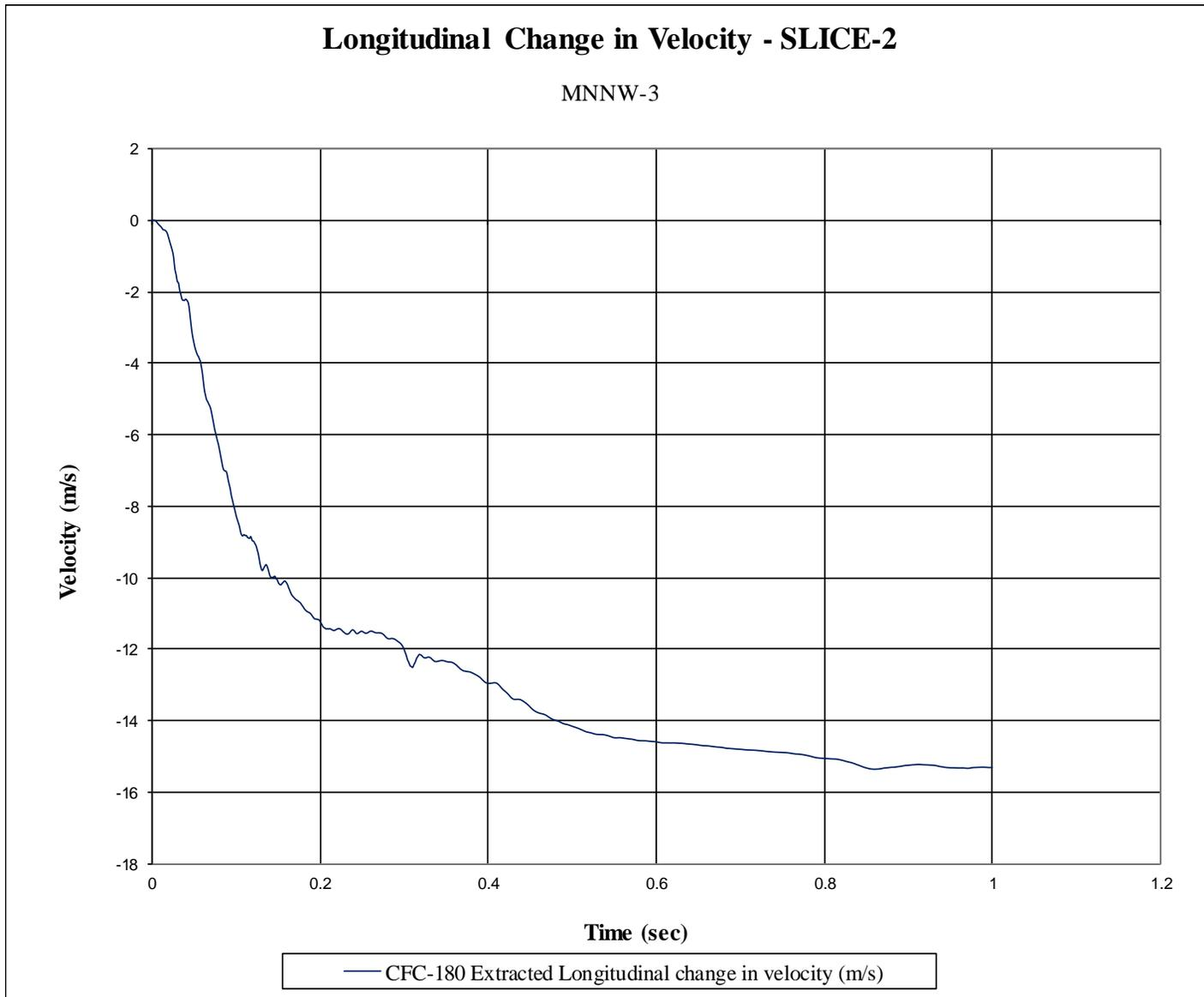
Figure H-10. Longitudinal Occupant Impact Velocity (SLICE-2), Test No. MNNW-3
