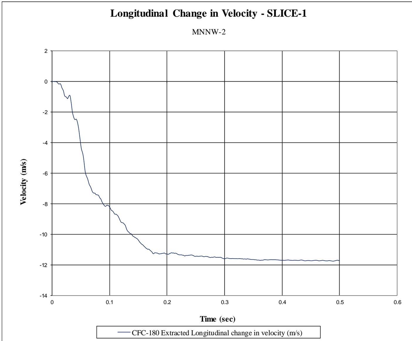
Figure G-2. Longitudinal Occupant Impact Velocity (SLICE-1), Test No. MNNW-2
