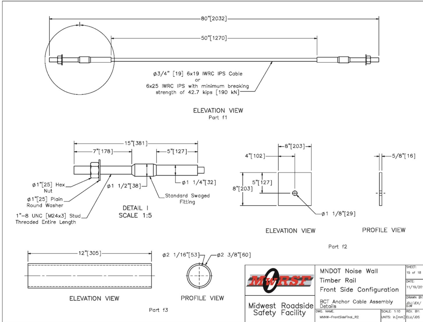
Figure 132. BCT Anchor Cable Assembly Details, Front-Side Noise Wall
