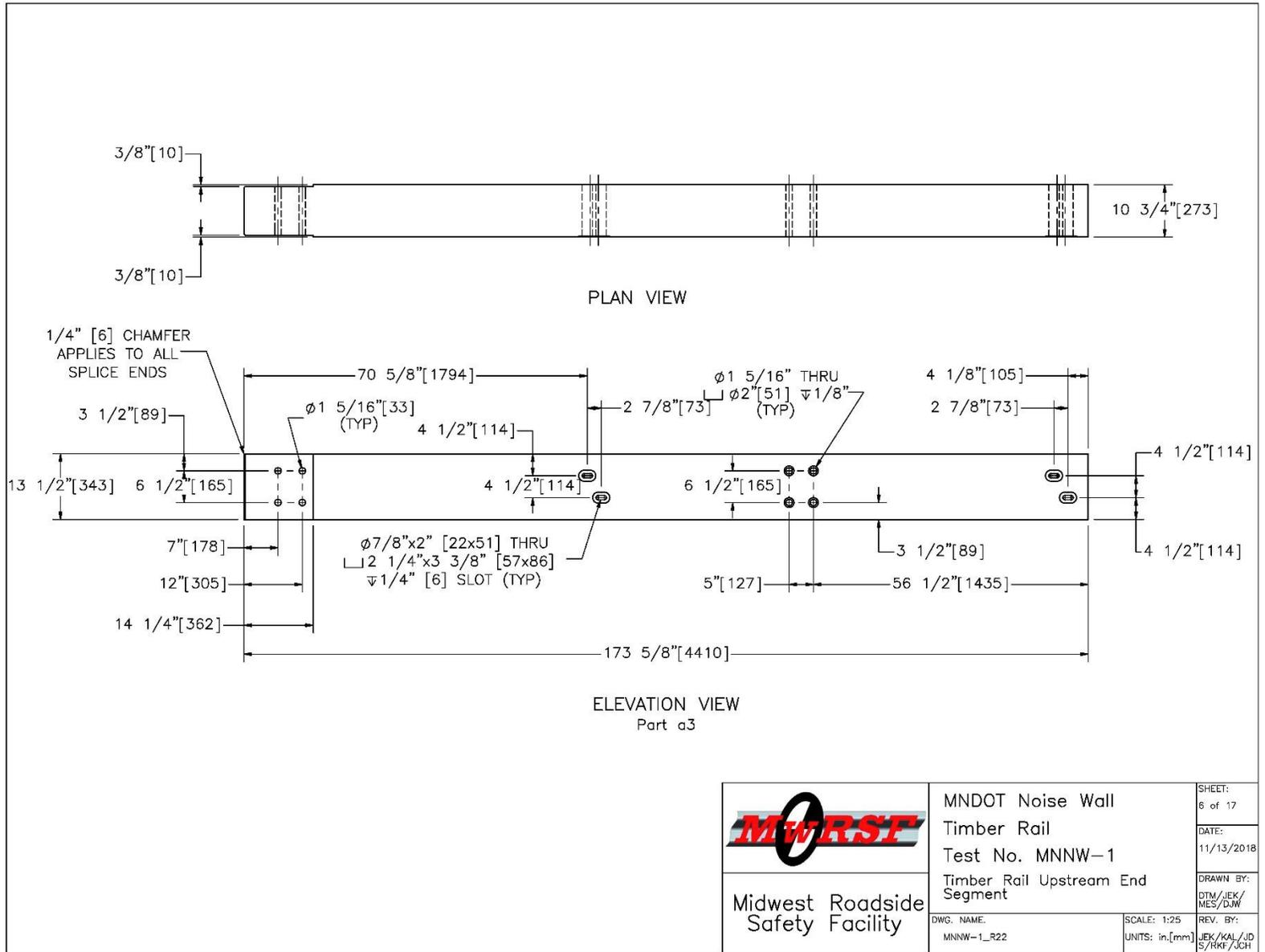
Figure 23. Timber Rail Upstream End Segment, Test Nos. MNNW-1 and MNNW-2 (Recommended updates provided in Chapter 12)
