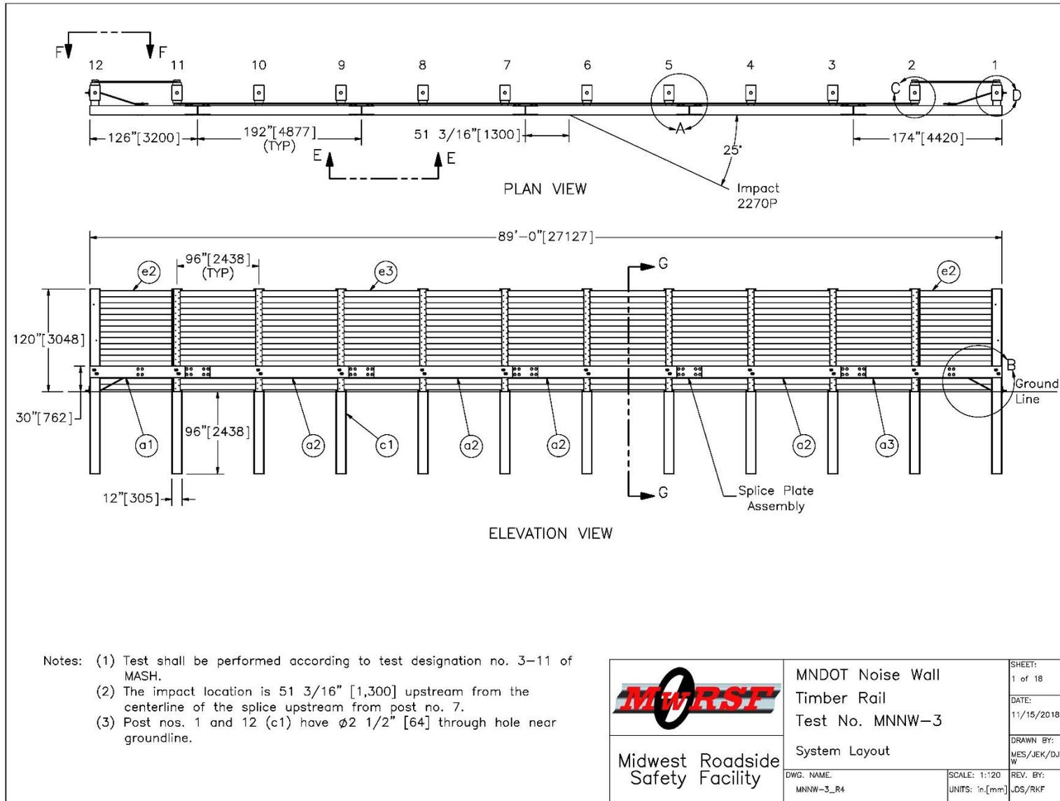
Figure 66. System Layout, Test No. MNNW-3 (Recommended updates provided in Chapter 12)
