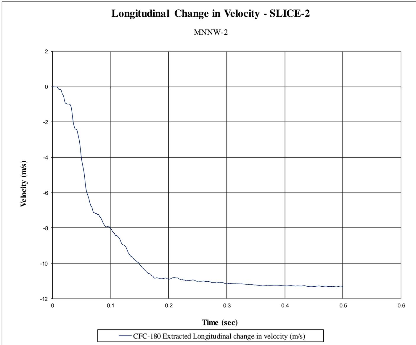
Figure G-10. Longitudinal Occupant Impact Velocity (SLICE-2), Test No. MNNW-2
