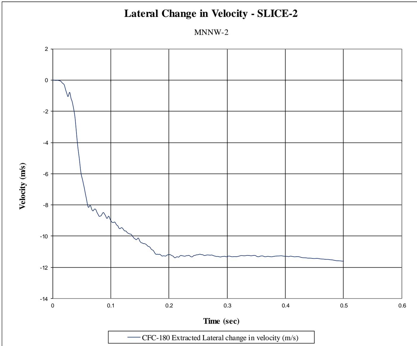
Figure G-13. Lateral Occupant Impact Velocity (SLICE-2), Test No. MNNW-2
