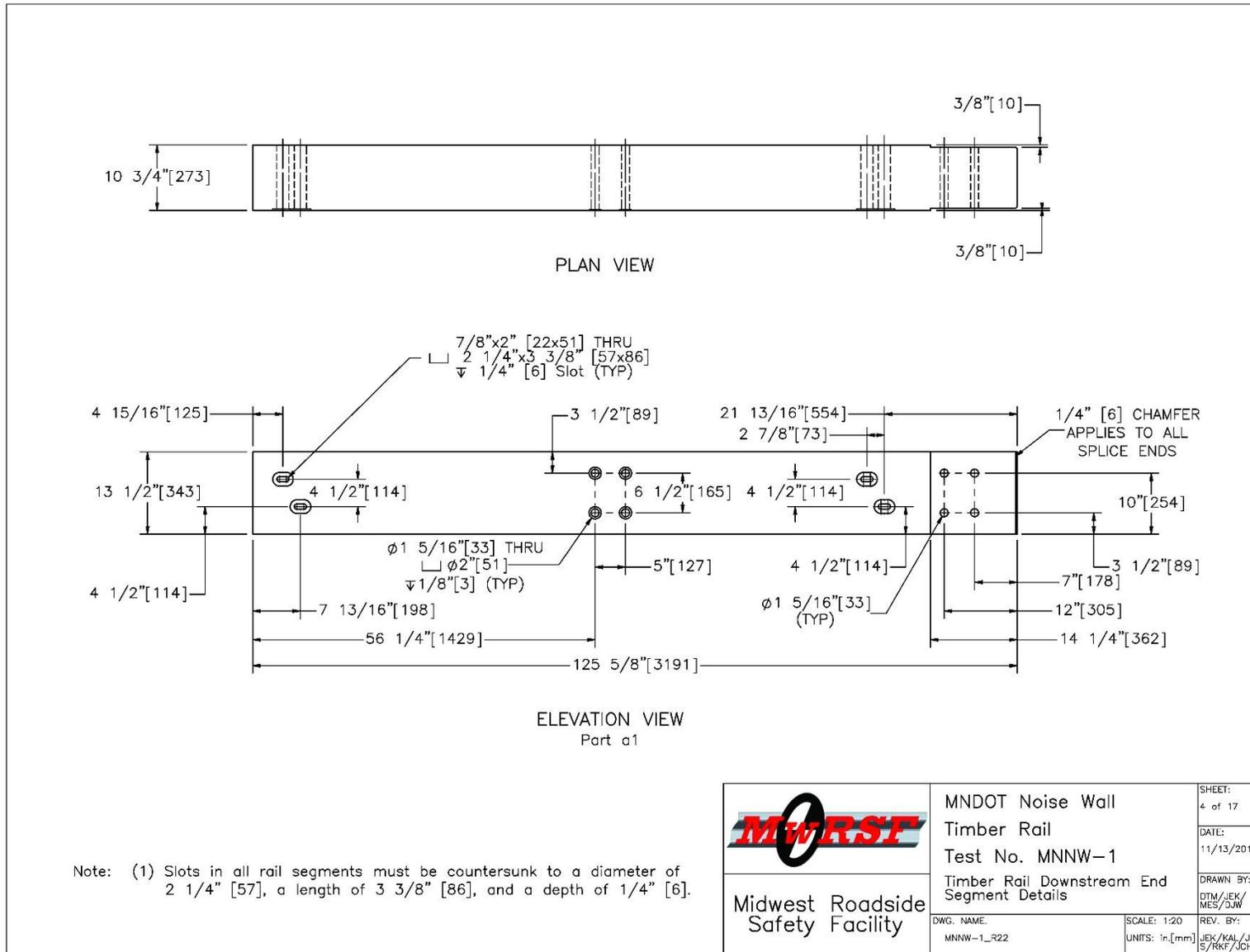
Figure 21. Timber Rail Downstream End Segment Details, Test Nos. MNNW-1 and MNNW-2 (Recommended updates provided in Chapter 12)
