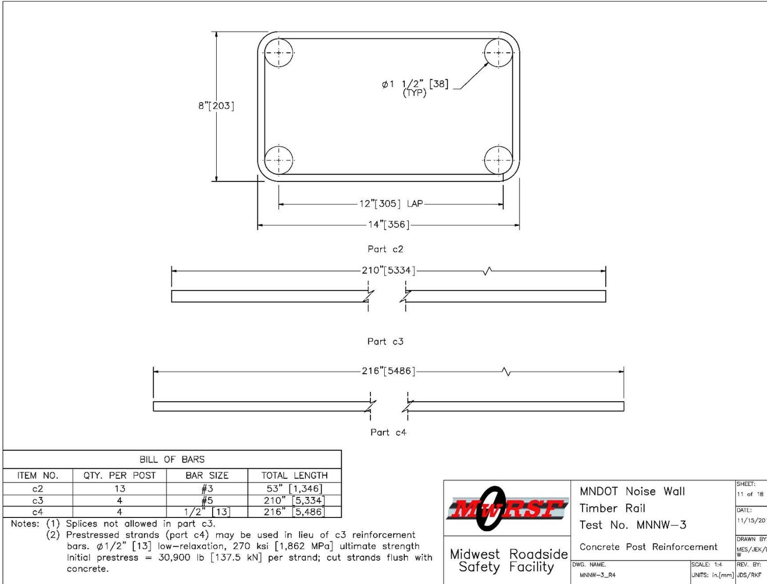
Figure 76. Concrete Post Reinforcement, Test No. MNNW-3 (Recommended updates provided in Chapter 12)
