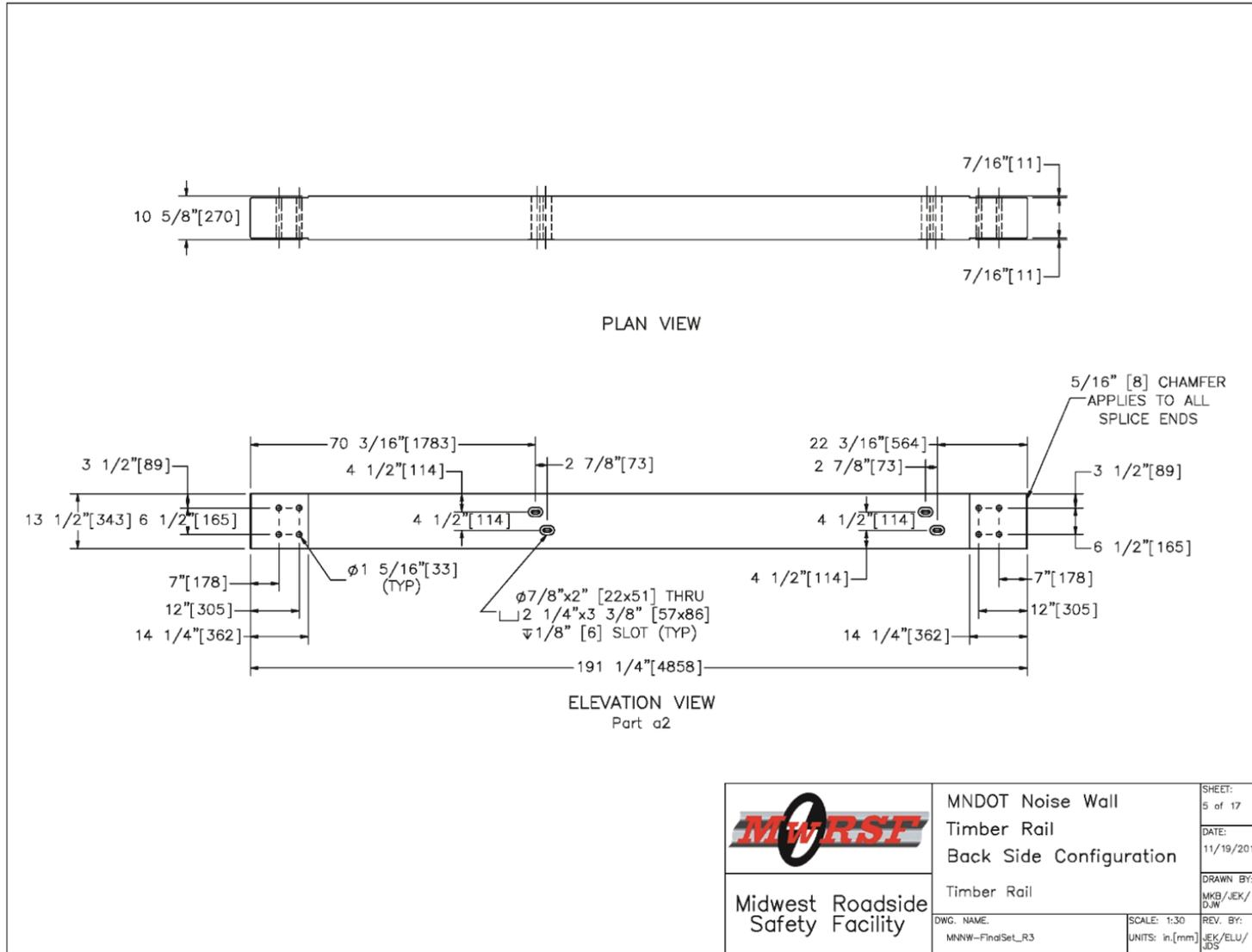
Figure 105. Timber Rail, Back-Side Noise Wall
