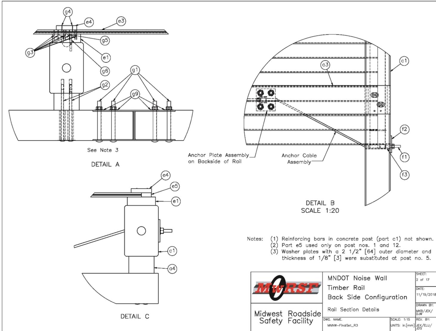
Figure 102. Rail Section Details, Back-Side Noise Wall
