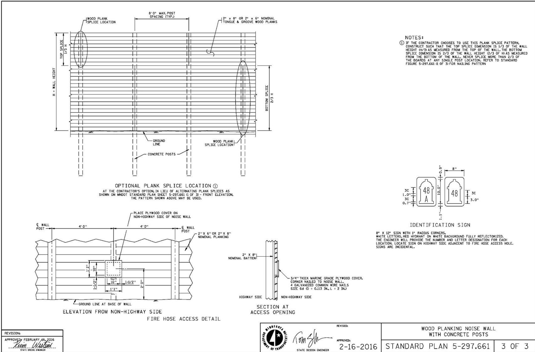
Figure A-3. Wood Planking Noise Wall with Concrete Posts
