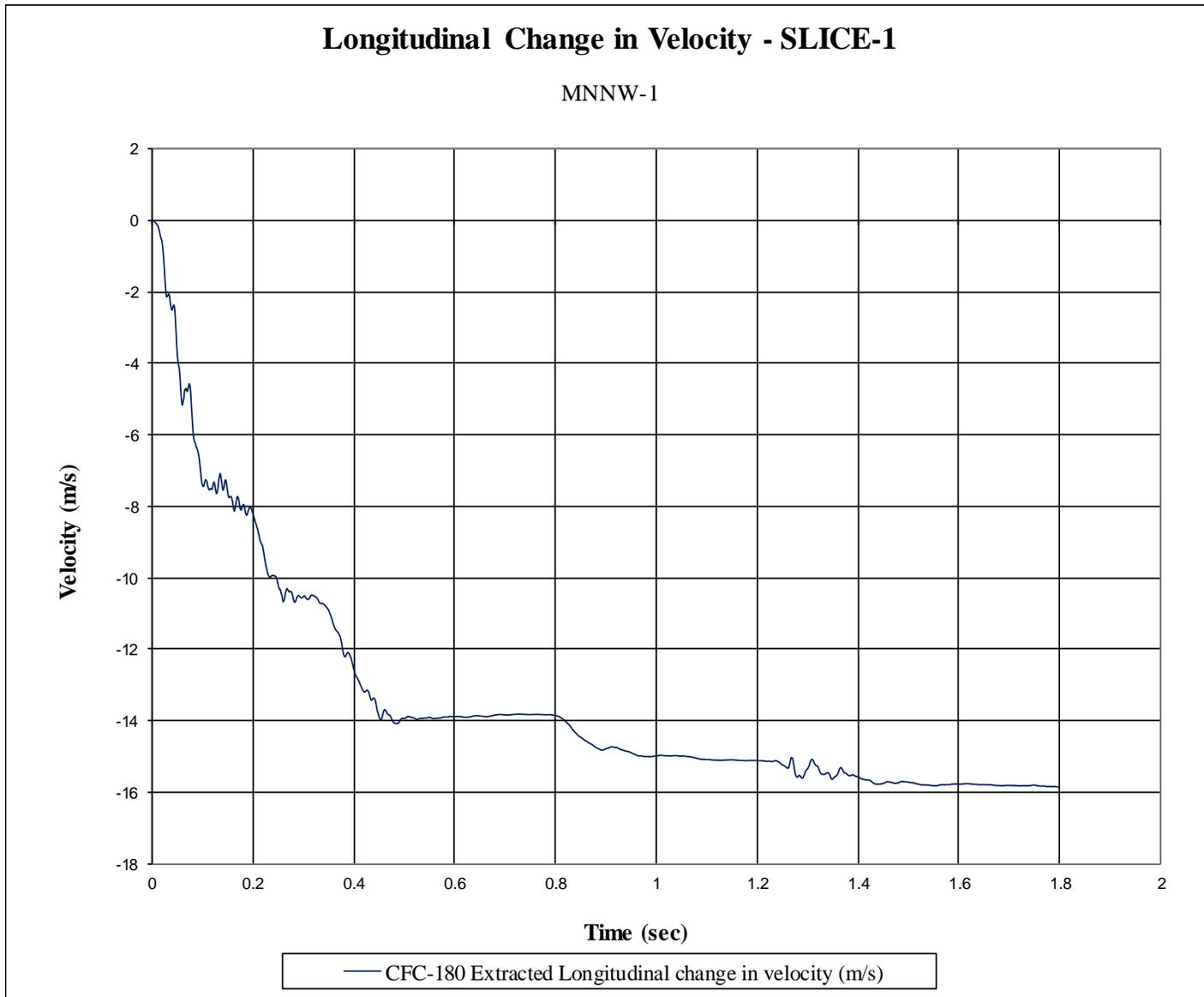
Figure F-2. Longitudinal Occupant Impact Velocity (SLICE-1), Test No. MNNW-1
