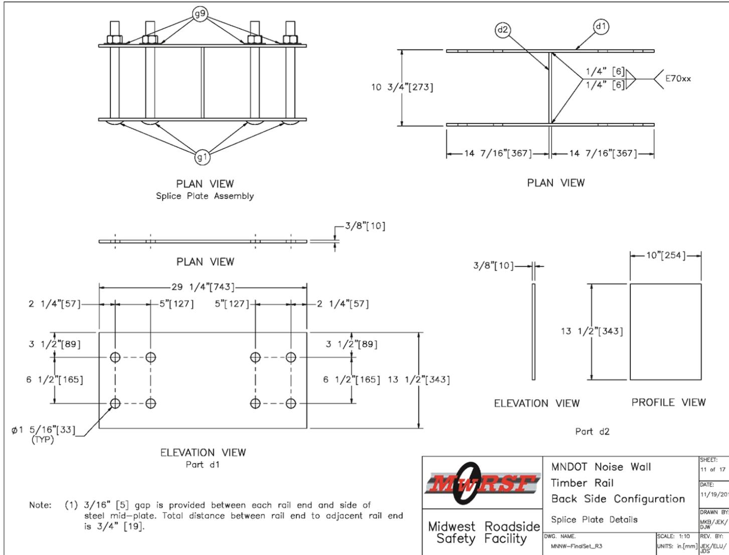
Figure 111. Splice Plate Details, Back-Side Noise Wall
