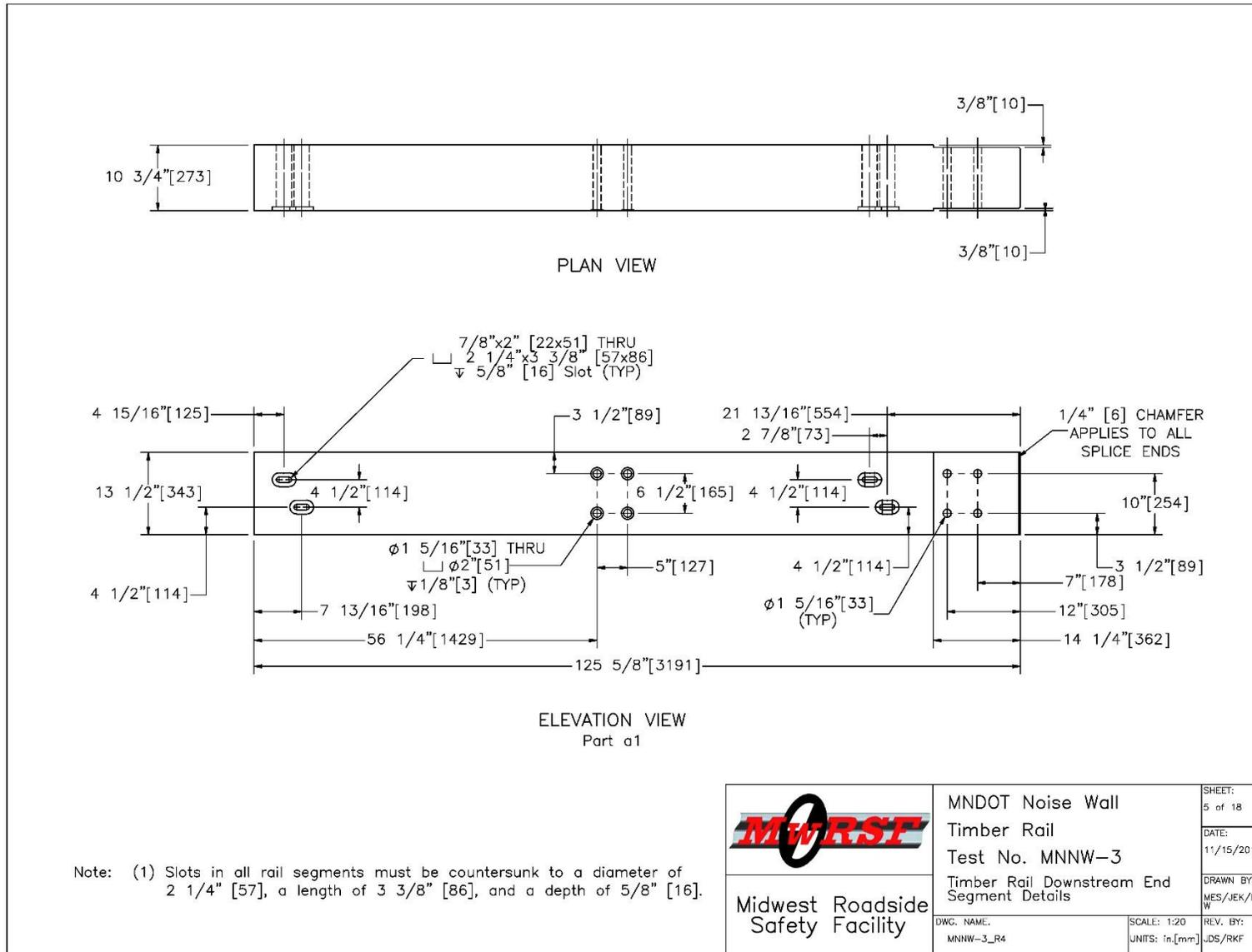
Figure 70. Timber Rail Downstream End Segment Details, Test No. MNNW-3 (Recommended updates provided in Chapter 12)
