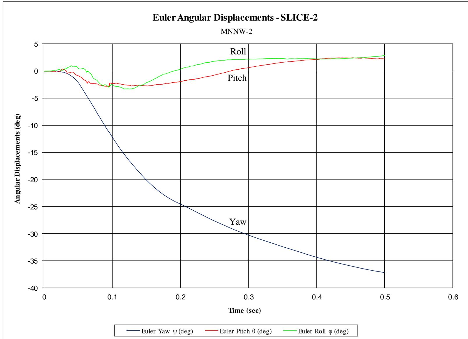
Figure G-15. Vehicle Angular Displacements (SLICE-2), Test No. MNNW-2
