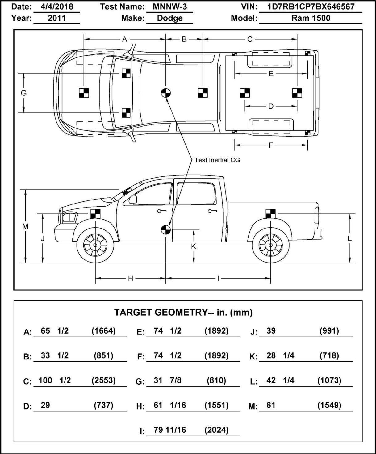
Figure 13. Target Geometry, Test No. MNNW-3
