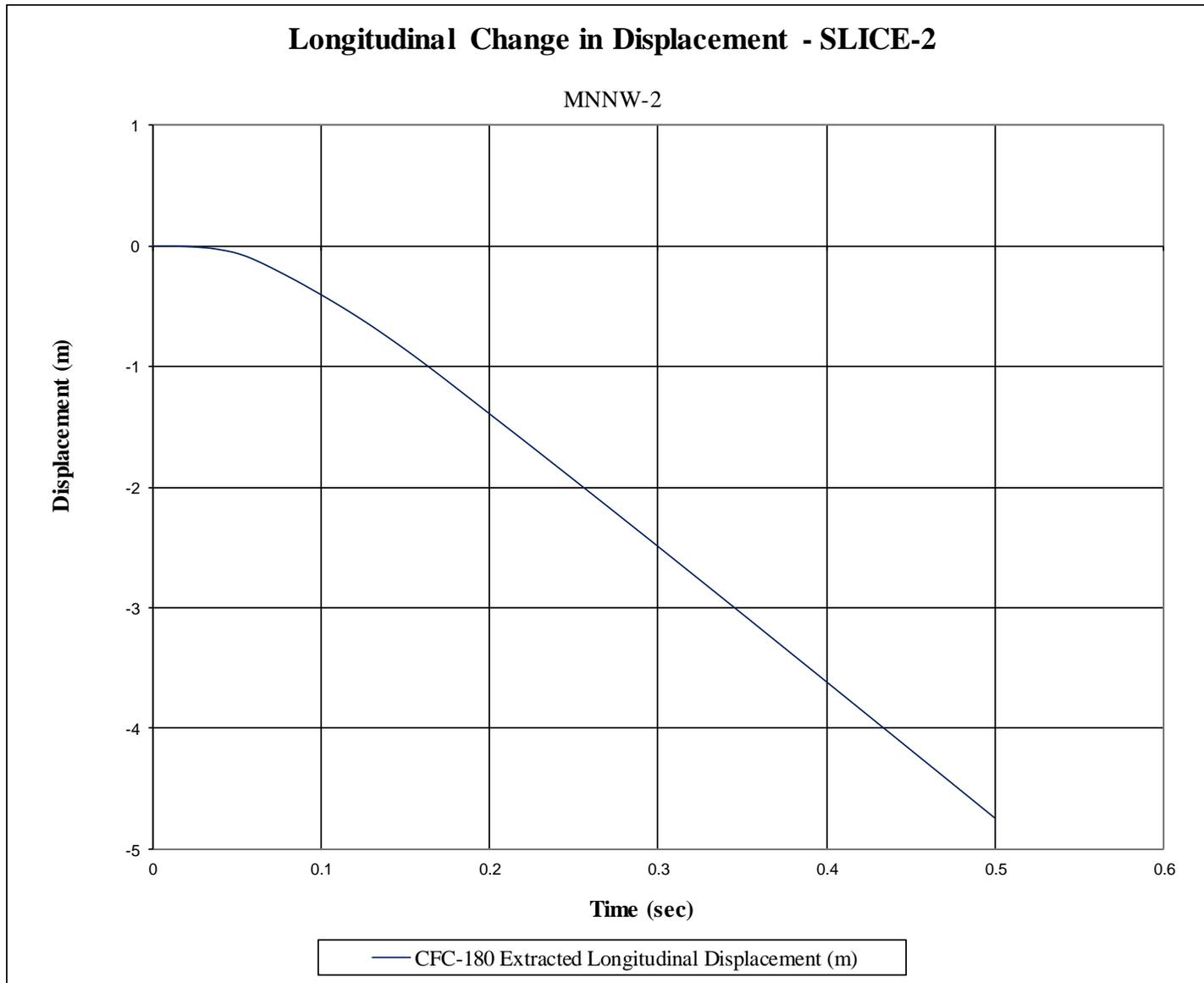
Figure G-11. Longitudinal Occupant Displacement (SLICE-2), Test No. MNNW-2
