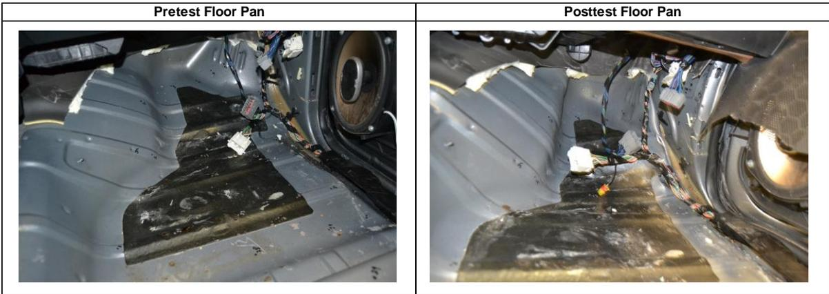
Figure E-14. Floor Pan Deformation Data – Set 2, Test No. MNNW-3
