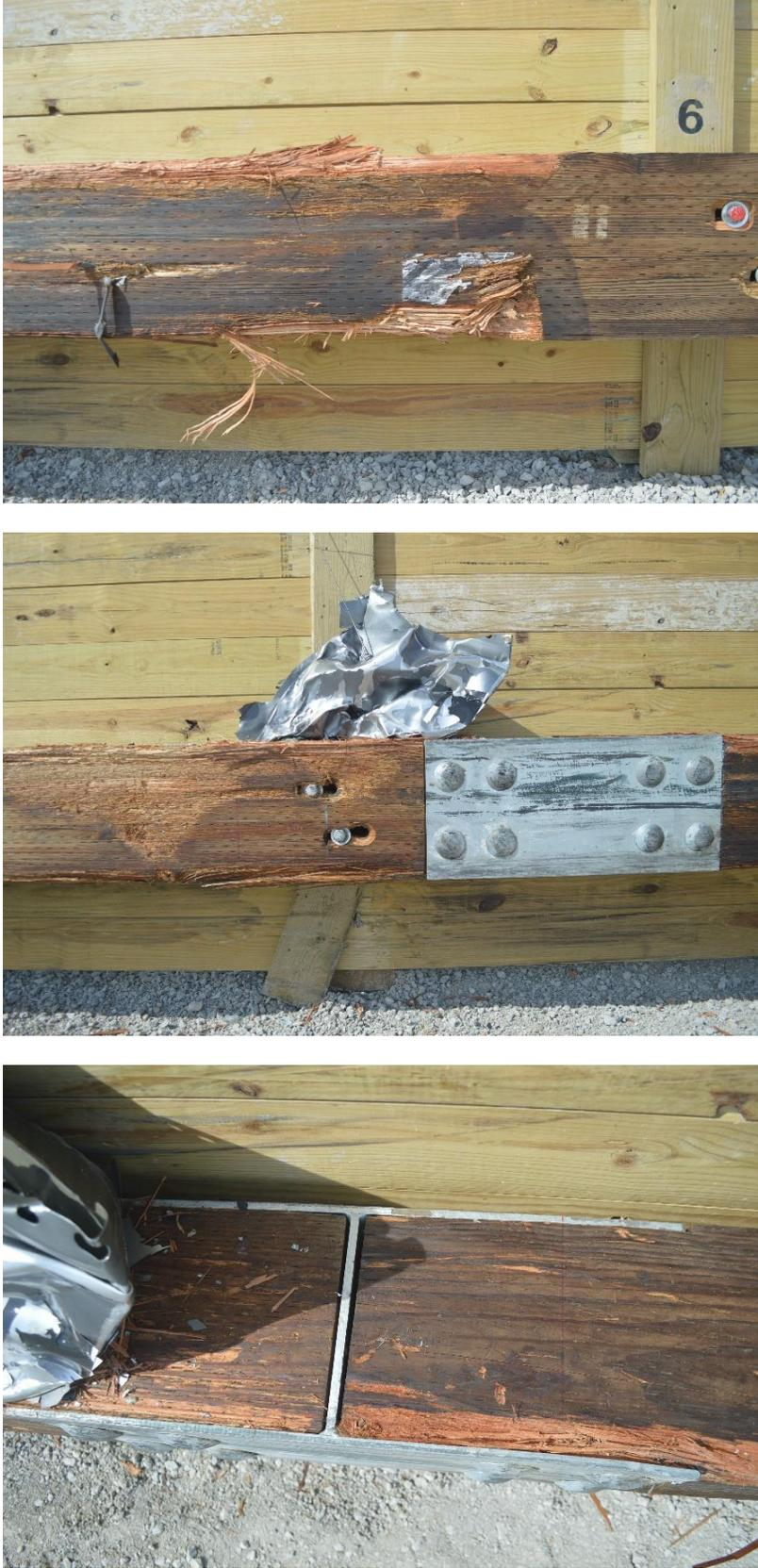
Figure 96. System Damage, Test No. MNNW-3
