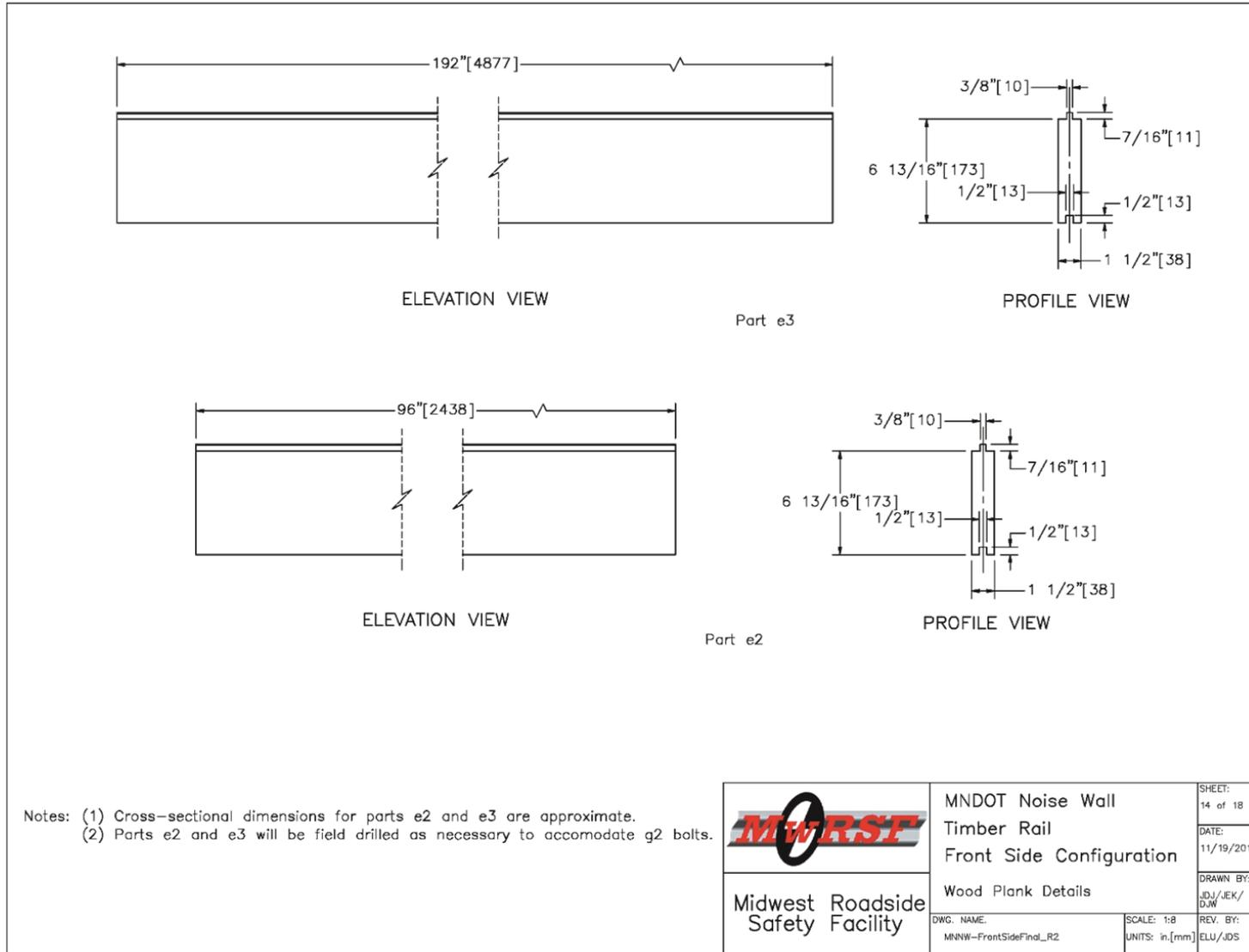
Figure 131. Wood Plank Details, Front-Side Noise Wall
