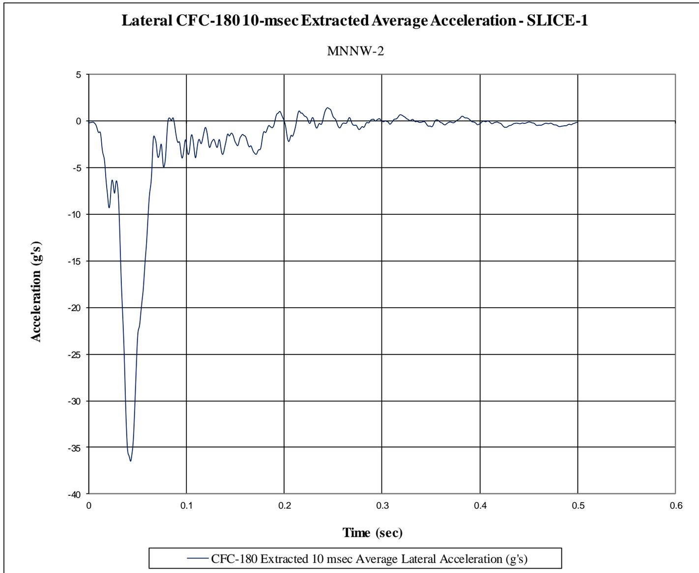
Figure G-4. 10-ms Average Lateral Deceleration (SLICE-1), Test No. MNNW-2
