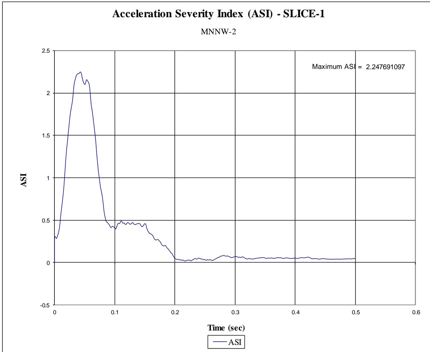
Figure G-8. Acceleration Severity Index (SLICE-1), Test No. MNNW-2
