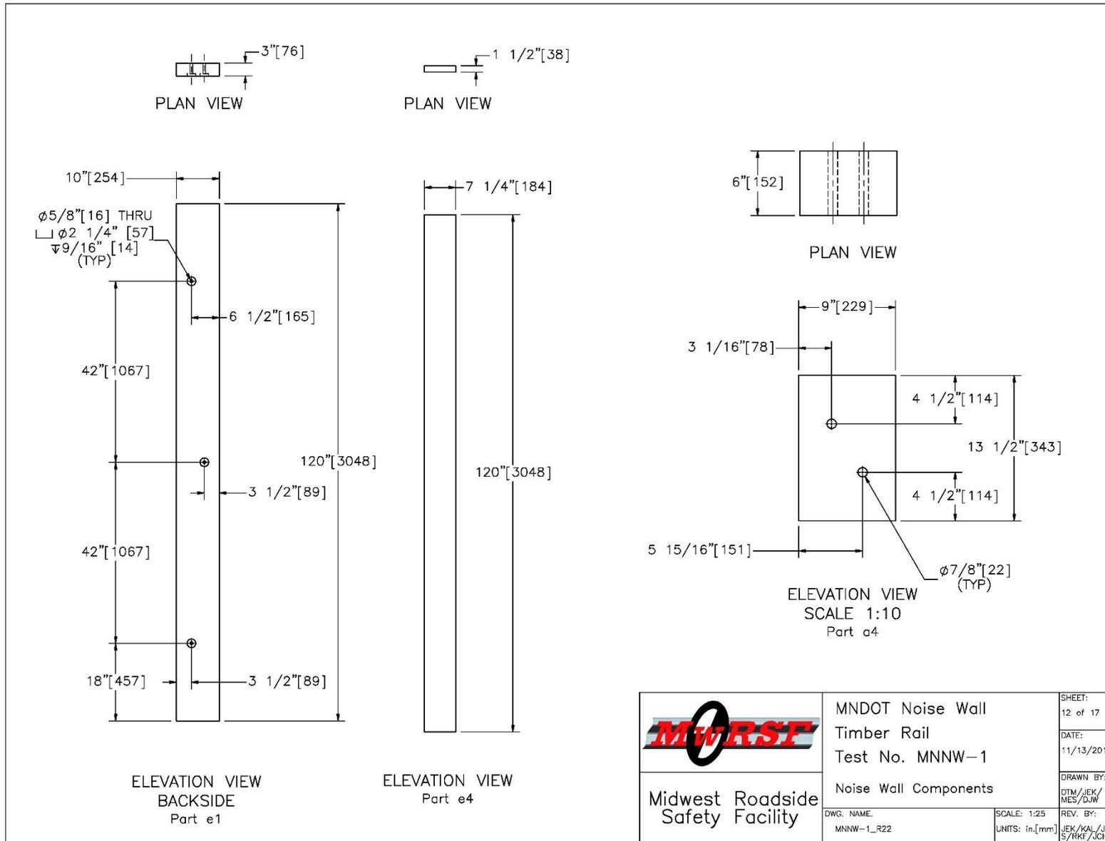
Figure 29. Noise Wall Components, Test Nos. MNNW-1 and MNNW-2 (Recommended updates provided in Chapter 12)
