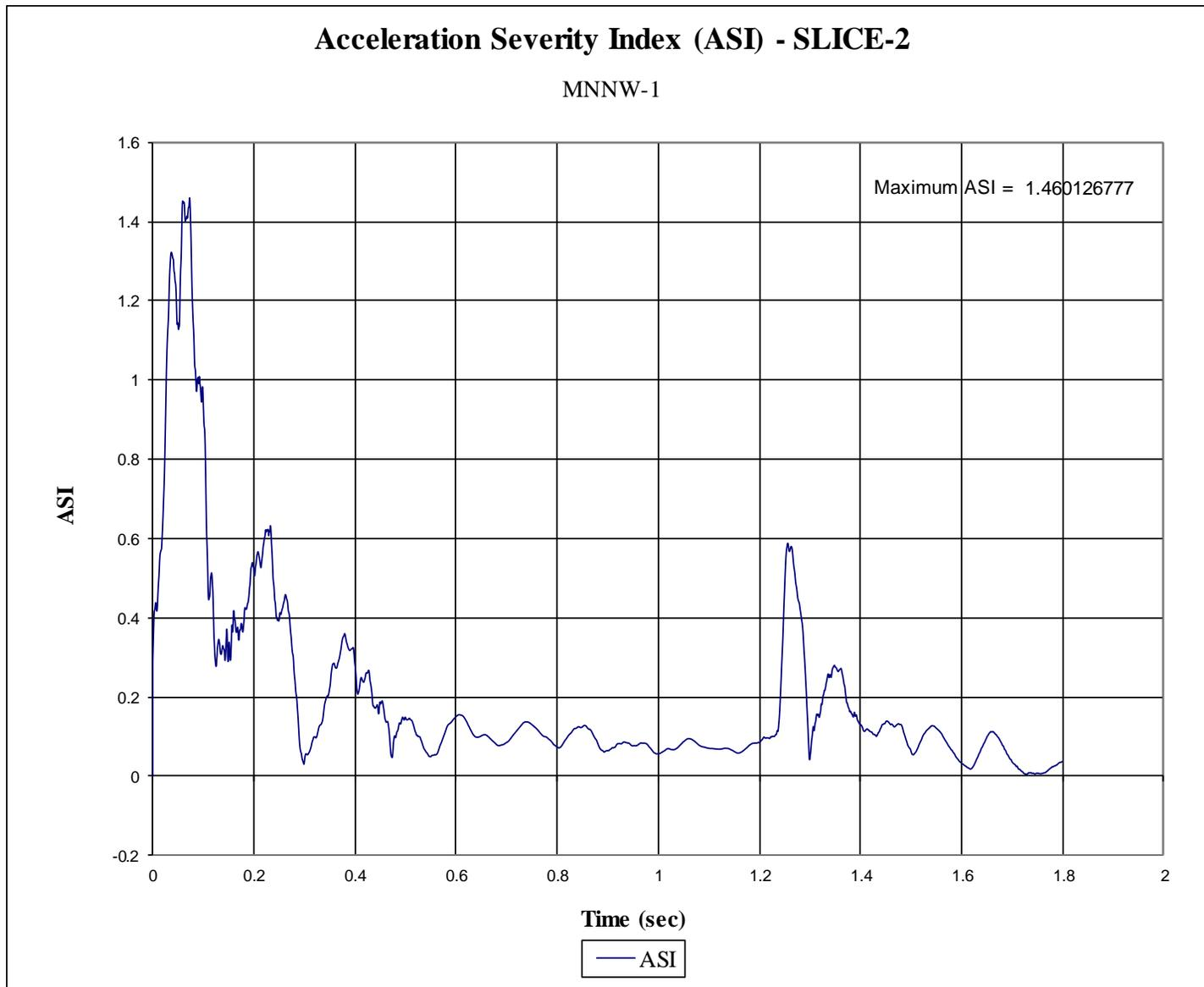
Figure F-16. Acceleration Severity Index (SLICE-2), Test No. MNNW-1
