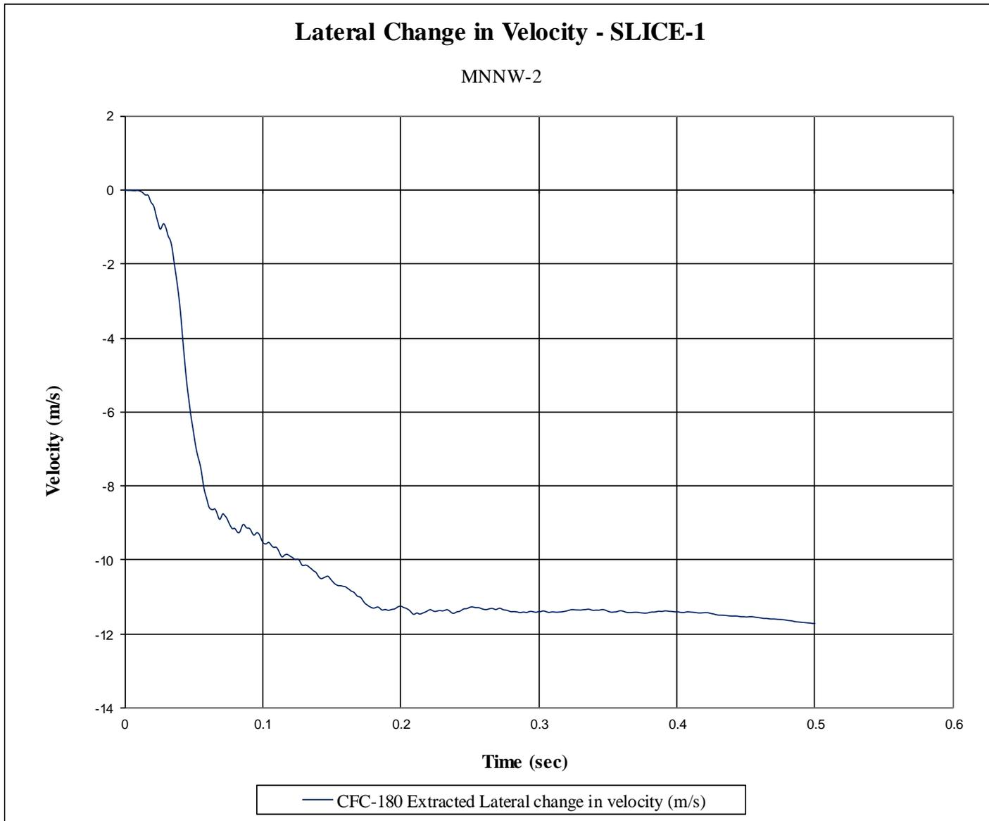
Figure G-5. Lateral Occupant Impact Velocity (SLICE-1), Test No. MNNW-2
