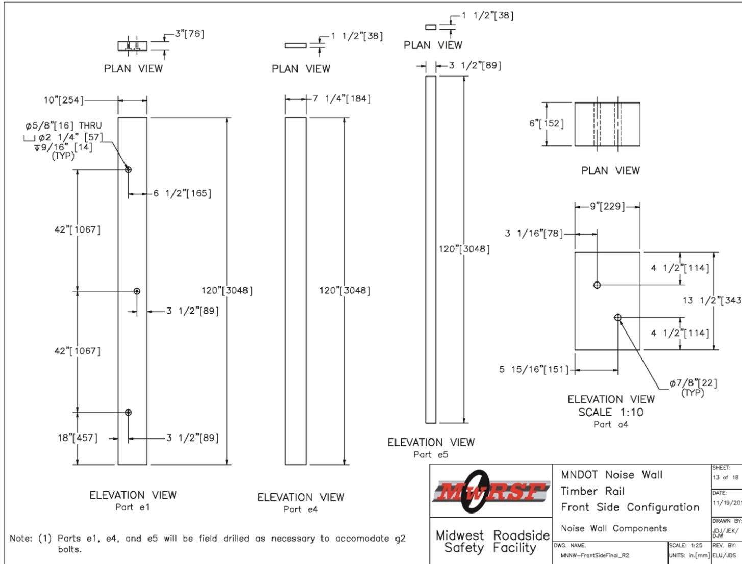
Figure 130. Noise Wall Components, Front-Side Noise Wall
