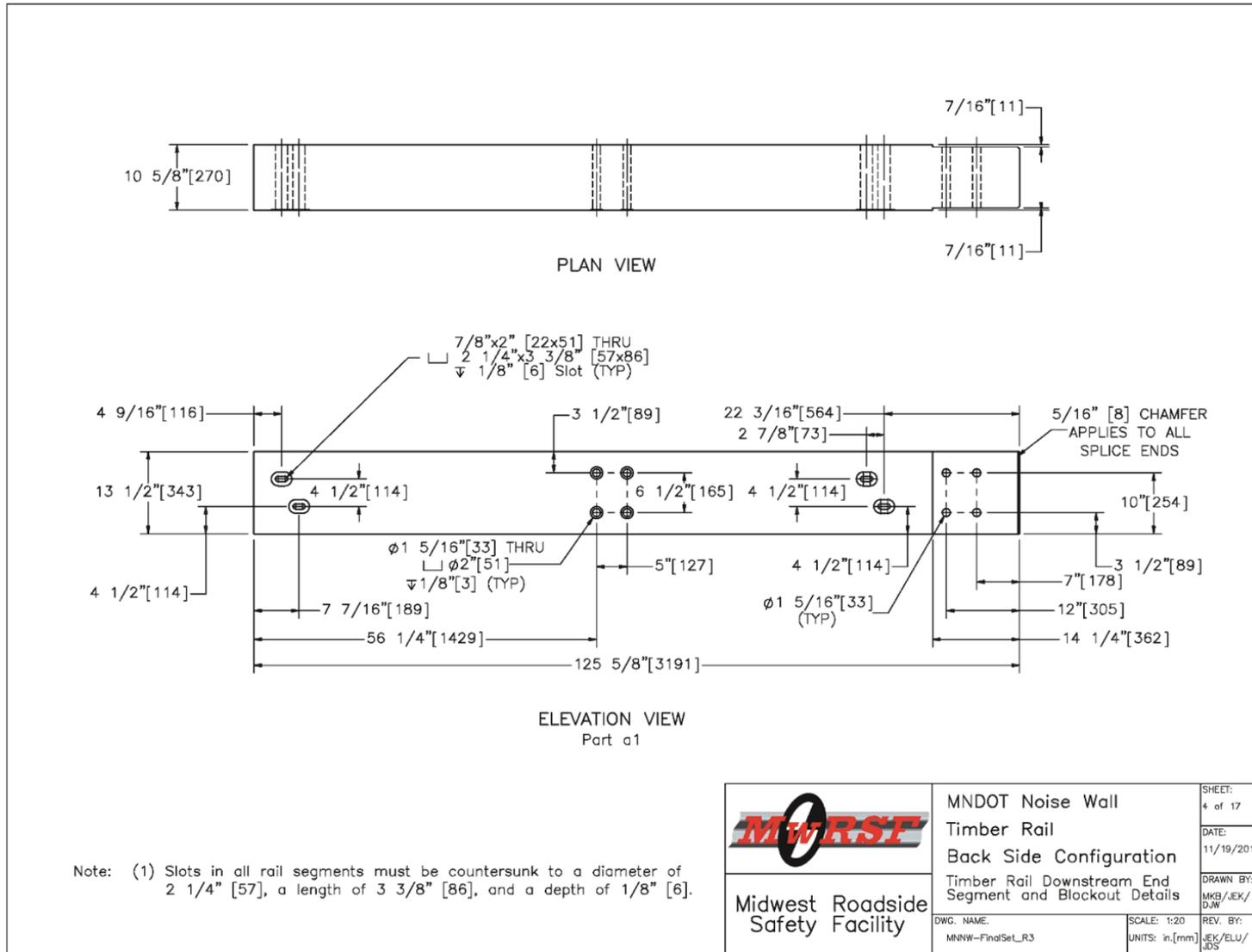
Figure 104. Timber Rail Downstream End Segment and Blockout Details, Back-Side Noise Wall
