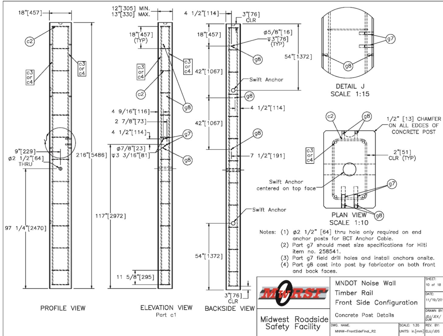
Figure 127. Concrete Post Details, Front-Side Noise Wall
