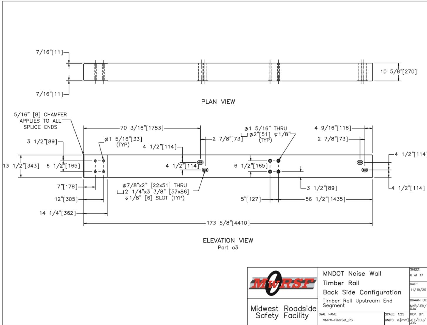
Figure 106. Timber Rail Upstream End Segment, Back-Side Noise Wall
