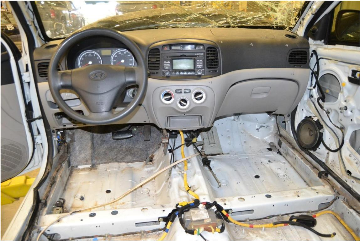
Figure 63. Vehicle Undercarriage and Occupant Compartment Damage, Test No. MNNW-2
