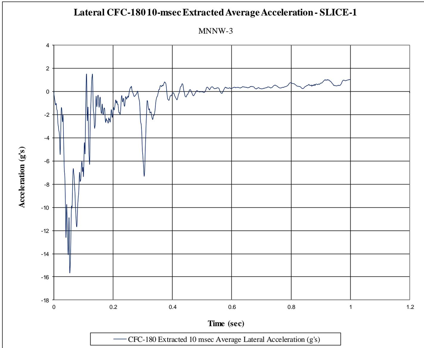
Figure H-4. 10-ms Average Lateral Deceleration (SLICE-1), Test No. MNNW-3
