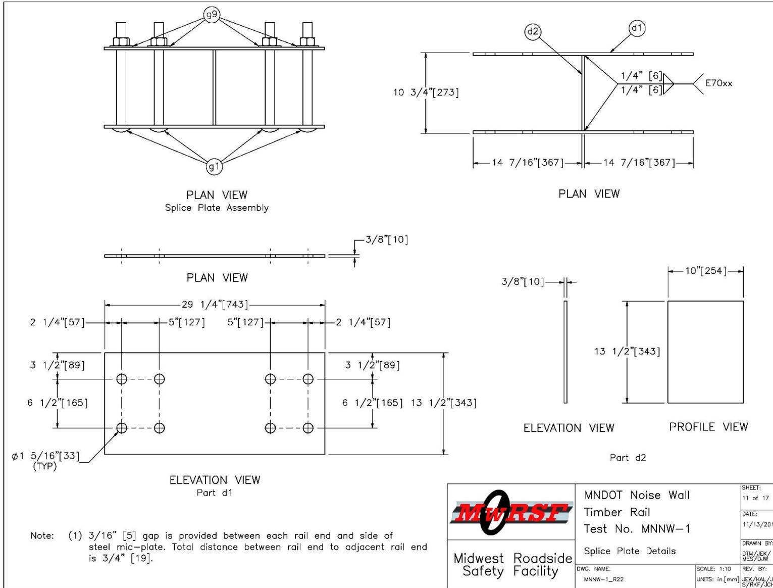
Figure 28. Splice Plate Details, Test Nos. MNNW-1 and MNNW-2 (Recommended updates provided in Chapter 12)
