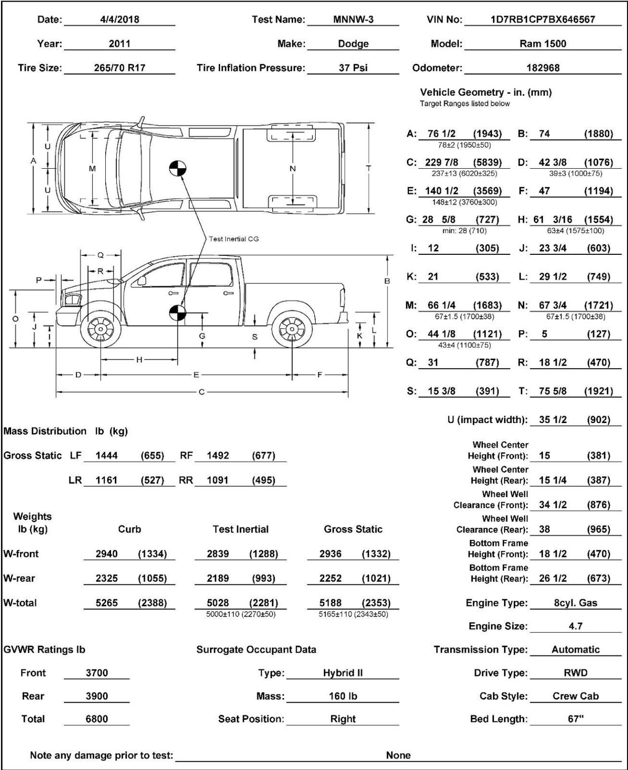
Figure 10. Vehicle Dimensions, Test No. MNNW-3
