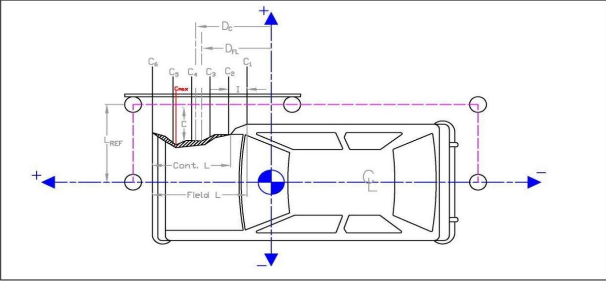
Distance from centerline to reference line -  $L_{REF}$ : 43 in. (1092) mm
