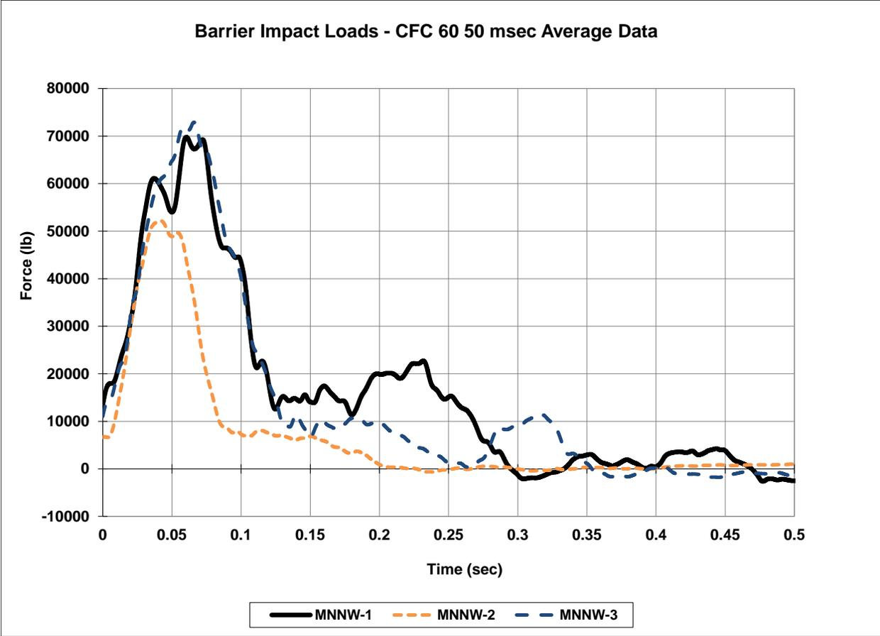
Figure 100. Estimated Lateral Barrier Loads, Test Nos. MNNW-1 through MNNW-3
