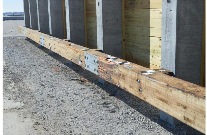
Figure 61. System Damage, Test No. MNNW-2
