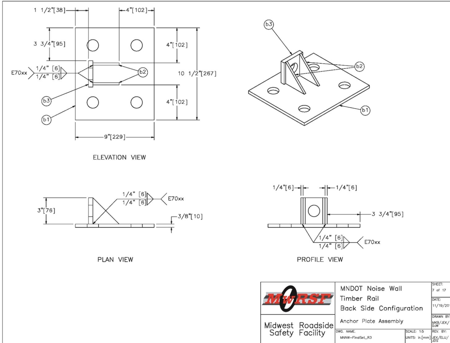
Figure 107. Anchor Plate Assembly, Back-Side Noise Wall
