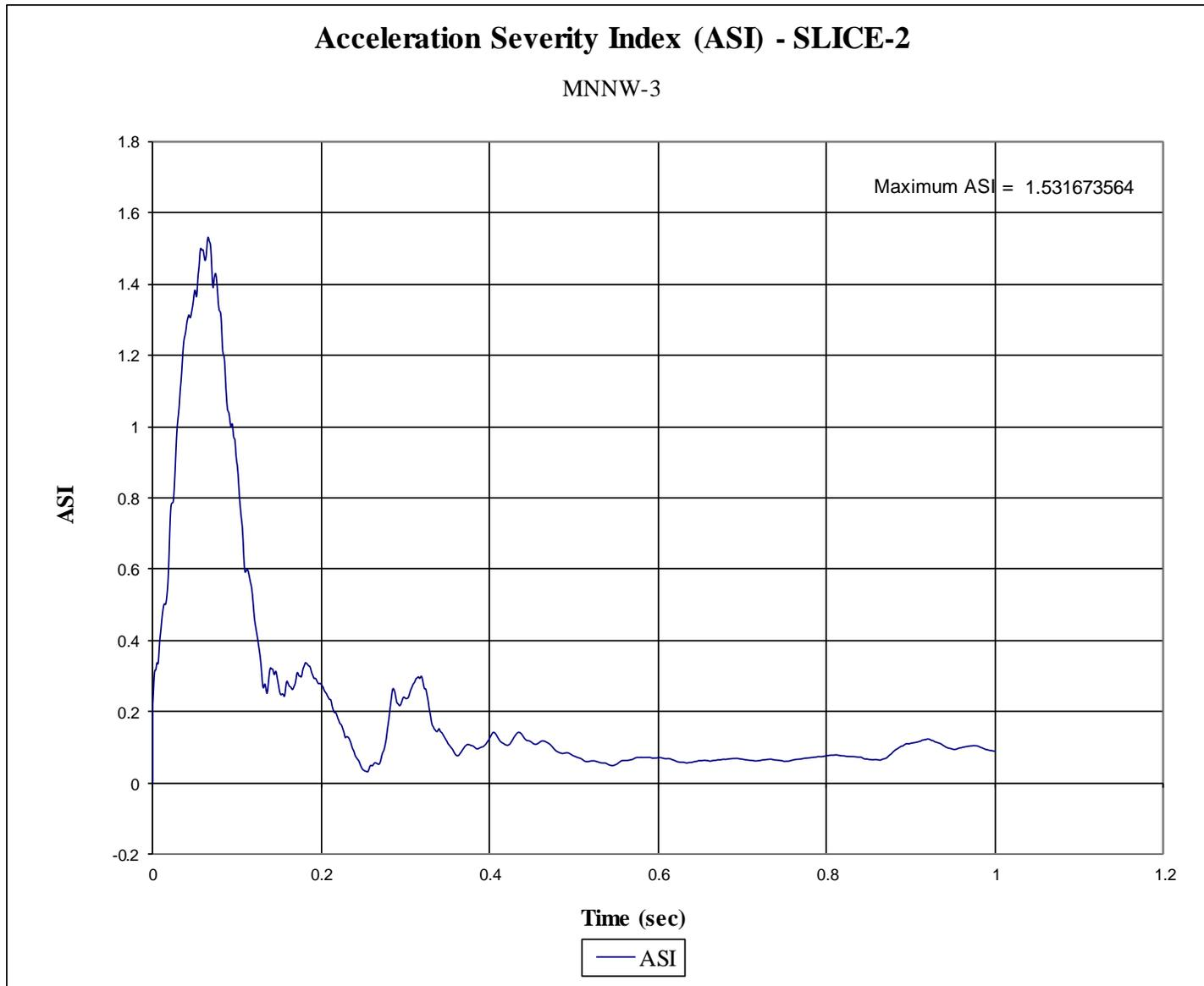
Figure H-16. Acceleration Severity Index (SLICE-2), Test No. MNNW-3
