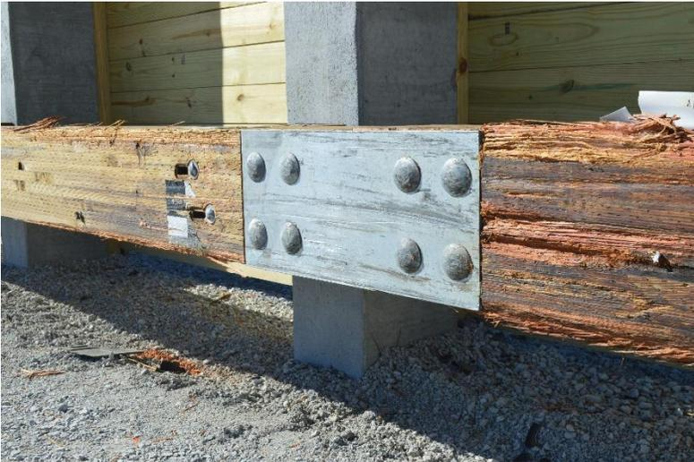
Figure 62. System Damage, Test No. MNNW-2
