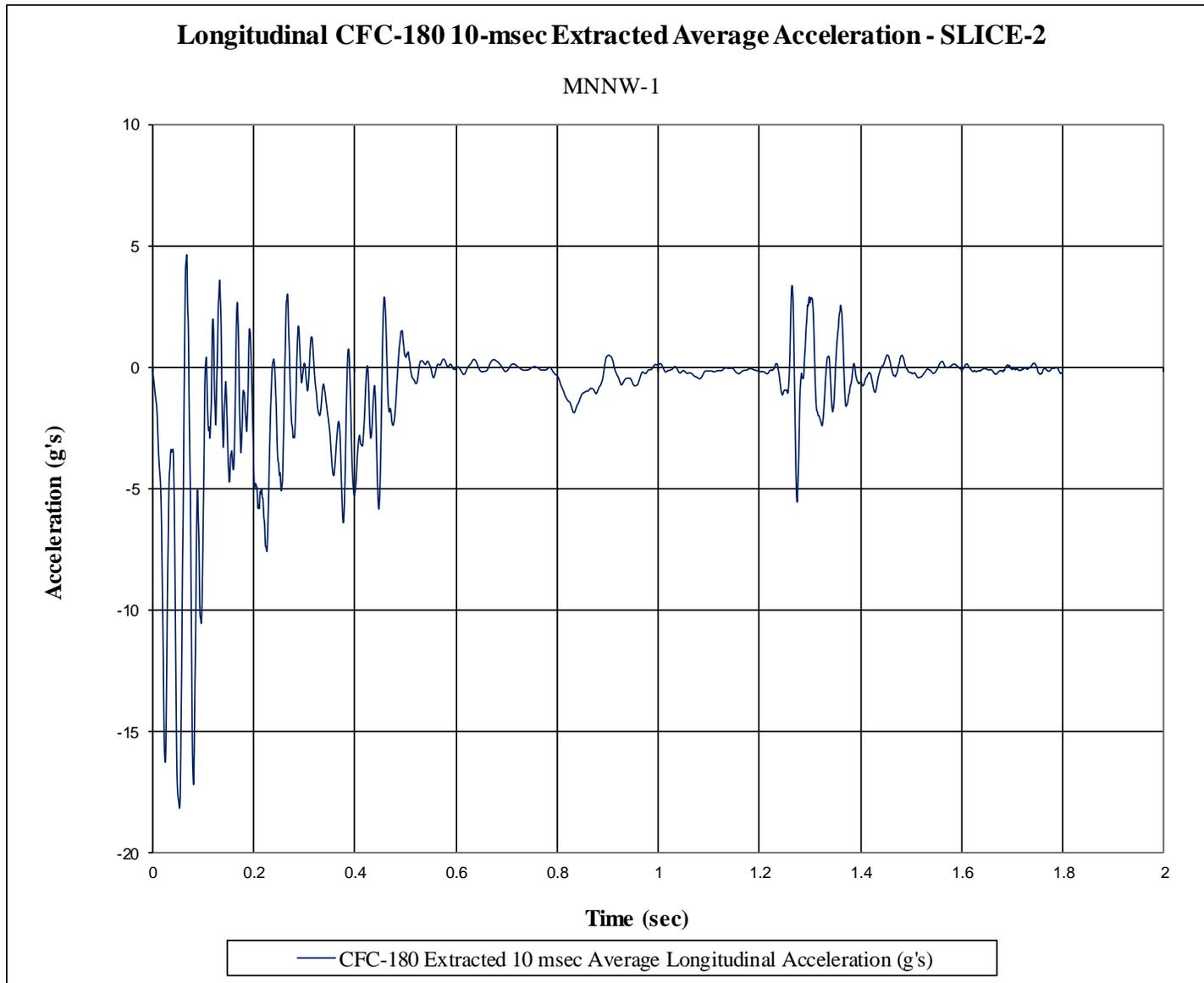
Figure F-9. 10-ms Average Longitudinal Deceleration (SLICE-2), Test No. MNNW-1
