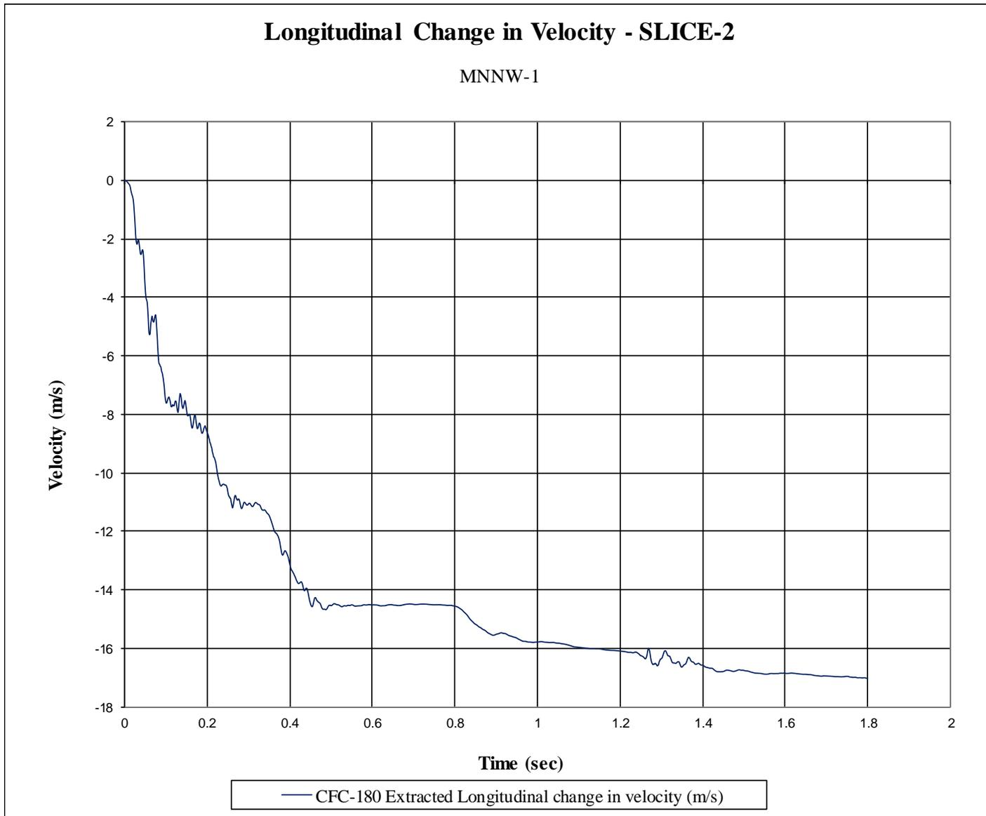
Figure F-10. Longitudinal Occupant Impact Velocity (SLICE-2), Test No. MNNW-1
