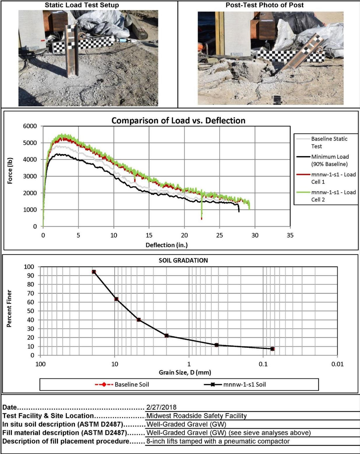
Figure D-2. Static Soil Test, Test No. MNNW-1
