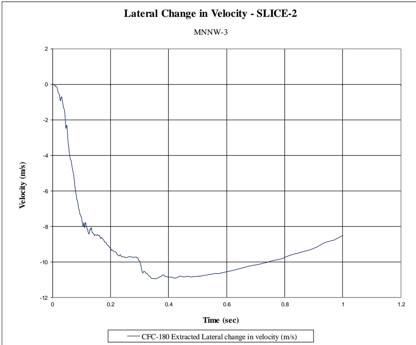
Figure H-13. Lateral Occupant Impact Velocity (SLICE-2), Test No. MNNW-3
