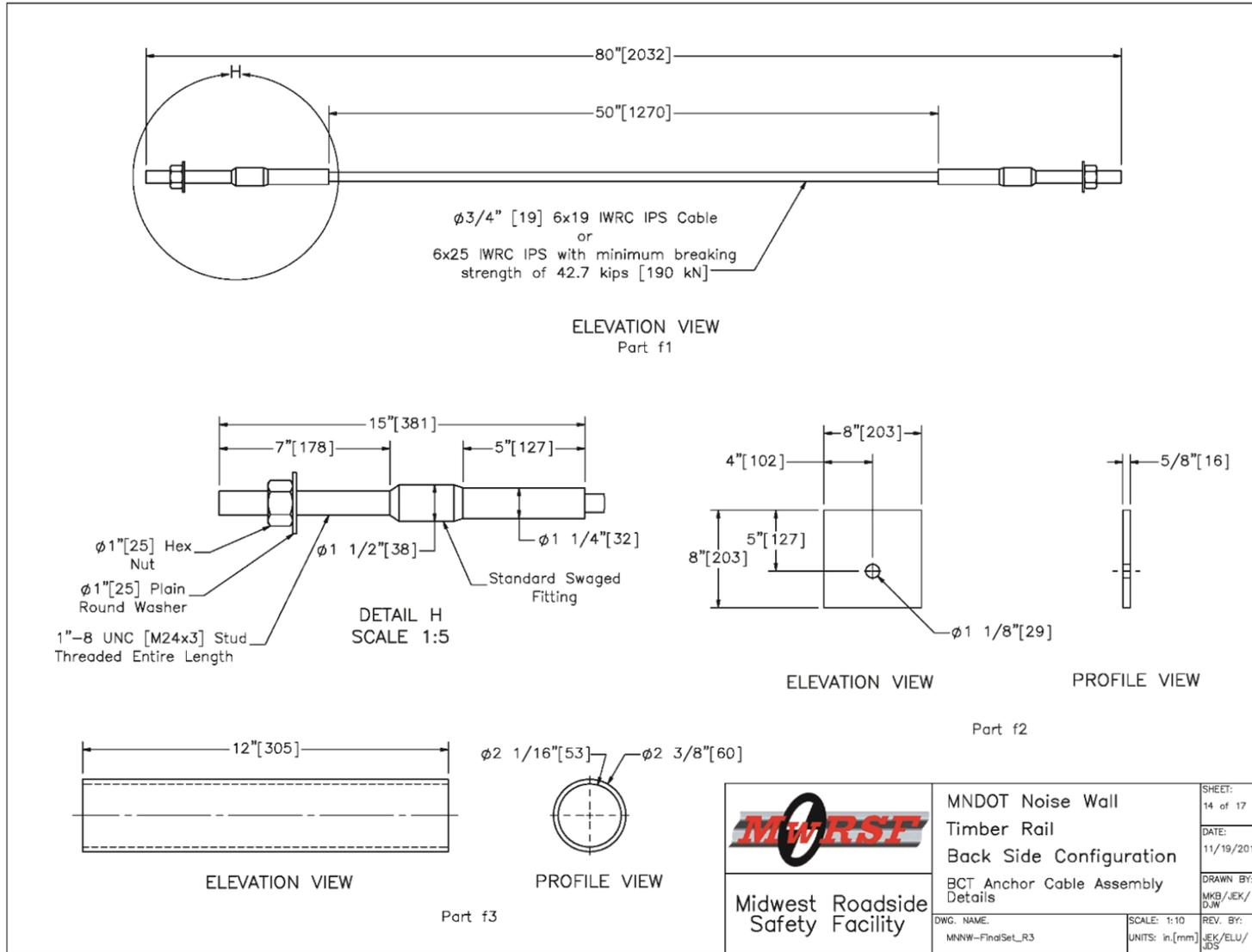
Figure 114. BCT Anchor Cable Assembly Details, Back-Side Noise Wall
