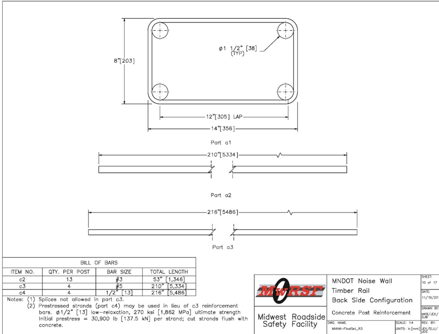
Figure 110. Concrete Post Reinforcement, Back-Side Noise Wall
