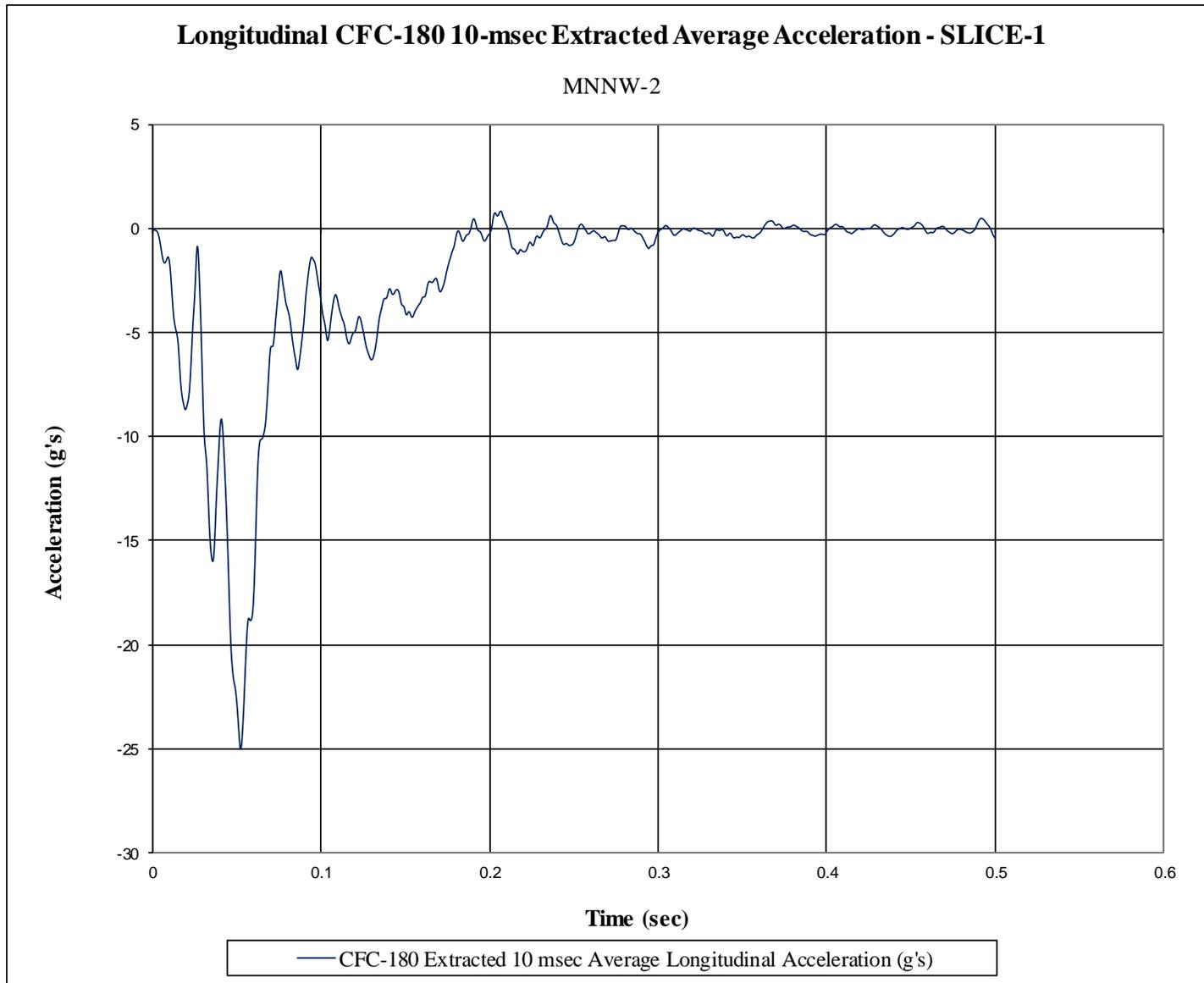
Figure G-1. 10-ms Average Longitudinal Deceleration (SLICE-1), Test No. MNNW-2
