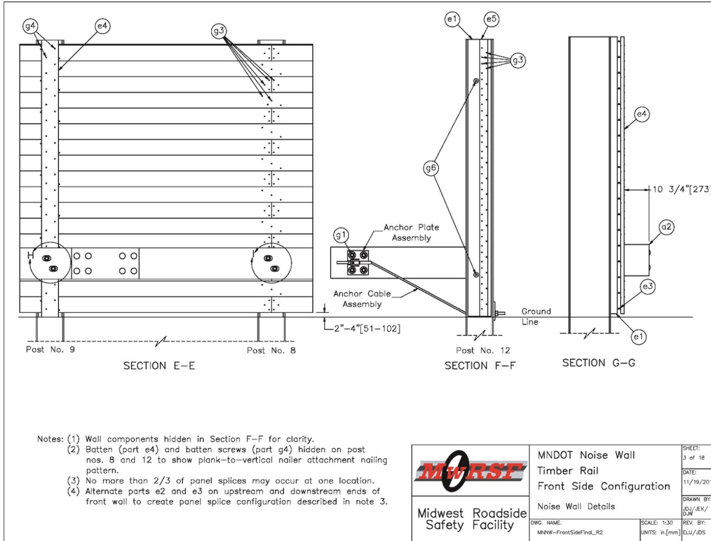
Figure 120. Noise Wall Details, Front-Side Noise Wall
