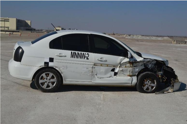
Figure 65. Vehicle Damage, Test No. MNNW-2
