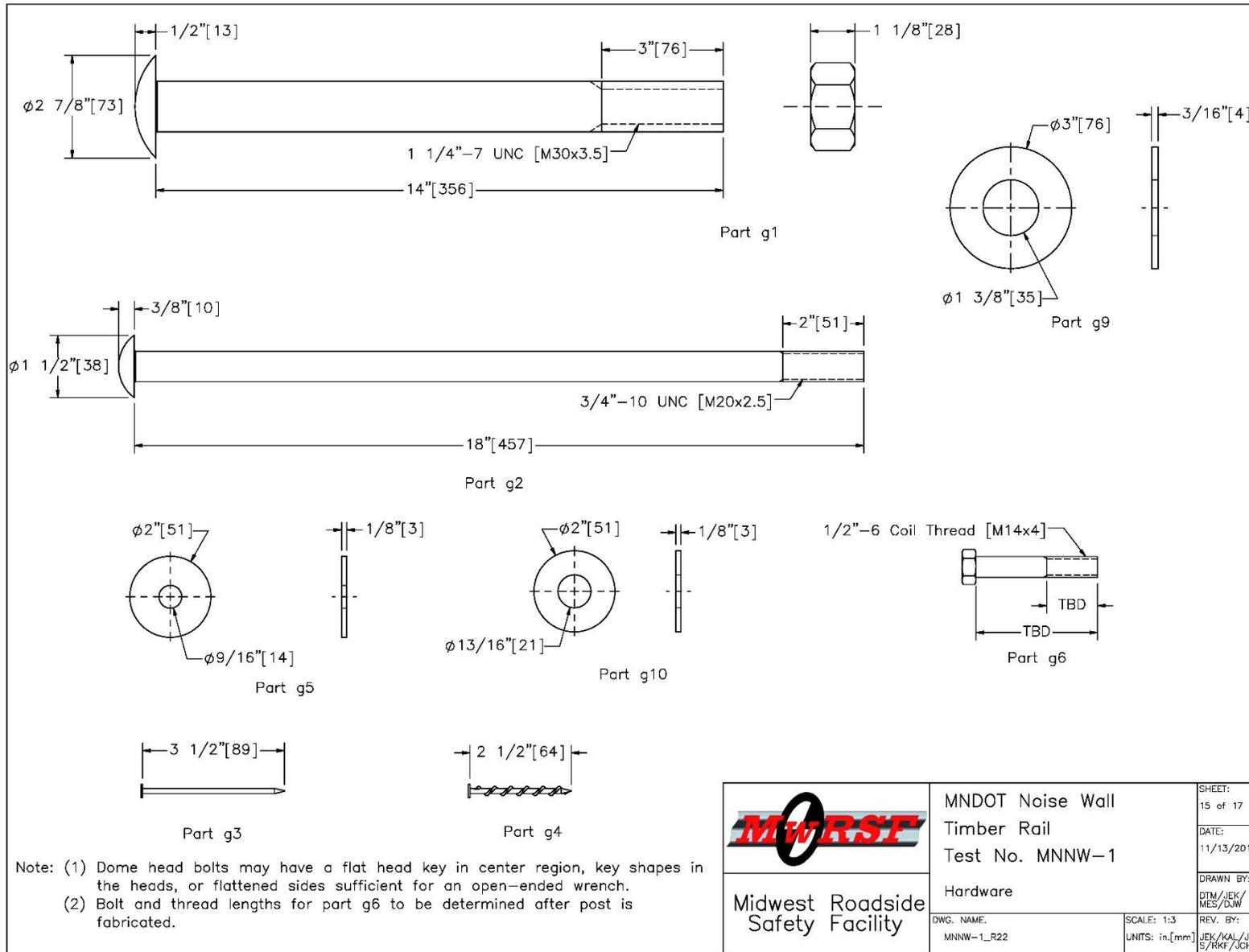
Figure 32. Hardware, Test Nos. MNNW-1 and MNNW-2 (Recommended updates provided in Chapter 12)
