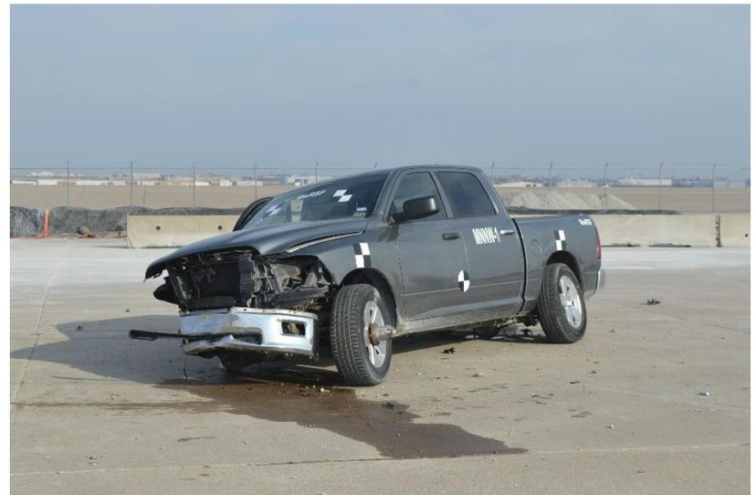
Figure 51. Vehicle Damage, Test No. MNNW-1
