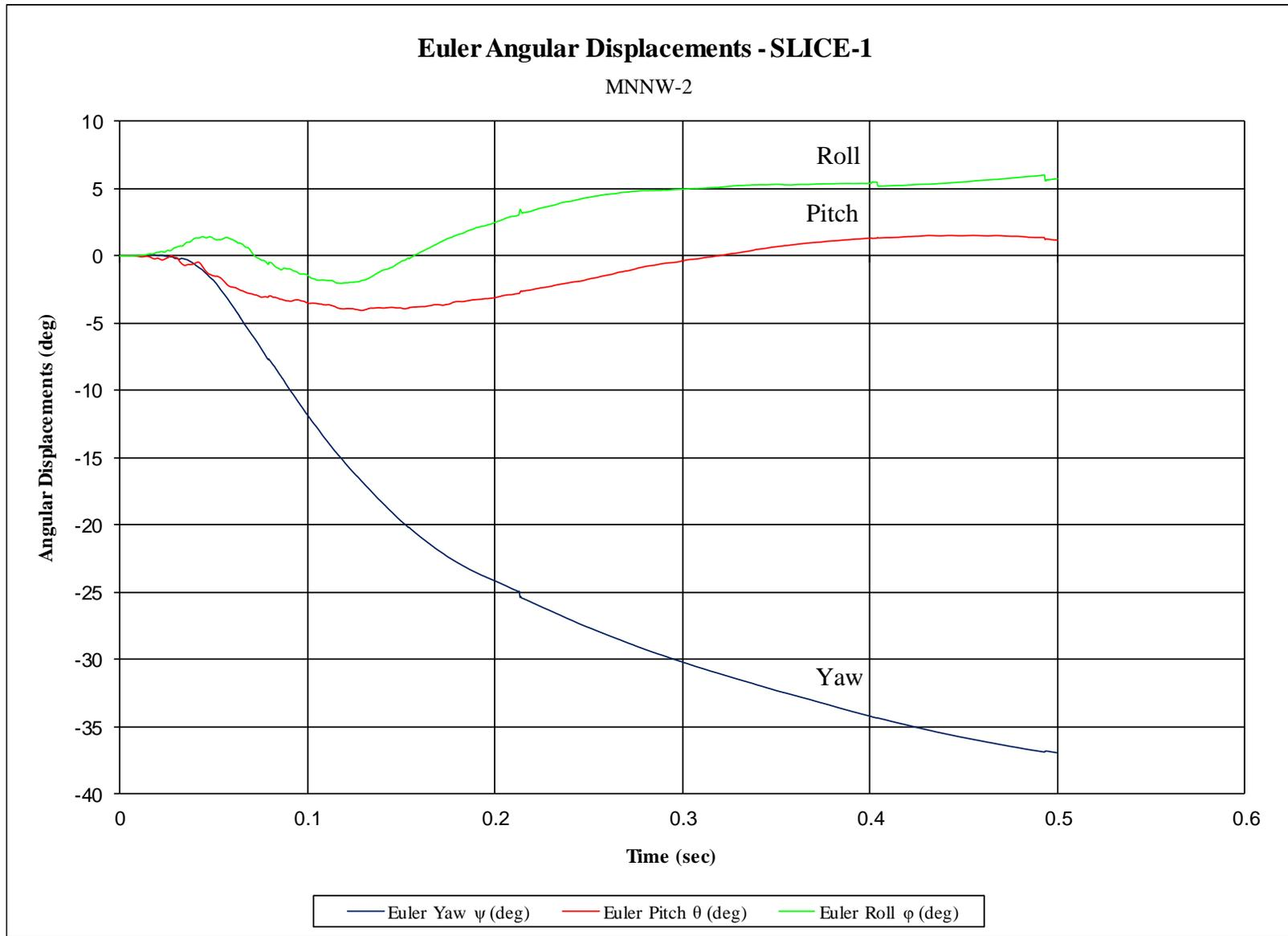
Figure G-7. Vehicle Angular Displacements (SLICE-1), Test No. MNNW-2
