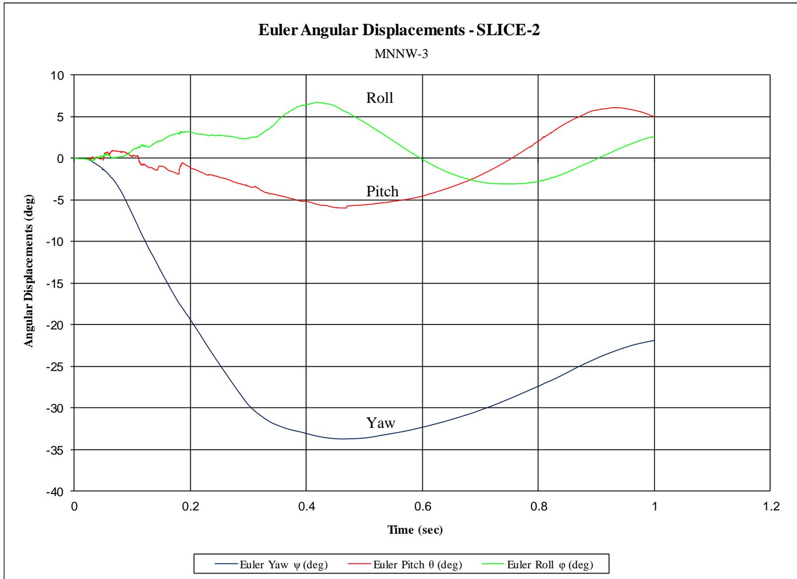
Figure H-15. Vehicle Angular Displacements (SLICE-2), Test No. MNNW-3
