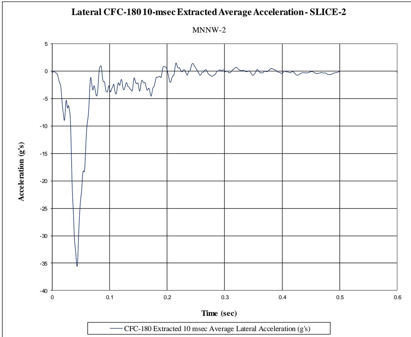
Figure G-12. 10-ms Average Lateral Deceleration (SLICE-2), Test No. MNNW-2
