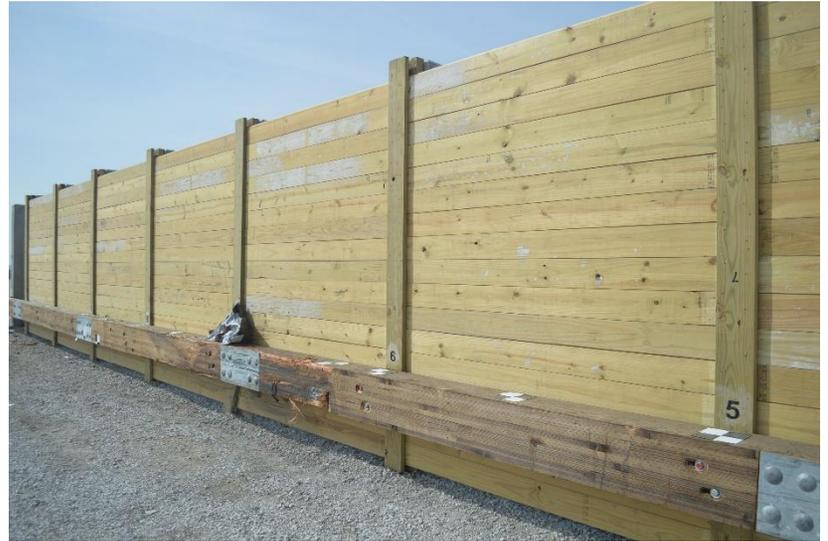
Figure 95. System Damage, Test No. MNNW-3
