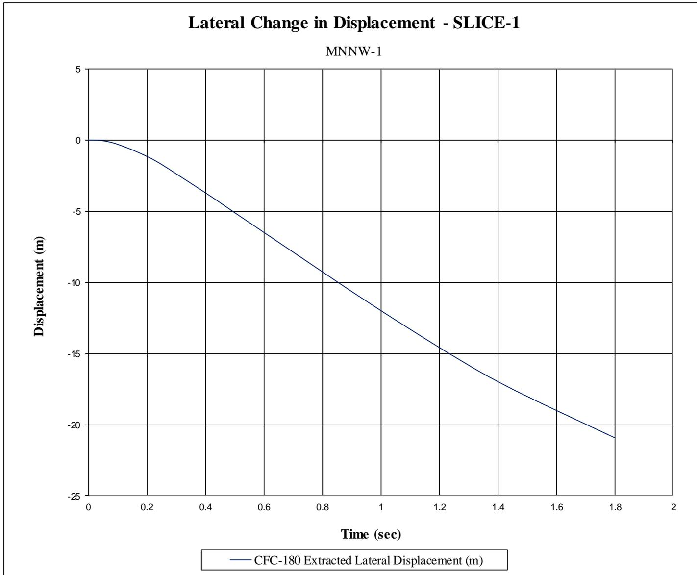
Figure F-6. Lateral Occupant Displacement (SLICE-1), Test No. MNNW-1
