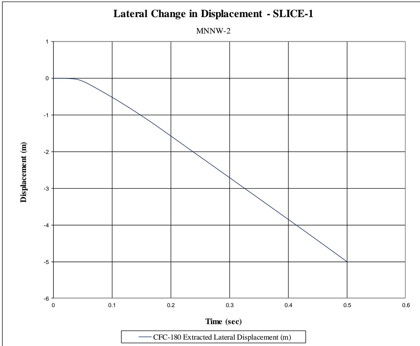
Figure G-6. Lateral Occupant Displacement (SLICE-1), Test No. MNNW-2
