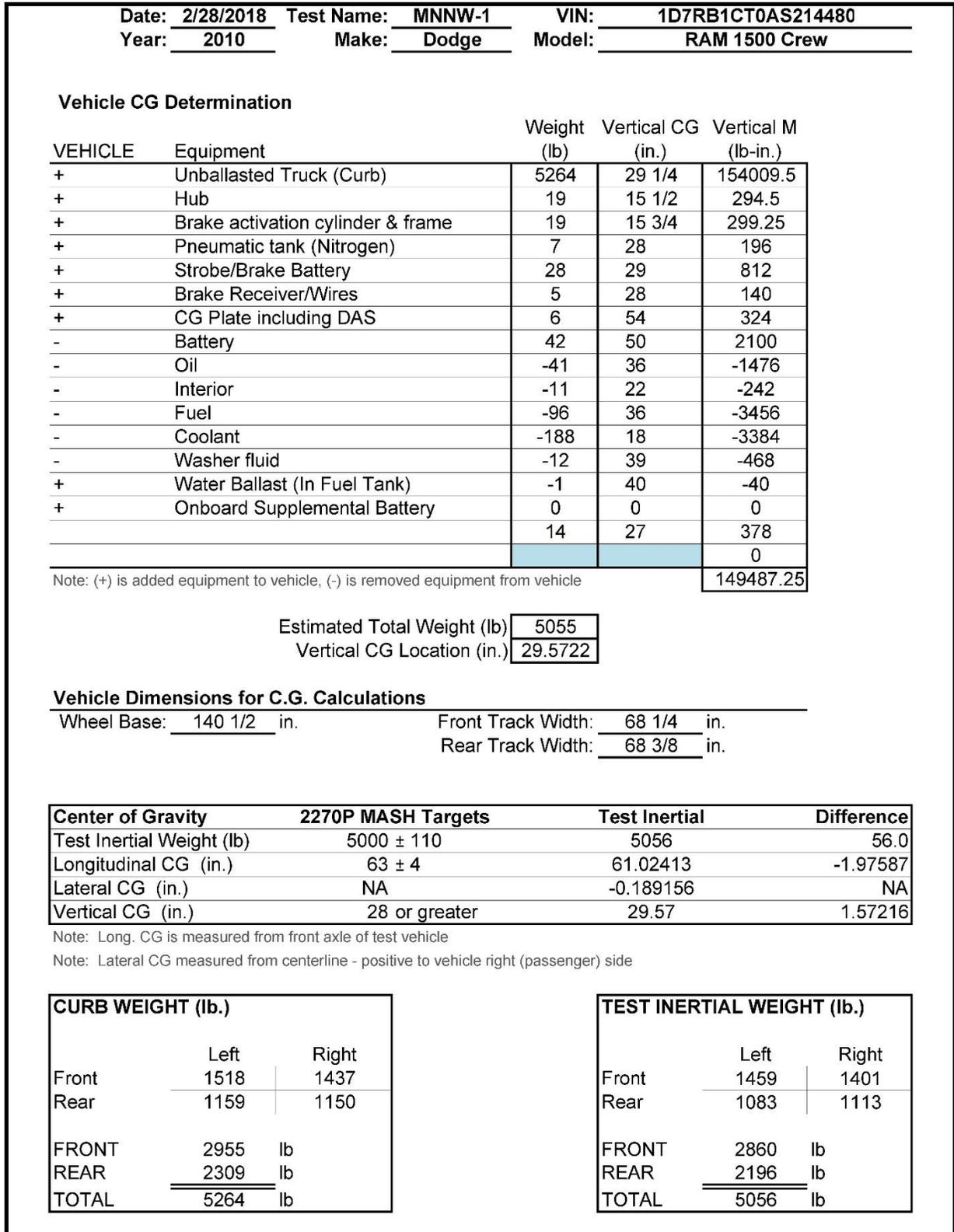
Figure B-1. Vehicle Mass Distribution, Test No. MNNW-1
