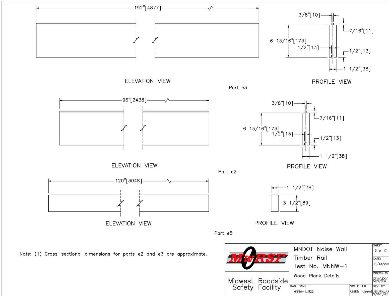
Figure 30. Wood Plank Details, Test Nos. MNNW-1 and MNNW-2 (Recommended updates provided in Chapter 12)
