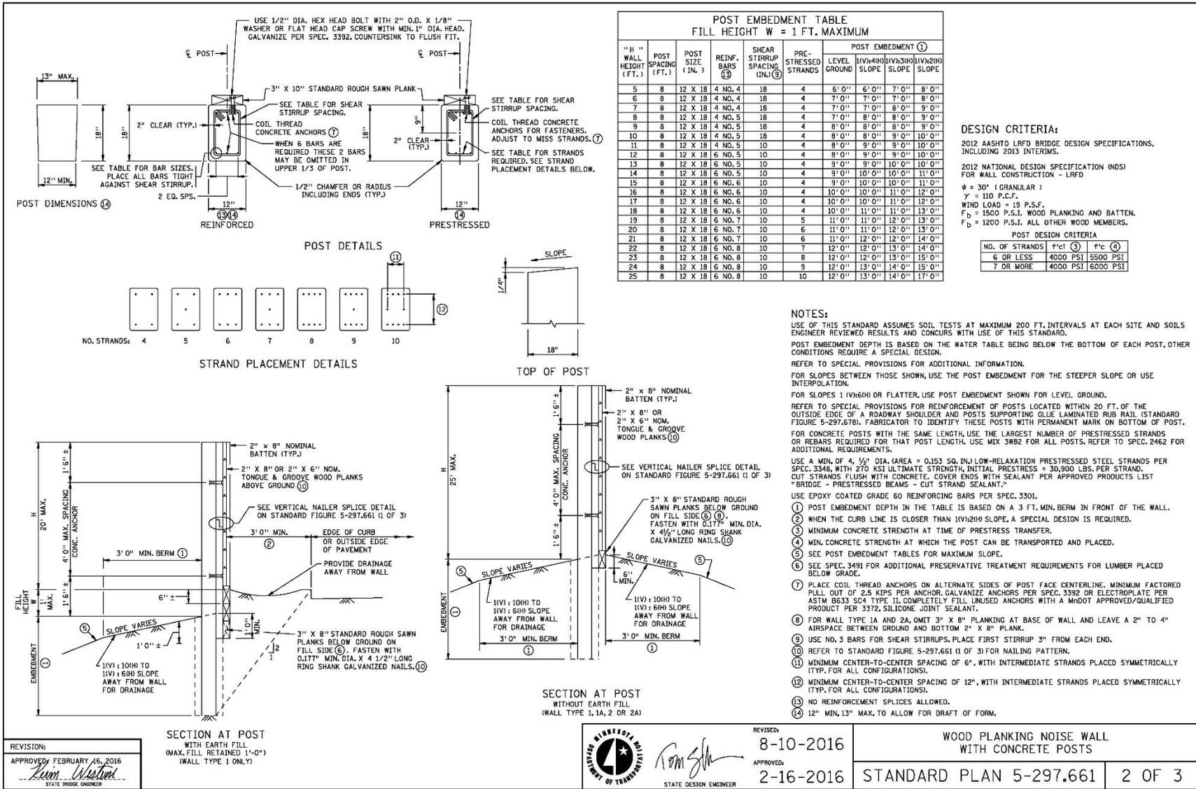
Figure A-2. Wood Planking Noise Wall with Concrete Posts
