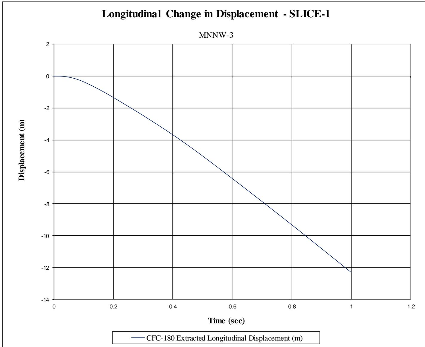
Figure H-3. Longitudinal Occupant Displacement (SLICE-1), Test No. MNNW-3
