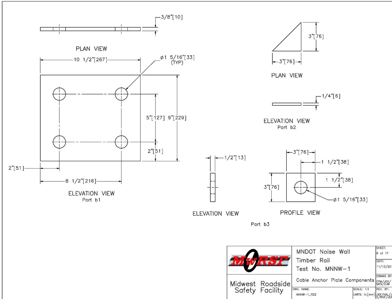
Figure 25. Cable Anchor Plate Components, Test Nos. MNNW-1 and MNNW-2 (Recommended updates provided in Chapter 12)
