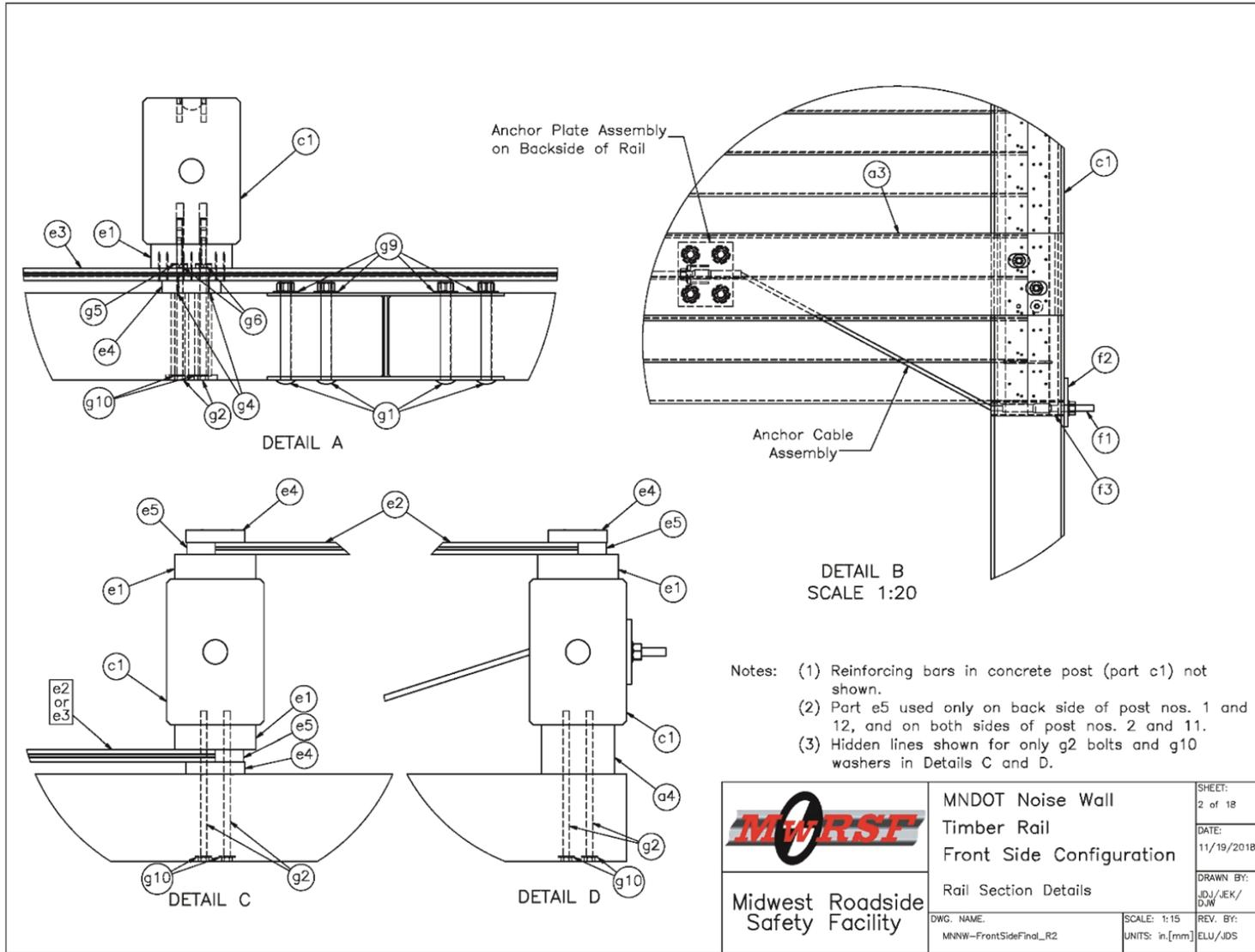
Figure 119. Rail Section Details, Front-Side Noise Wall
