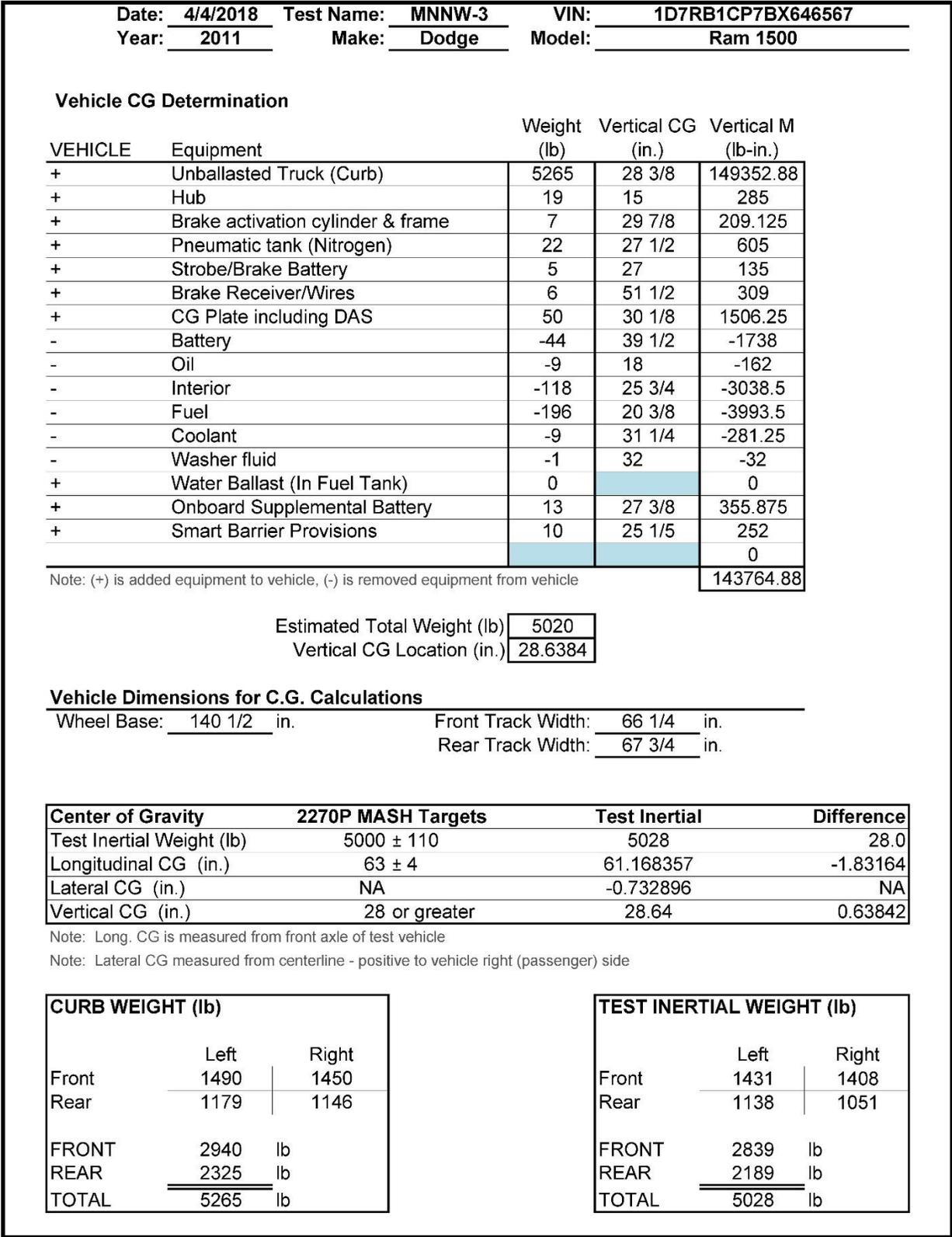
Figure B-3. Vehicle Mass Distribution, Test No. MNNW-3
