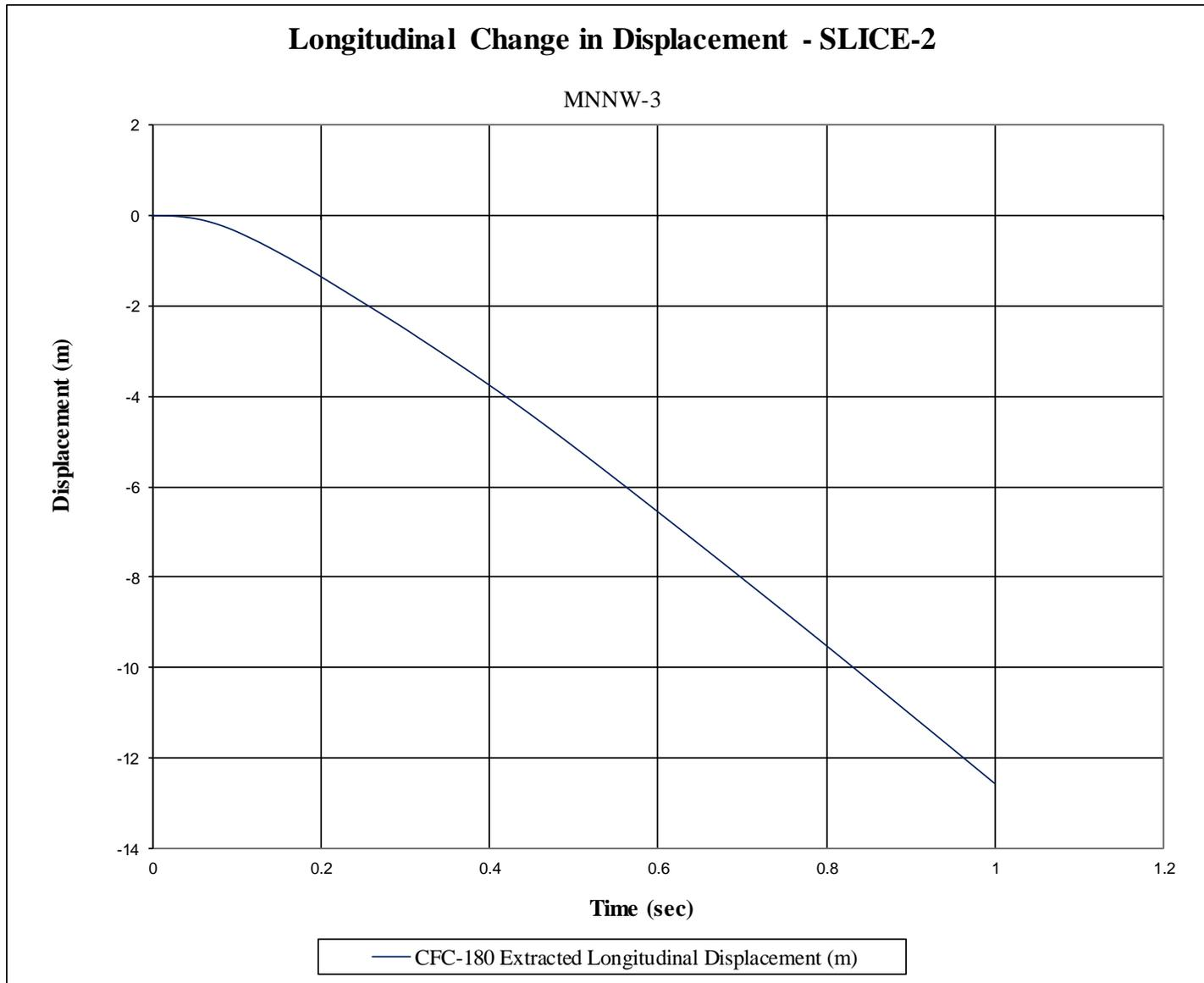
Figure H-11. Longitudinal Occupant Displacement (SLICE-2), Test No. MNNW-3
