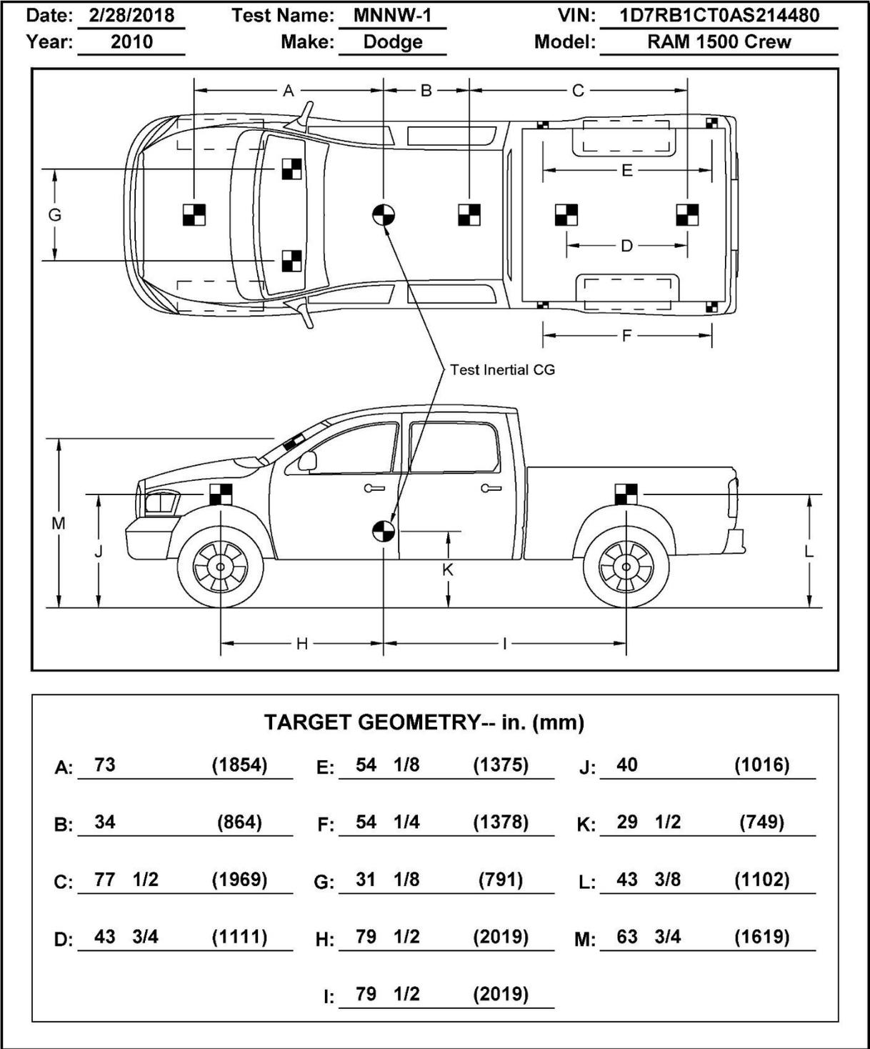
Figure 11. Target Geometry, Test No. MNNW-1
