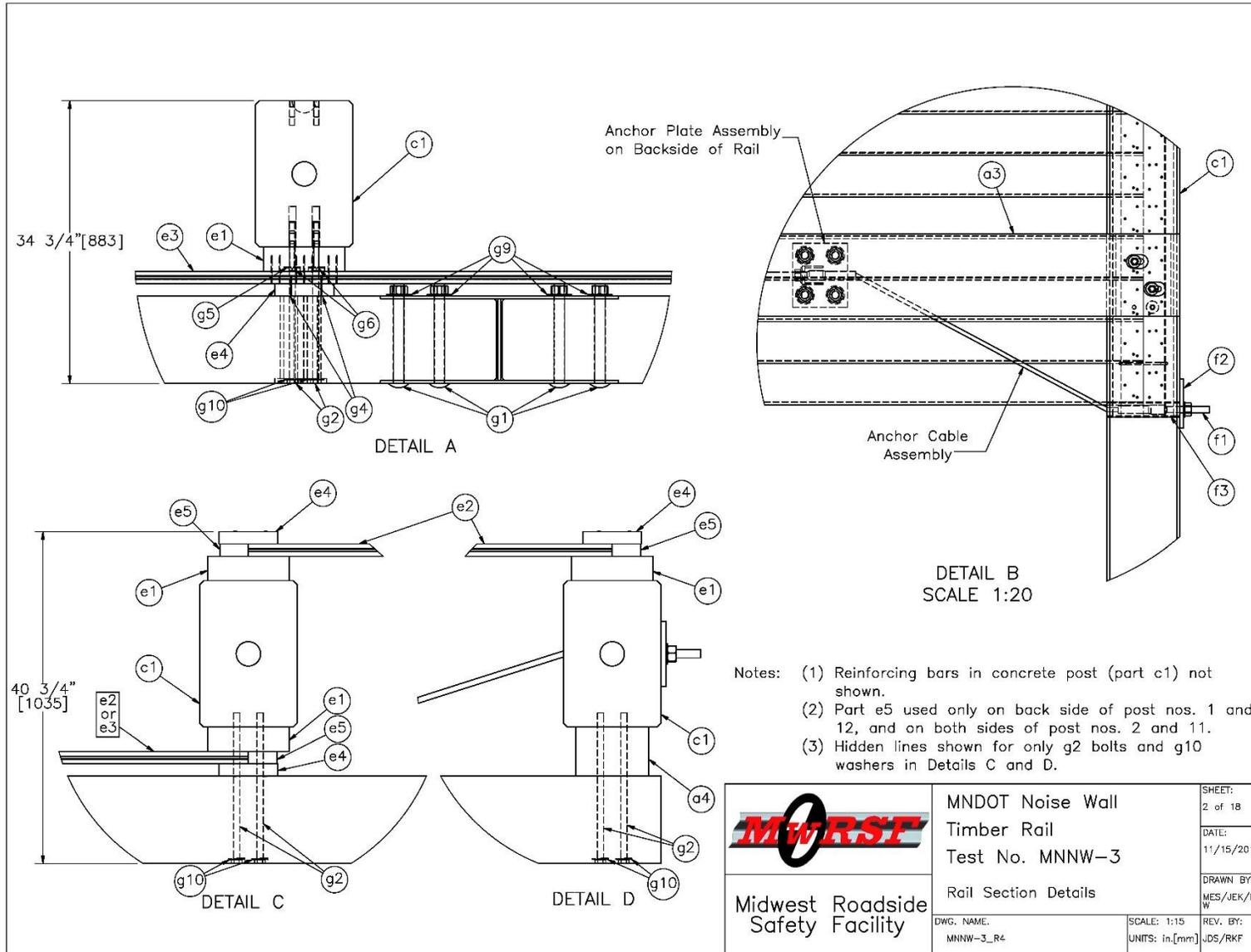
Figure 67. Rail Section Details, Test No. MNNW-3 (Recommended updates provided in Chapter 12)
