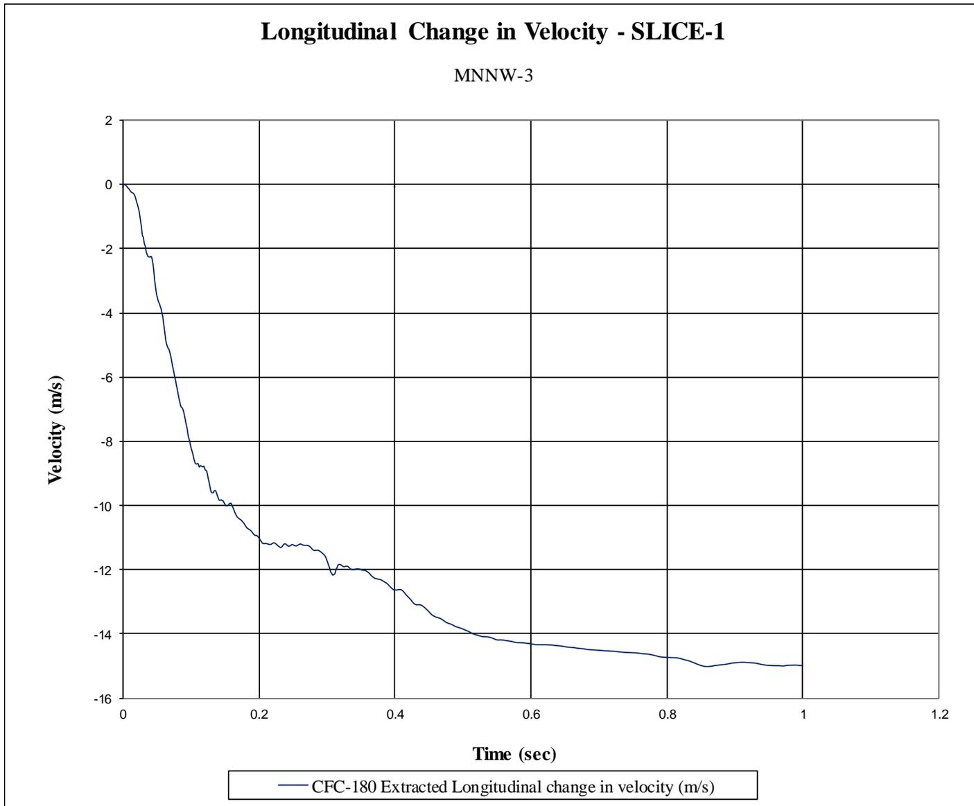
Figure H-2. Longitudinal Occupant Impact Velocity (SLICE-1), Test No. MNNW-3
