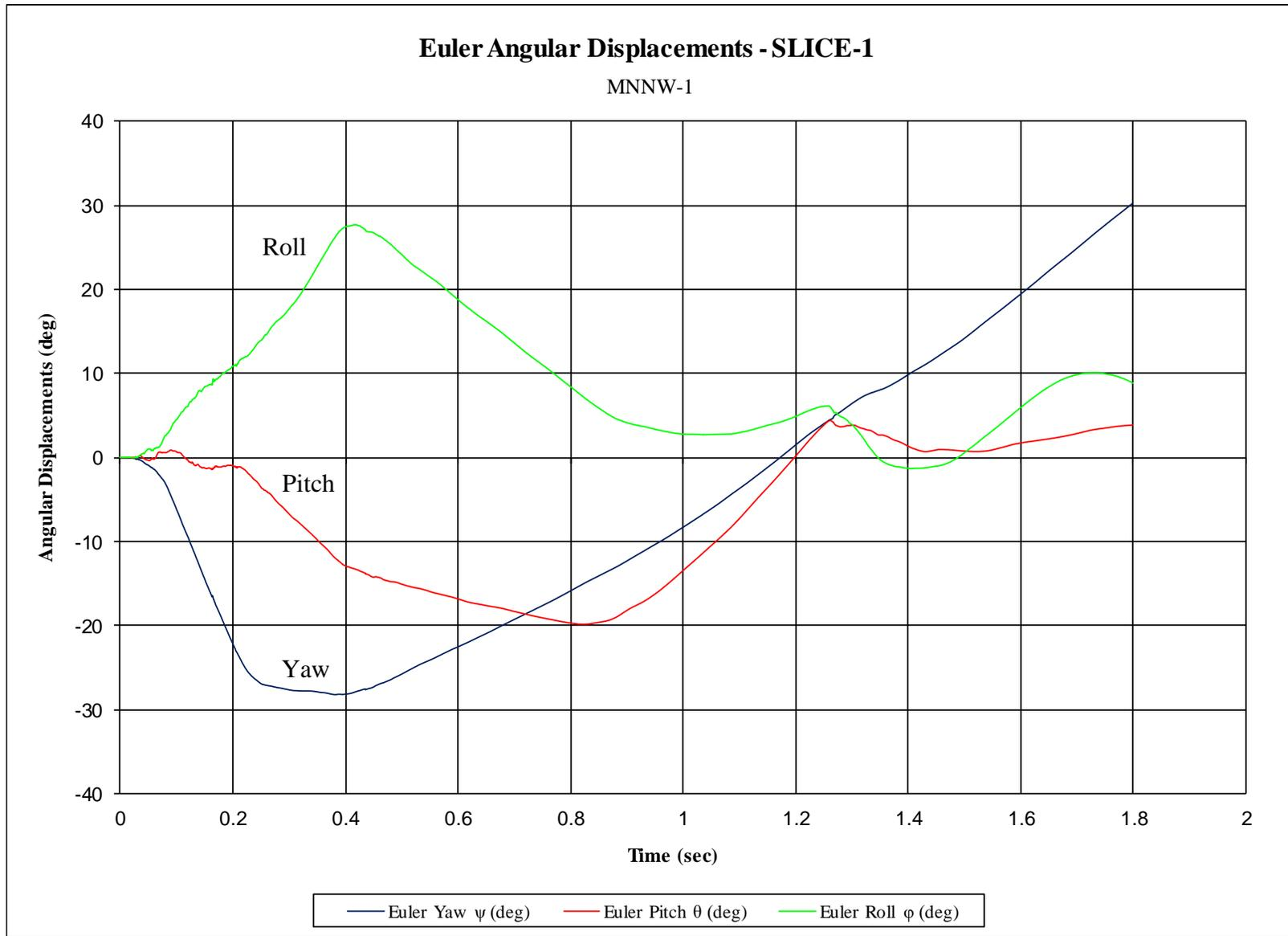
Figure F-7. Vehicle Angular Displacements (SLICE-1), Test No. MNNW-1
