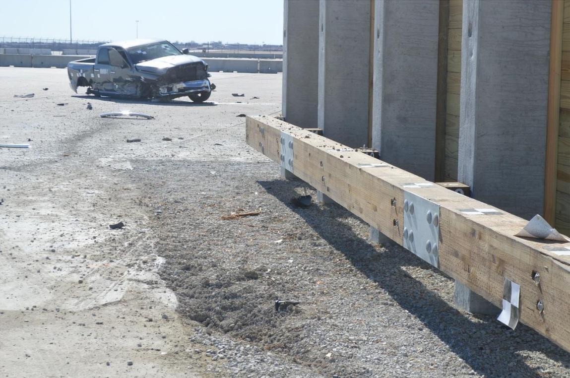
Figure 47. Vehicle Final Position and Trajectory Marks, Test No. MNNW-1
