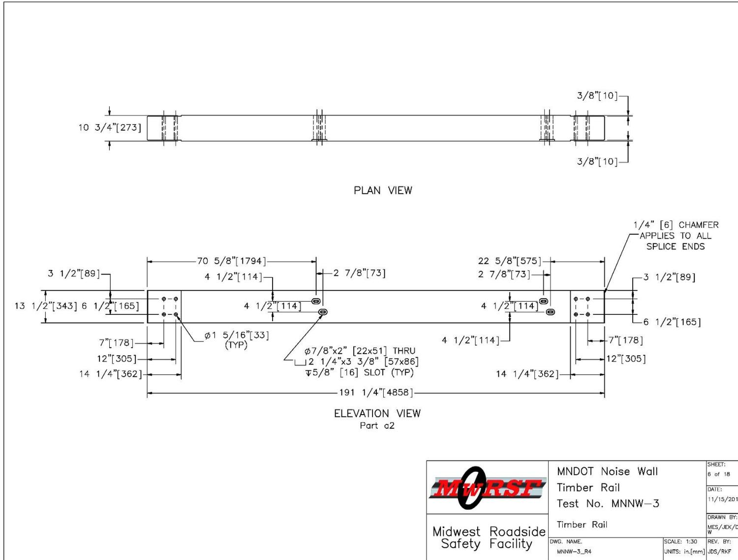
Figure 71. Timber Rail, Test Nos. Test No. MNNW-3 (Recommended updates provided in Chapter 12)
