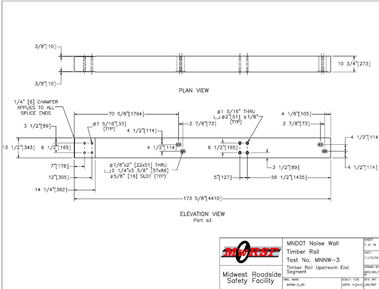
Figure 72. Timber Rail Upstream End Segment, Test No. MNNW-3 (Recommended updates provided in Chapter 12)
