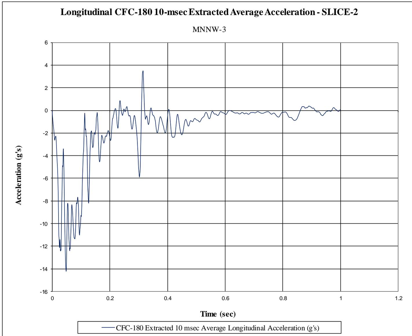
Figure H-9. 10-ms Average Longitudinal Deceleration (SLICE-2), Test No. MNNW-3
