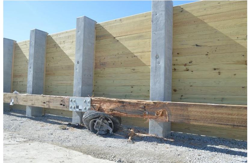
Figure 49. System Damage, Test No. MNNW-1
