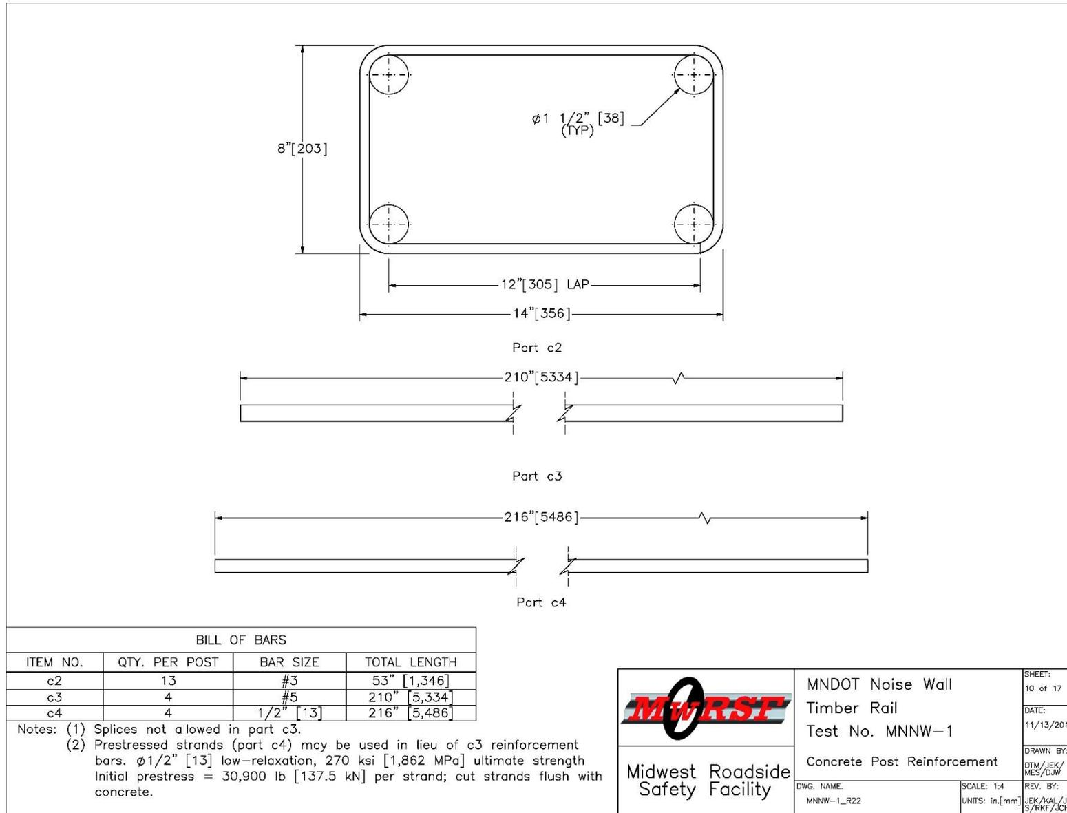
Figure 27. Concrete Post Reinforcement, Test Nos. MNNW-1 and MNNW-2 (Recommended updates provided in Chapter 12)
