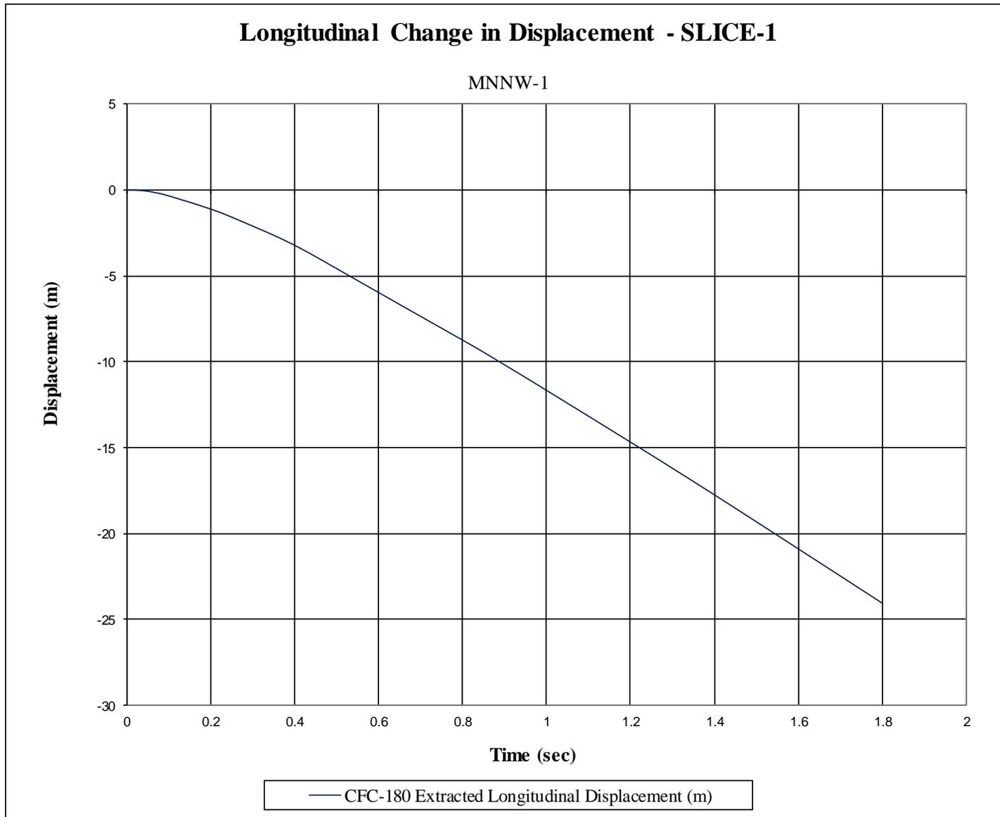
Figure F-3. Longitudinal Occupant Displacement (SLICE-1), Test No. MNNW-1
