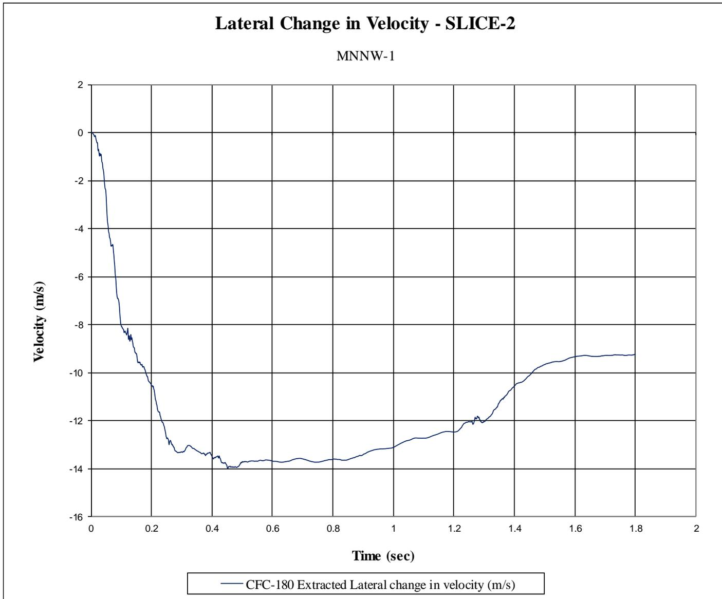
Figure F-13. Lateral Occupant Impact Velocity (SLICE-2), Test No. MNNW-1
