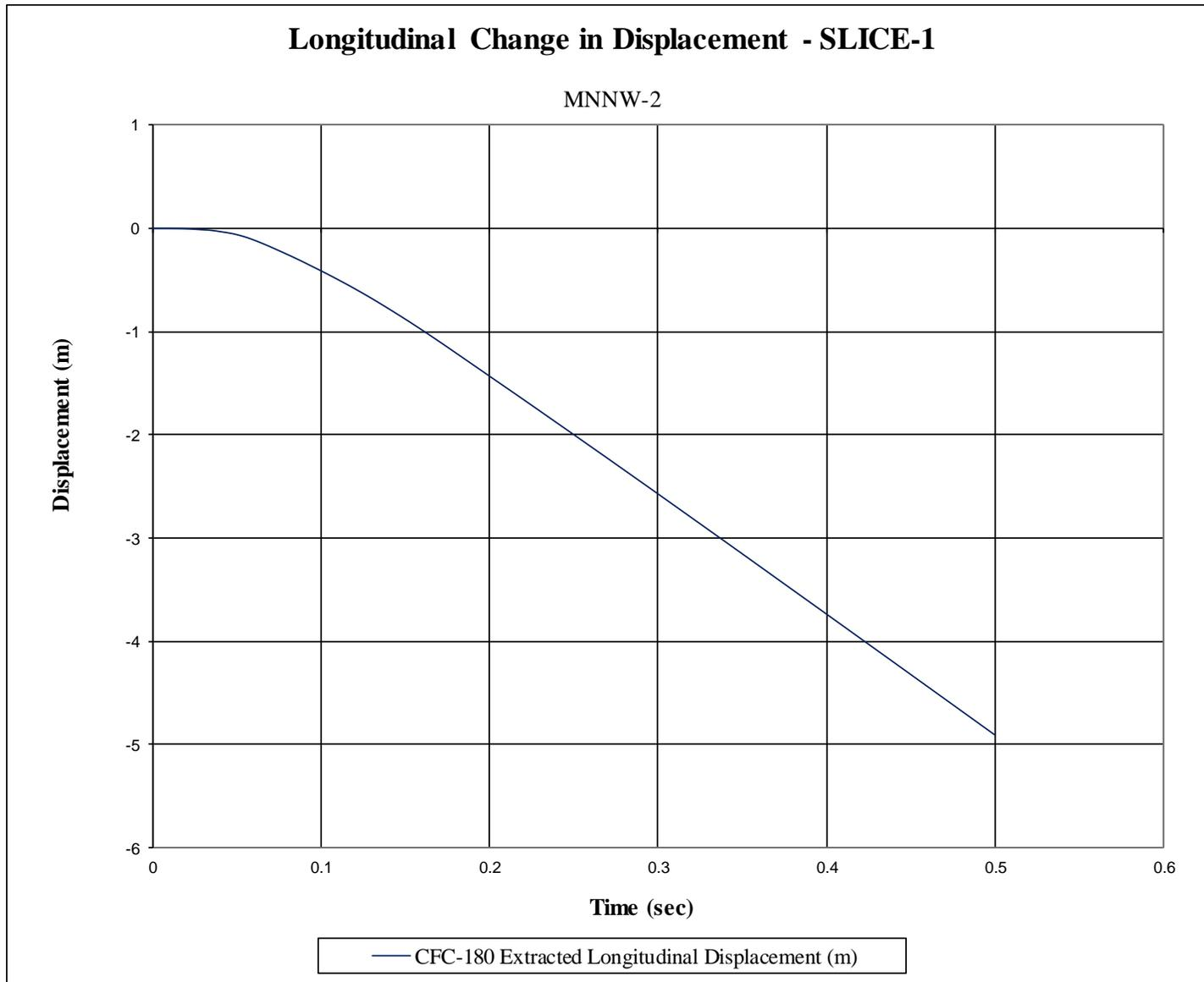
Figure G-3. Longitudinal Occupant Displacement (SLICE-1), Test No. MNNW-2
