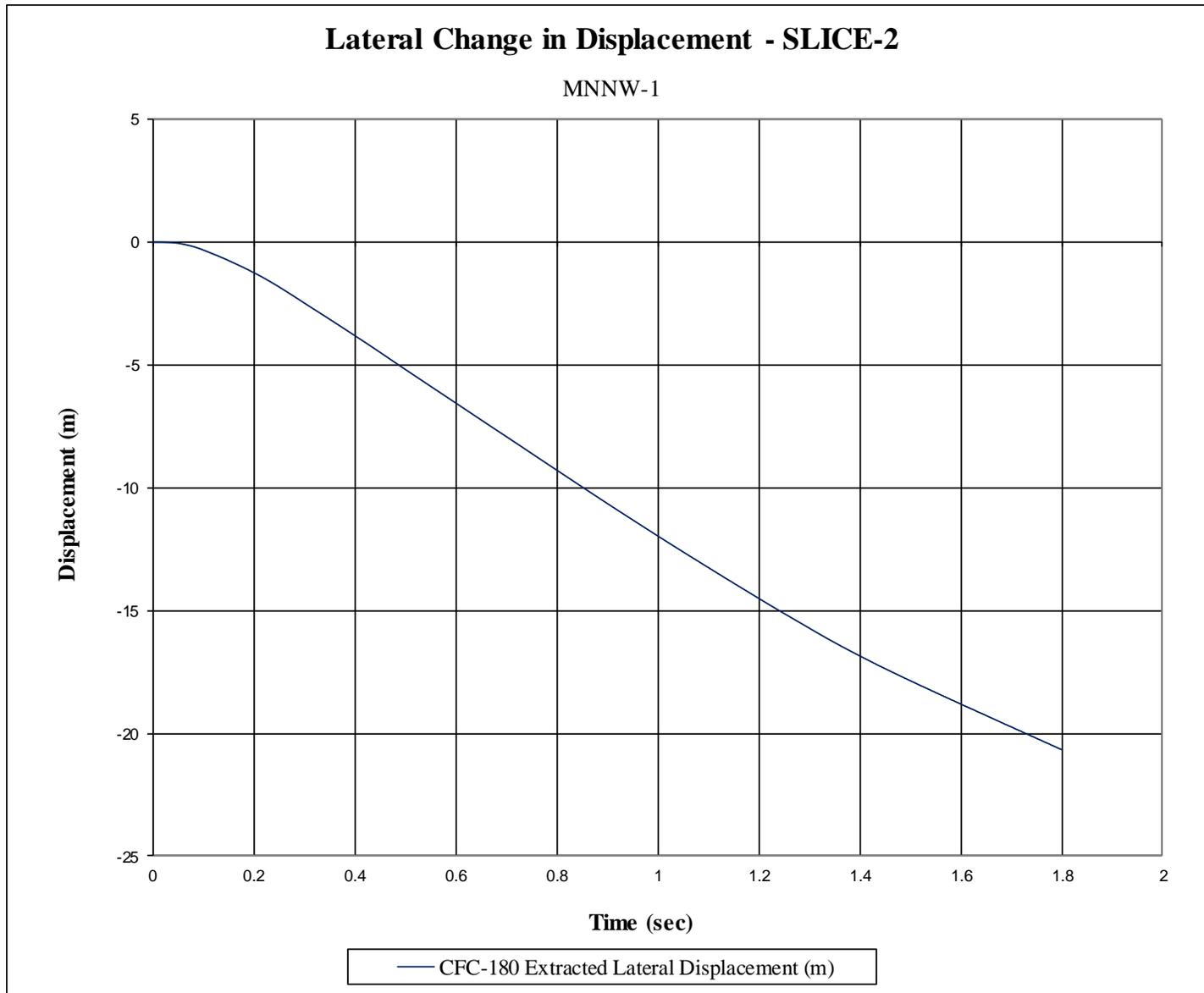
Figure F-14. Lateral Occupant Displacement (SLICE-2), Test No. MNNW-1
