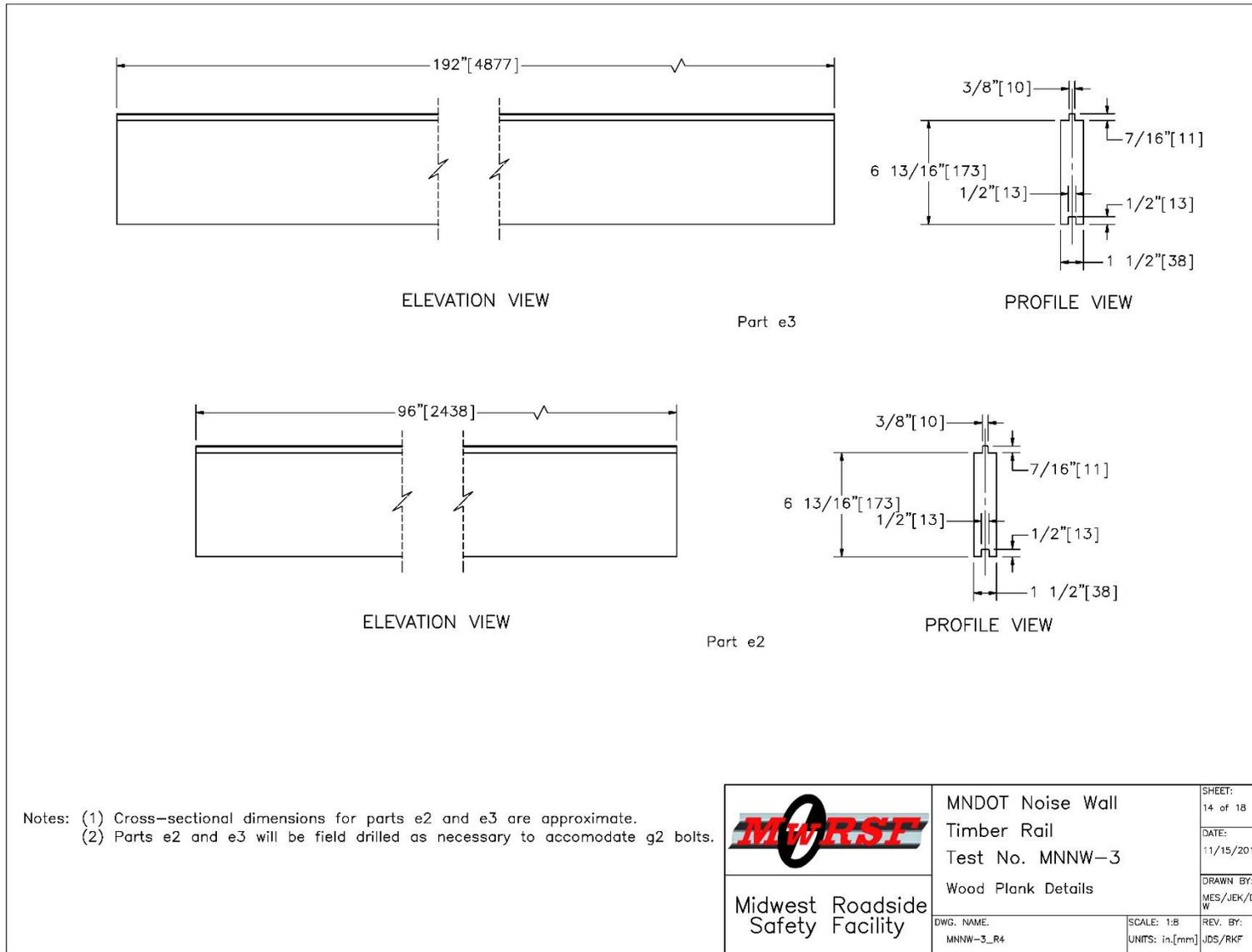
Figure 79. Wood Plank Details, Test No. MNNW-3 (Recommended updates provided in Chapter 12)
