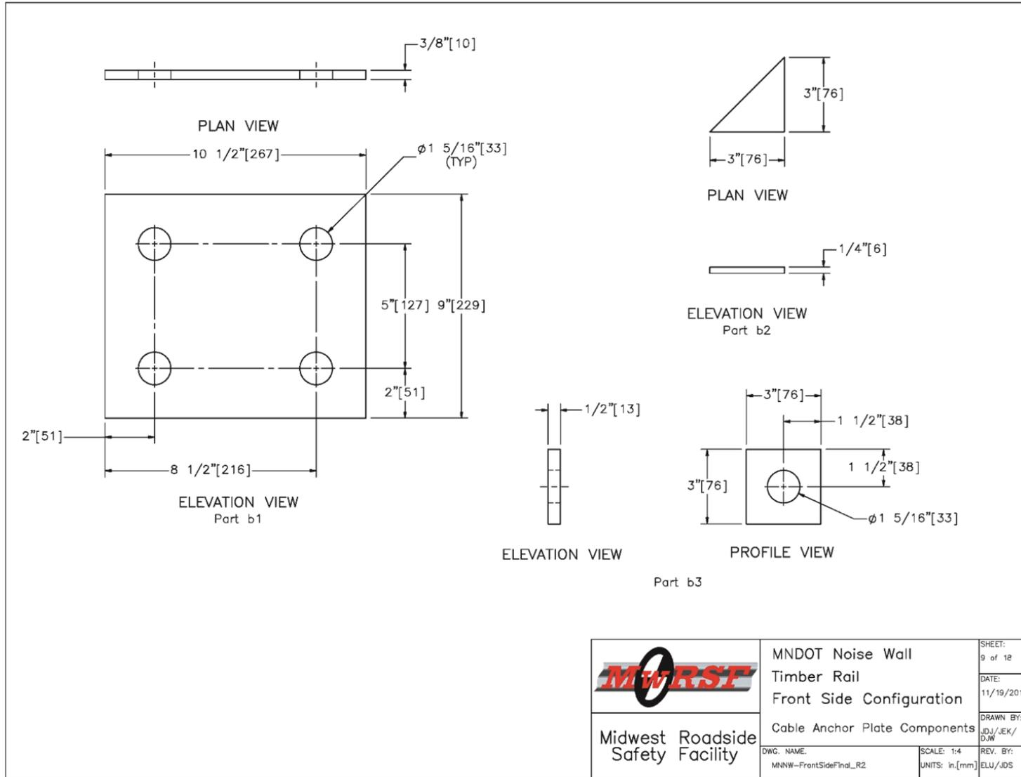
Figure 126. Cable Anchor Plate Components, Front-Side Noise Wall
