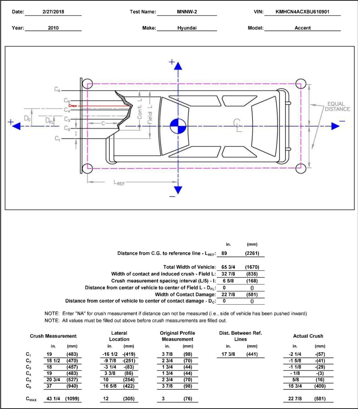
Figure E-11. Exterior Vehicle Crush (NASS) - Front, Test No. MNNW-2
