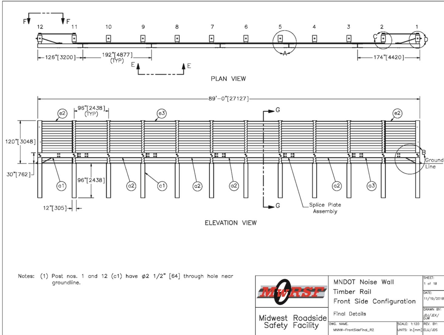
Figure 118. Final Details, Front-Side Noise Wall
