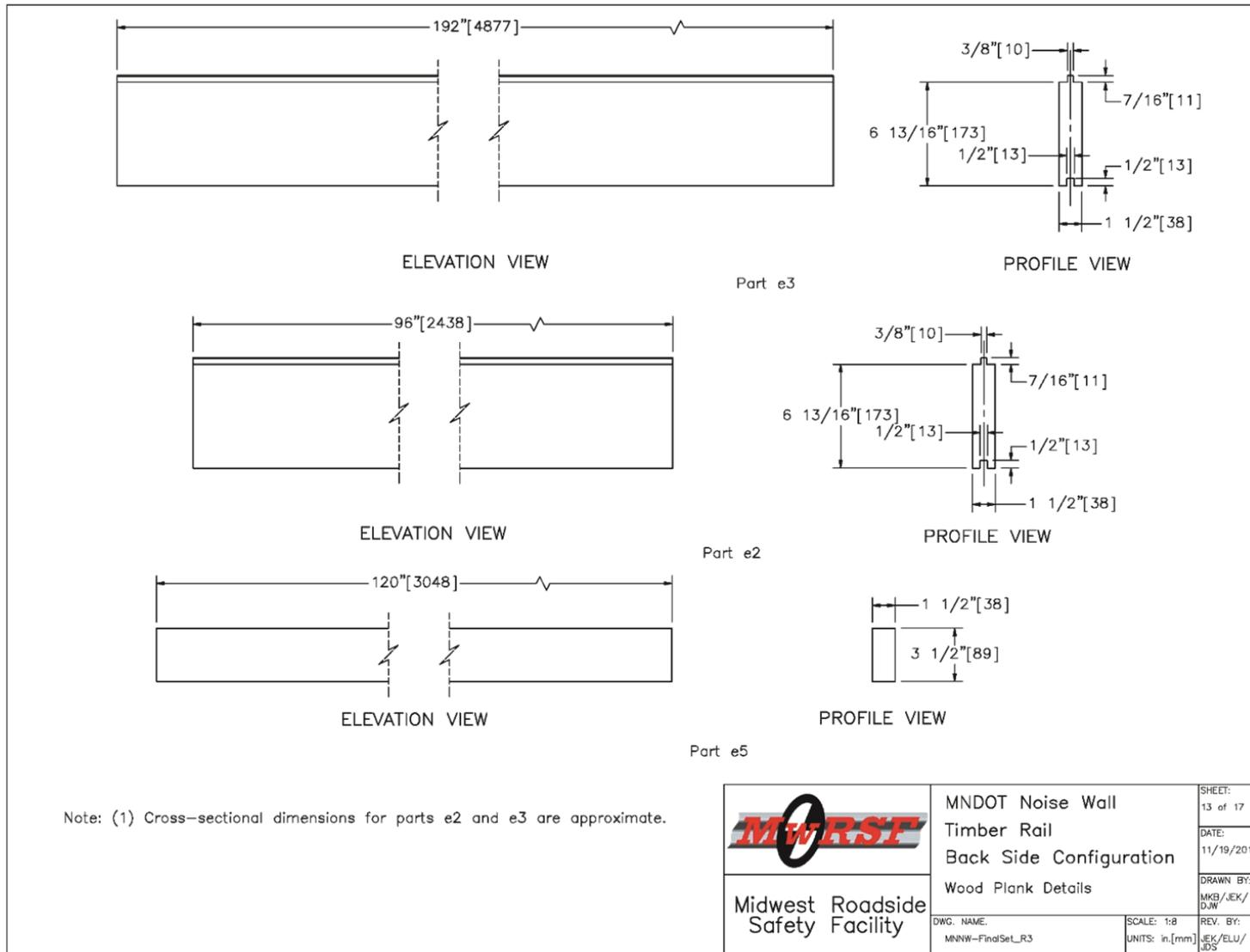
Figure 113. Wood Plank Details, Back-Side Noise Wall
