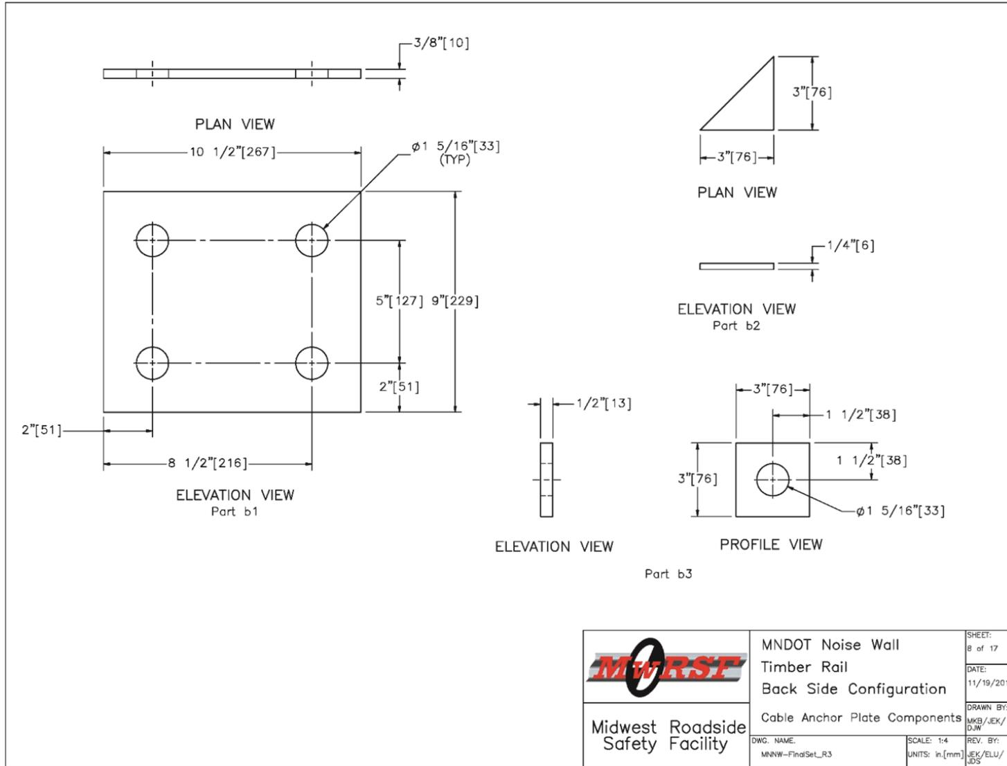
Figure 108. Cable Anchor Plate Components, Back-Side Noise Wall
