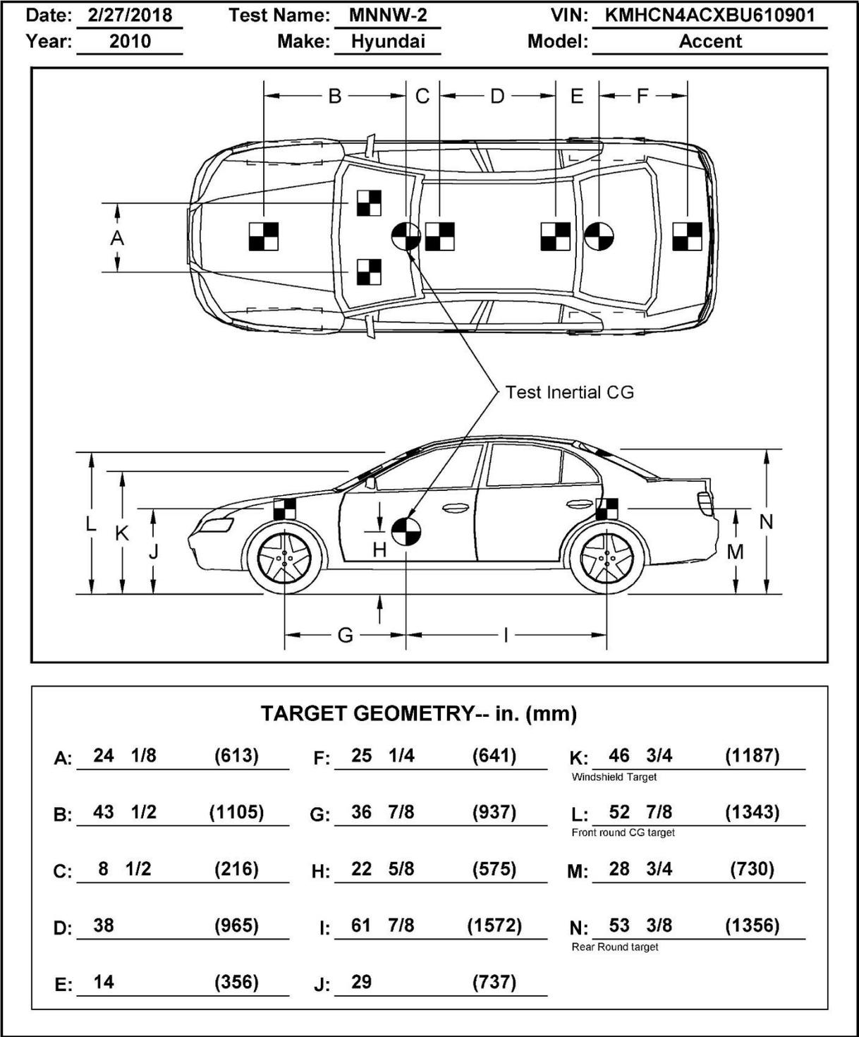
Figure 12. Target Geometry, Test No. MNNW-2
