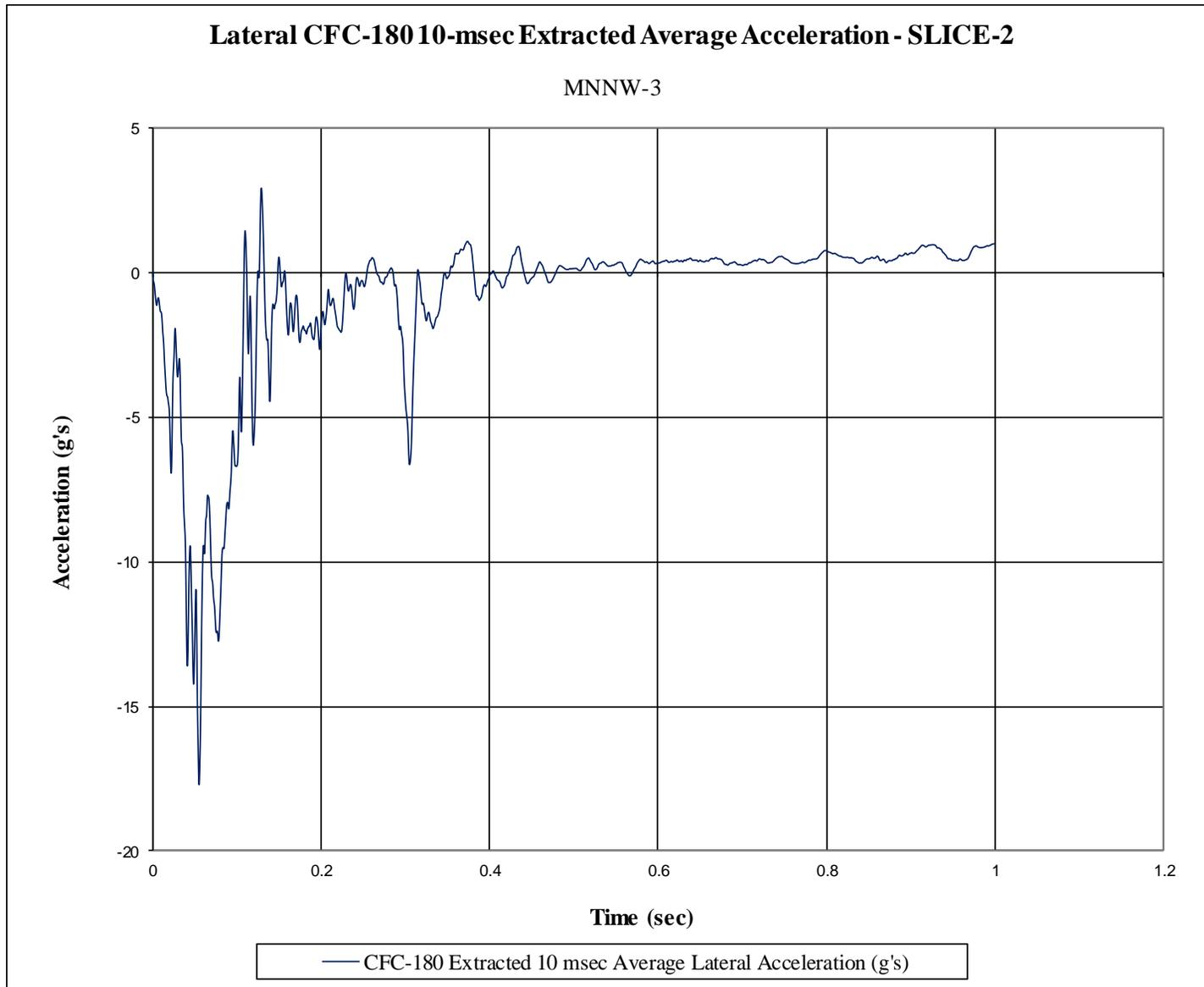
Figure H-12. 10-ms Average Lateral Deceleration (SLICE-2), Test No. MNNW-3
