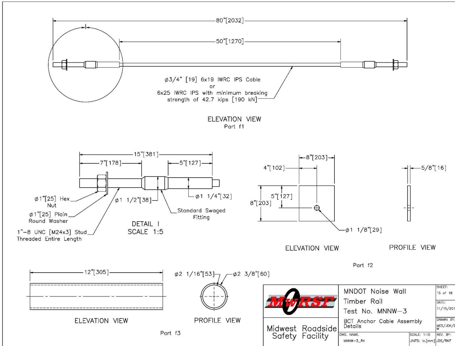
Figure 80. BCT Anchor Cable Assembly Details, Test No. MNNW-3 (Recommended updates provided in Chapter 12)
