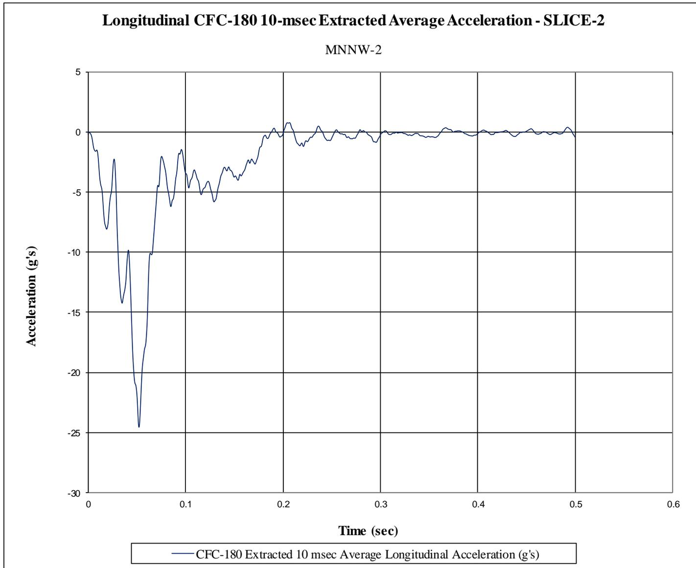
Figure G-9. 10-ms Average Longitudinal Deceleration (SLICE-2), Test No. MNNW-2
