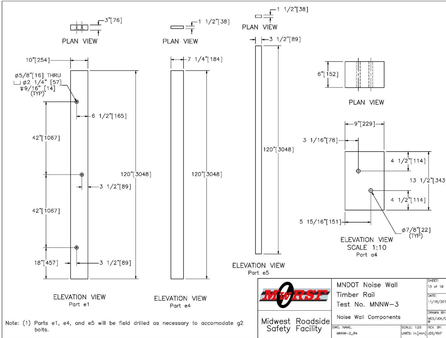
Figure 78. Noise Wall Components, Test Nos. Test No. MNNW-3 (Recommended updates provided in Chapter 12)
