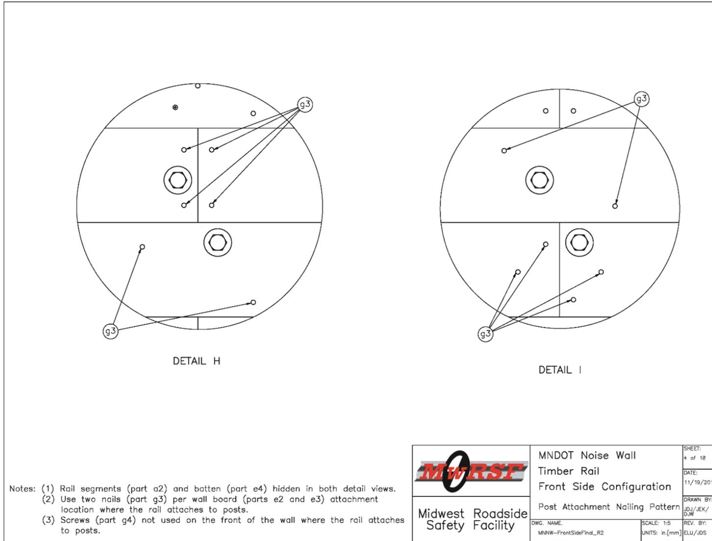
Figure 121. Post Attachment Nailing Pattern, Front-Side Noise Wall
