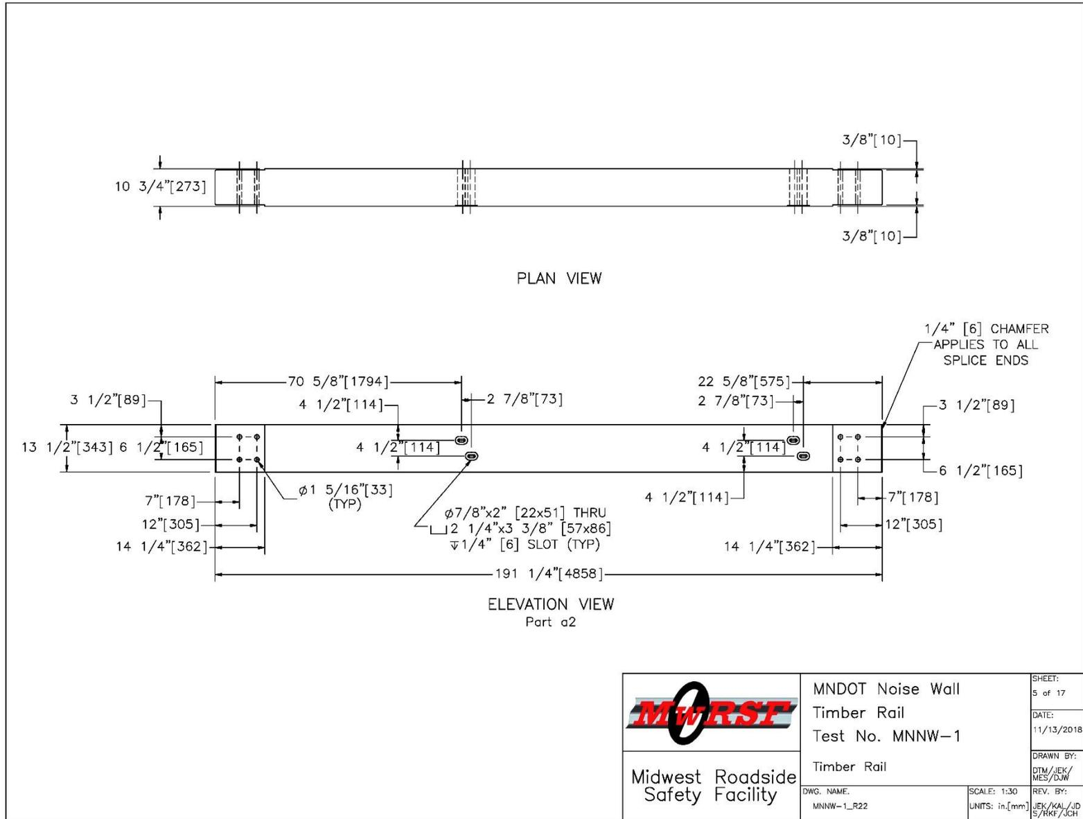
Figure 22. Timber Rail, Test Nos. MNNW-1 and MNNW-2 (Recommended updates provided in Chapter 12)
