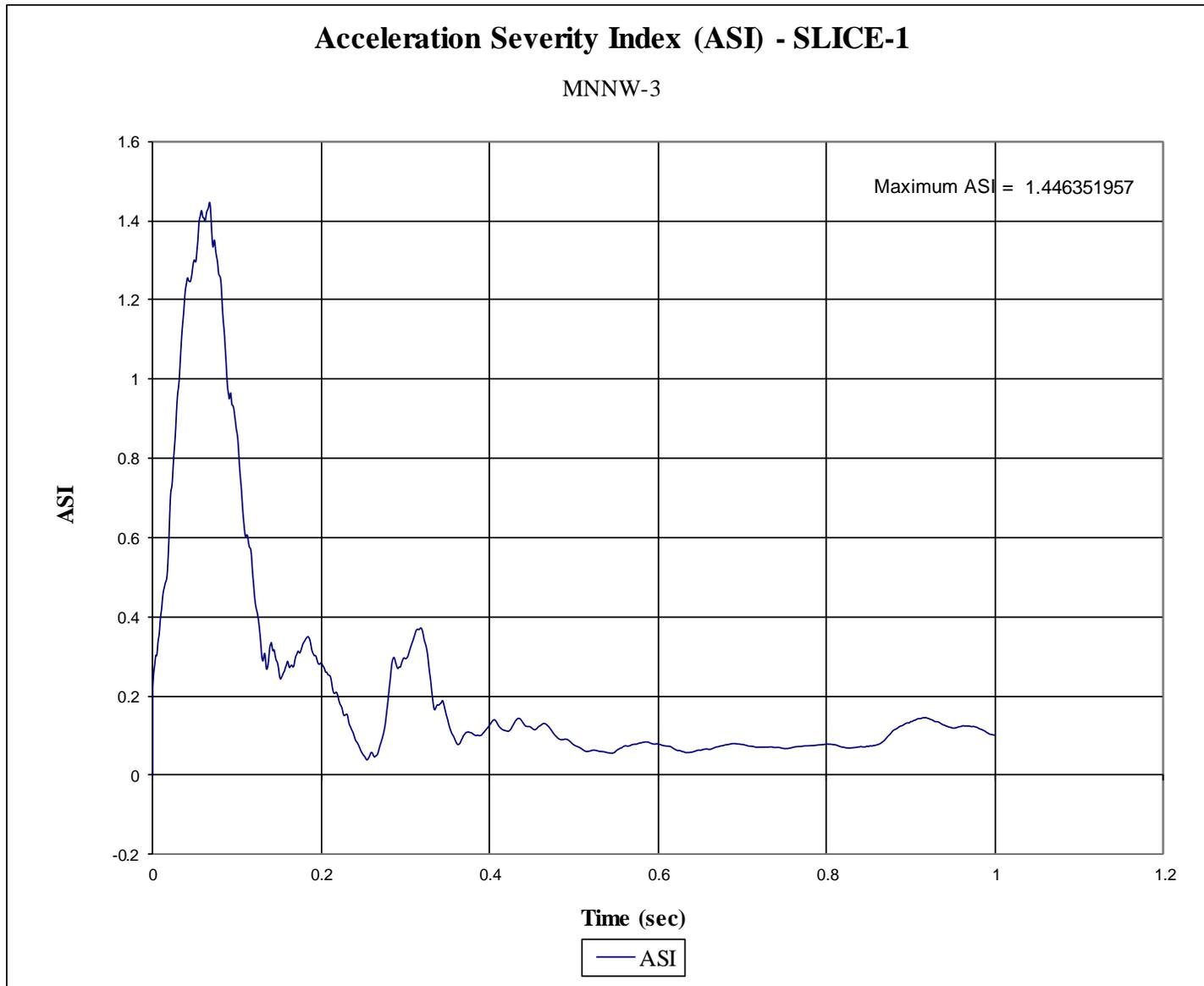
Figure H-8. Acceleration Severity Index (SLICE-1), Test No. MNNW-3
