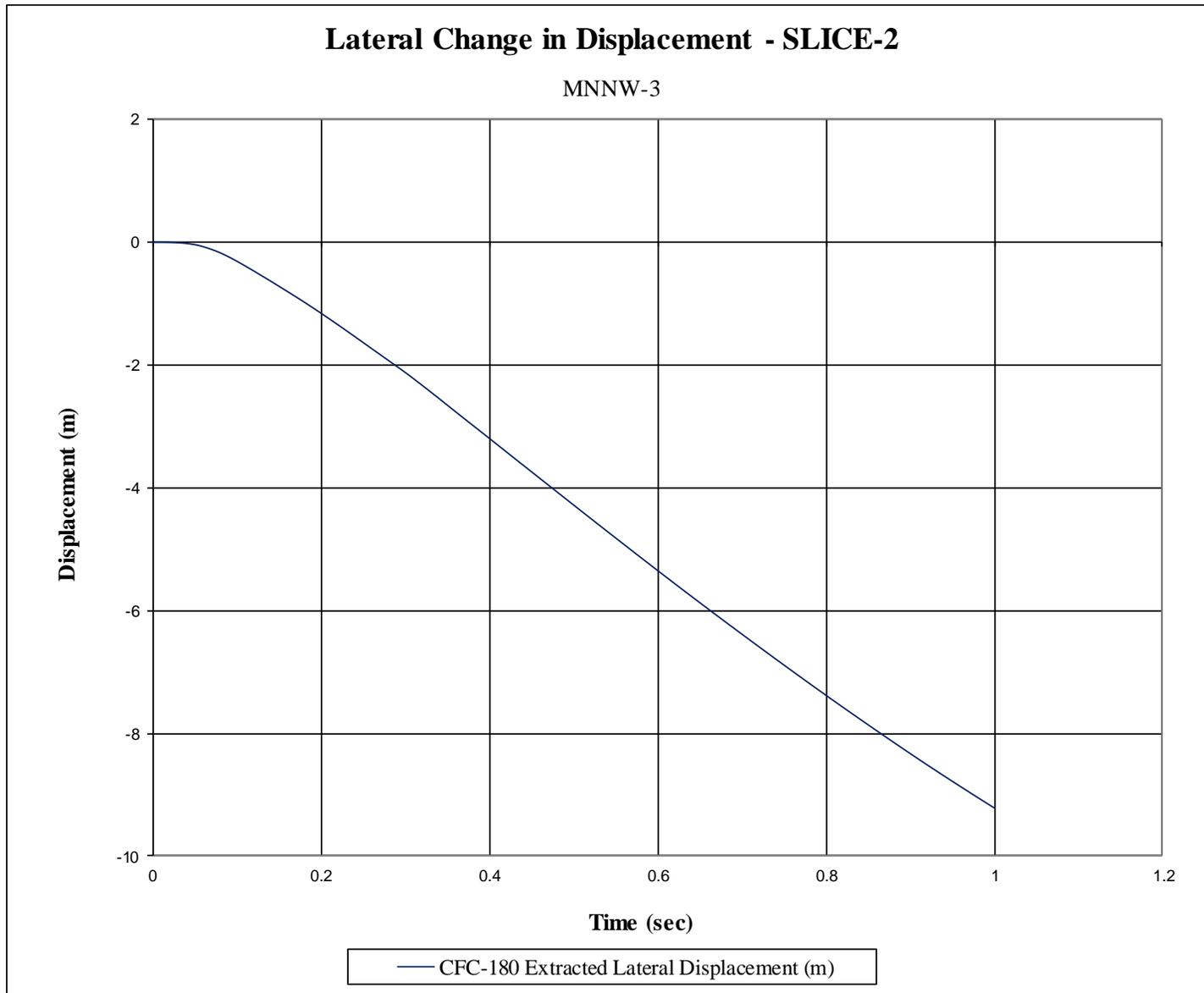
Figure H-14. Lateral Occupant Displacement (SLICE-2), Test No. MNNW-3
