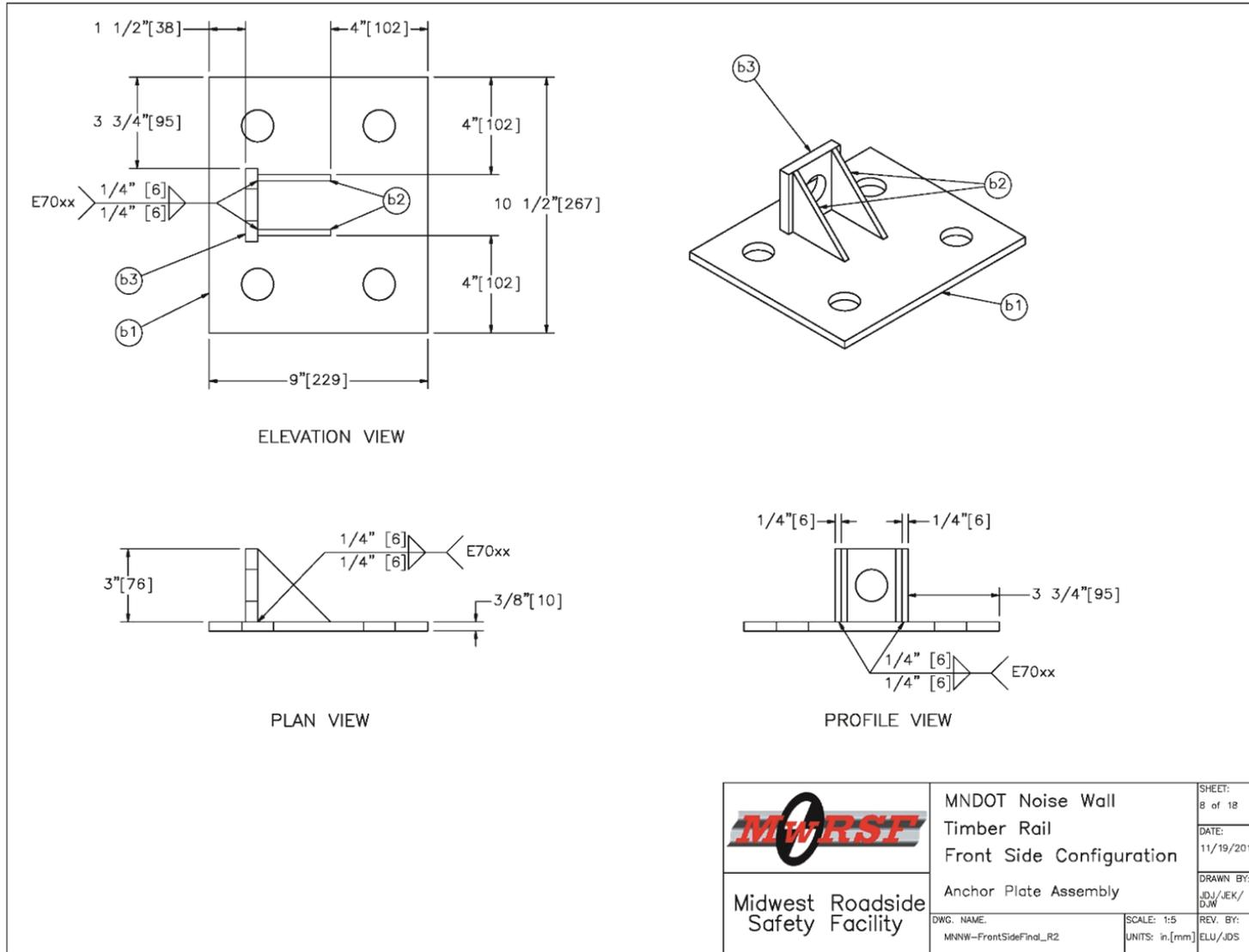
Figure 125. Anchor Plate Assembly, Front-Side Noise Wall
