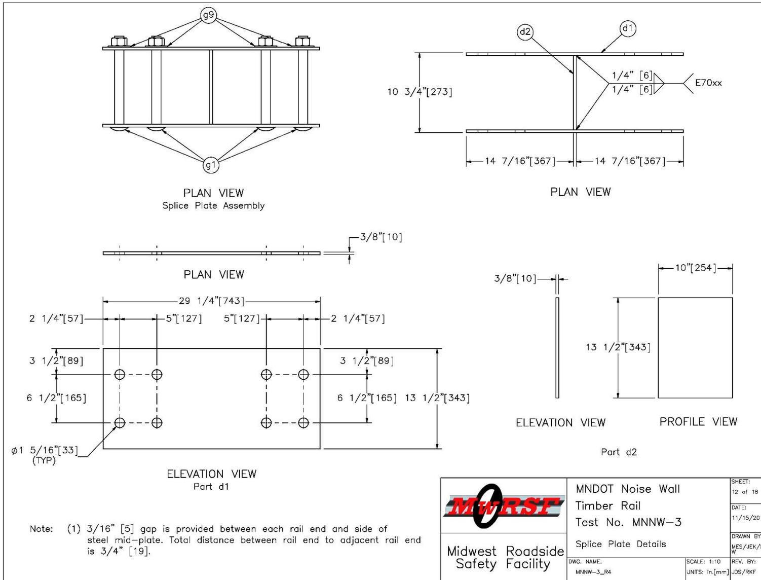
Figure 77. Splice Plate Details, Test No. MNNW-3 (Recommended updates provided in Chapter 12)
