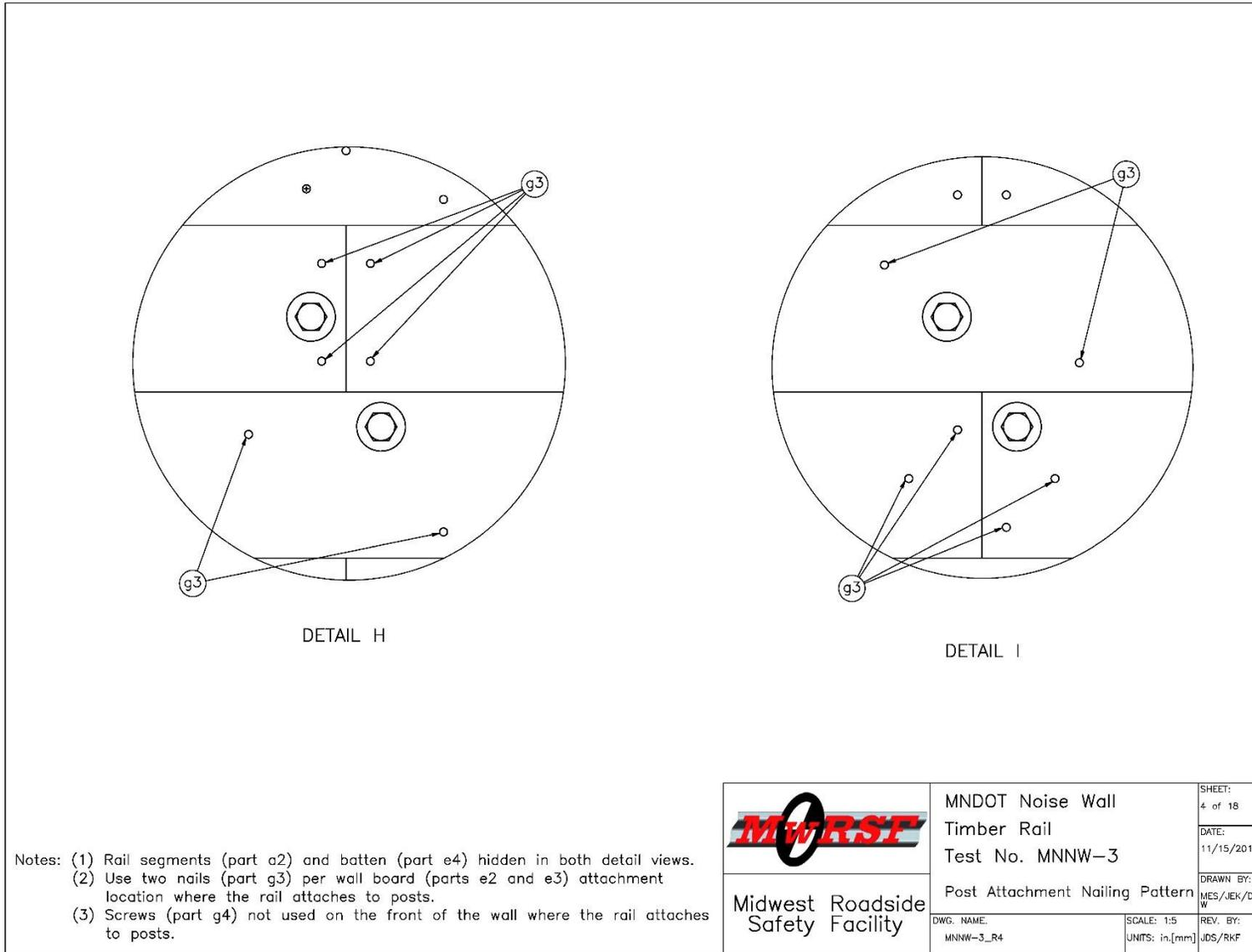
Figure 69. Post Attachment Nailing Pattern, Test No. MNNW-3 (Recommended updates provided in Chapter 12)
