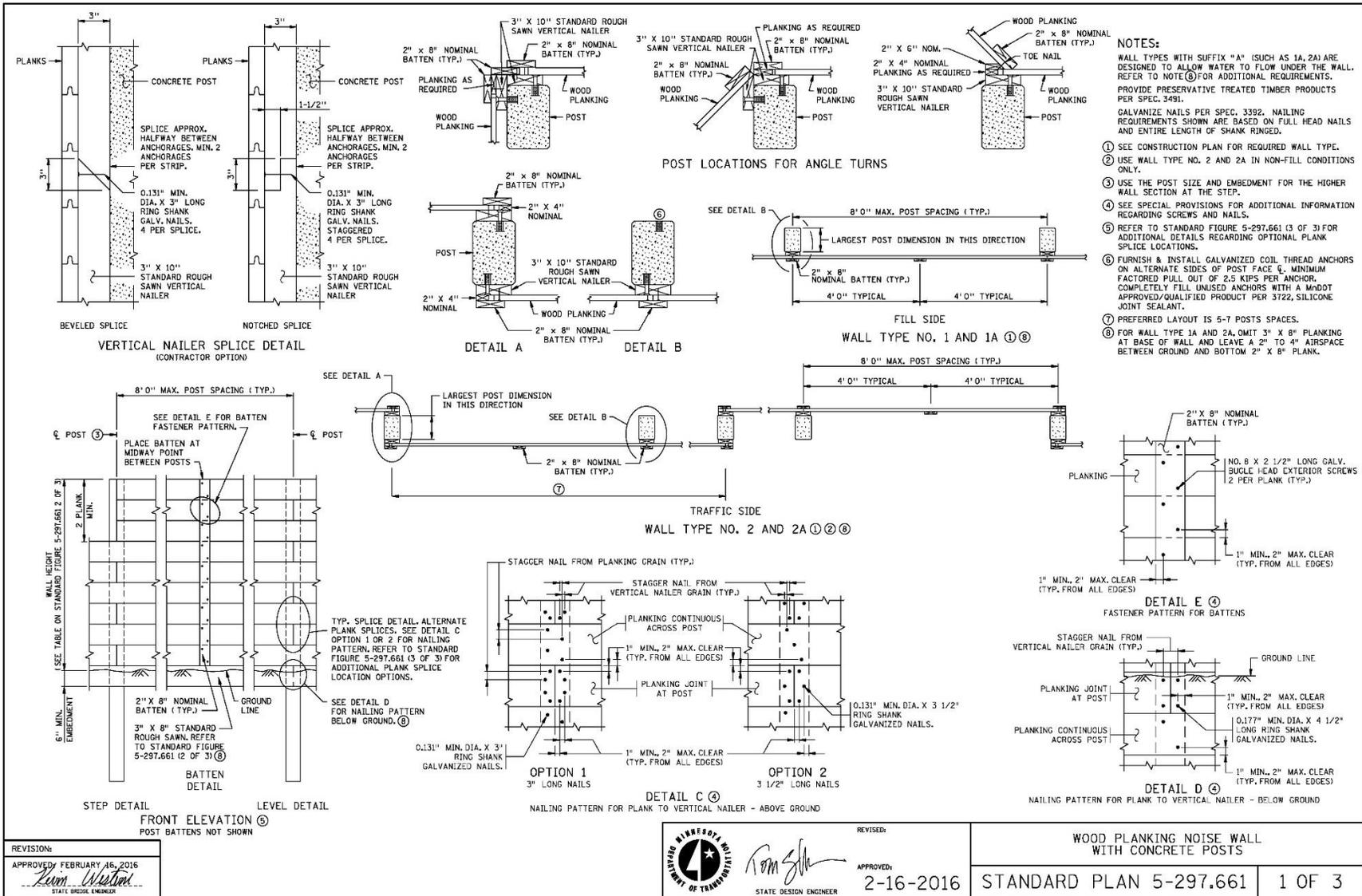
Figure A-1. Wood Planking Noise Wall with Concrete Posts
