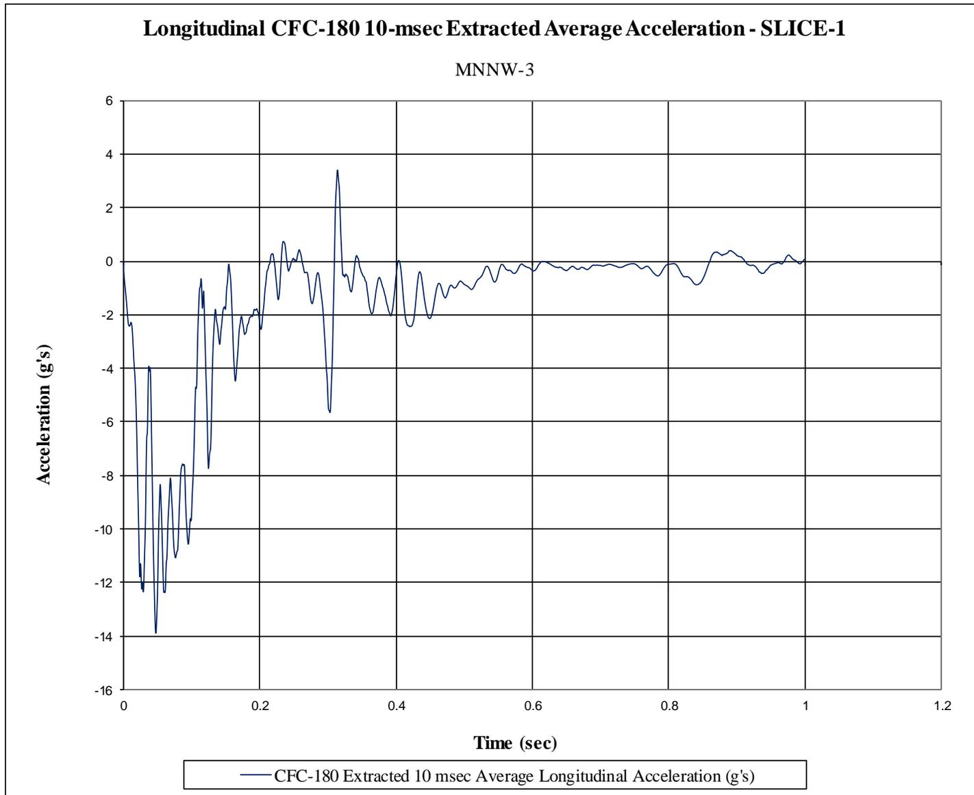
Figure H-1. 10-ms Average Longitudinal Deceleration (SLICE-1), Test No. MNNW-3
