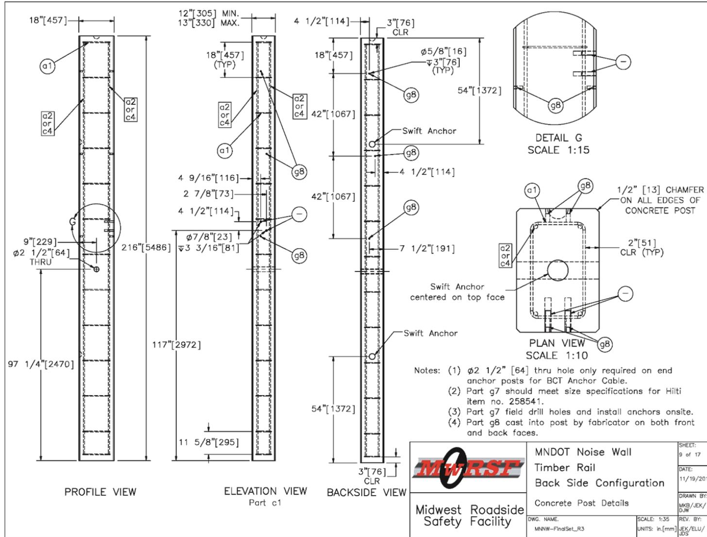
Figure 109. Concrete Post Details, Back-Side Noise Wall
