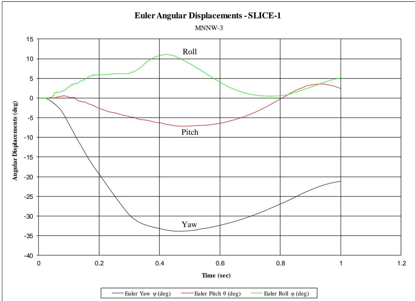
Figure H-7. Vehicle Angular Displacements (SLICE-1), Test No. MNNW-3
