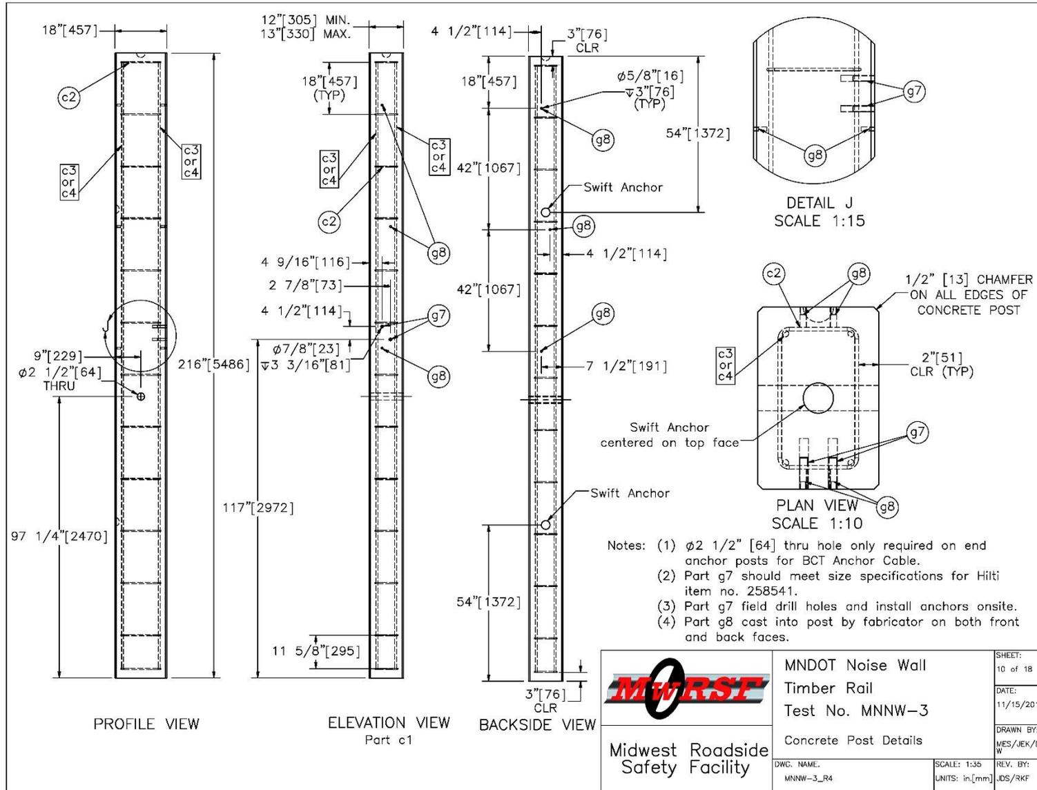
Figure 75. Concrete Post Details, Test No. MNNW-3 (Recommended updates provided in Chapter 12)
