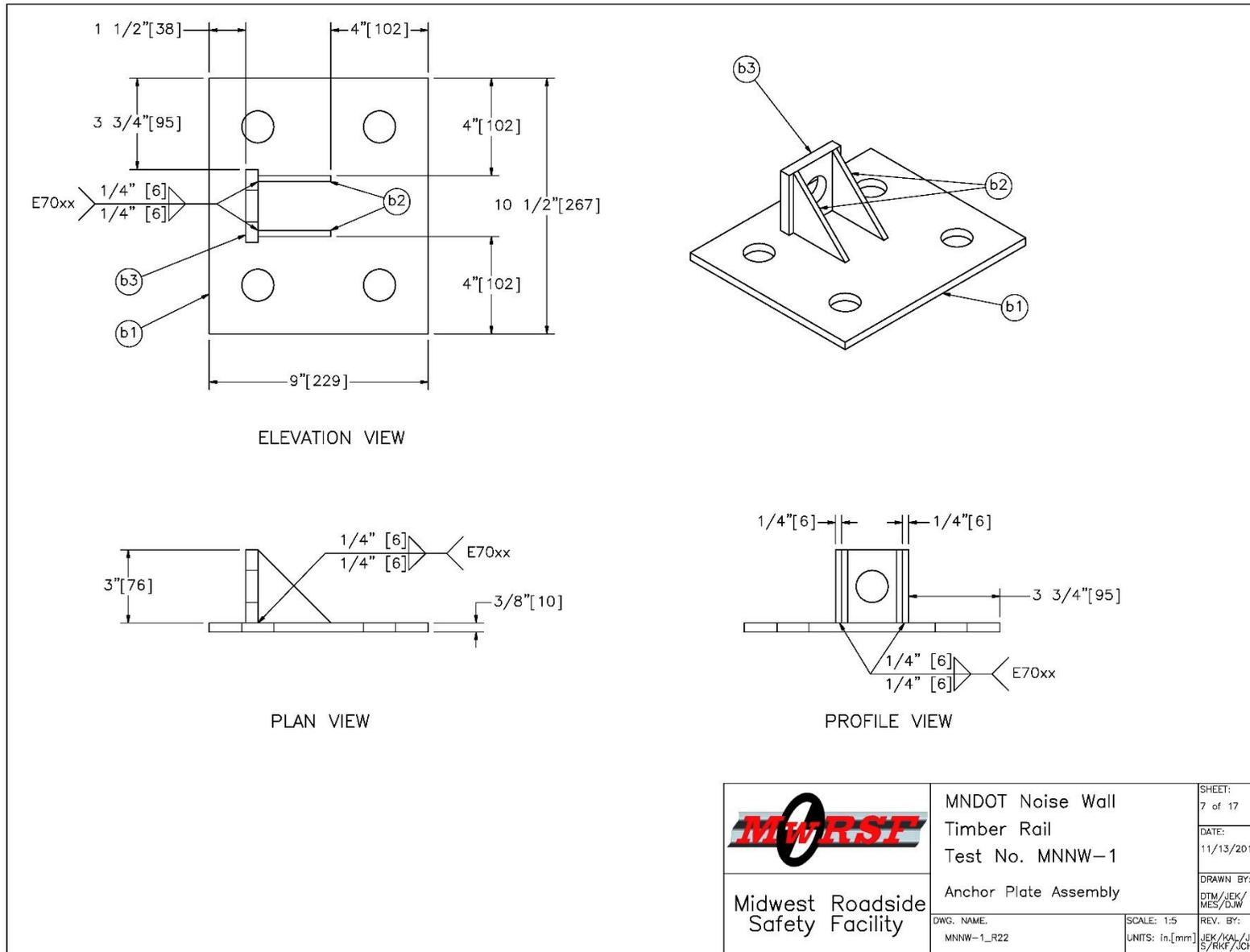
Figure 24. Anchor Plate Assembly, Test Nos. MNNW-1 and MNNW-2 (Recommended updates provided in Chapter 12)
