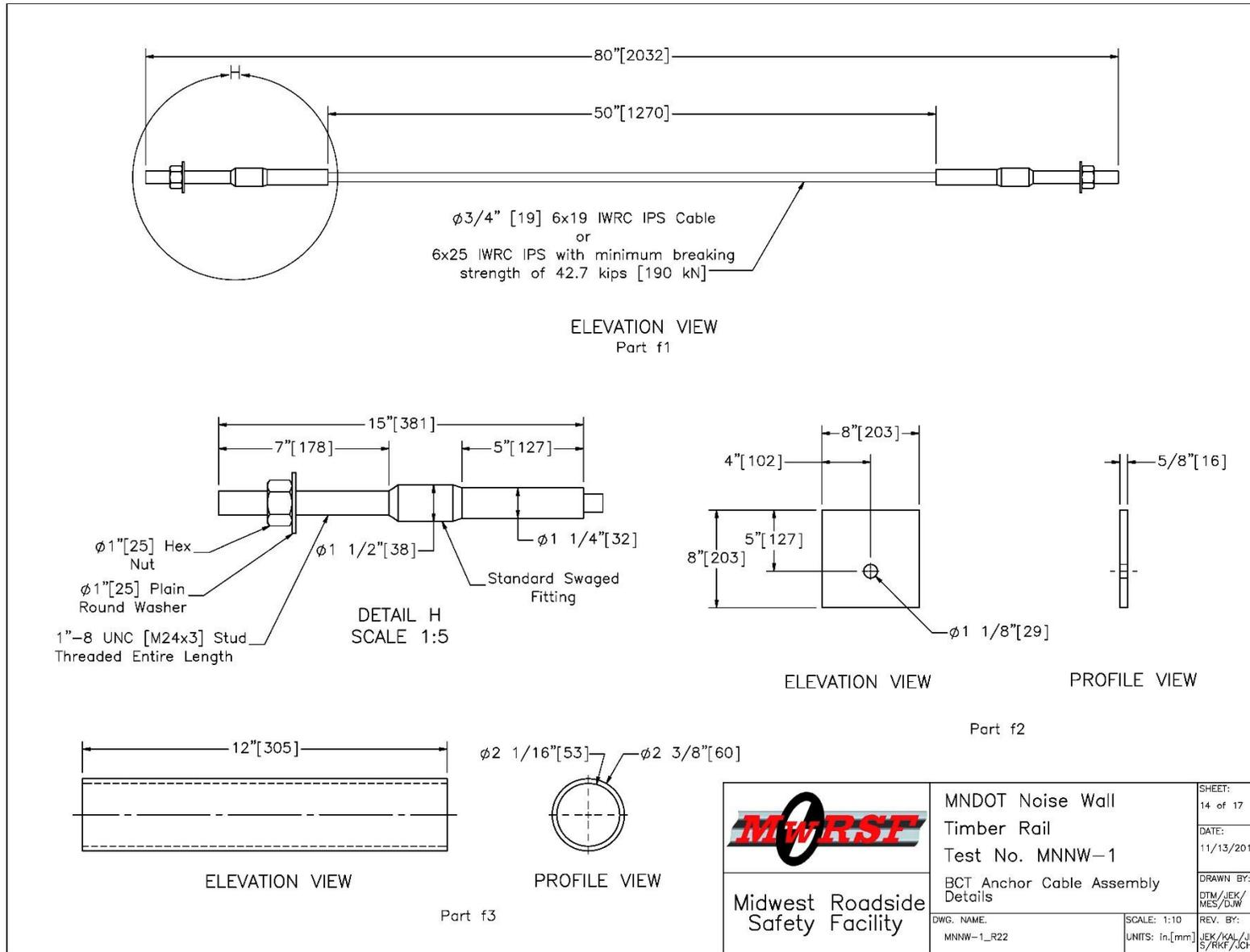
Figure 31. BCT Anchor Cable Assembly Details, Test Nos. MNNW-1 and MNNW-2 (Recommended updates provided in Chapter 12)
