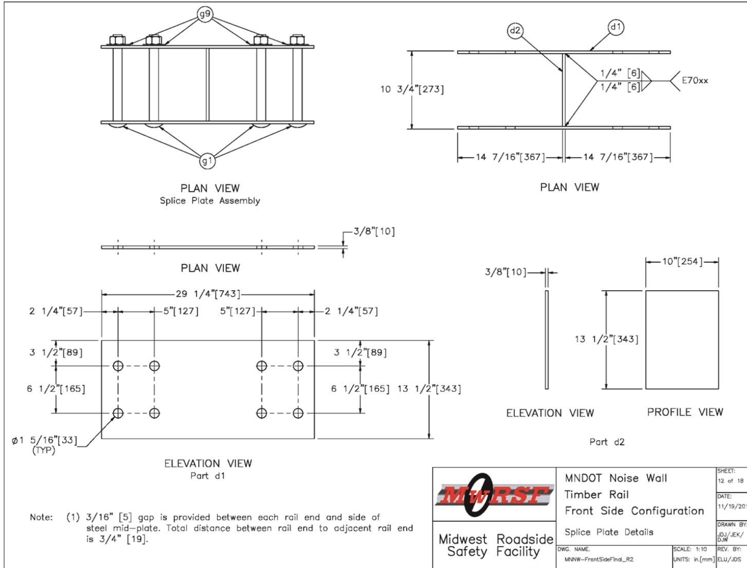
Figure 129. Splice Plate Details, Front-Side Noise Wall
