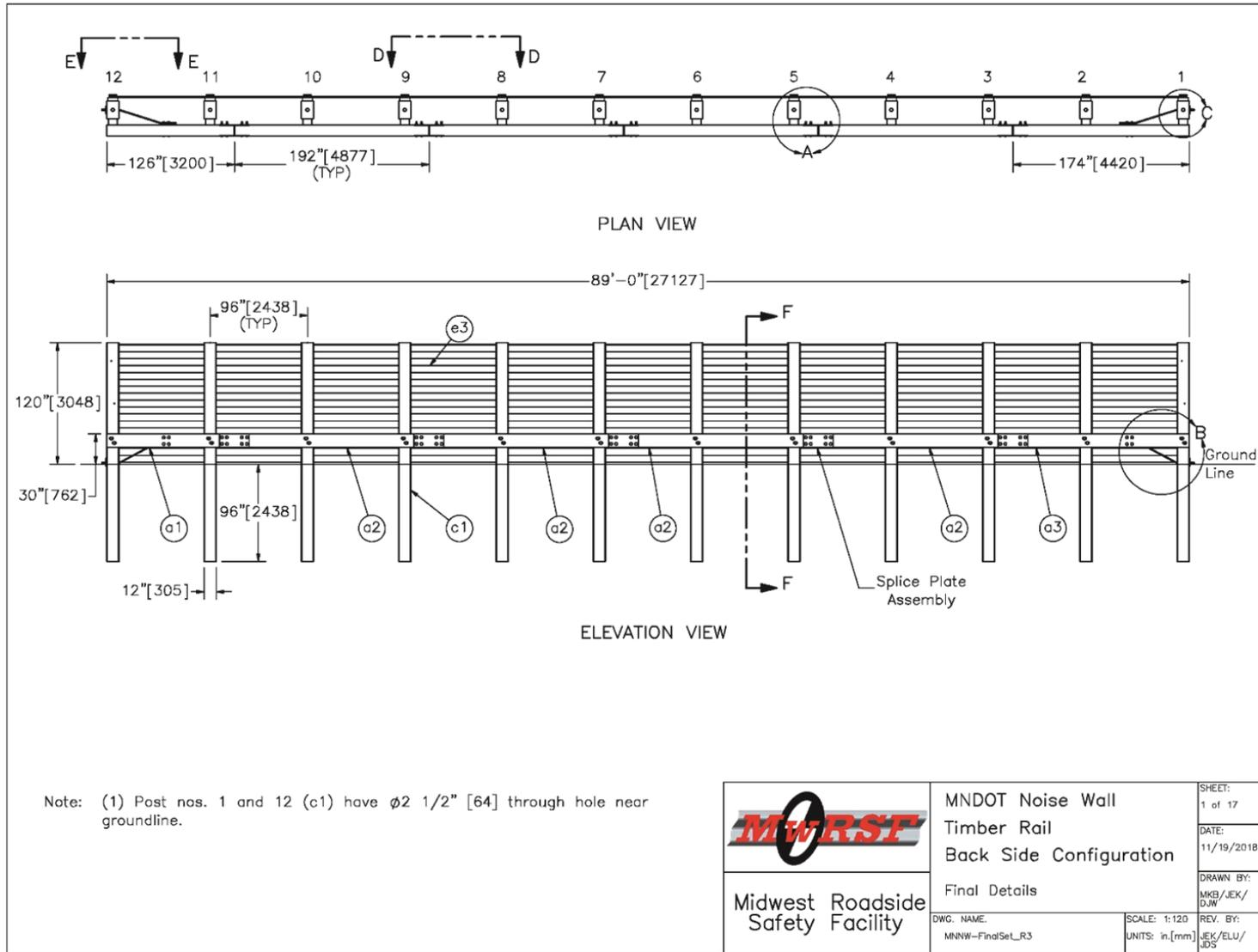
Figure 101. Final Details, Back-Side Noise Wall
