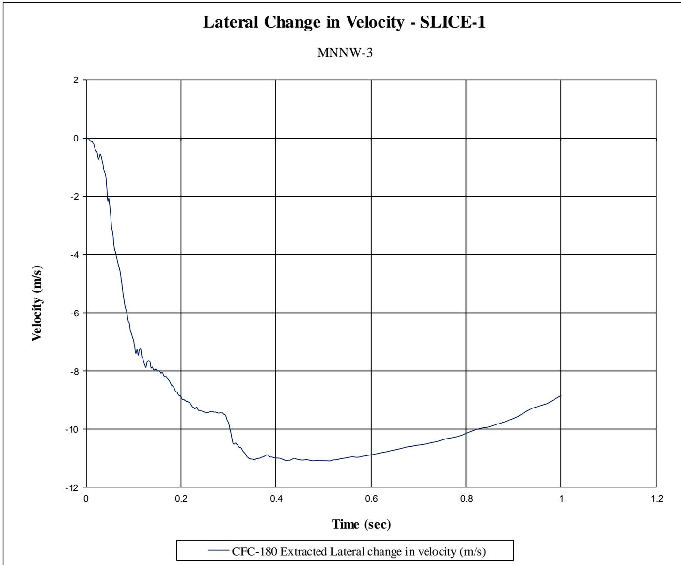
Figure H-5. Lateral Occupant Impact Velocity (SLICE-1), Test No. MNNW-3
