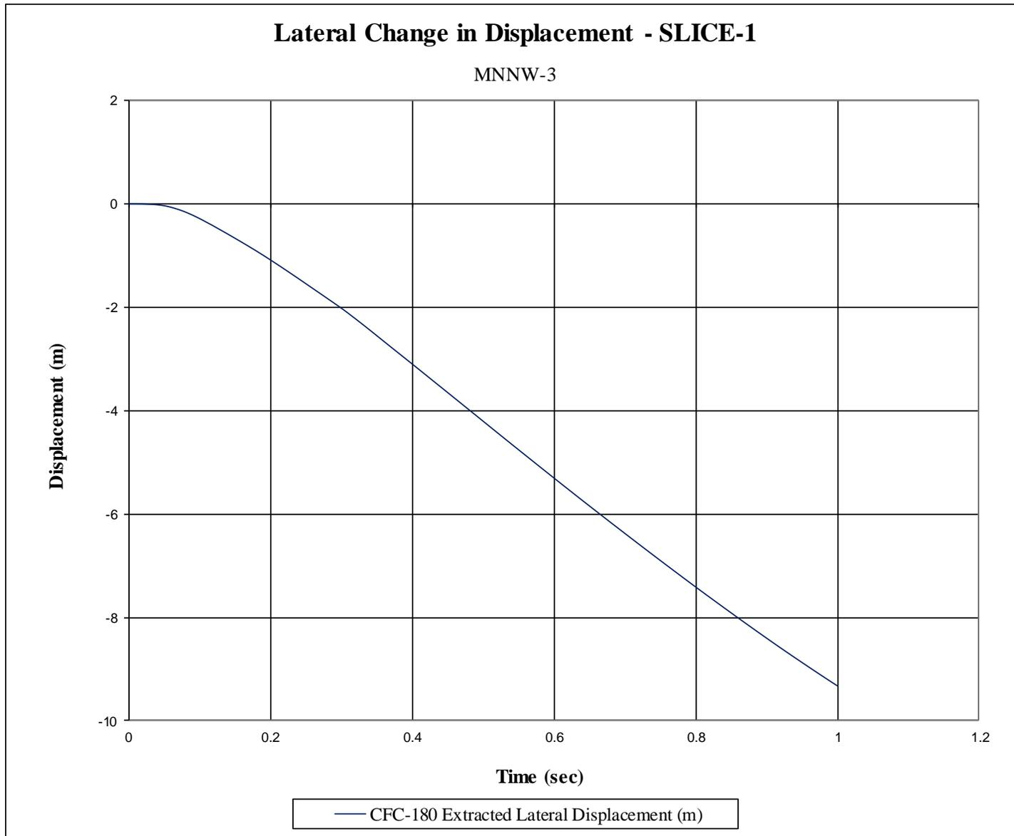
Figure H-6. Lateral Occupant Displacement (SLICE-1), Test No. MNNW-3
