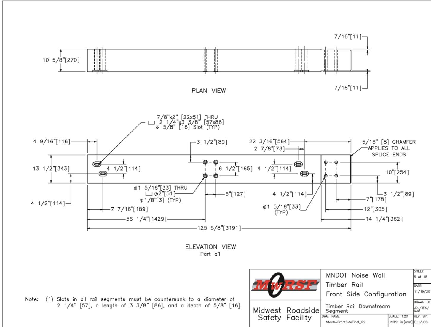
Figure 122. Timber Rail Downstream Segment, Front-Side Noise Wall
