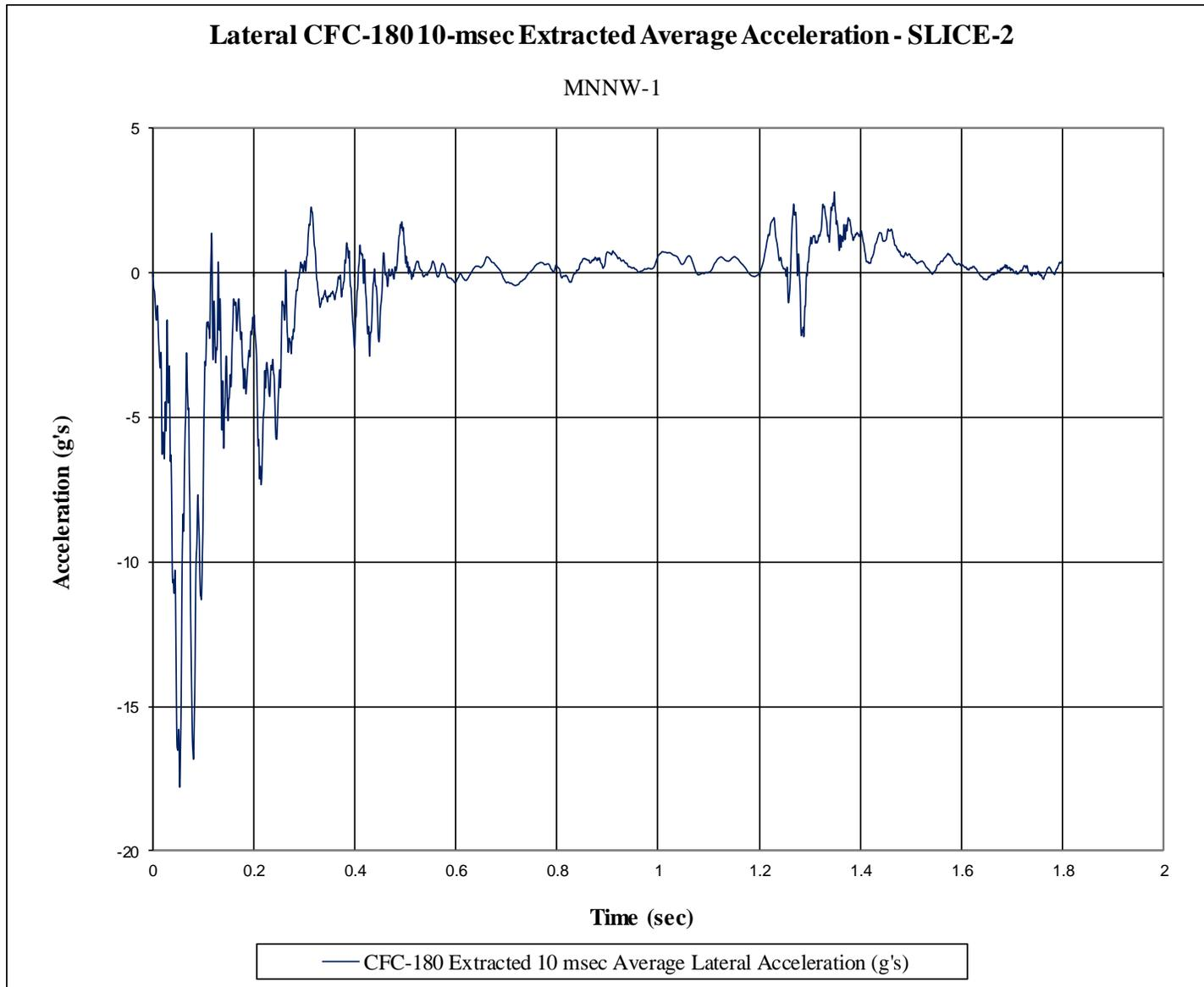
Figure F-12. 10-ms Average Lateral Deceleration (SLICE-2), Test No. MNNW-1
