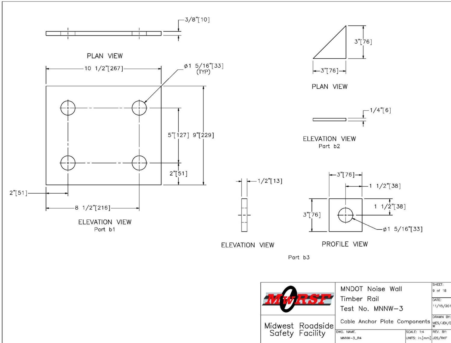
Figure 74. Cable Anchor Plate Components, Test No. MNNW-3 (Recommended updates provided in Chapter 12)
