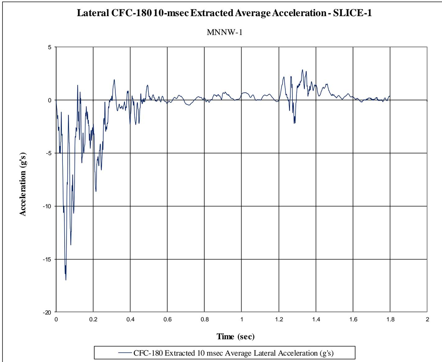
Figure F-4. 10-ms Average Lateral Deceleration (SLICE-1), Test No. MNNW-1
