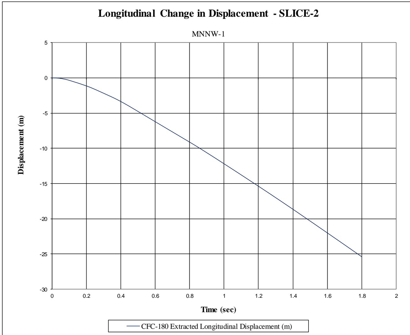
Figure F-11. Longitudinal Occupant Displacement (SLICE-2), Test No. MNNW-1
