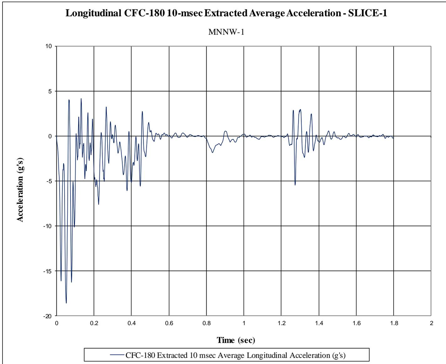
Figure F-1. 10-ms Average Longitudinal Deceleration (SLICE-1), Test No. MNNW-1
