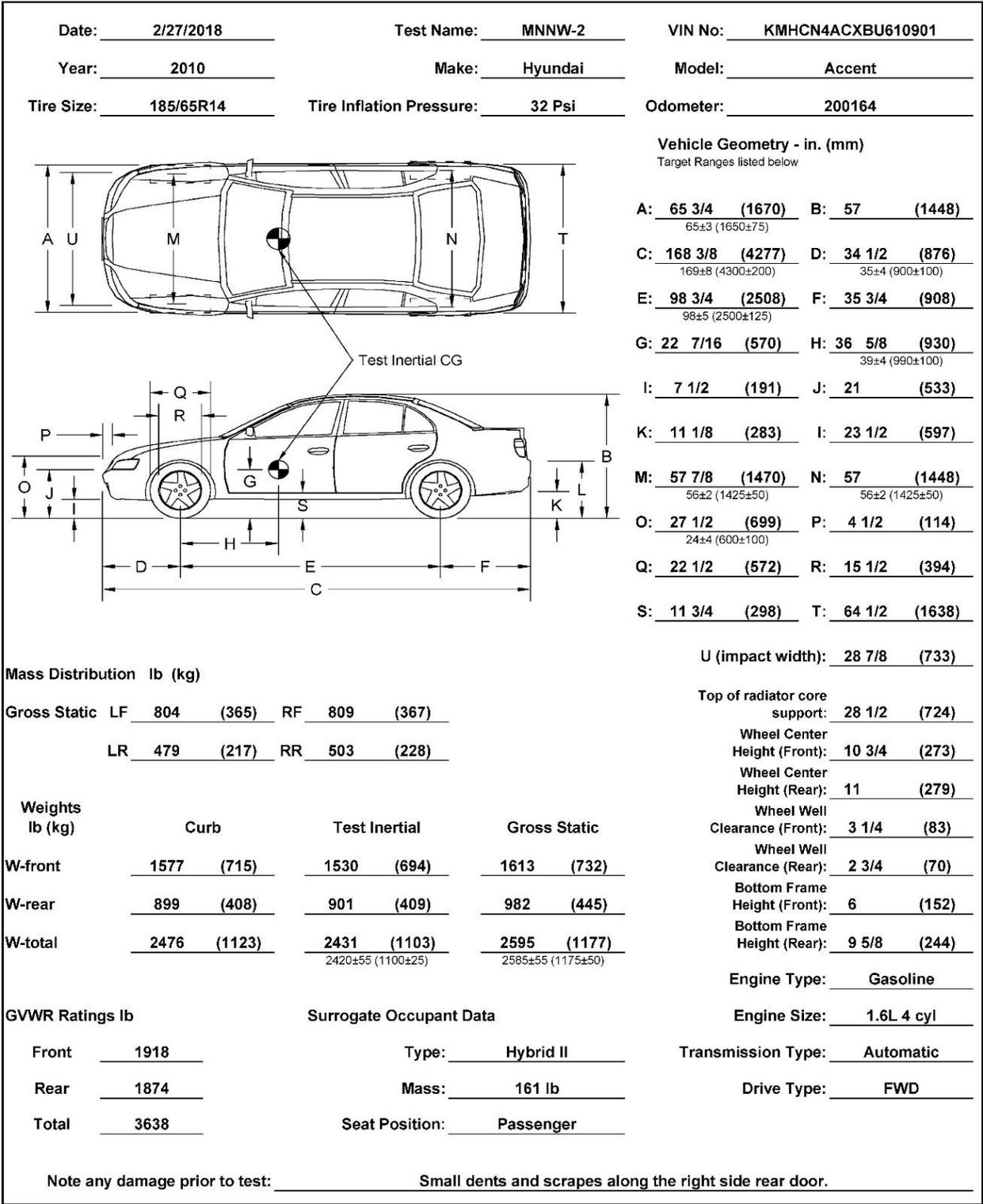
Figure 7. Vehicle Dimensions, Test No. MNNW-2
