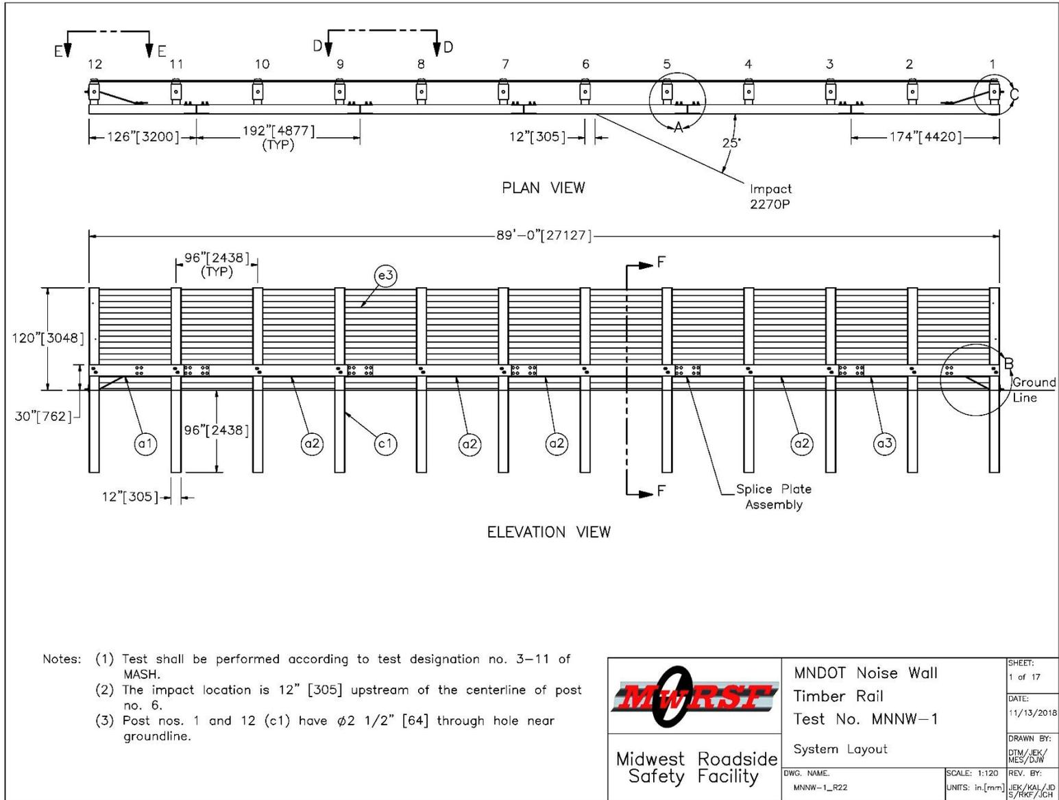
Figure 17. System Layout, Test No. MNNW-1 (Recommended updates provided in Chapter 12)
