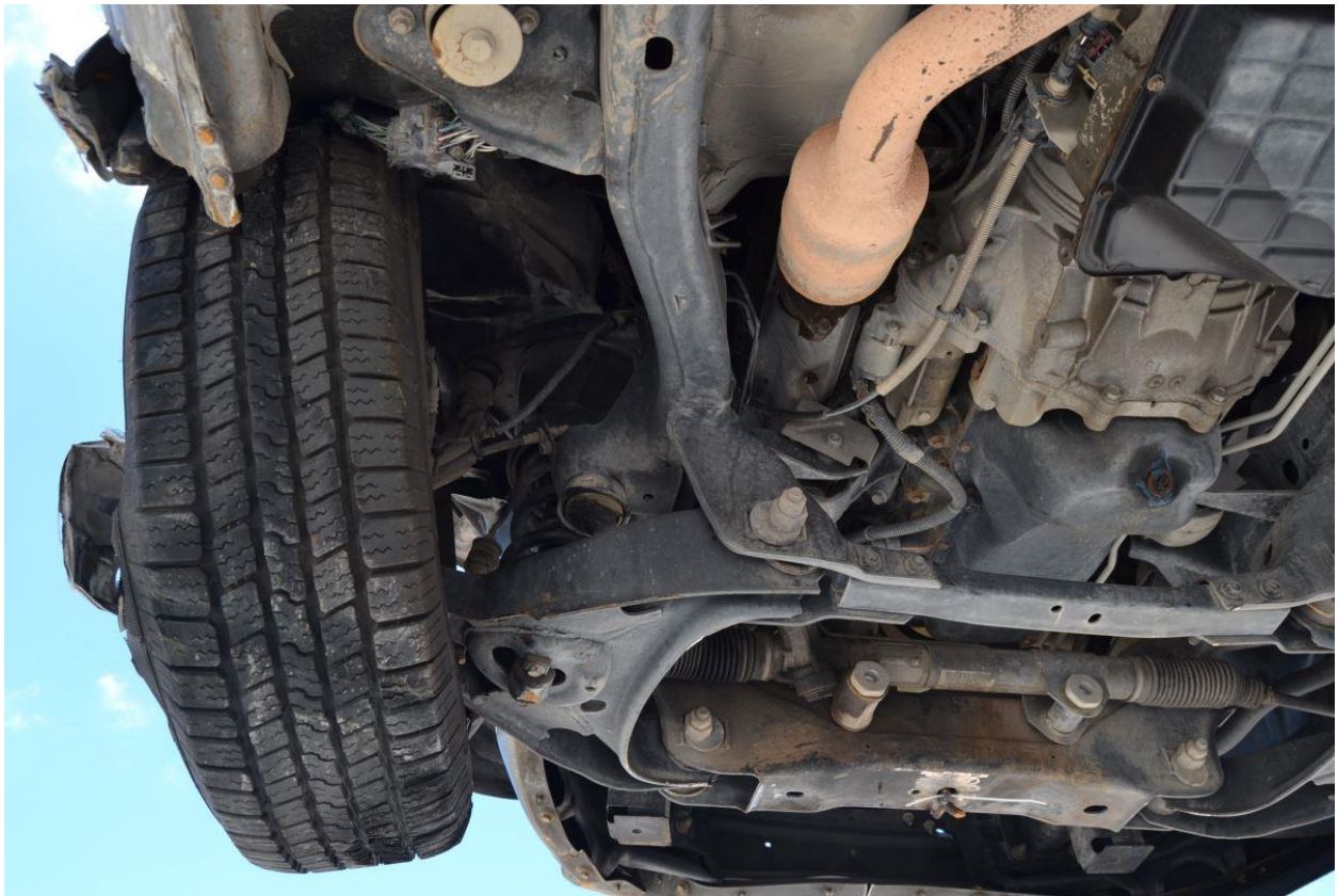
Figure 43. Undercarriage Damage, Test No. NJPCB-7
