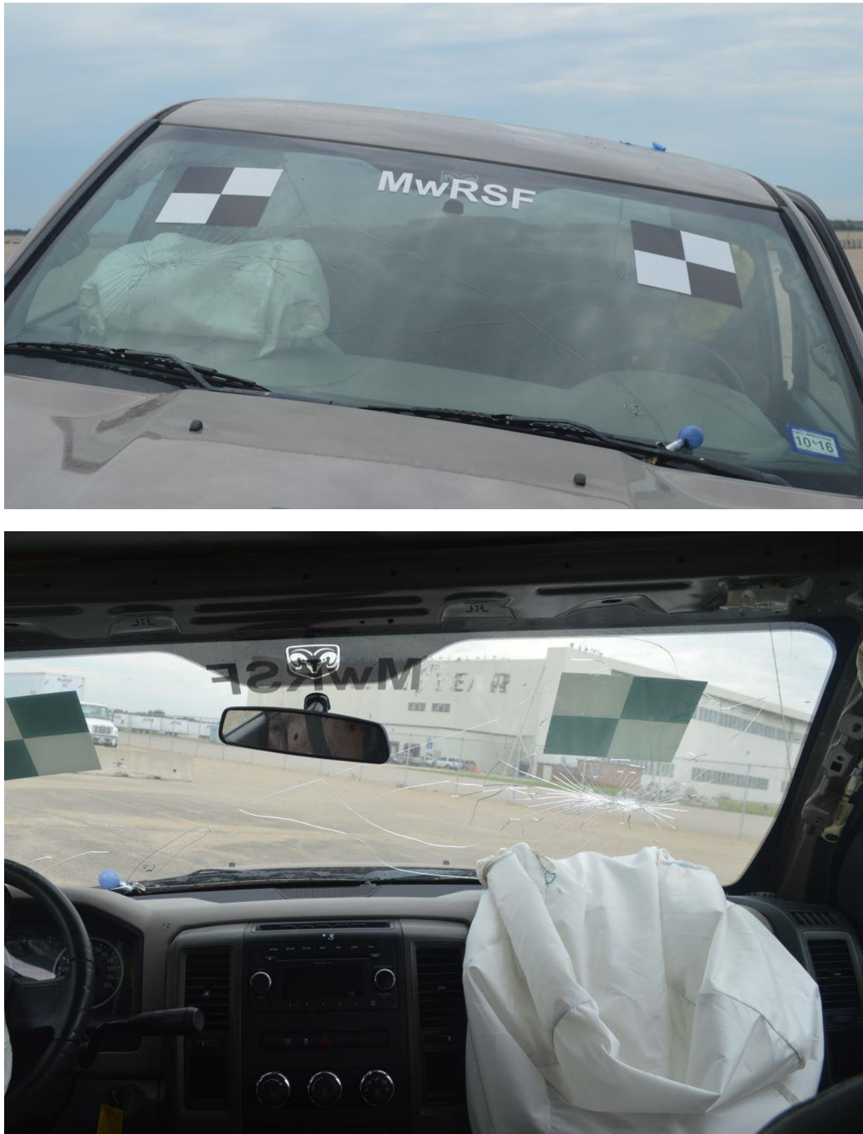
Figure 41. Vehicle Windshield Damage, Test No. NJPCB-7
