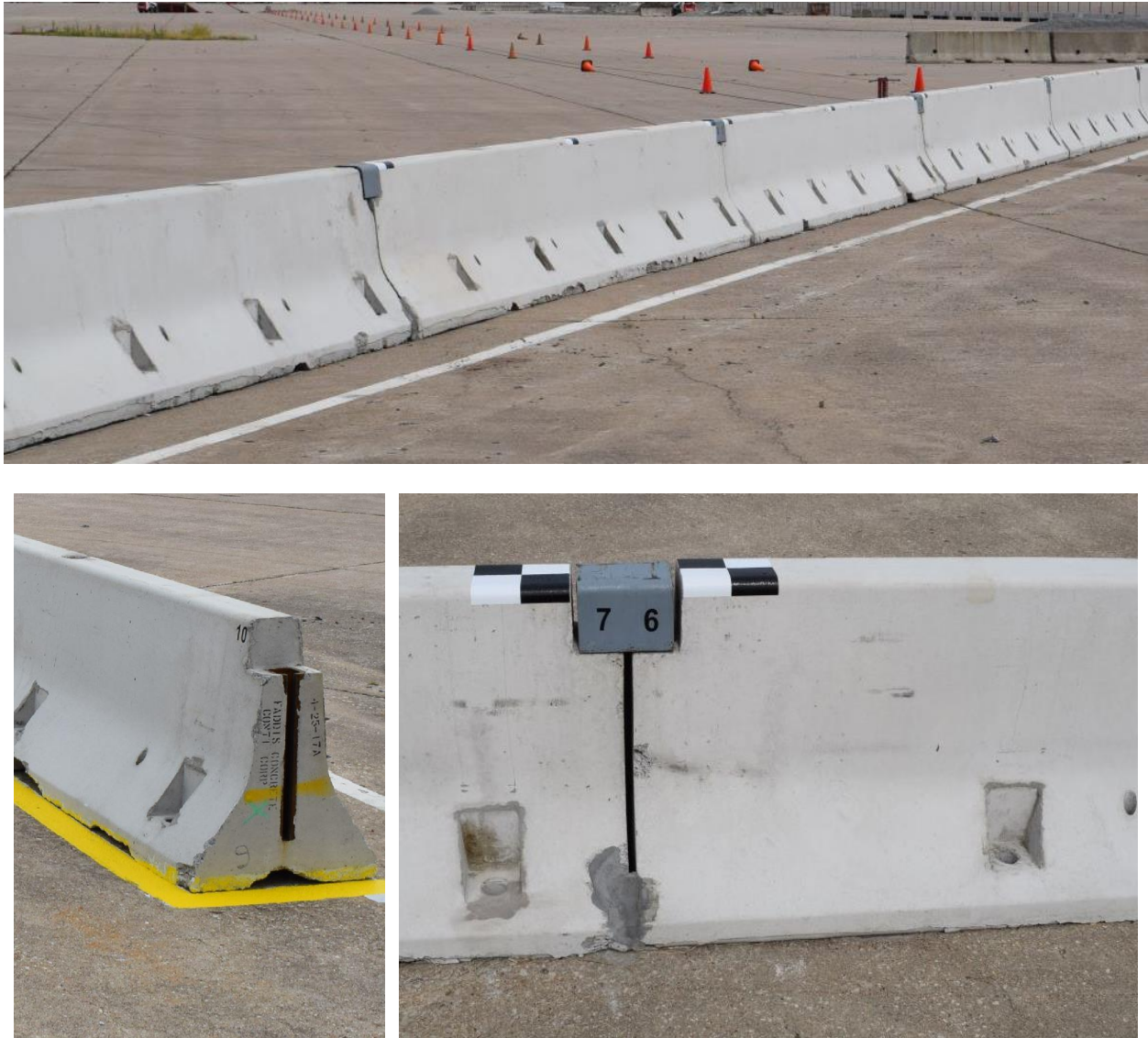
Figure 16. PCB Connection Key and Connection Socket, Test No. NJPCB-7
