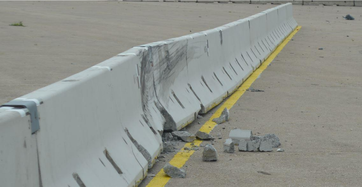
Figure 35. Barrier Nos. 4 and 5 Damage, Test No. NJPCB-7
