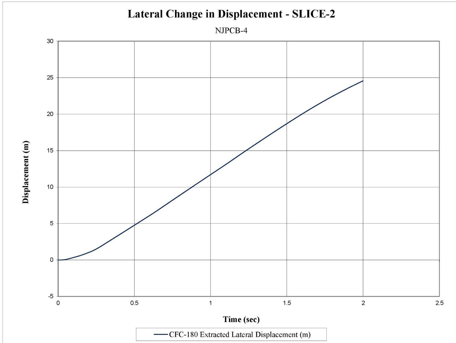
Figure F-14. Lateral Occupant Displacement (SLICE-2), Test No. NJPCB-4
