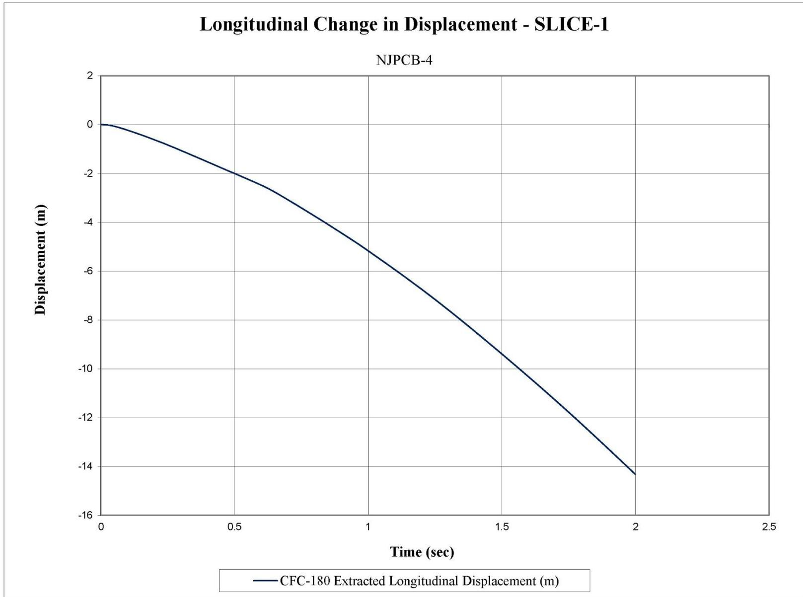
Figure F-3. Longitudinal Occupant Displacement (SLICE-1), Test No. NJPCB-4
