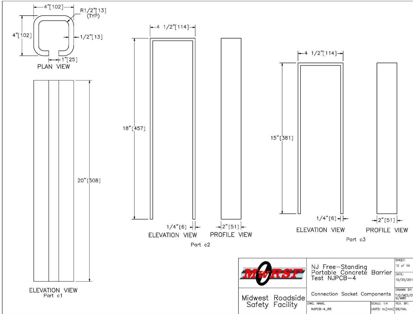
Figure 10. PCB Connection Socket Component Details, Test No. NJPCB-4
