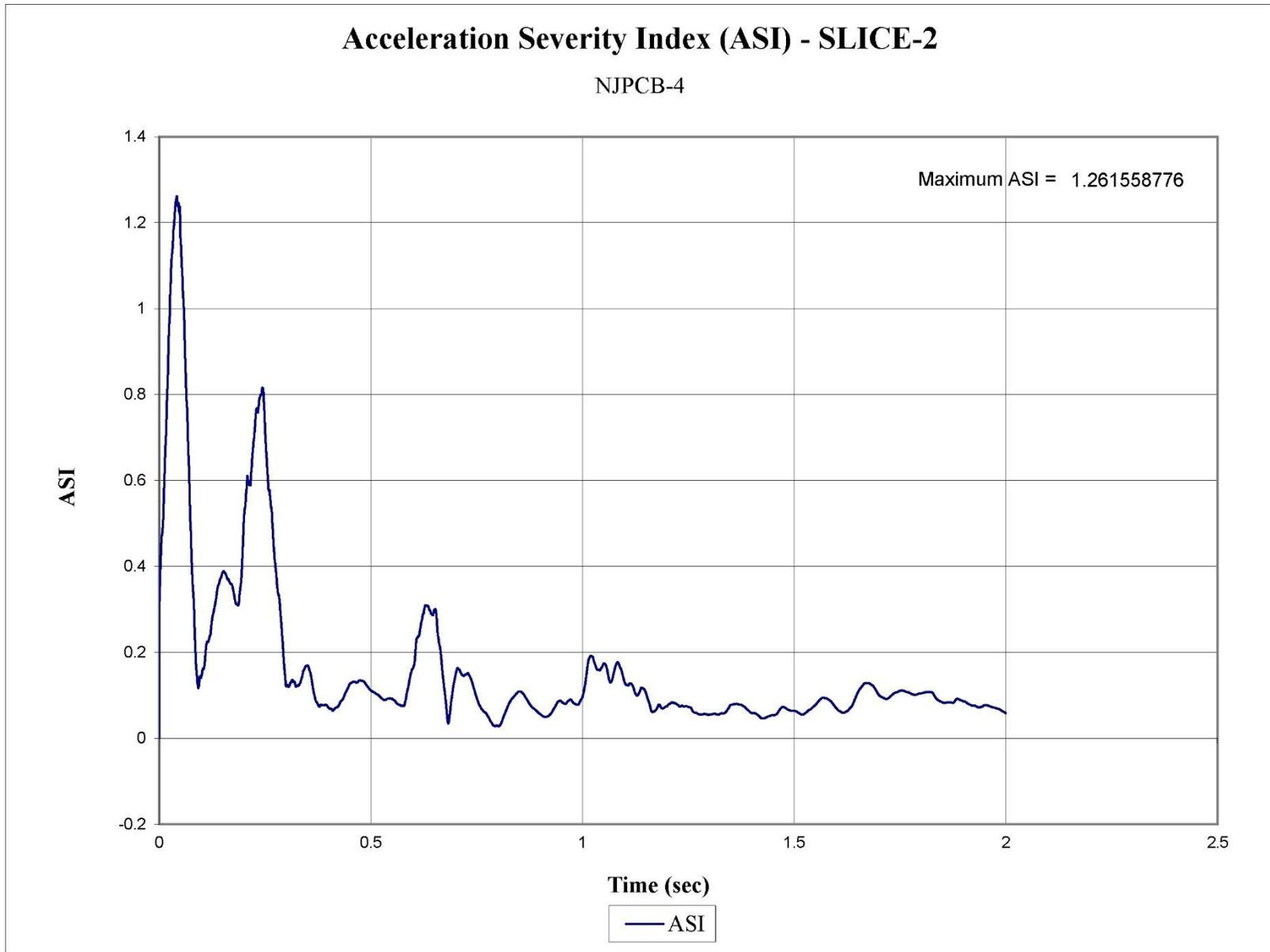
Figure F-16. Acceleration Severity Index (SLICE-2), Test No. NJPCB-4
