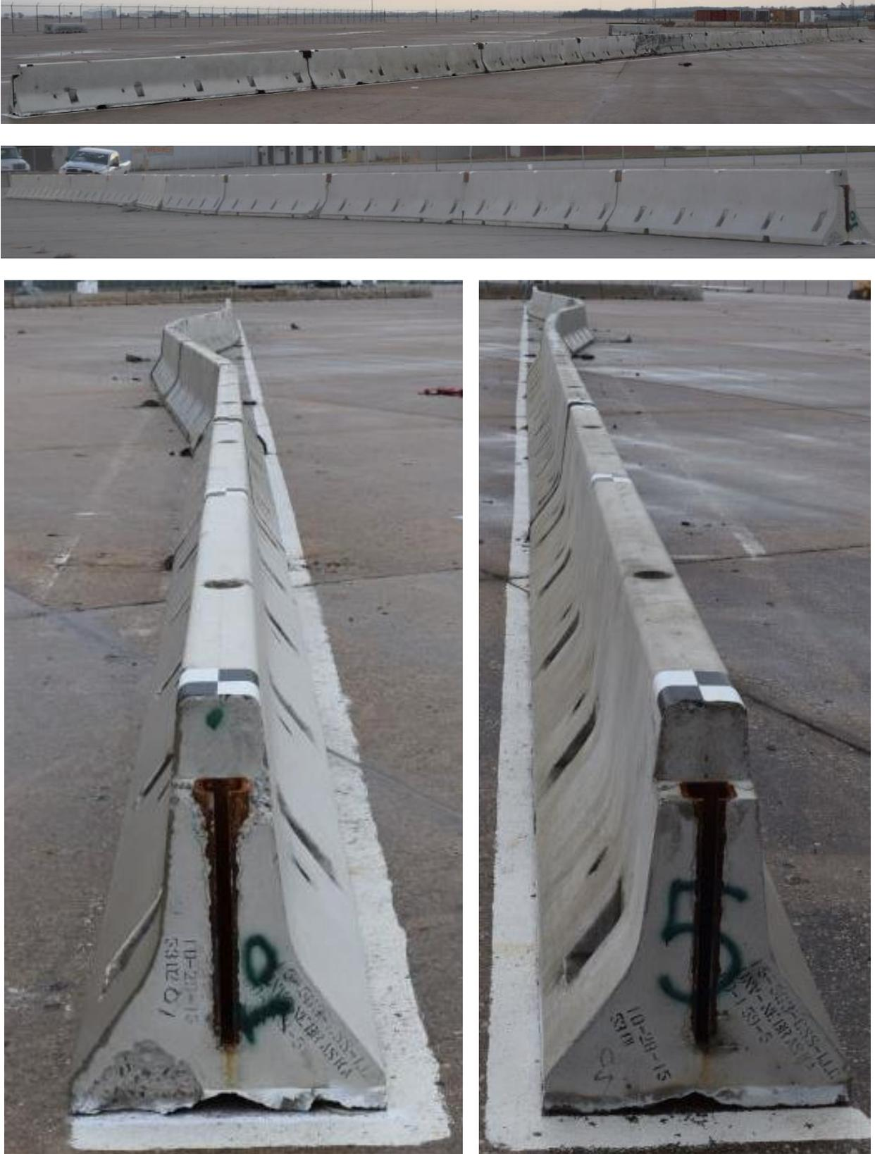
Figure 30. System Damage – Front, Back, Upstream, and Downstream End, Test No. NJPCB-4
