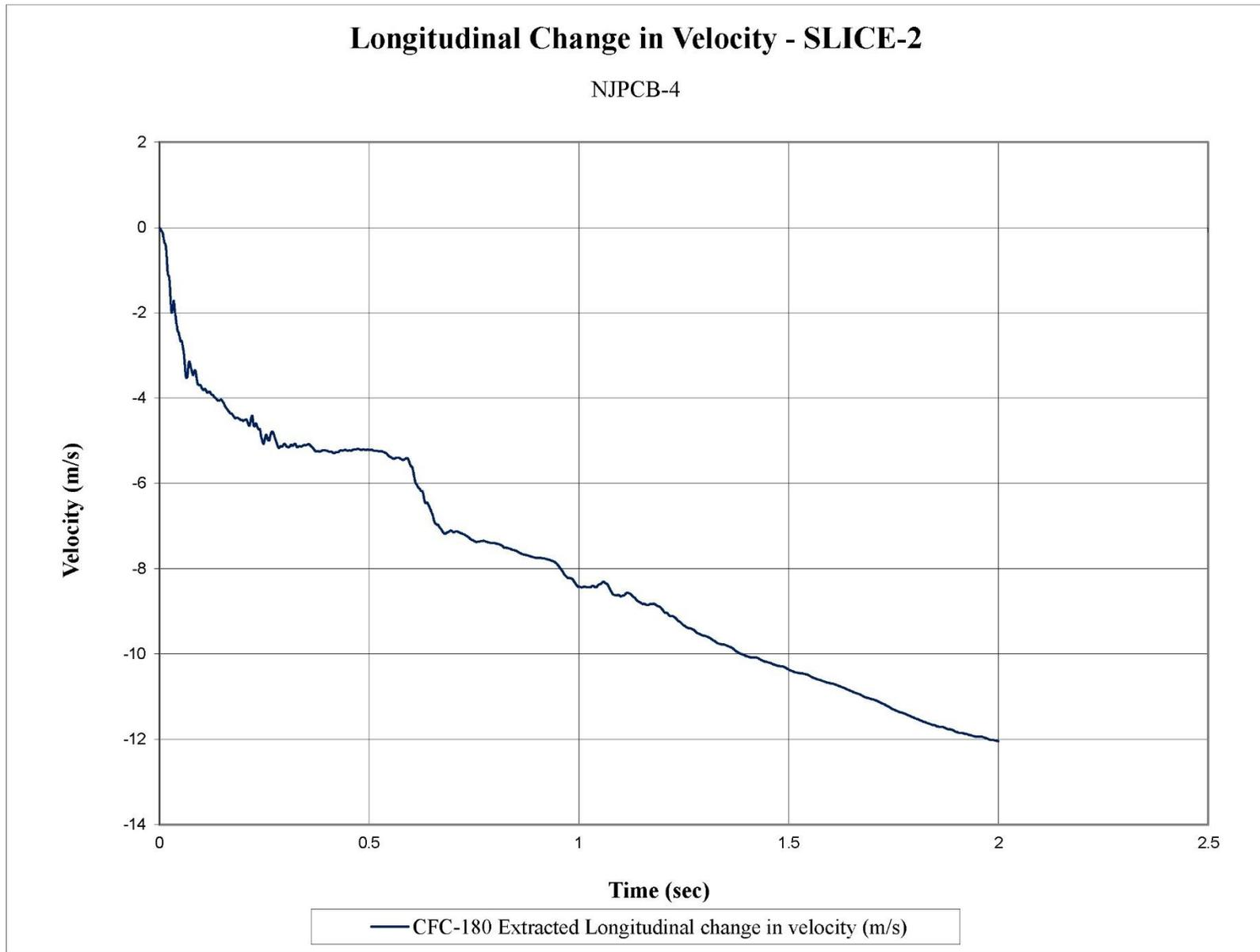
Figure F-10. Longitudinal Occupant Impact Velocity (SLICE-2), Test No. NJPCB-4
