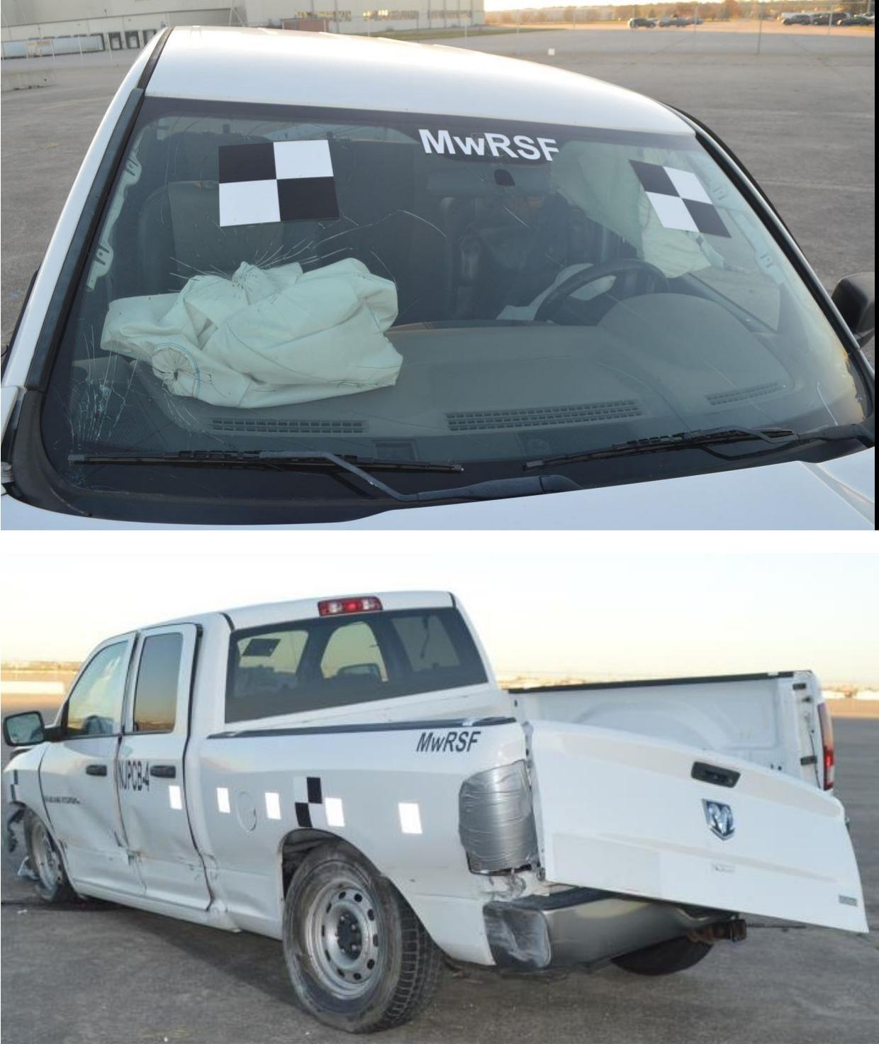
Figure 39. Vehicle Windshield, Quarter Panel, and Tailgate Damage, Test No. NJPCB-4
