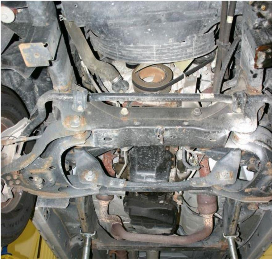
Figure 41. Undercarriage Damage, Test No. NJPCB-4
