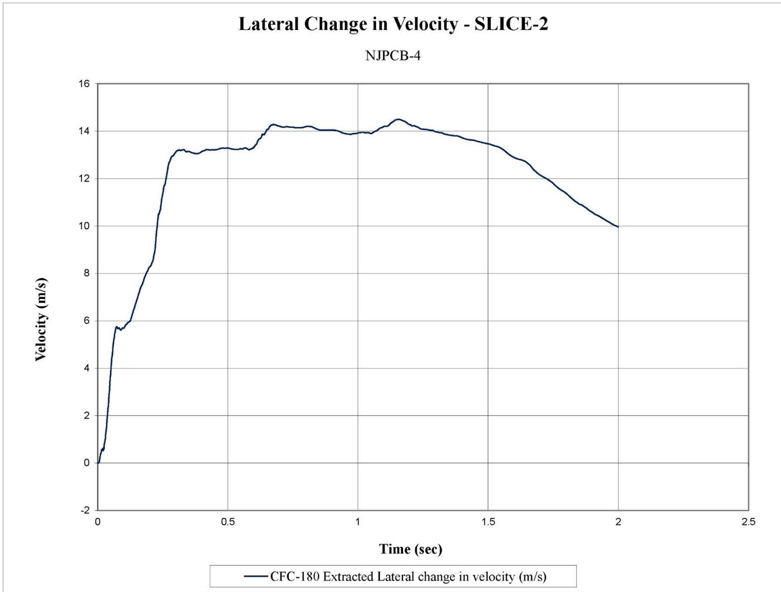
Figure F-13. Lateral Occupant Impact Velocity (SLICE-2), Test No. NJPCB-4
