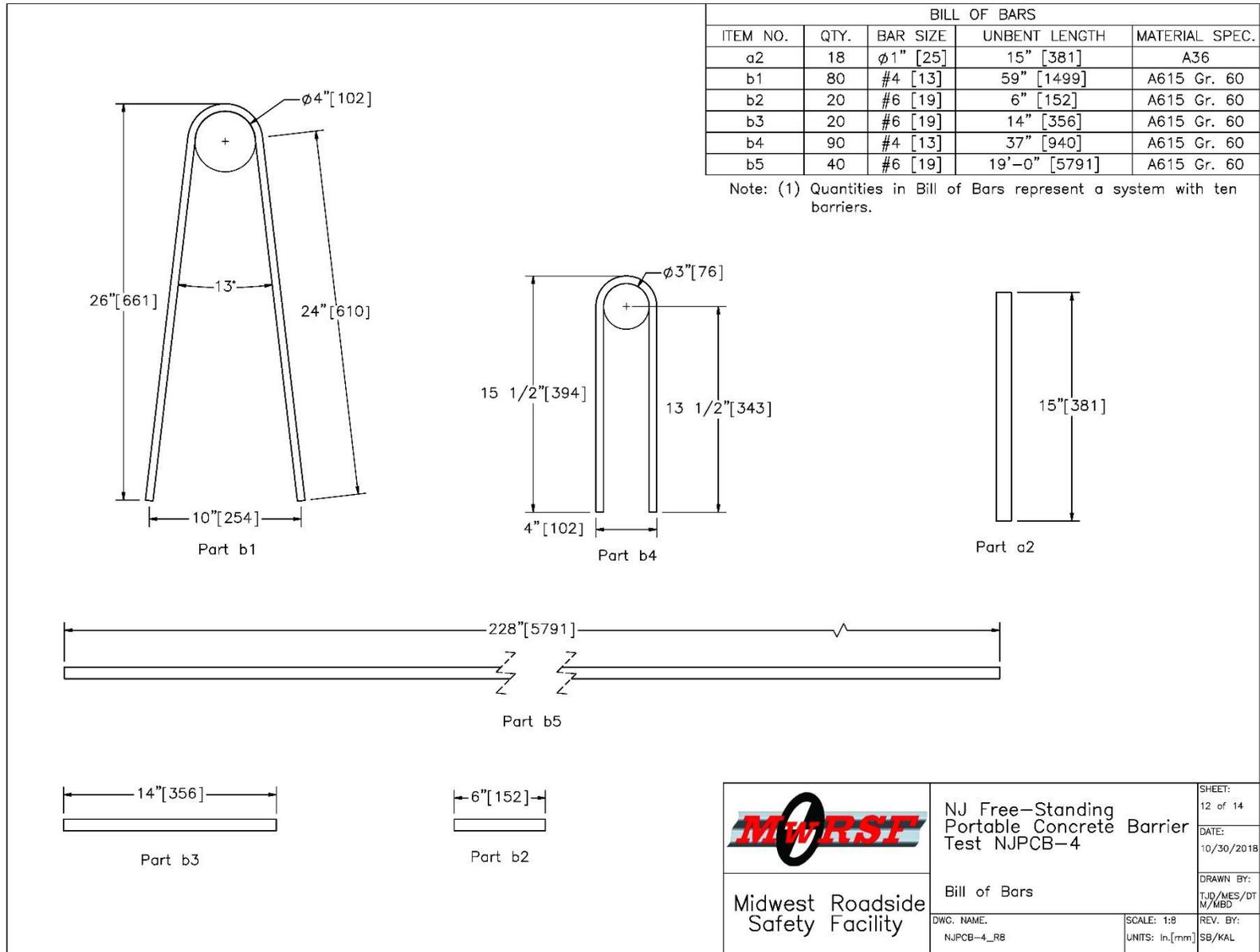
Figure 12. PCB Reinforcement Details, Test No. NJPCB-4
