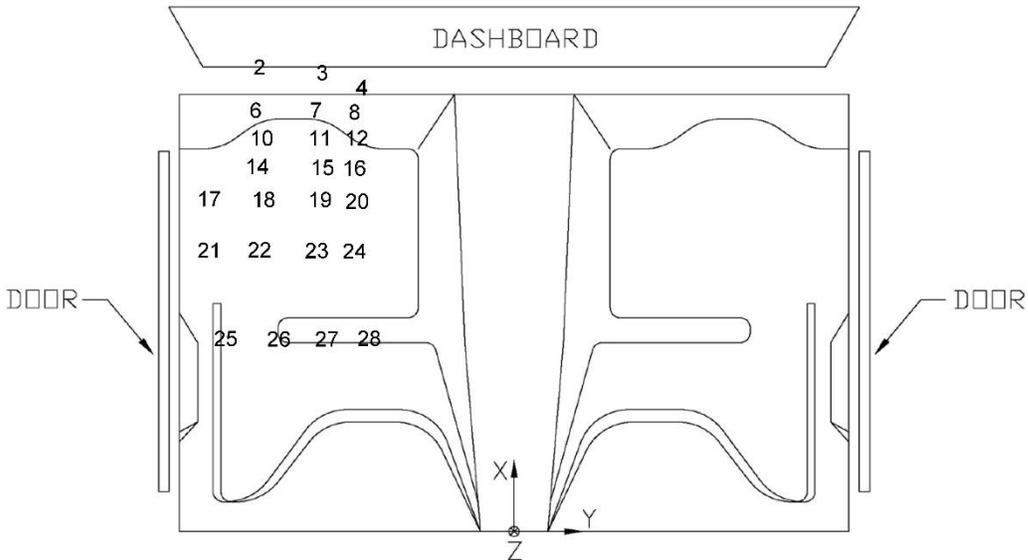
Figure E-2. Floor Pan Deformation Data – Set 2, Test No. NJPCB-4
