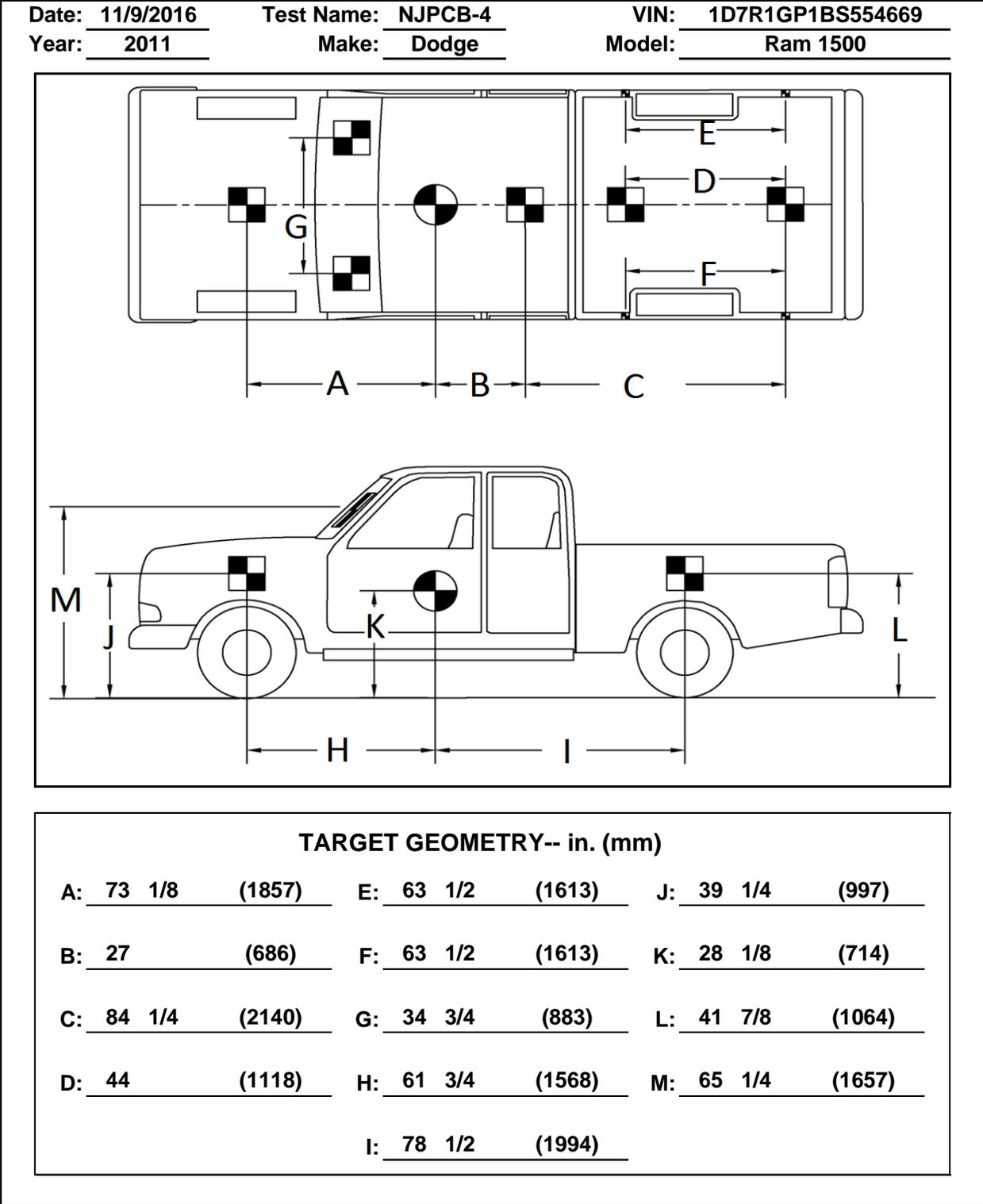
Figure 21. Target Geometry, Test No. NJPCB-4
