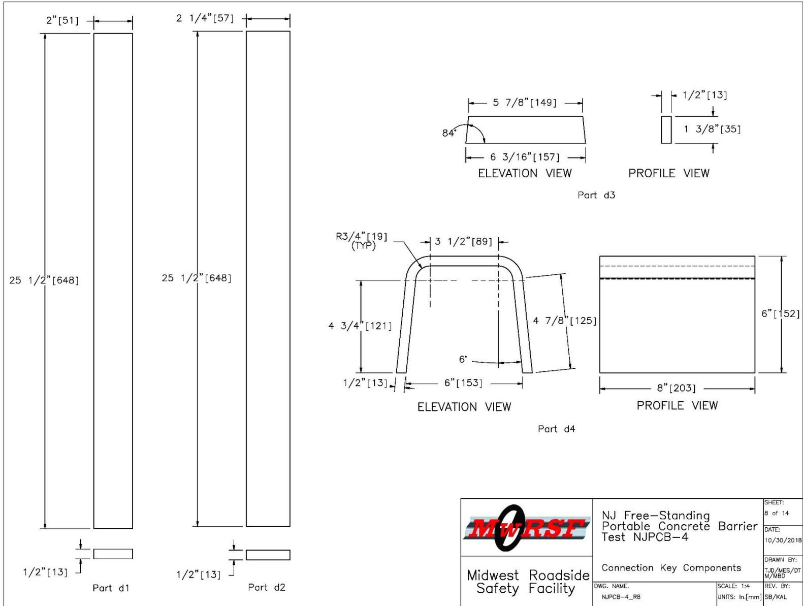
Figure 8. Connection Key Component Details, Test No. NJPCB-4
