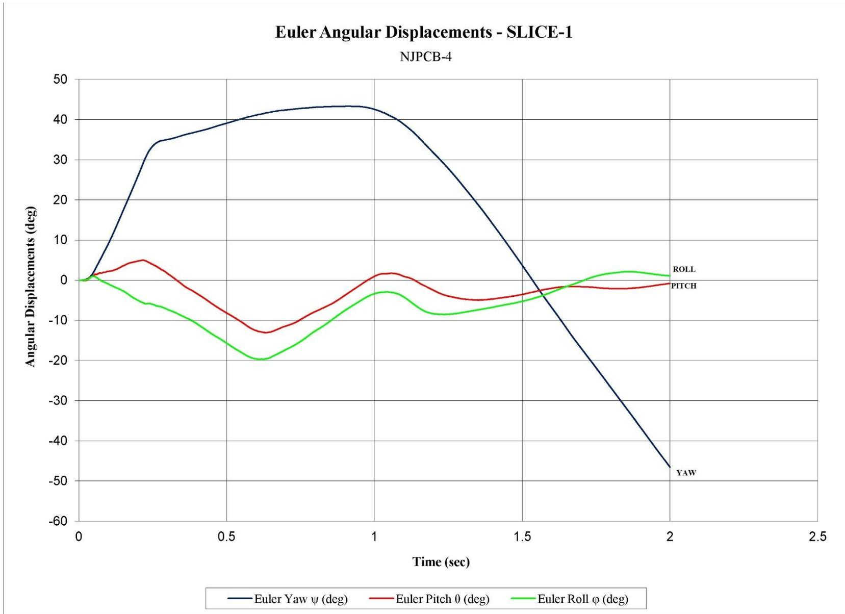
Figure F-7. Vehicle Angular Displacements (SLICE-1), Test No. NJPCB-4
