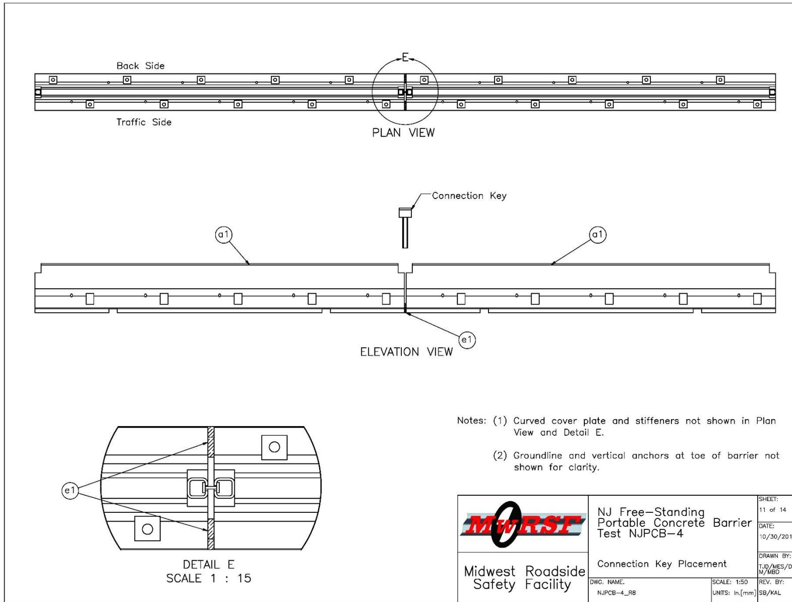
Figure 11. Connection Key Placement Details, Test No. NJPCB-4
