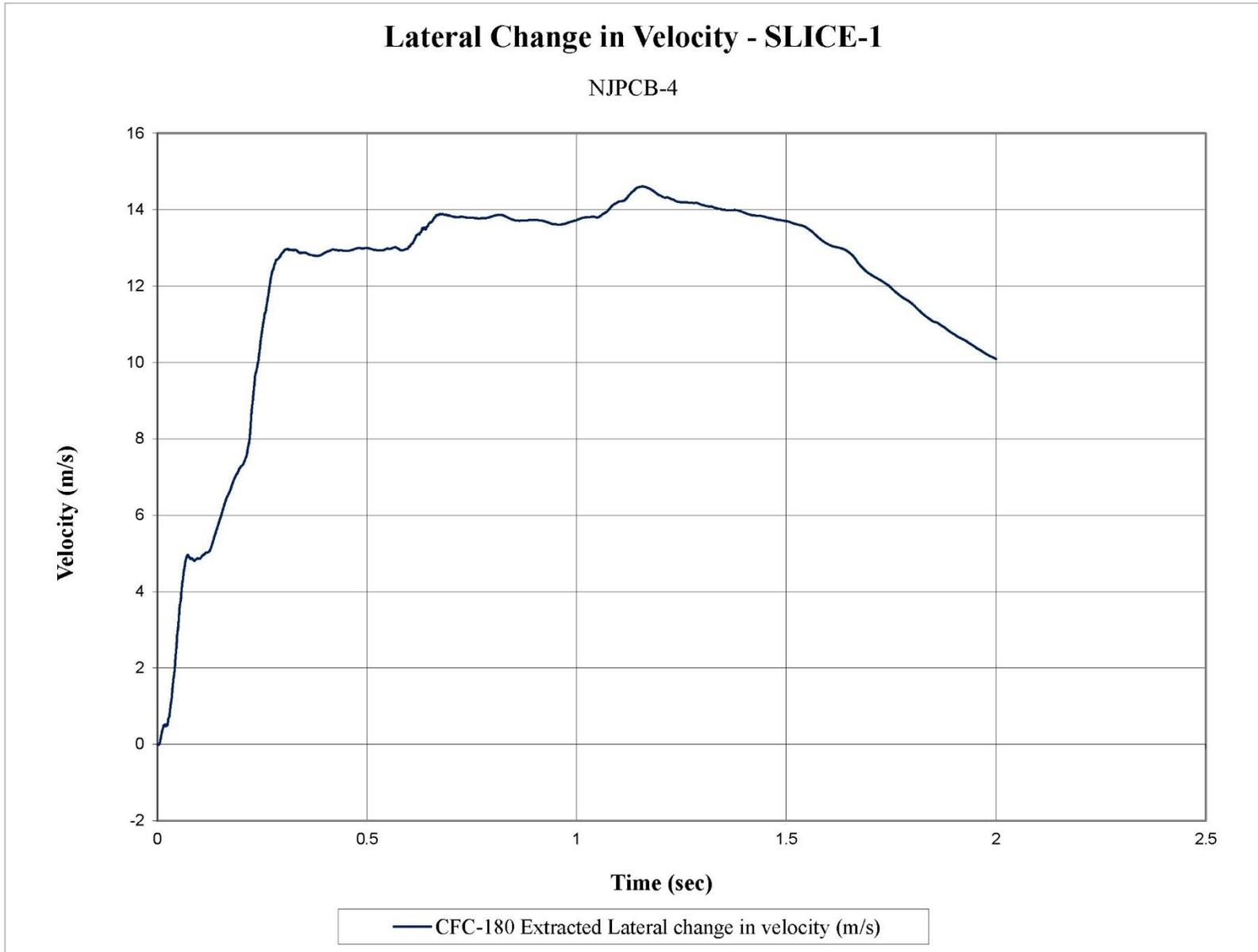
Figure F-5. Lateral Occupant Impact Velocity (SLICE-1), Test No. NJPCB-4
