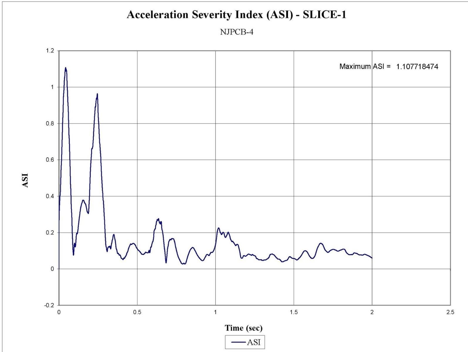
Figure F-8. Acceleration Severity Index (SLICE-1), Test No. NJPCB-4
