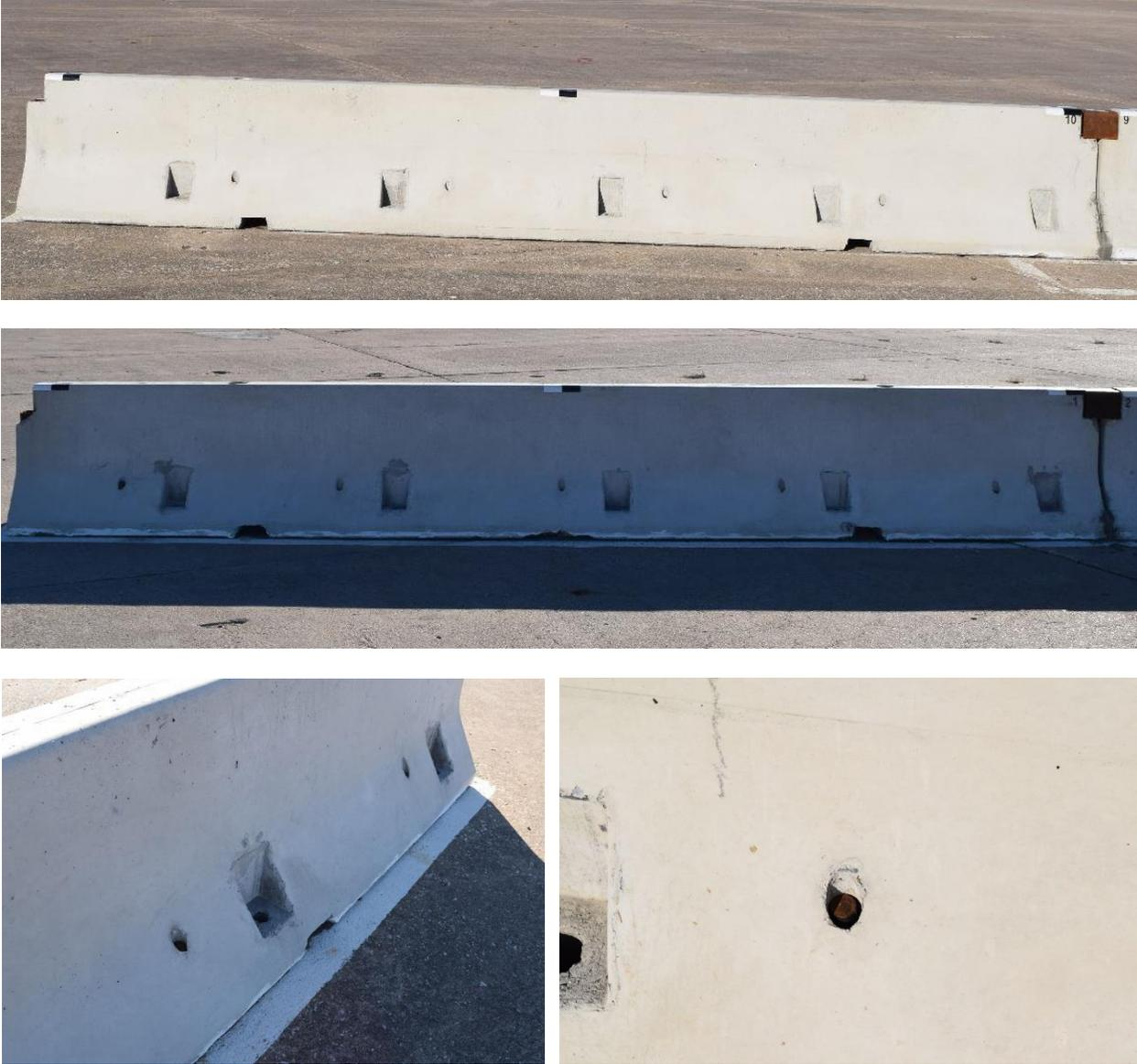
Figure 17. PCB Pin Anchor Recesses – Barrier Nos. 1 and 10, Test No. NJPCB-4
