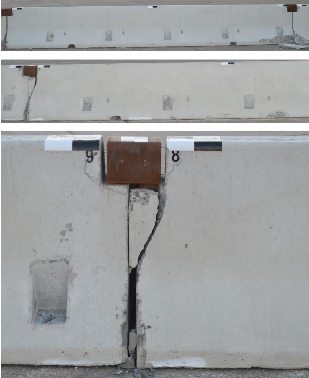
Figure 36. Barrier Nos. 7 and 8 – Back Side Damage, Test No. NJPCB-4
