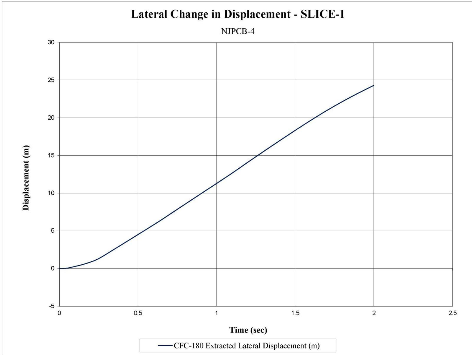
Figure F-6. Lateral Occupant Displacement (SLICE-1), Test No. NJPCB-4
