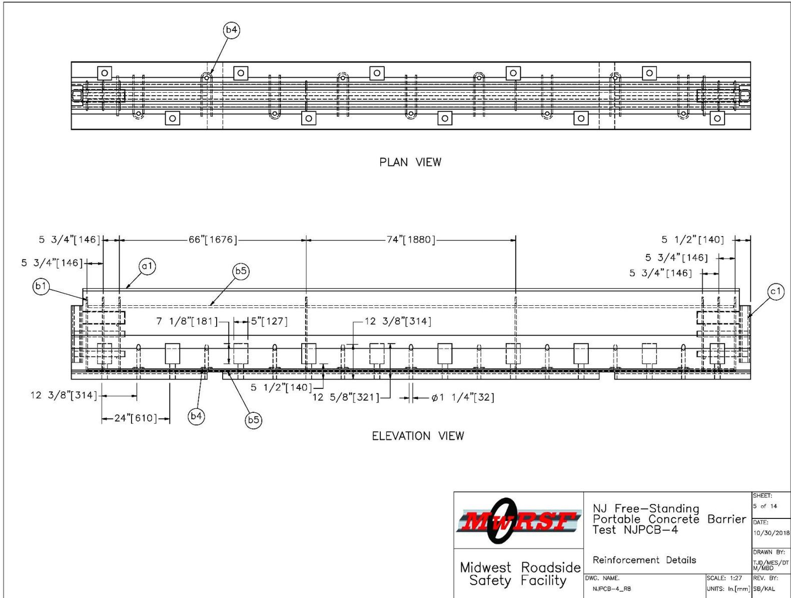
Figure 5. PCB Reinforcement Details, Test No. NJPCB-4
