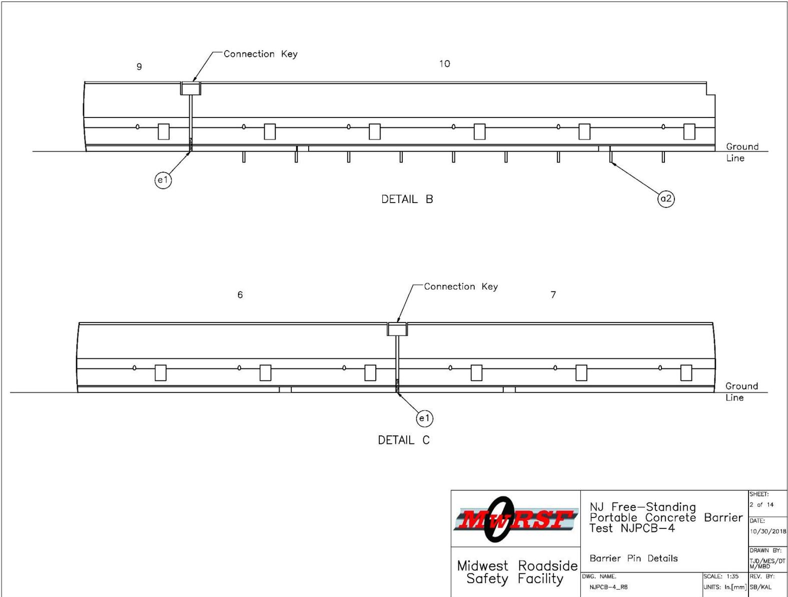
Figure 2. PCB Pin Anchor Details, Test No. NJPCB-4
