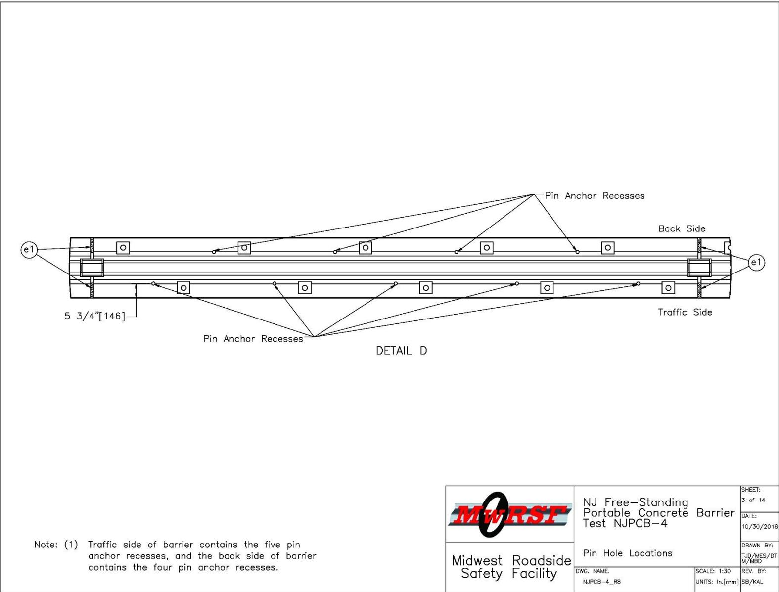
Figure 3. PCB Pin Anchor Recess Locations, Test No. NJPCB-4
