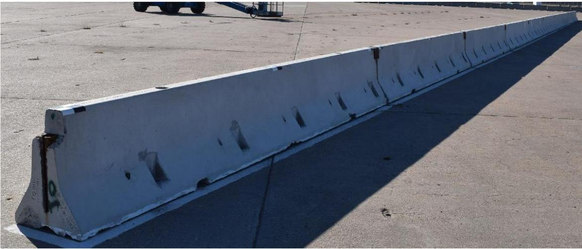
Figure 15. NJDOT PCB with Free-Standing Configuration and Grouted Toes Test Installation, Test No. NJPCB-4
