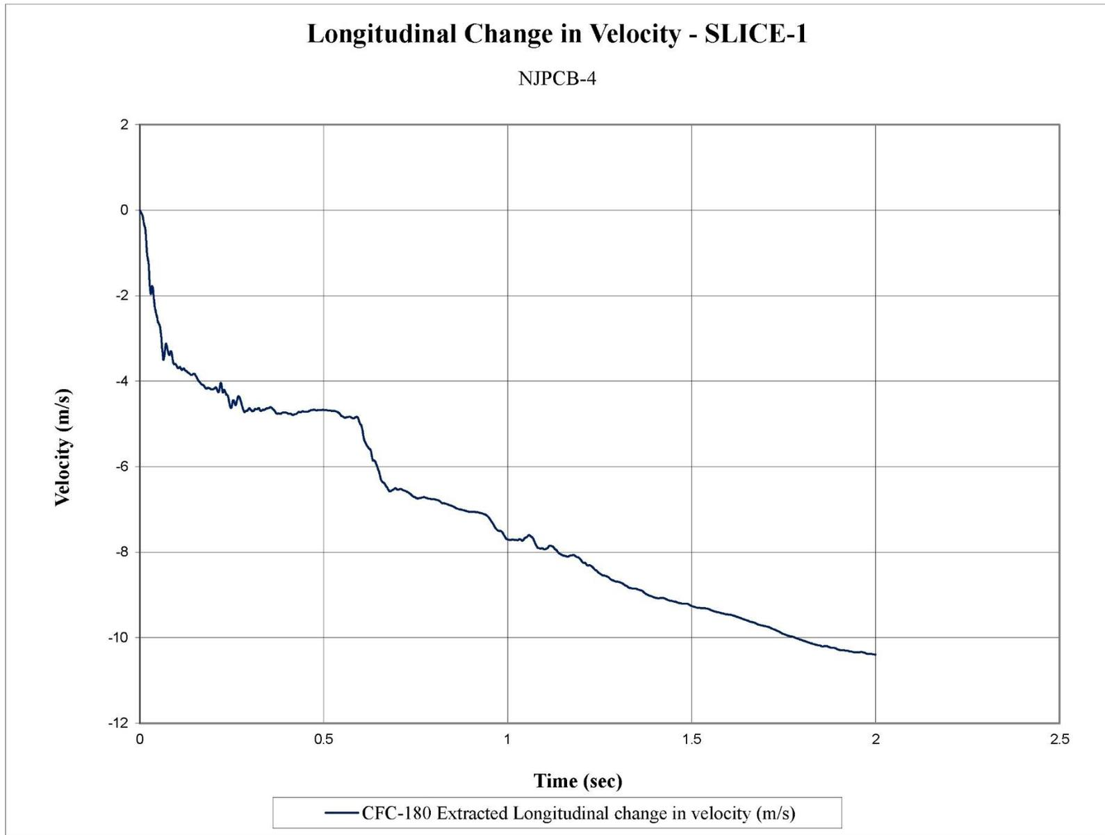
Figure F-2. Longitudinal Occupant Impact Velocity (SLICE-1), Test No. NJPCB-4
