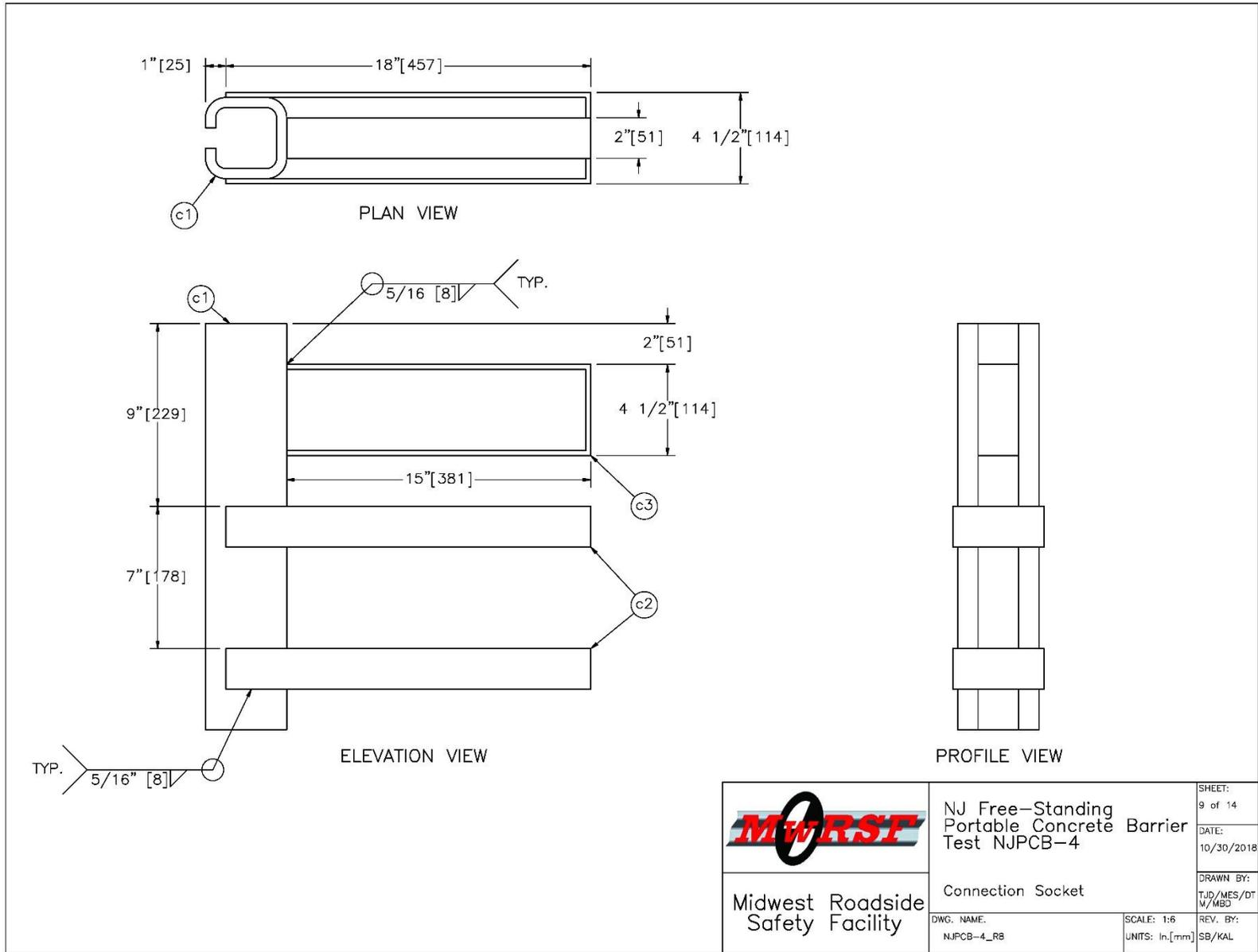
Figure 9. PCB Connection Socket Details, Test No. NJPCB-4
