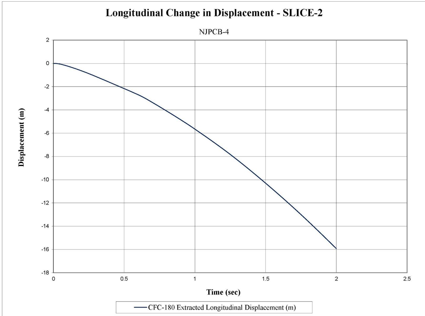
Figure F-11. Longitudinal Occupant Displacement (SLICE-2), Test No. NJPCB-4
