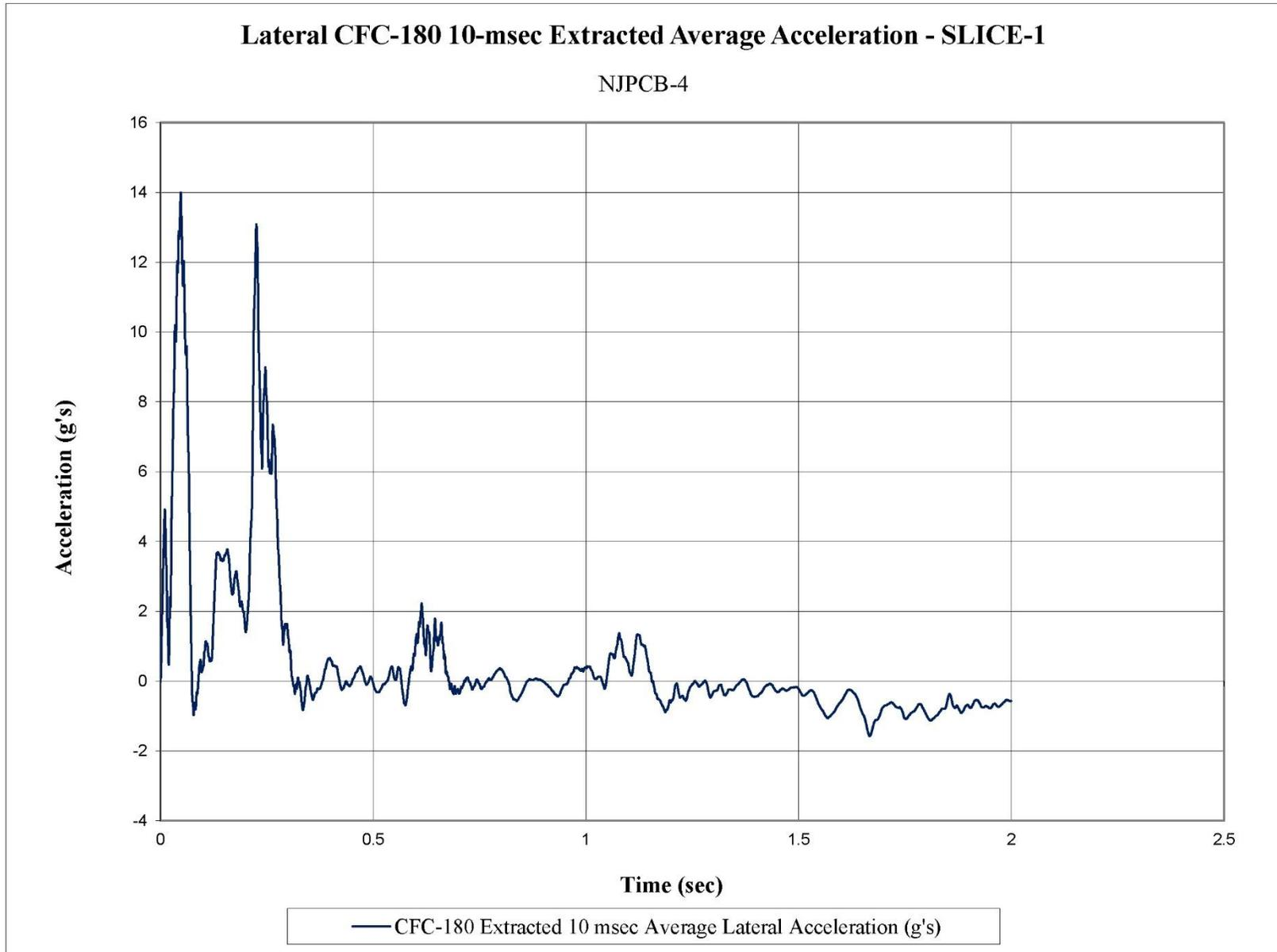
Figure F-4. 10-ms Average Lateral Deceleration (SLICE-1), Test No. NJPCB-4
