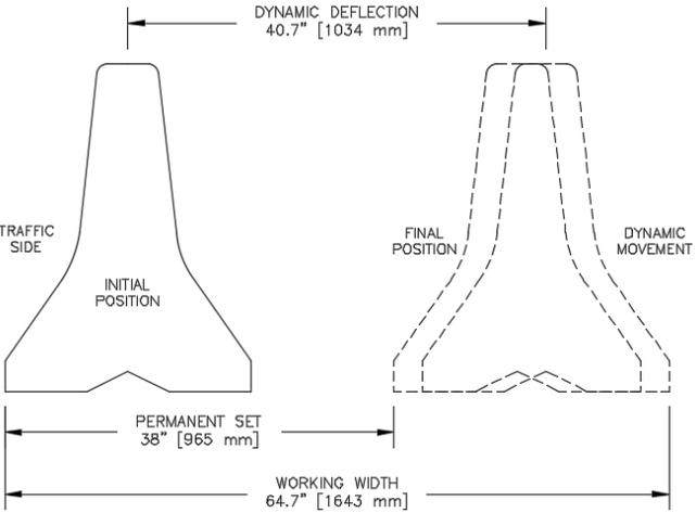
NJPCB-4 – Free-Standing, Joint Slack Removed, Grouted Toes
