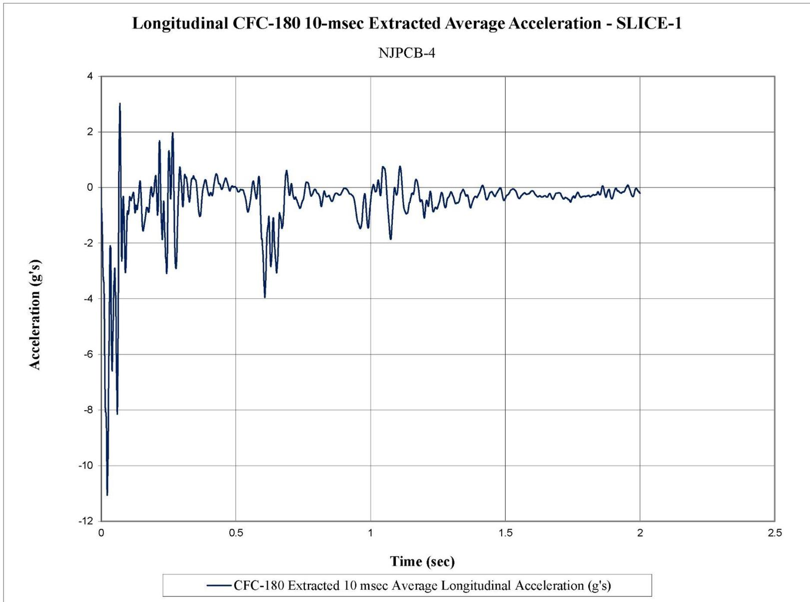
Figure F-1. 10-ms Average Longitudinal Deceleration (SLICE-1), Test No. NJPCB-4
