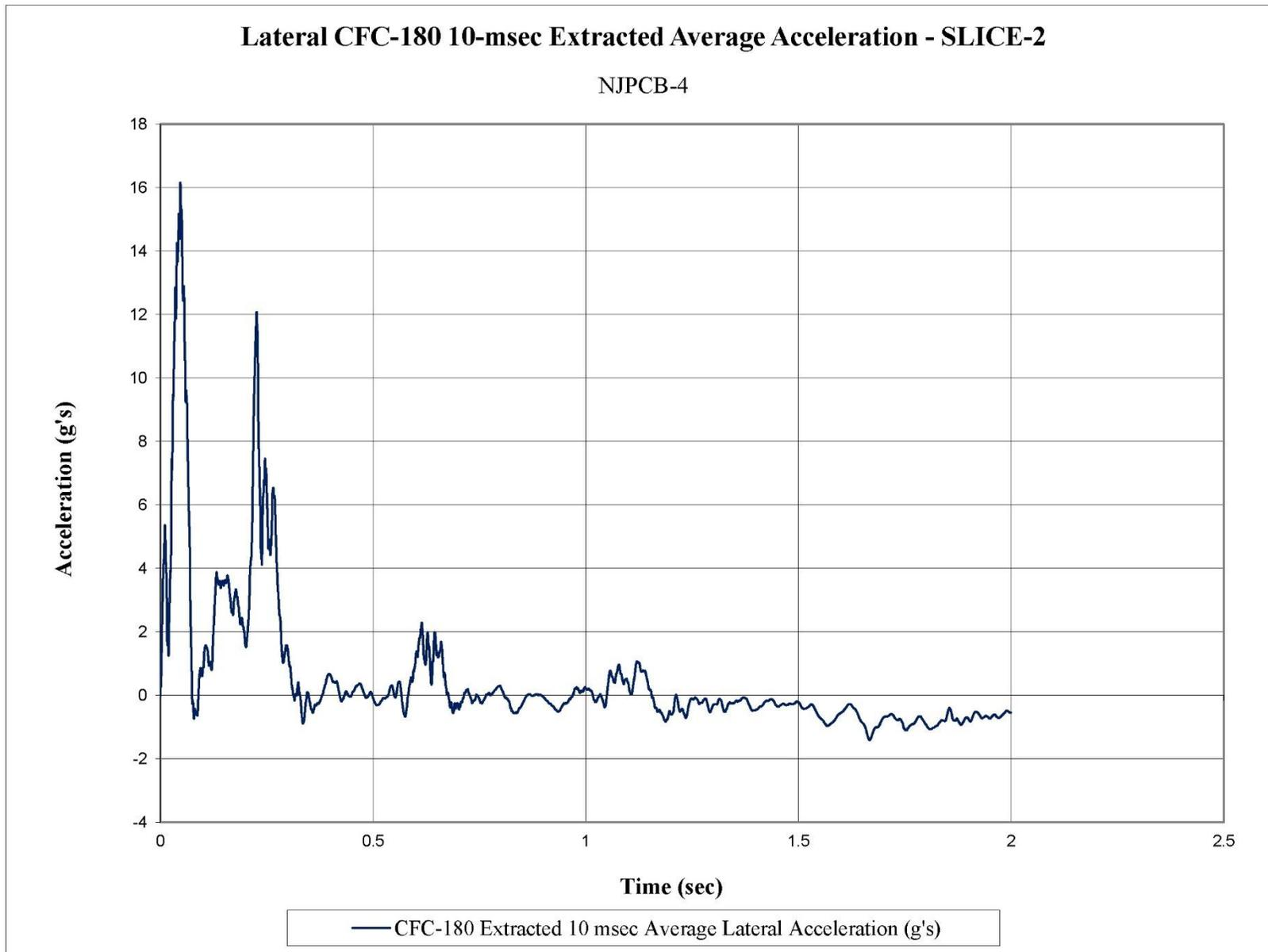
Figure F-12. 10-ms Average Lateral Deceleration (SLICE-2), Test No. NJPCB-4
