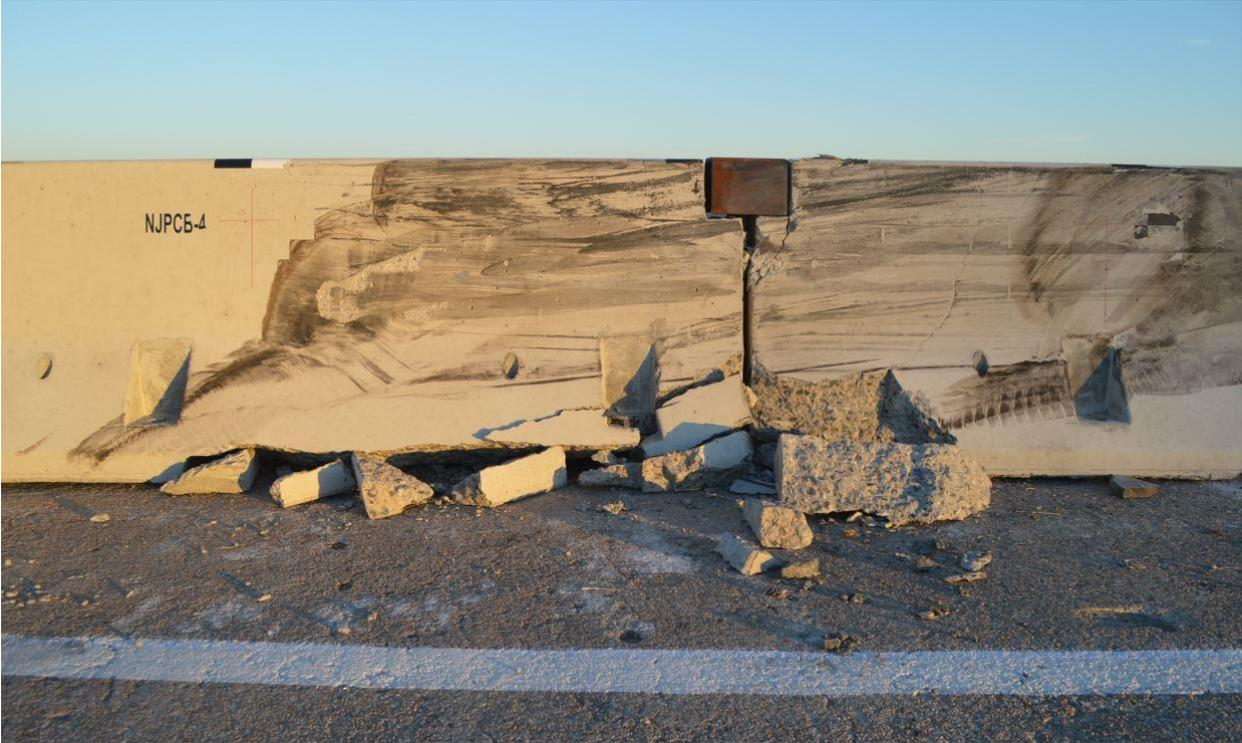
Figure 32. Barrier Nos. 4 and 5 Damage, Test No. NJPCB-4
