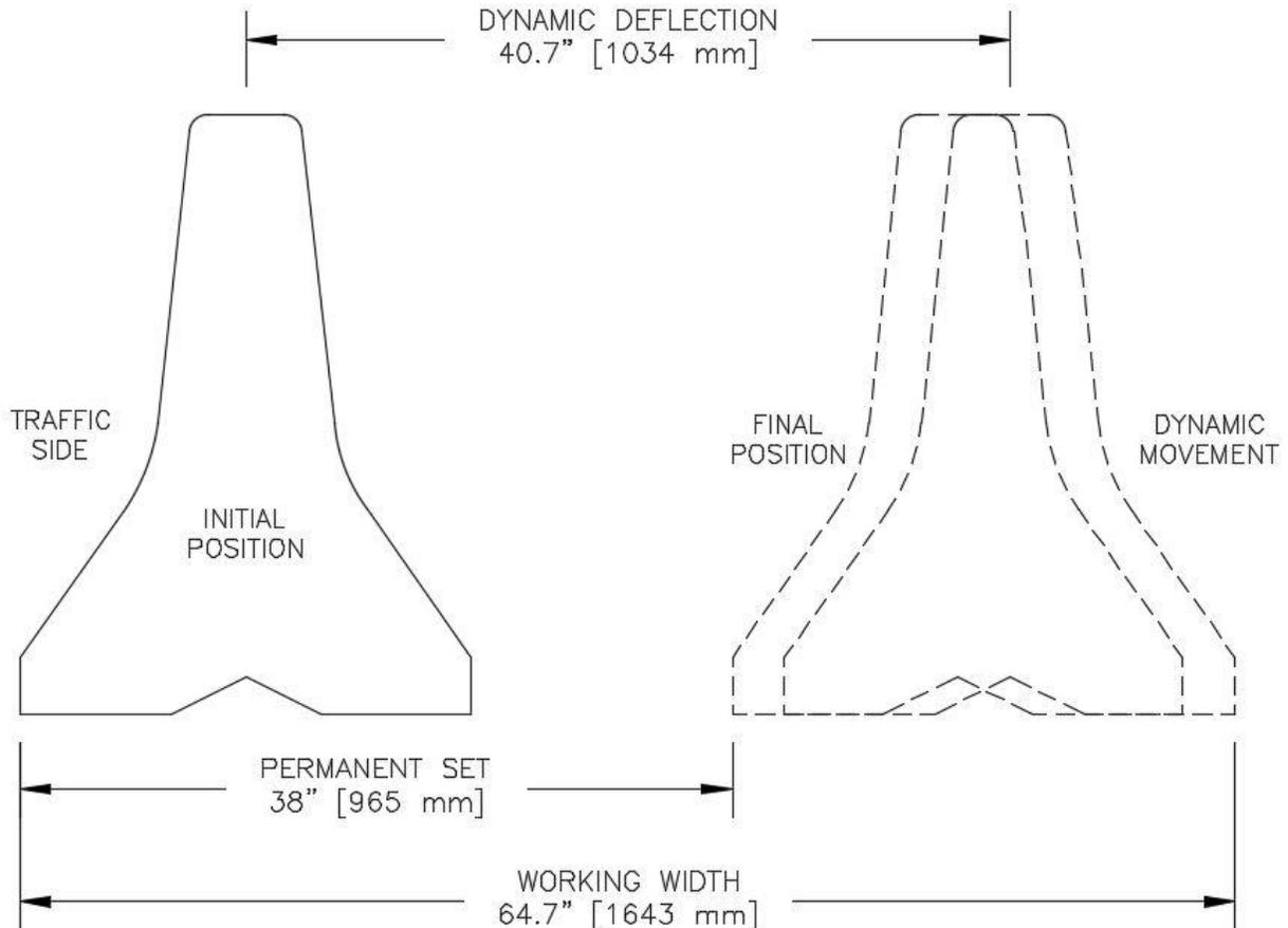
Figure 23. Permanent Set Deflection, Dynamic Deflection, and Working Width, Test No. NJPCB-4
