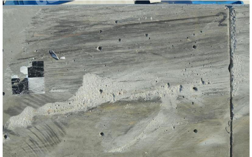
Figure 27. Barrier No. 2 Damage, Test No. OSSB-1
