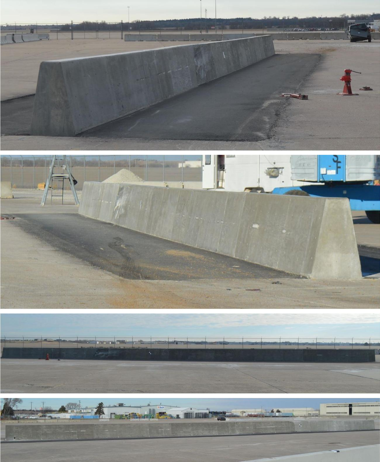
Figure 25. System Damage, Test No. OSSB-1
