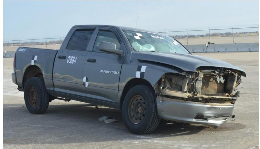
Figure 31. Additional Vehicle Damage, Test No. OSSB-1
