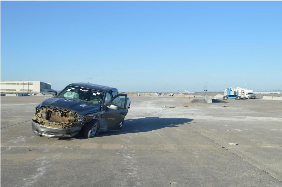
Figure 24. Vehicle Final Position and Trajectory Marks, Test No. OSSB-1
