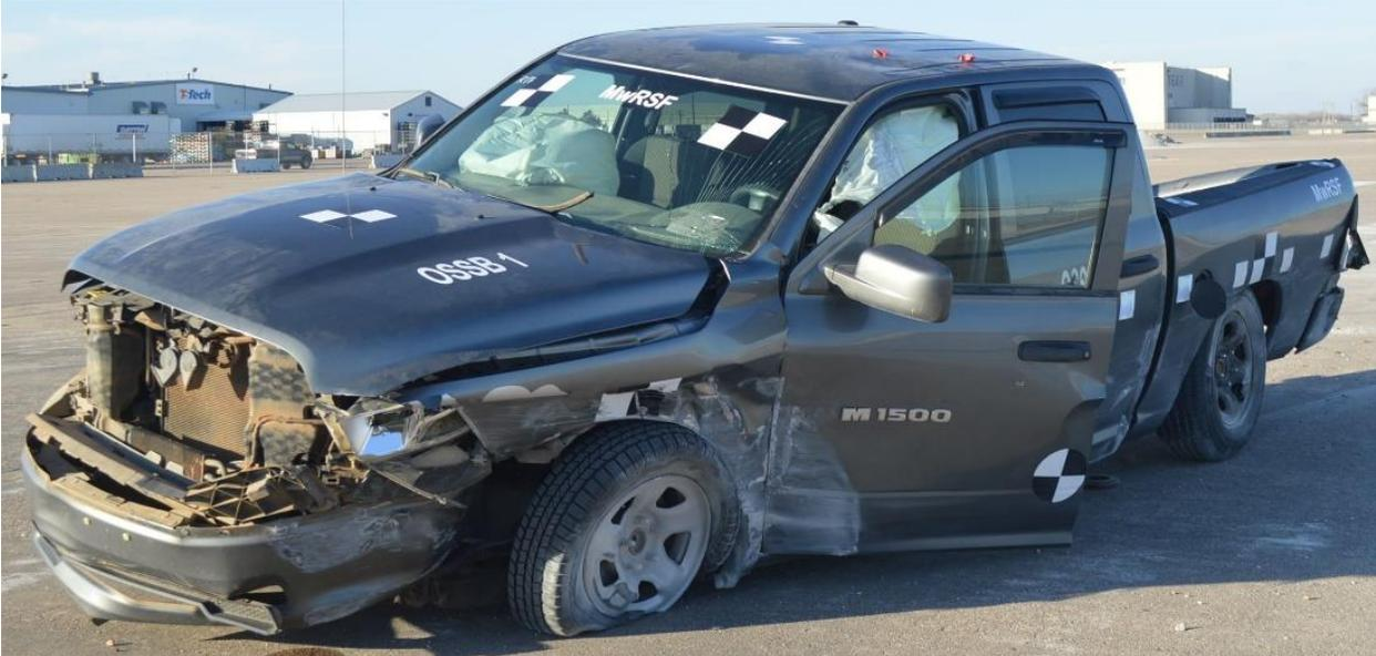
Figure 30. Additional Vehicle Damage, Test No. OSSB-1
