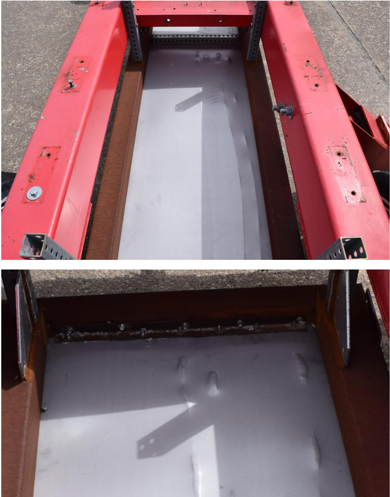
Figure 32. Simulated Floor Pan Damage, Test No. MWPFP-24
