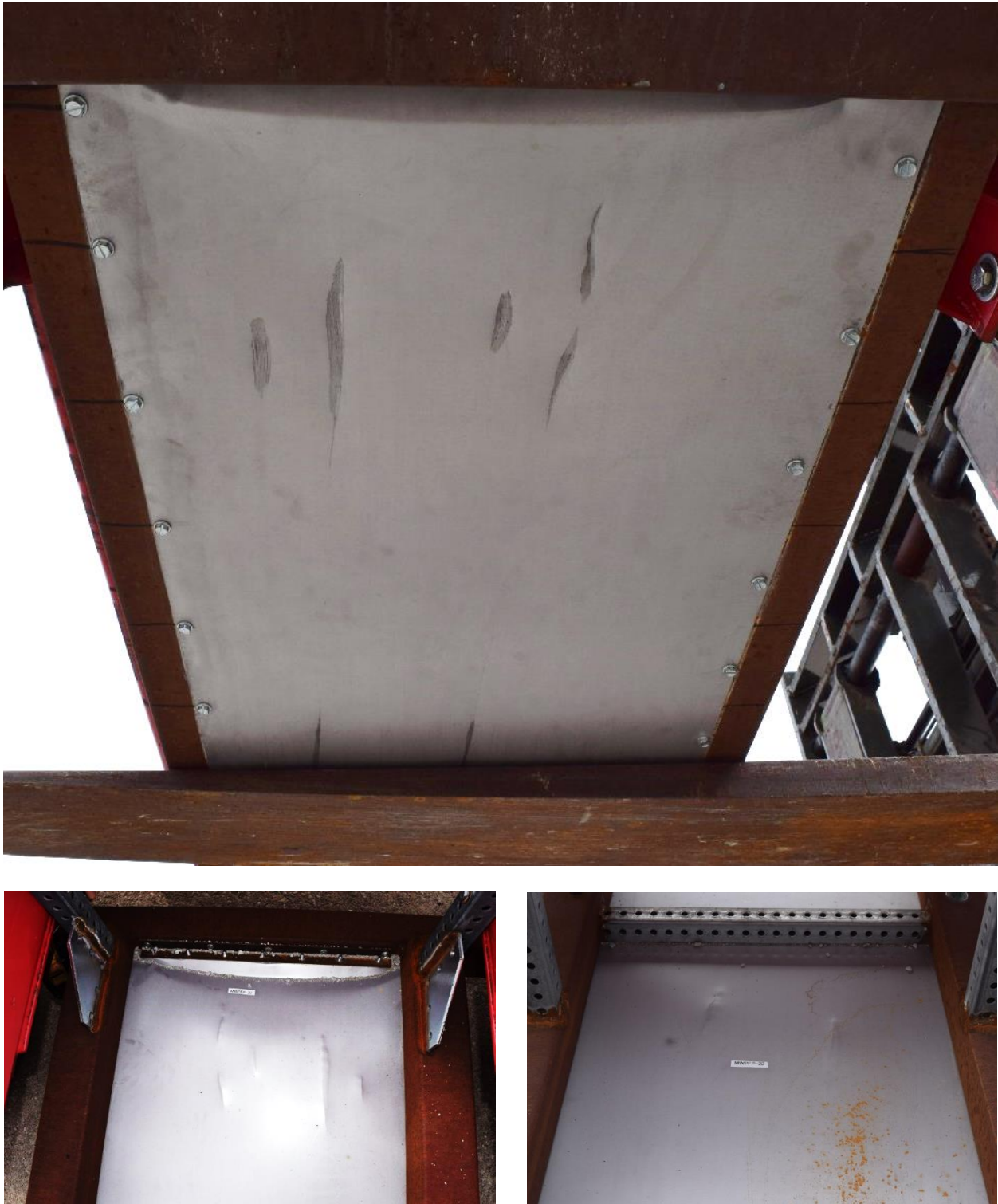
Figure 26. Simulated Floor Pan Damage, Test No. MWFPF-22
