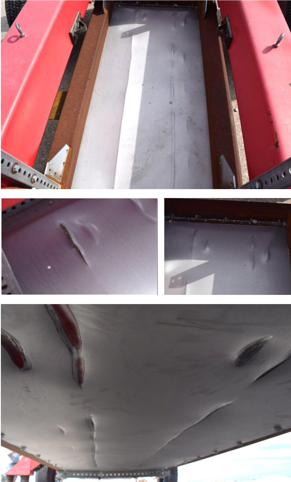
Figure 29. Simulated Floor Pan Damage, Test No. MWPFP-23
