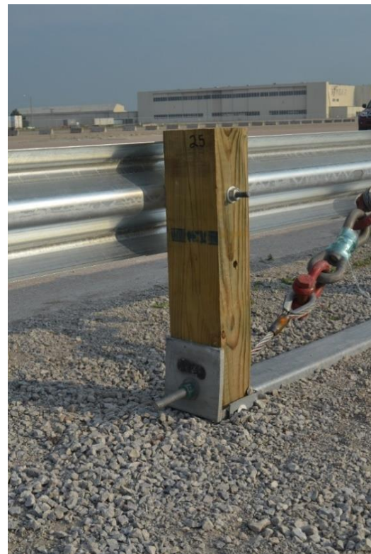
Figure 3. Long-Span End-Anchorage System, Test No. MGSLS-2
