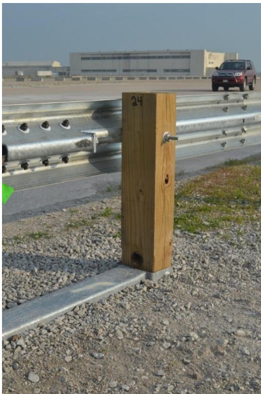
Figure 3. Long-Span End-Anchorage System, Test No. MGSLS-2
