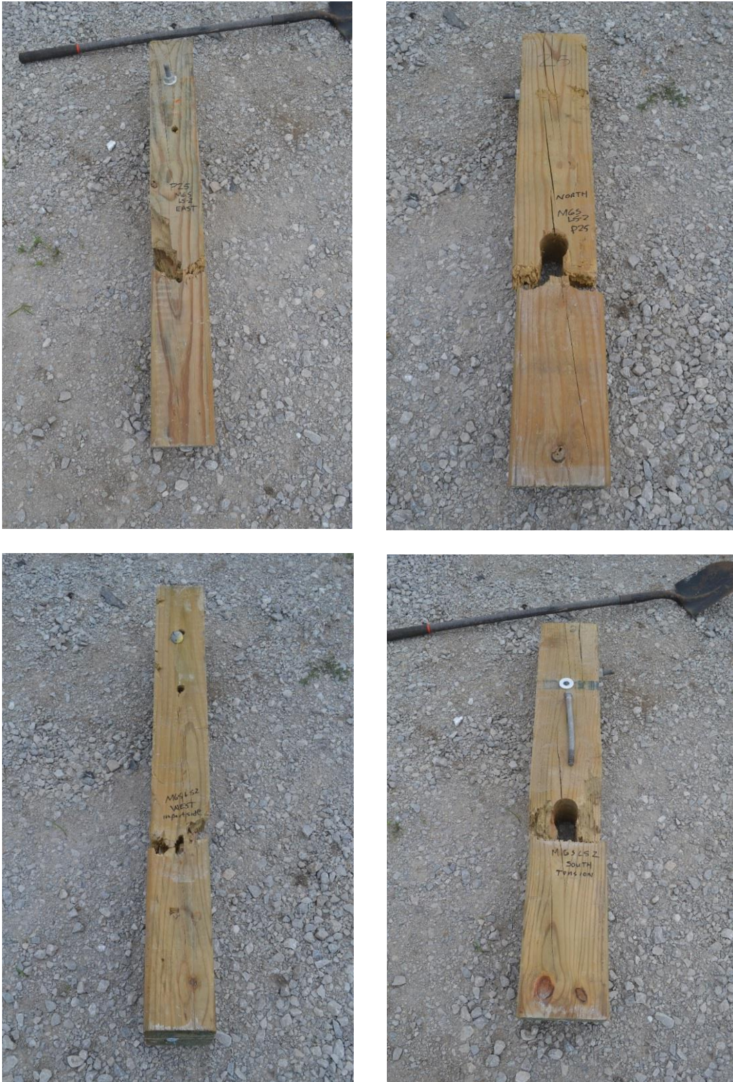
Figure 9. Post No. 25 Damage, Test No. MGSLs-2
