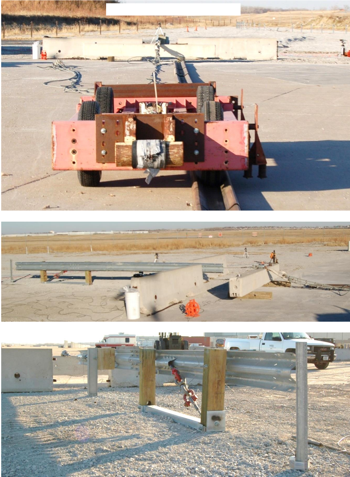
Figure 22. Dynamic End Anchorage Test Setup, Test No. DSAP-2
