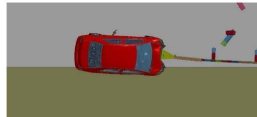
Simulation No. MASH-32-5deg-flared-6''
