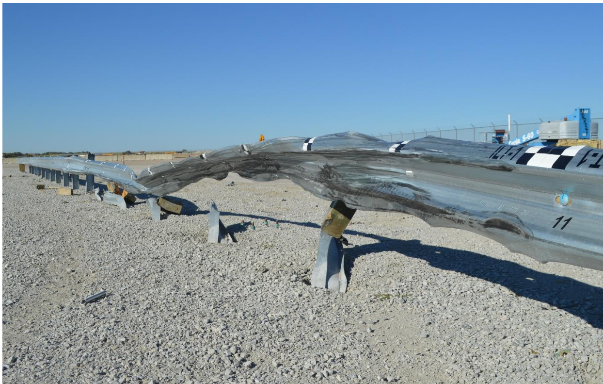
Figure 113. Midwest Guardrail System Damage, Test No. ILT-1
