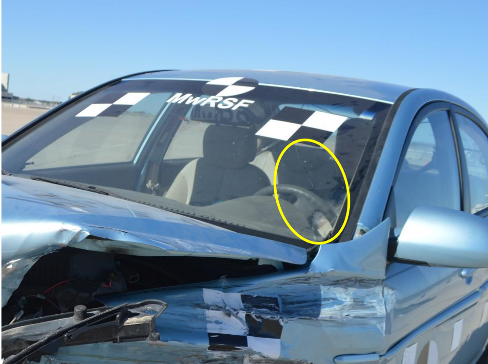
Figure 135. Vehicle Windshield Crack, Test No. ILT-2
