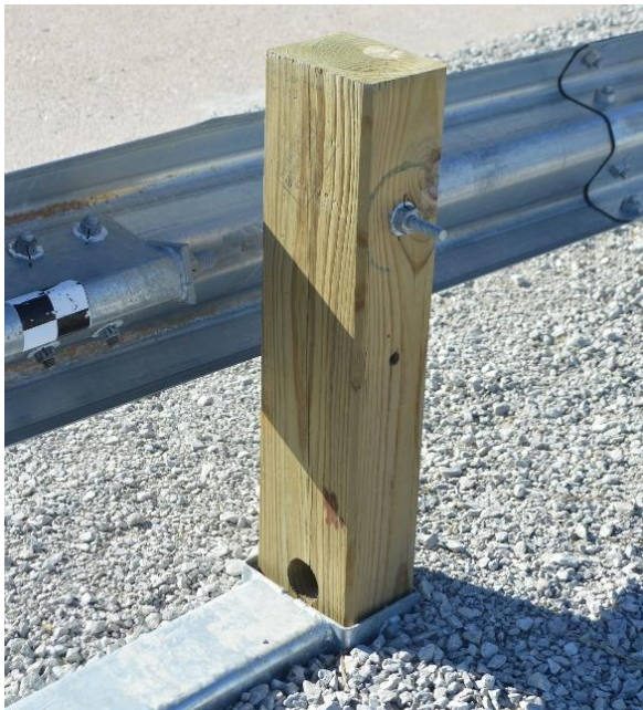
Figure 117. Upstream Anchor Damage, Test No. ILT-1
