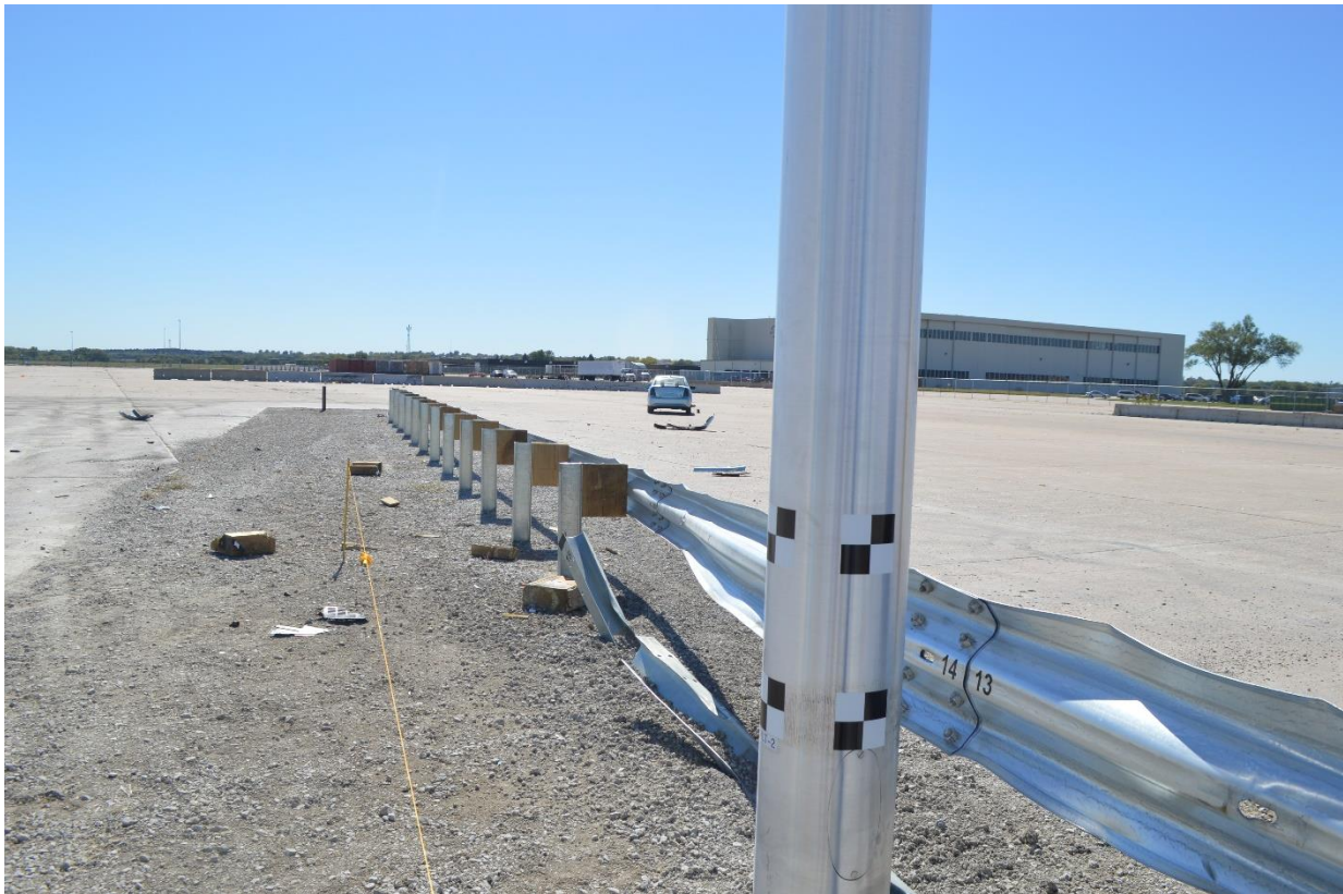
Figure 128. Midwest Guardrail System Damage, Test No. ILT-2
