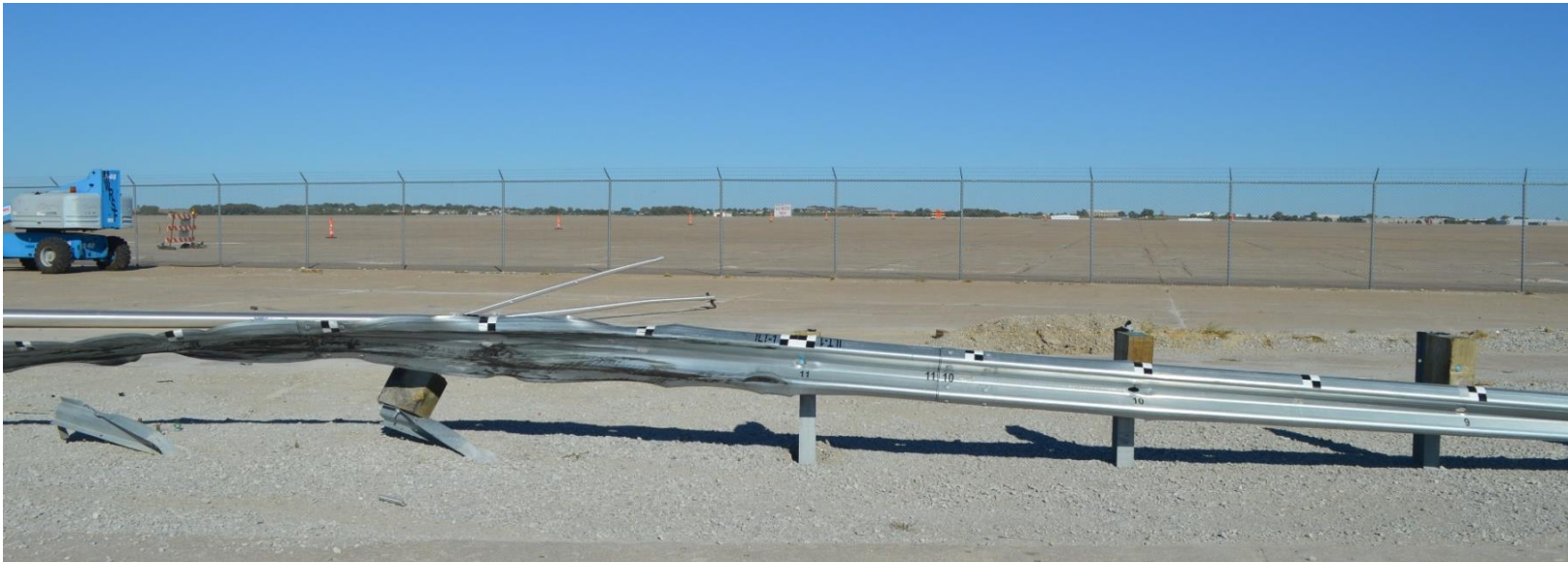
Figure 115. System Damage, Post Nos. 8 through 14, Test No. ILT-1
