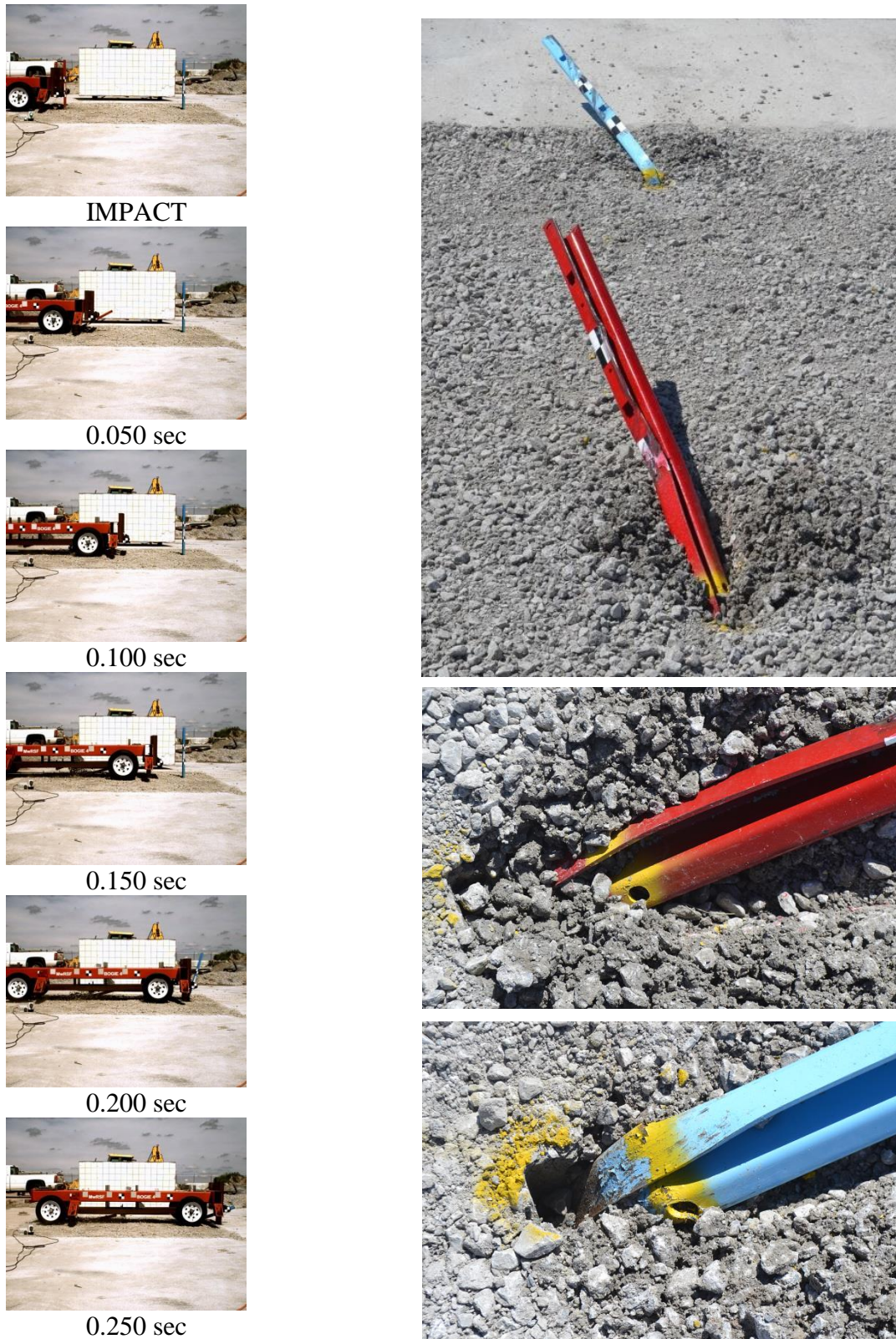
Figure 48. Time-Sequential and Post Damage Photographs, Test No. MWFPF-8
