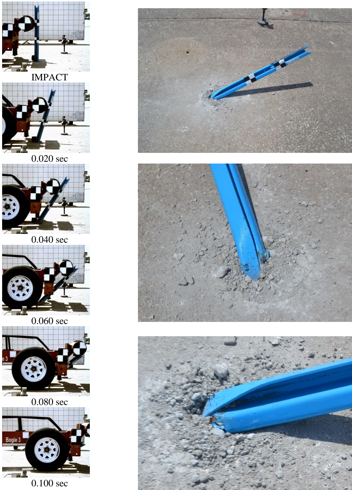
Figure 80. Time-Sequential and Post-Impact Photographs, Test No. MWPFP-9
