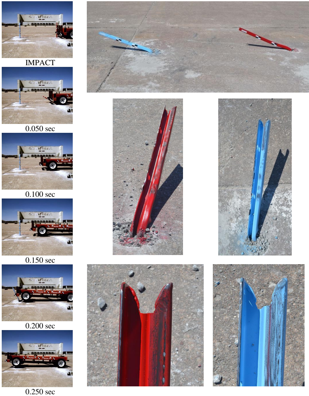
Figure 42. Time-Sequential and Post Damage Photographs, Test No. MWFPF-6
