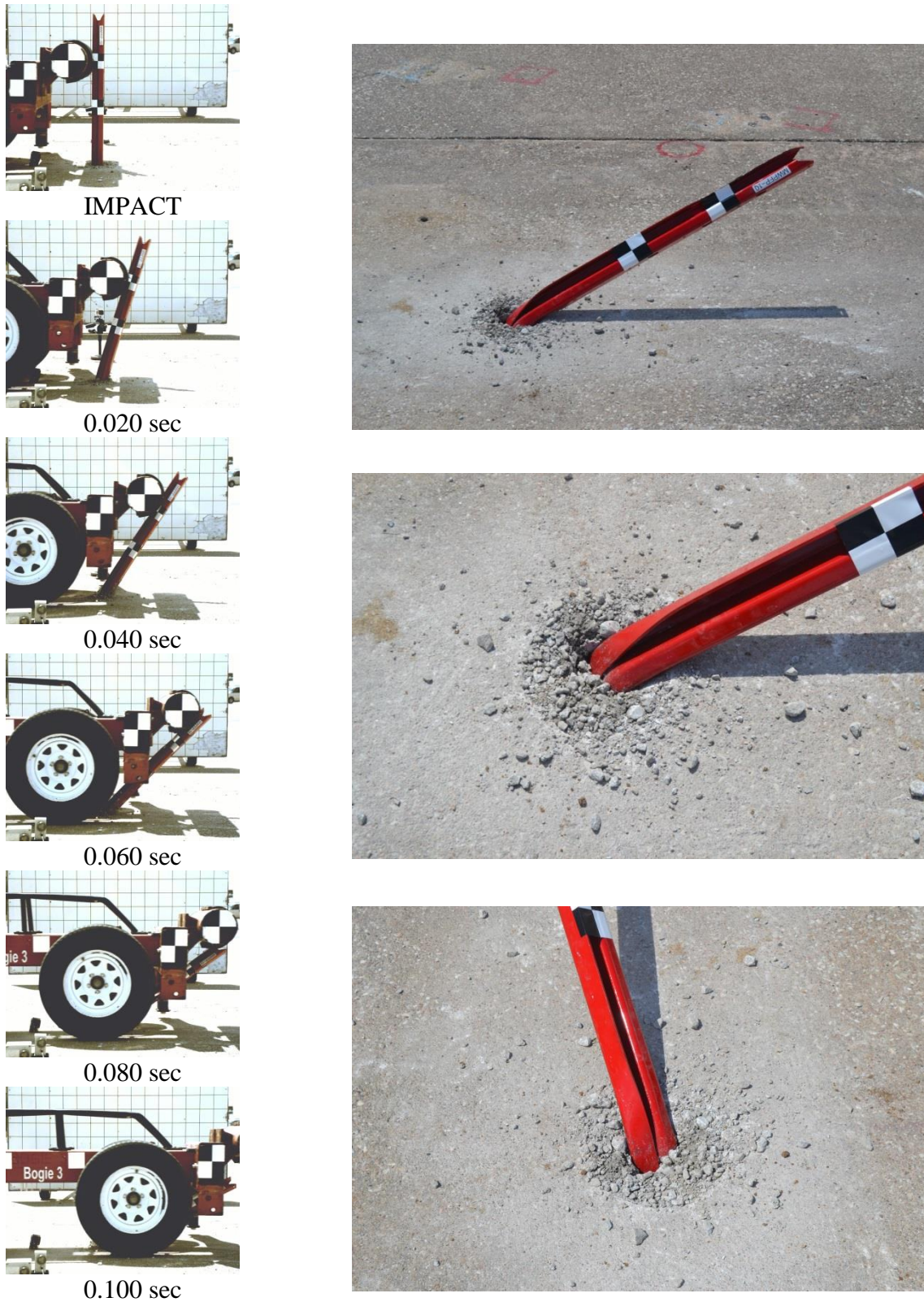
Figure 82. Time-Sequential and Post-Impact Photographs, Test No. MWPFP-10
