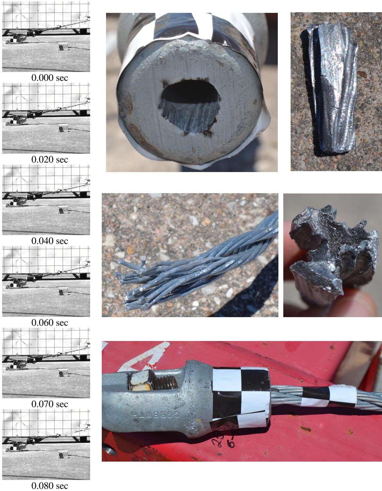
Figure 107. Time-Sequential and Post-Test Photographs, Test No. BBNC-2
