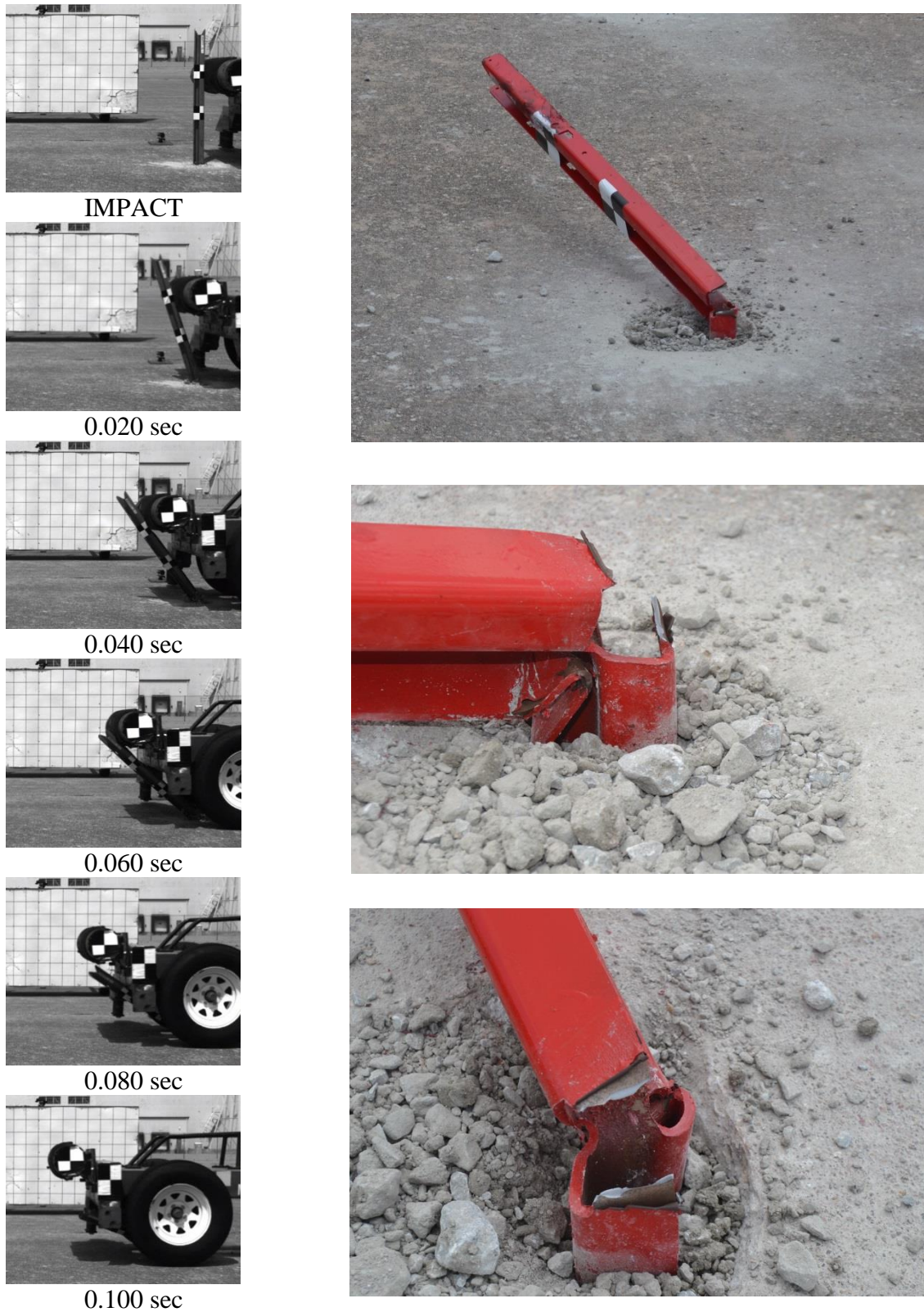
Figure 88. Time-Sequential and Post-Impact Photographs, Test No. MWPFP-17 Post 1
