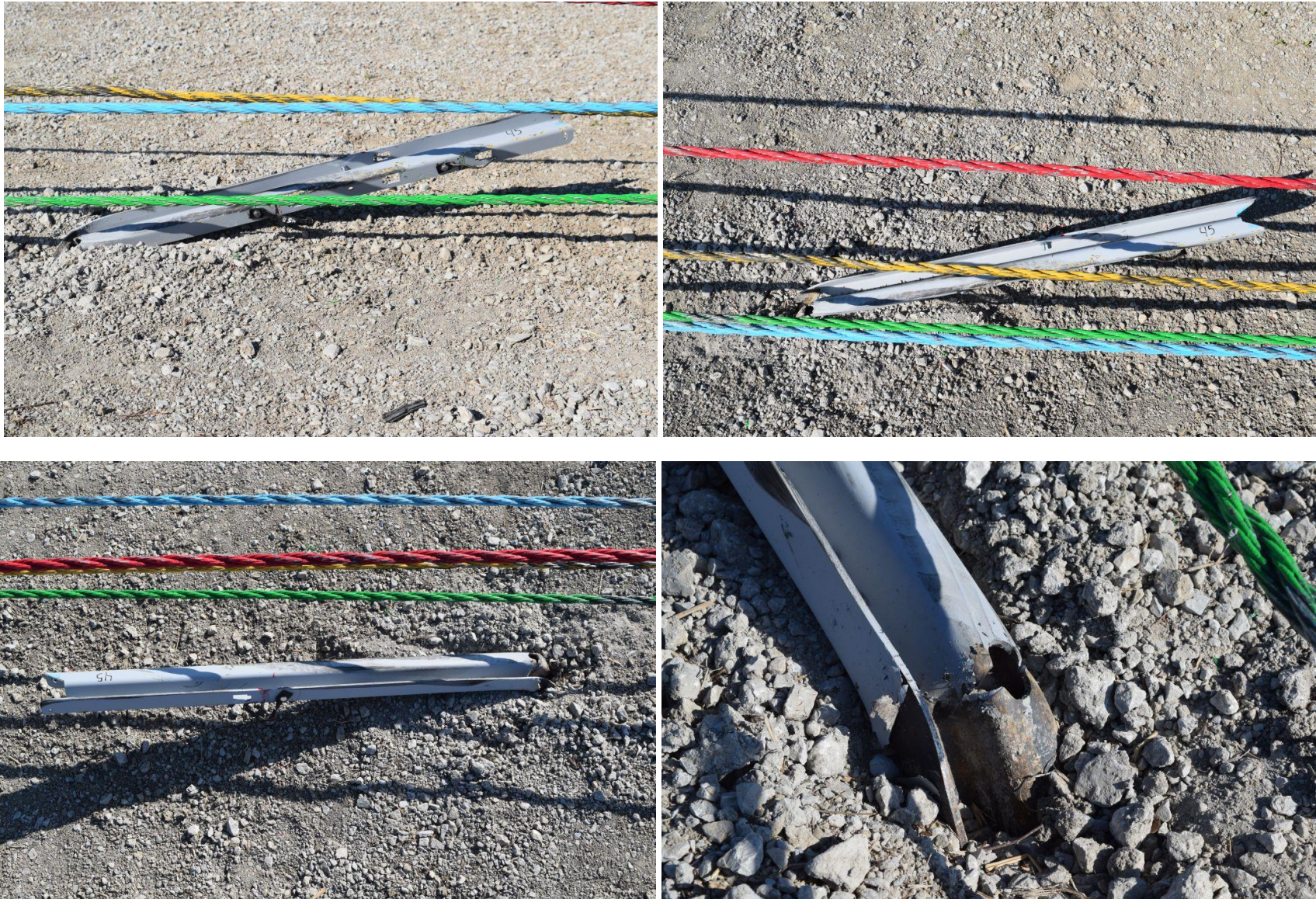
Figure 64. Post No. 45 Damage, Test No. MWP-8
