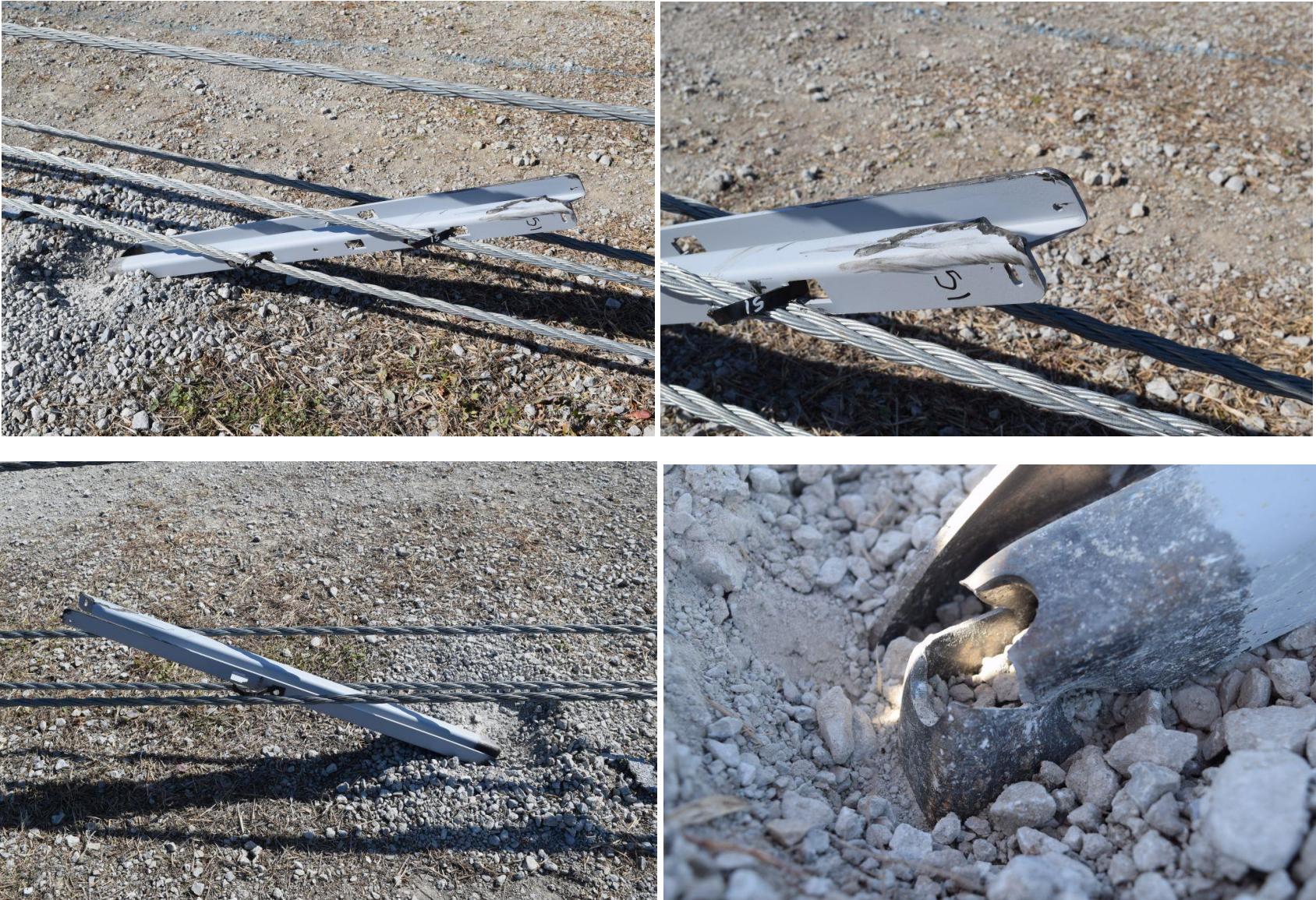
Figure 70. Post No. 51 Damage, Test No. MWP-8
