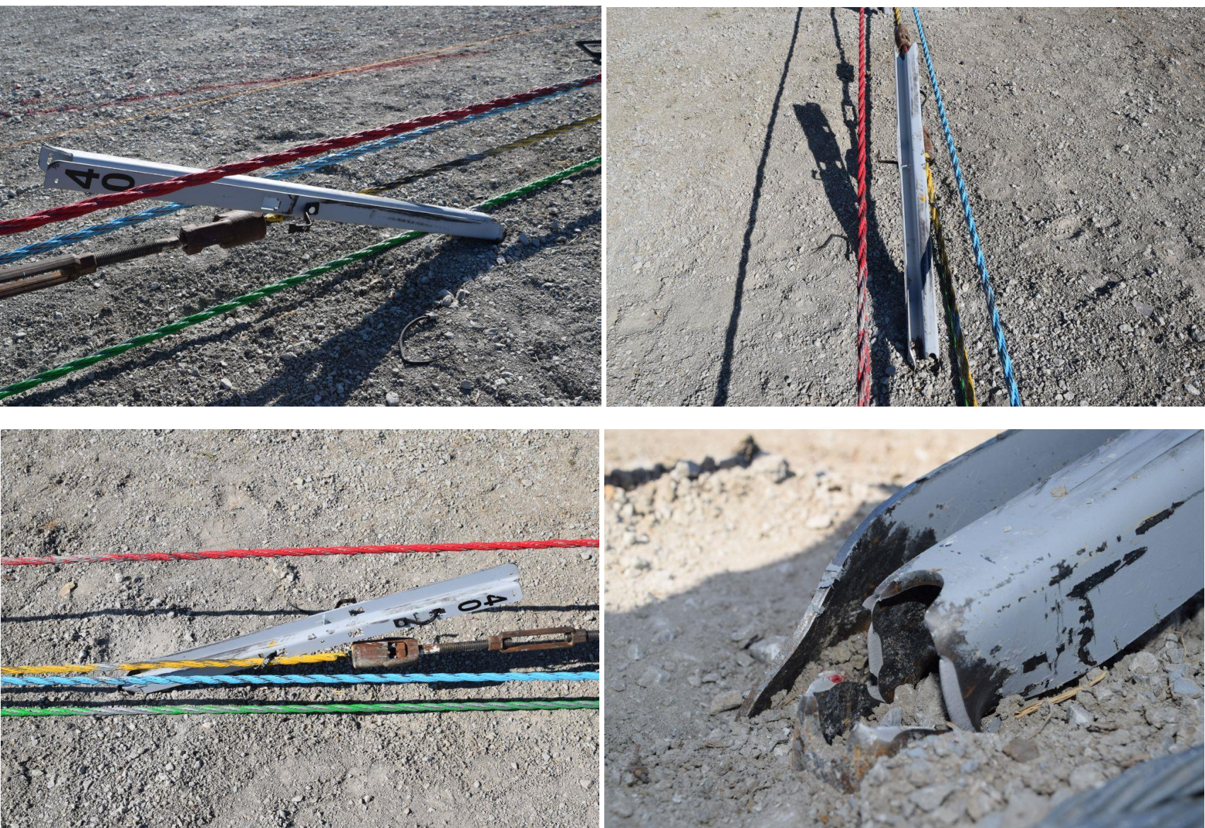
Figure 59. Post No. 40 Damage, Test No. MWP-8
