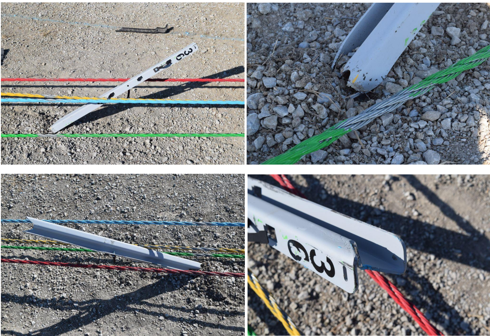
Figure 55. Post No. 36 Damage, Test No. MWP-8
