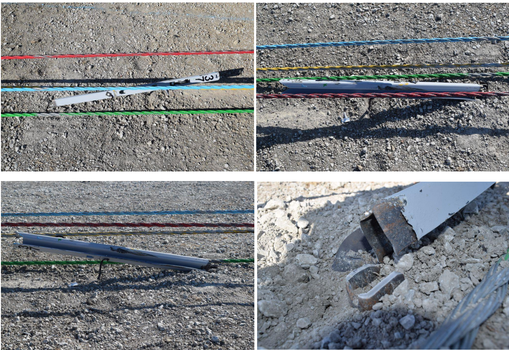
Figure 56. Post No. 37 Damage, Test No. MWP-8
