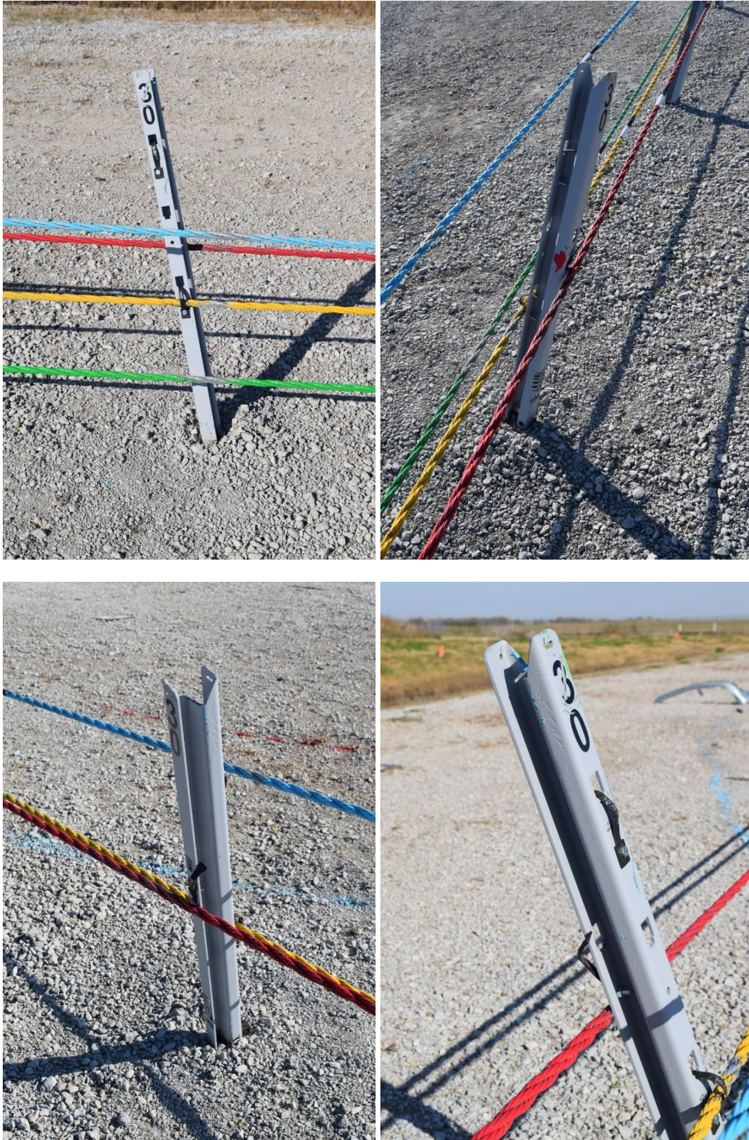
Figure 49. Post No. 30 Damage, Test No. MWP-8
