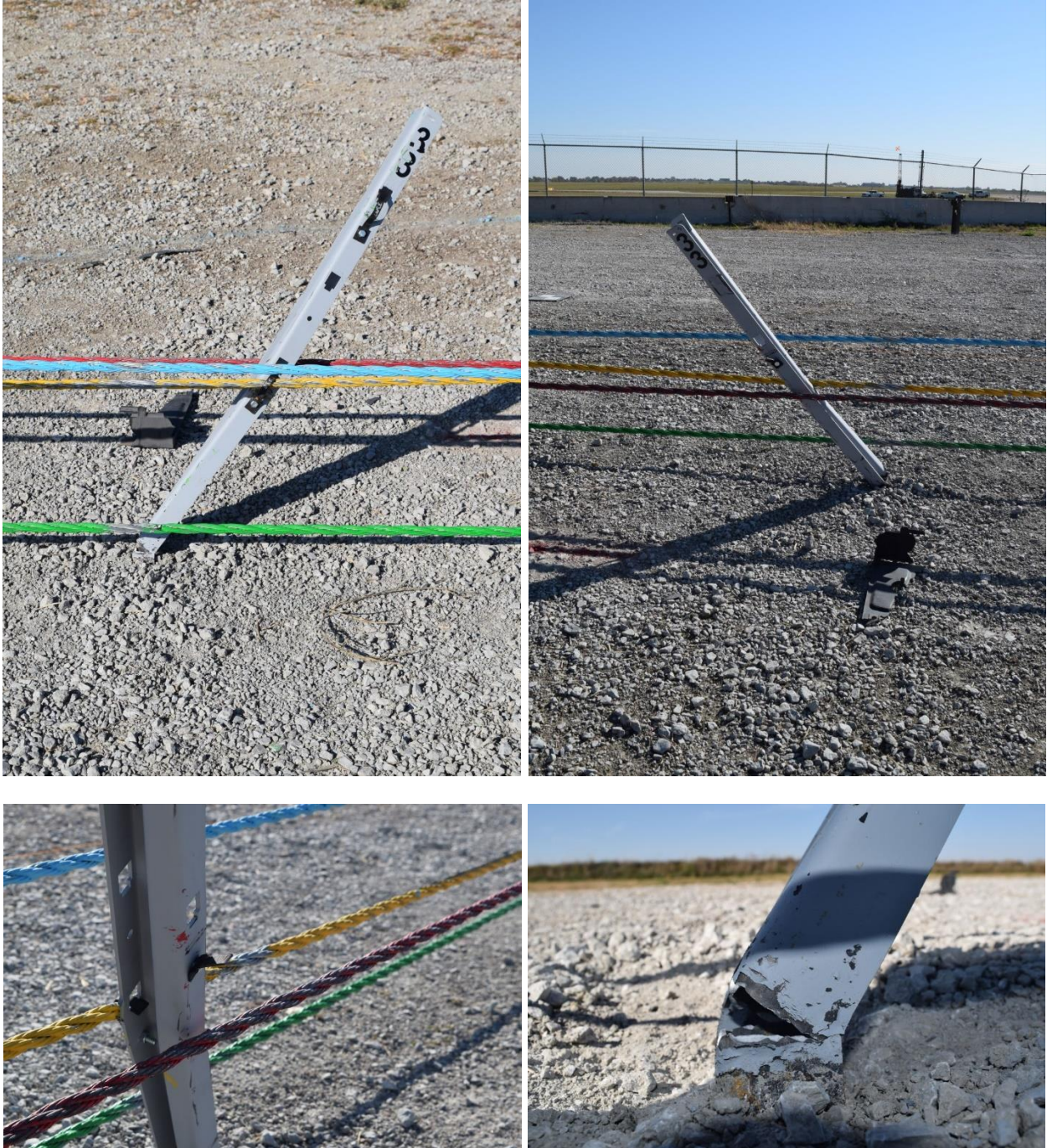
Figure 52. Post No. 33 Damage, Test No. MWP-8
