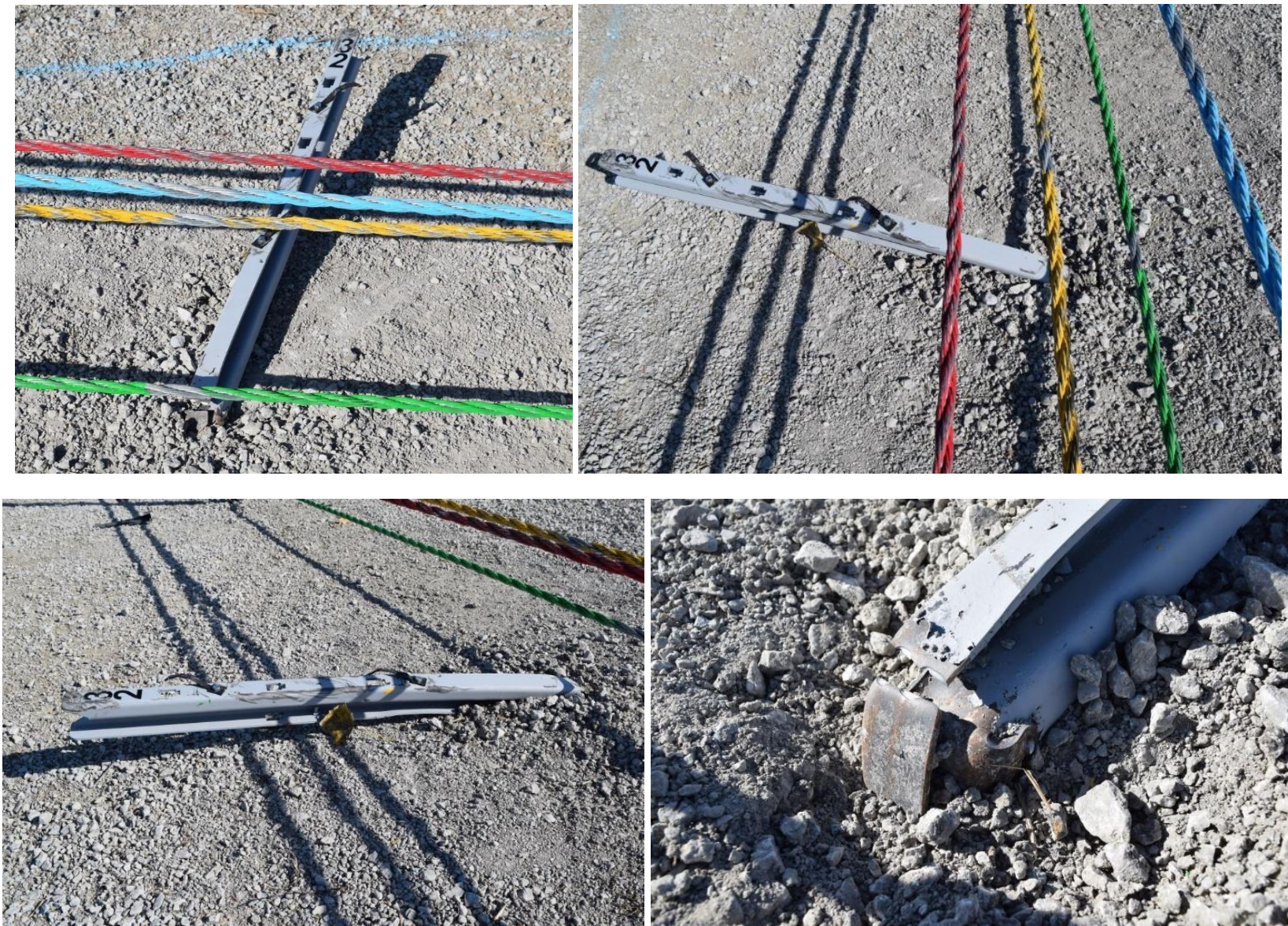
Figure 51. Post No. 32 Damage, Test No. MWP-8
