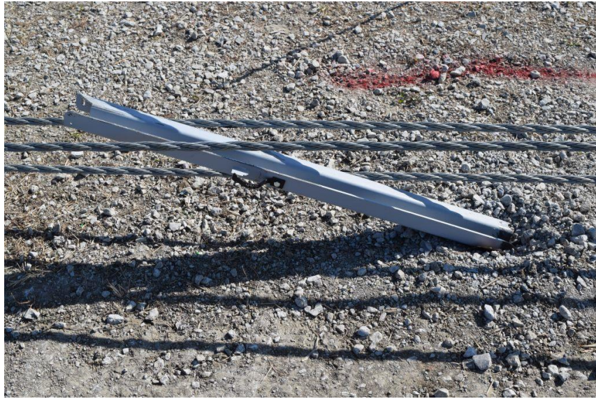
Figure 68. Post No. 49 Damage, Test No. MWP-8
