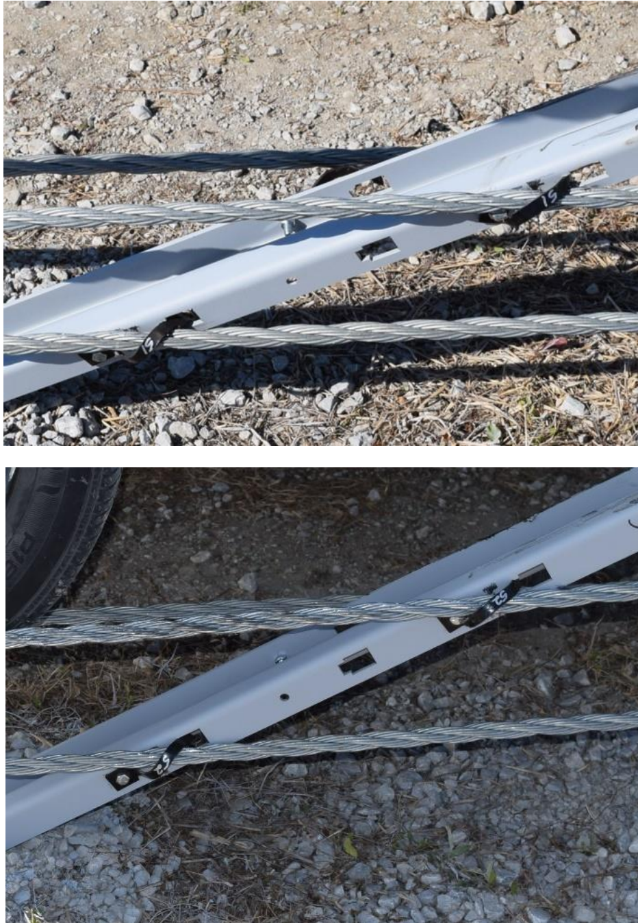
Figure 80. Cable Mounting Bracket Twisting – Post Nos. 51 and 52, Test No. MWP-8
