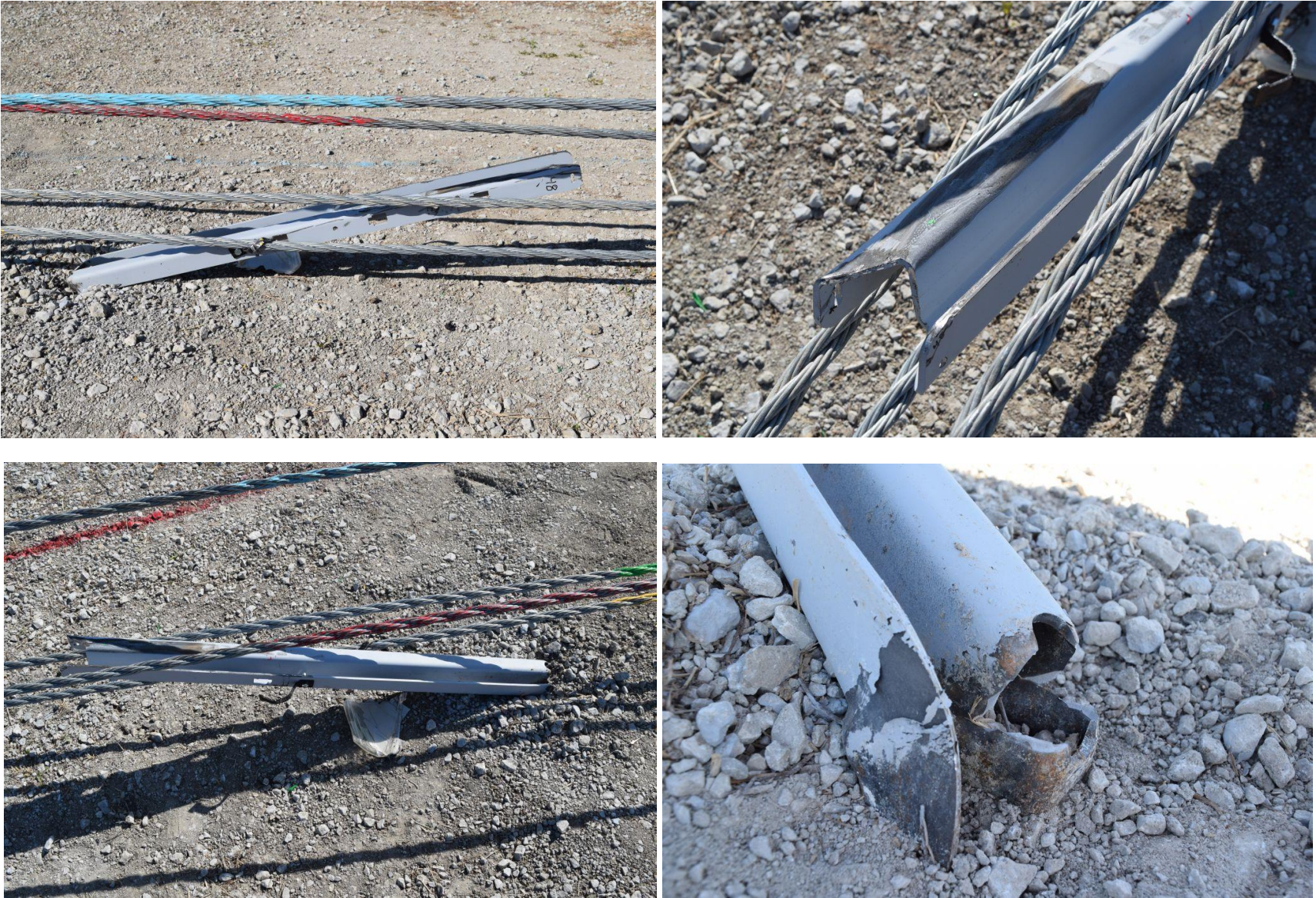
Figure 67. Post No. 48 Damage, Test No. MWP-8
