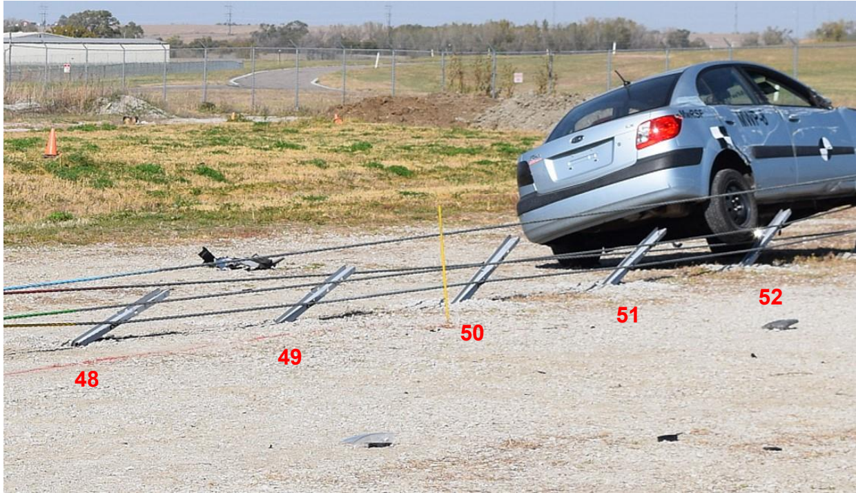
Figure 79. Post Deformation Difference – Post Nos. 48 Through 52, Test No. MWP-8
