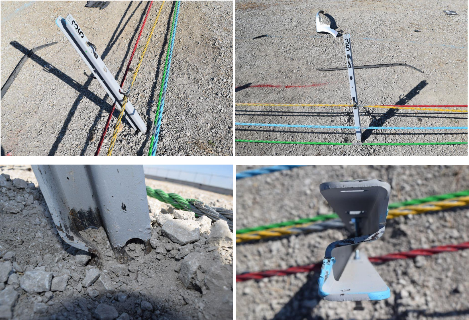
Figure 54. Post No. 35 Damage, Test No. MWP-8
