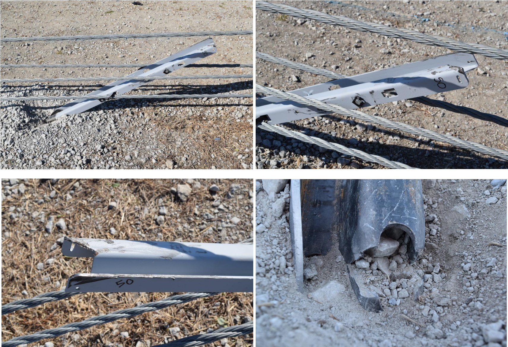
Figure 69. Post No. 50 Damage, Test No. MWP-8
