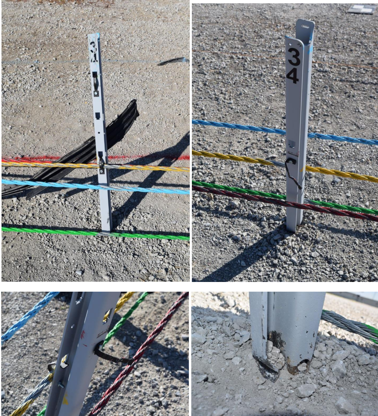
Figure 53. Post No. 34 Damage, Test No. MWP-8
