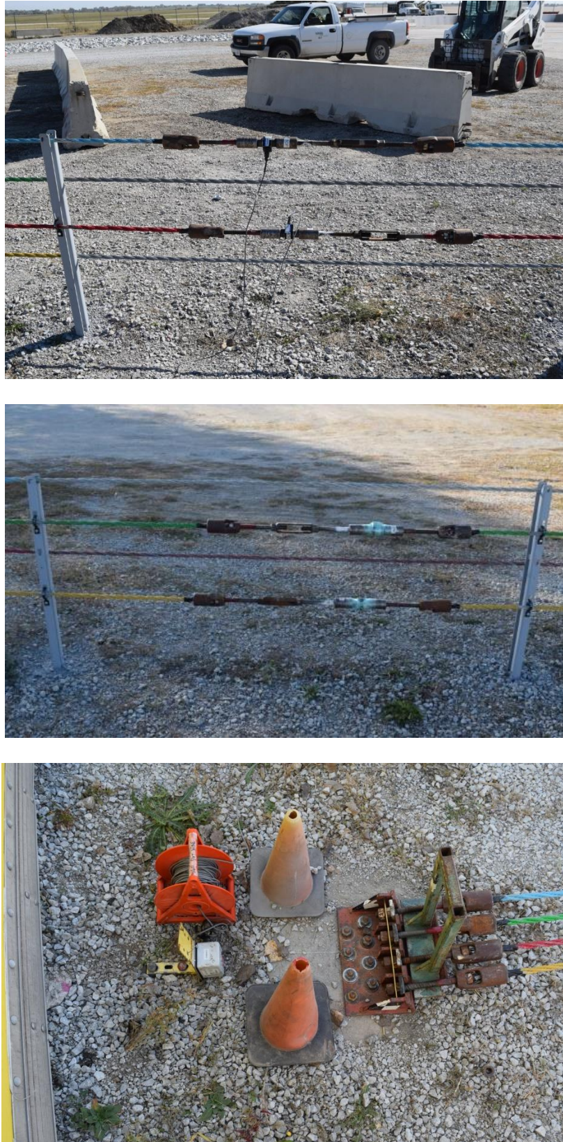
Figure 36. Location of Load Cells and String Potentiometers, Test No. MWP-8
