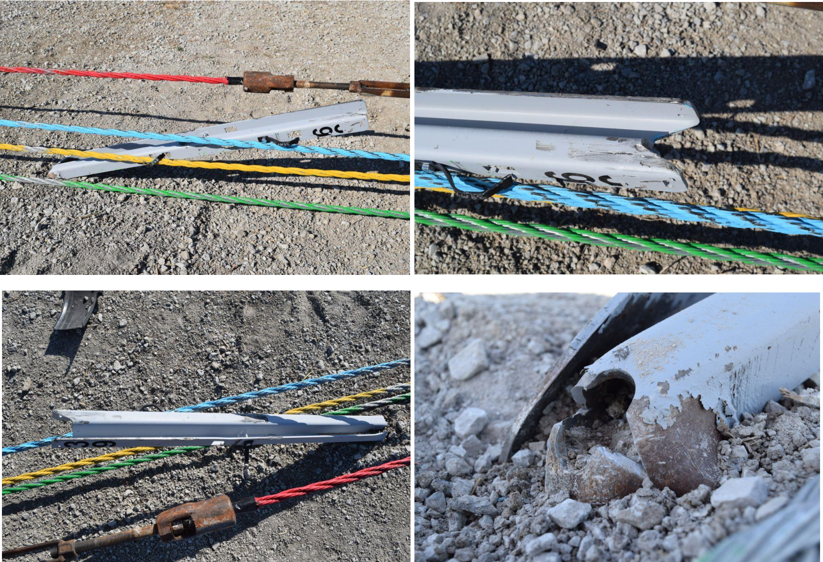
Figure 58. Post No. 39 Damage, Test No. MWP-8
