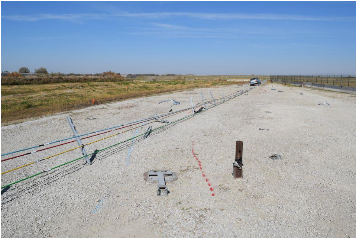
Figure 44. Vehicle Final Position and Trajectory Marks, Test No. MWP-8
