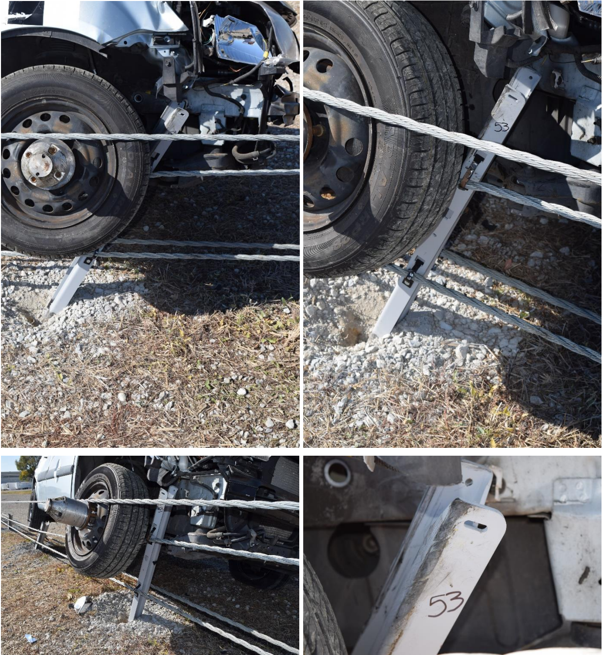
Figure 72. Post No. 53 Damage, Test No. MWP-8
