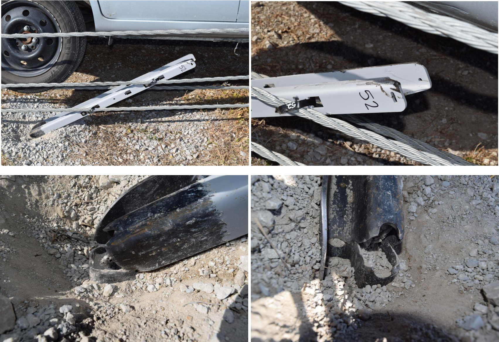
Figure 71. Post No. 52 Damage, Test No. MWP-8
