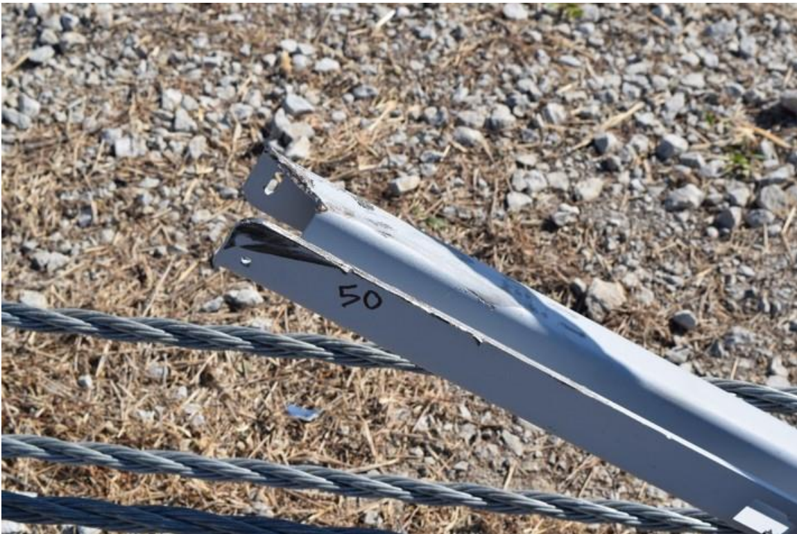
Figure 78. Post No. 50 Damage, Test No. MWP-8
