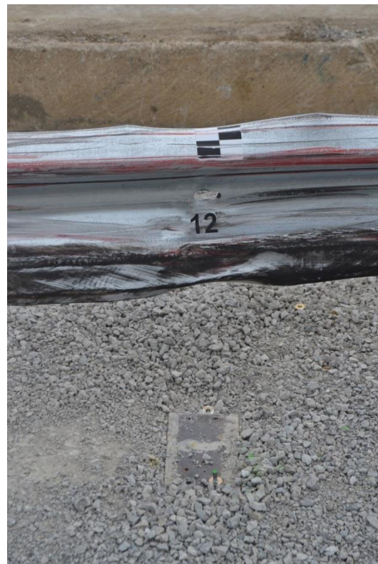
Figure 51. Damage Between Post Nos. 10 and 12, Test No. MGSLs-1
