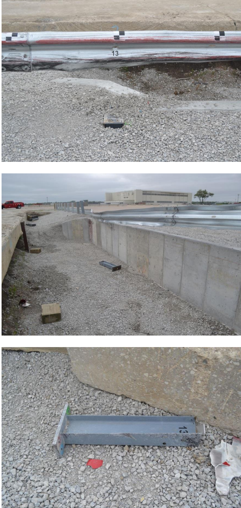
Figure 52. Damage at Post No. 13, Test No. MGSLs-1
