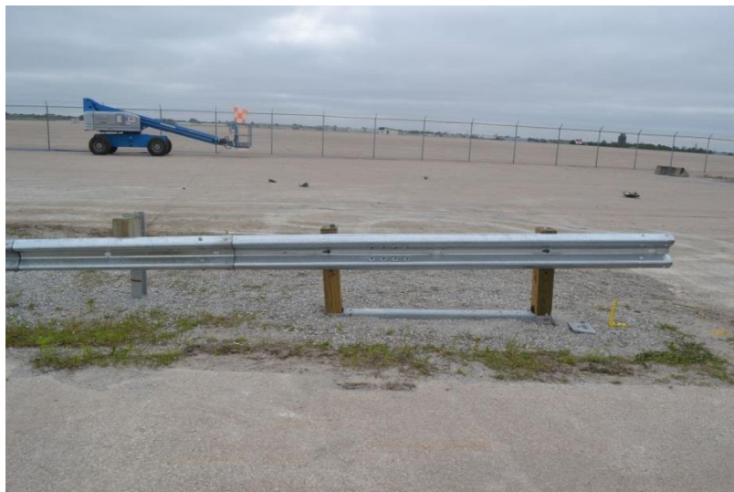
Figure 55. Damage Between Post Nos. 17 and 25, Test No. MGSLS-1
