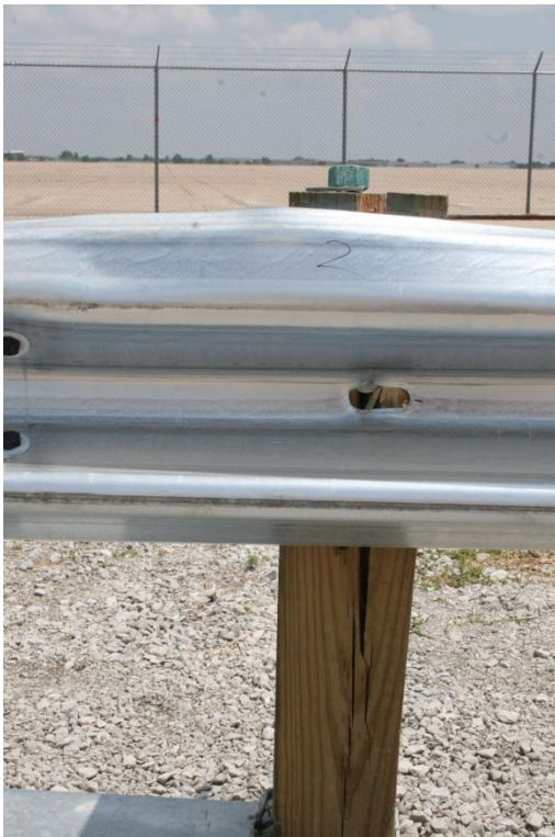
Figure 69. Upstream End Anchor Damage, Test No. MGSLS-2
