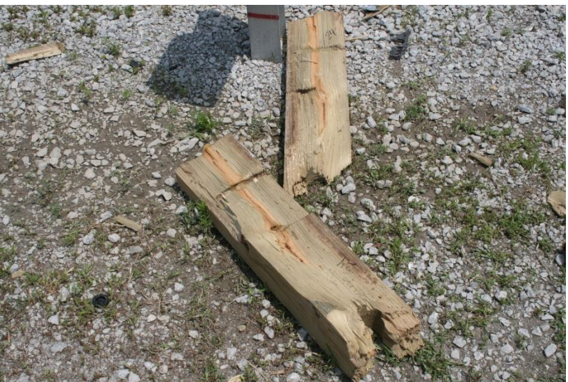
Figure 80. Downstream Anchorage Damage, Test No. MGSLS-2
