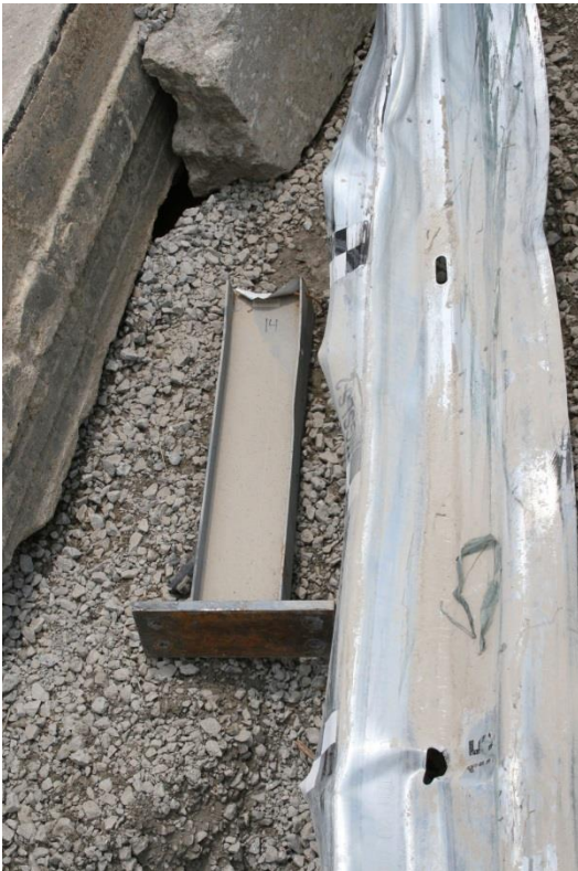
Figure 73. Damage at Post No. 14, Test No. MGSLS-2
