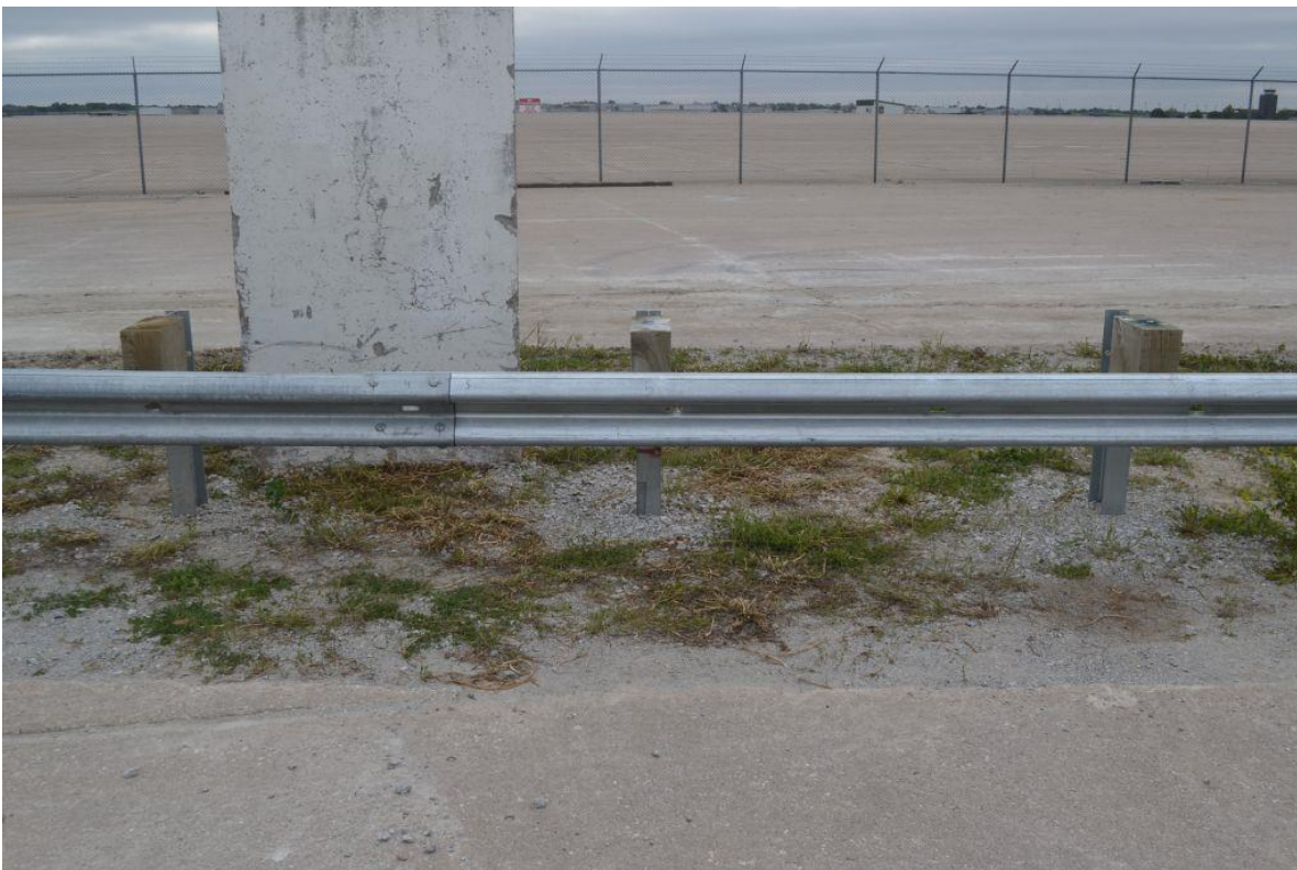
Figure 50. System Damage Between Post Nos. 3 and 9, Test No. MGSLS-1
