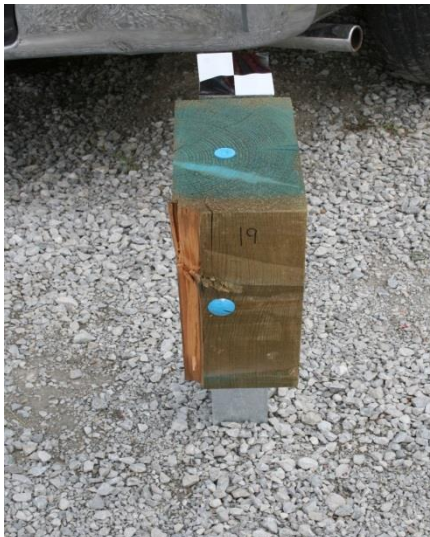
Figure 76. Damage to Post Nos. 17 through 19, Test No. MGSLs-2
