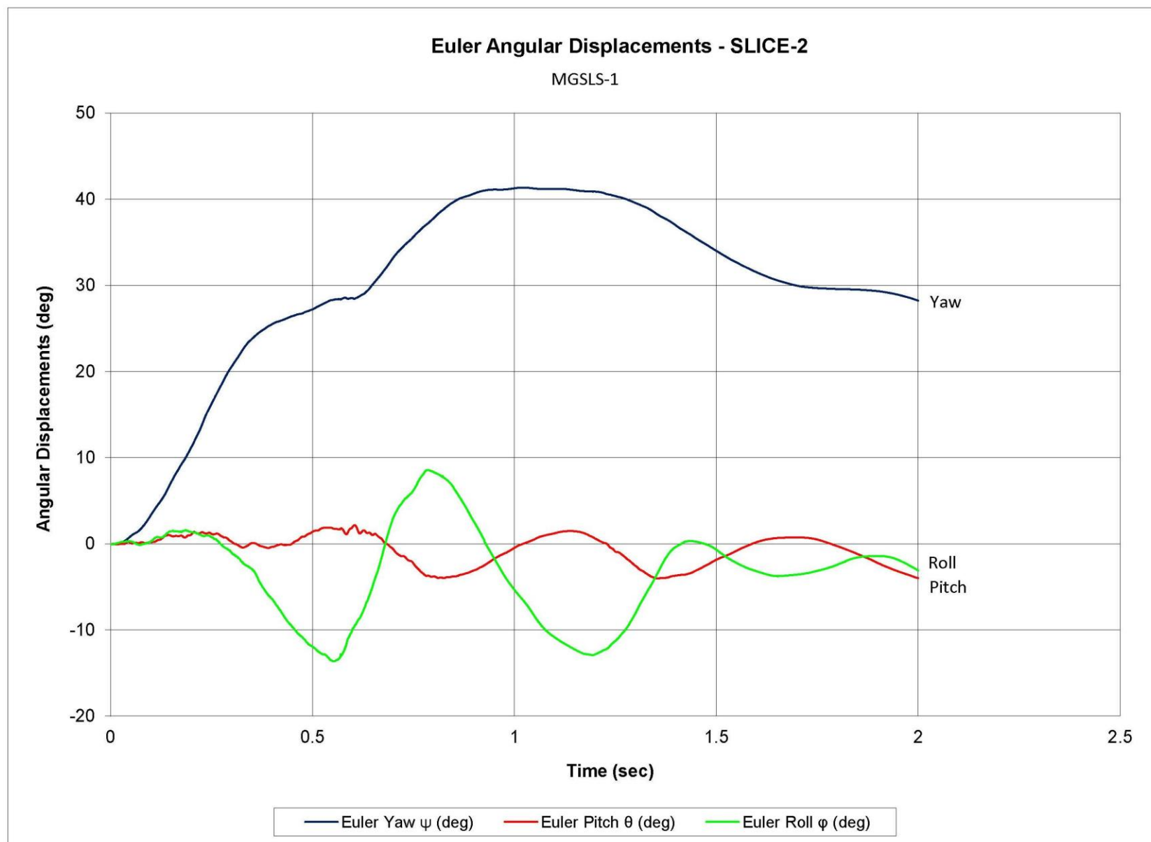
Figure E-15. Vehicle Angular Displacements (SLICE-2), Test No. MGSLs-1
