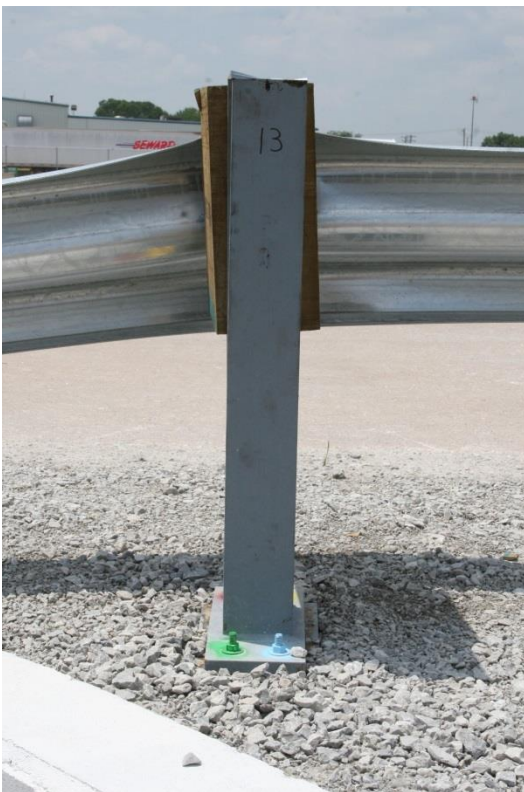
Figure 71. Damage at Post No. 13, Test No. MGSLS-2
