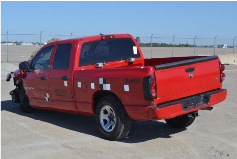
Figure 56. Vehicle Damage, Test No. MGSLS-1
