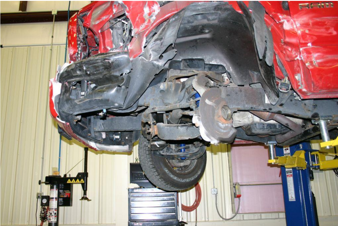
Figure 58. Vehicle Undercarriage Damage, Test No. MGSLS-1
