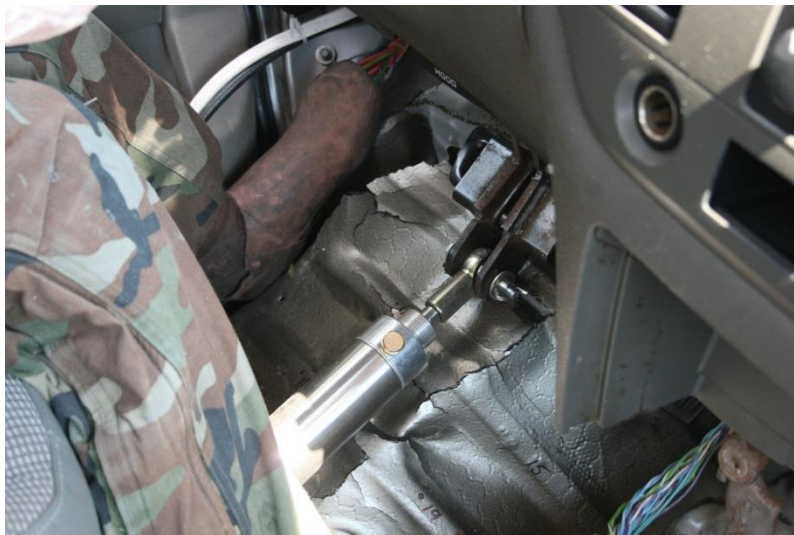
Figure 84. Occupant Compartment Damage, Test No. MGSLS-2
