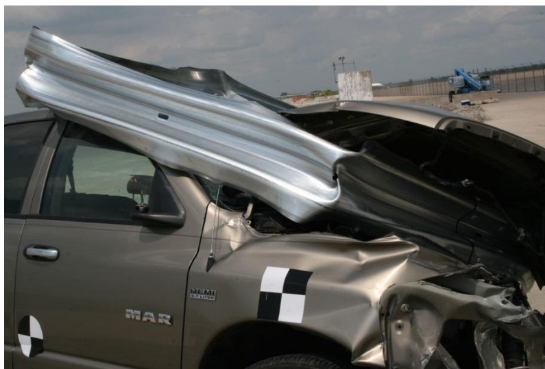
Figure 78. Damage to Barrier System Between Post Nos. 20 through 22, Test No. MGSL-2
