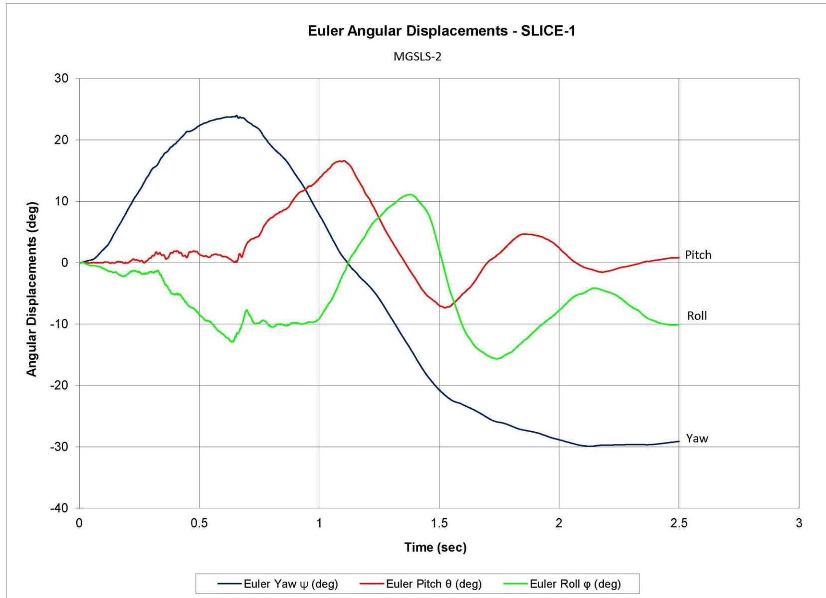
Figure F-7. Vehicle Angular Displacements (SLICE-1), Test No. MGSLS-2
