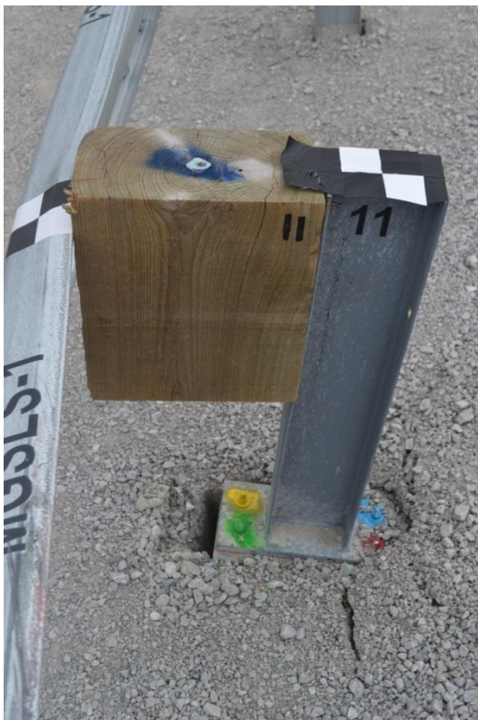
Figure 51. Damage Between Post Nos. 10 and 12, Test No. MGSLs-1
