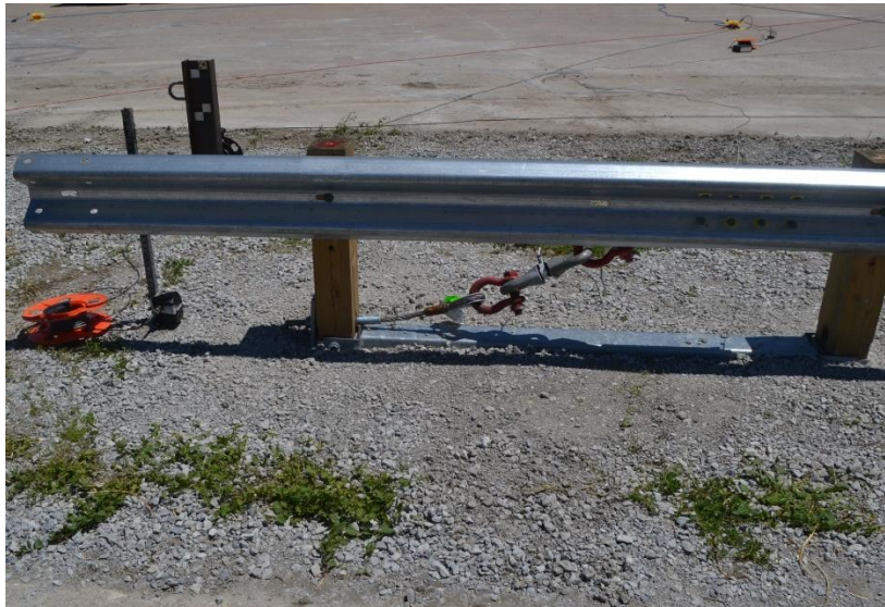
Figure 8. Location of Load Cells and String Potentiometers, Test No. MGSLS-1
