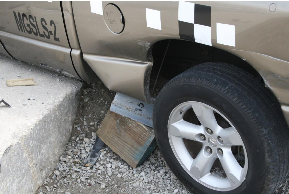
Figure 74. Damage at Post No. 15, Test No. MGSL-2
