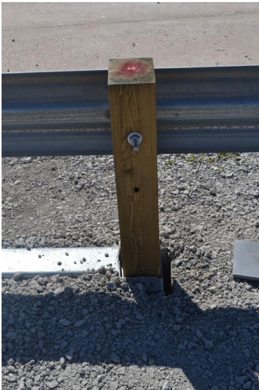
Figure 49. Upstream End Anchor Damage, Test No. MGSLS-1
