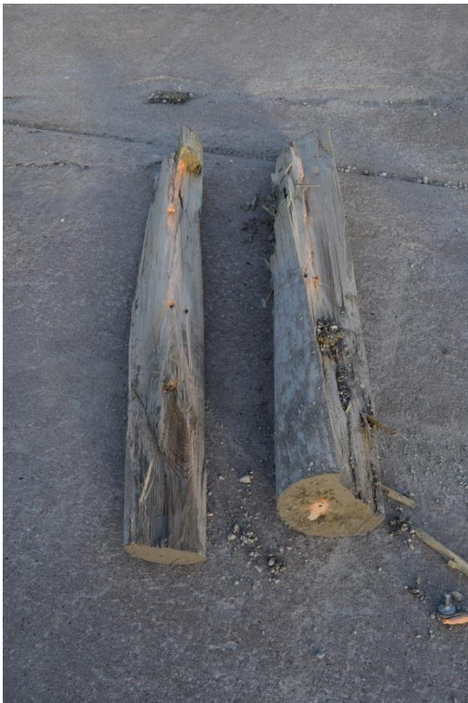
Figure 38. Post Nos. 13 and 14 Damage After Removed from Ground, Test No. AZRP-1
