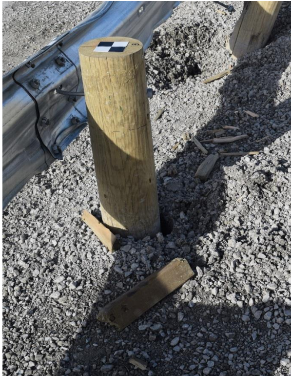
Figure 33. Post No. 13 Damage, Test No. AZRP-1
