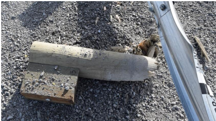
Figure 35. Post No. 15 Damage, Test No. AZRP-1
