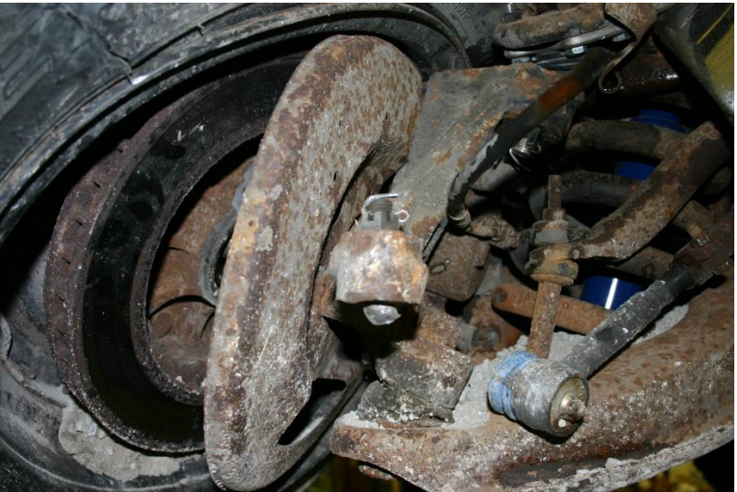
Figure 44. Vehicle Undercarriage Damage, Test No. AZRP-1
