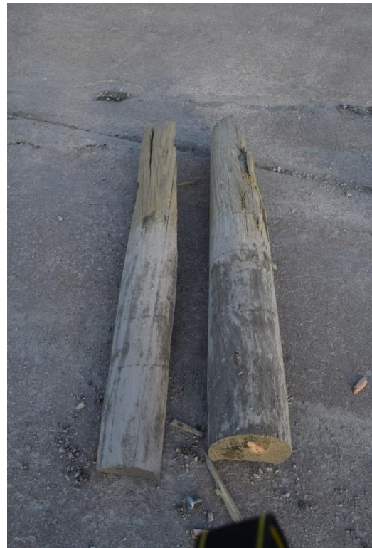
Figure 38. Post Nos. 13 and 14 Damage After Removed from Ground, Test No. AZRP-1
