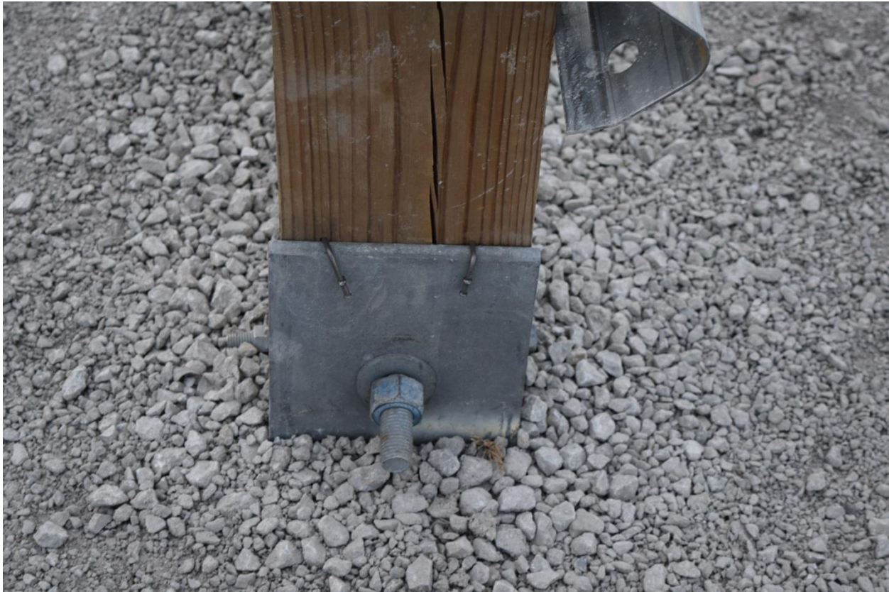
Figure 17. Test Installation End Anchorage Photographs, Test No. AZRP-1
