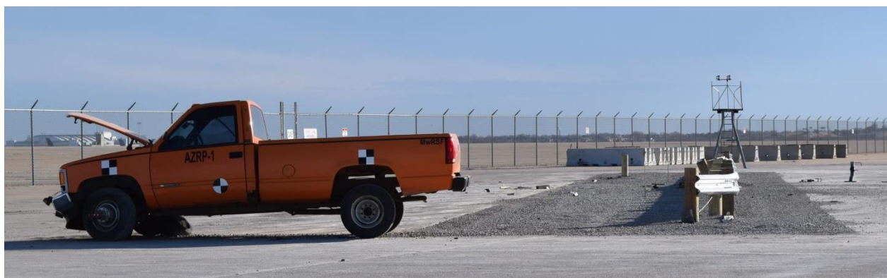
Figure 29. Vehicle Final Position and Trajectory Marks, Test No. AZRP-1
