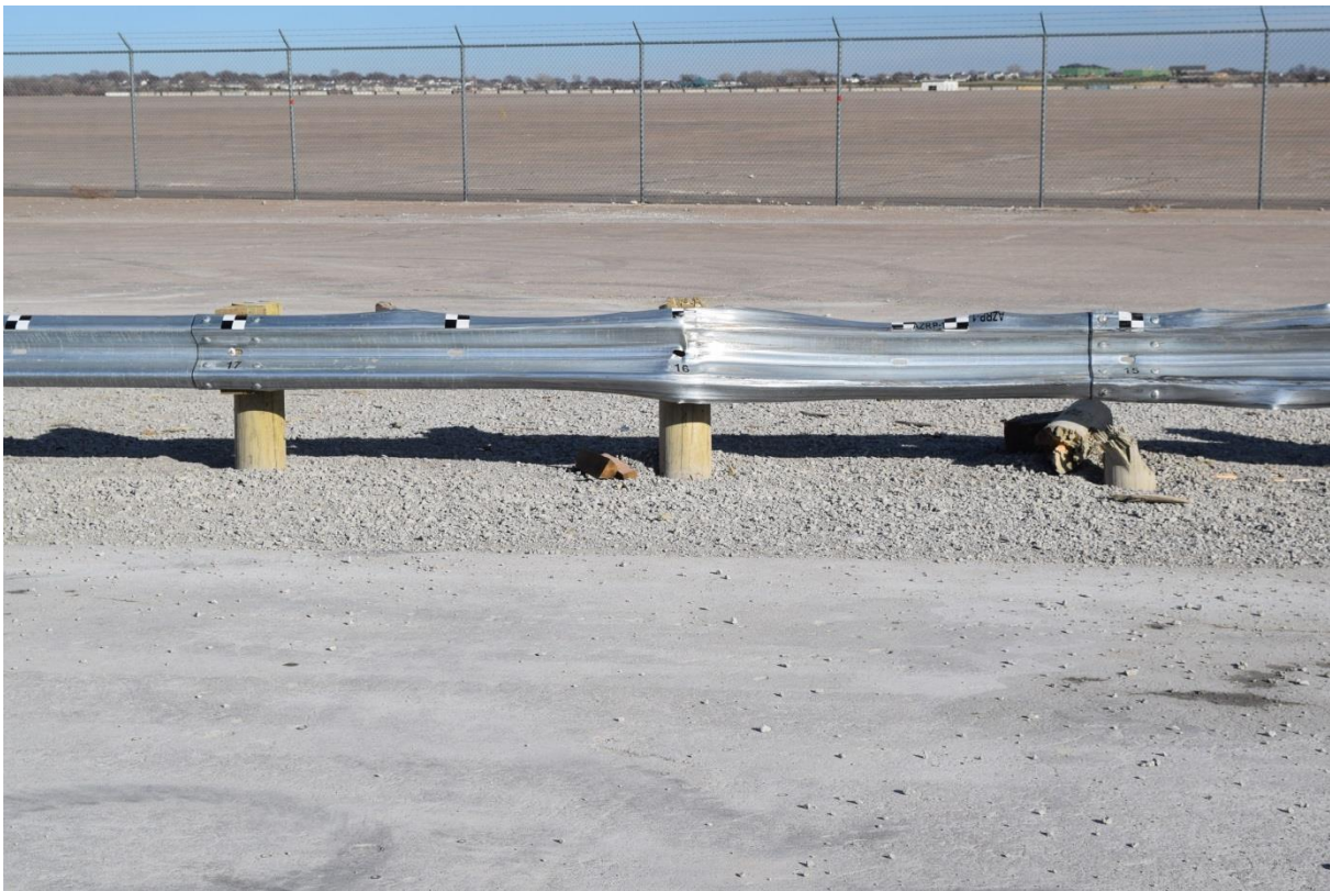
Figure 32. Rail Damage Between Post Nos. 12 and 17, Test No. AZRP-1
