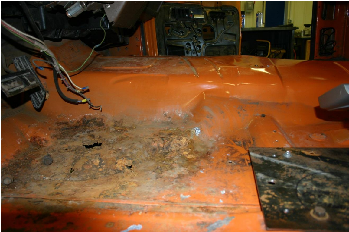
Figure 43. Vehicle Left-Side Floorboard Deformation, Test No. AZRP-1
