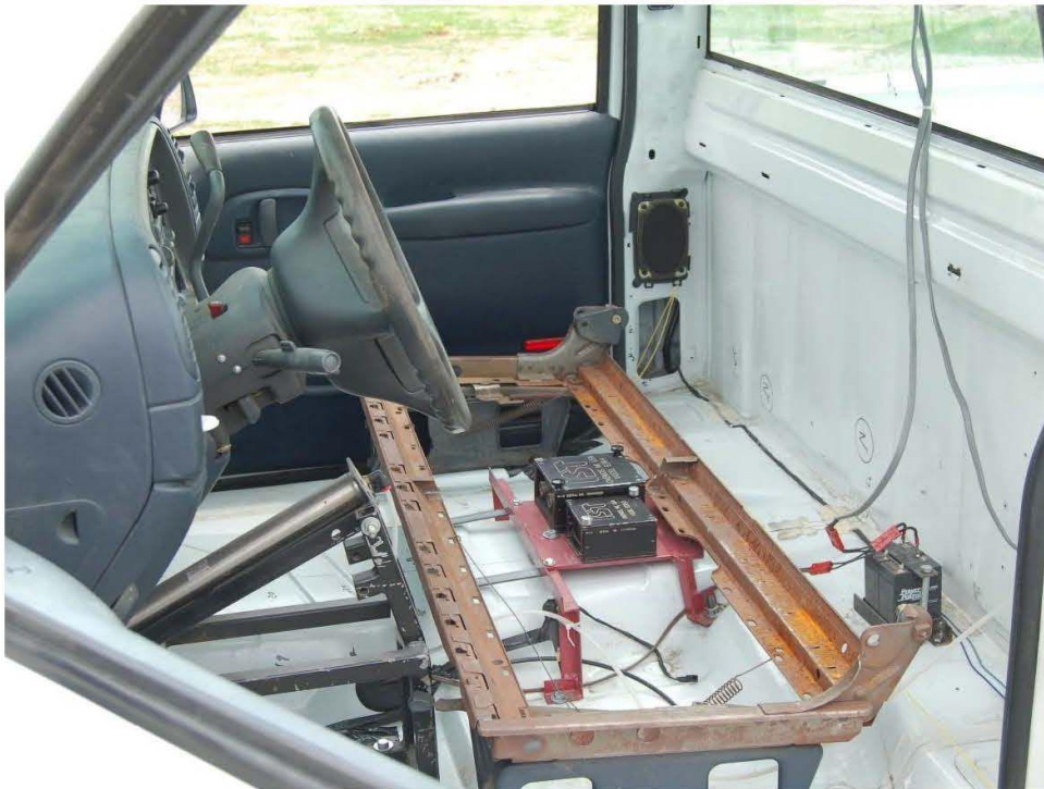
b) Typical NCHRP Report No. 350 Transducer Installation for 2000P Vehicle
