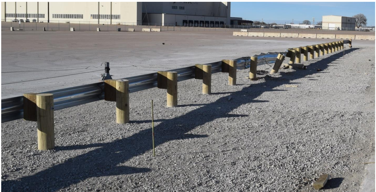
Figure 31. System Damage, Test No. AZRP-1
