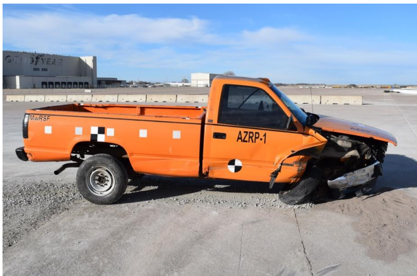
Figure 40. Vehicle Damage, Test No. AZRP-1
