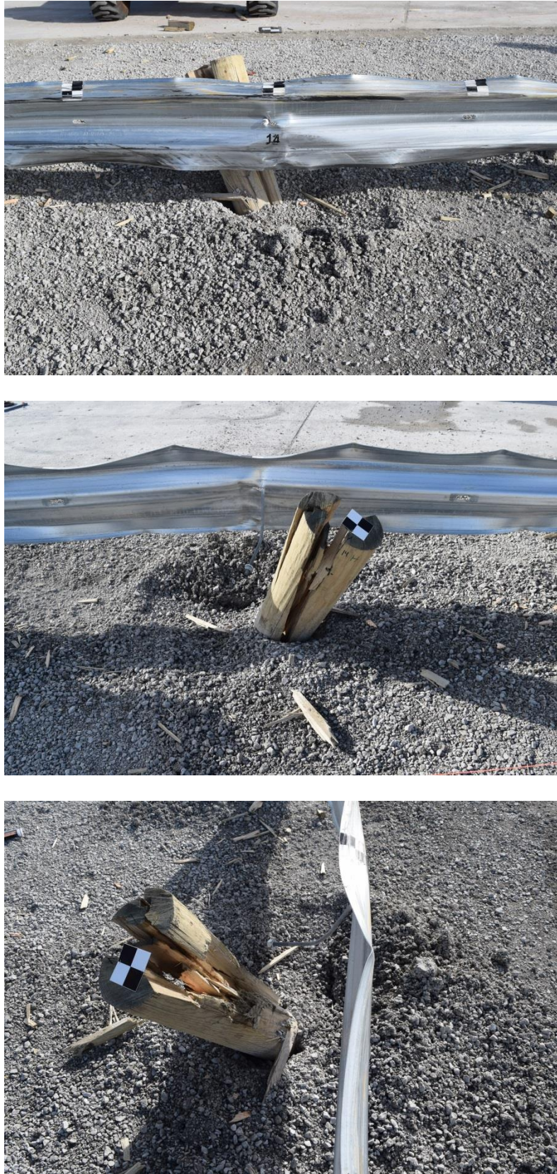
Figure 34. Post No. 14 Damage, Test No. AZRP-1
