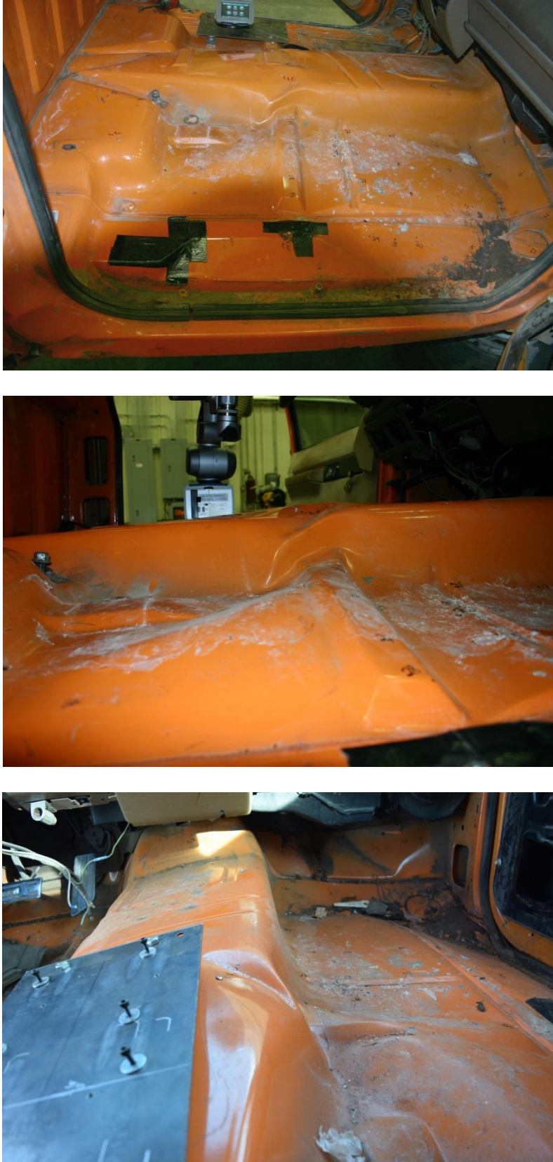
Figure 42. Vehicle Right-Side Floorboard Deformation, Test No. AZRP-1
