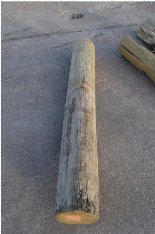
Figure 39. Post Nos. 15 and 16 Damage After Removed from Ground, Test No. AZRP-1
