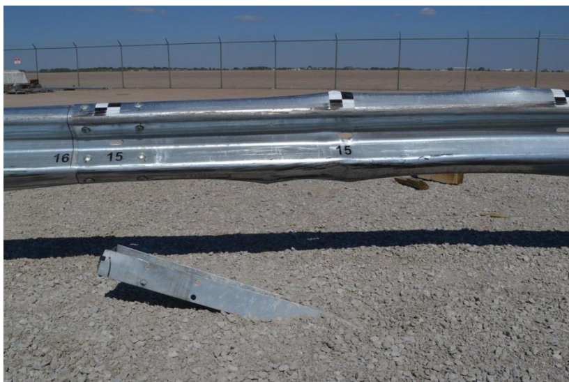
Figure 27. Post nos. 14 through 17 Damage, Test No. MGSMP-1
