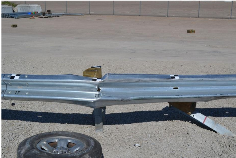
Figure 25. Rail Damage Between Post Nos. 12 and 17, Test No. MGSMP-1
