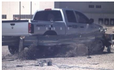
Figure 20. Additional Sequential Photographs, Test No. MGSMP-1
