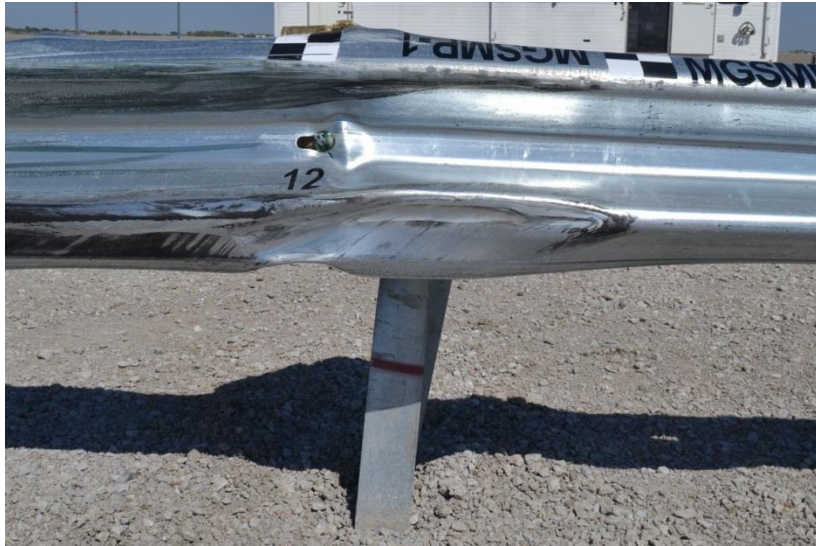
Figure 26. Post nos. 7 through 13 Damage, Test No. MGSMP-1
