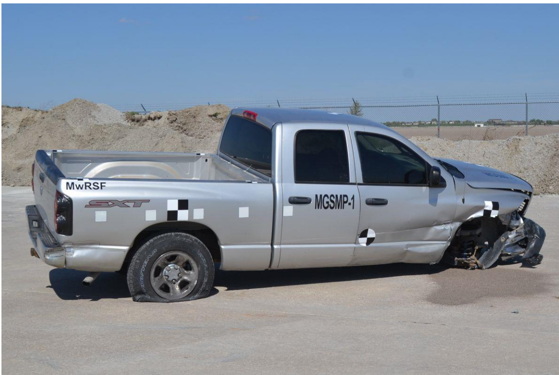
Figure 23. Vehicle Final Position and Trajectory, Test No. MGSM-1
