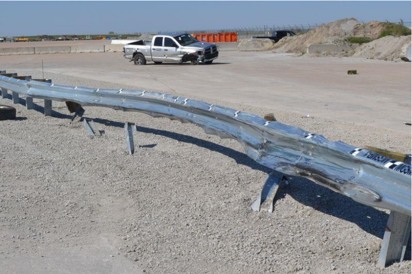
Figure 24. System Damage, Test No. MGSMP-1
