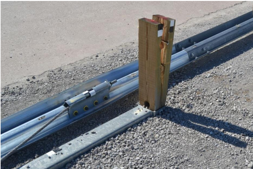
Figure 28. Upstream Anchor Damage, Test No. MGSMP-1
