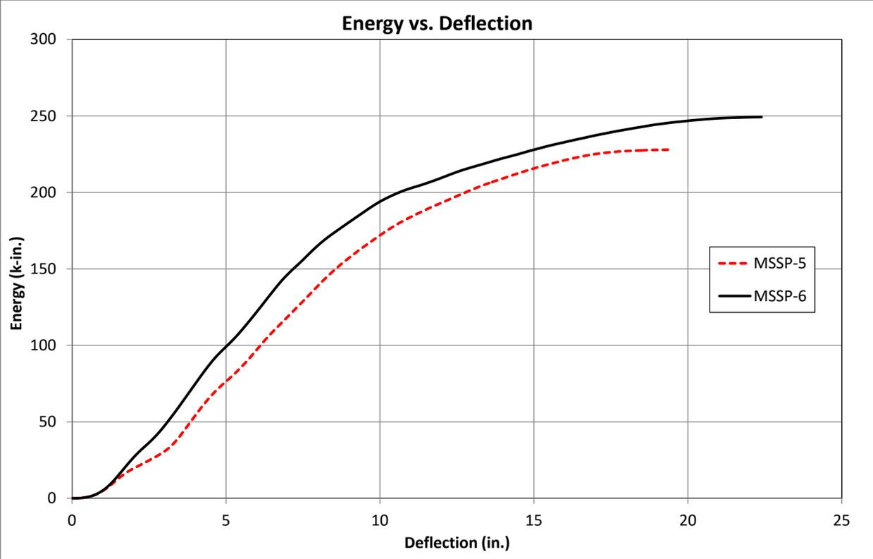
Figure 54. Energy vs. Deflection Comparison, Component Testing - Round 3
