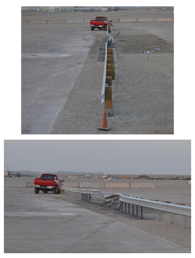
Figure 81. Vehicle Final Position and Trajectory Marks, Test No. MGSMS-1
