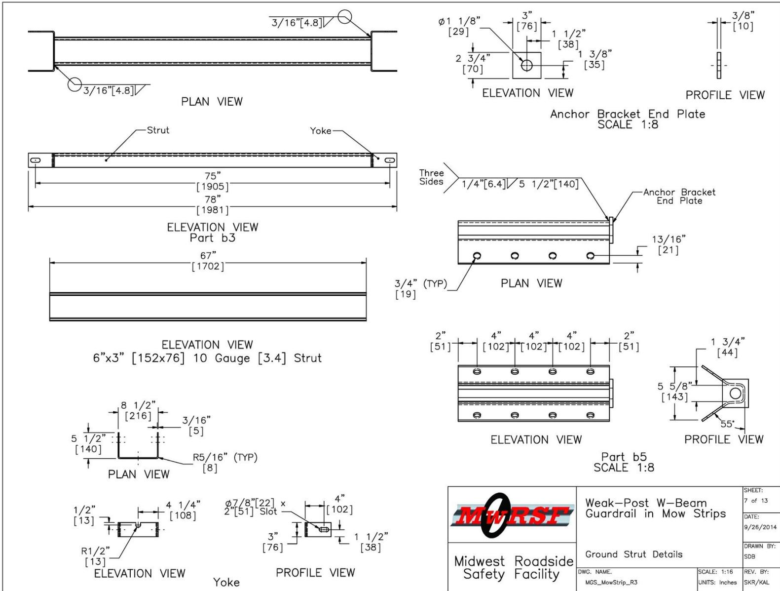
Figure 61. Anchorage Components Details, Test No. MGSMS-1
