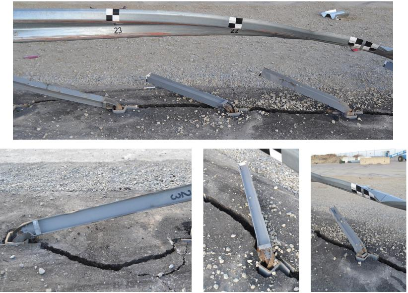
Figure 85. System Damage – Post Nos. 21 Through 23, Test No. MGSMS-1
