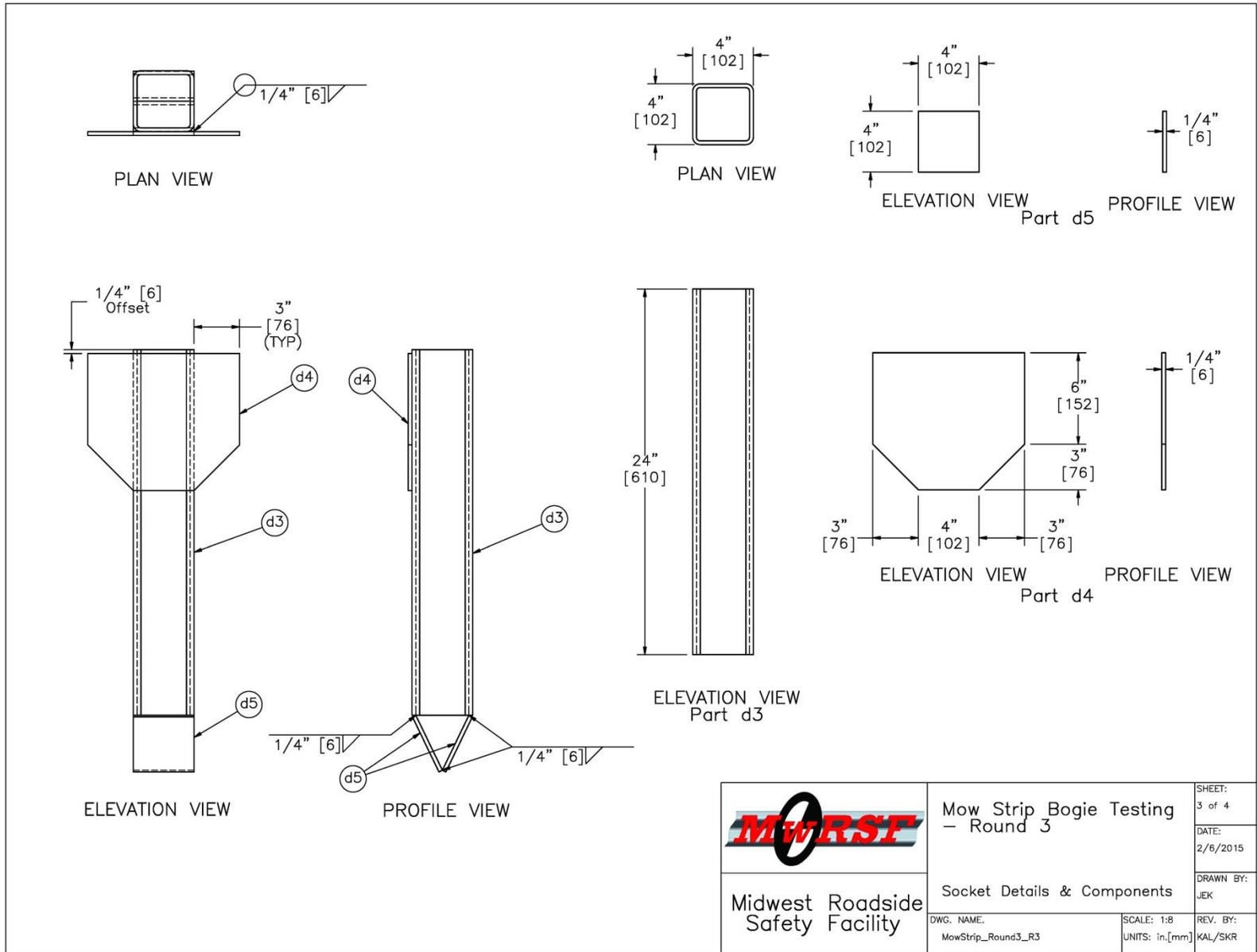
Figure 45. Post Socket Details, Component Testing Round 3
