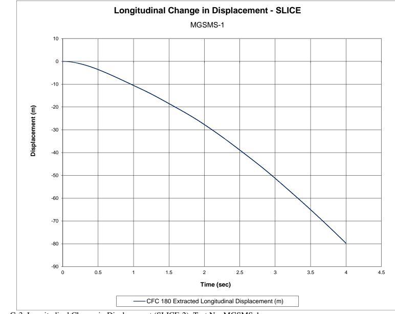
Figure G-3. Longitudinal Change in Displacement (SLICE-2), Test No. MGSMS-1
