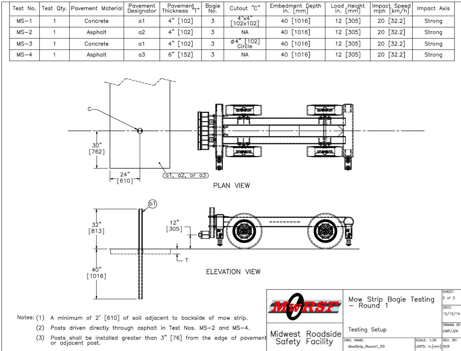
Figure 5. Bogie Testing Matrix and Setup, Component Testing Round 1
