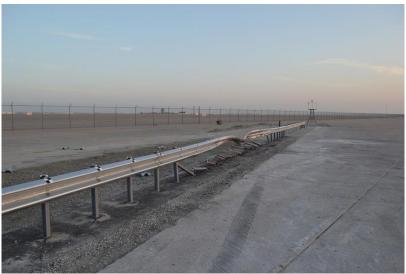
Figure 82. System Damage, Test No. MGSMS-1
