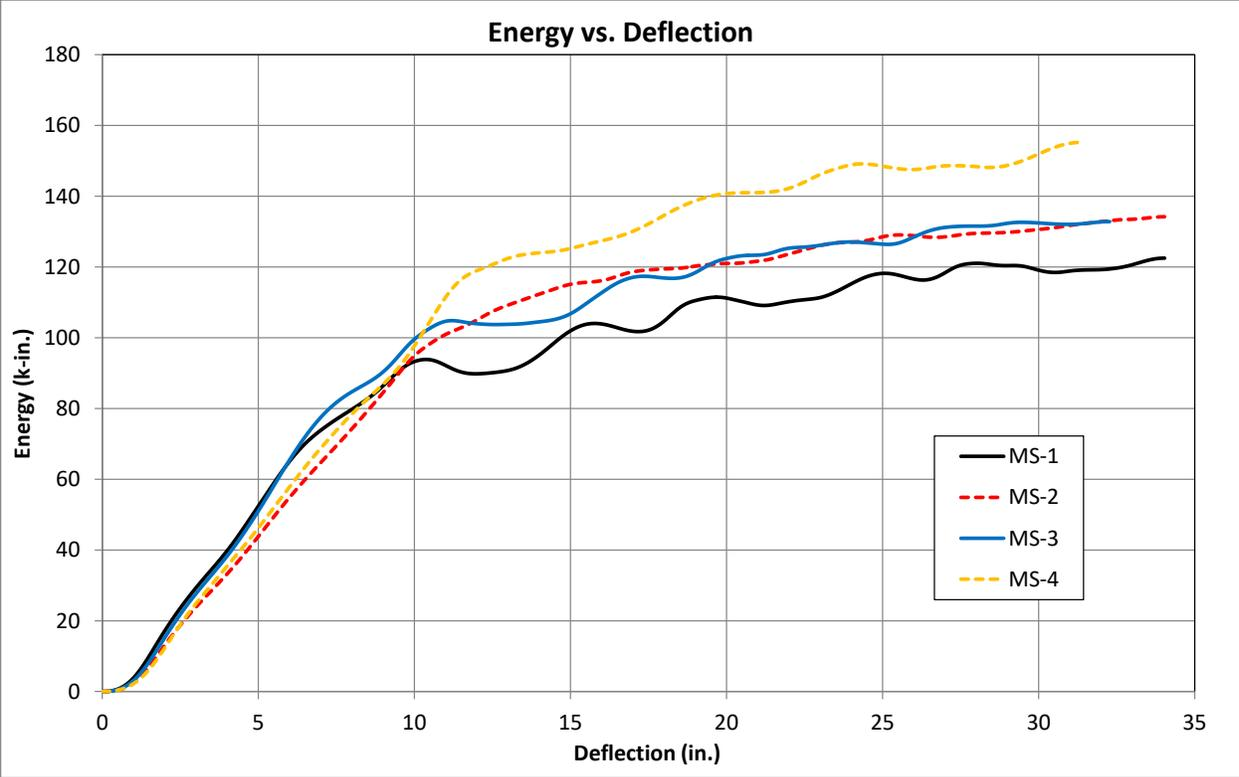
Figure 20. Energy vs. Deflection Comparison, Component Testing - Round 1
