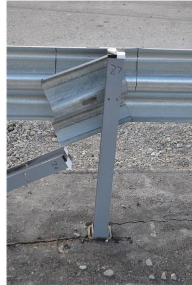
Figure 86. System Damage – Post Nos. 24 Through 29, Test No. MGSMS-1
