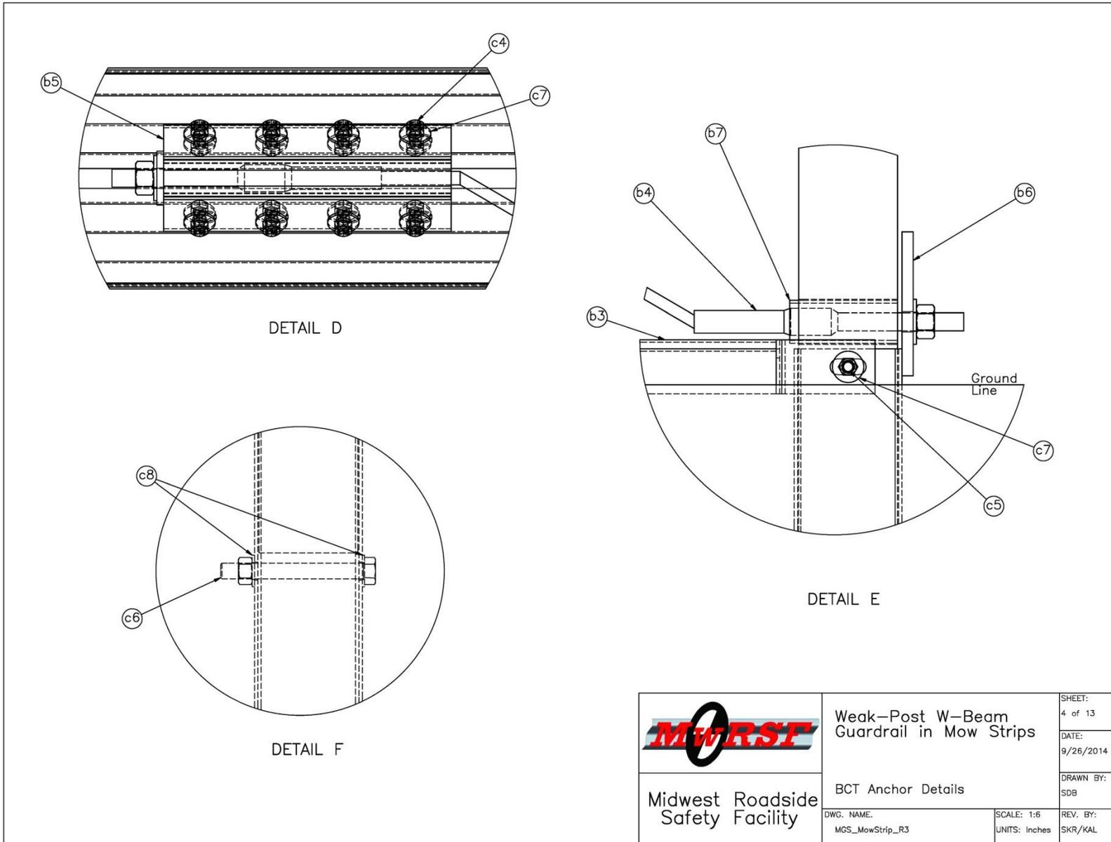
Figure 58. Anchorage Component Details, Test No. MGSMS-1
