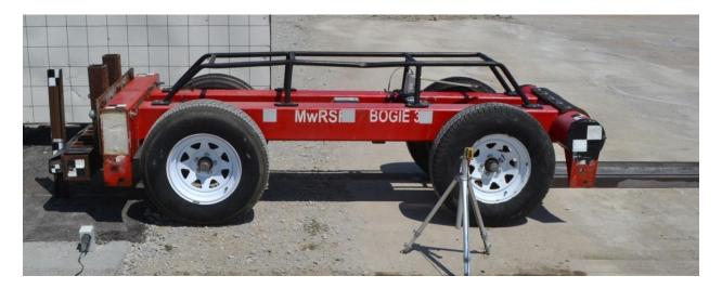
Figure 3. Rigid-Frame Bogie on Guidance Track
