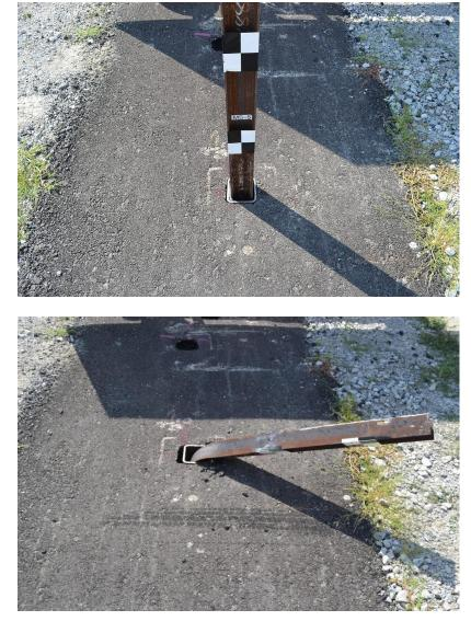
Figure 28. Pre- and Post-Impact Photographs, Test No. MS-5
