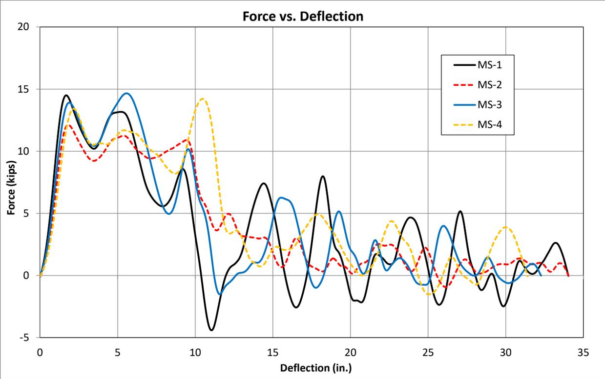
Figure 19. Force vs. Deflection Comparison, Component Testing - Round 1
