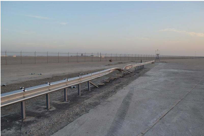
Figure 82. System Damage, Test No. MGSMS-1
