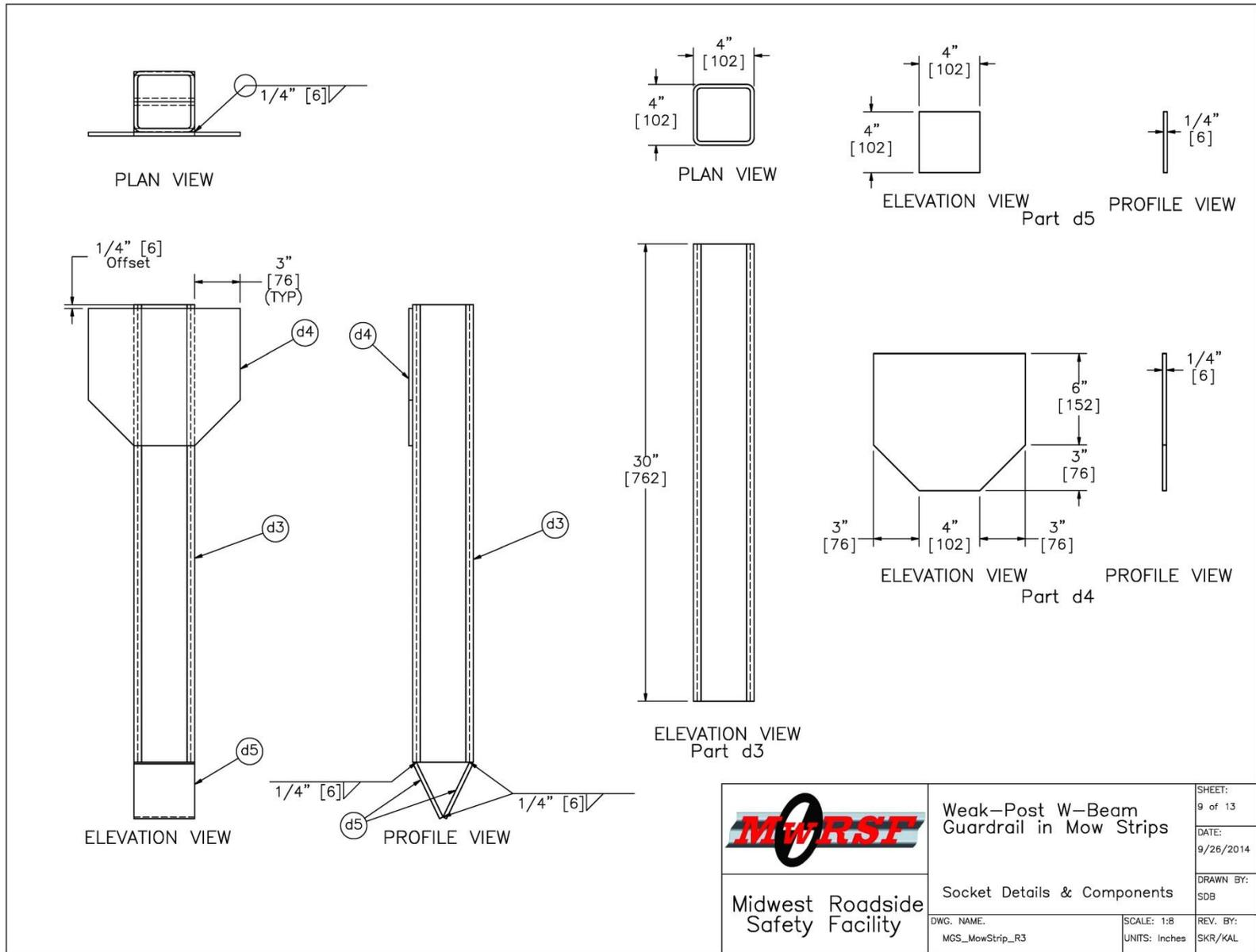
Figure 63. Post Socket Details, Test No. MGSMS-1
