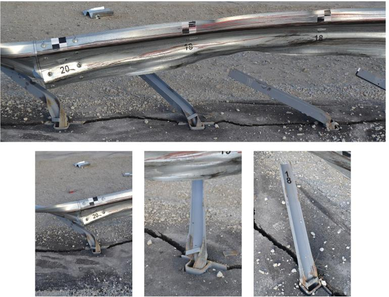
Figure 84. System Damage – Post Nos. 18 Through 20, Test No. MGSMS-1
