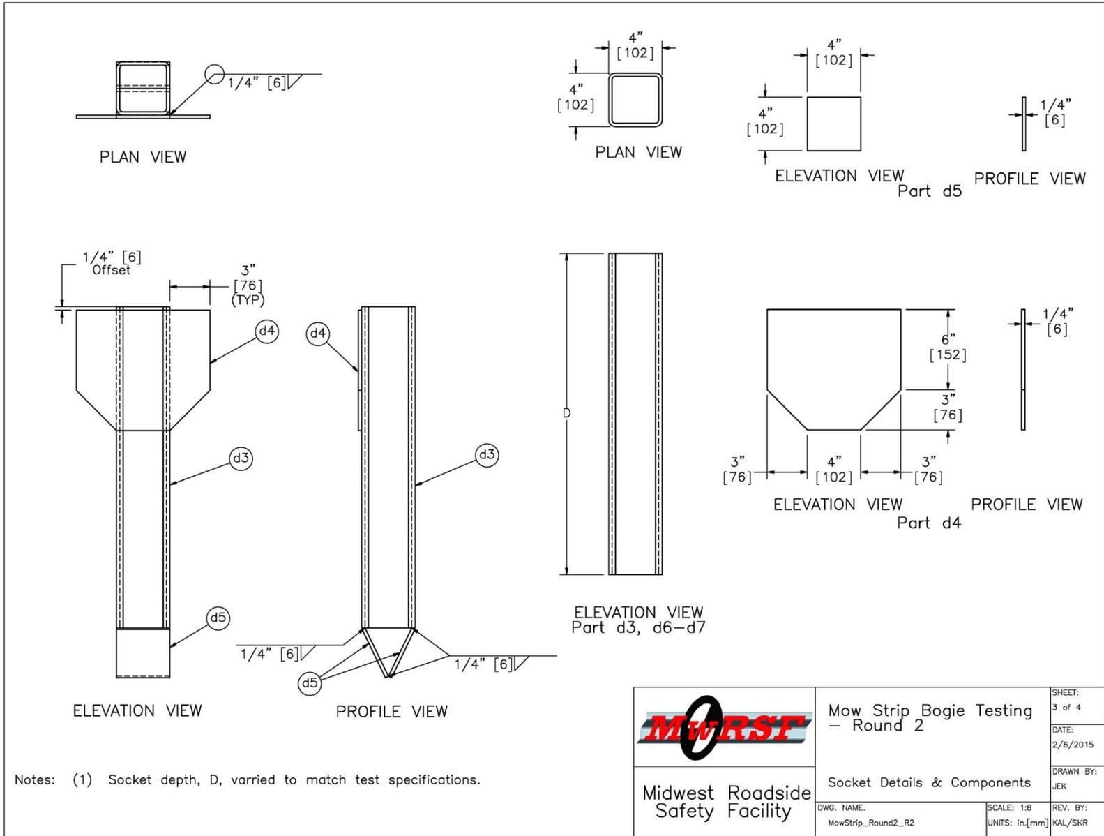
Figure 23. Post Socket Details, Component Testing Round 2
