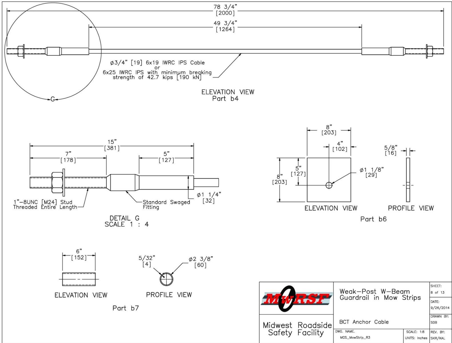
Figure 62. Cable Anchor Details, Test No. MGSMS-1
