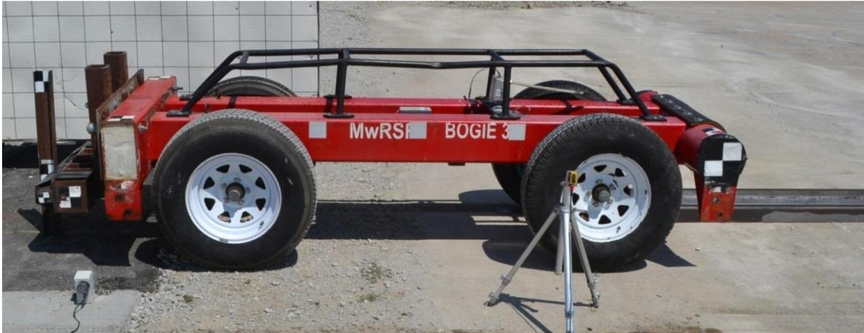
Figure 3. Rigid-Frame Bogie on Guidance Track
