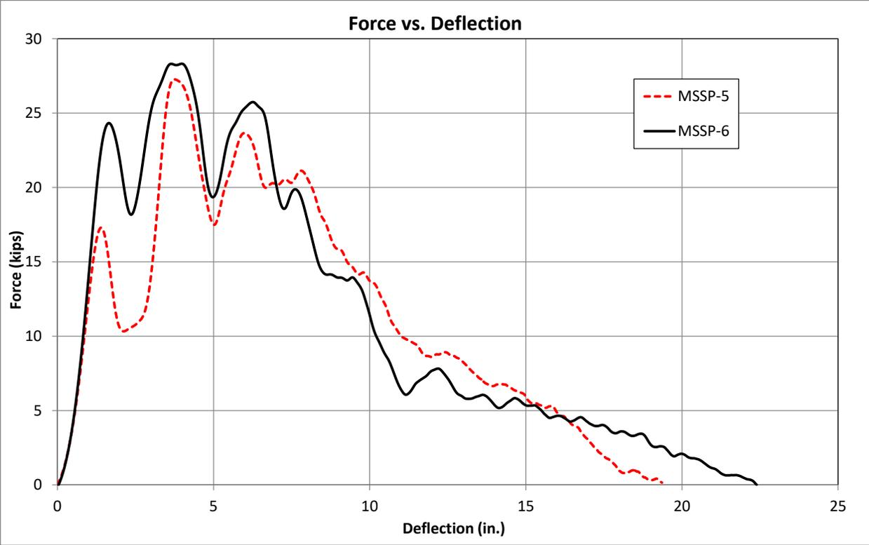
Figure 53. Force vs. Deflection Comparison, Component Testing - Round 3
