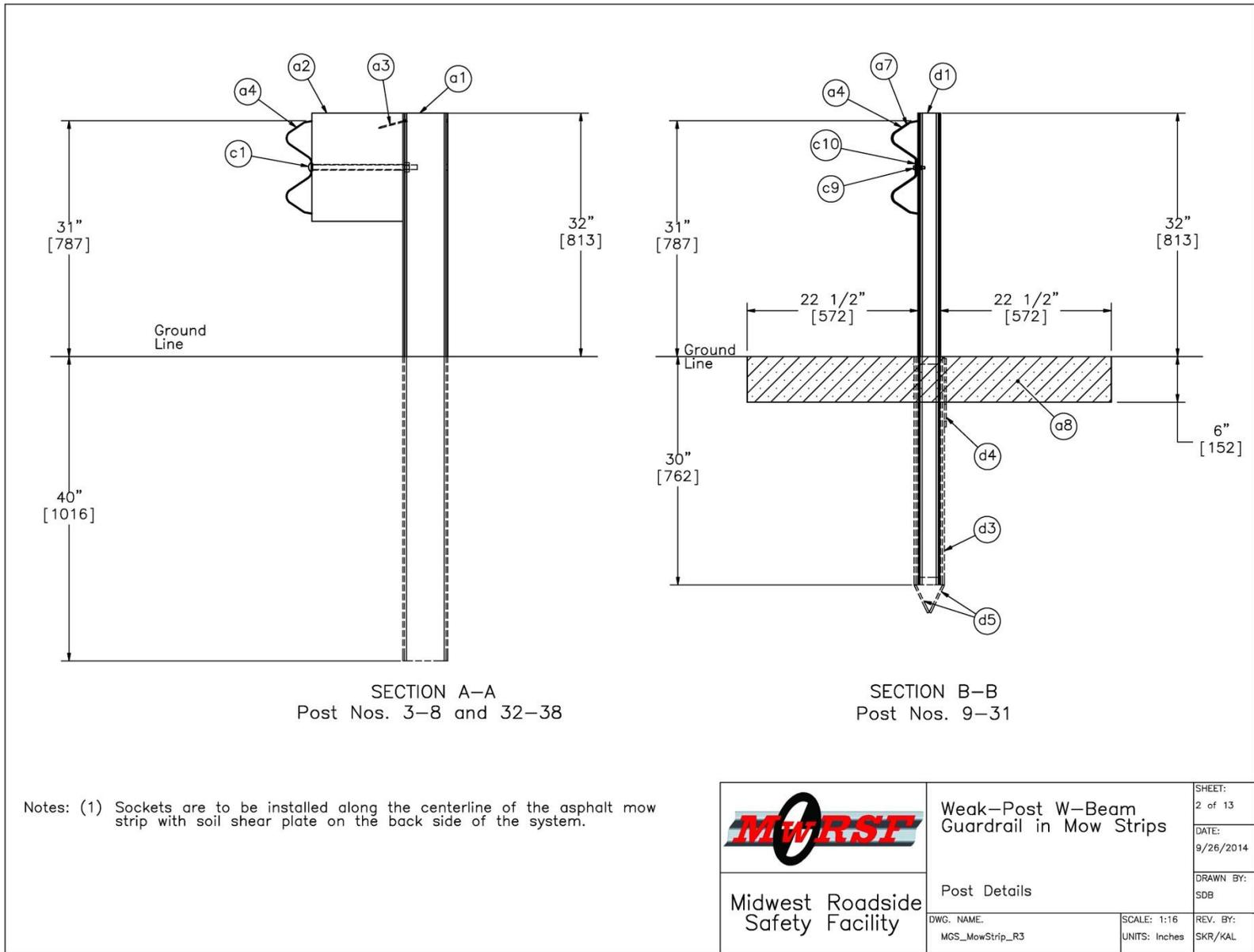
Figure 56. Guardrail Post Details, Test No. MGSMS-1
