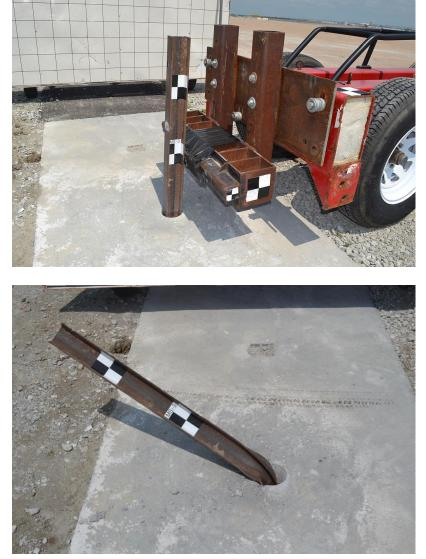
Figure 15. Pre- and Post-Impact Photographs, Test No. MS-3
