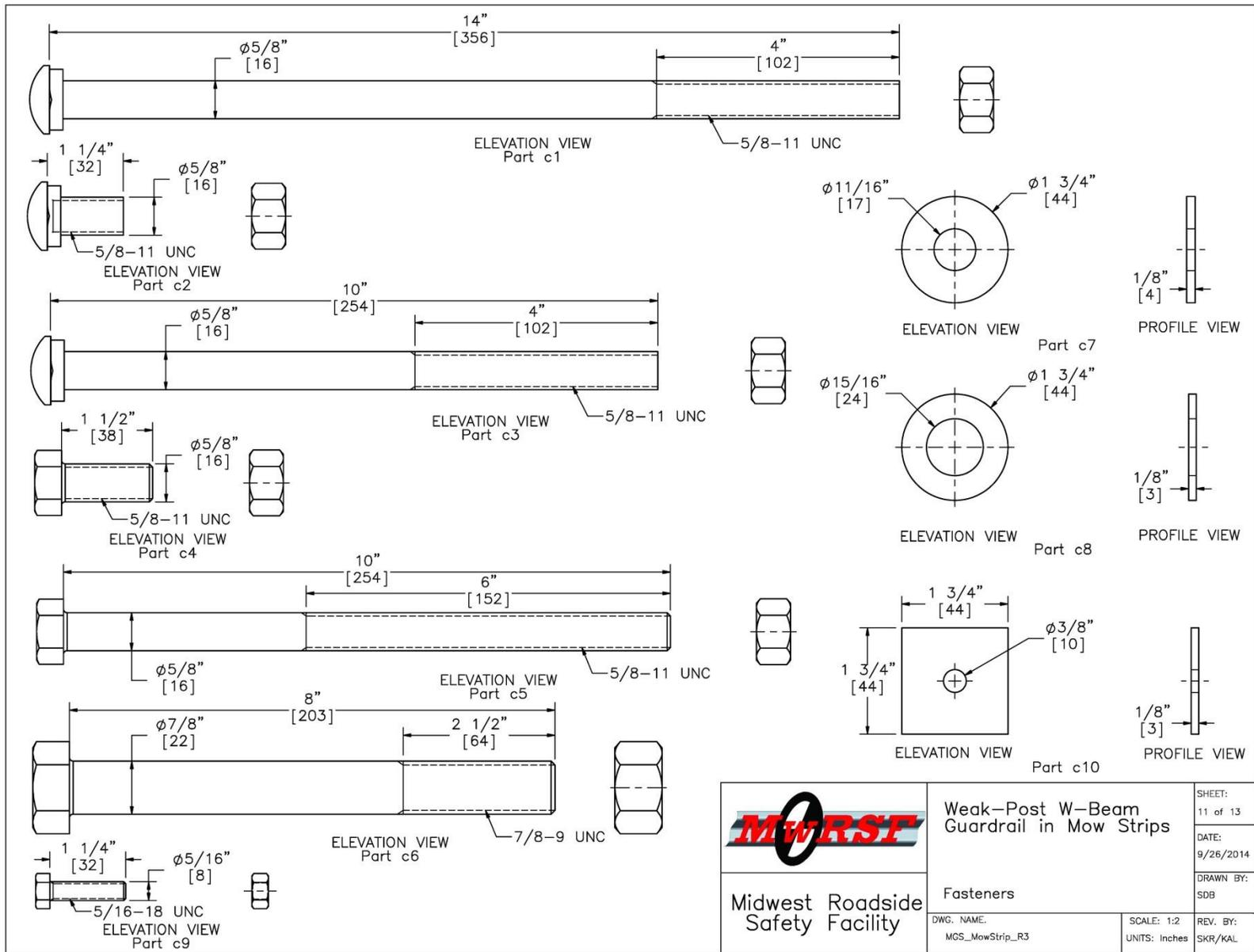
Figure 65. Attachment Hardware Details, Test No. MGSMS-1
