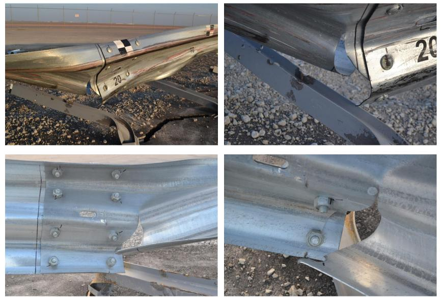
Figure 88. System Damage – Rail Tearing, Test No. MGSMS-1
