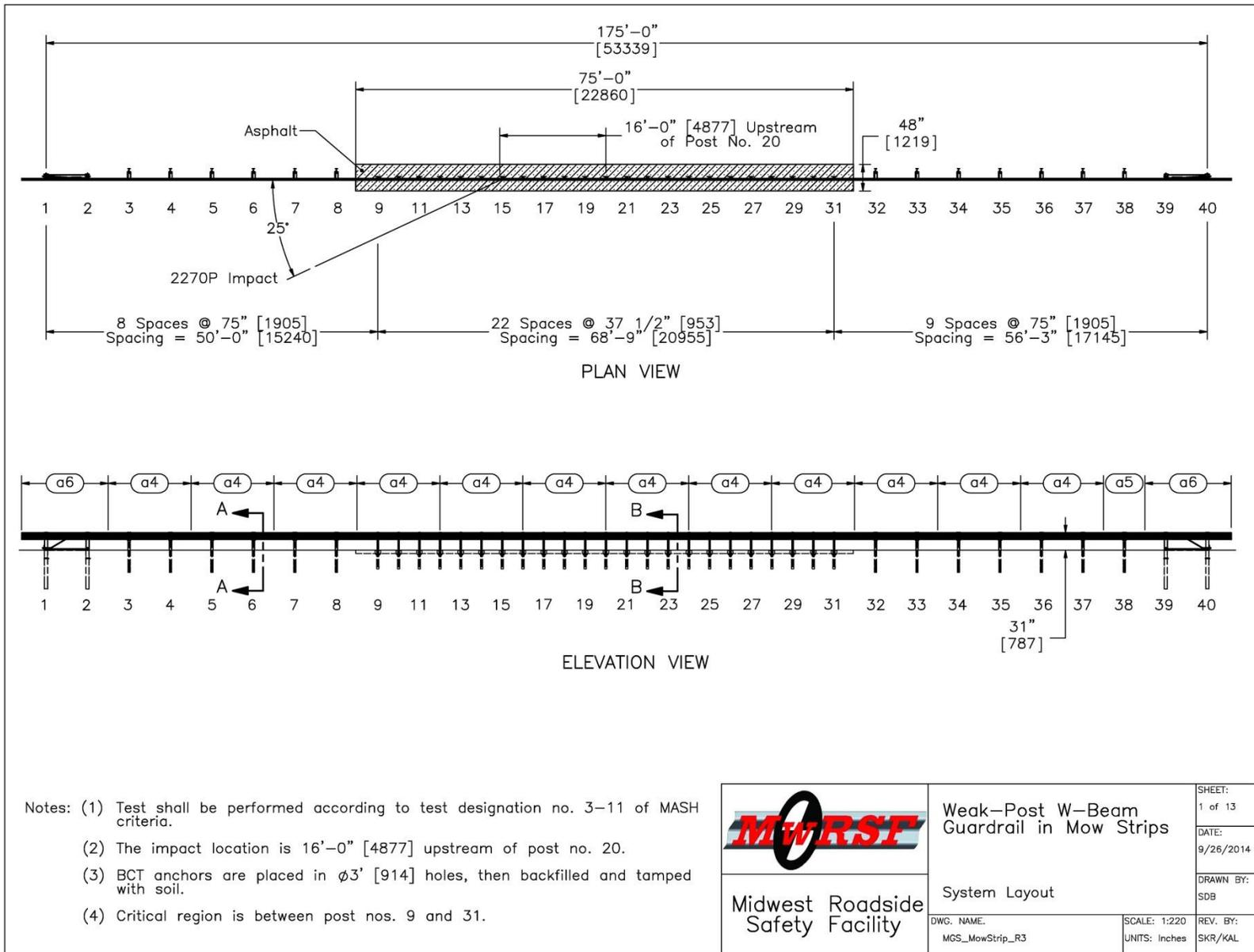
Figure 55. Test Installation Layout, Test No. MGSMS-1
