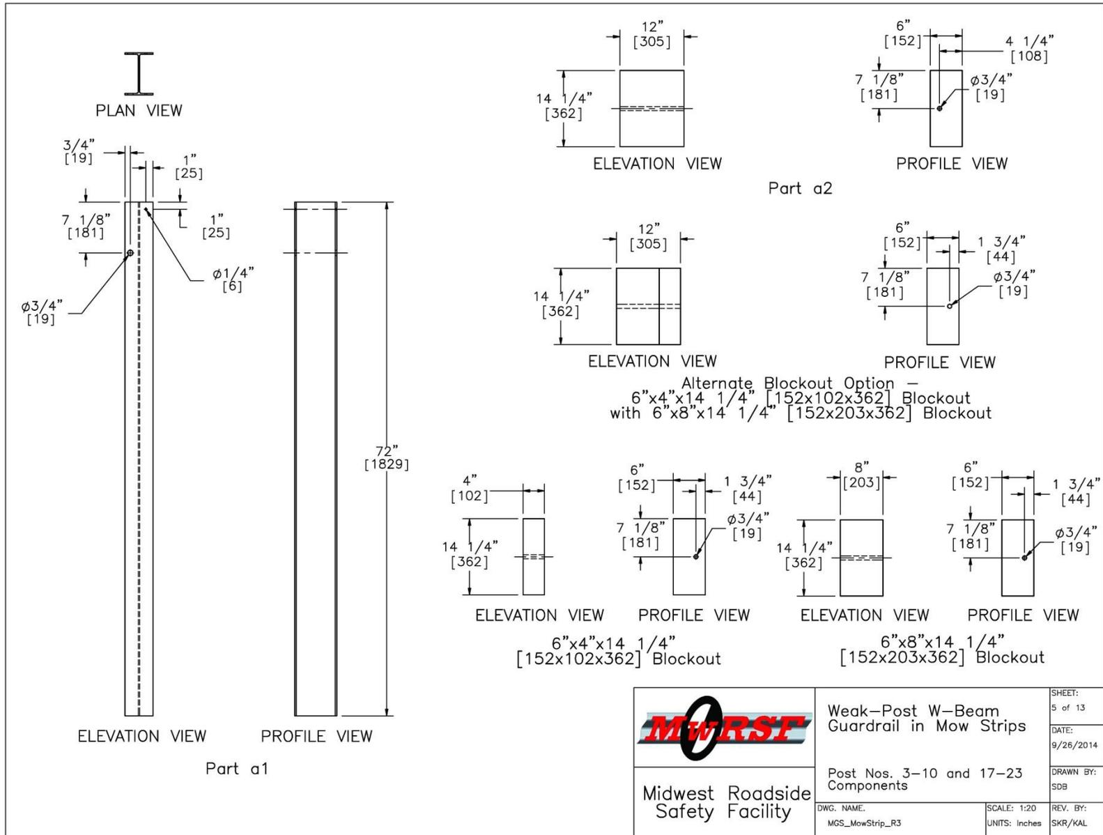
Figure 59. Post and Blockout Details, Test No. MGSMS-1
