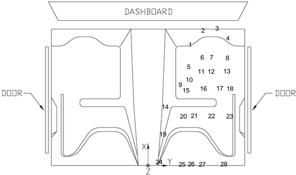
Figure F-1. Floor Pan Deformation Data, Test No. MGSMS-1
