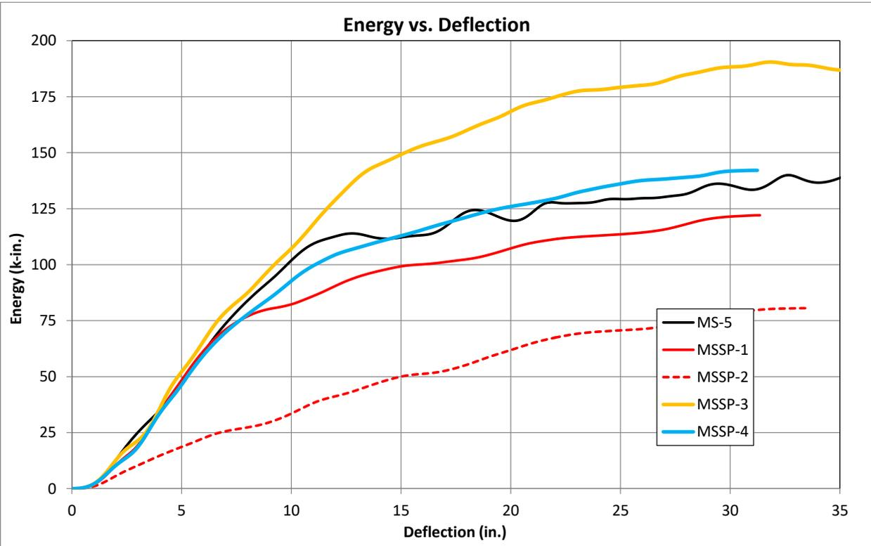
Figure 42. Energy vs. Deflection Comparison, Component Testing - Round 2
