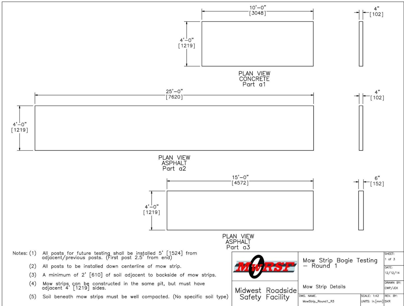
Figure 4. Testing Mow Strip Configurations, Component Testing Round 1
