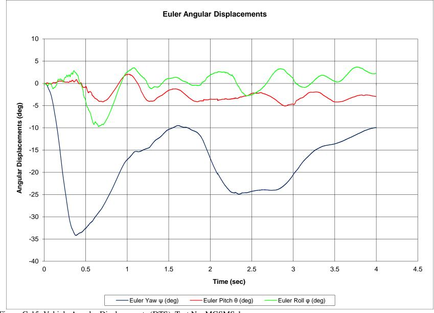
Figure G-15. Vehicle Angular Displacements (DTS), Test No. MGSMS-1
