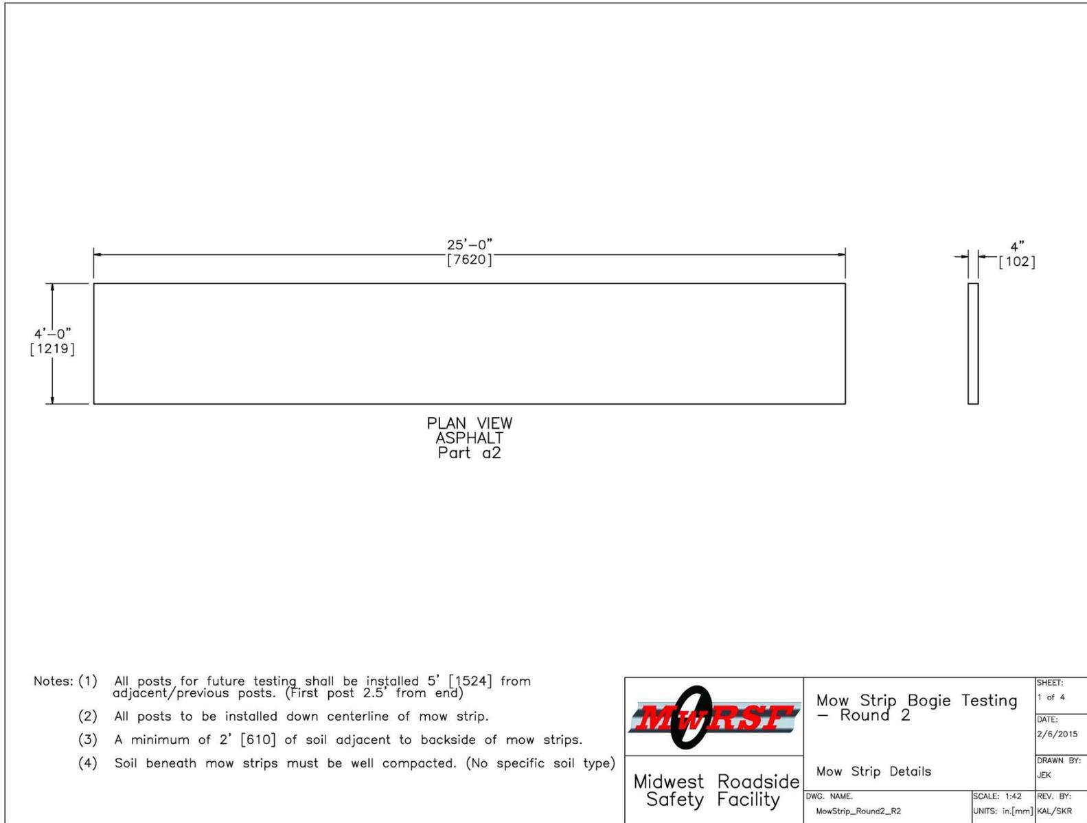
Figure 21. Mow Strip Configuration, Component Testing Round 2
