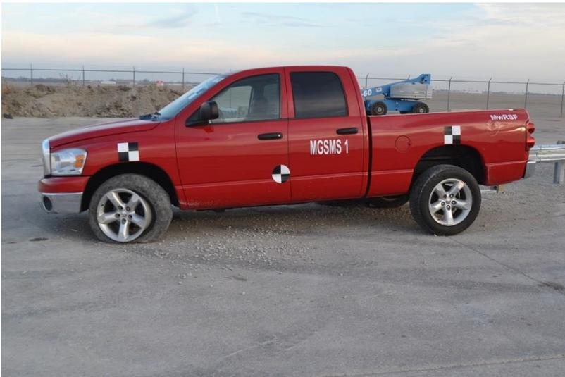
Figure 90. Vehicle Damage, Test No. MGSMS-1
