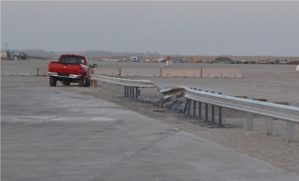
Figure 81. Vehicle Final Position and Trajectory Marks, Test No. MGSMS-1
