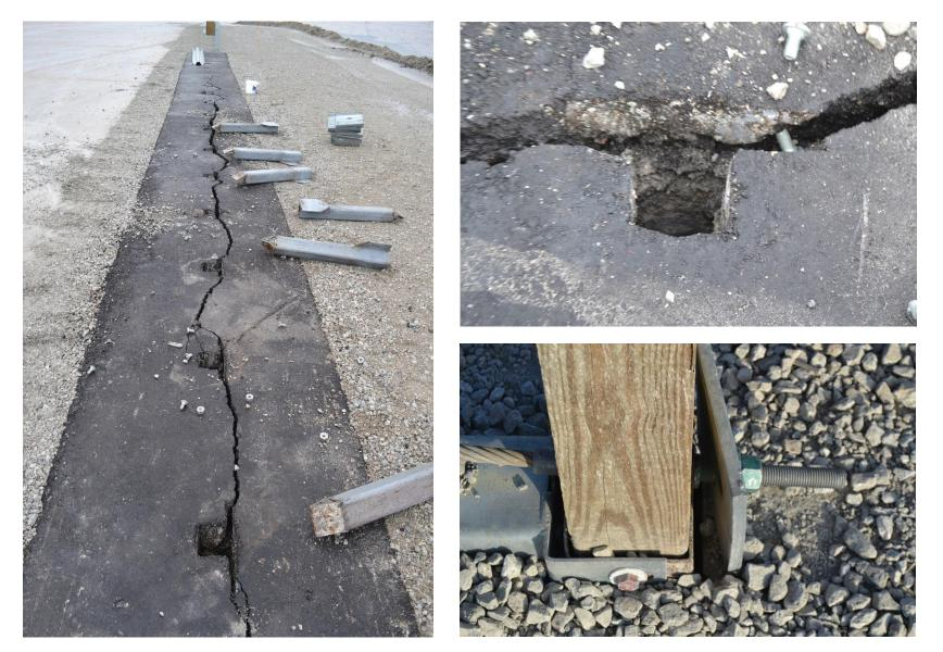
Figure 87. System Damage – Asphalt Fracture and Anchor Movement, Test No. MGSMS-1
