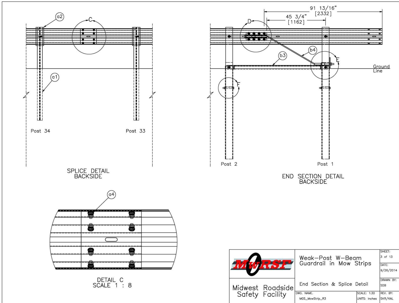
Figure 57. Anchorage and Splice Details, Test No. MGSMS-1
