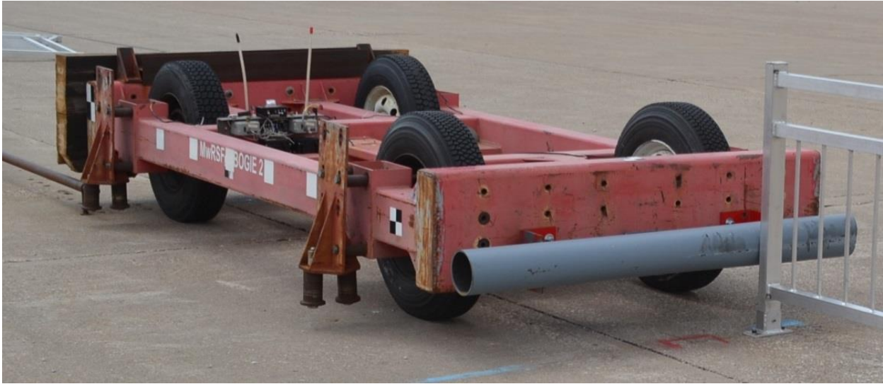
Figure 127. Rigid-Frame Bogie Vehicle on Guidance Track
