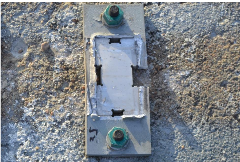
Figure 199. Panel No. 3 Damage, Test No. APR-2
