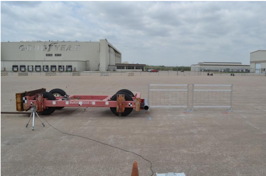
Figure 126. Typical Bogie Testing Setup
