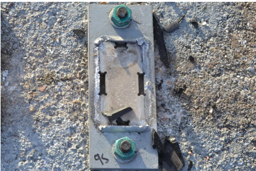
Figure 205. Panel No. 9 Damage, Test No. APR-2
