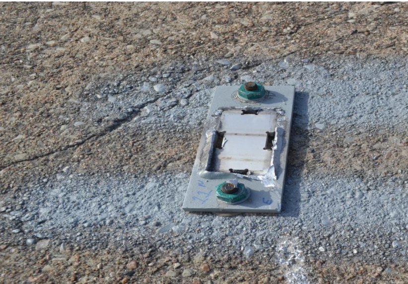
Figure 182. Panel No. 11 Damage, Test No. APR-1
