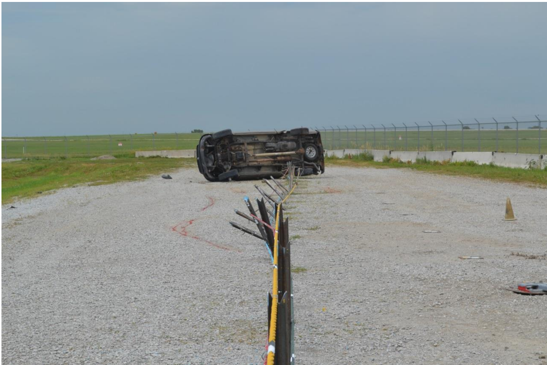
Figure 102. Vehicle Final Position and Trajectory Marks, Test No. MWP-3
