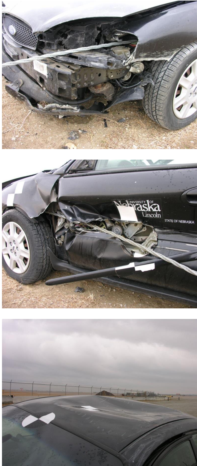
Figure 52. Vehicle Damage, Left Side and Roof, Test No. MWP-1
