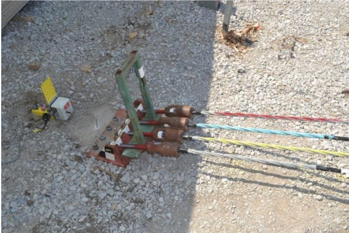
String Potentiometer, Test Nos. MWP-1 through MWP-3
