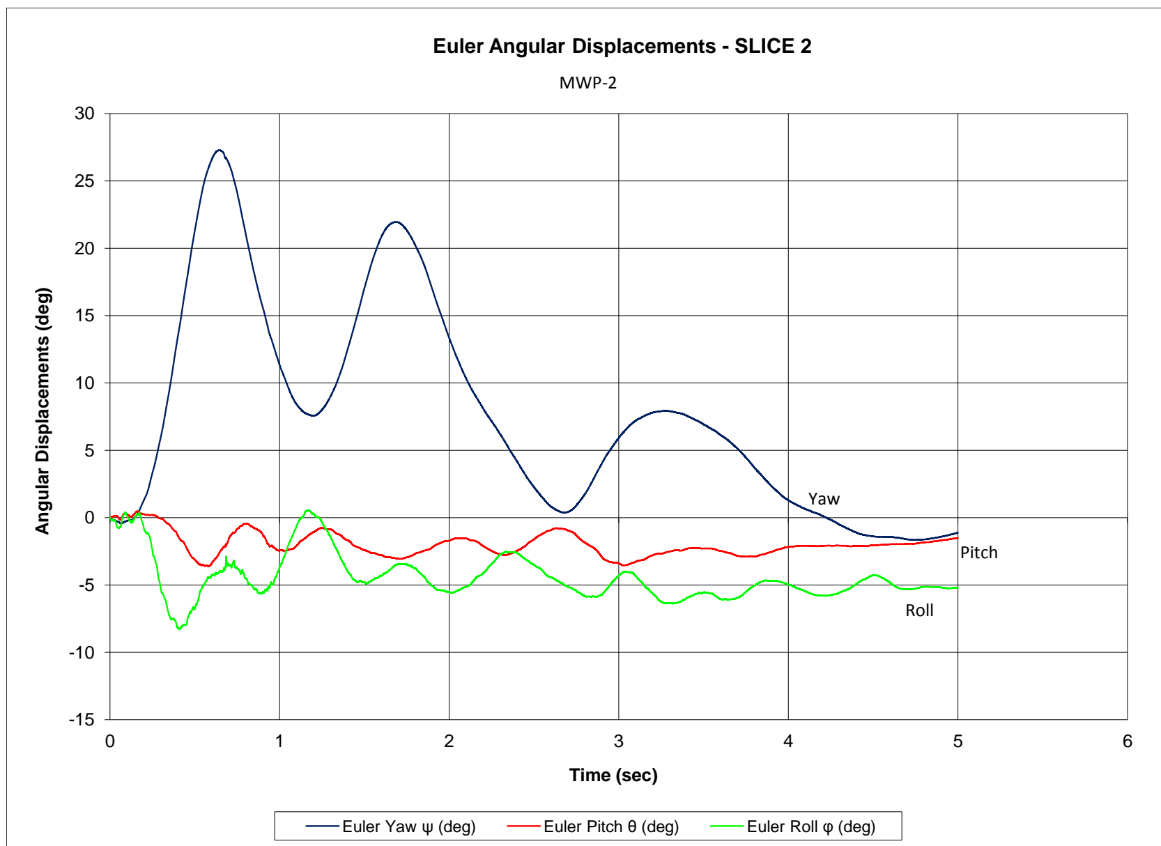
Figure G-15. Vehicle Angular Displacements (SLICE 2), Test No. MWP-2
