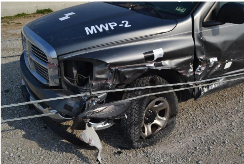
Figure 68. Vehicle Damage, Test No. MWP-2
