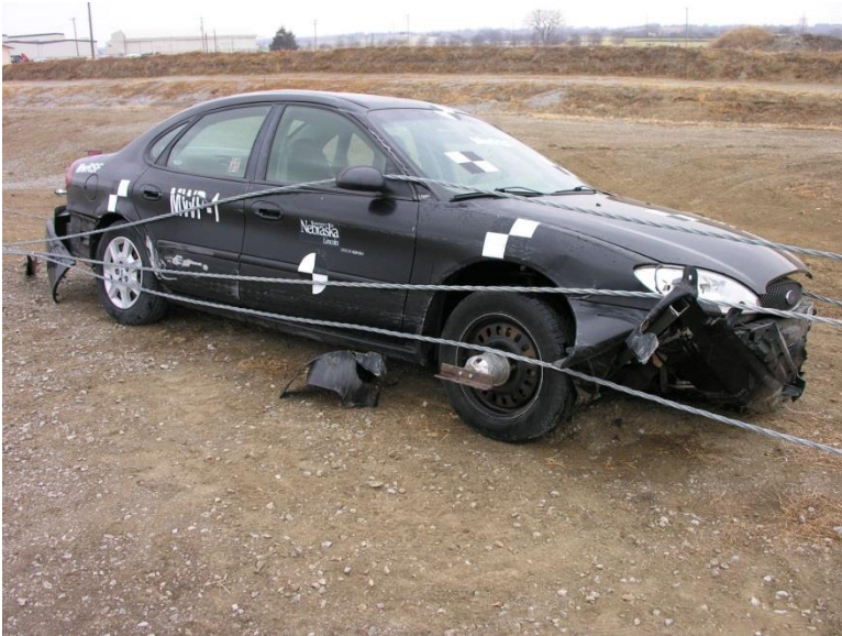
Figure 51. Vehicle Damage, Test No. MWP-1
