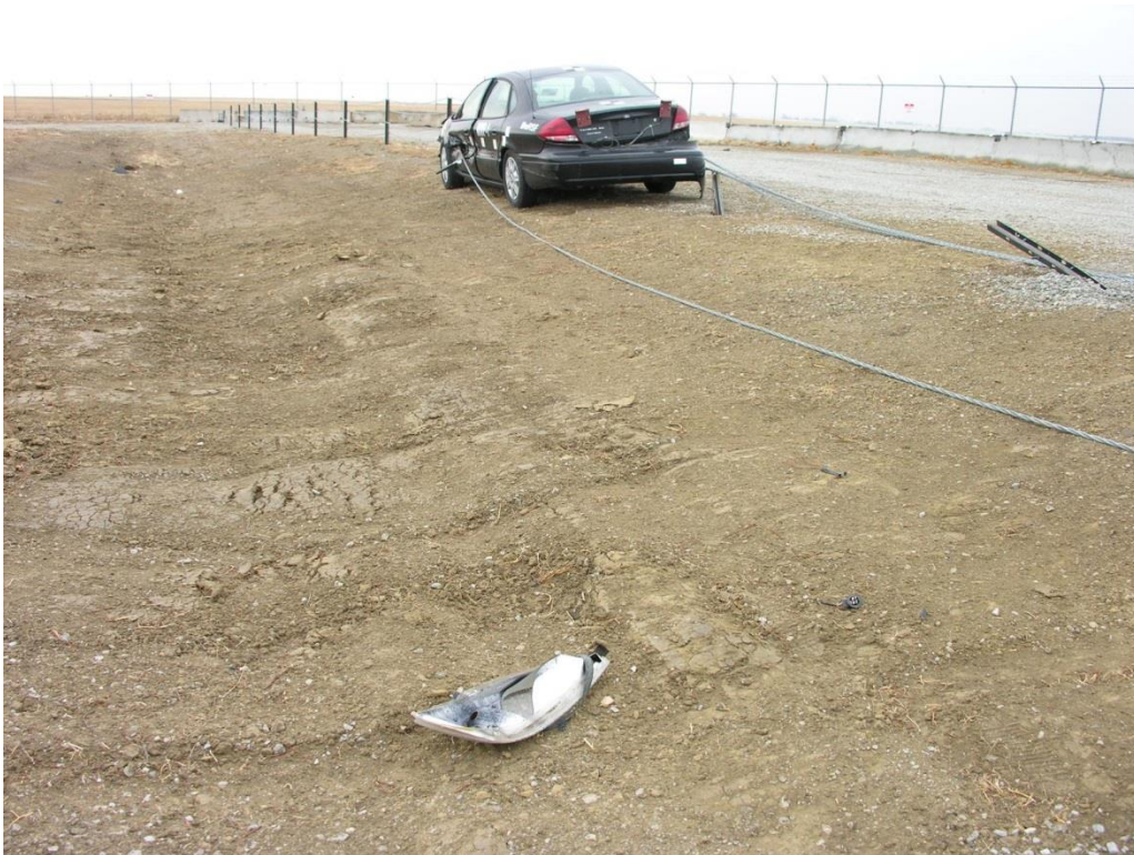
Figure 45. Vehicle Final Position and Trajectory Marks, Test No. MWP-1
