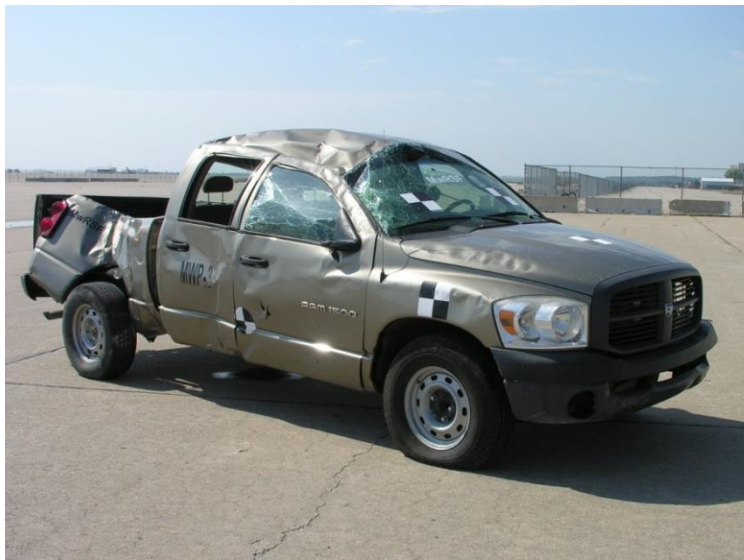
Figure 110. Vehicle Damage, Upright, Test No. MWP-3
