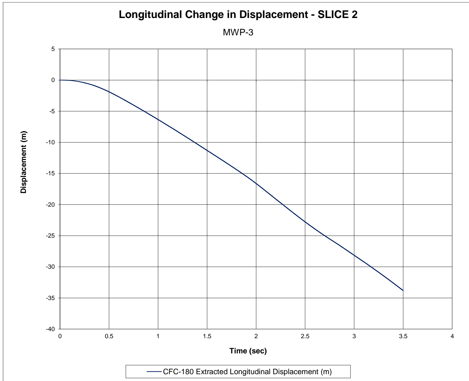
Figure I-11. Longitudinal Occupant Displacement (SLICE 2), Test No. MWP-3
