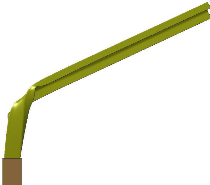
Figure 86. Deformed Post Shape, Test Nos. 4CMBC-11 and 4CMBC-12, and LS-DYNA Simulation
