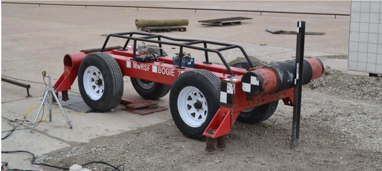
Figure 4. Rigid Frame Bogie and Guidance Track
