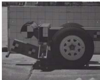
Figure 11. Strong-Axis CRT Post Impact, LS-DYNA Simulation vs Bogie Test
