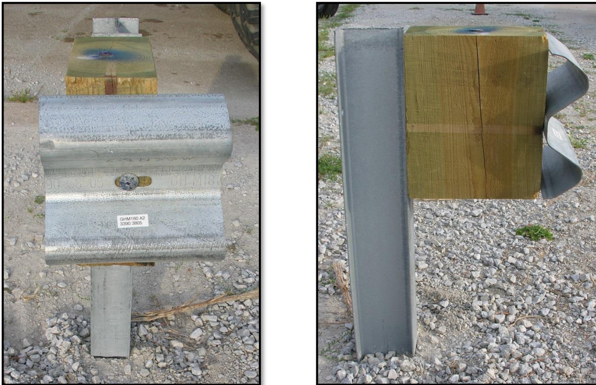
Figure 114. Test Setup to Measure Guardrail Bolt Torque
