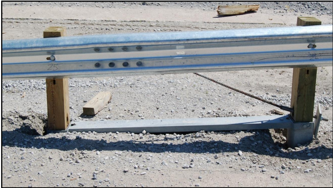
(a) Downstream Anchor, Test No. LSC-1
