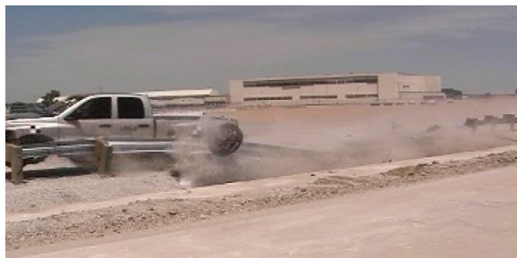
Figure 38. Sequentials – Test No. LSC-2 and LS-DYNA Simulation with Silverado-v3r-SF
