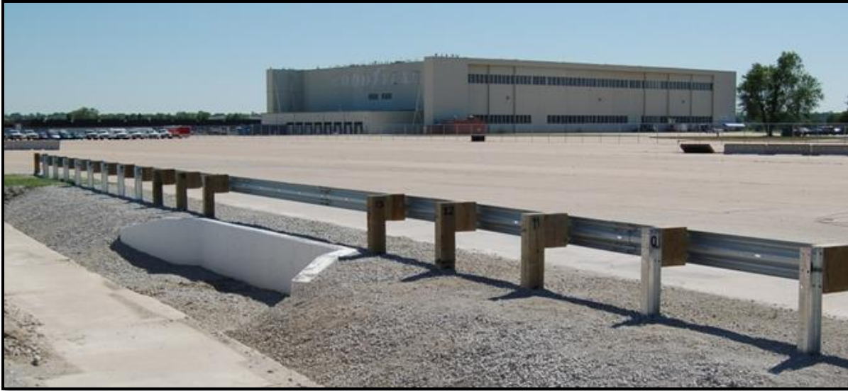
Figure 1. Midwest Guardrail System 25-ft Long-Span Design
