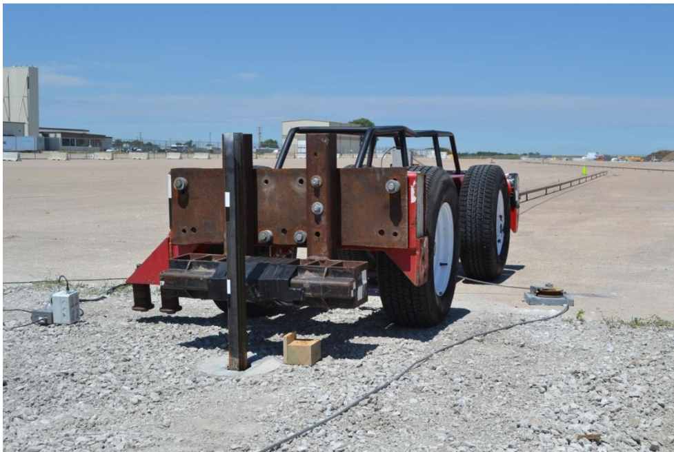
Figure 13. Rigid-Frame Bogie on Guidance Track
