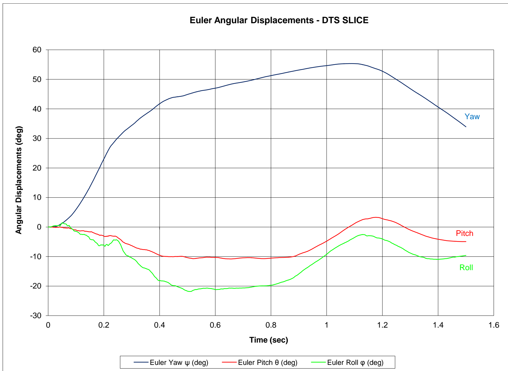
Figure G-15. Figure 102. Vehicle Angular Displacements (DTS SLICE), Test No. MWTC-3
