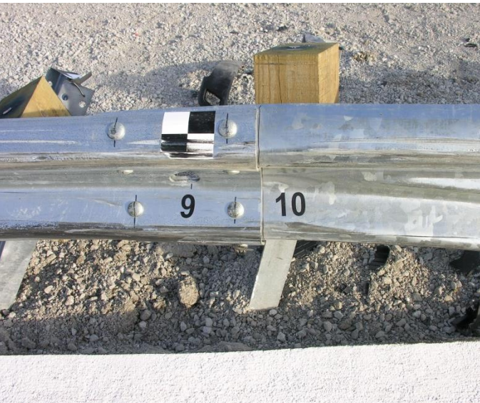
Figure 91. Post and Blockout System Damage, Test No. MWTC-2
