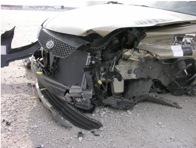
Figure 92. Vehicle Damage, Test No. MWTC-2
