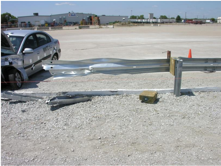
Figure 51. Rail Pocketing and Rupture, Test No. MWTC-1
