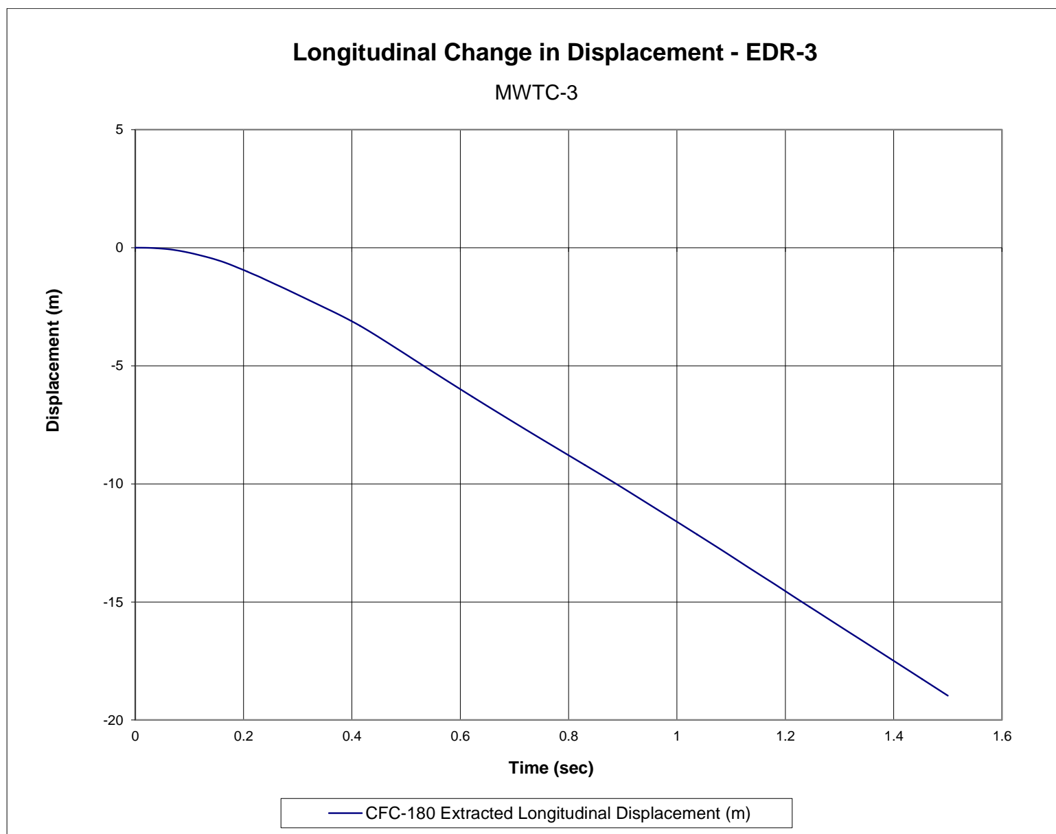
Figure G-19. Longitudinal Occupant Displacement (EDR-3), Test No. MWTC-3
