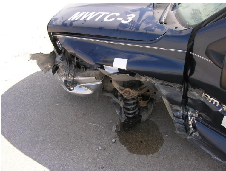
Figure 101. Vehicle Damage, Test No. MWTC-3
