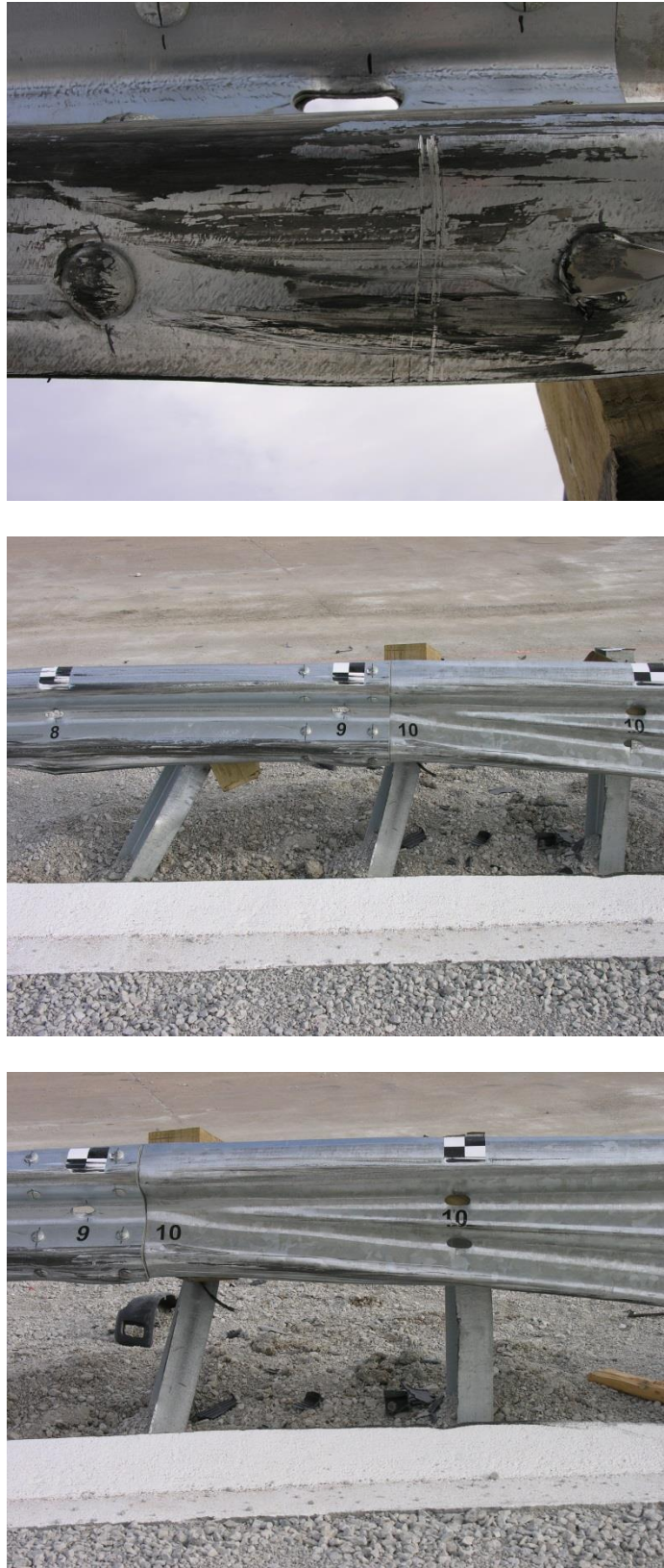
Figure 90. Rail System Damage, Test No. MWTC-2
