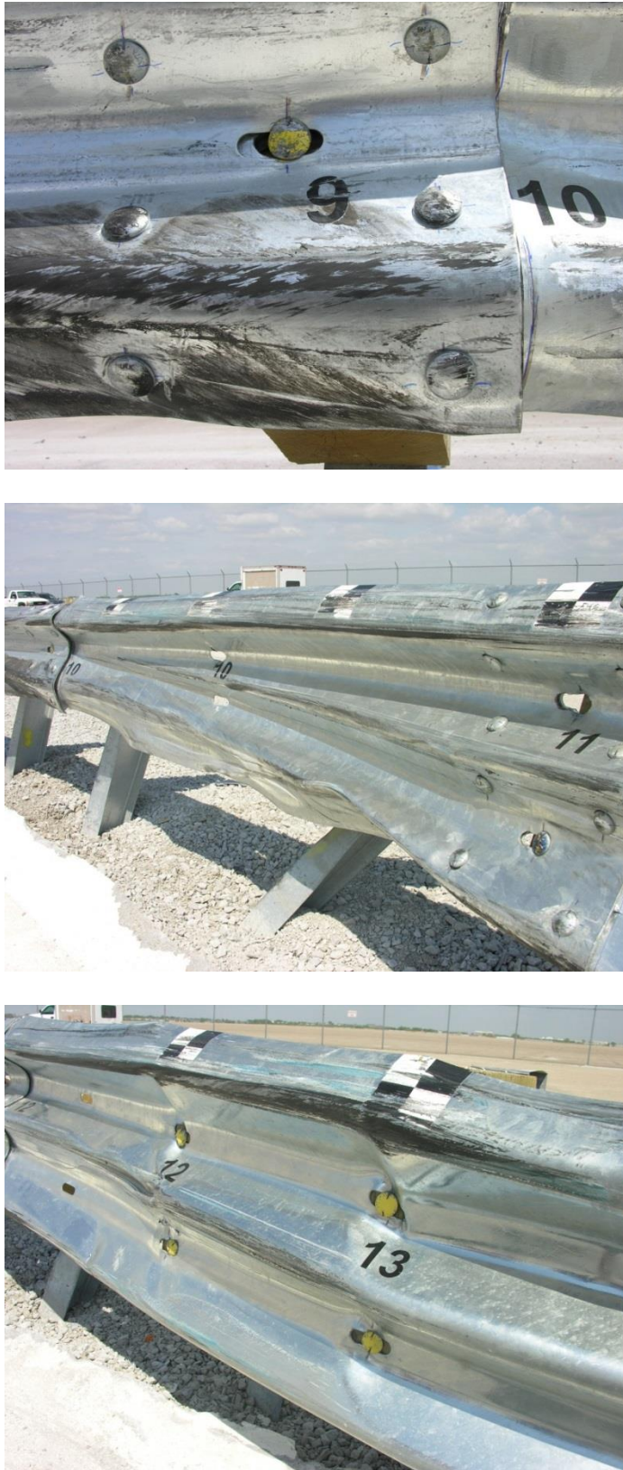
Figure 99. System Damage, Test No. MWTC-3
