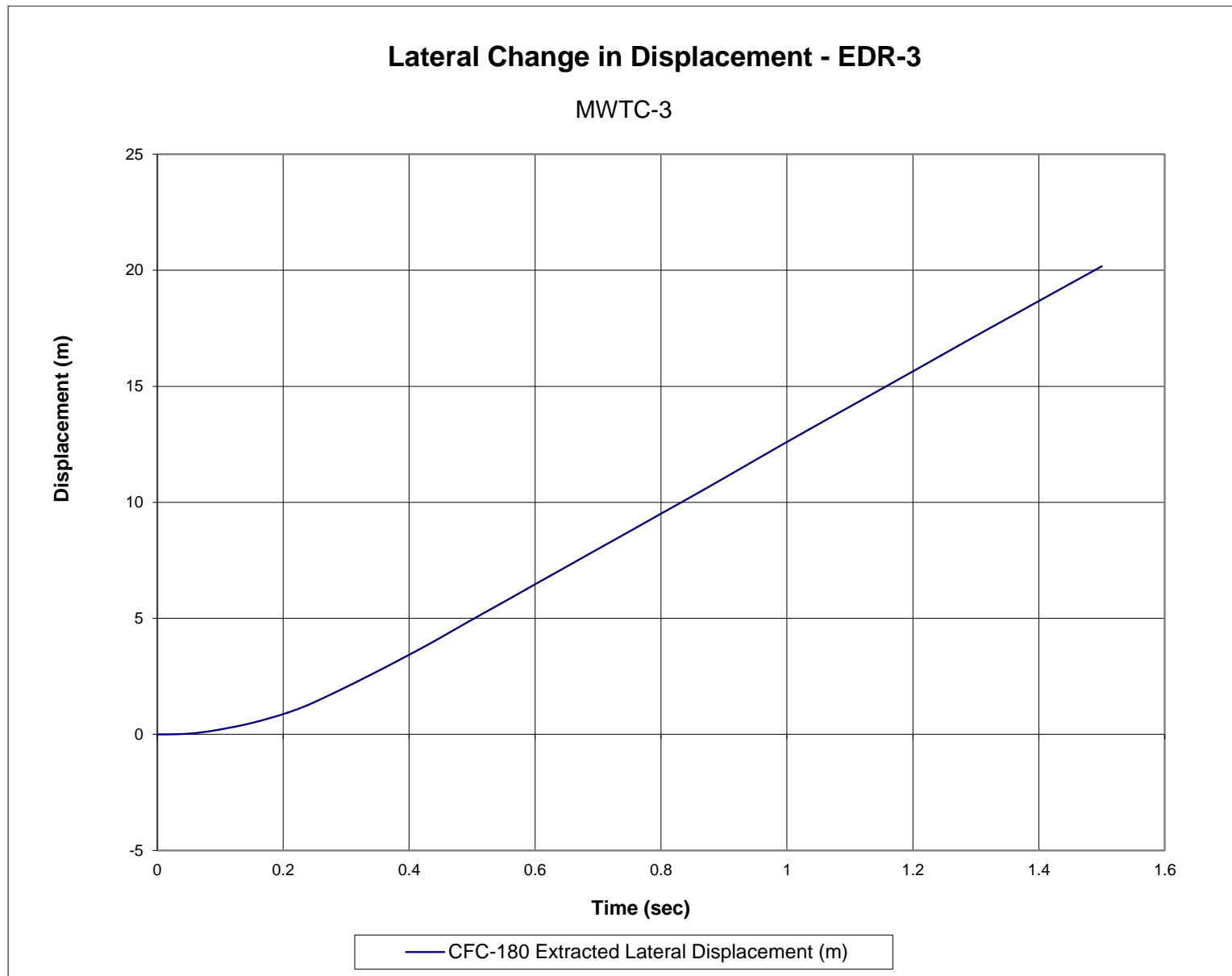
Figure G-22. Lateral Occupant Displacement (EDR-3), Test No. MWTC-3
