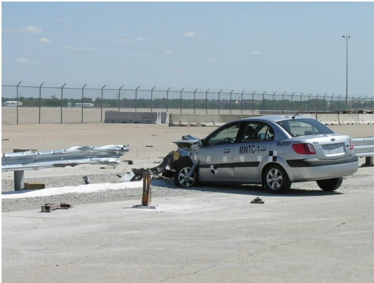
Figure 50. System Damage, Test No. MWTC-1
