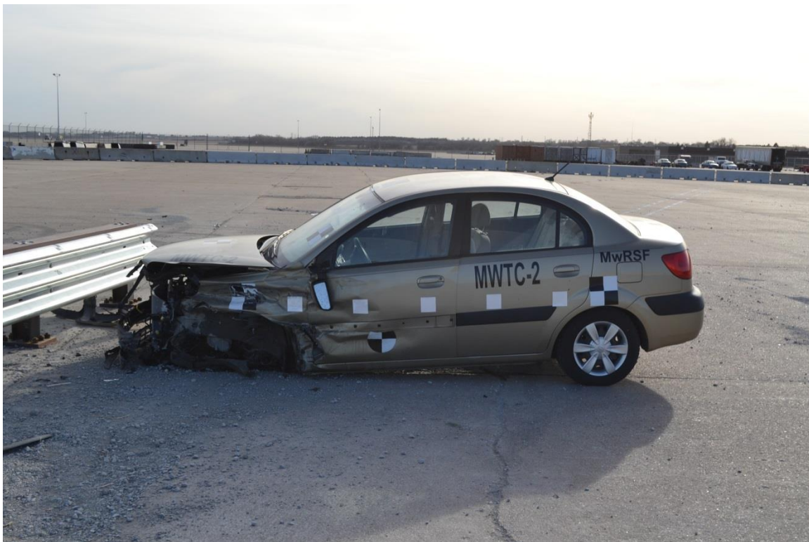
Figure 88. Vehicle Final Position, Test No. MWTC-2
