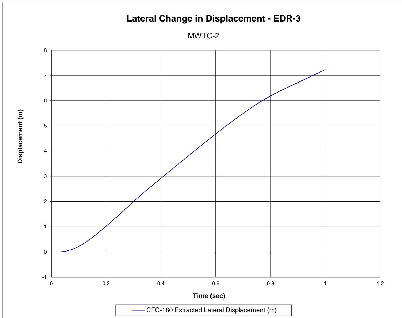
Figure F-22. Lateral Occupant Displacement (EDR-3), Test No. MWTC-2
