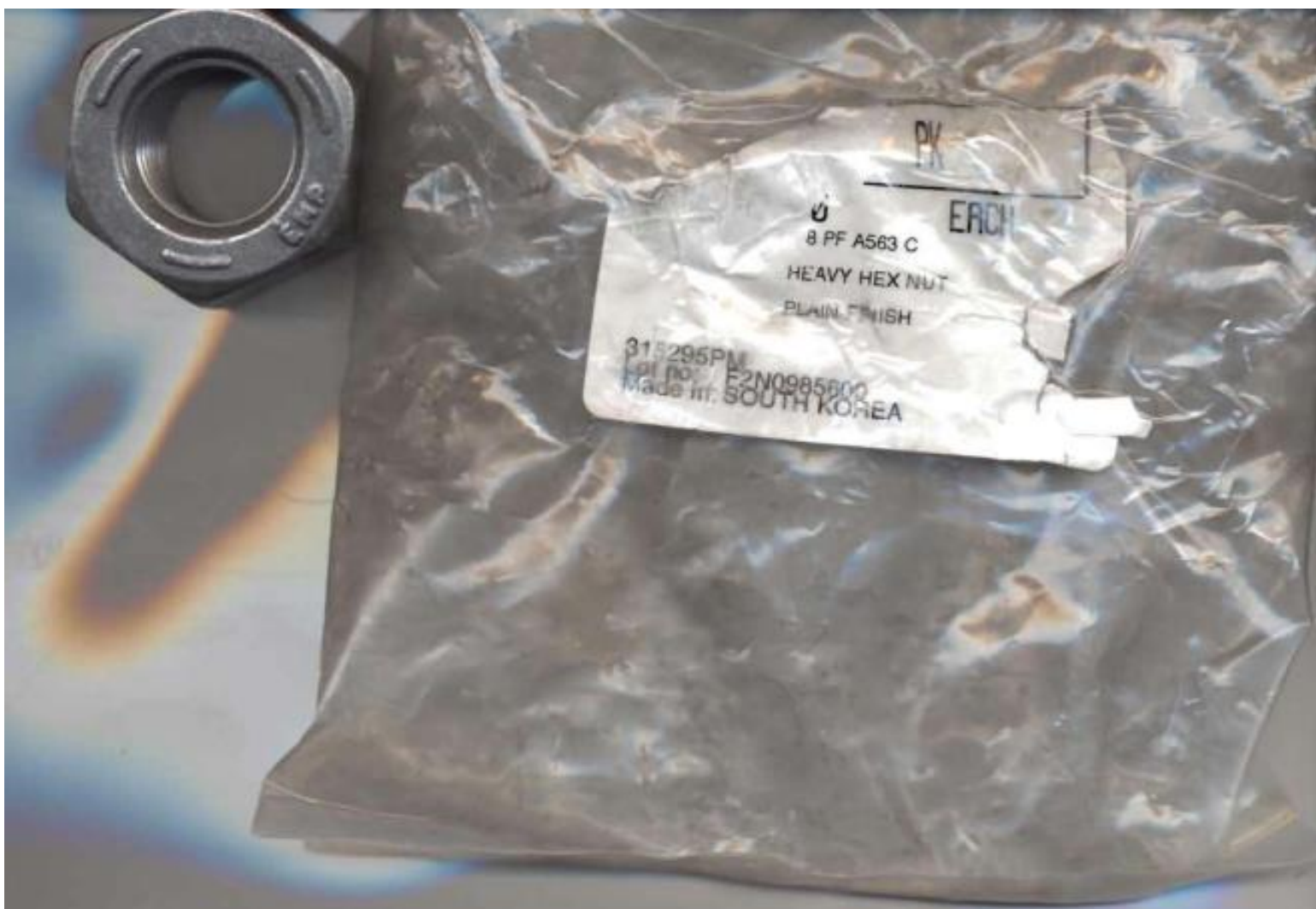
Figure B-19. Heavy Hex Nut for Test Nos. MWTC-1 through MWTC-3
