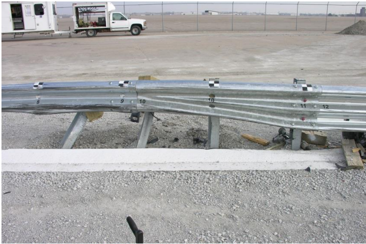
Figure 89. Impact Region Damage, Test No. MWTC-2
