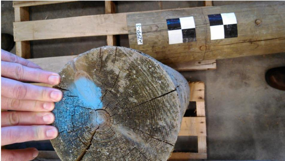
Figure AZPP-3: Ring Shake and some Slope of Grain Concern
