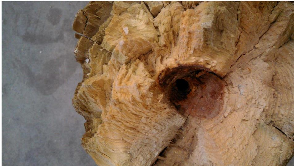
Figure AZPP-9: Wound with large amount of bark present also clear indications of a decayed core.
