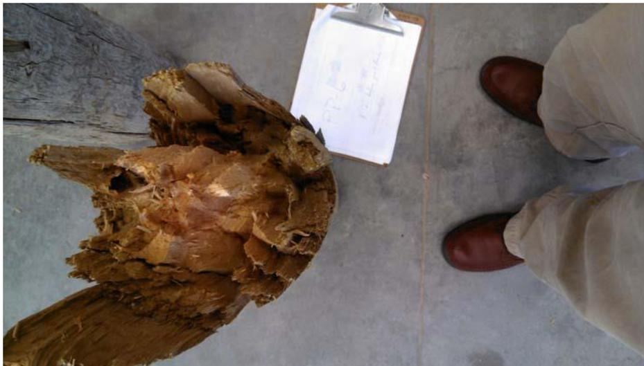
Figure AZPP-6: Substantial Slope of grain present in the posts.
