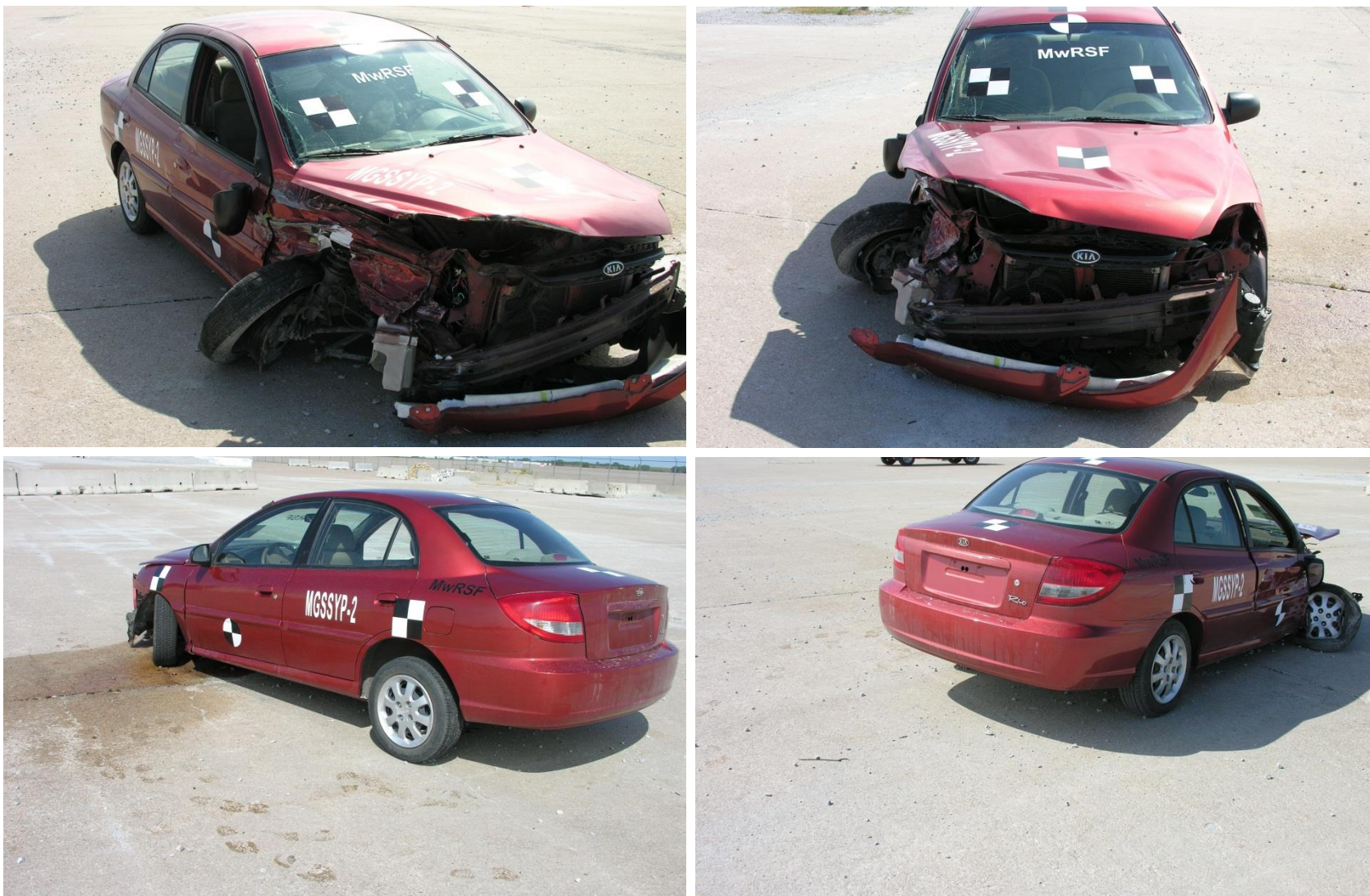
Figure 61. Vehicle Damage, Test No. MGSSYP-2
