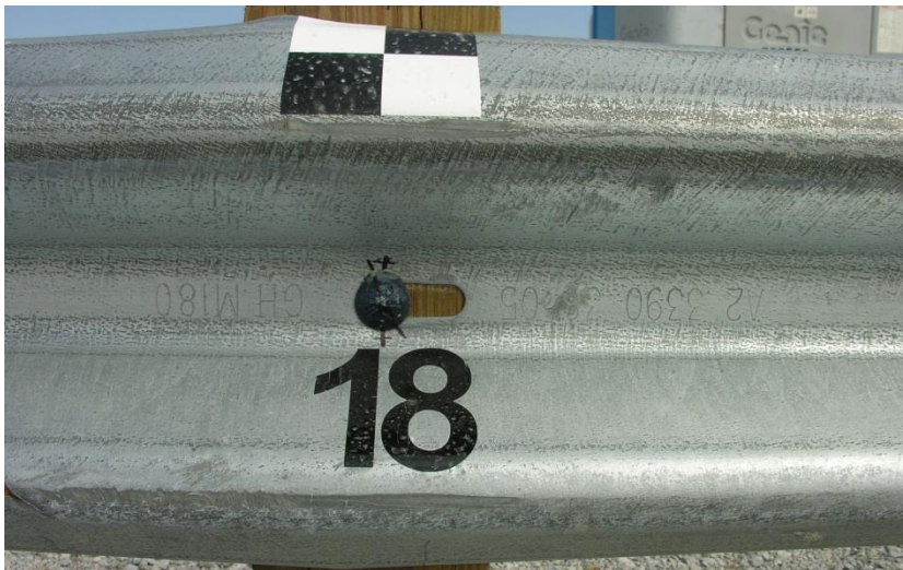
Figure 56. Rail Damage Between Post Nos. 16 and 18, Test No. MGSSYP-2
