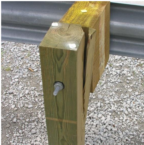
Figure 39. Post Nos. 6 and 10 Damage, Test No. MGSSYP-1
