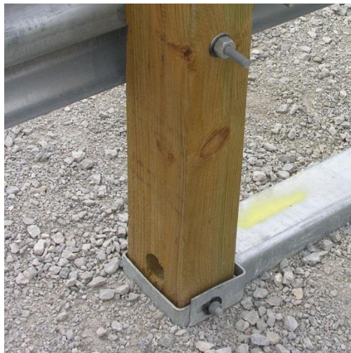
Figure 46. Downstream Anchor Damage, Test No. MGSSYP-1
