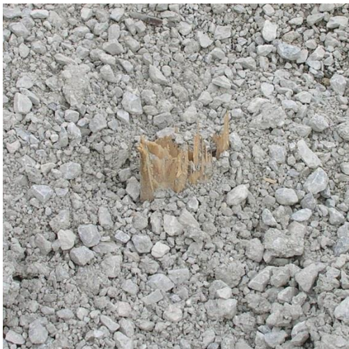
Figure 42. Post Nos. 15 and 16 Damage, Test No. MGSSYP-1
