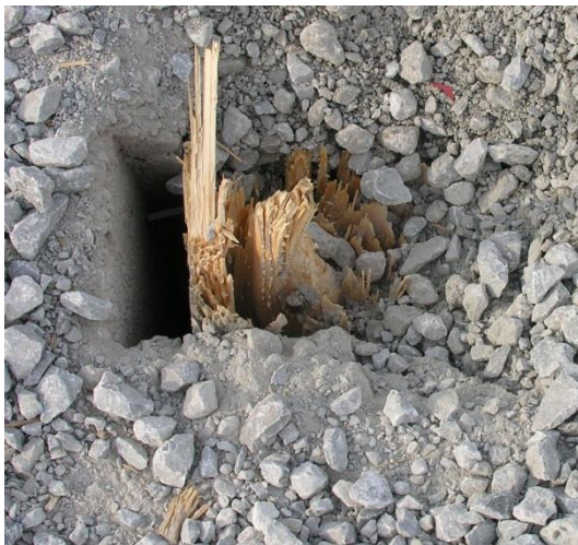
Figure 58. Post Nos. 15 and 16 Damage, Test No. MGSSYP-2
