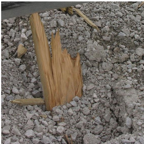
Figure 43. Post Nos. 17 and 18 Damage, Test No. MGSSYP-1
