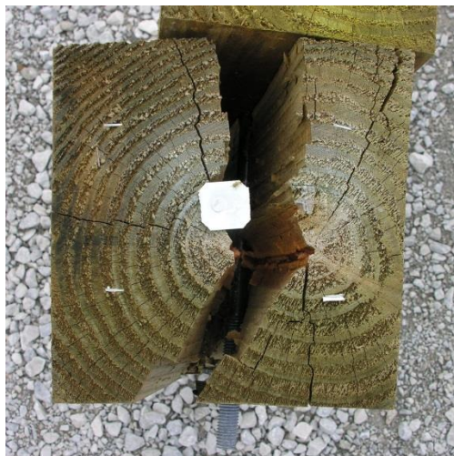
Figure 40. Post Nos. 11 and 12 Damage, Test No. MGSSYP-1.
