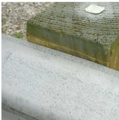
Figure 45. Upstream Anchor Damage, Test No. MGSSYP-1
