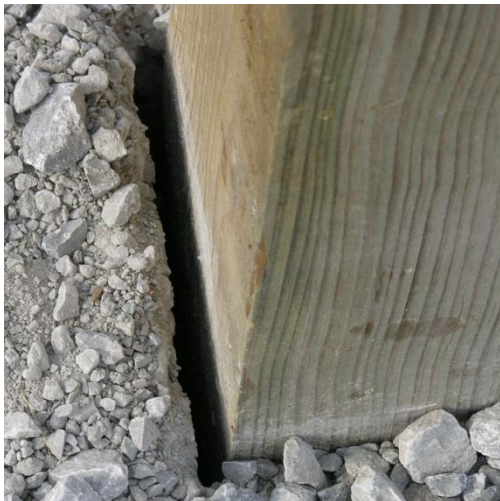
Figure 57. Post Nos. 13 and 14 Damage, Test No. MGSSYP-2
