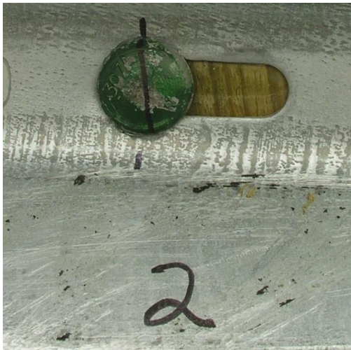
Figure 60. Upstream Anchor Damage, Test No. MGSSYP-2
