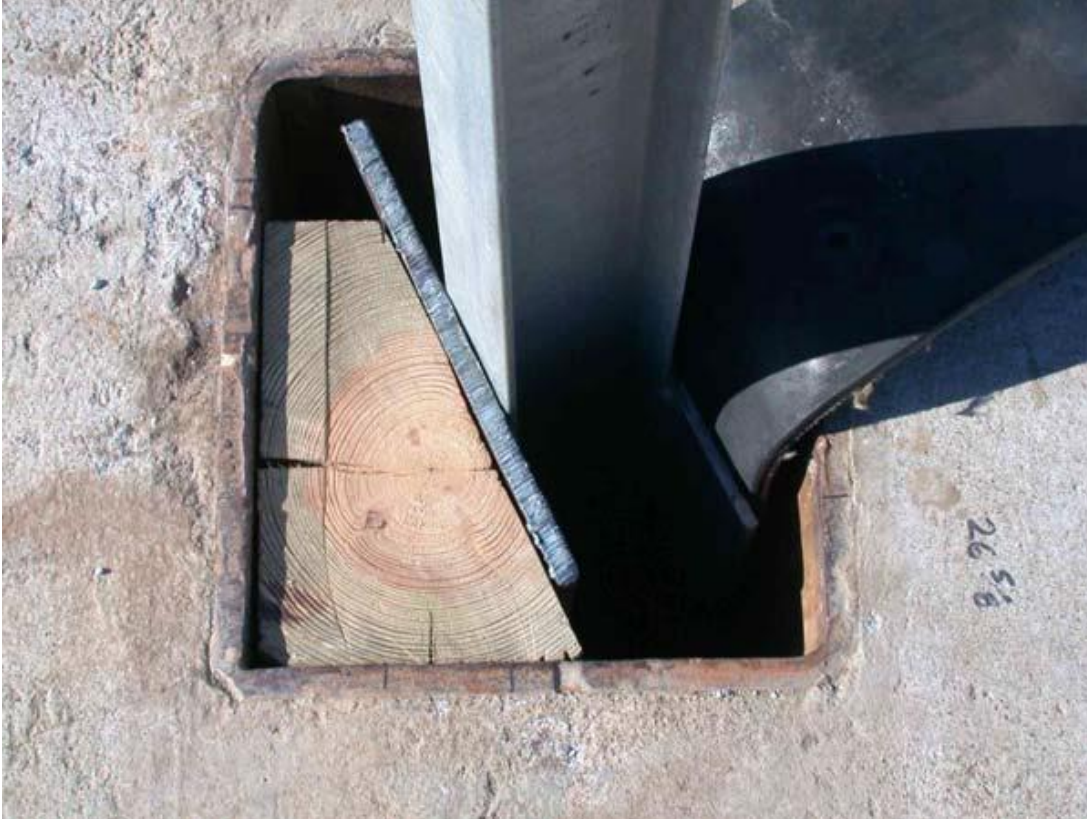
Figure A-5. Typical Post and Wood Block Setup
