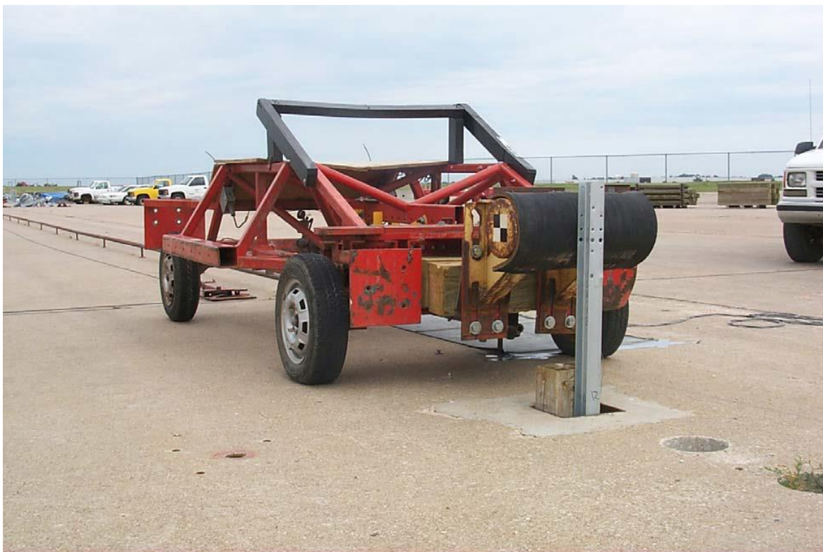
Figure A-2. Bogie and Test Setup – CPB Series
