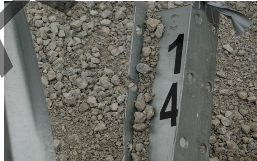
d. Post No. 14, Post Bolt Hole Tear
