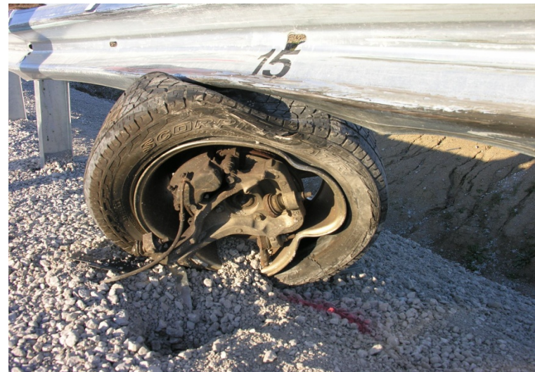
d. Wheel Lodged Under Rail
