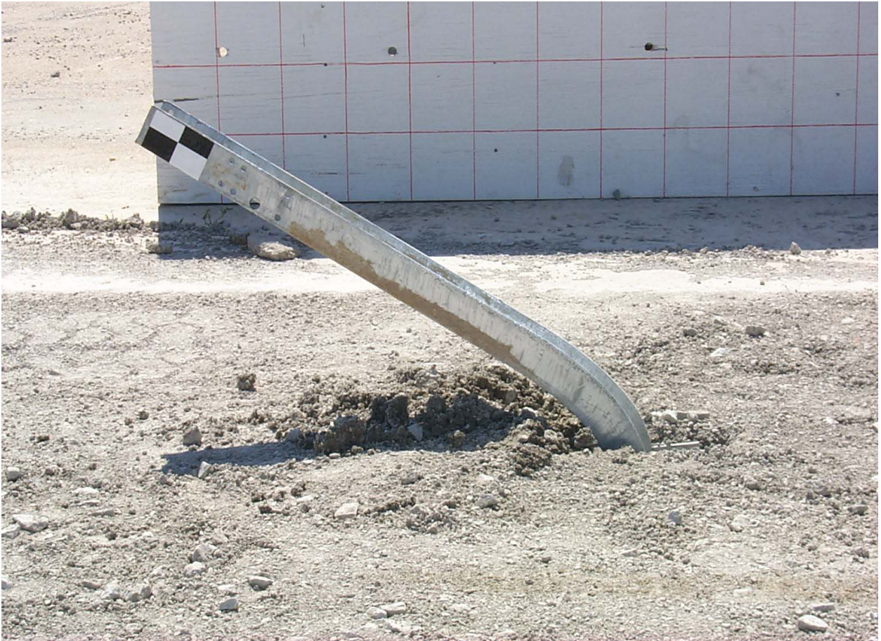
Figure 15. Plastically deformed post for test CPB-5
