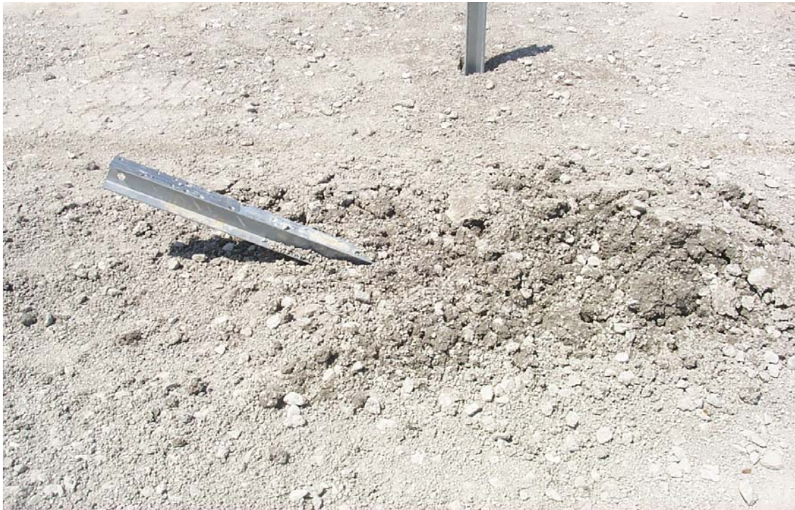
Figure 14. Post impact scenario for test CBP-2
