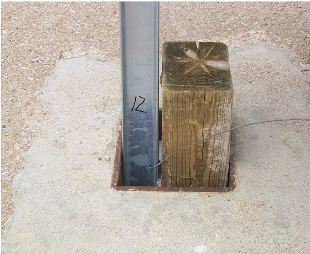
Figure 6. Post and woodblock setup for tests CPB-12 through CPB-14
