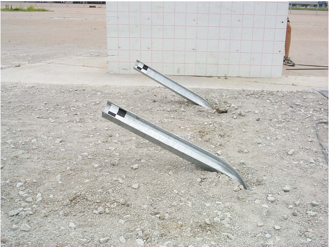
Figure 16. CPB-8 and CPB-9 deformed post geometries
