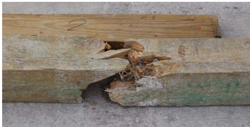
i. Close up of Post Fracture
