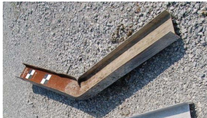
i. Post After Impact – Removed, Showing Deformation
