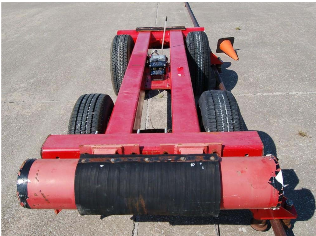
Figure 7. Photo. Rigid Frame Bogie on Pipe Guide Track System.
