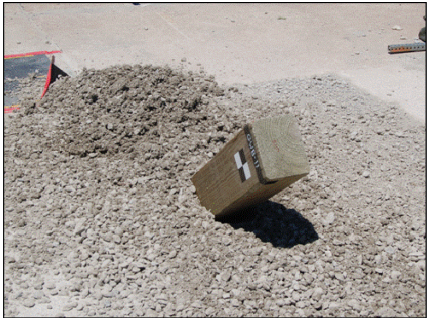
g. Post After Impact – Rear Quarter View
