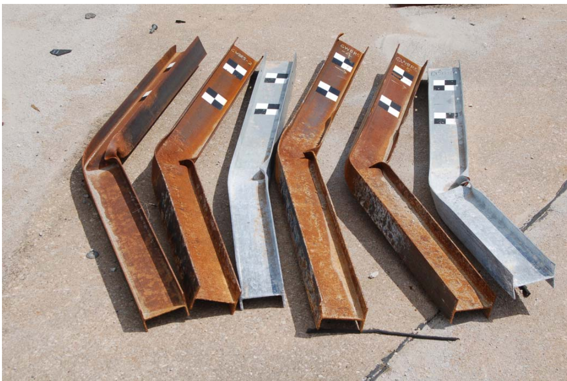
Figure 74. Photo. Post Damage – Round 4 (Ascending Left to Right).
