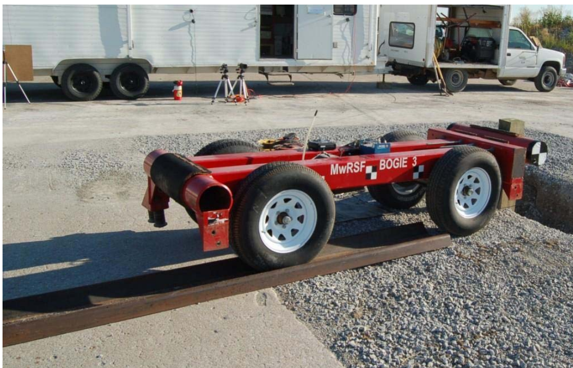
Figure 8. Photo. Rigid Frame Bogie on Corrugated Beam.
