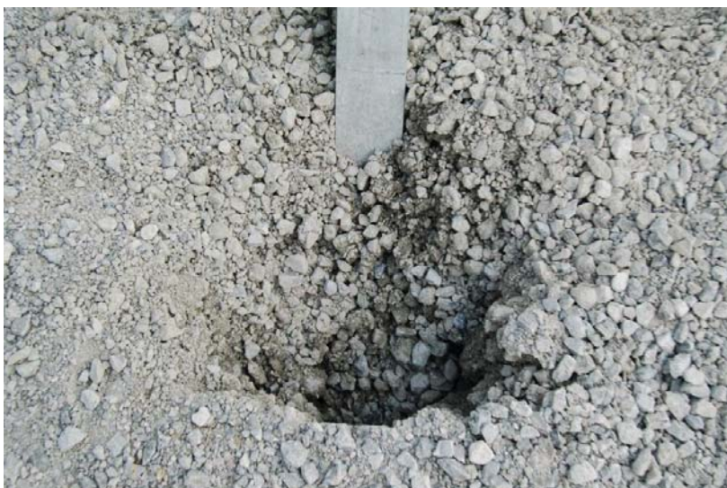
h. Soil Displacement of Post After Impact
