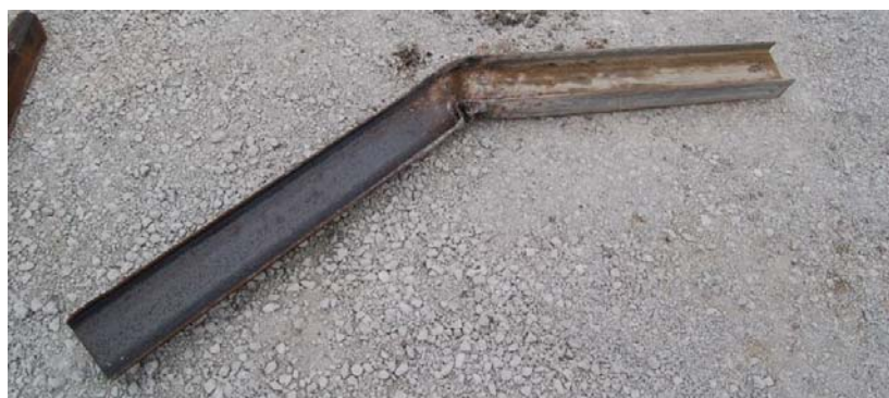
i. Post After Impact – Removed, Showing Deformation
