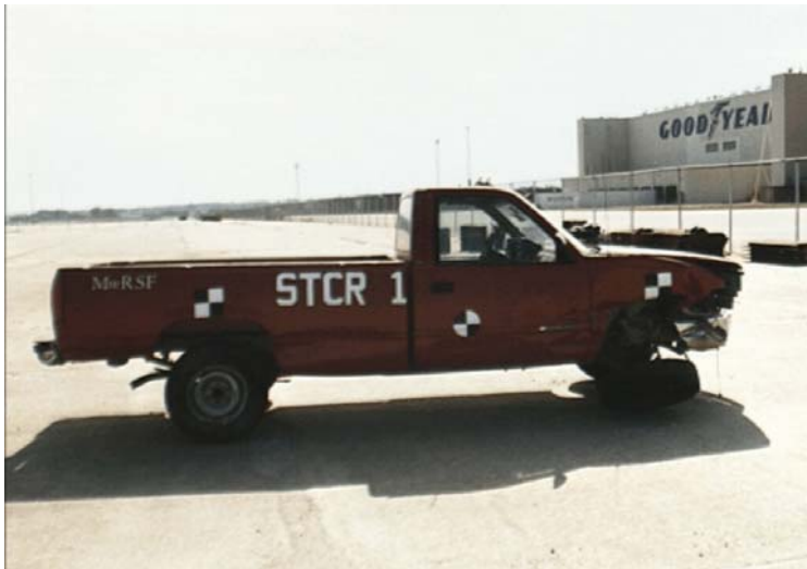
Figure 65. Vehicle Damage, Test STCR-1
