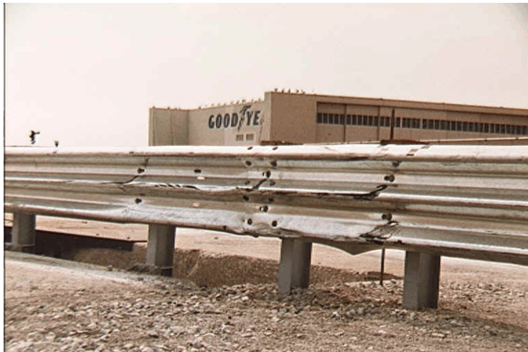
Figure 76. Barrier Damage, Test STCR-2
