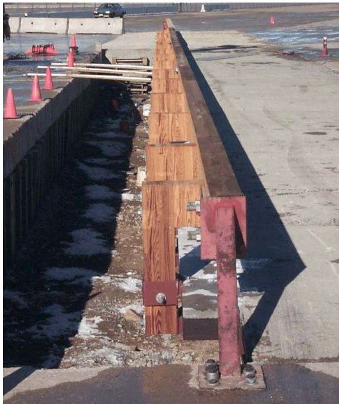
Figure 85. Wood Bridge Railing System
