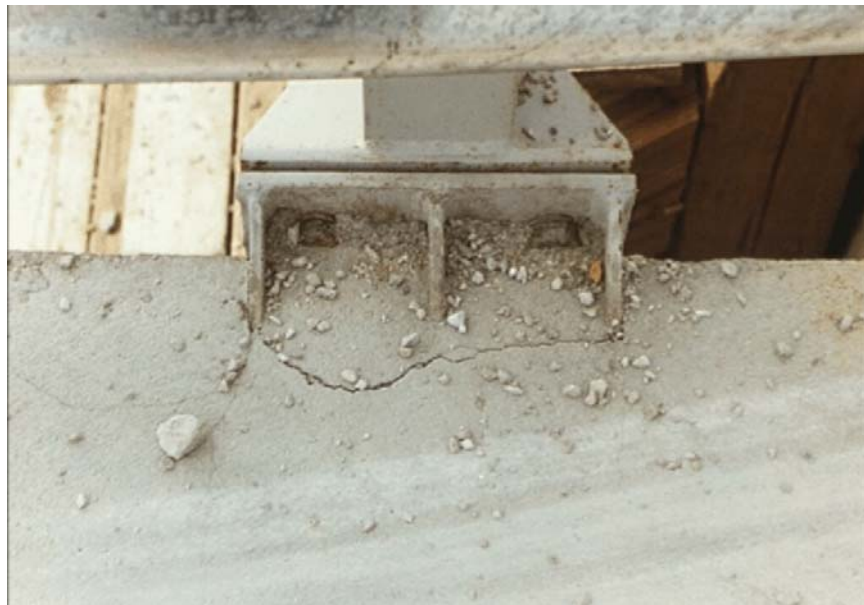
Figure 79. Bridge Post No. 1 Damage, Test STCR-2
