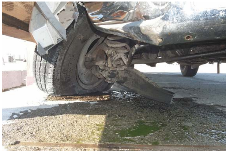
Figure 129. Vehicle Damage, Test WRBP-2
