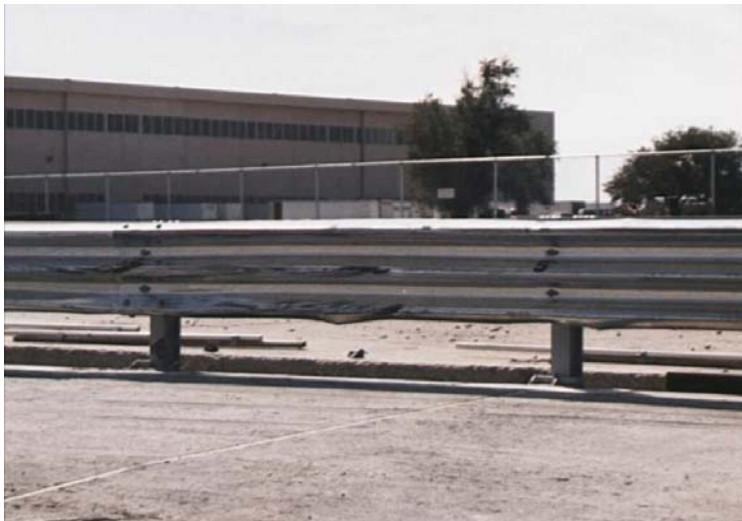
Figure 60. Barrier Damage, Test STCR-1
