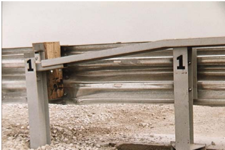
Figure 77. Barrier Damage, Test STCR-2
