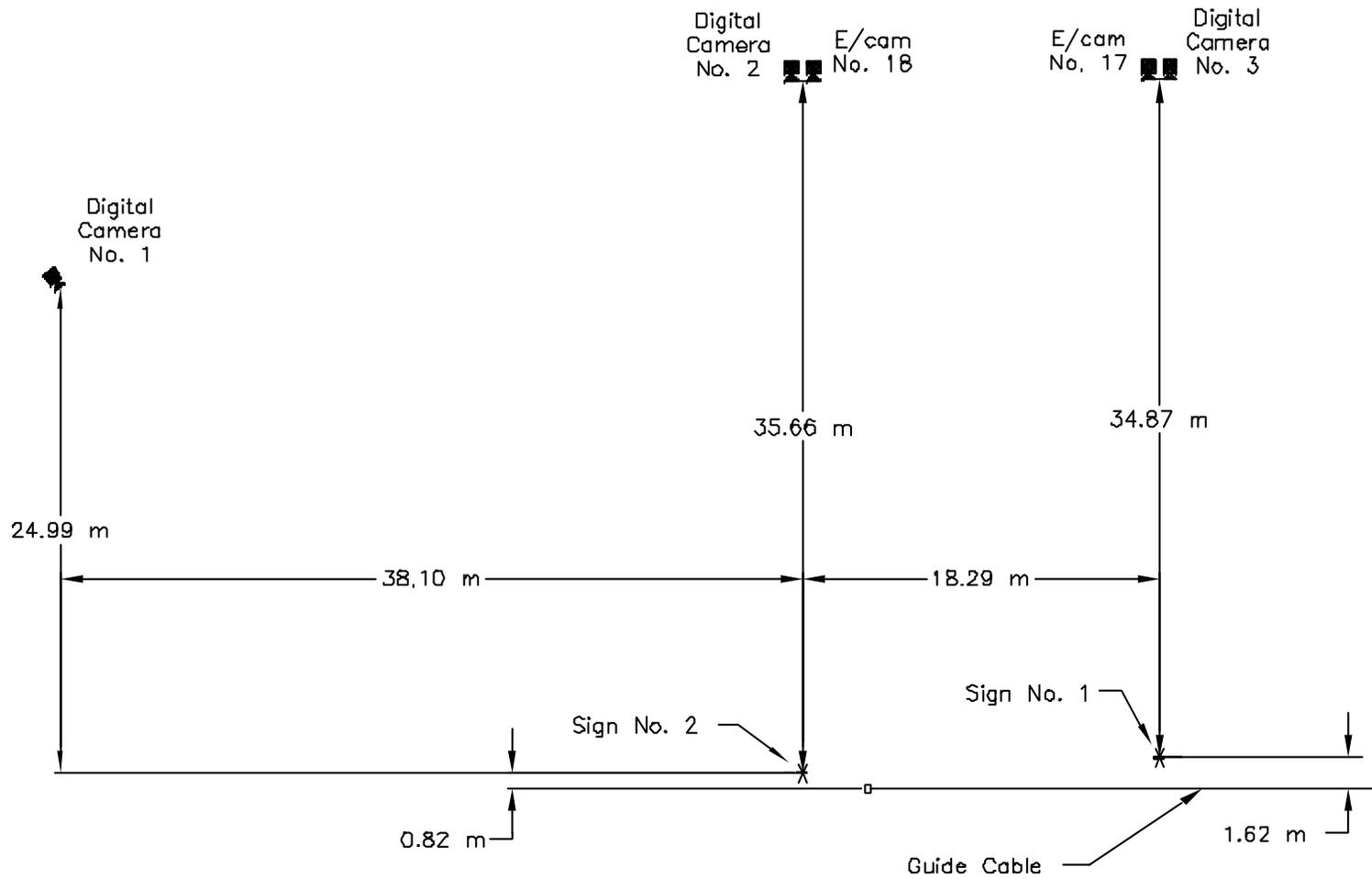
Figure 21. Location of High-Speed Cameras, Test MNS-3
