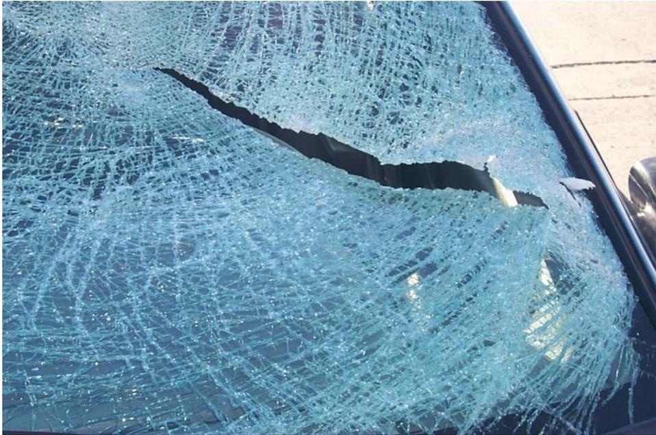
Figure 34. Windshield Damage, Test MNS-1
