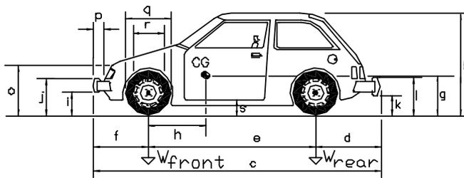
Vehicle Geometry - mm
