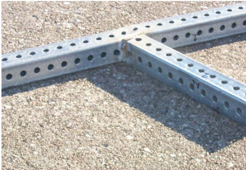
Figure 31. System No. 1 Damage, Test MNS-1
