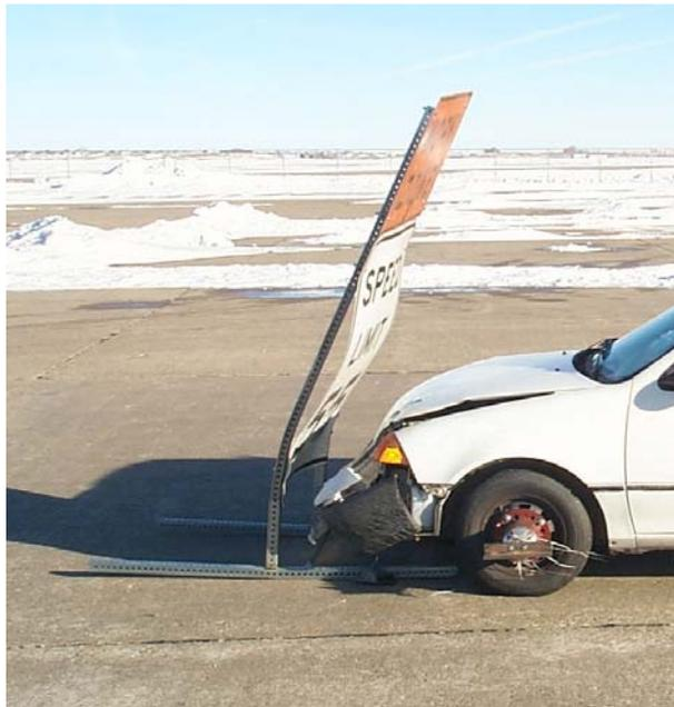
Figure 43. System No. 3 Damage, Test MNS-2
