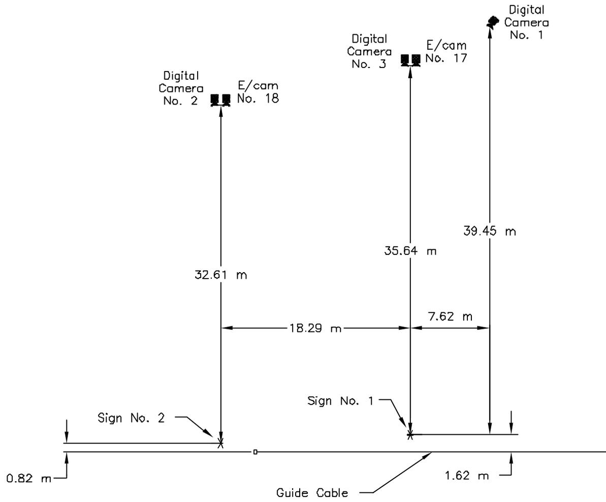
Figure 20. Location of High-Speed Cameras, Tests MNS-1 and MNS-2
