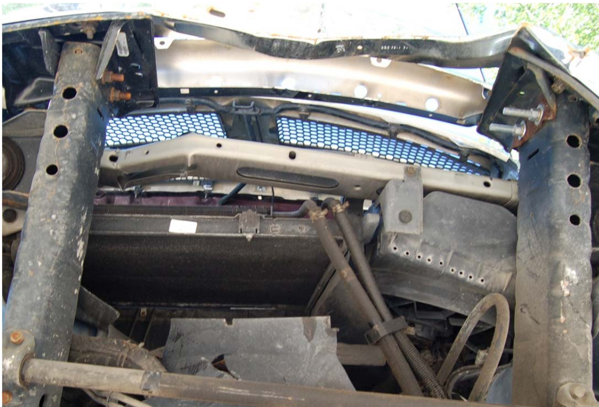
Figure 86. Undercarriage Damage, Test No. 4CMB-5
