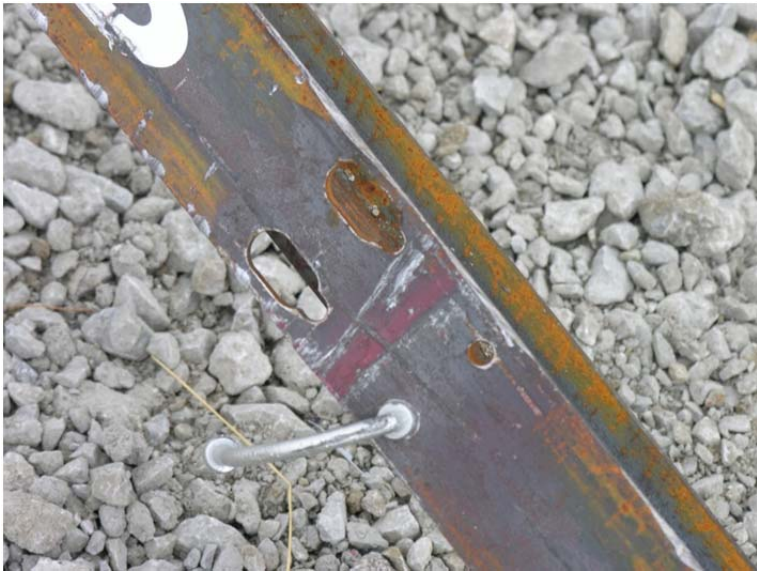
Figure 44. Post and Keyway Bolt Damage, Test No. 4CMB-4
