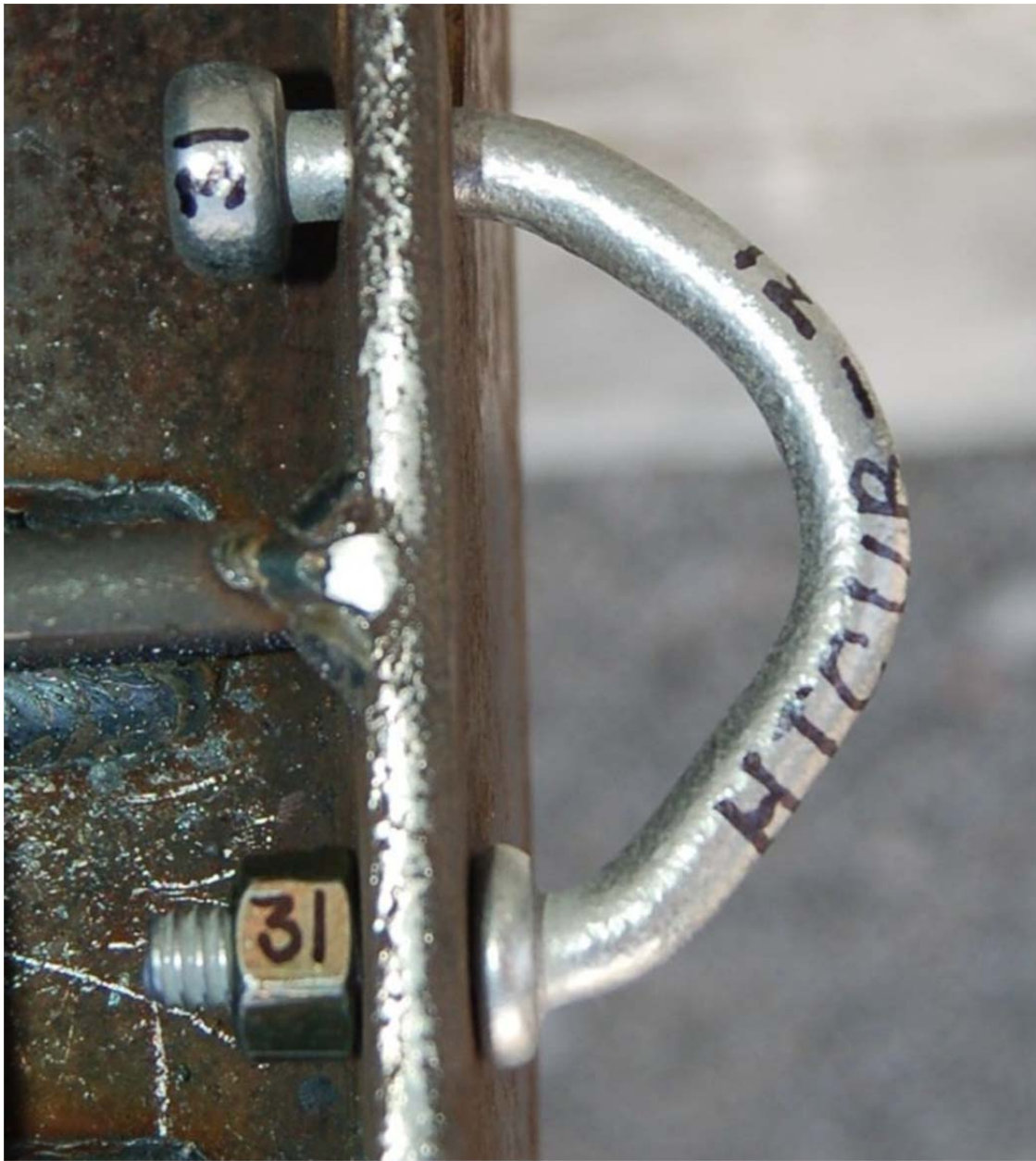
Figure 2. Updated Cable Attachment: Angled Keyway Bolt
