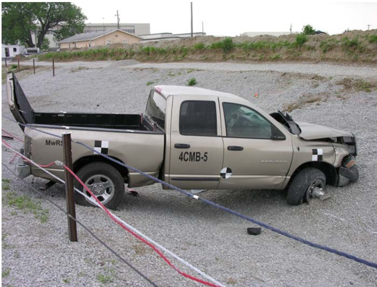
Figure 83. Vehicle Damage, Test No. 4CMB-5
