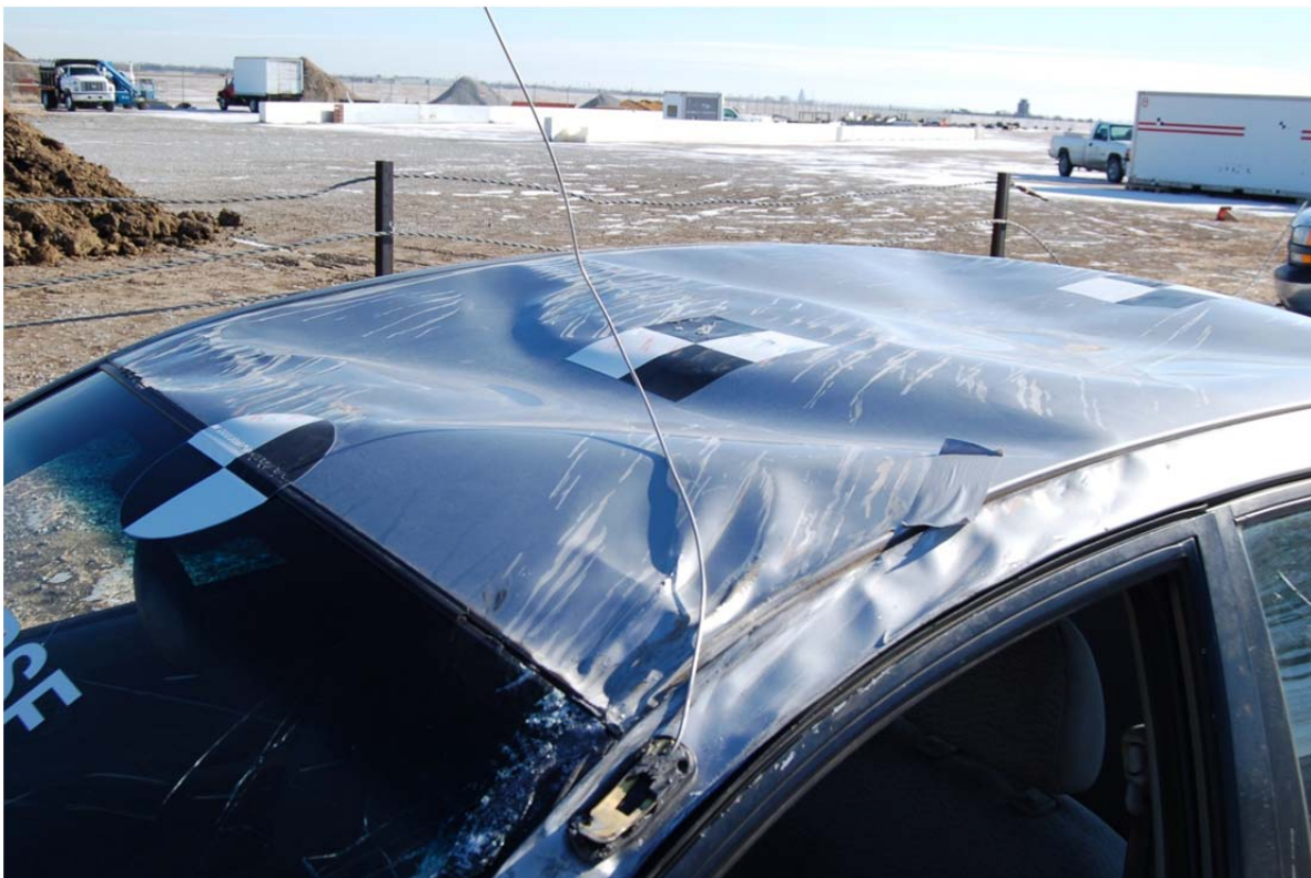
Figure 48. Occupant Compartment Damage, Test No. 4CMB-4
