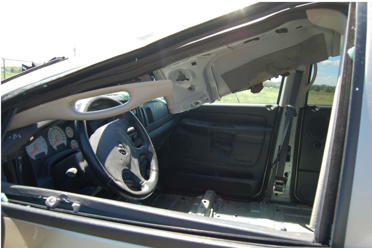
Figure 85. Occupant Compartment Damage, Test No. 4CMB-5
