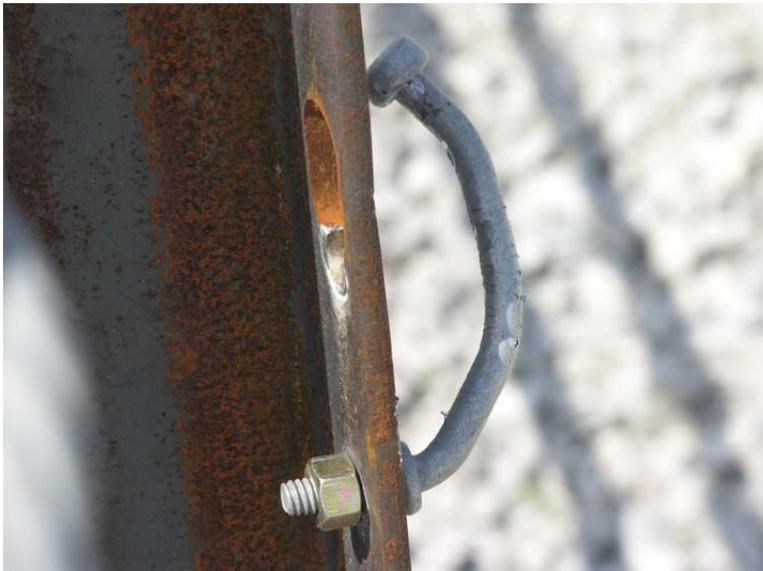
Figure 82. Post and Splice Damage, Test No. 4CMB-5
