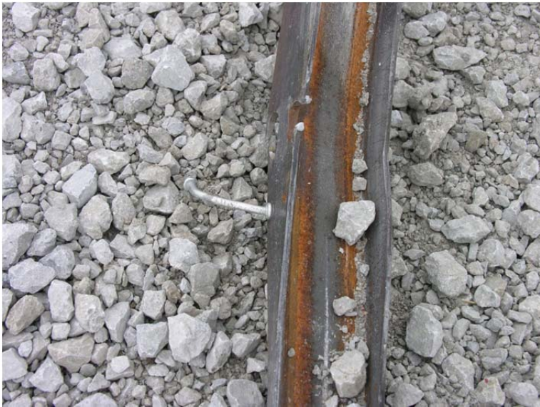
Figure 43. Post and Keyway Bolt Damage, Test No. 4CMB-4
