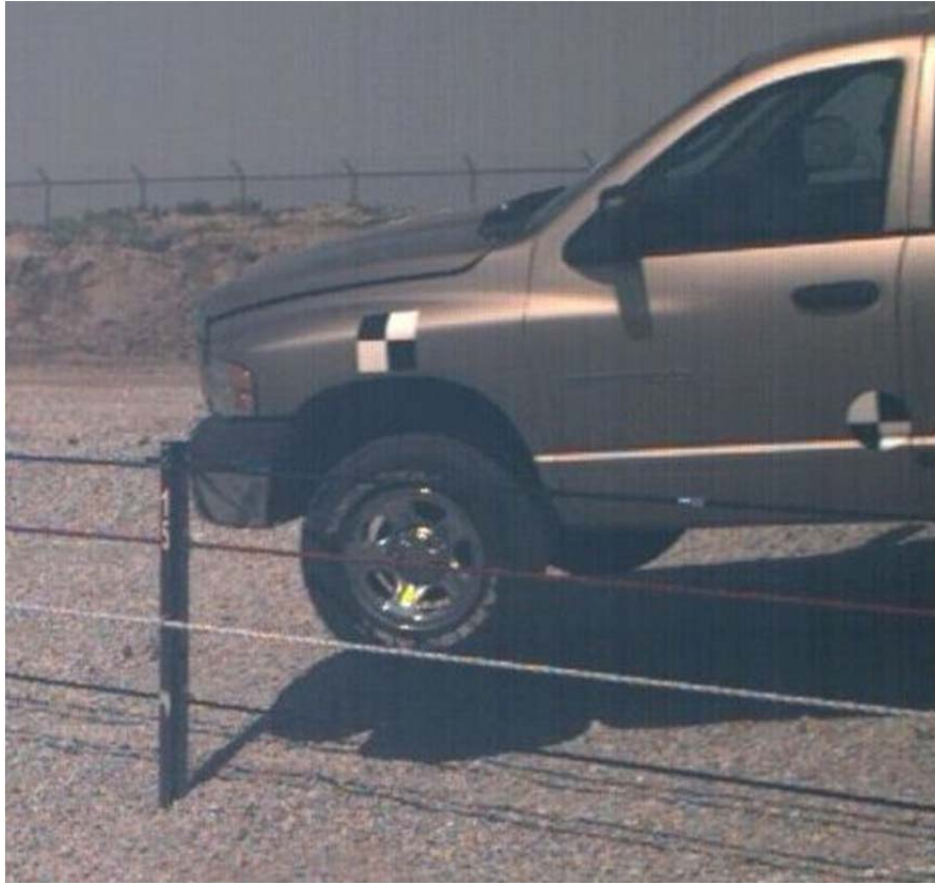
Figure 87. Bumper-to-Cable Relation at Impact, Test No. 4CMB-5
