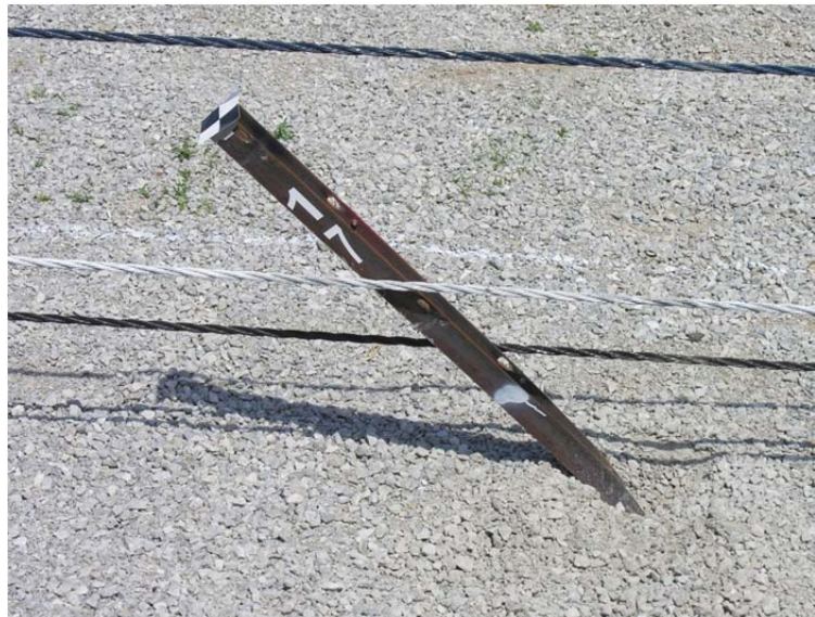
Figure 81. Post Damage, Test No. 4CMB-5
