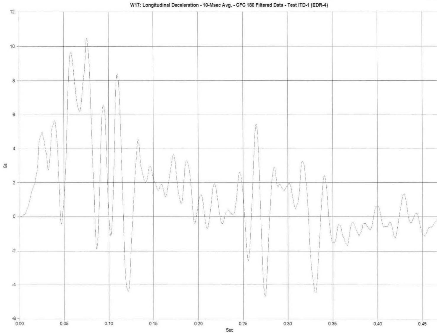
Figure G-1. Graph of Longitudinal Deceleration - Filtered Data, Test ITD-1
