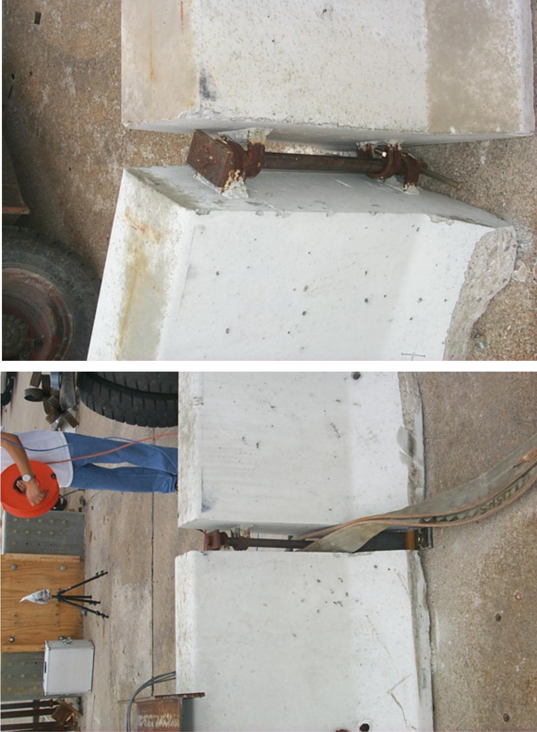
Figure 16. Configuration for Bogie Testing of Strap Tie-Down Concept, Test ITDB-2
