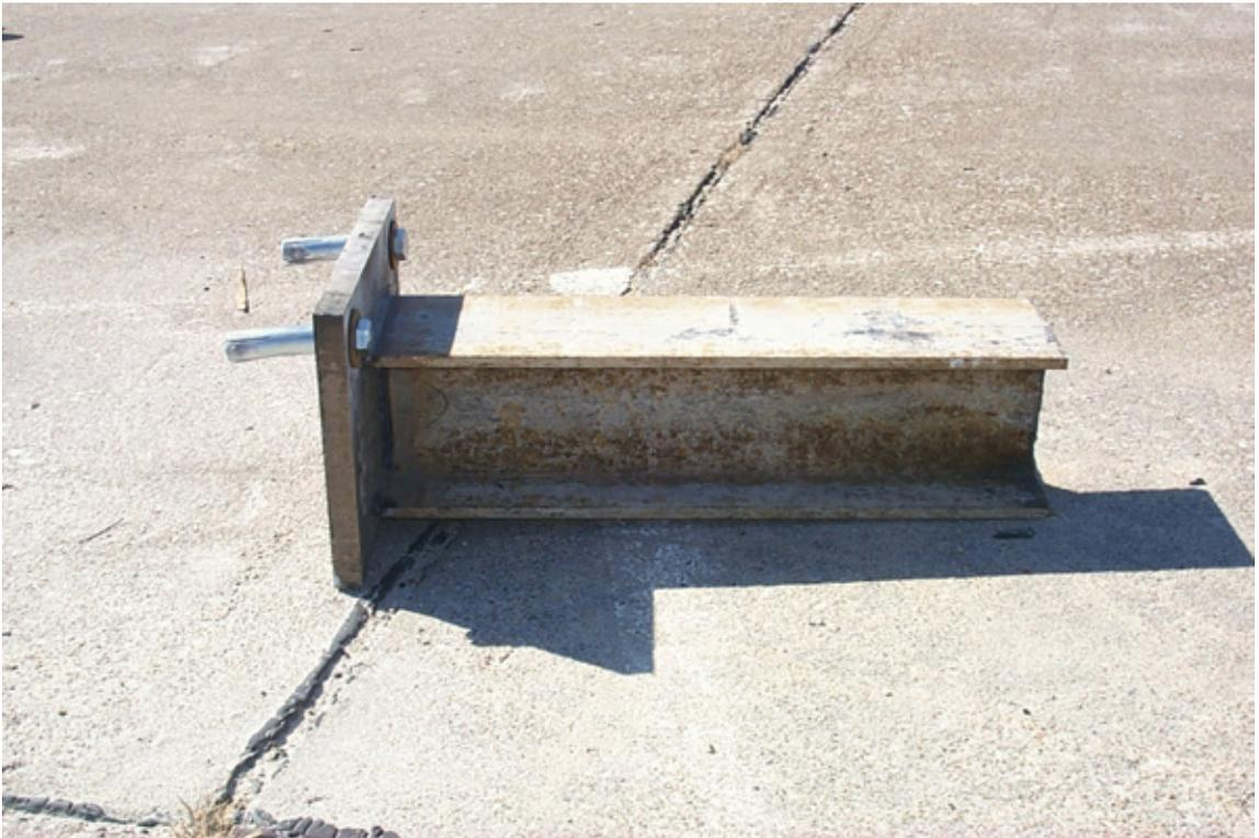
**Figure 5. Drop-In Anchor Component Testing**
