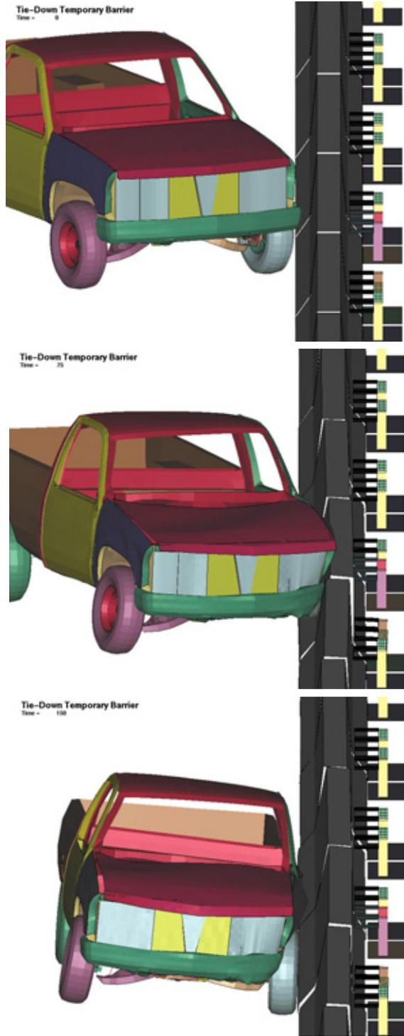
Figure 10a. With Tie-Down Anchors
