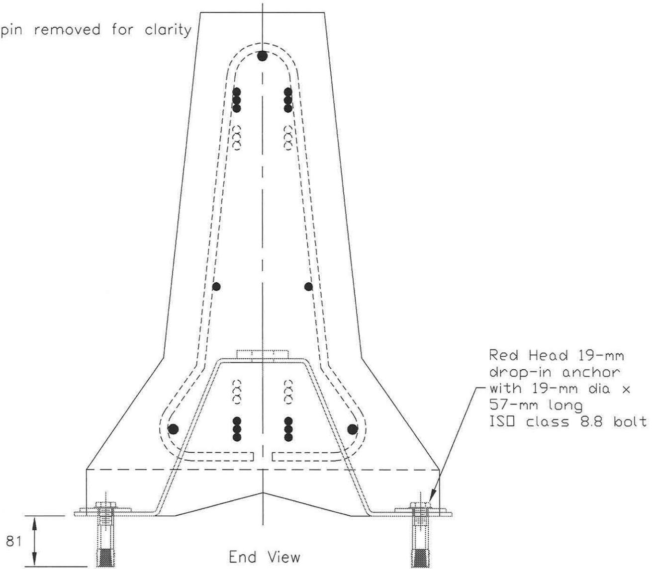
Figure 25. Tie-Down Temporary Barrier System Details
