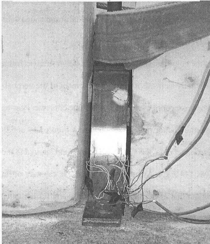
Figure 17. Strain Gauge Locations, Test ITDB-2
