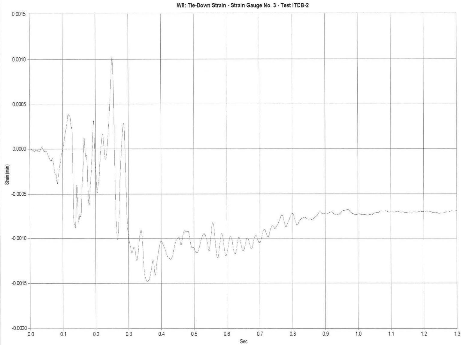
Figure D-3. Graph of Outer Flange Gauge No. 3 Top Peak Strain, Test ITDB-2
