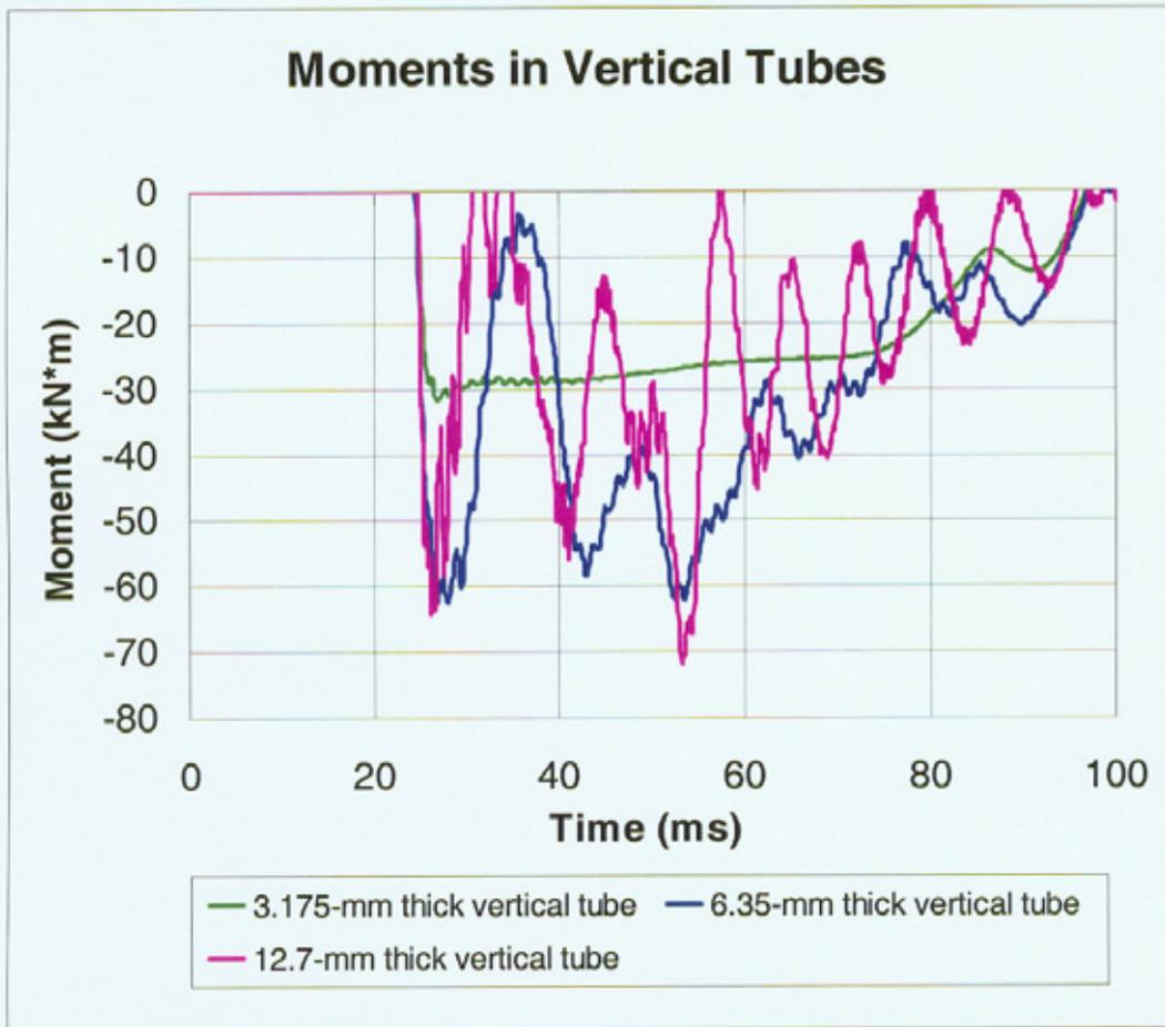
Figure 4. Comparison of Vertical Tube Moments
