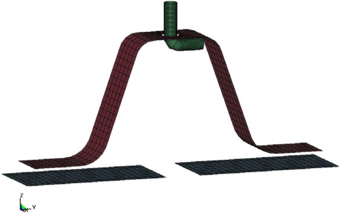
Figure 11. Double Steel Strap Tie-Down Simulation Model
