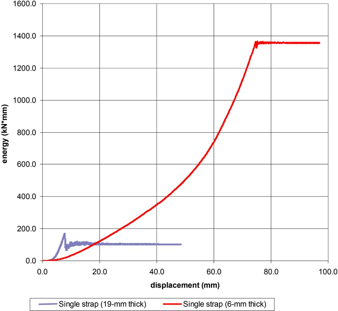
Figure 10. Single Steel Strap Tie-Down Simulation Model Energies
