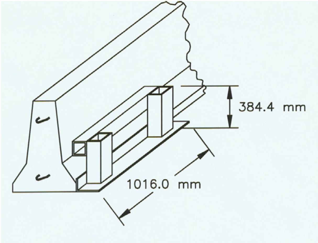
**Figure 2. Initial Design Concept**
