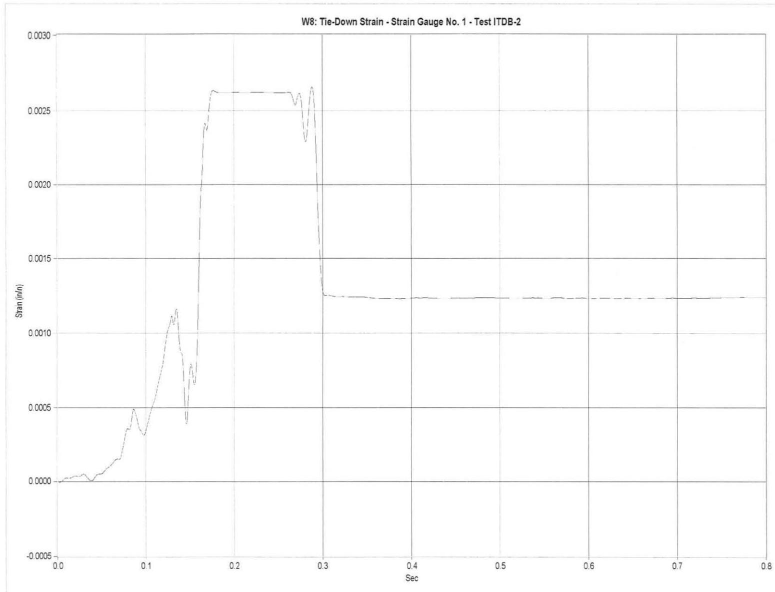
Figure D-1. Graph of Inner Flange Gauge No. 1 Top Peak Strain, Test ITDB-2
