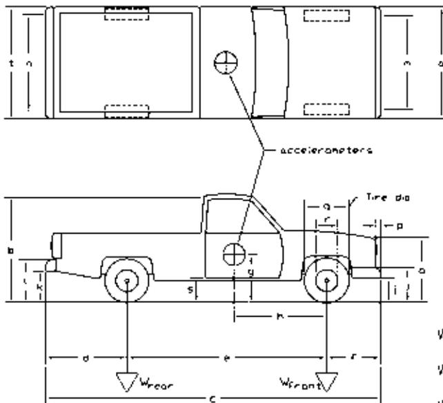
Vehicle Geometry - mm
