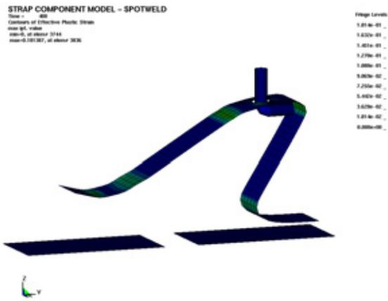
Figure 12. Double Steel Strap Tie-Down Simulation
