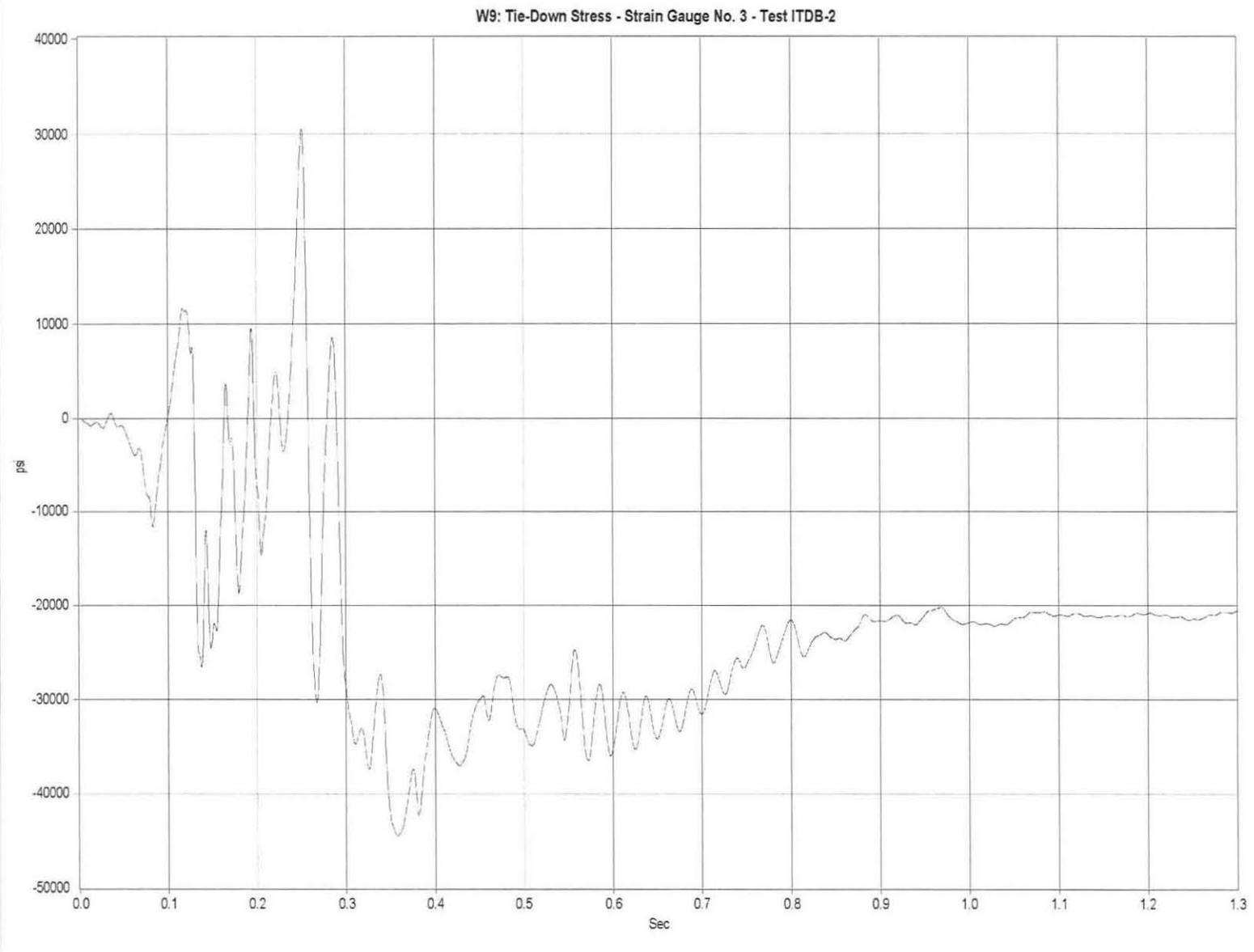
Figure D-4. Graph of Outer Flange Gauge No. 3 Top Peak Stress, Test ITDB-2
