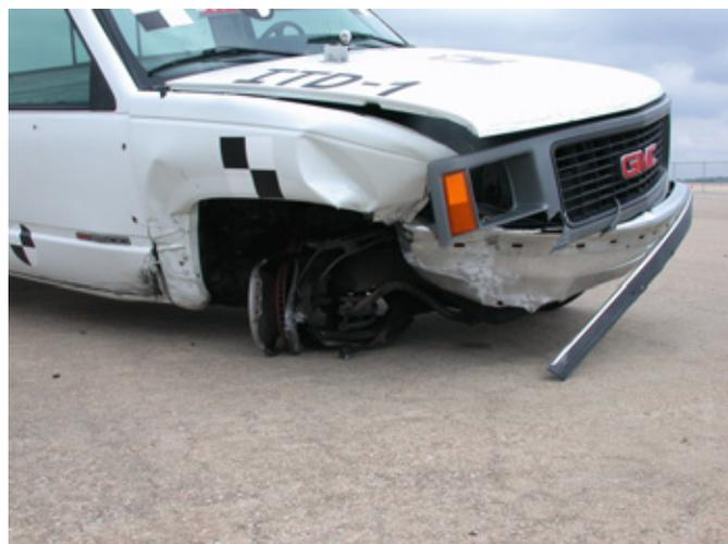
Figure 43. Vehicle Damage, Test ITD-1
