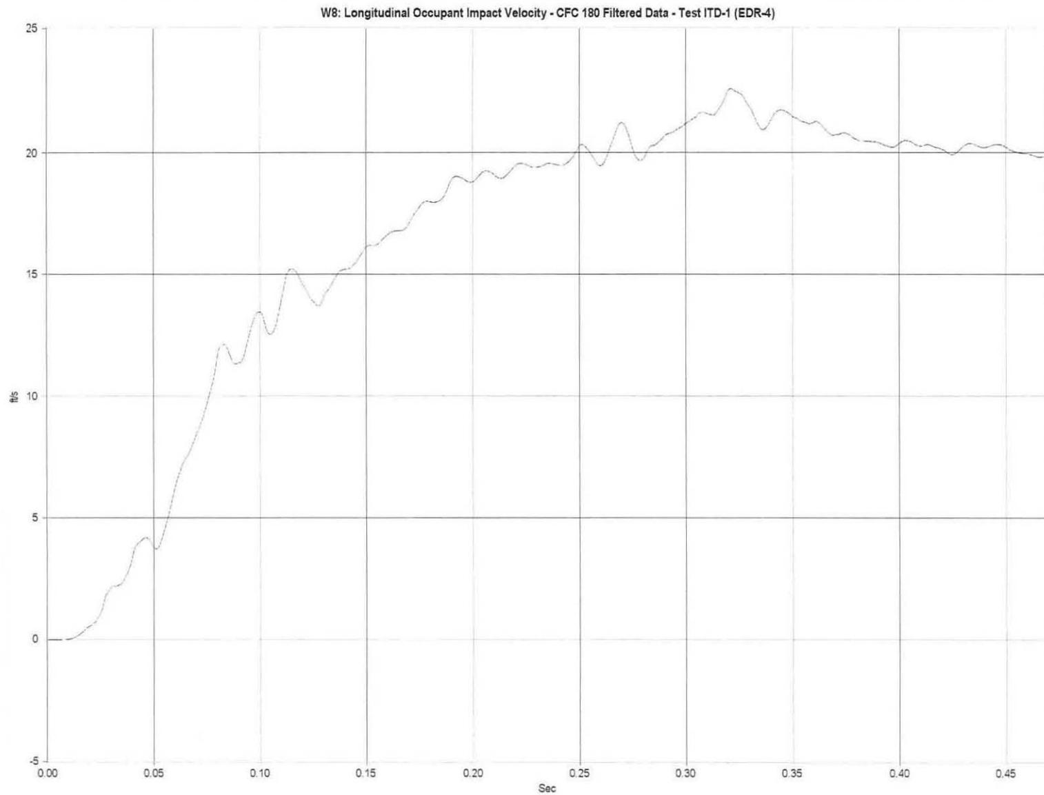
Figure G-2. Graph of Longitudinal Occupant Impact Velocity - Filtered Data, Test ITD-1
