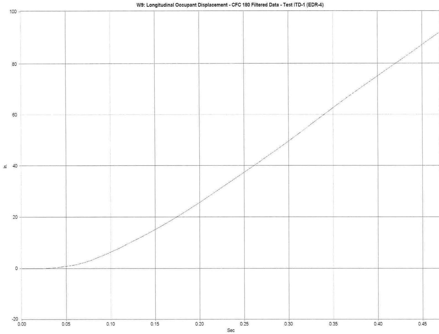
Figure G-3. Graph of Longitudinal Occupant Displacement - Filtered Data, Test ITD-1
