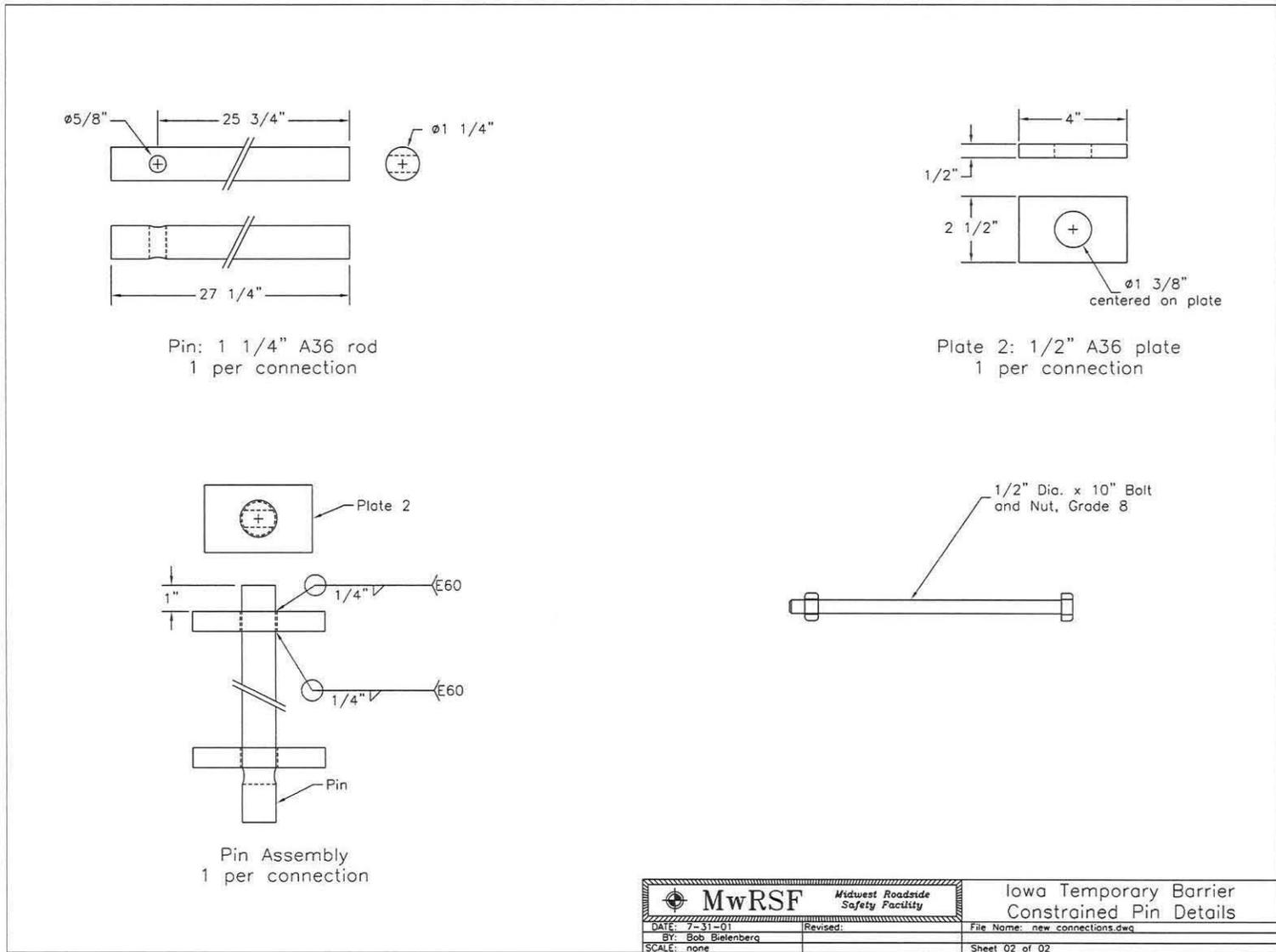
Figure 23. Iowa Temporary Barrier Details
