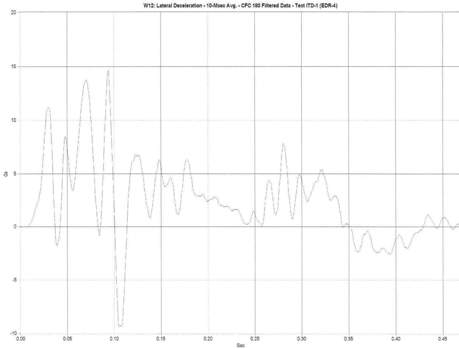
Figure G-4. Graph of Lateral Deceleration - Filtered Data, Test ITD-1
