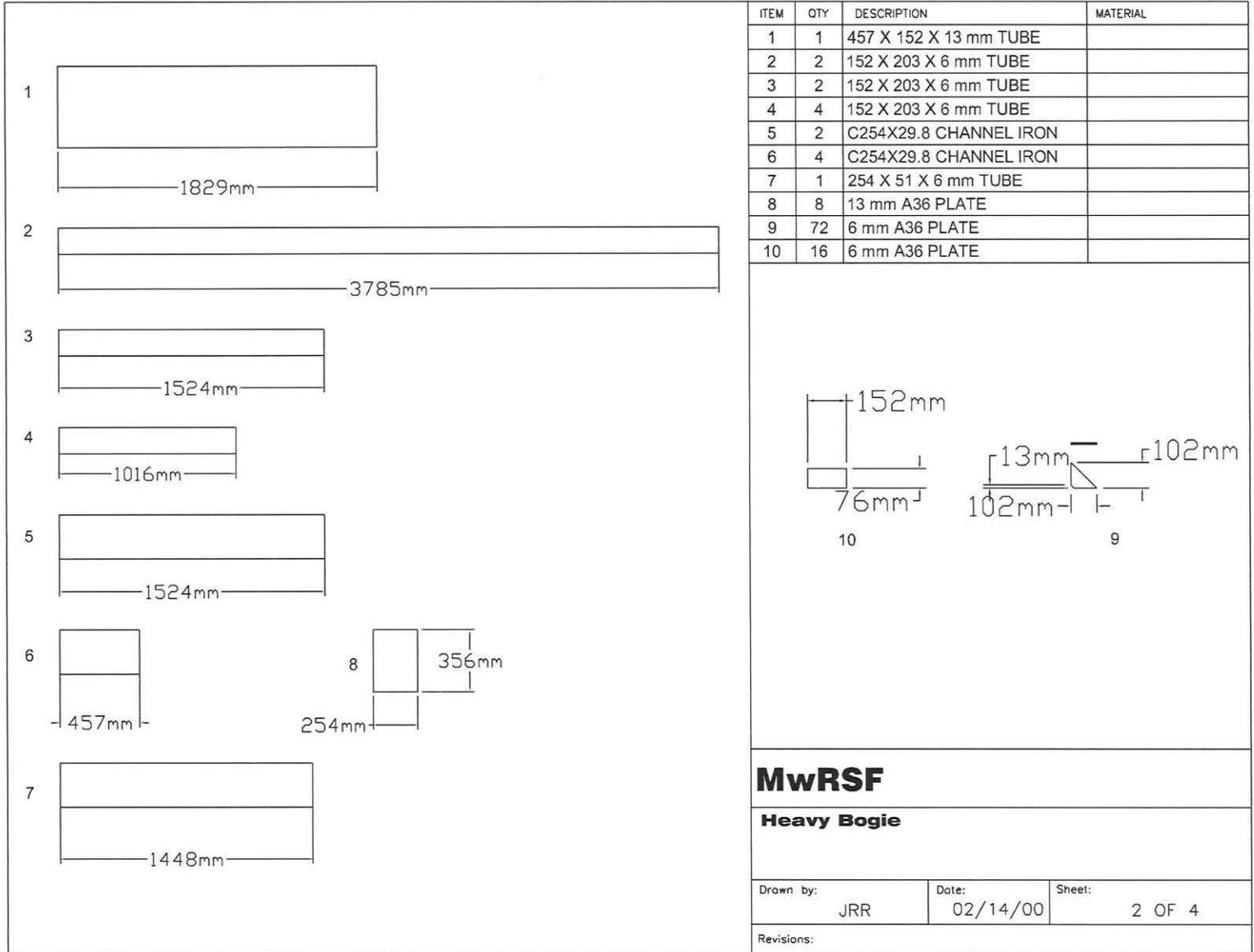
Figure B-5. Bogie Vehicle Details
