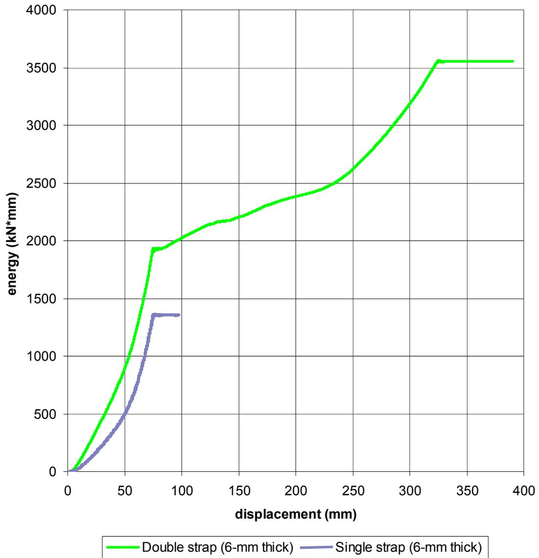
Figure 13. Comparison of Energy Absorption for the Single and Double Steel Strap Concepts
