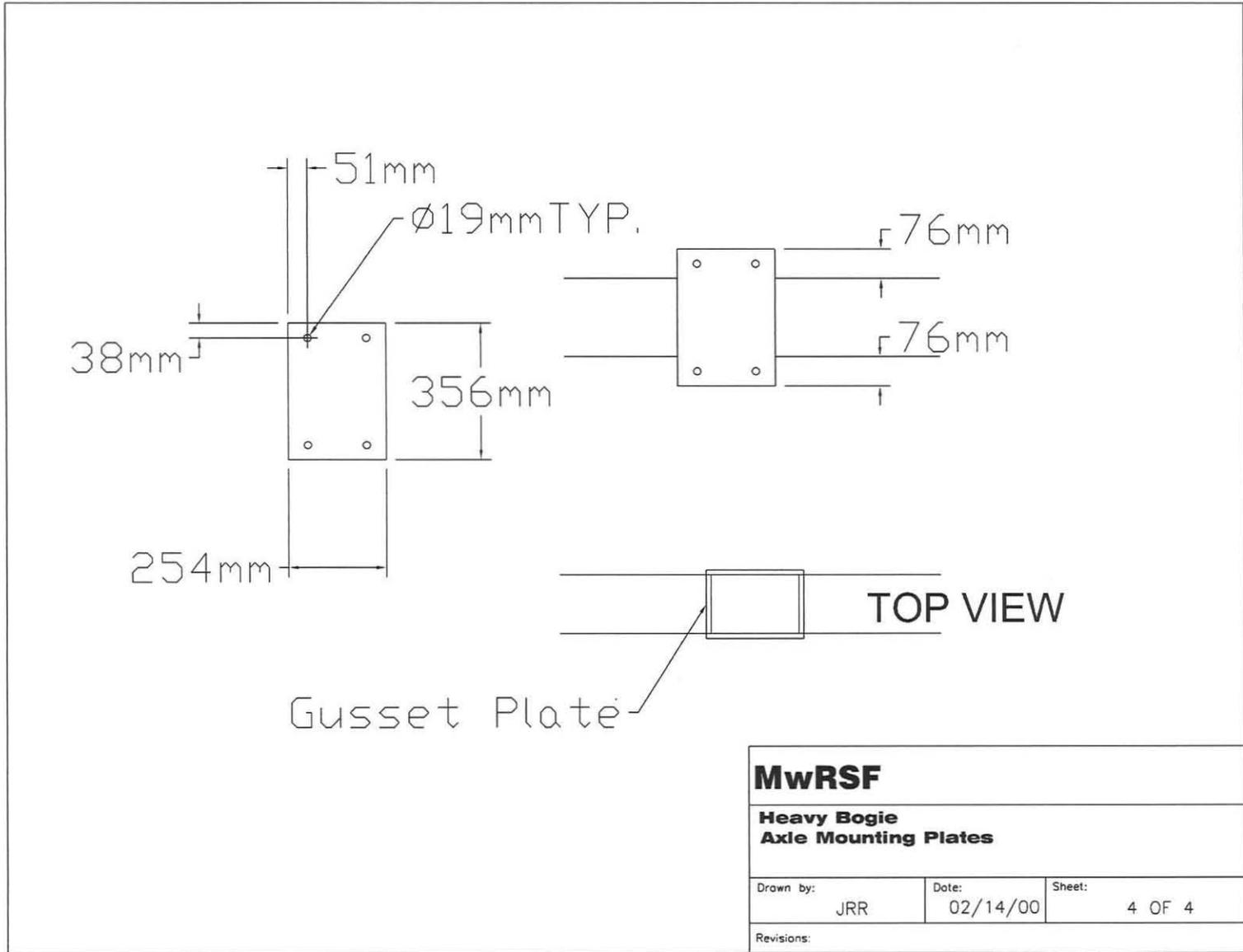
Figure B-4. Bogie Vehicle Details
