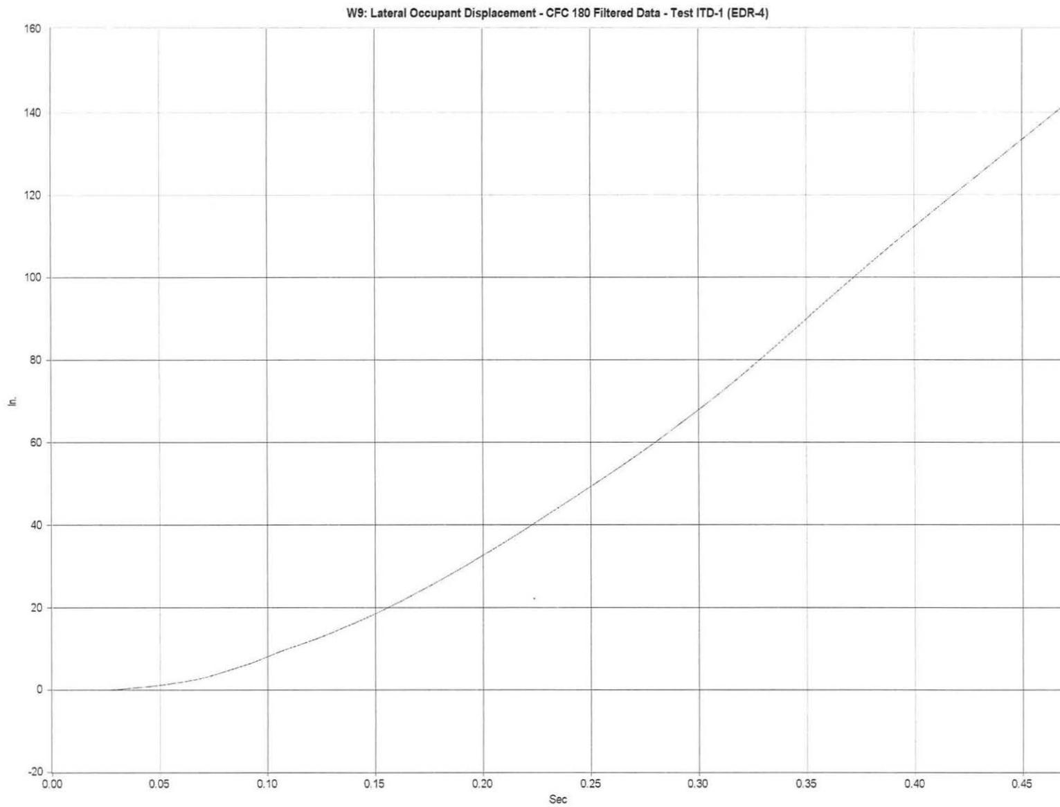
Figure G-6. Graph of Lateral Occupant Displacement - Filtered Data, Test ITD-1
