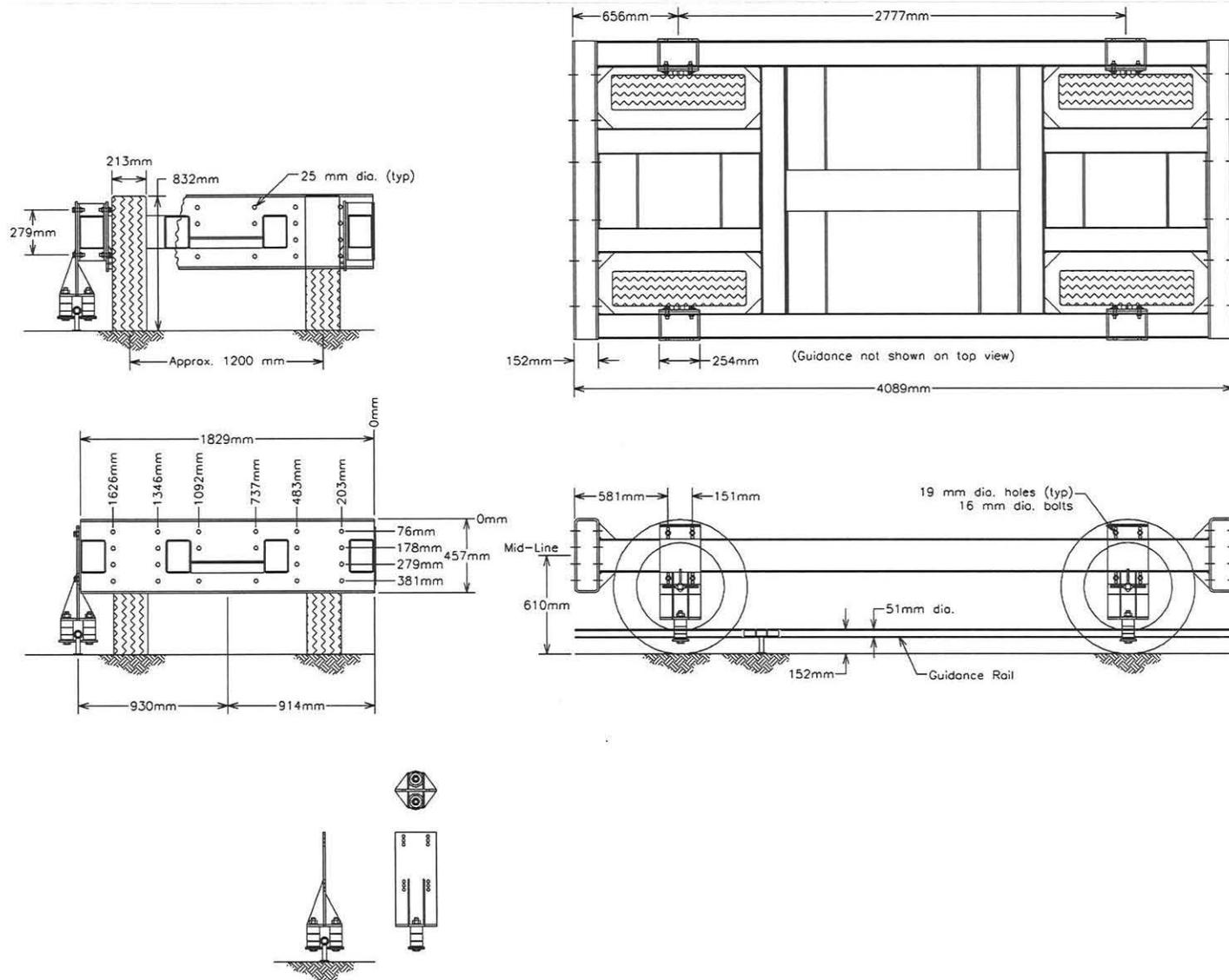
Figure B-1. Bogie Vehicle Details
