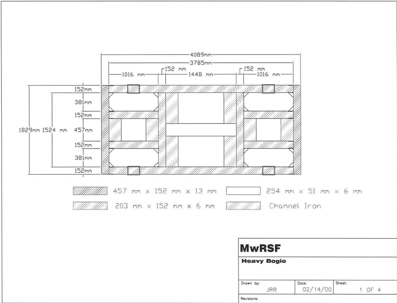
Figure B-3. Bogie Vehicle Details
