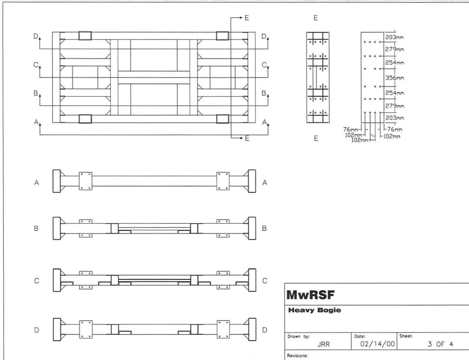
Figure B-2. Bogie Vehicle Details
