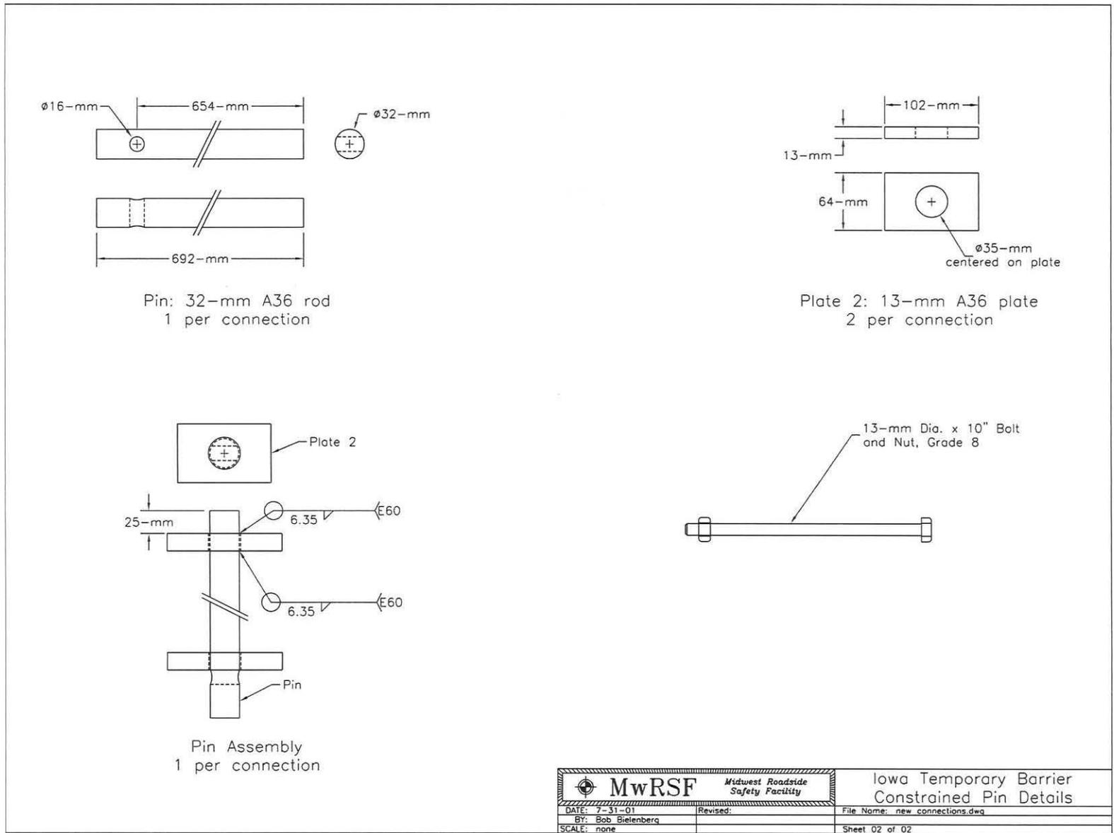
Figure E-5. Tie-Down Temporary Barrier System Details
