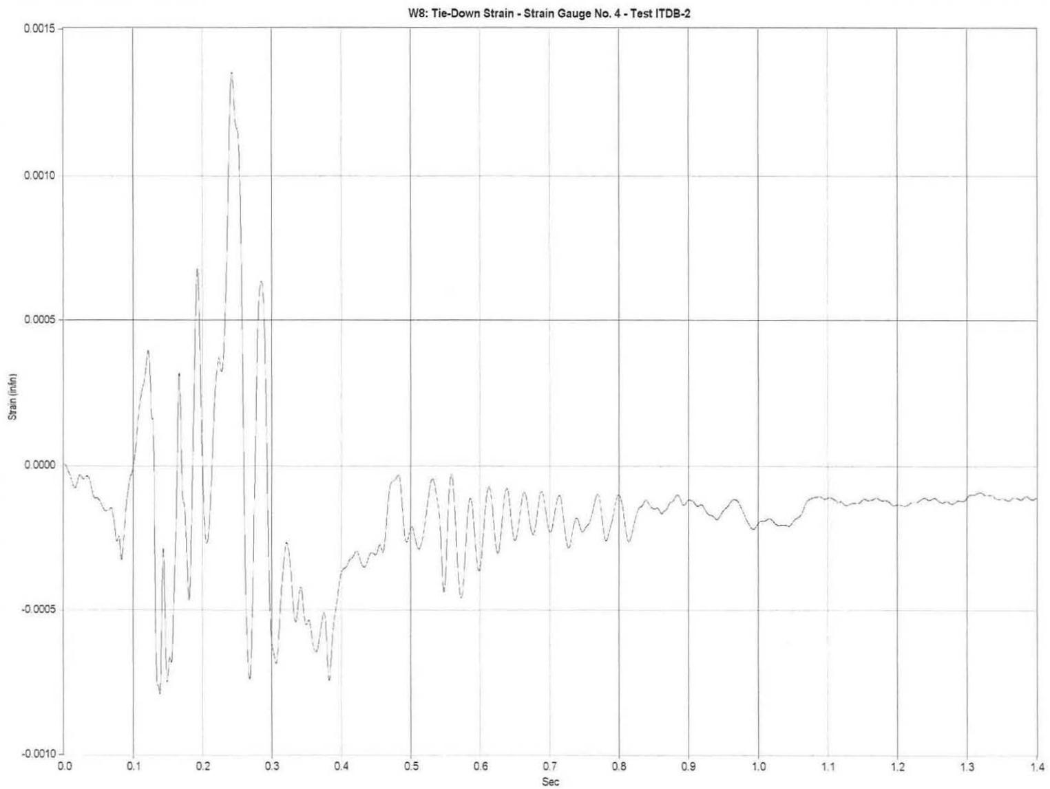
Figure D-5. Graph of Outer Flange Gauge No. 4 Top Peak Strain, Test ITDB-2
