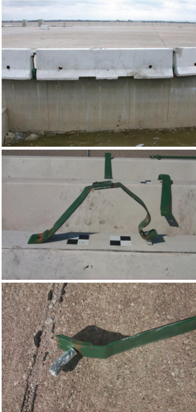
Figure 42. System Damage, Test ITD-1
