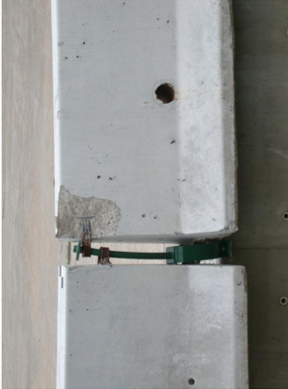
Figure 41. System Damage, Test ITD-1
