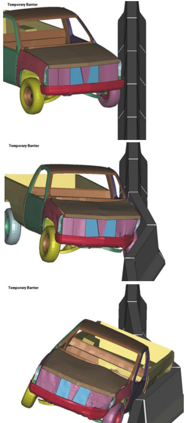
Figure 10b. Without Tie-Down Anchors
