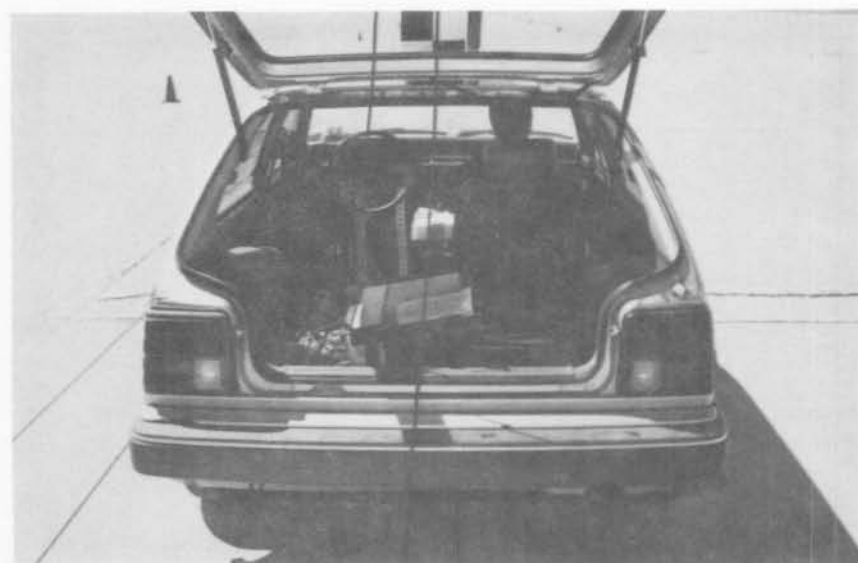
FIGURE 10. PHOTOGRAPHS OF THE ONBOARD DATA ACQUISITION SYSTEM
