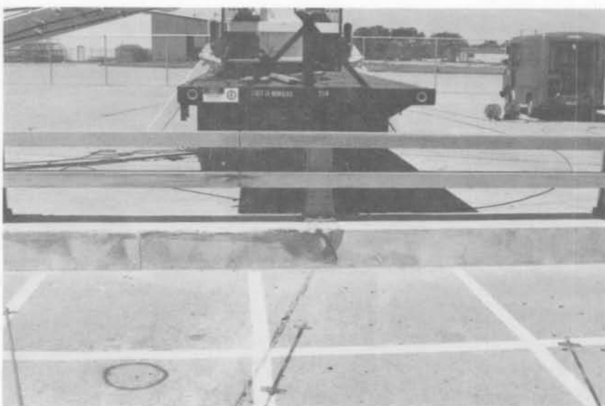
FIGURE 16. PHOTOGRAPHS OF BOX-ALUMINUM BRIDGE RAIL DAMAGE, TEST 11-1
