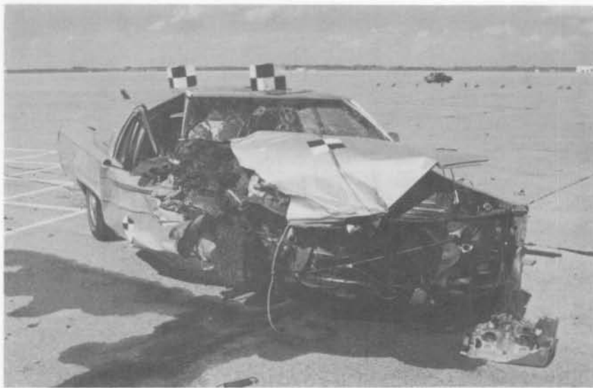
FIGURE 18. PHOTOGRAPHS OF VEHICLE DAMAGE, TEST 11-2
