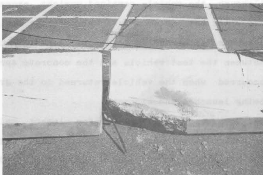
FIGURE 17. TEMPORARY CONCRETE BARRIER RAIL CONNECTOR DAMAGE
