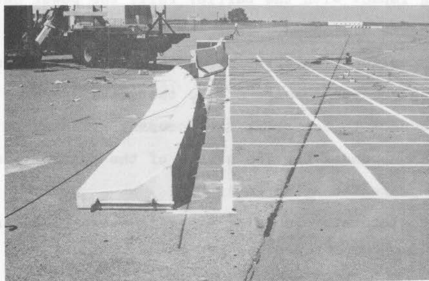
FIGURE 16. TEMPORARY CONCRETE BARRIER RAIL DAMAGE
