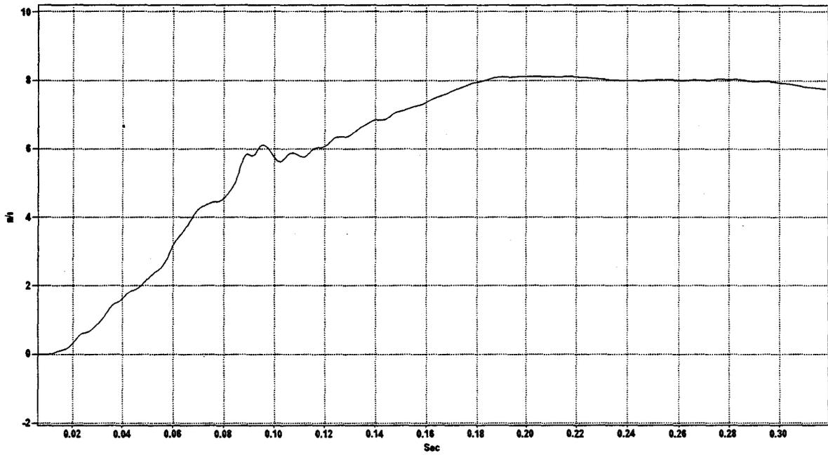
Figure C-2. Graph of Longitudinal Occupant Impact Velocity, Test KTS-1
