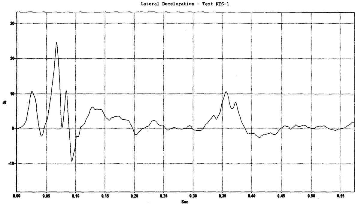
Figure C-4. Graph of Lateral Deceleration, Test KTS-1
