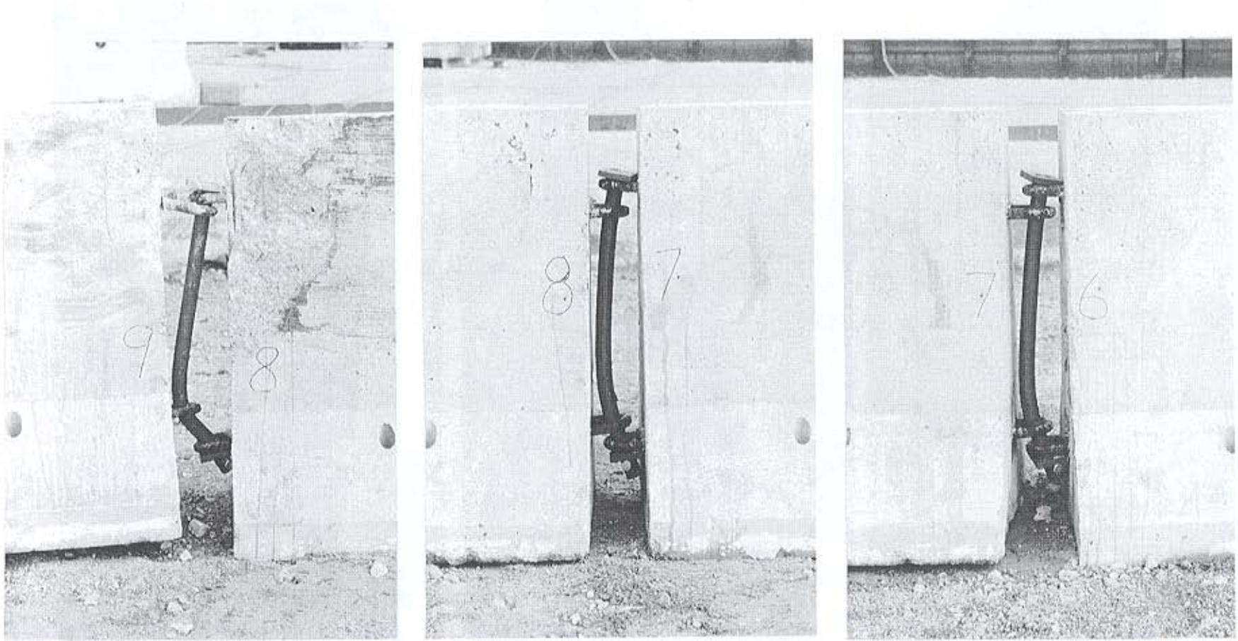
Figure 17. Damage of Barrier Ends (Traffic Side), KTS-1
