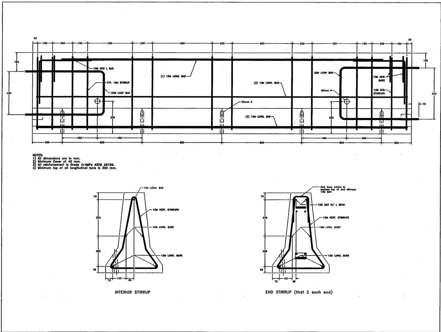
Figure B-5. Reinforcement Details for KTS-1
