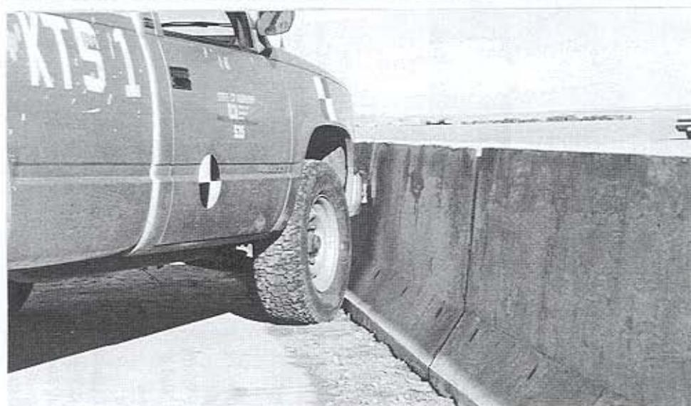
Figure 9. Impact Location, Test KTS-1
