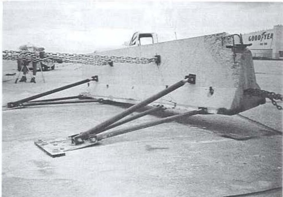
Figure 3. Angled Load Static Test
