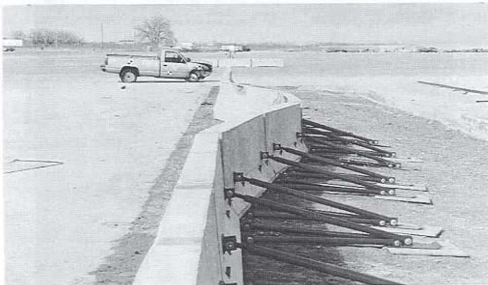
Figure 15. Barrier Damage, Test KTS-1
