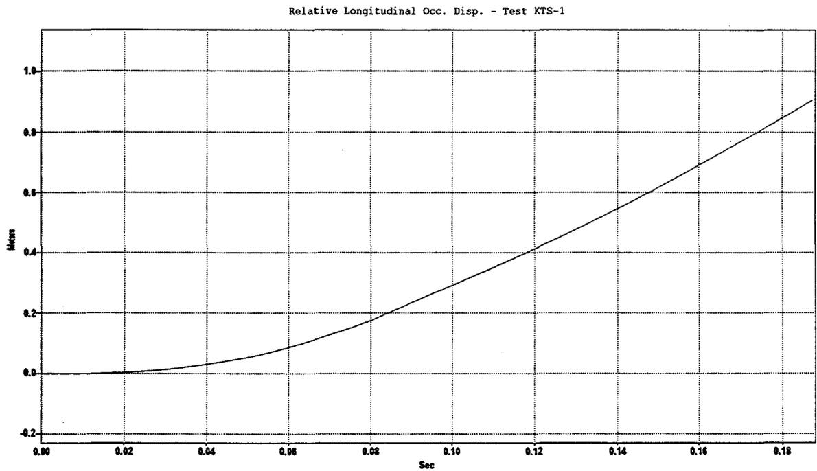
Figure C-3. Graph of Longitudinal Occupant Displacement, Test KTS-1
