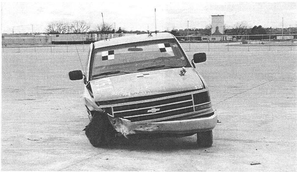
Figure 14. Vehicle Damage, Test KTS-1
