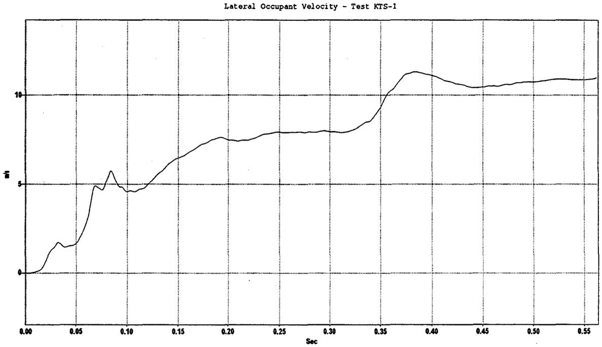
Figure C-5. Graph of Lateral Occupant Impact Velocity, Test KTS-1
