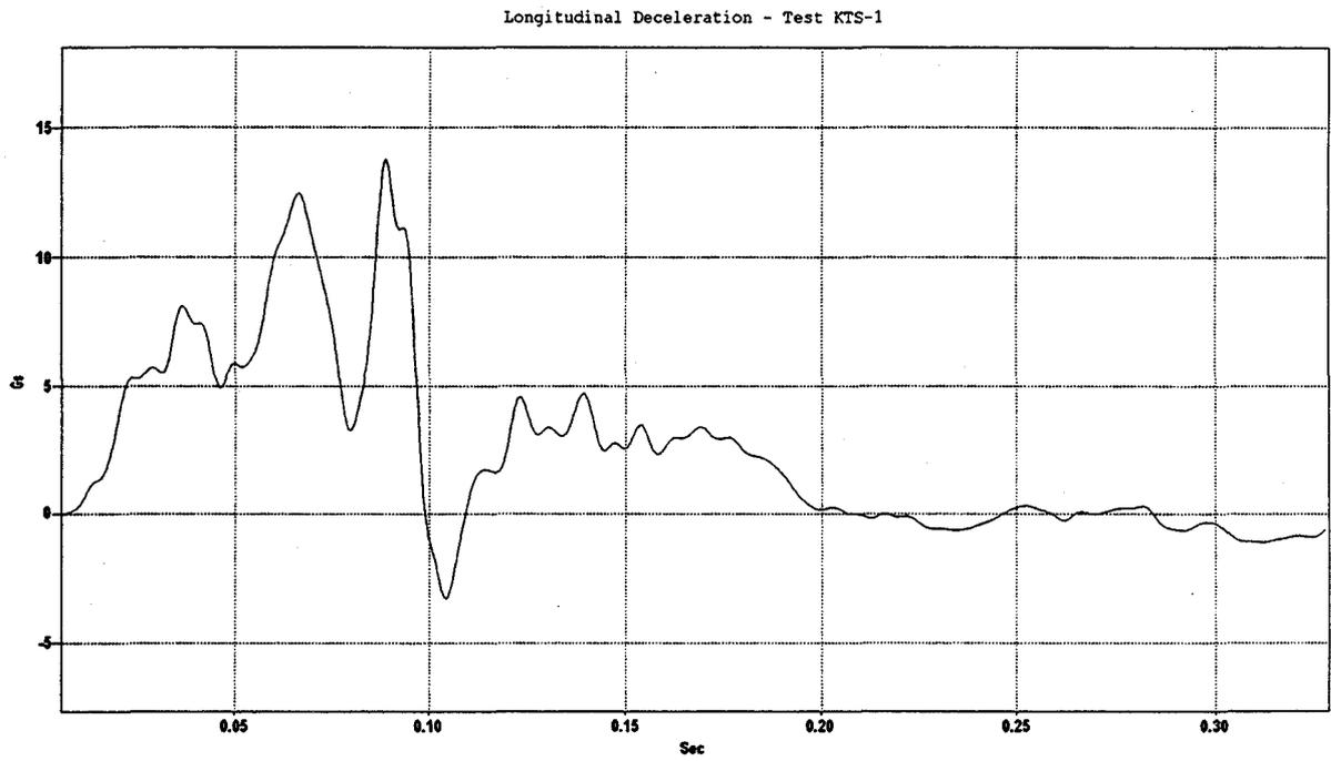
Figure C-1. Graph of Longitudinal Deceleration, Test KTS-1
