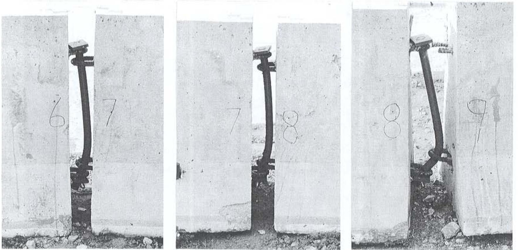
Figure 16. Damage of Barrier Ends (Back Side), KTS-1
