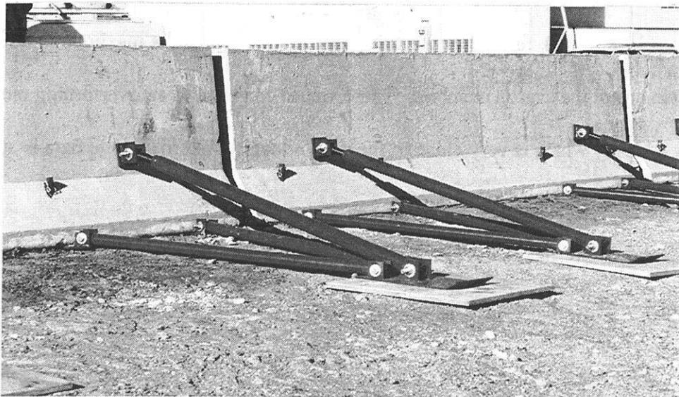
Figure 8. Portable Concrete Barrier System with Ski Design, Test KTS-1
