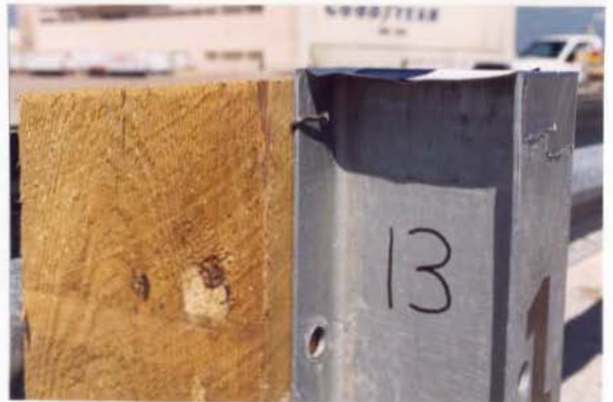
Figure 4. Post-to-Rail Attachment for the Type B (W-beam) Longitudinal Barrier System
