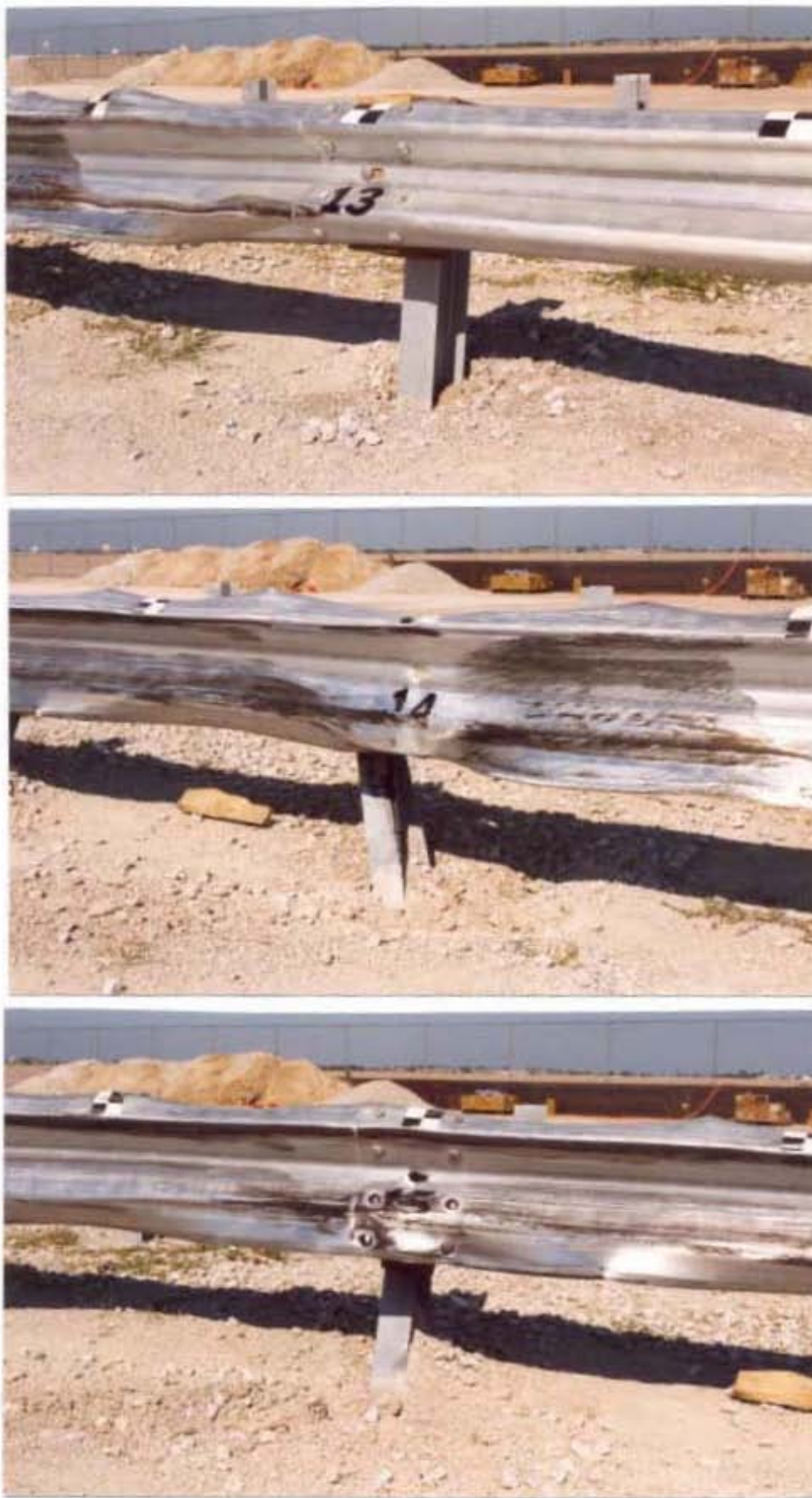
Figure 19. Type B Longitudinal Barrier Rail and Post Damage, Test MIW-1
