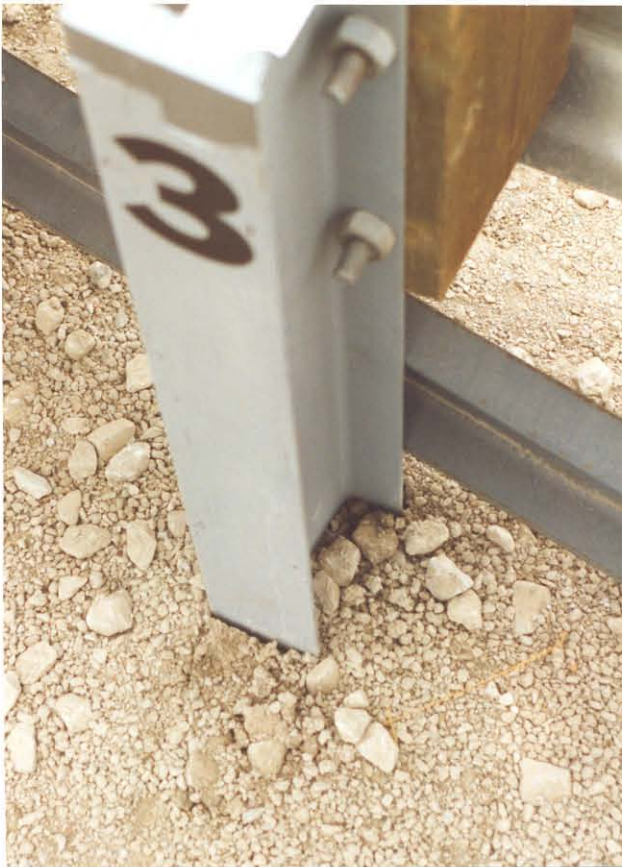
Figure 46. Permanent Set Deflections, Test MST-2
