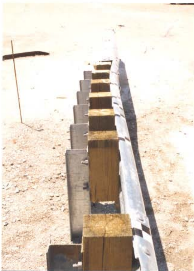
Figure 25. Permanent Set Deflections, Test MST-1
