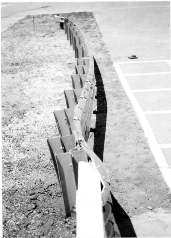
Figure 23. Bridge Anchor Section Damage, Test MBAS-1
