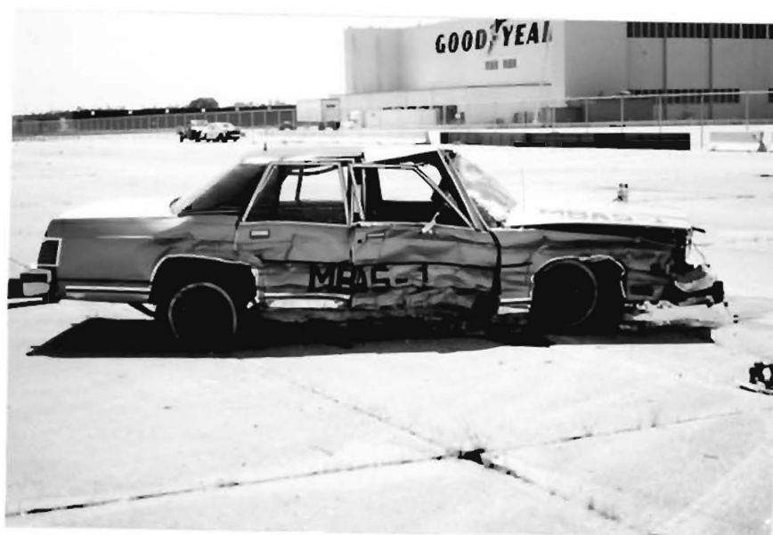
Figure 18. Vehicle Damage, Test MBAS-1
