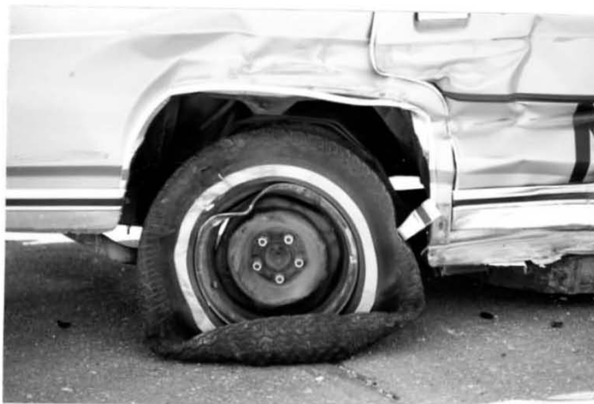
Figure 19. Vehicle Damage, Test MBAS-1
