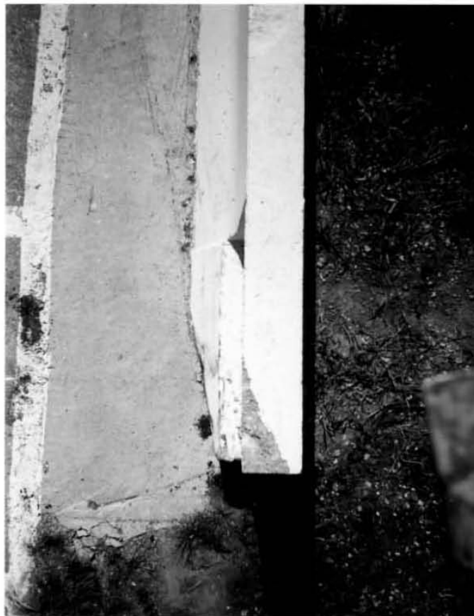
Figure 24. Concrete End Section Damage, Test MBAS-1
