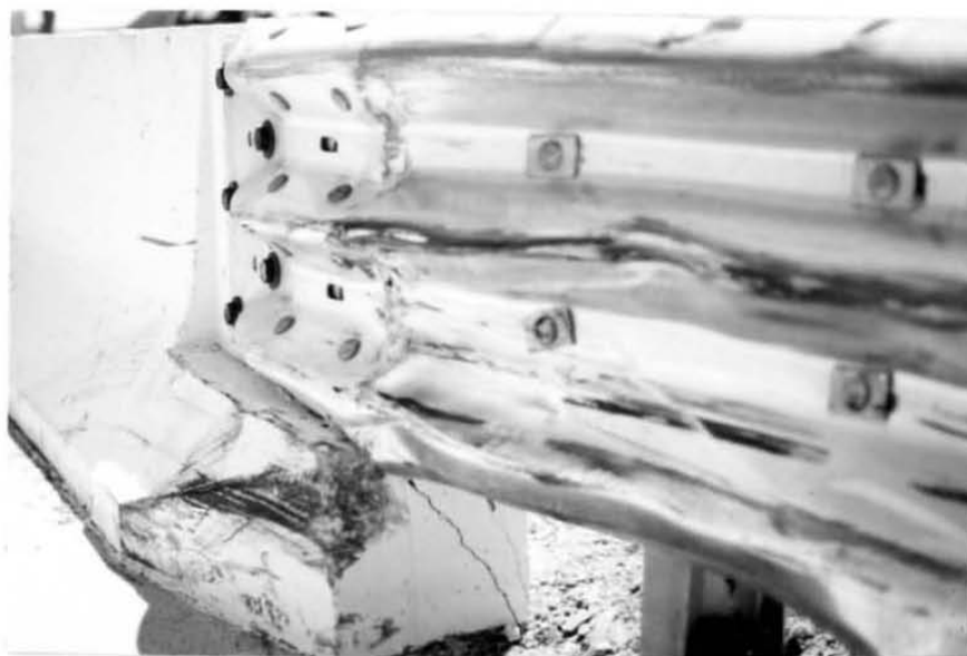
Figure 22. Bridge Anchor Section Damage, Test MBAS-1
