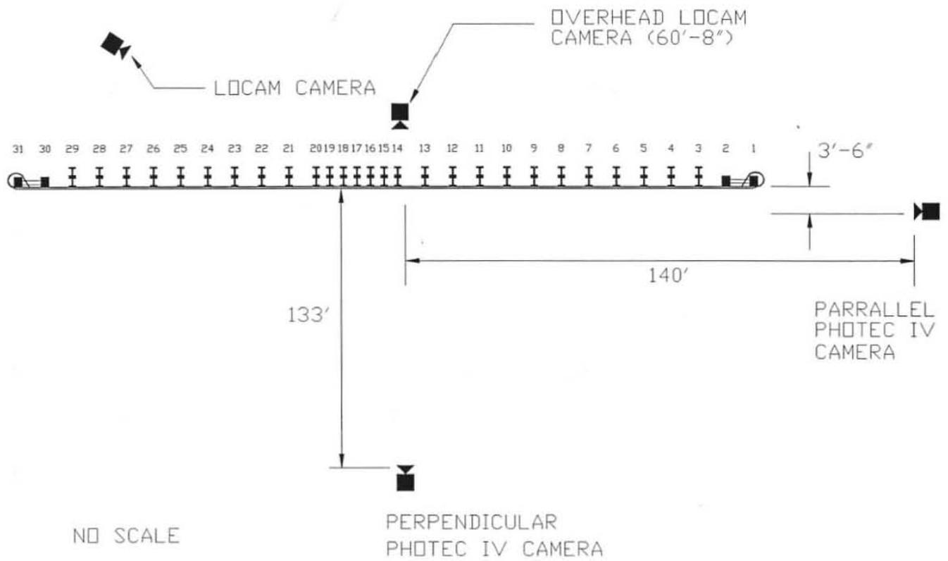
FIGURE 5. Schematic of camera locations
