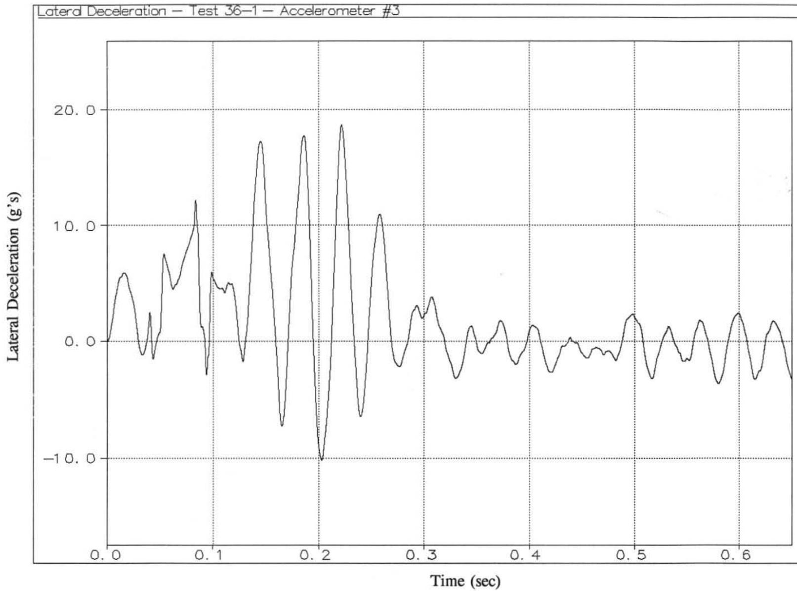
Figure A-2. Graph of Lateral Deceleration, Test 36-1
