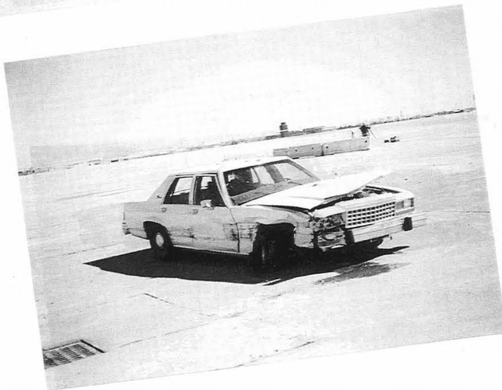
Figure 49. Vehicle Damage, Test SBT-5 (cont.).
