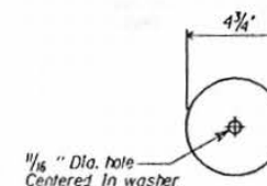
PLATE WASHER DETAIL 4 3/4" Dia. x 1/4"
