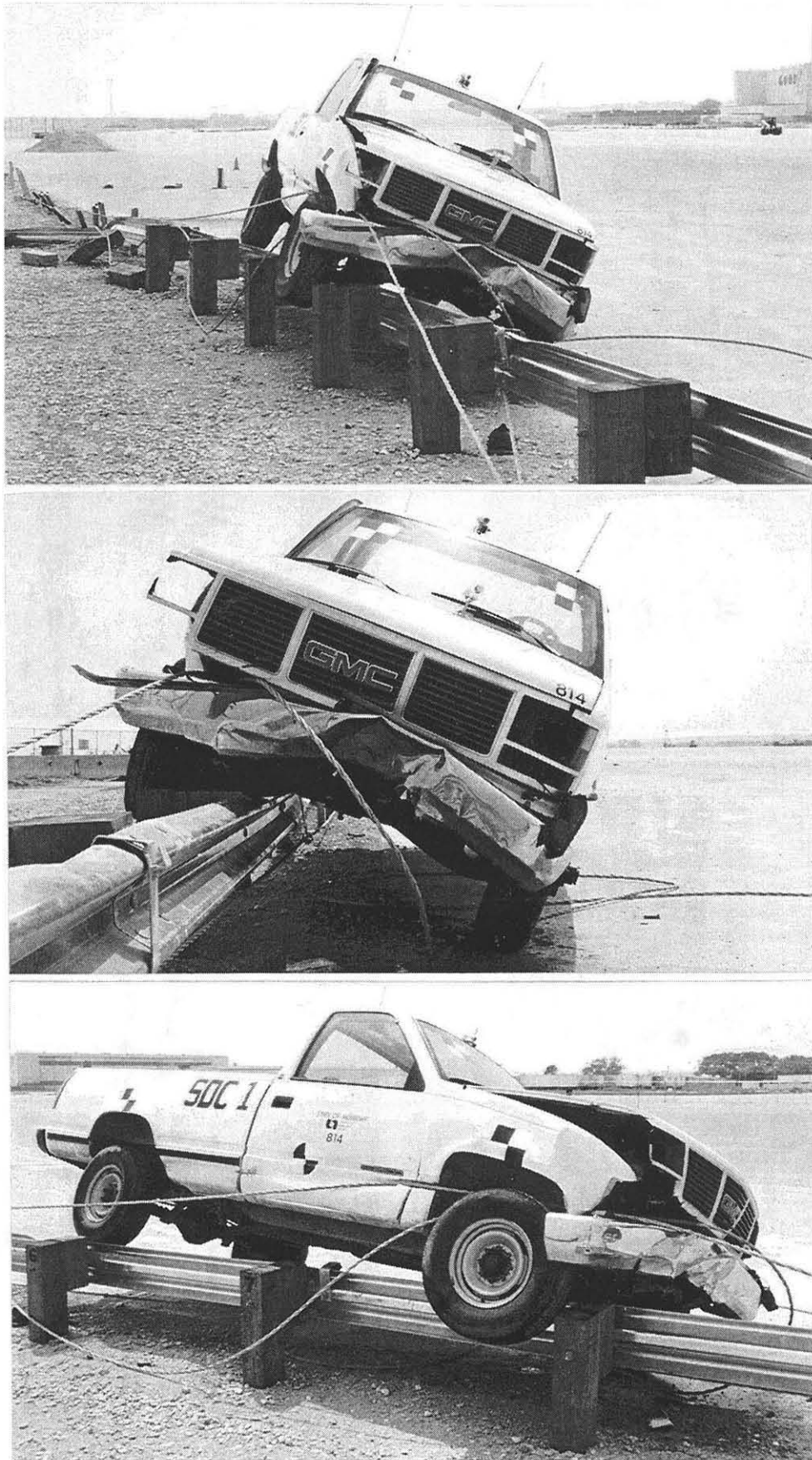
Figure 29. Vehicle Damage, Test SDC-1
