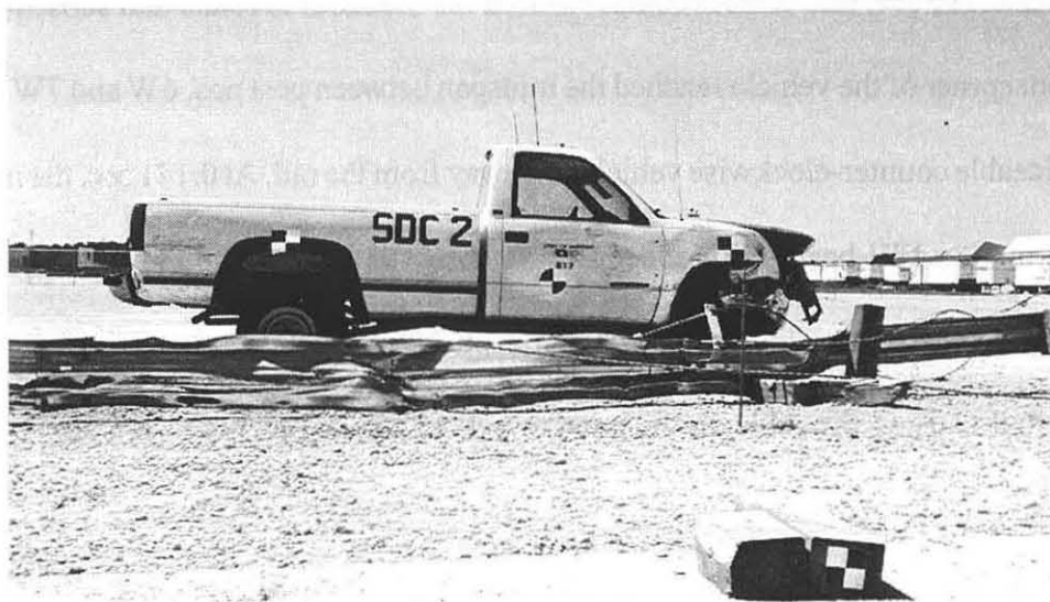
Figure 40. Vehicle Damage, Test SDC-2
