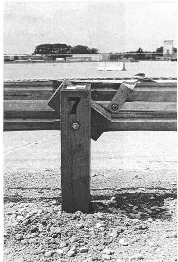
Figure 47. Cable Guardrail to W-Beam Transition Damage, Test SDC-3
