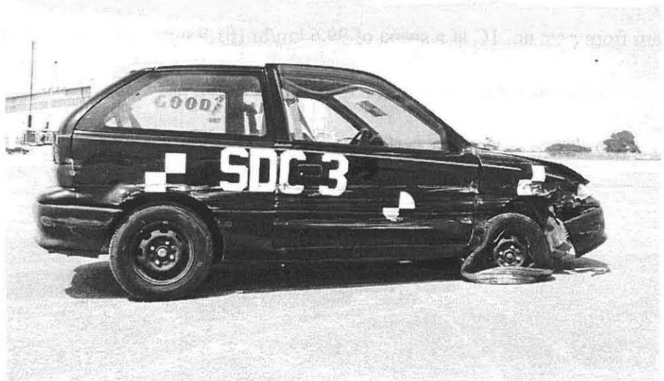
Figure 48. Vehicle Damage, Test SDC-3
