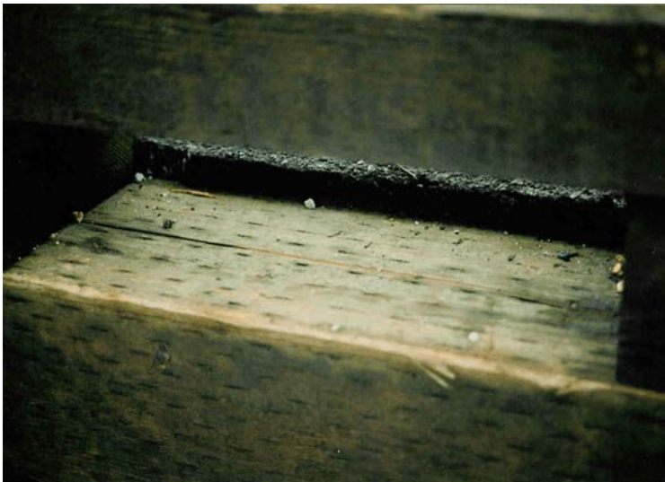
Figure 107. Deck Cracking Between Post Nos. 6 and 7, 8 and 9, Test FSCR-4
