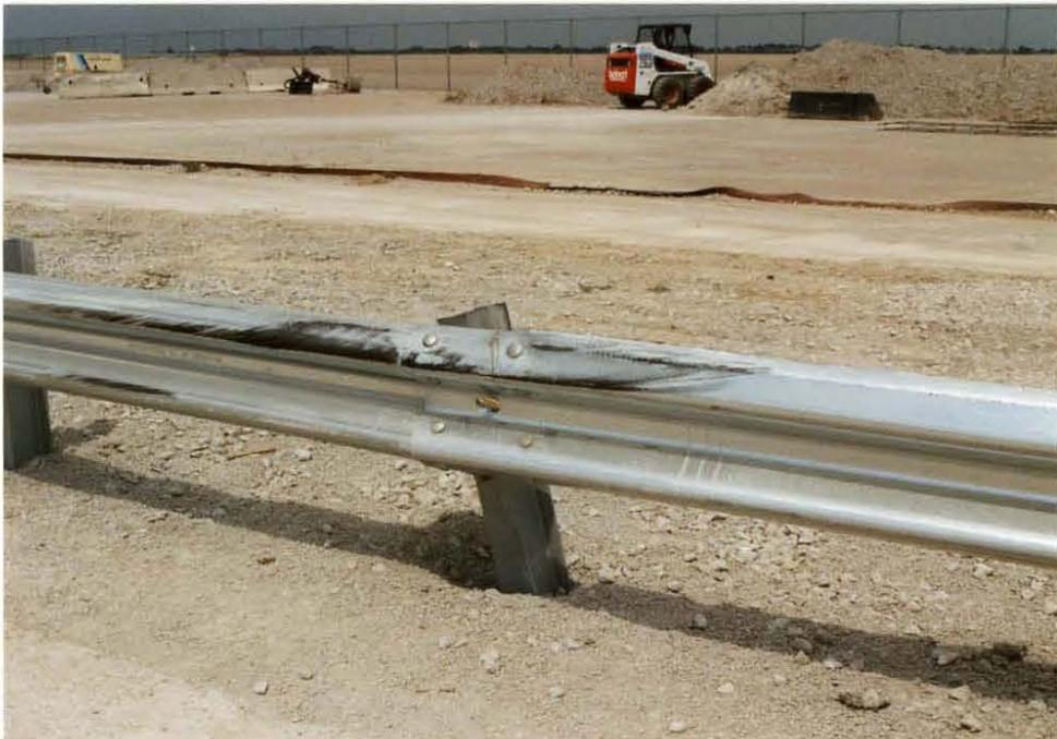
Figure 16. Guardrail Over Curb System Damage, Test NEC-2
