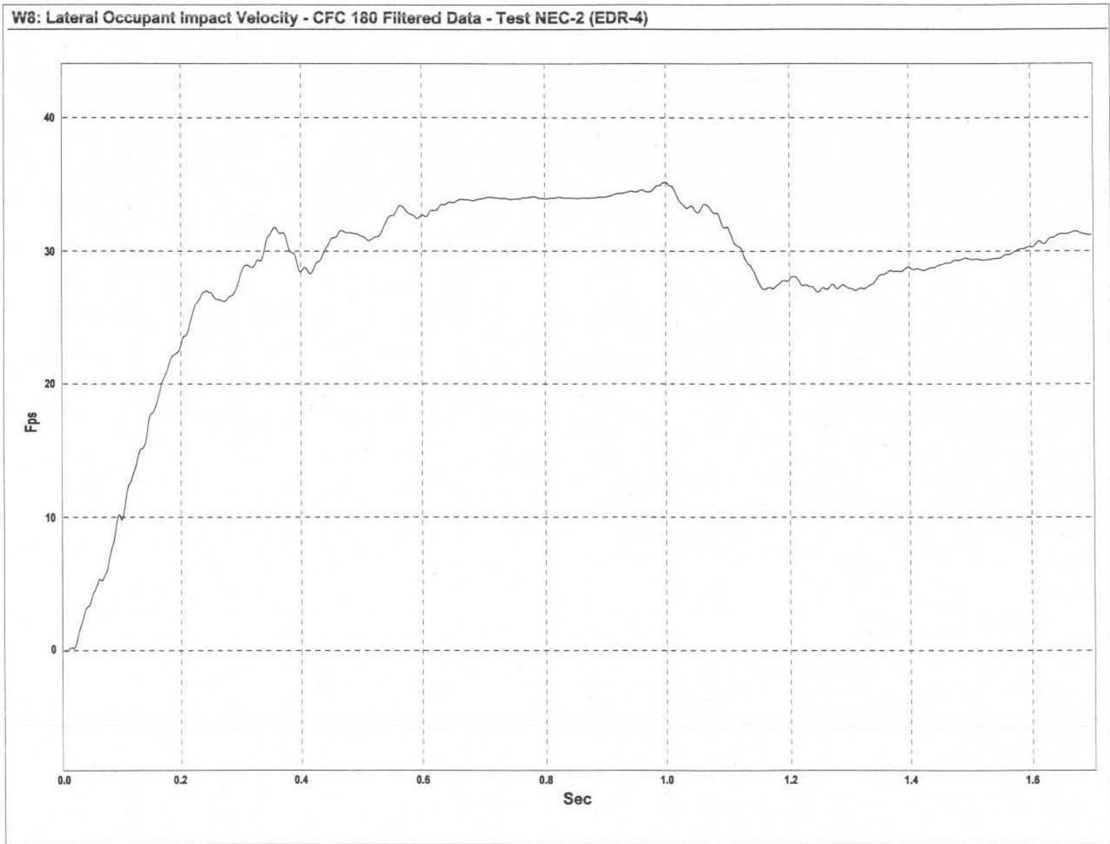
Figure A-5. Graph of Lateral Occupant Impact Velocity, Test NEC-2
