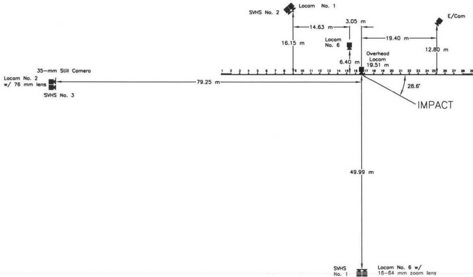
Figure 7. Location of High-Speed Cameras, Test NEC-2
