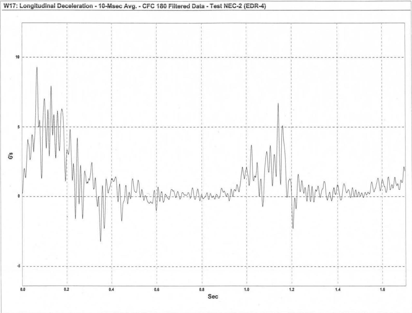
Figure A-1. Graph of Longitudinal Deceleration, Test NEC-2
