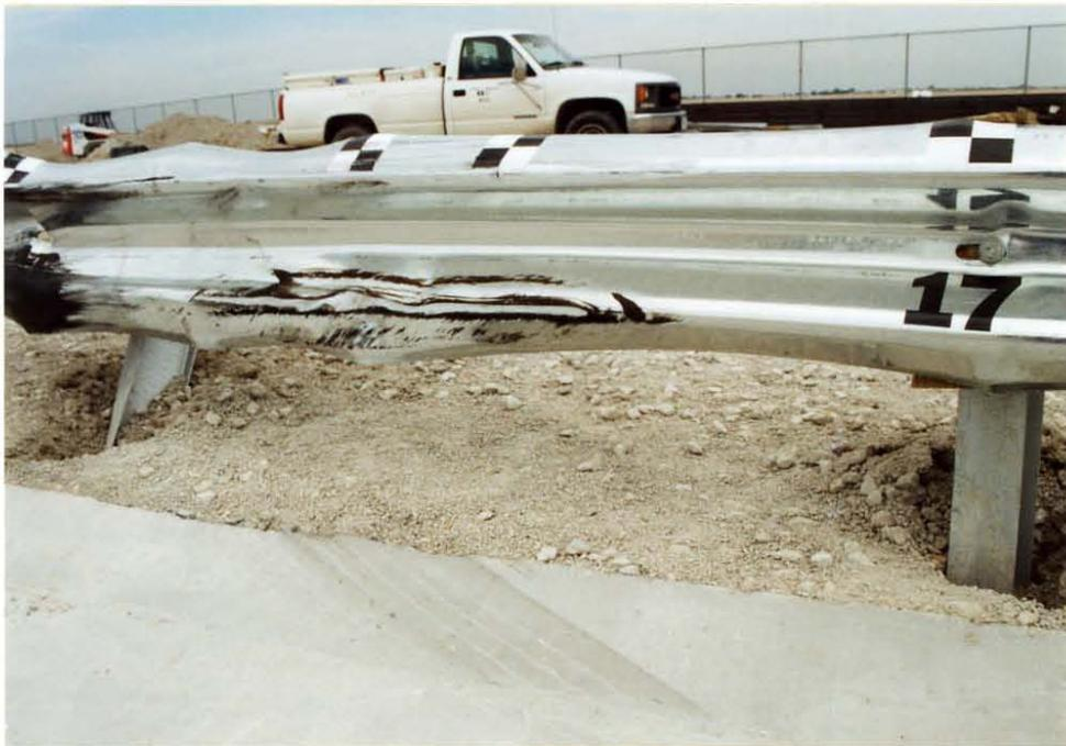
Figure 18. Guardrail Over Curb System Rail and Post Damage, Test NEC-2
