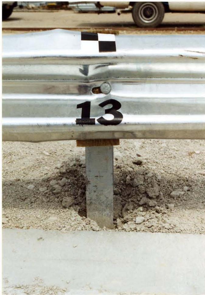
Figure 20. Guardrail Over Curb System Rail and Post Damage, Test NEC-2
