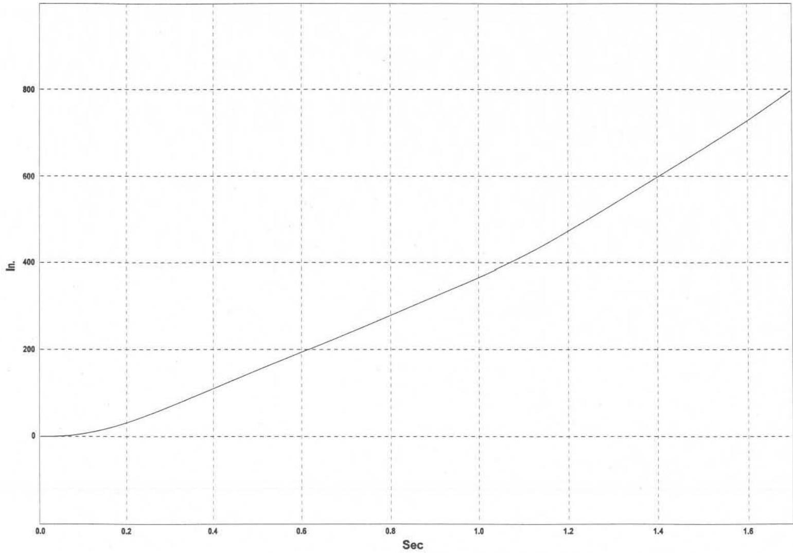
Figure A-3. Graph of Longitudinal Occupant Displacement, Test NEC-2
