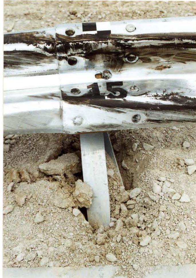
Figure 19. Guardrail Over Curb System Rail and Post Damage, Test NEC-2
