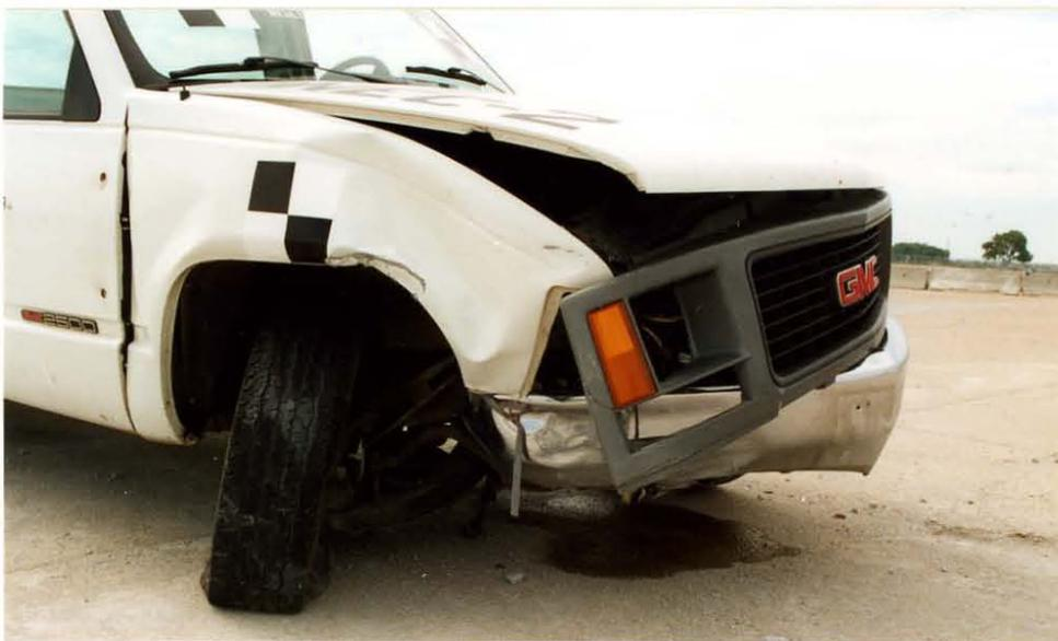
Figure 27. Front-End Vehicle Damage, Test NEC-2
