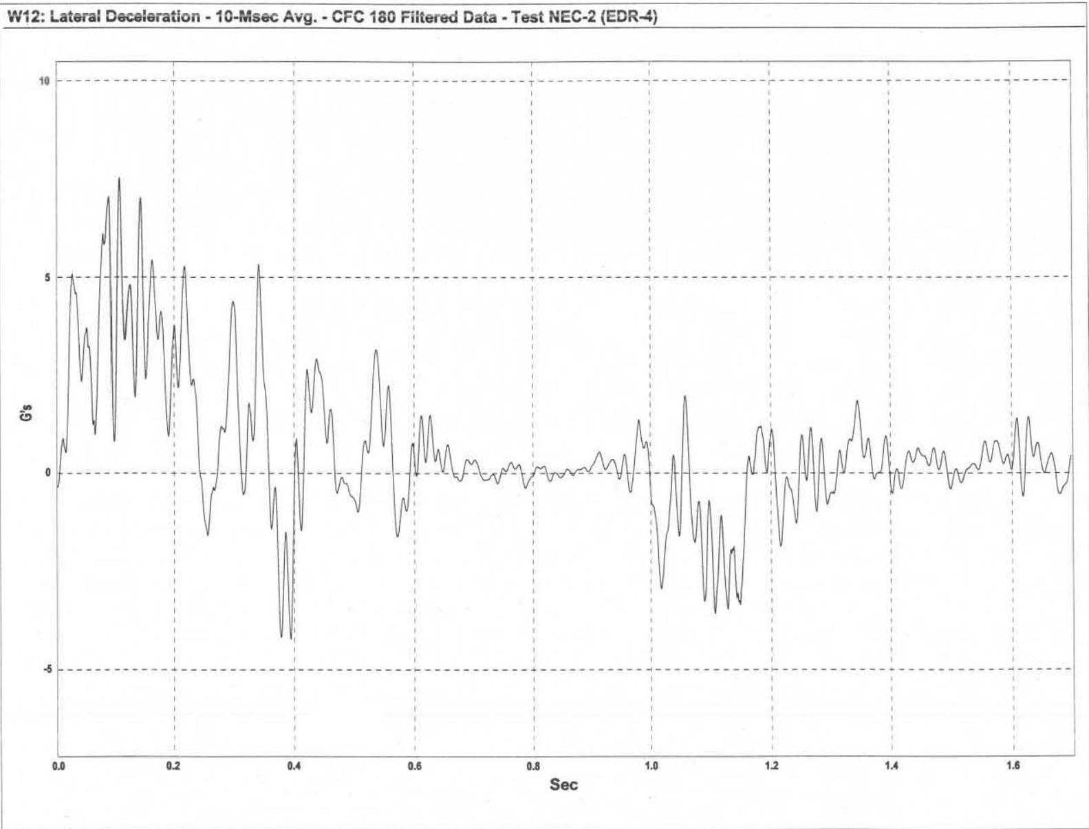
Figure A-4. Graph of Lateral Deceleration, Test NEC-2
