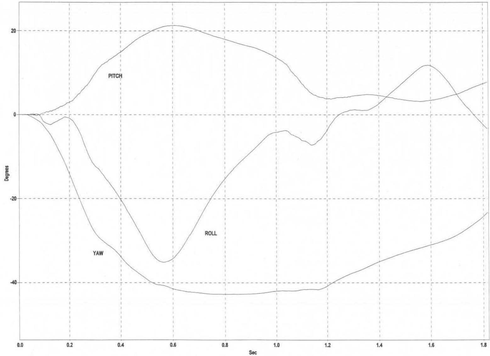
Figure B-1. Graph of Roll, Pitch, and Yaw Angular Displacements, Test NEC-2
