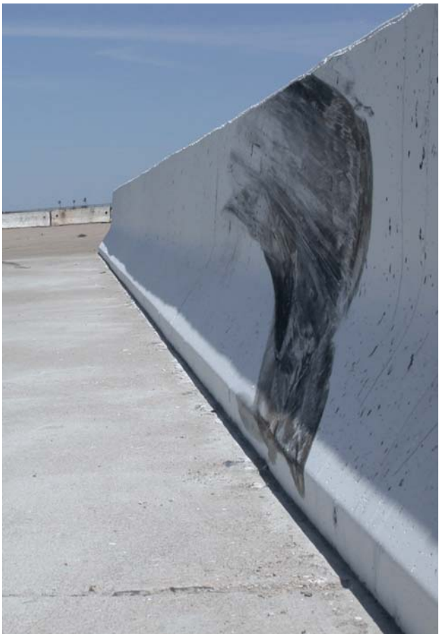
Figure 22. Permanent New Jersey Safety Shape Barrier Damage, Test 2214NJ-1
