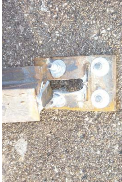
Figure 24. Post and Plate Damage, Bogie Test KCB-1b
