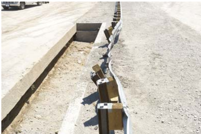
Figure 48. W-Beam Guardrail System Damage, Test KC-1
