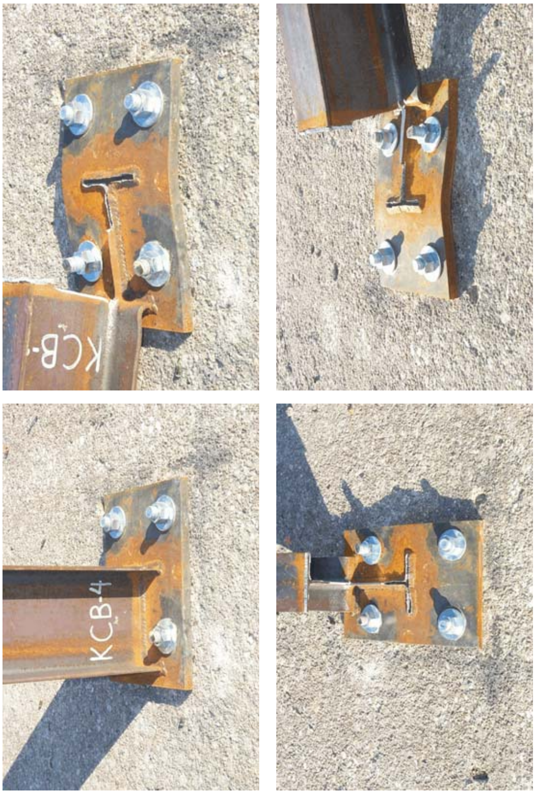
Figure 27. Post and Plate Damage, Bogie Test KCB-4
