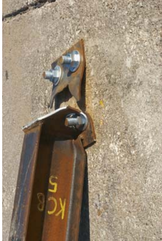
Figure 28. Post and Plate Damage, Bogie Test KCB-5
