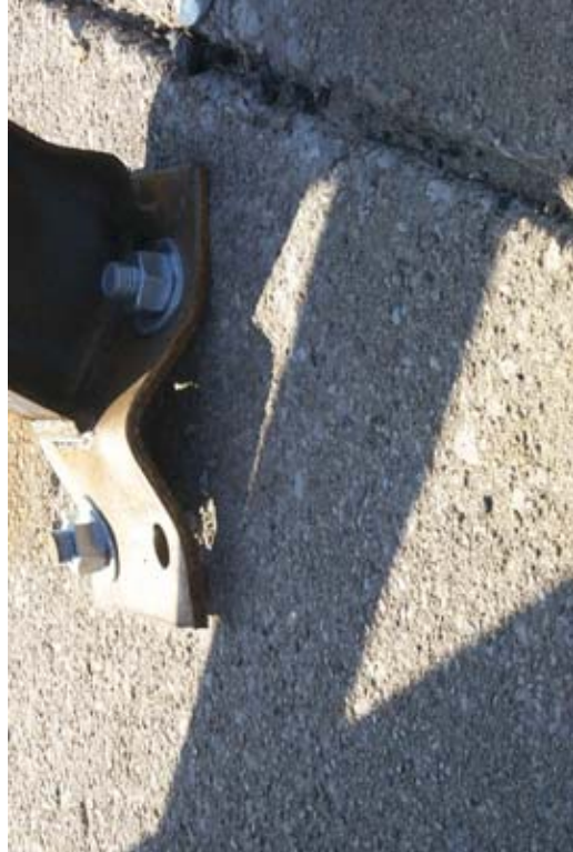
Figure 29. Post and Plate Damage, Bogie Test KCB-6
