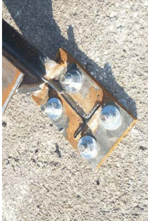
Figure 25. Post and Plate Damage, Bogie Test KCB-2
