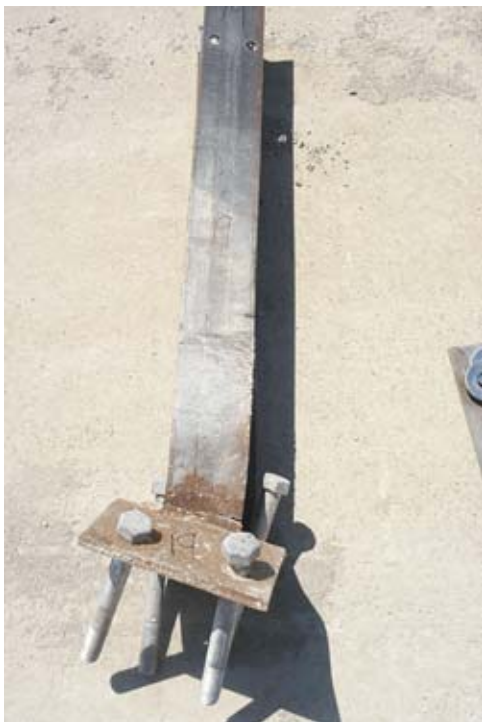
Figure 53. Post Nos.18 and 19 Damage, Test KC-1
