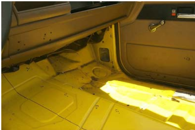
Figure 65. Occupant Compartment Deformations, Test KC-1
