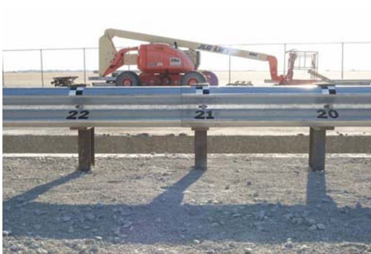
Figure 36. W-Beam Guardrail Attached to a Low-Fill Culvert (Option No. 1)
