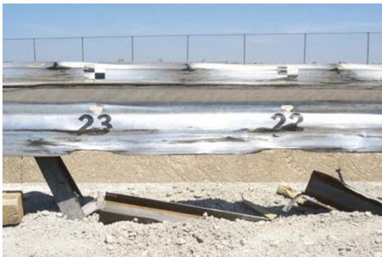
Figure 50. W-Beam Guardrail System Damage, Test KC-1
