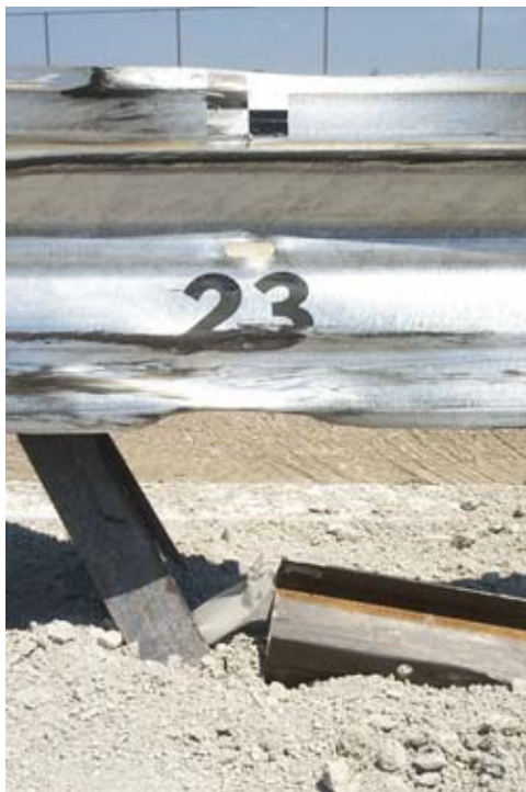
Figure 56. Post Nos. 22 and 23 Damage, Test KC-1
