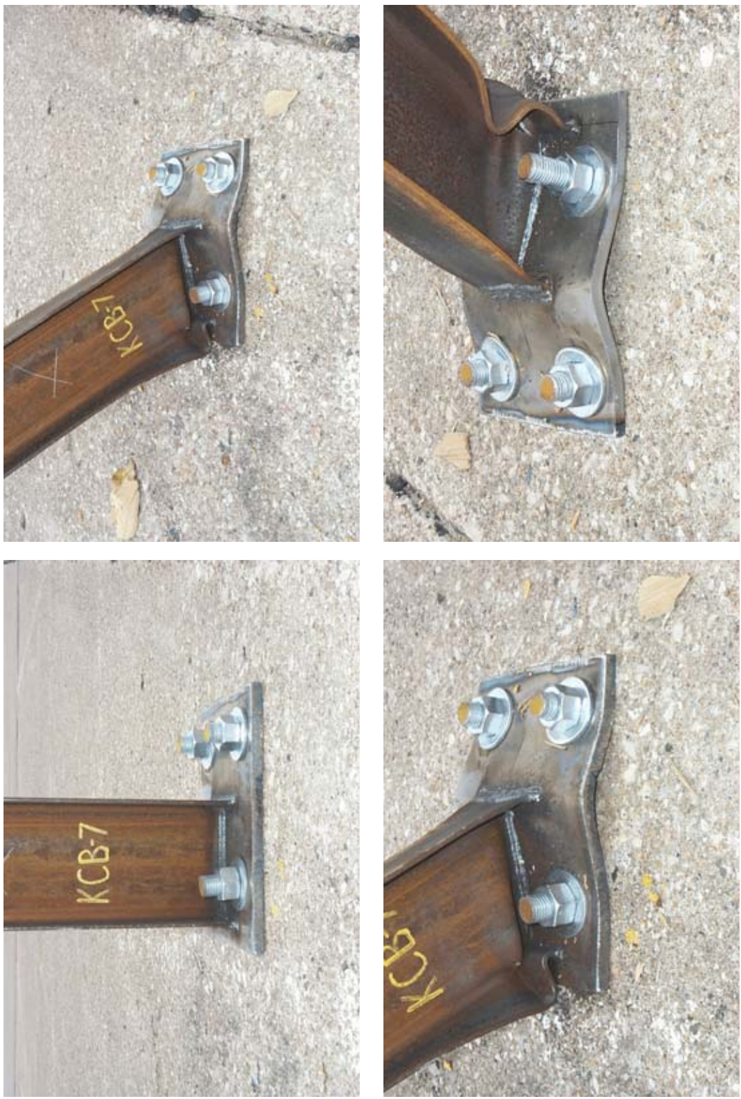
Figure 30. Post and Plate Damage, Bogie Test KCB-7
