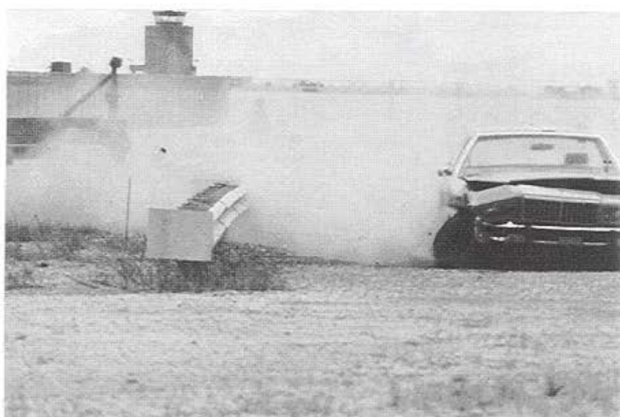
Figure 38. Full-Scale Crash Test (continued), KSWB-4
