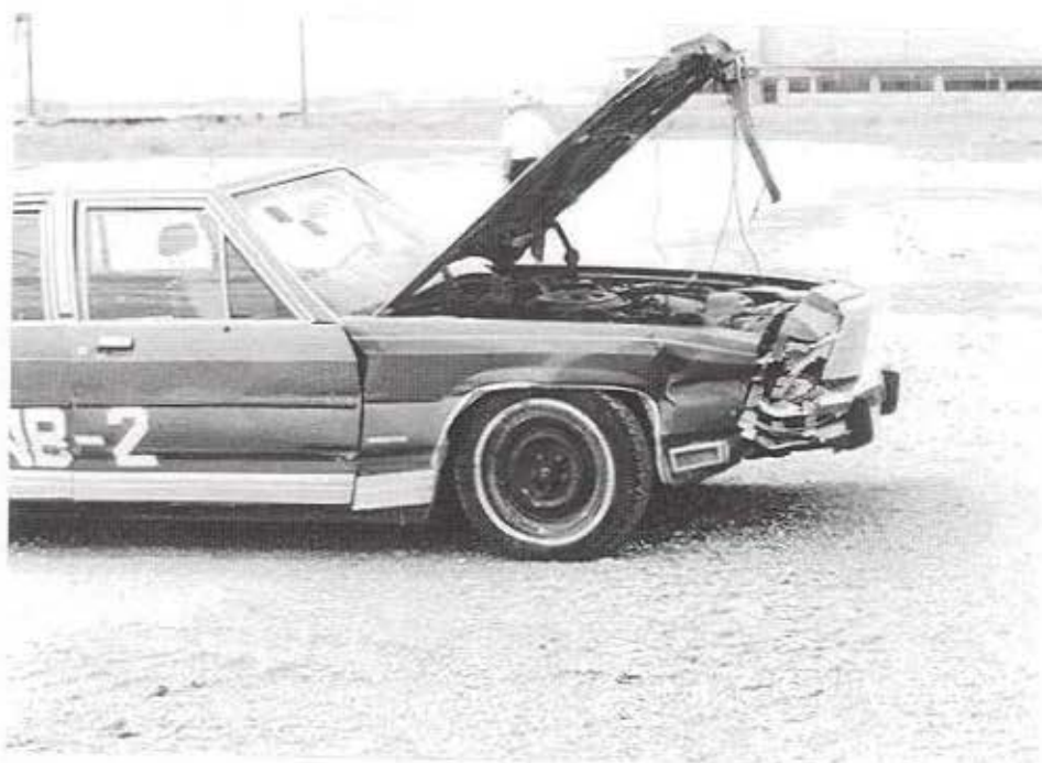
Figure 25. Test Vehicle Damage, KSWB-2
