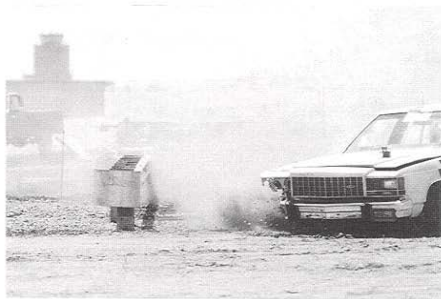
Figure 17. Full-Scale Crash Test (continued), KSWB-1
