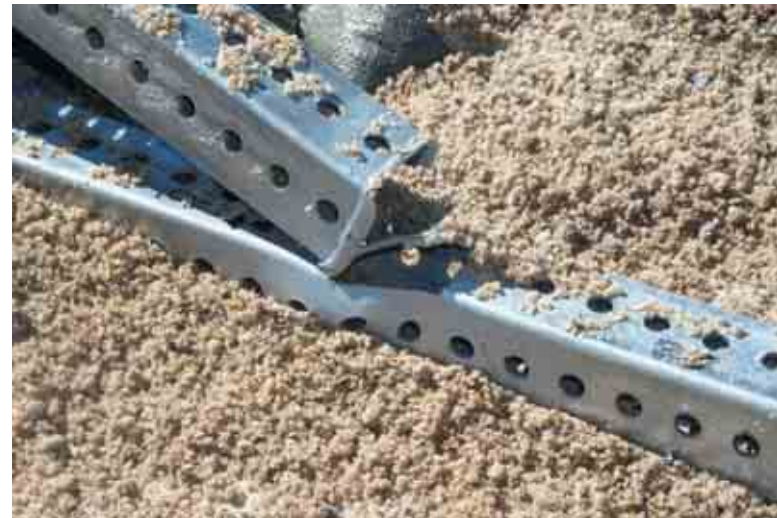
Figure 55. Stop Sign System with 7' Mounting Height Damage, Bogie Test MN8A-90 (90 degrees)
