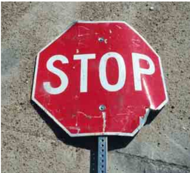
Figure 55. Stop Sign System with 7' Mounting Height Damage, Bogie Test MN8A-90 (90 degrees)
