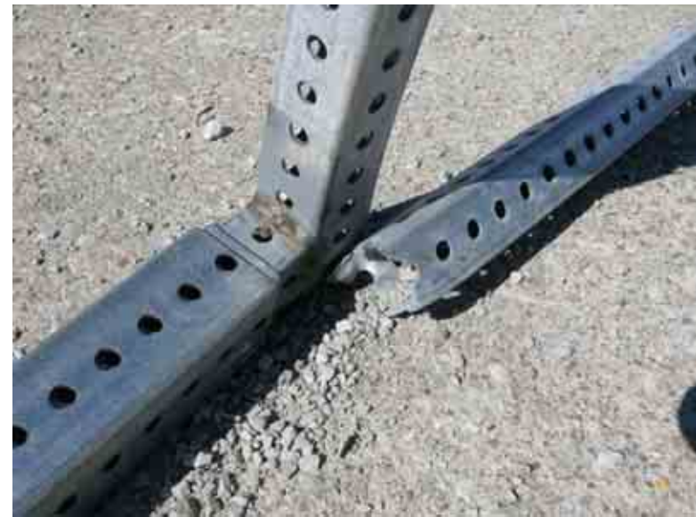
Figure 48. 48" x 48" Diamond Panel Work Zone Sign System with 7' Mounting Height Damage, Bogie Test MN7A-90 (90 degrees)
