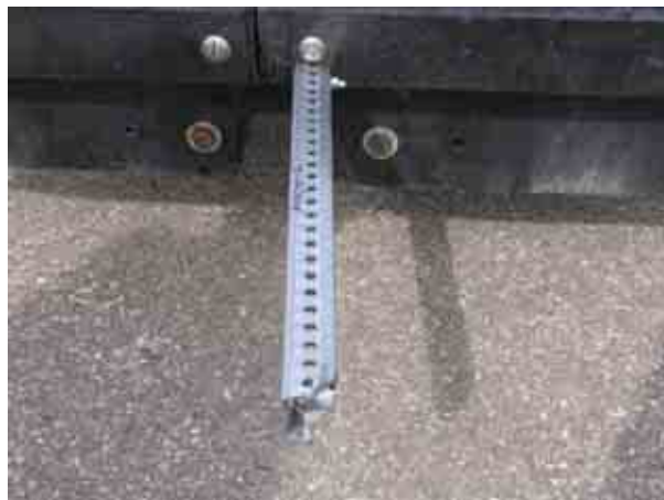
Figure 31. 36" x 36" Diamond Work Zone Sign System Damage, Bogie Tests MN5C-90-2
