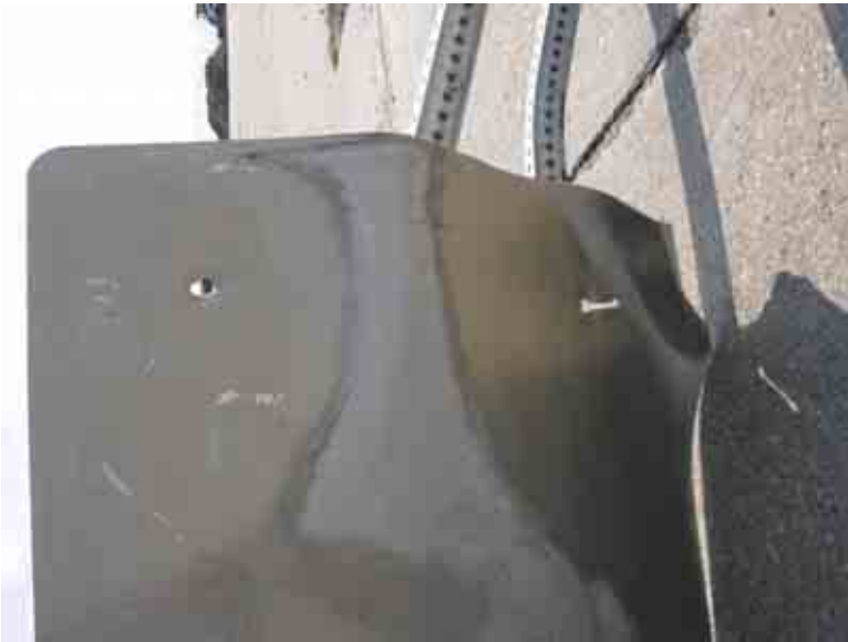
Figure 22. Work Zone Speed Limit Sign System Damage, Bogie Test MN3B-90 (90 degrees)
