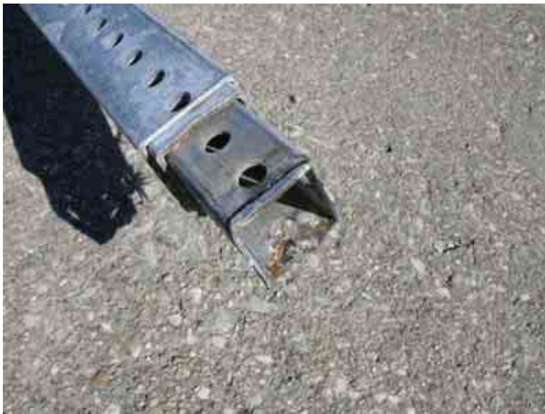
Figure 21. Work Zone Speed Limit Sign System Damage, Bogie Test MN3B-0-2 (0 degrees)
