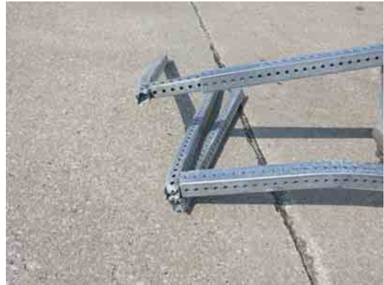
Figure 22. Work Zone Speed Limit Sign System Damage, Bogie Test MN3B-90 (90 degrees)
