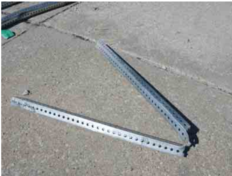
Figure 48. 48" x 48" Diamond Panel Work Zone Sign System with 7' Mounting Height Damage, Bogie Test MN7A-90 (90 degrees)
