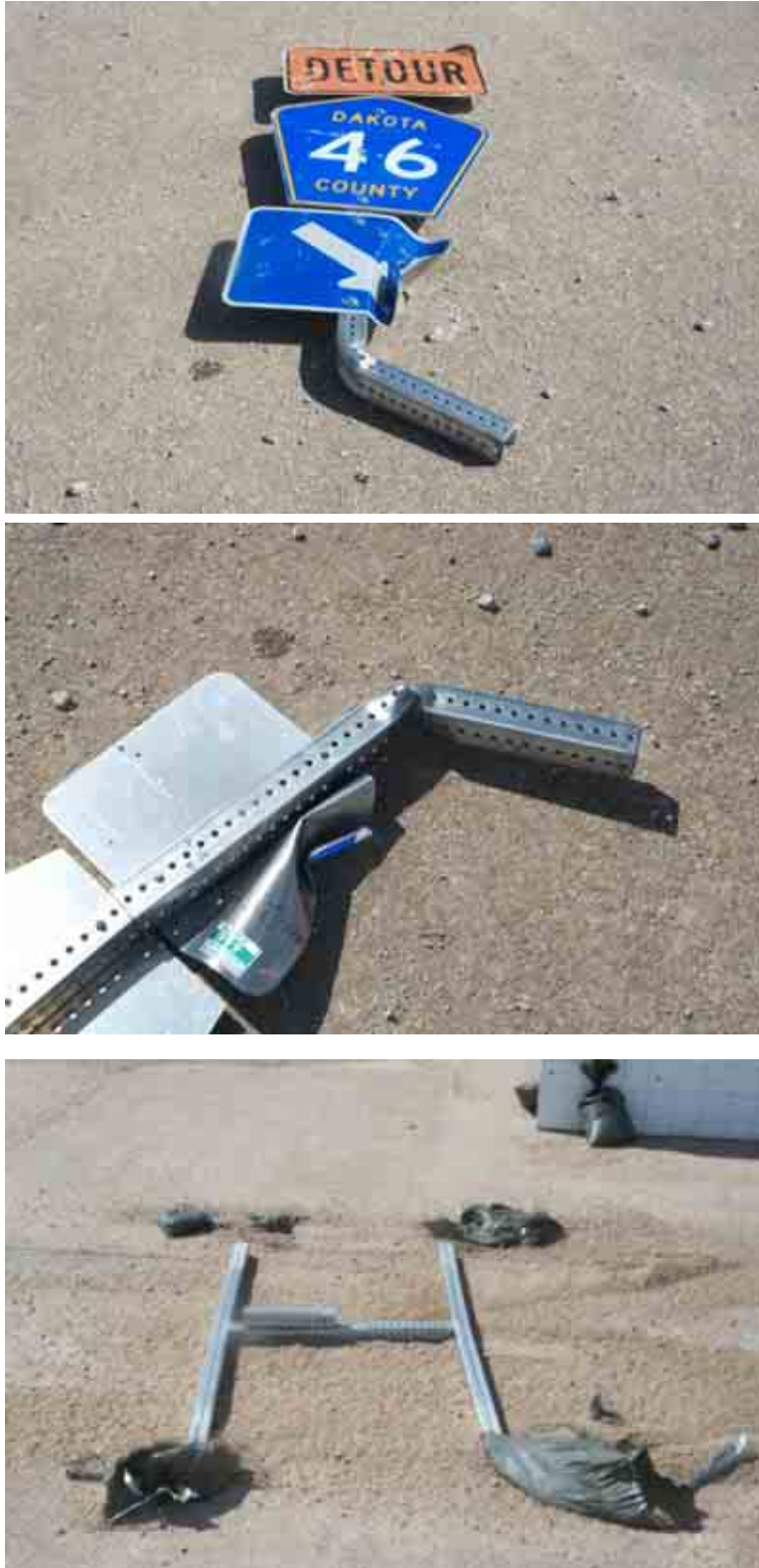
Figure 14. Route Marker Assembly System Damage, Bogie Test MN2C-90 (90 degrees)
