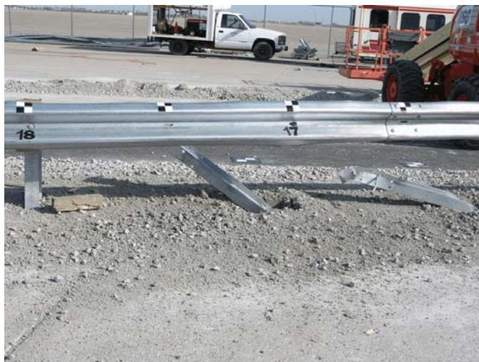
Figure 23. System Damage - Post Nos. 14 through 18, Test 2214MG-3
