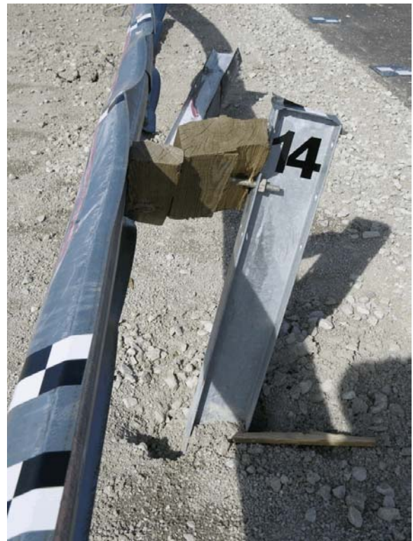
Figure 22. System Damage - Post Nos. 13 and 14, Test 2214MG-3
