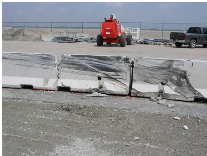
Figure 55. System Damage, Test FTB-2
