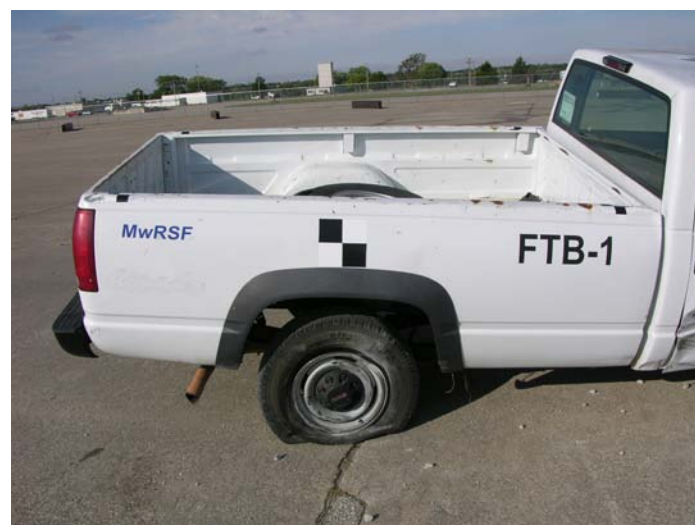
Figure 31. Vehicle Damage, Test FTB-1
