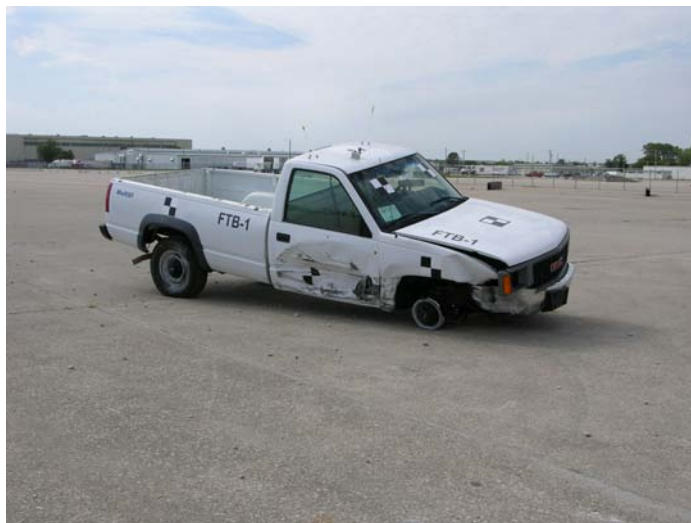
Figure 30. Vehicle Damage, Test FTB-1
