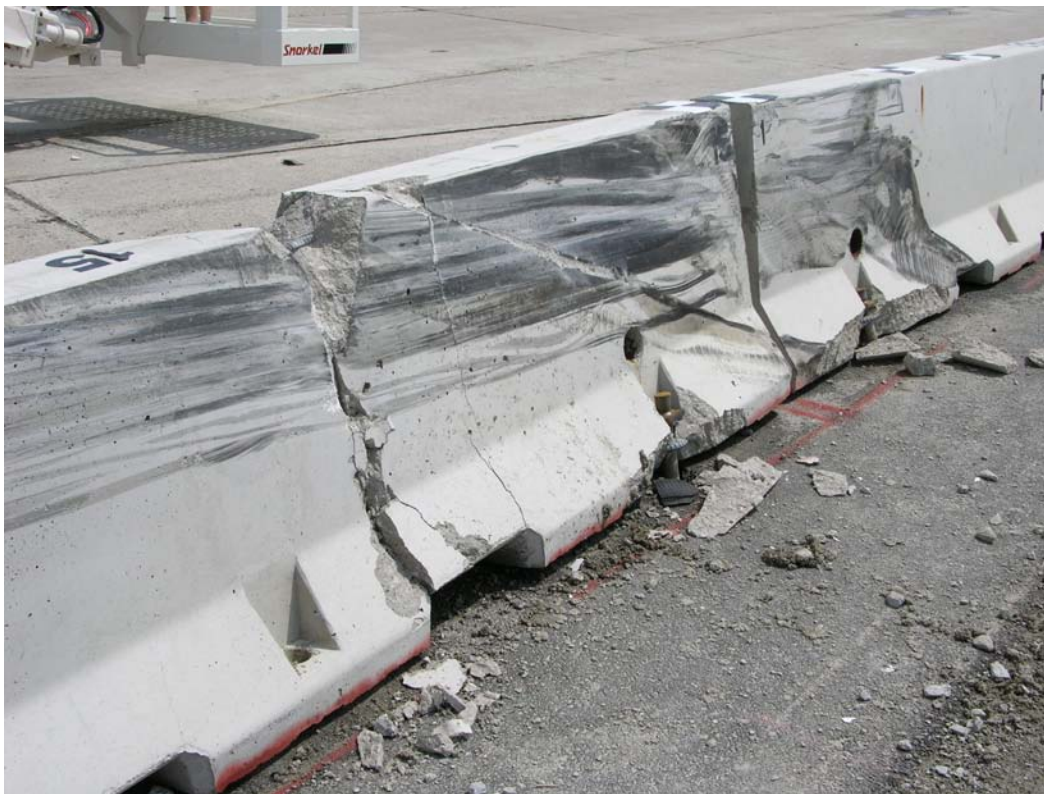
Figure 54. System Damage, Test FTB-2
