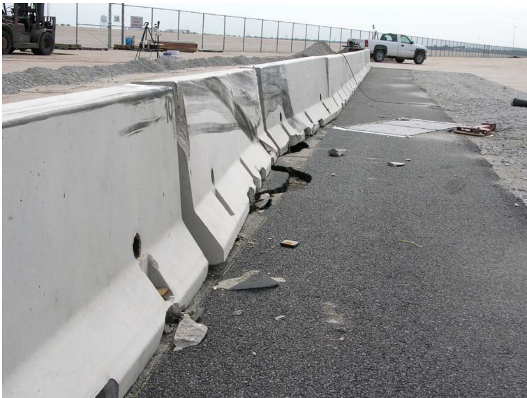
Figure 27. System Damage, Test FTB-1
