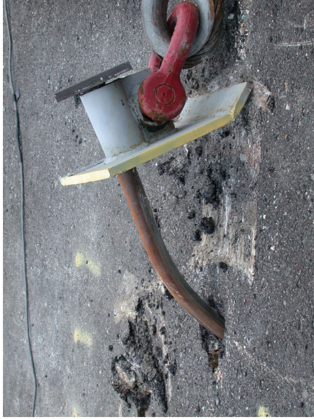
a) 28.575 mm Diameter Pin Peak Load = 84.6 kN
