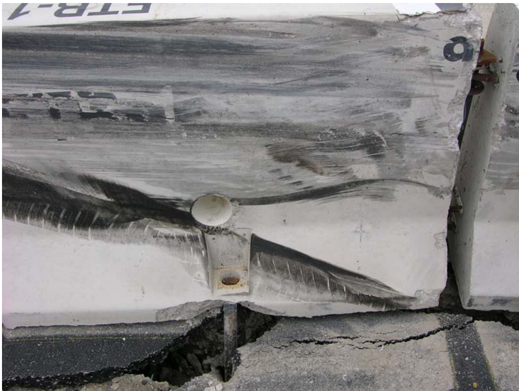
Figure 29. System Damage, Test FTB-1
