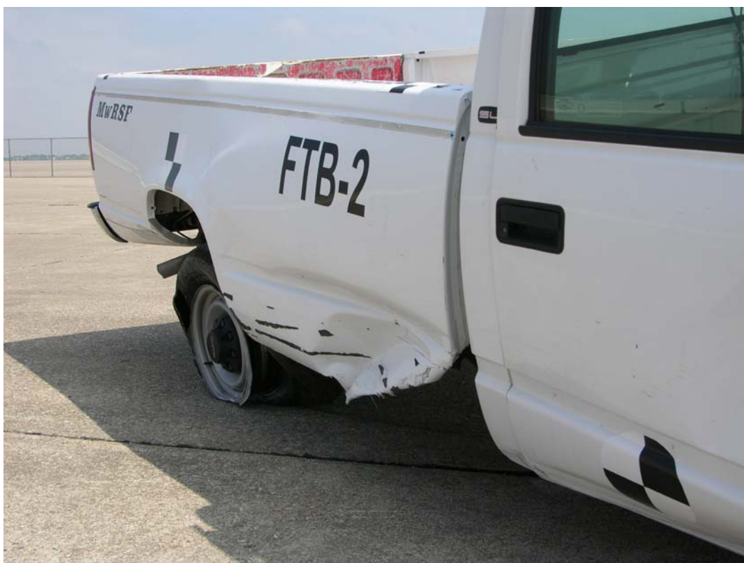
Figure 58. Vehicle Damage, Test FTB-2
