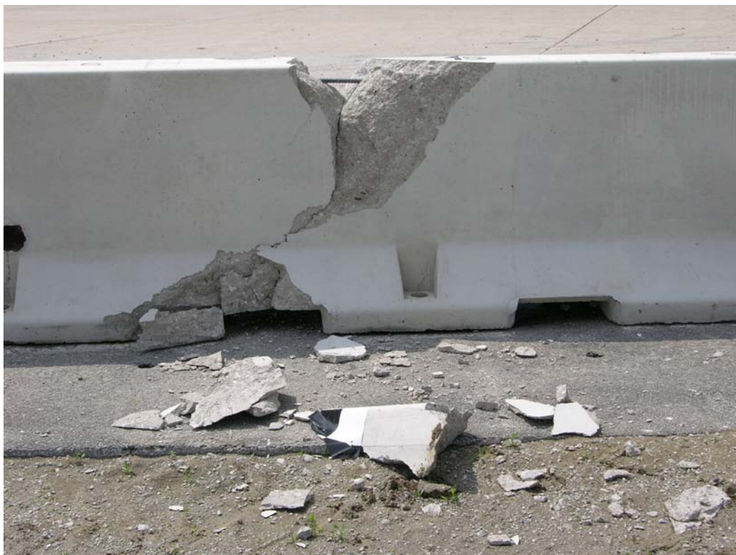
Figure 56. System Damage, Test FTB-2
