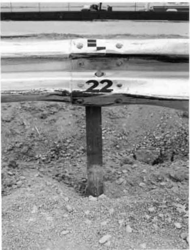
Figure 33. Post Nos. 21 and 22 Damage, Test MOSW-1
