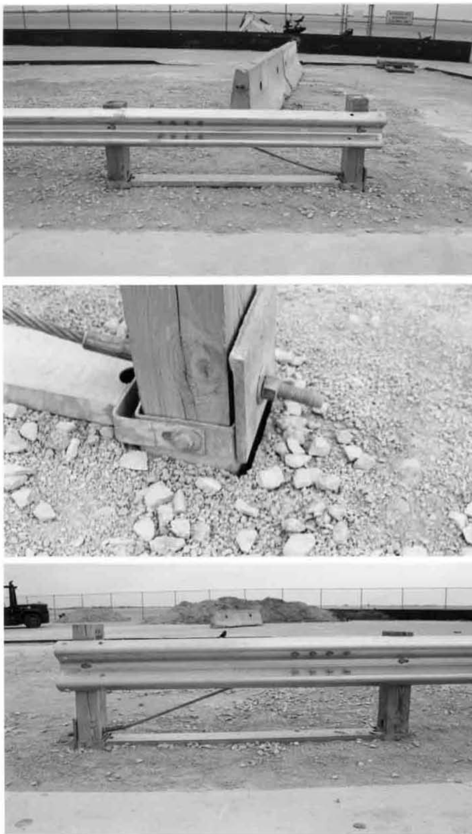
Figure 36. Permanent Set Deflections, Test MOSW-1
