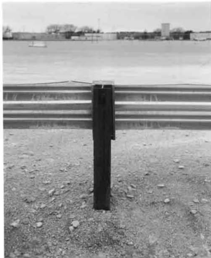
Figure 35. Post Nos. 25 and 26 Damage, Test MOSW-1
