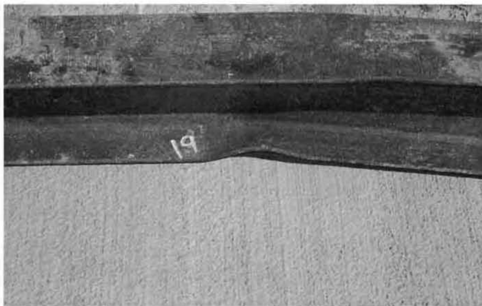
Figure 31. Post No. 19 Damage, Test MOSW-1
