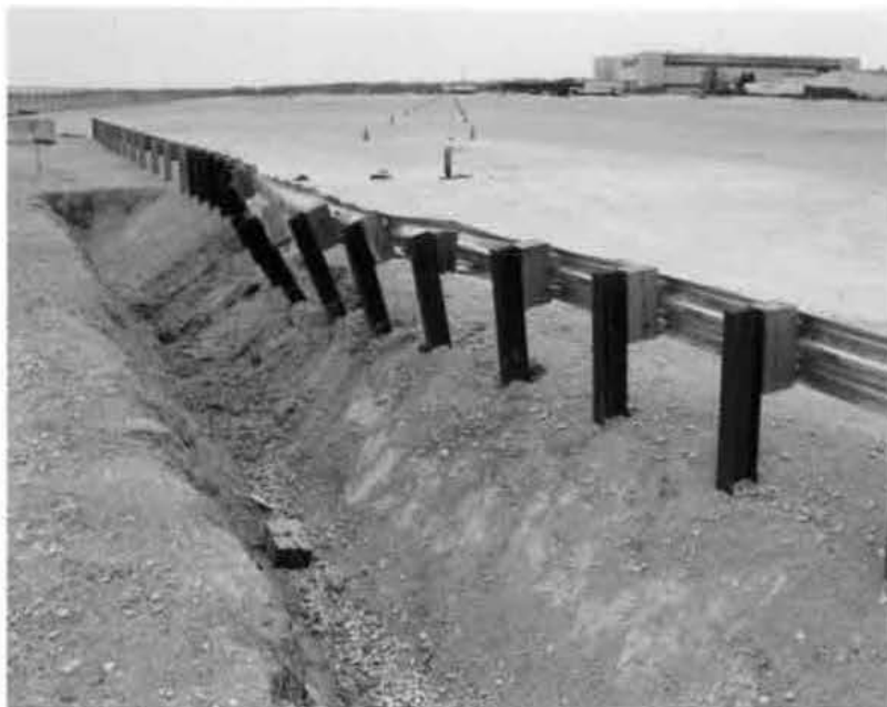
Figure 26. W-beam Guardrail System Damage, Test MOSW-1
