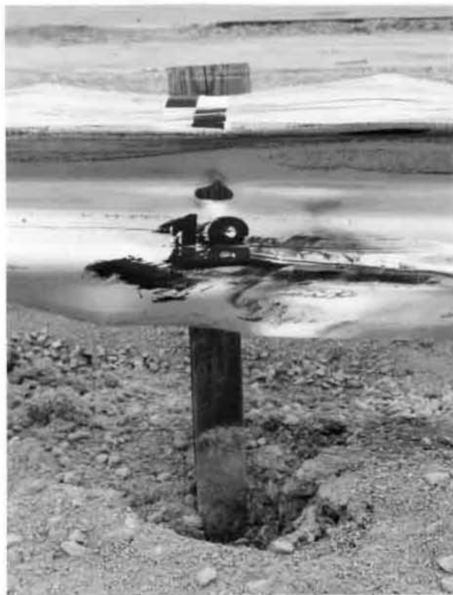
Figure 29. Post Nos. 17 and 18 Damage, Test MOSW-1
