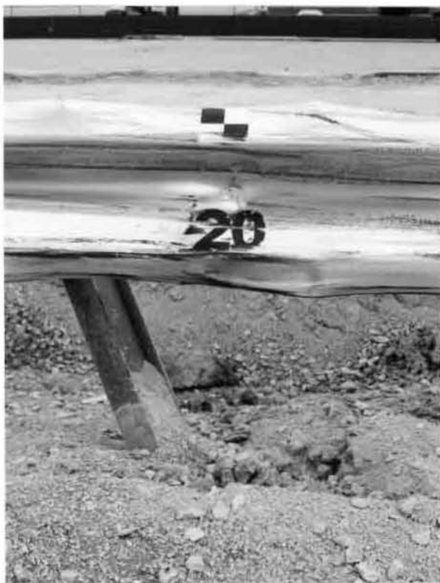
Figure 30. Post Nos. 19 and 20 Damage, Test MOSW-1
